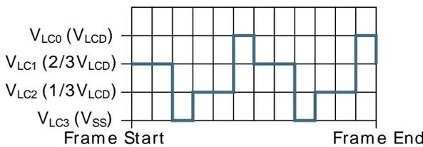
**1/3 bias and triplex multiplexing - LCD\_SEG0**
