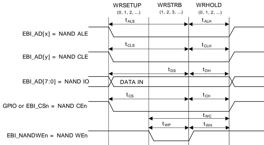
The EBI\_WRTIMING(n) setting requirements for satisfying the NAND Flash timing parameters for command latching, address latching and data input timing are shown in Table 14.5 (p. 193) .
