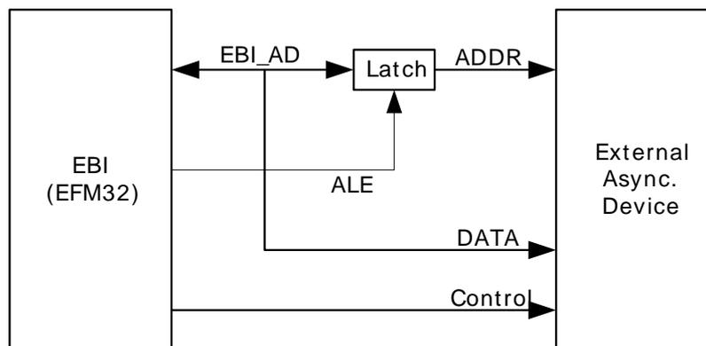
At the start of the transaction the address is output on the EBI\_AD lines. The Latch is controlled by the ALE (Address Latch Enable) signal and stores the address. Then the data is read or written according
