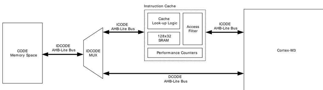
By default, the instruction cache is automatically invalidated when the contents of the flash is changed (i.e. written or erased). In many cases, however, the application only makes changes to data in the flash, not code. In this case, the automatic invalidate feature can be disabled by setting AIDIS in MSC\_READCTRL. The cache can (independent of the AIDIS setting) be manually invalidated by writing 1 to INVCACHE in MSC\_CMD.
