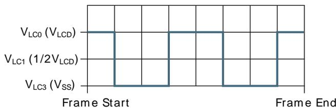
**Figure 33.8. LCD 1/2 Bias and Duplex Multiplexing - LCD\_SEG0 Connection**
