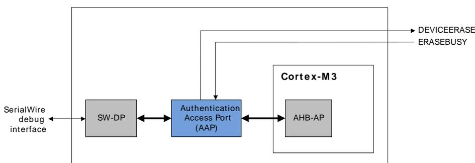
Obtaining debug access by unlocking the device must take place during the AAP window. The AAP window can also be extended giving the debugger more time to access the device by issuing the bit pattern on swdio/swclk as shown in Figure 6.3 (p. 28) . After the AAP window has closed, program execution will start if the device was successfully unlocked.
