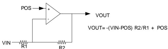
**Table 30.3. Inverting input PGA Configuration**
