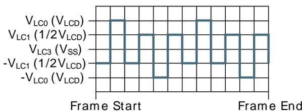
1/2 bias and triplex multiplexing - LCD\_SEG0-LCD\_COM2
