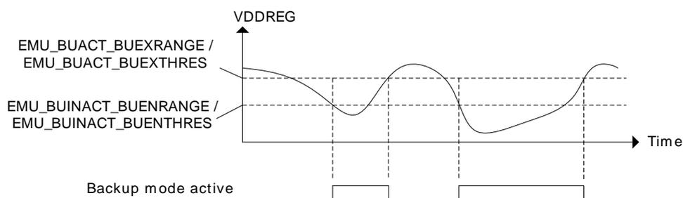
Figure 10.4 (p. 114) illustrates how the BOD sensing on VDD\_DREG can be programmed to implement hysteresis on entering and exiting backup mode.
