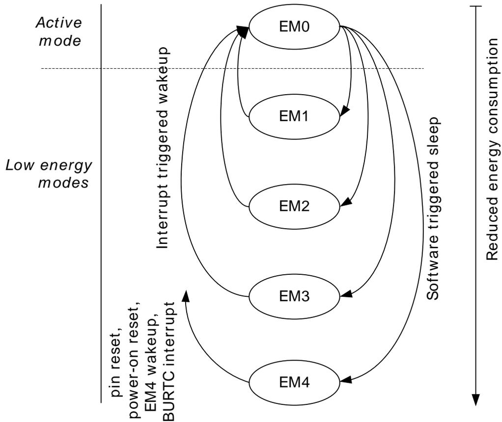
No direct transitions between EM1, EM2 or EM3 are available, as can also be seen from Figure 10.2 (p. 108) . Instead, a wakeup will transition back to EM0, in which software can enter any other low energy mode. An overview of the supported energy modes and the functionality available in each mode is shown in Table 10.1 (p. 109) . Most peripheral functionality indicated as On in a particular energy mode can also be turned off from software in order to save further energy.
