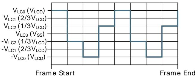
1/3 bias and duplex multiplexing - LCD\_SEG0-LCD\_COM0
