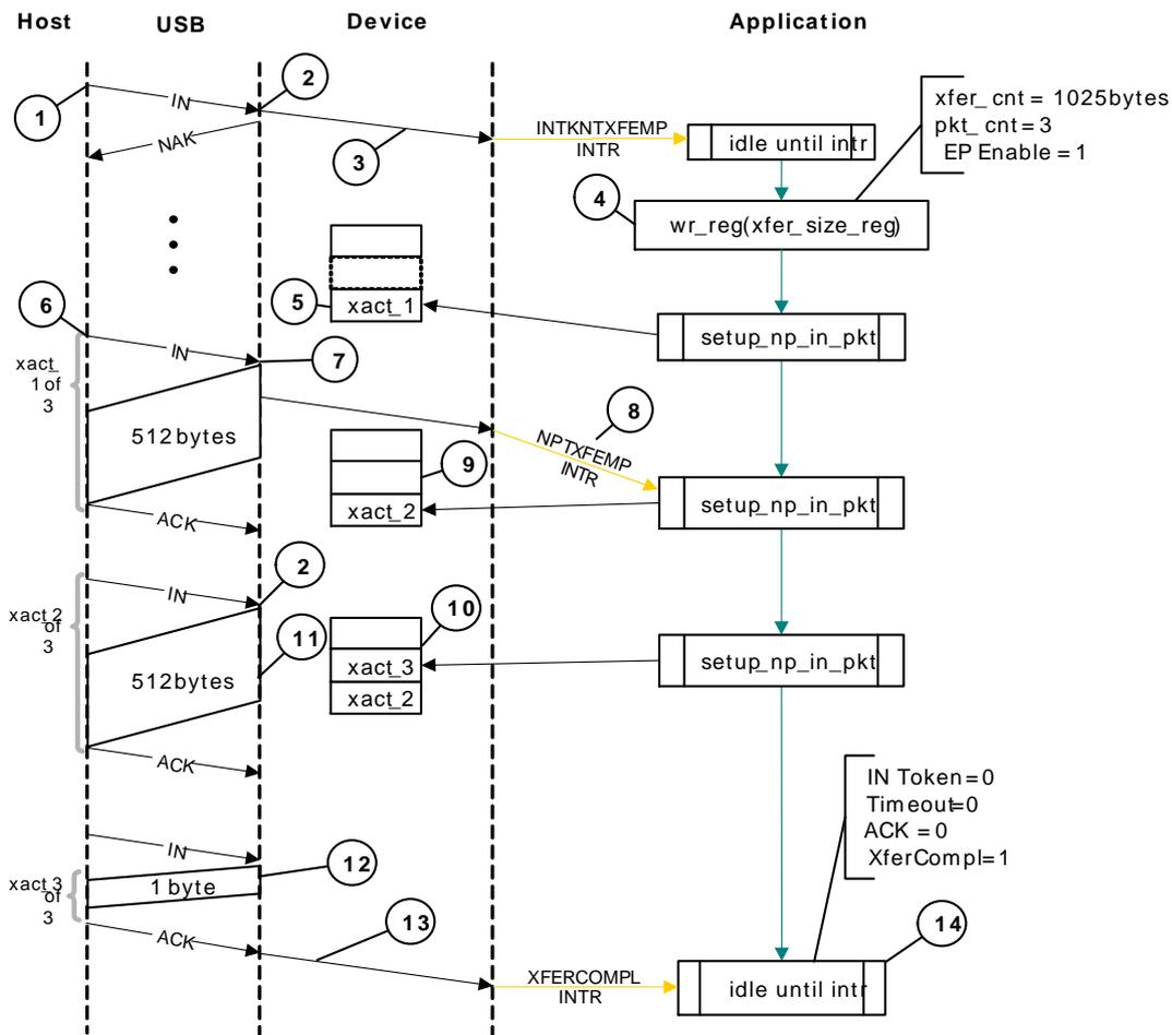
**Slave Mode Bulk IN Two-Endpoint Transfer**
