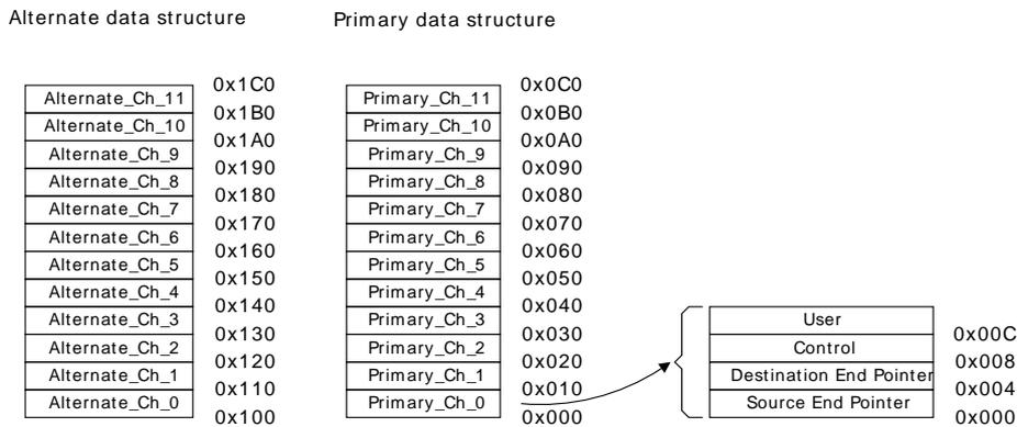
This structure in Figure 8.6 (p. 63) uses 448 bytes of system memory. The controller uses the lower 8 address bits to enable it to access all of the elements in the structure and therefore the base address must be at 0xXXXXXX00.
