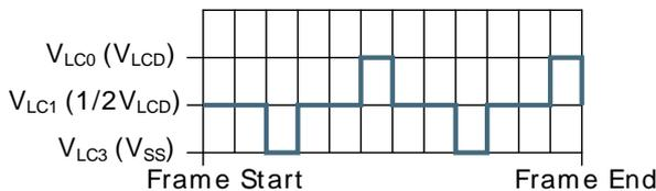
**1/2 bias and triplex multiplexing - LCD\_SEG0**
