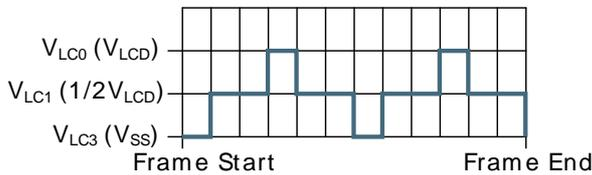
**Figure 33.18. LCD 1/2 Bias and Triplex Multiplexing - LCD\_COM1**
