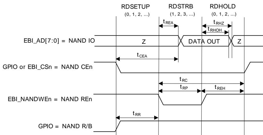
The EBI\_RDTIMING(n) setting requirements for satisfying the NAND Flash timing parameters for data output timing are shown in Table 14.6 (p. 194) .
