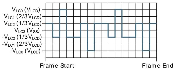
1/3 bias and quadruplex multiplexing - LCD\_SEG0-LCD\_COM3
