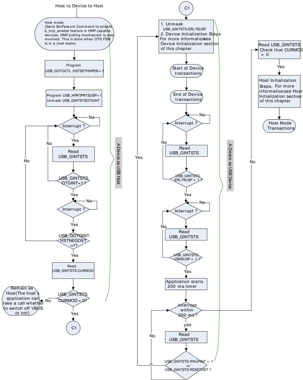
Figure 15.35 (p. 328) shows the programming steps that need to be performed by B-device's application (core as B-device) in order to change its role to Host. In Figure 15.35 (p. 328) , the B-device performs a role change, becomes a Host and then reverts back to Device mode of operation.
