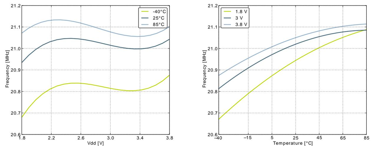
Figure 3.12. Calibrated HFRCO 28 MHz Band Frequency vs Temperature and Supply Voltage
