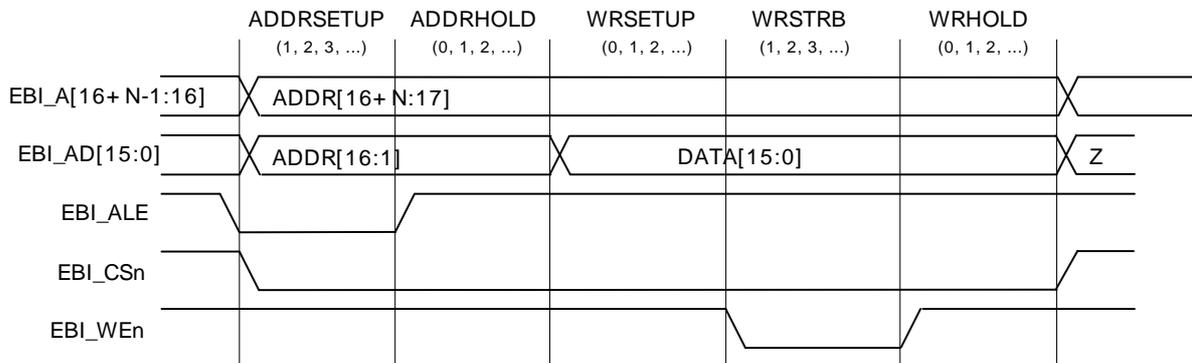
In order to minimize the pin requirements both the lower bound and the upper bound of the enabled EBI\_A lines can be set. This is done in the ALB and APEN bitfields of the EBI\_ROUTE register respectively. For example, in case all memory banks use the 8-bit addressing mode D8A8, then the
