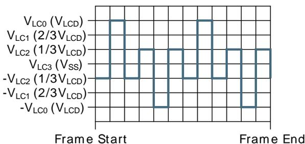
1/3 bias and triplex multiplexing - LCD\_SEG0-LCD\_COM2
