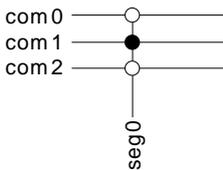
1/2 bias and triplex multiplexing - LCD\_SEG0-LCD\_COM0
