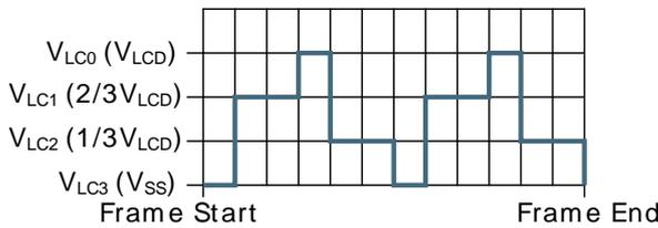
**Figure 33.26. LCD 1/3 Bias and Triplex Multiplexing - LCD\_COM1**
