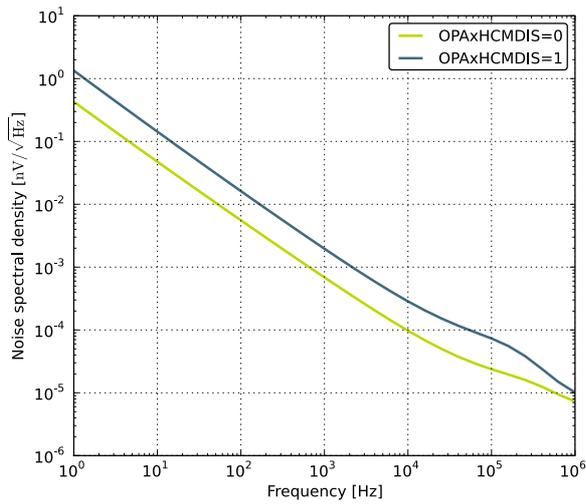
**Figure 3.27. OPAMP Voltage Noise Spectral Density (Non-Unity Gain)**
