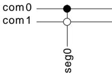
1/3 bias and duplex multiplexing - LCD\_SEG0-LCD\_COM0
