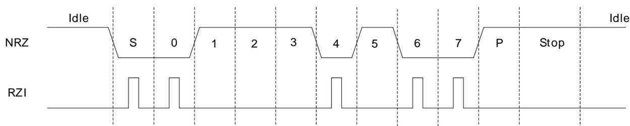
If PULSEEN in LEUARTn\_PULSECTRL is set while INV in LEUARTn\_CTRL is cleared, the output waveform will like RZI shown in Figure 19.7 (p. 504) , only inverted.
