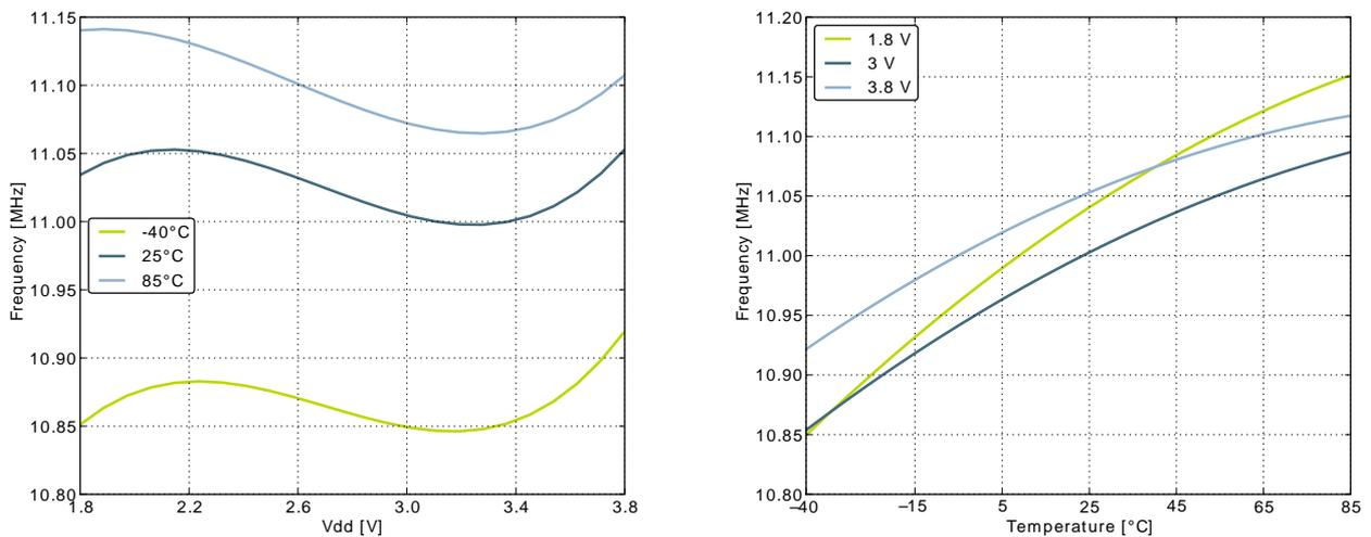
**Figure 3.12. Calibrated HFRCO 14 MHz Band Frequency vs Temperature and Supply Voltage**
