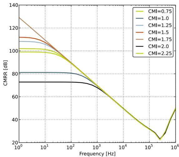
Figure 3.24. OPAMP Positive Power Supply Rejection Ratio
