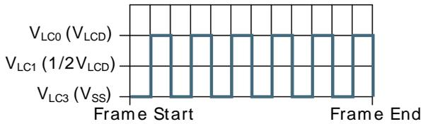
**Figure 33.21. LCD 1/2 Bias and Triplex Multiplexing - LCD\_SEG0 Connection**
