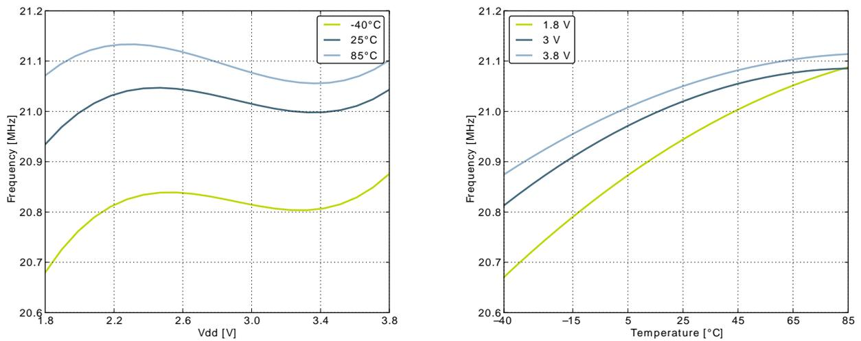
**Figure 3.14. Calibrated HFRCO 28 MHz Band Frequency vs Temperature and Supply Voltage**
