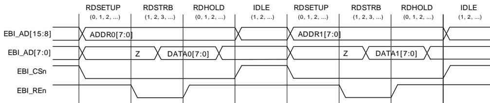
**Figure 14.22. EBI No Enforced IDLE cycles between Transactions**
