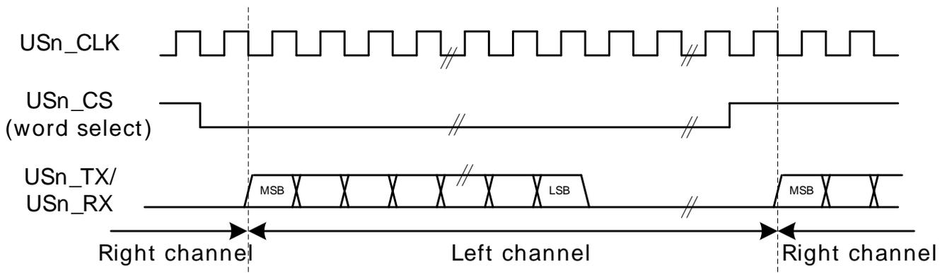
A left-justified stream is shown in Figure 17.18 (p. 466). Note that the MSB comes directly after the edge on the word-select signal in contradiction to the regular I2S waveform where it comes one bit-period after.
