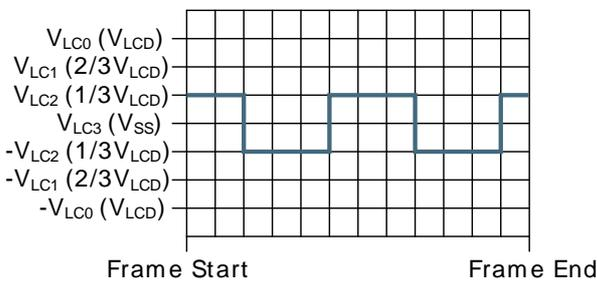
1/3 bias and triplex multiplexing - LCD\_SEG0-LCD\_COM1
