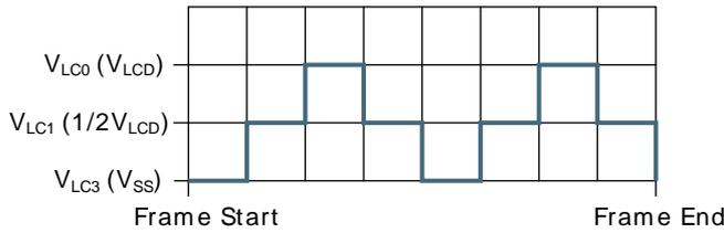
**Figure 33.6. LCD 1/2 Bias and Duplex Multiplexing - LCD\_COM1**
