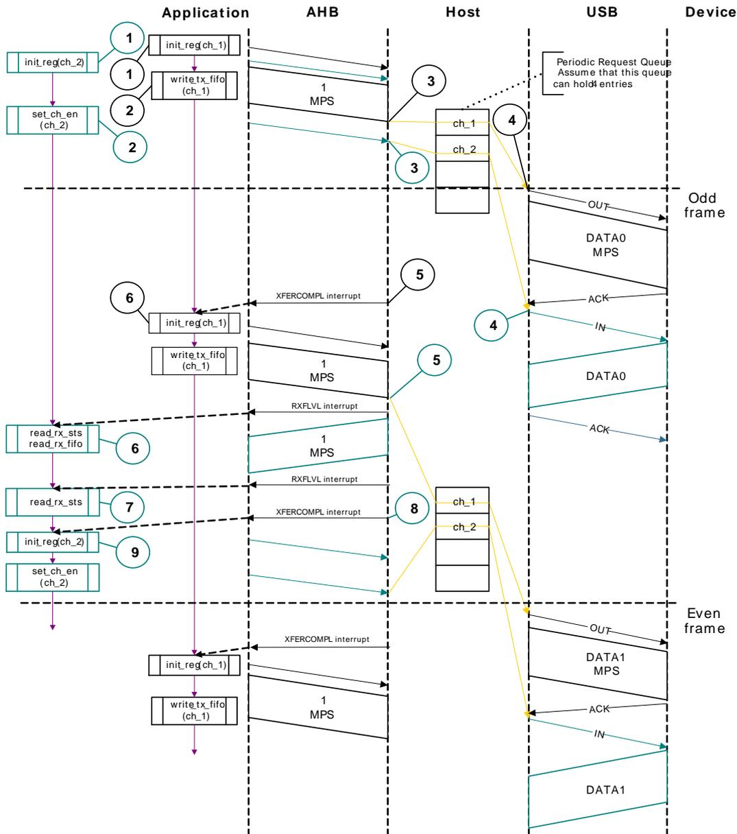
**Interrupt Service Routine for Interrupt OUT Transactions in Slave Mode**
