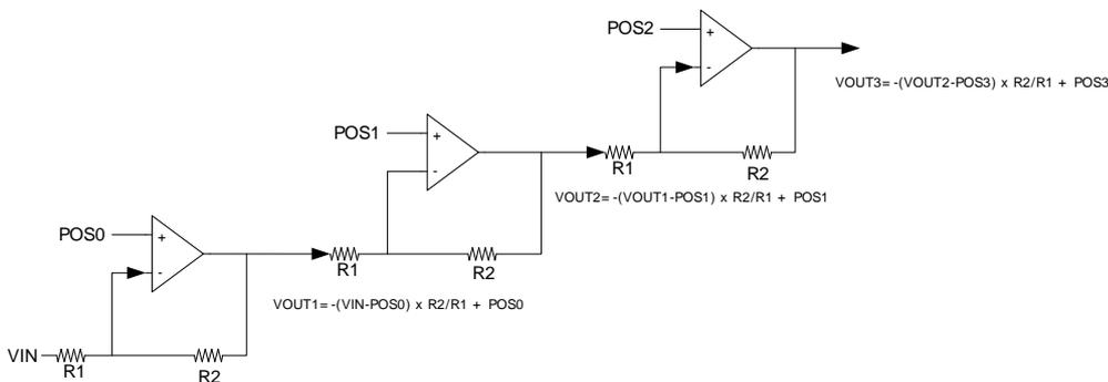
**Table 30.5. Cascaded Inverting PGA Configuration**
