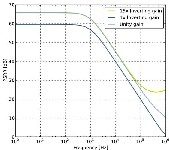
**Figure 3.25. OPAMP Negative Power Supply Rejection Ratio**
