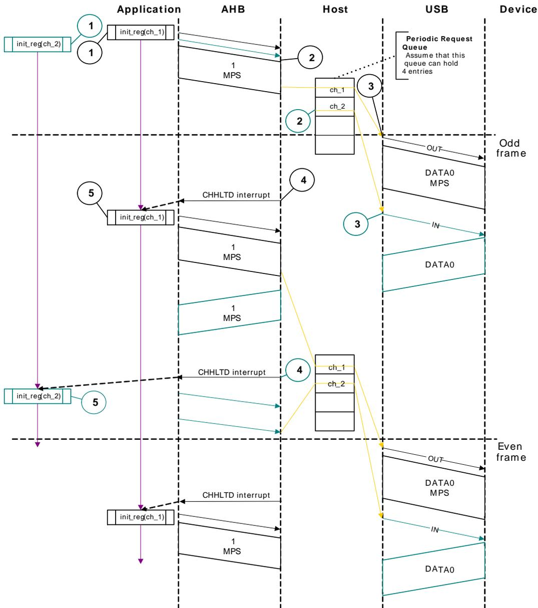
**Interrupt Service Routine for Isochronous OUT Transactions in DMA Mode**
