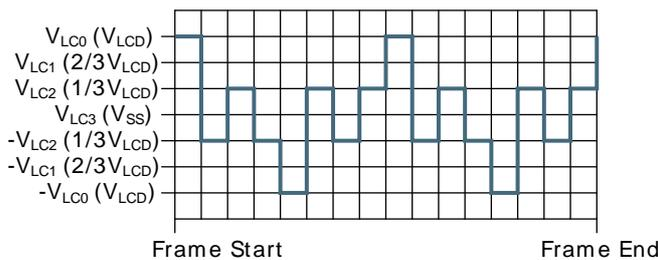
1/3 bias and quadruplex multiplexing - LCD\_SEG0-LCD\_COM1
