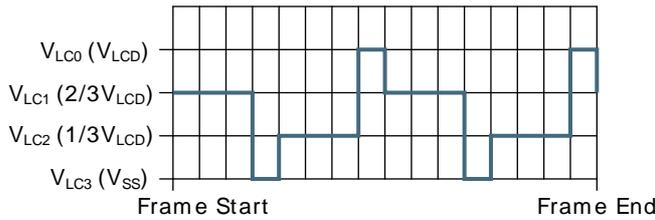
1/3 bias and quadruplex multiplexing - LCD\_SEG0
