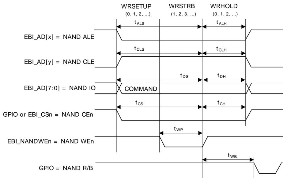
**Figure 14.28. EBI NAND Flash Address Latch Timing**
