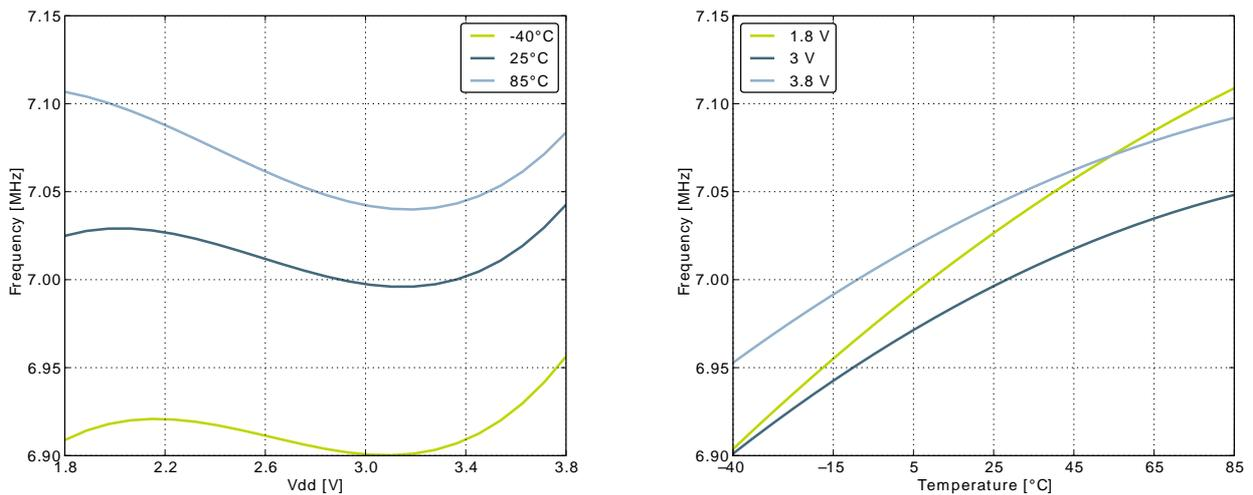
**Figure 3.11. Calibrated HFRCO 11 MHz Band Frequency vs Temperature and Supply Voltage**
