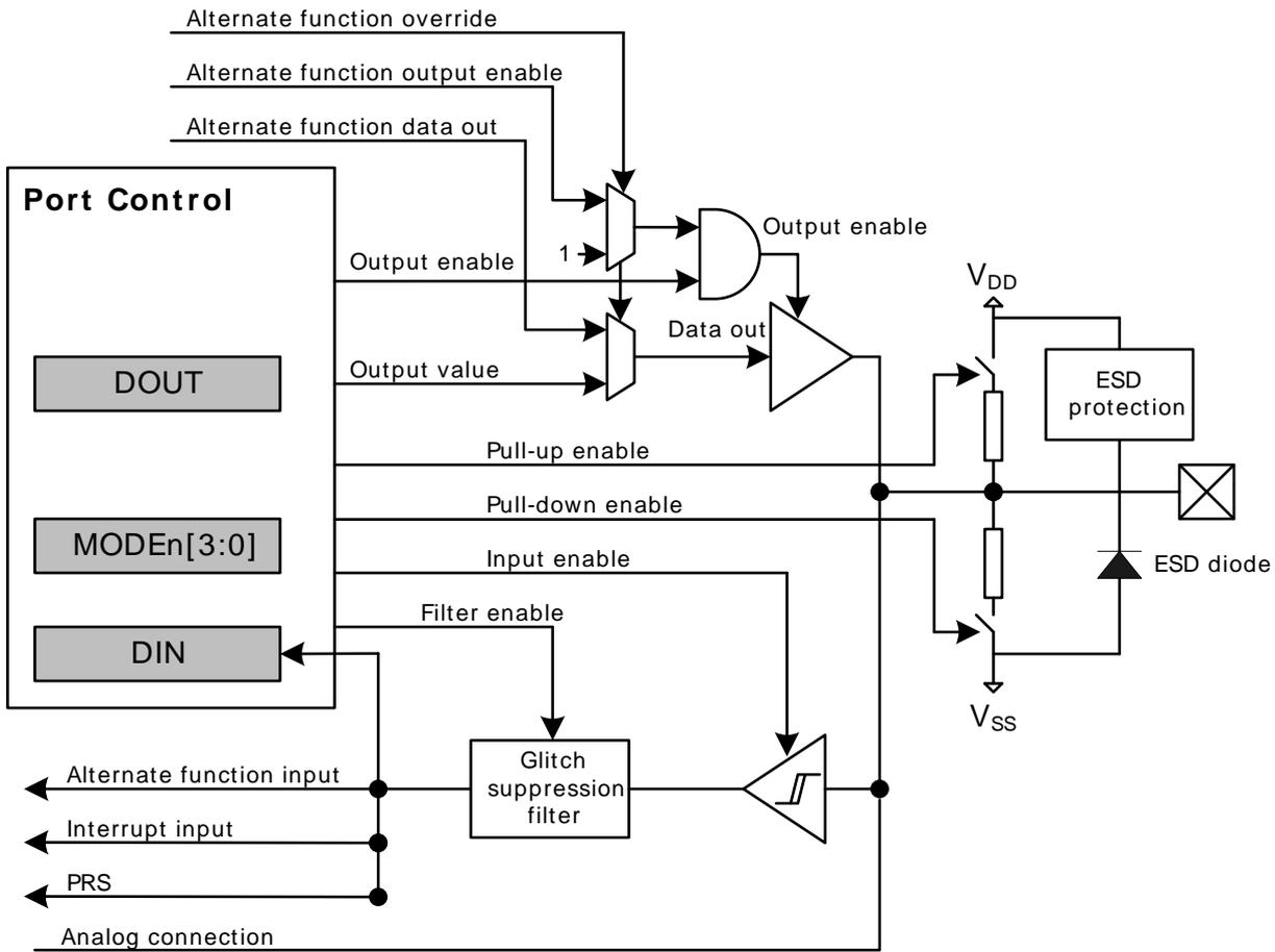
**Note** There is no ESD diode to Vdd because if using LCD voltage boost the pin voltage will be higher than Vdd. Nevertheless there is an ESD protection block against over voltage.
