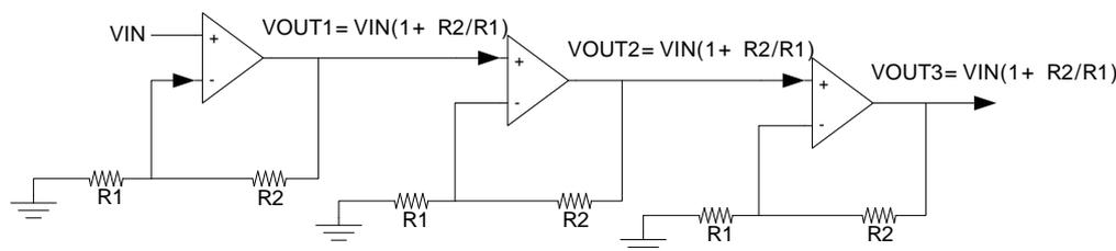
Table 30.6. Cascaded Non-inverting PGA Configuration
