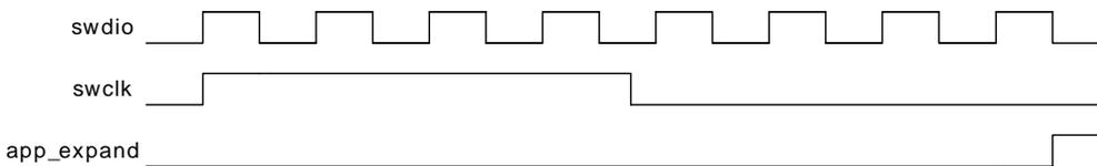
The device is unlocked by writing to the AAP\_CMDKEY register and then setting the DEVICEERASE bit of the AAP\_CMD register via the debug interface. This erase operation erases the main block of flash, all lock bits are reset and debug access through the AHB-AP is enabled. The operation takes 125 ms to complete. Note that the SRAM contents will also be deleted during a device erase.
