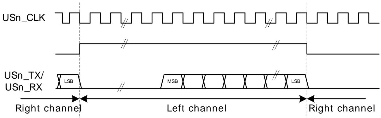
In mono-mode, the word-select signal pulses at the beginning of each word instead of toggling for each word. Mono I2S waveform is shown in Figure 17.20 (p. 467) .
