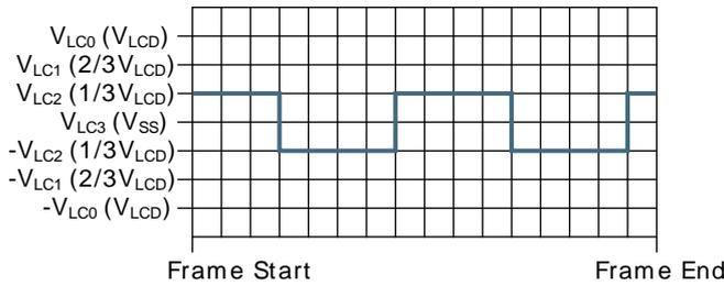
1/3 bias and quadruplex multiplexing - LCD\_SEG0-LCD\_COM2
