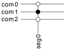
1/3 bias and triplex multiplexing - LCD\_SEG0-LCD\_COM0
