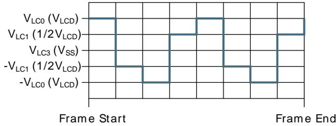
1/2 bias and duplex multiplexing - LCD\_SEG0-LCD\_COM1
