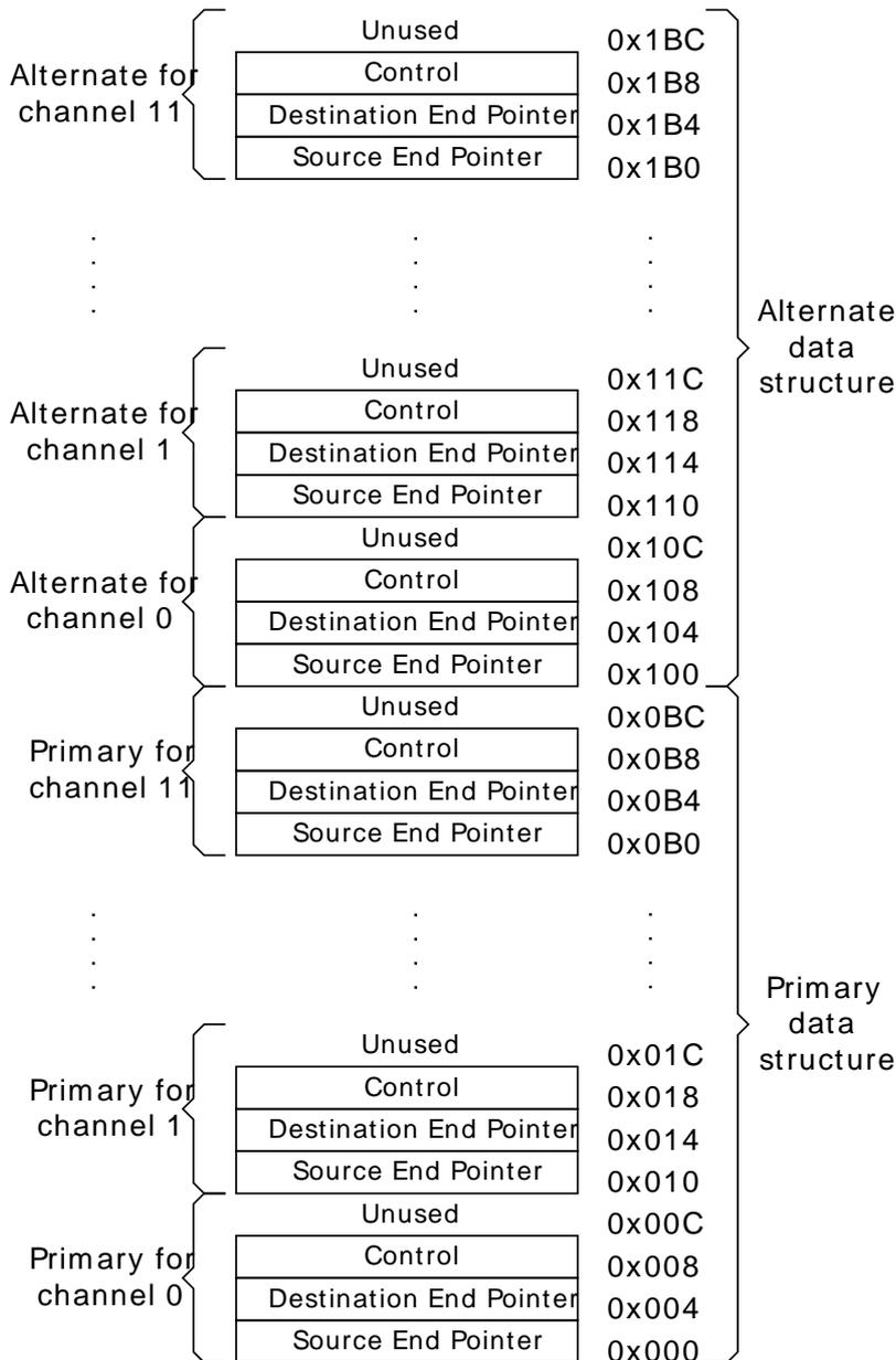
The controller uses the system memory to enable it to access two pointers and the control information that it requires for each channel. The following subsections will describe these 32-bit memory locations and how the controller calculates the DMA transfer address.
