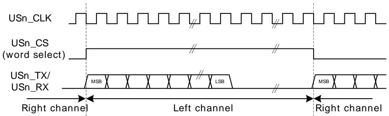
A right-justified stream is shown in Figure 17.19 (p. 467). The left and right justified streams are equal when the data-size is equal to the word-width.
