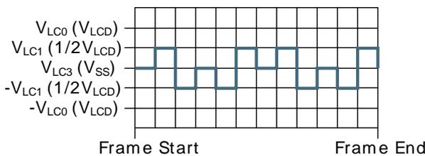
1/2 bias and triplex multiplexing - LCD\_SEG0-LCD\_COM1
