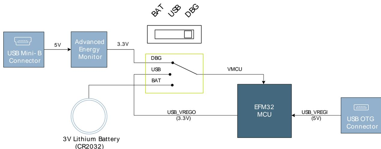
With the switch in the *DBG* position, an on-board low noise LDO with a fixed output voltage of 3.3V is used to power the MCU. This LDO is again powered from the "J-Link" USB cable. The Advanced Energy Monitor is now also connected in series, allowing accurate high speed current measurements and energy debugging/profiling.
