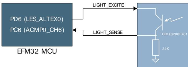
Two pins are used for the light sensor operation: one for excitation, and one for sensing. The sense pin is connected to ACMP0 CH6. Both the excitation pin and the sense pin can be controlled directly from the EFM32's LESENSE module.
