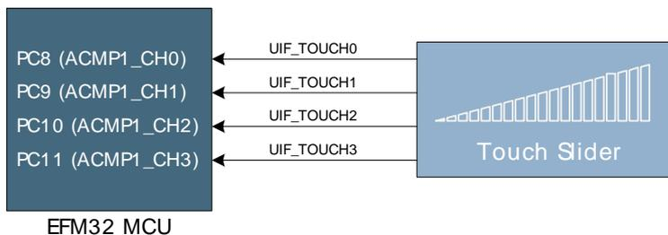
The capacitive touch slider works by sensing changes in the capacitance of the pads when touched by a human finger. Sensing the changes in capacitance is done by setting up the touch pad as part of an RC relaxation oscillator using the EFM32's analog comparator, and then counting the number of oscillations during a fixed period of time.
