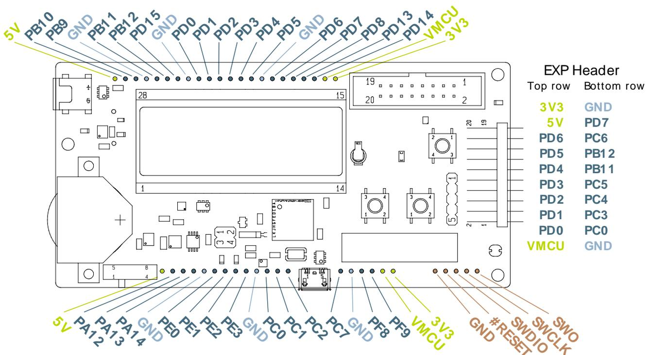
**Note** Pins PC3, PC4, PC5 and PC6 are also available as surface mounted pads beneath the USB Micro-AB connector
