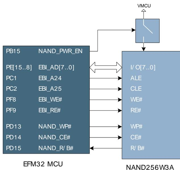
A separate power switch is used to enable/disable the NAND flash, thus avoiding excess current draw when not used. When *NAND\_PWR\_EN* is high, the NAND flash is powered from the same supply as the EFM32 MCU. It is recommended to keep the write-protect line low during power transitions.
