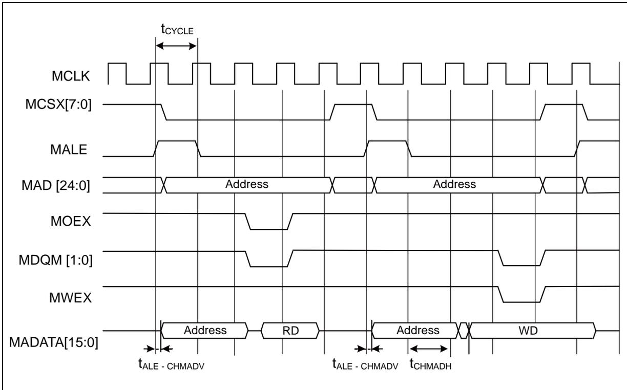
• Multiplexed Bus Access Synchronous SRAM Mode
