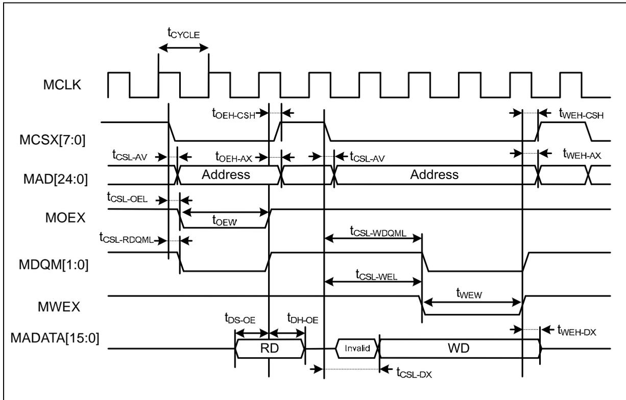
• Separate Bus Access Synchronous SRAM Mode
