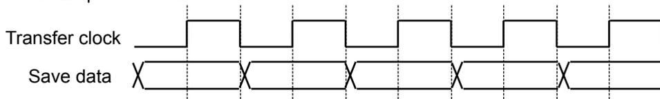
The save data is output from the buffer at a falling edge of the transfer clock and is written to the register at a rising edge of the transfer clock.
