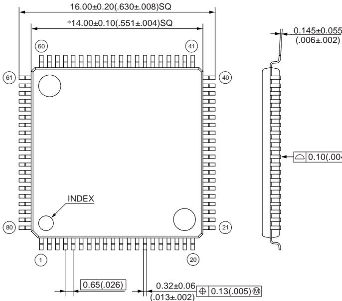
Note 1) \* : These dimensions do not include resin protrusion.
