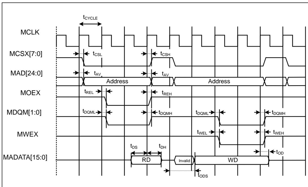
• Multiplexed Bus Access Asynchronous SRAM Mode
