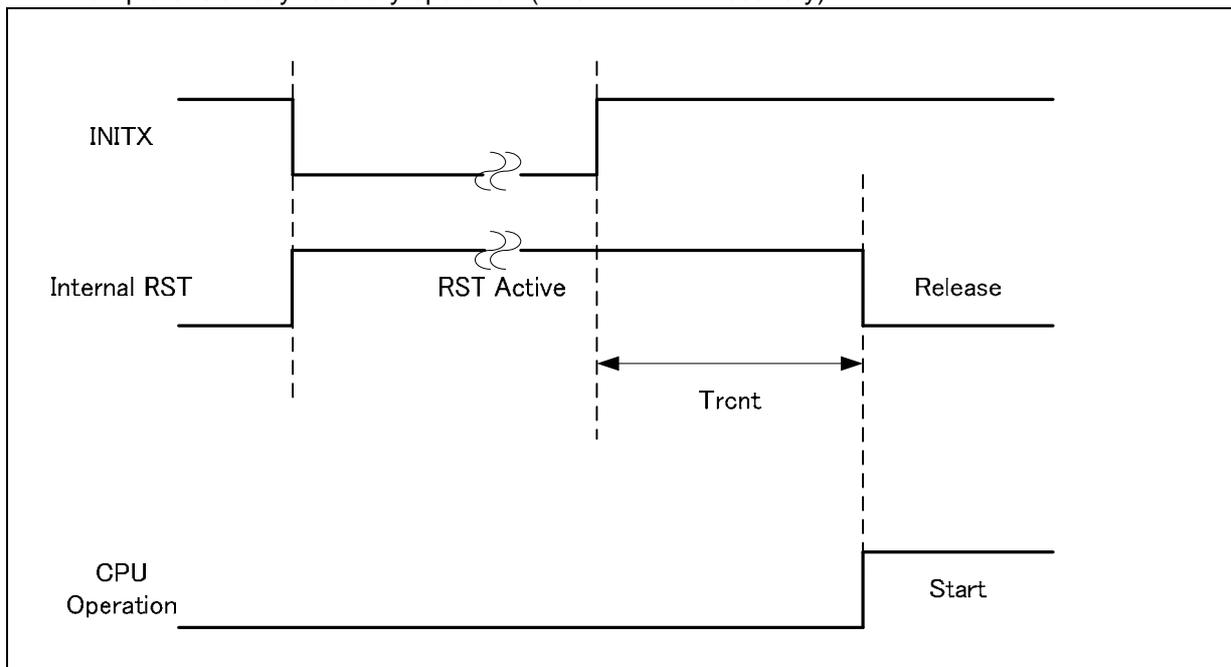
• Example of standby recovery operation (when in internal resource reset recovery\*)
