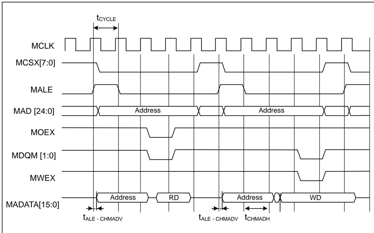
• Multiplexed Bus Access Synchronous SRAM Mode
