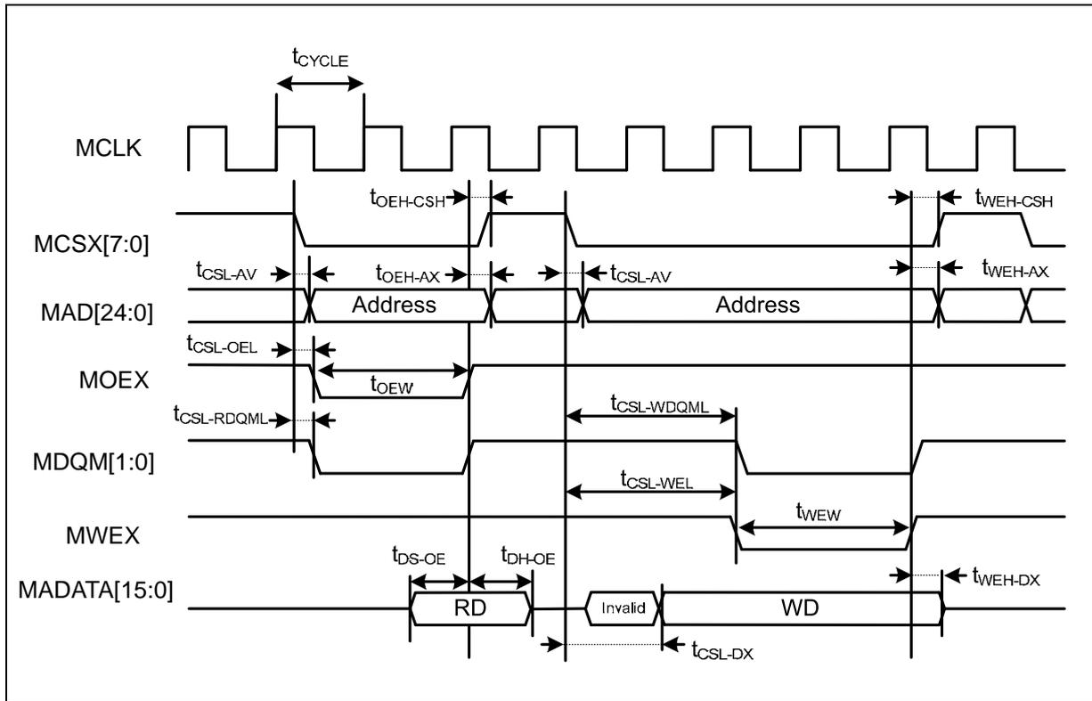
• Separate Bus Access Synchronous SRAM Mode
