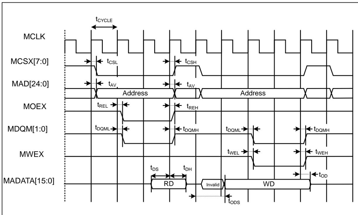
• Multiplexed Bus Access Asynchronous SRAM Mode
