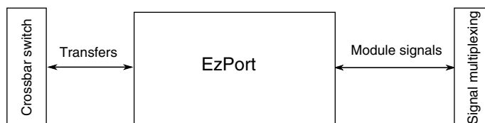
Figure 3-30. EzPort configuration
