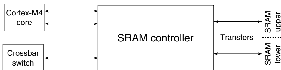
Figure 3-24. SRAM controller configuration
