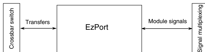
Figure 3-27. EzPort configuration
