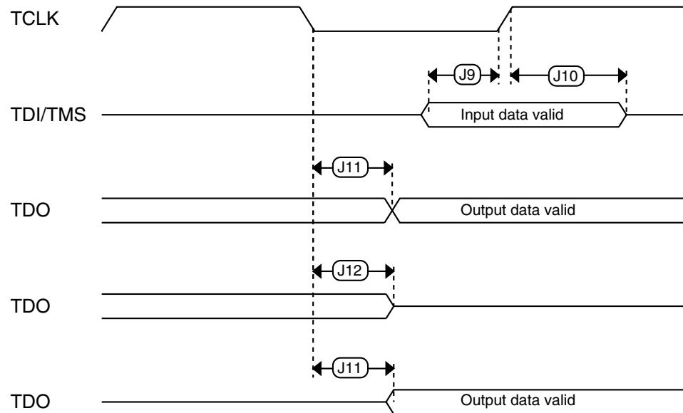
**Figure 7. Test Access Port timing**
