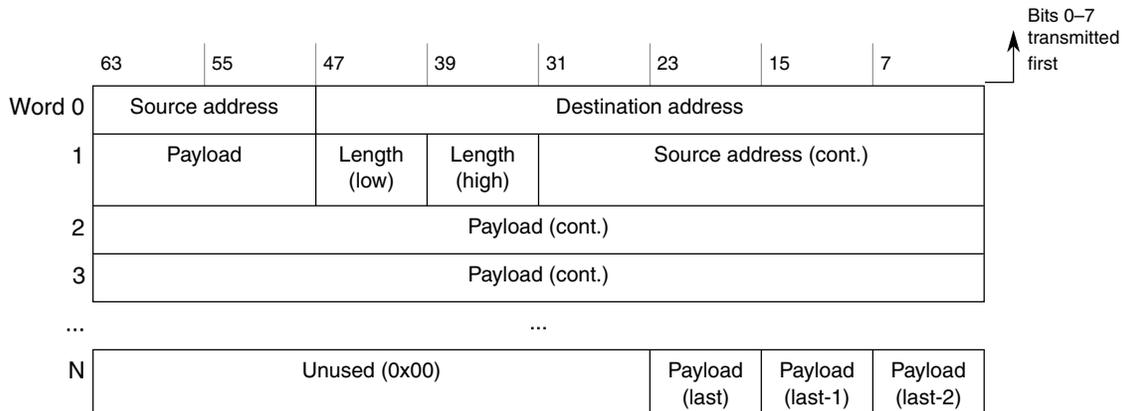
**Figure 47-64. Normal Ethernet Frame 64-bit Mapping Example**
