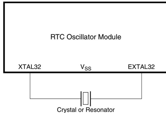
**Figure 27-2. Crystal Connections**
