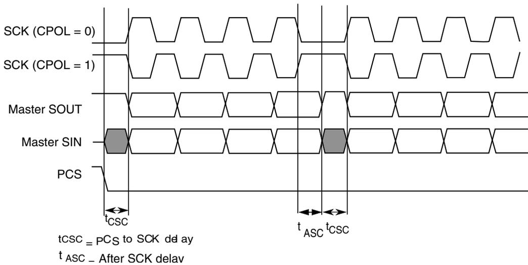
**Figure 53-97. Example of Continuous Transfer (CPHA=1, CONT=1)**
