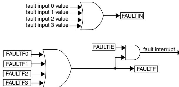
**Figure 42-275. FAULTF and FAULTIN Bits and Fault Interrupt**
