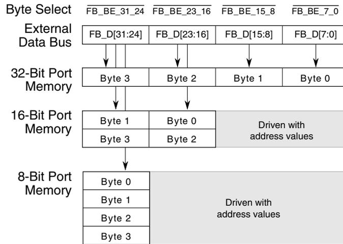
Figure 33-23. Connections for External Memory Port Sizes ( $\text{CSCR}_n[\text{BLS}] = 0$ )
