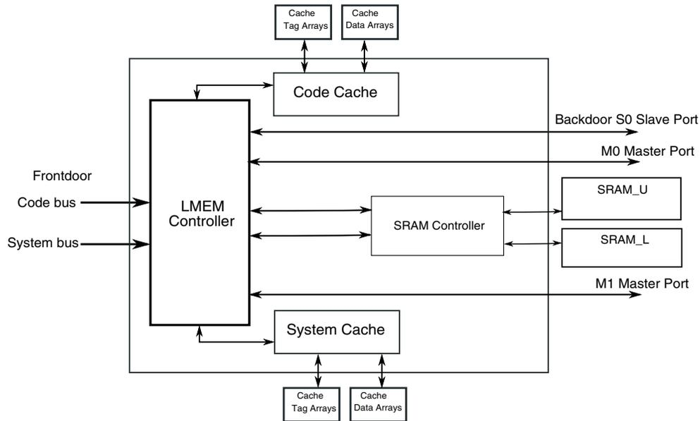
**Figure 28-12. SRAM Configuration**
