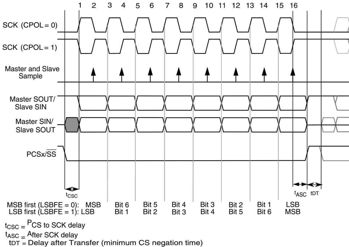
**Figure 53-95. DSPI Transfer Timing Diagram (MTFE=0, CPHA=1, FMSZ=8)**
