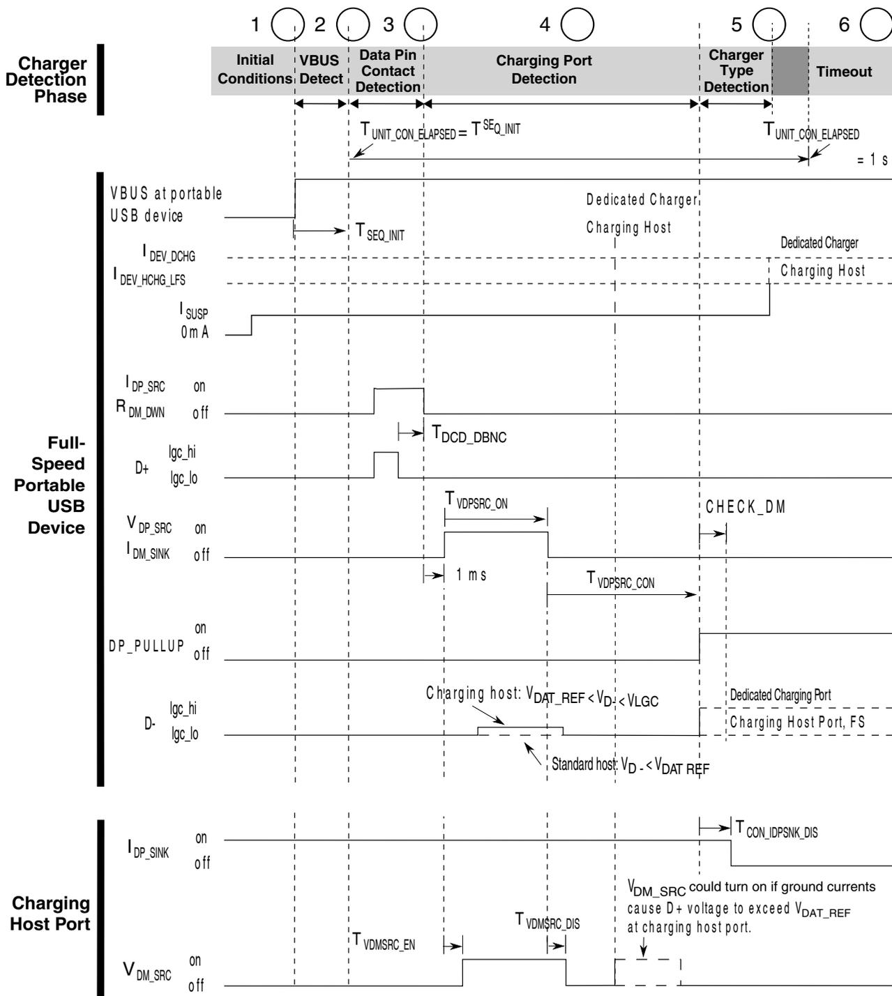
Figure 49-9. Full Speed Charger Detection Timing
