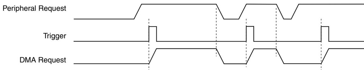
**Figure 21-54. DMA MUX channel triggering: normal operation**
