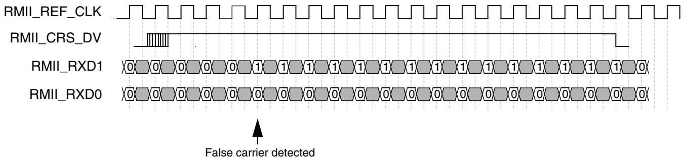
**Figure 47-70. RMIi receive operation with false carrier**
