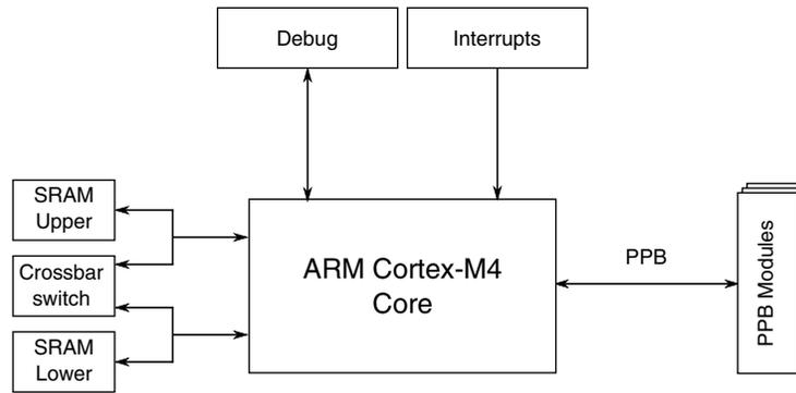
Figure 3-1. Core configuration
