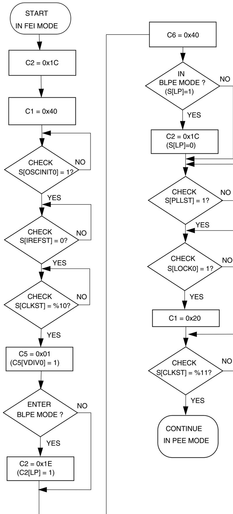
Figure 25-19. Flowchart of FEI to PEE Mode Transition using an 16 MHz crystal
