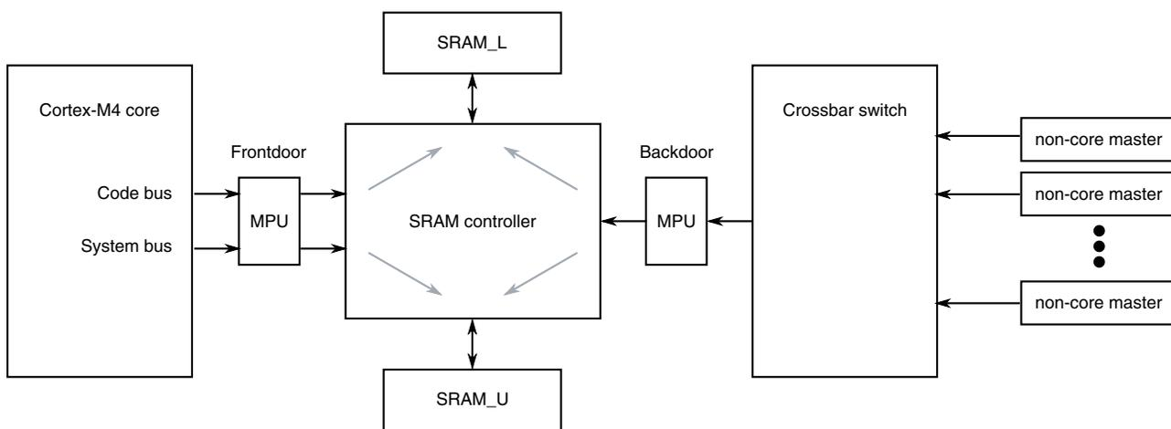
**Figure 3-27. SRAM access diagram**
