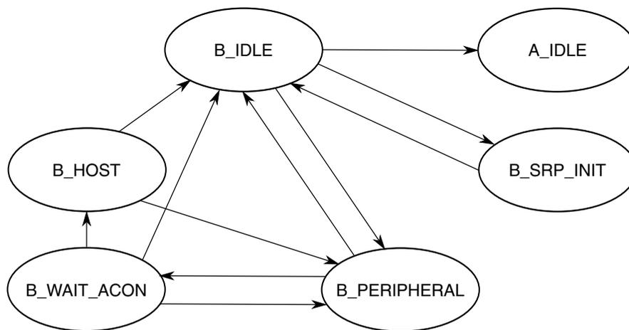
Figure 48-94. Dual Role B Device Flow Diagram
