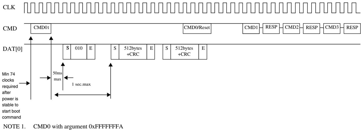
**Figure 56-38. MultiMediaCard state diagram (alternative boot mode)**
