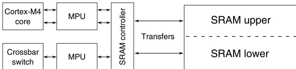
Figure 3-25. SRAM configuration
