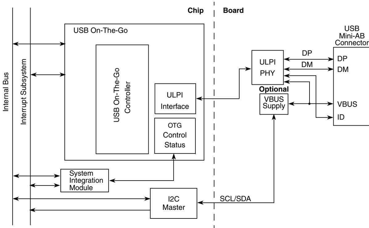
Figure 3-65. USB HS OTG module and ULPI PHY
