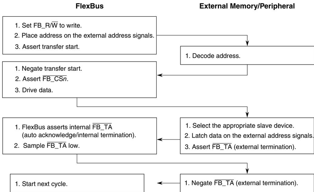
**Figure 33-28. Write-Cycle Flowchart**
