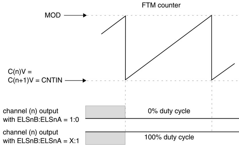
**Figure 42-236. Channel (n) Output If  $(C(n)V = C(n+1)V = CNTIN)$**
