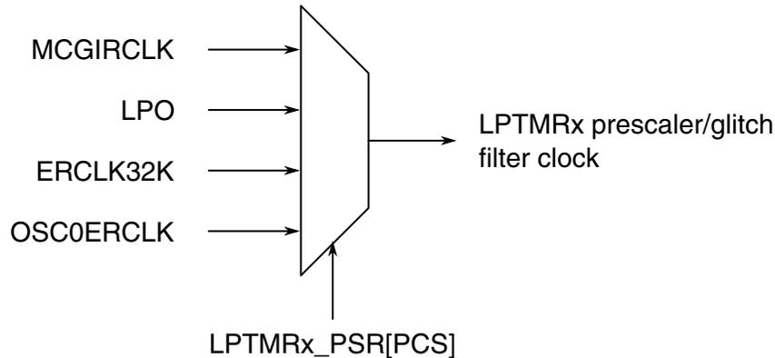
**Figure 5-6. LPTMR<sub>x</sub> prescaler/glitch filter clock generation**
