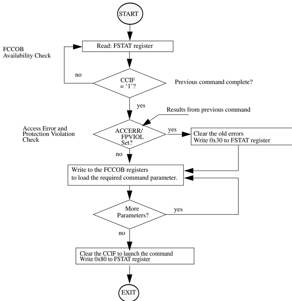
**Figure 30-33. Generic Flash Command Write Sequence Flowchart**
