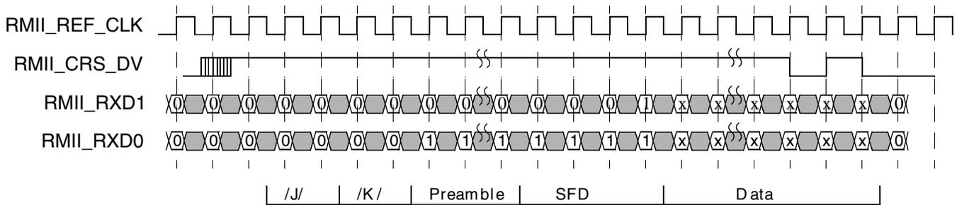
**Figure 47-69. RMIi receive operation**
