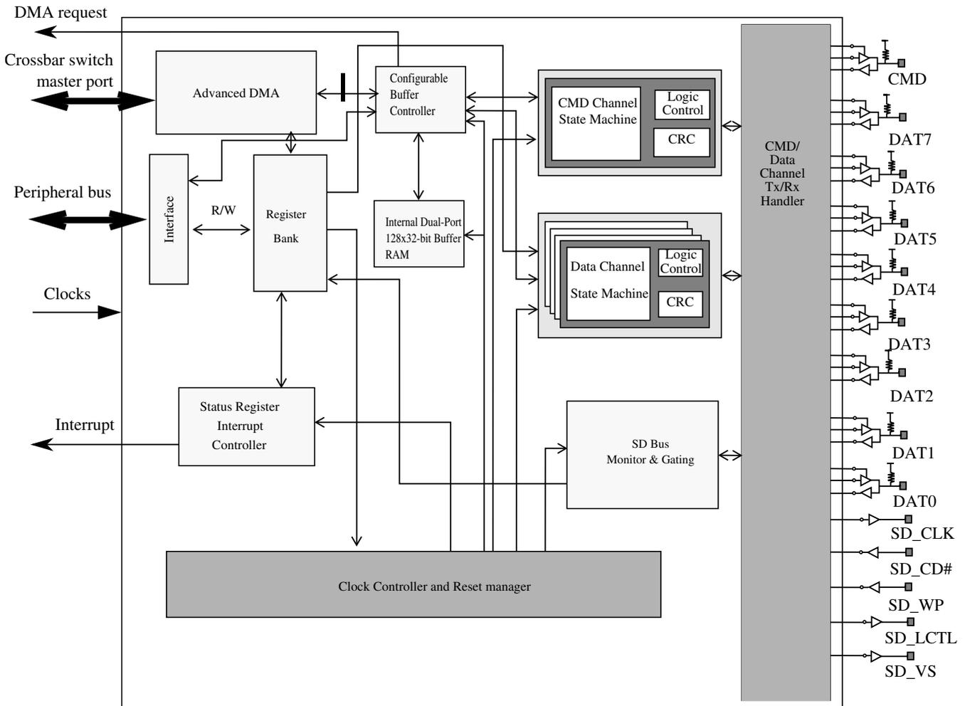
Figure 56-2. Enhanced secure digital host controller block diagram
