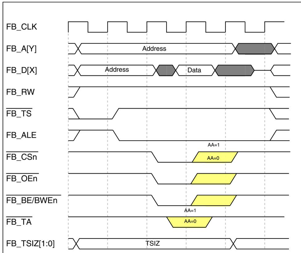
Figure 33-40. Read-Bus Cycle with Two-Clock Address Setup (No Wait States)
