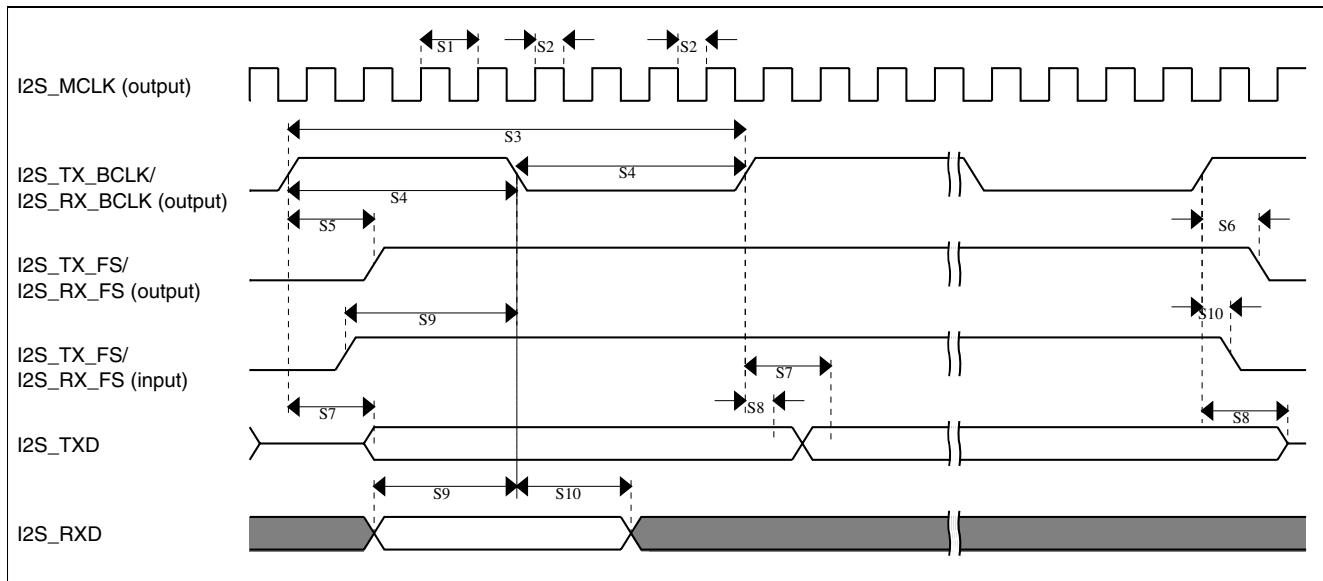
**Figure 30. I2S/SAI timing — master modes****Table 51. I2S/SAI slave mode timing in Normal Run, Wait and Stop modes (full voltage range)**
