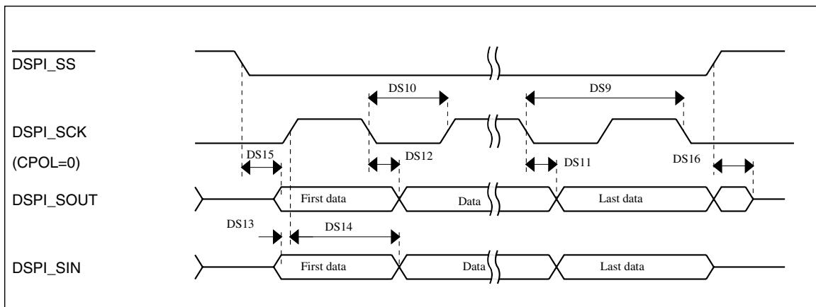
**Figure 23. DSPI classic SPI timing — slave mode**
