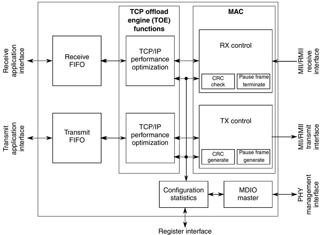
Figure 47-1. 10/100 Ethernet MAC-NET Core Block Diagram
