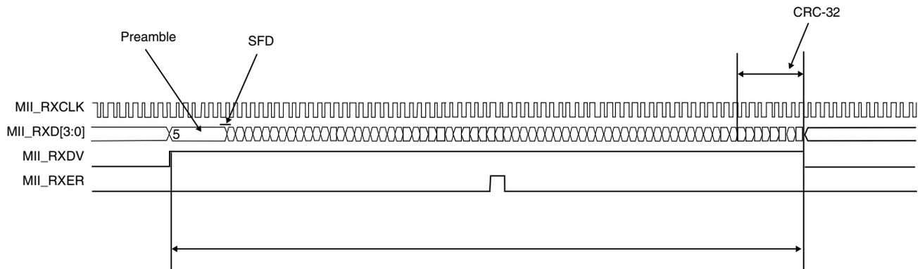
**Figure 47-76. MII Receive Operation — Errored Frame**
