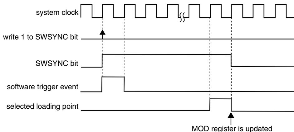
**Figure 42-254. MOD Synchronization with (SYNCMODE = 0) and (PWMSYNC = 1)**
