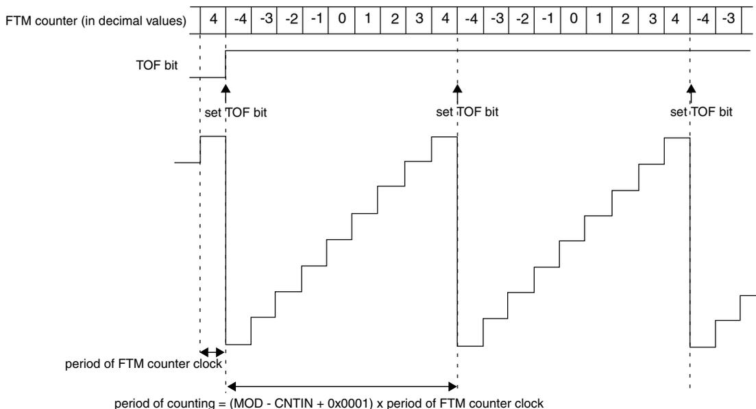
**Figure 42-209. Example of FTM Up and Signed Counting**
