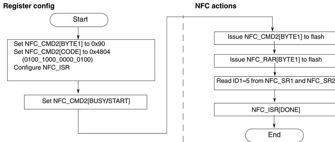
Figure 32-23. Flow Chart of Read ID Operation
