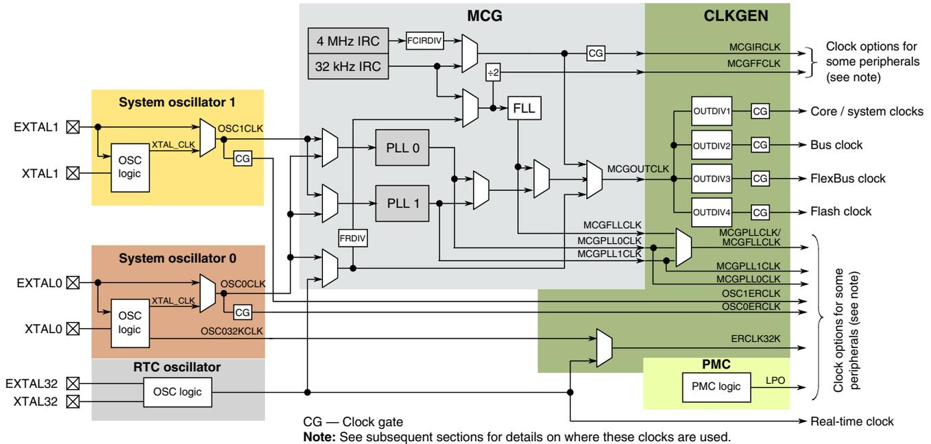
Figure 5-1. Clocking diagram
