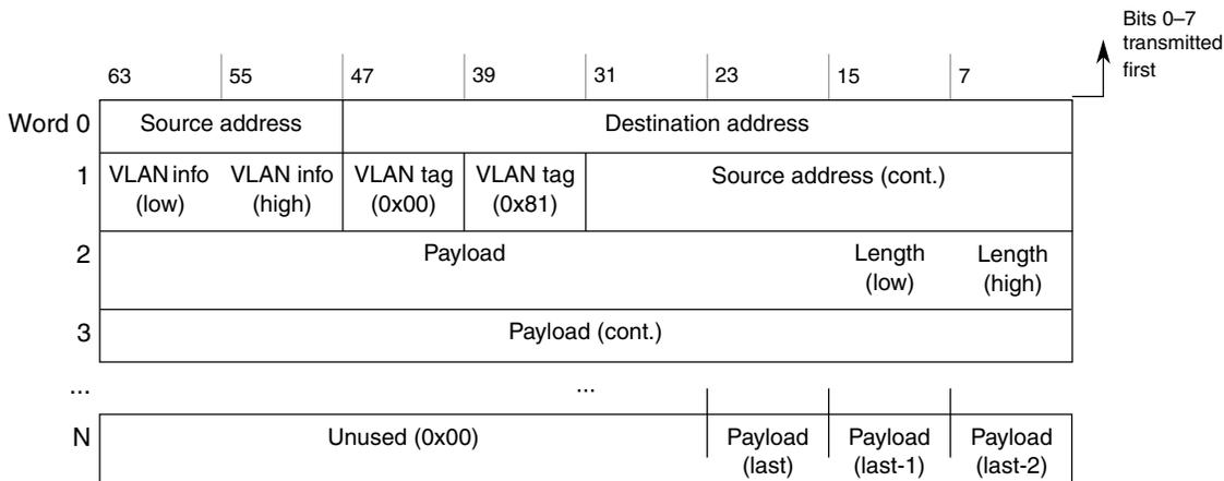
**Figure 47-65. VLAN tagged Frame 64-bit Mapping Example**
