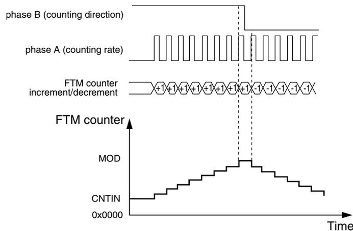
**Figure 42-292. Quadrature Decoder – Count and Direction Encoding Mode**
