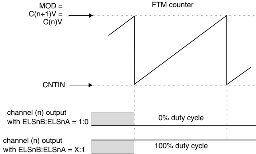
**Figure 42-237. Channel (n) Output If  $(C(n)V = C(n+1)V = MOD)$**
