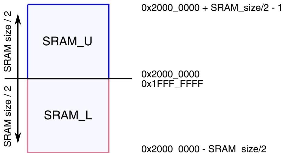
**Figure 28-13. SRAM Arrays**
