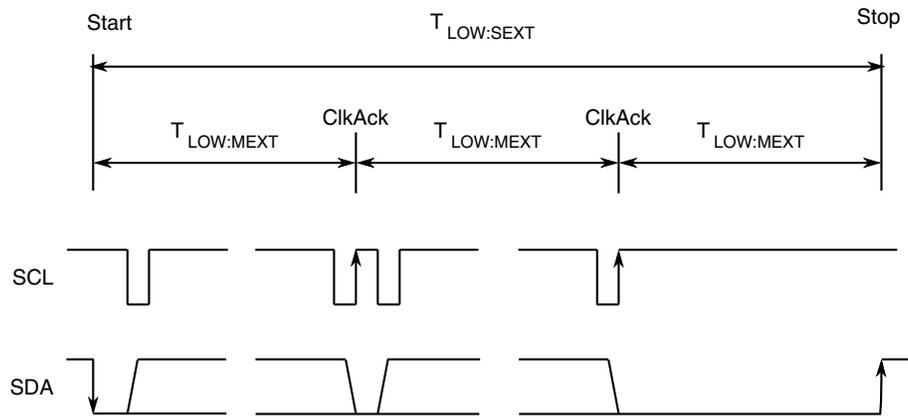
**Figure 54-40. Timeout measurement intervals**
