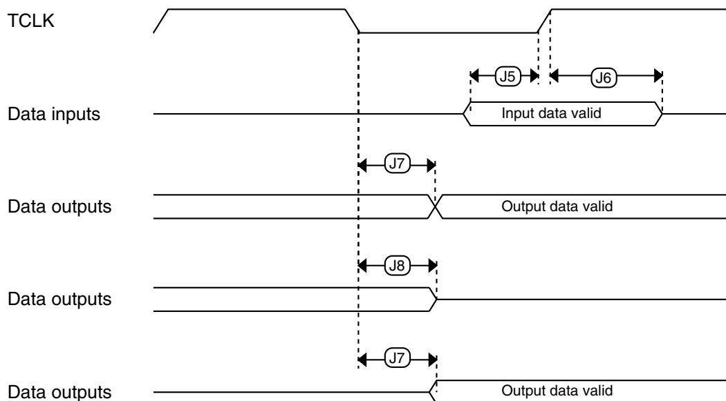
**Figure 6. Boundary scan (JTAG) timing**
