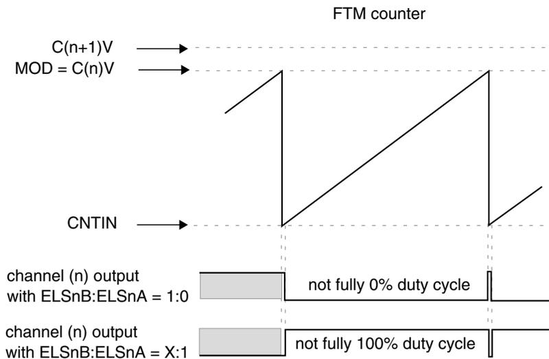
**Figure 42-243. Channel (n) Output If  $(C(n+1)V > MOD)$  and  $(CNTIN < C(n)V = MOD)$**
