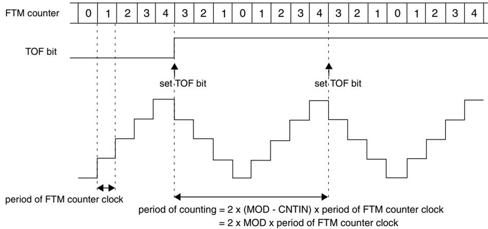
Figure 42-212. Example of Up-Down Counting When CNTIN = 0x0000
