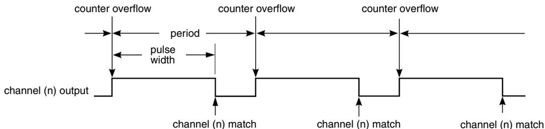
**Figure 42-222. EPWM Period and Pulse Width with ELSnB:ELSnA = 1:0**
