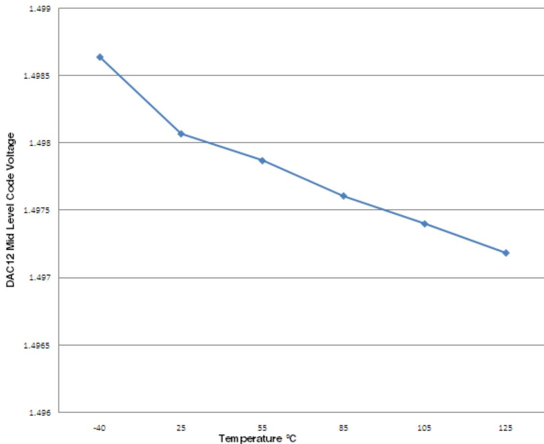
**Figure 19. Offset at half scale vs. temperature**
