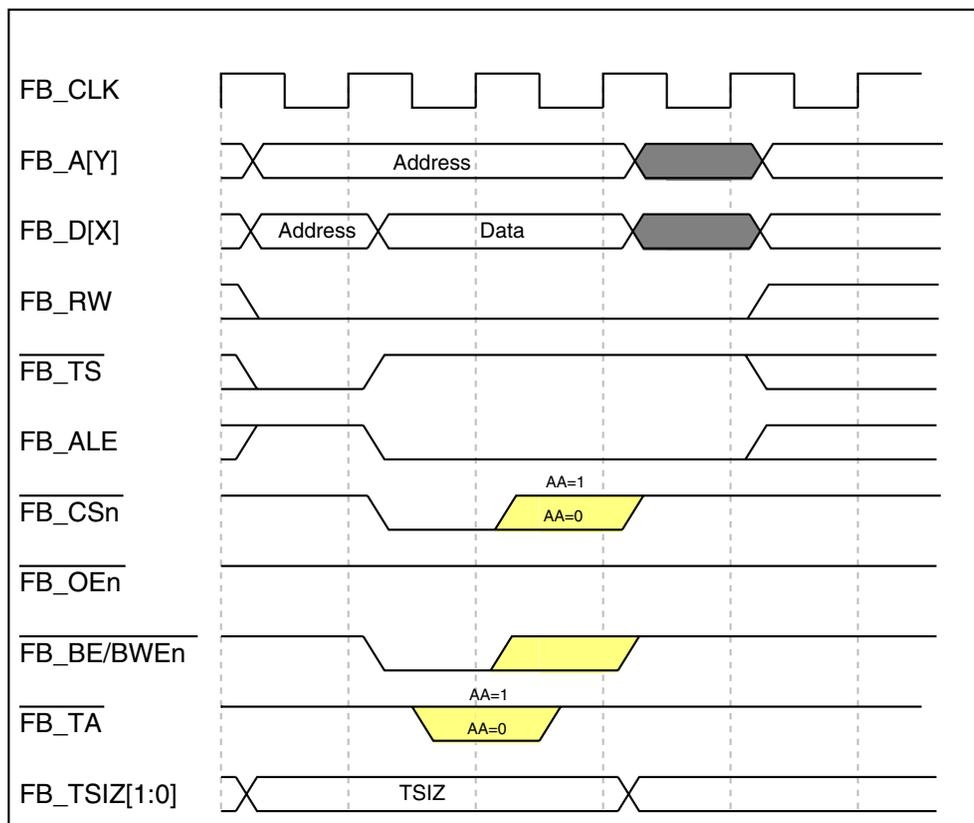
**Figure 33-37. Basic Write-Bus Cycle (No Wait States)**
