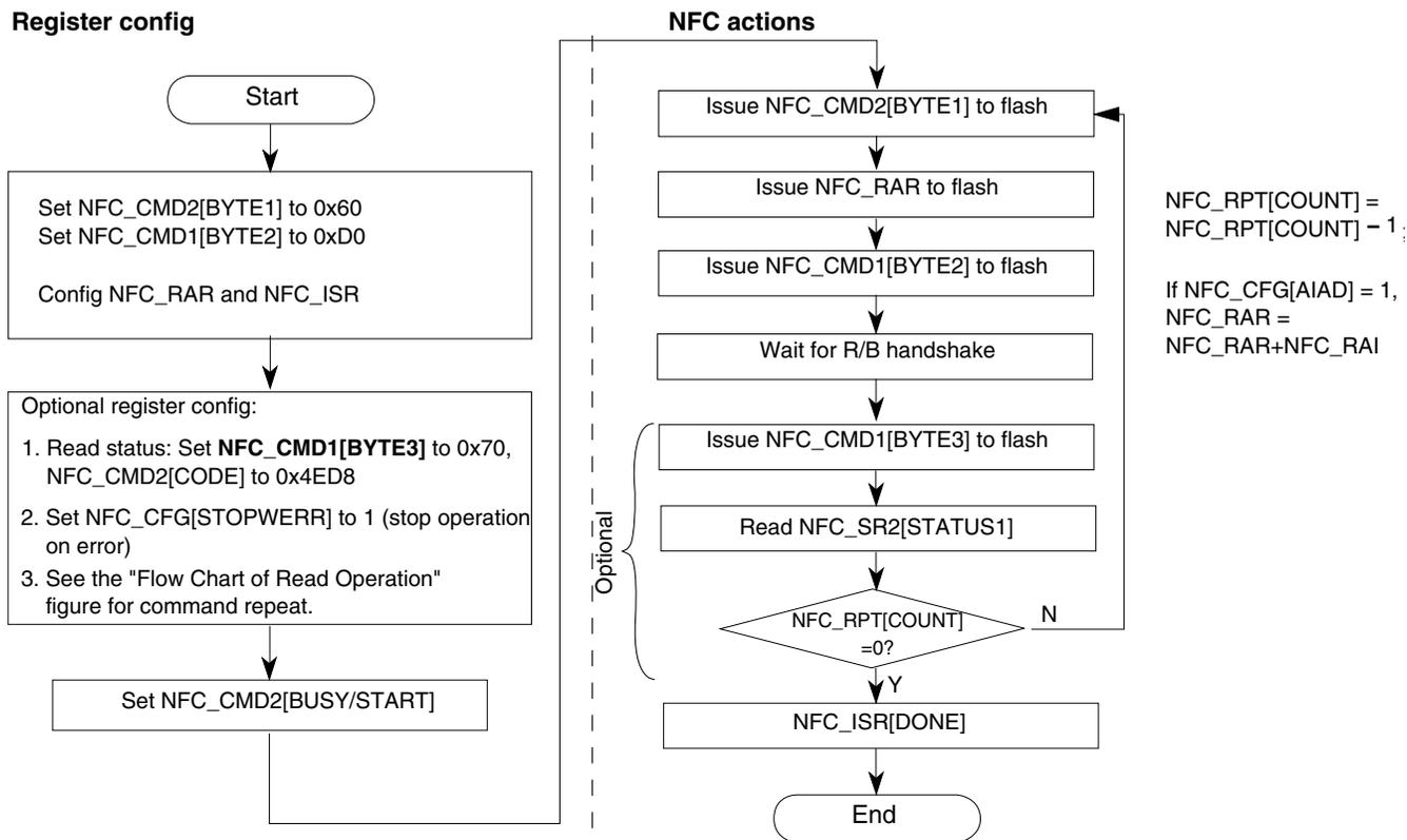
Figure 32-22. Flow Chart of Block Erase Operation
