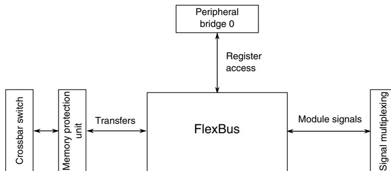
Figure 3-32. FlexBus configuration
