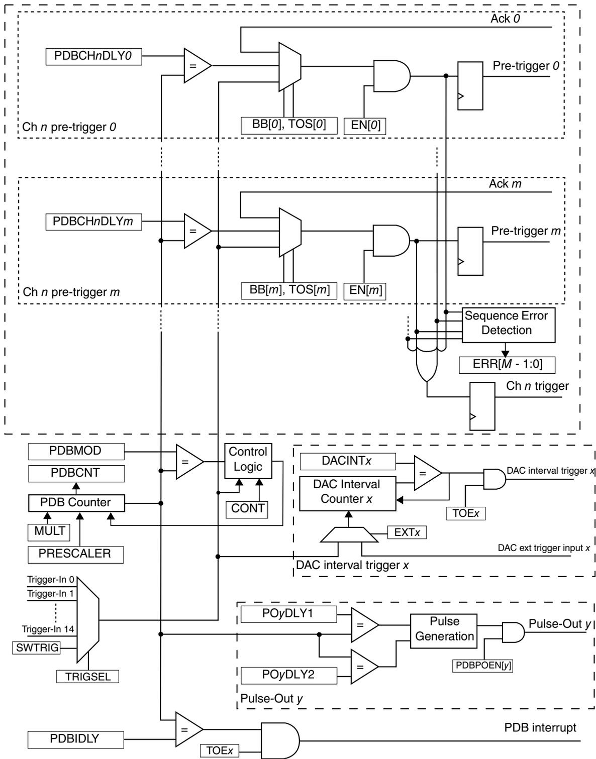
**Figure 41-1. PDB Block Diagram**
