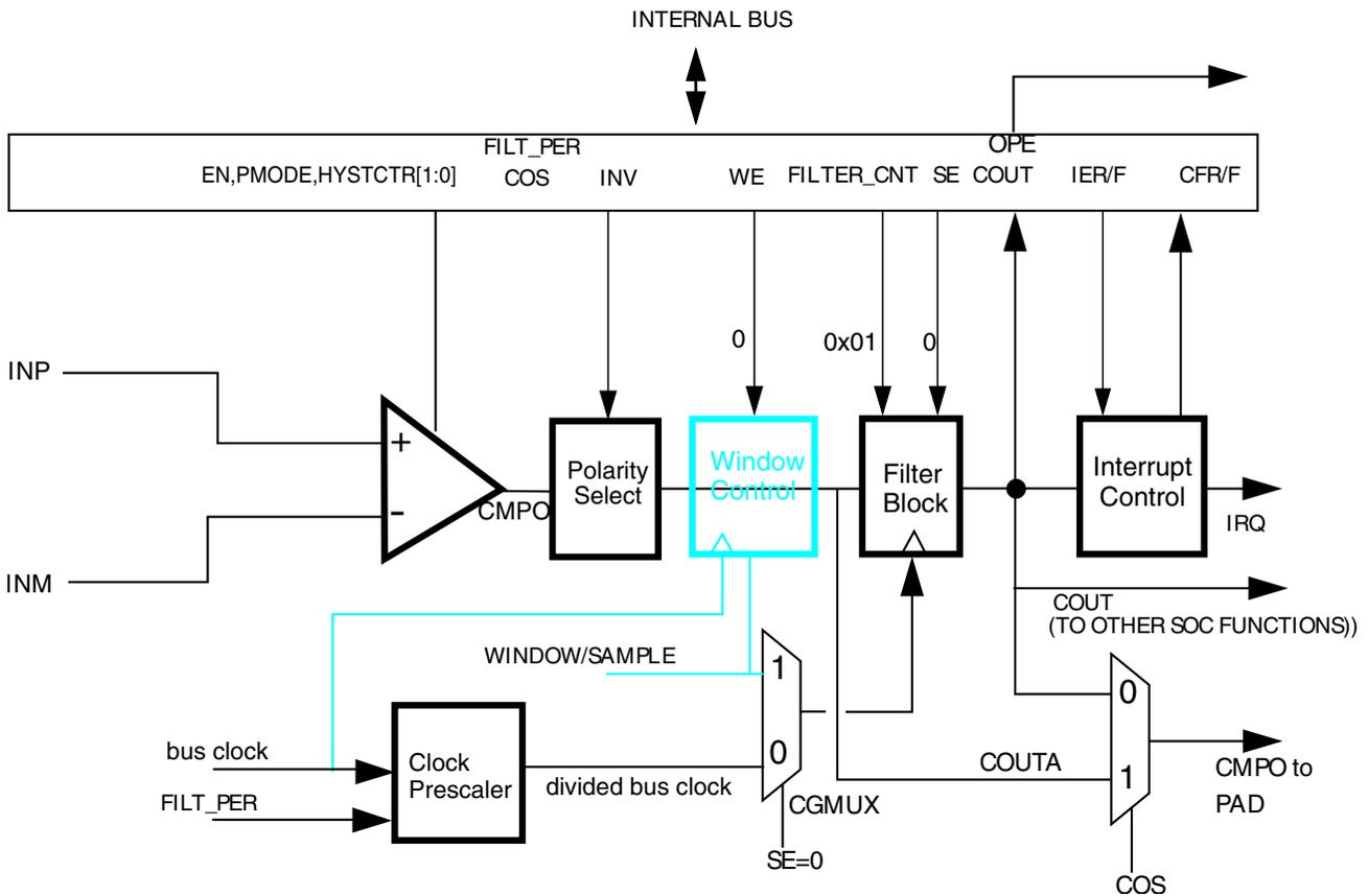
Figure 38-35. Sampled, Non-Filtered (# 3B): Sampling interval internally derived
