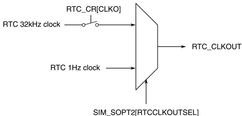
Figure 3-55. RTC\_CLKOUT generation
