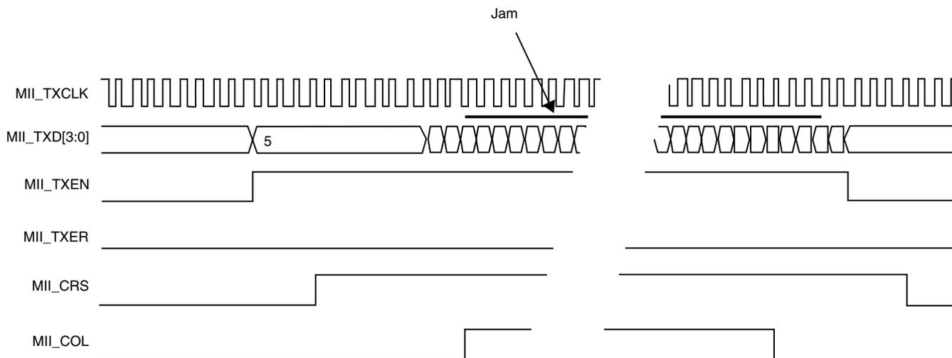
Figure 47-74. MII Transmit Operation — Transmission with Collision
