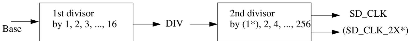
**Figure 56-35. Two stages of the clock divider**
