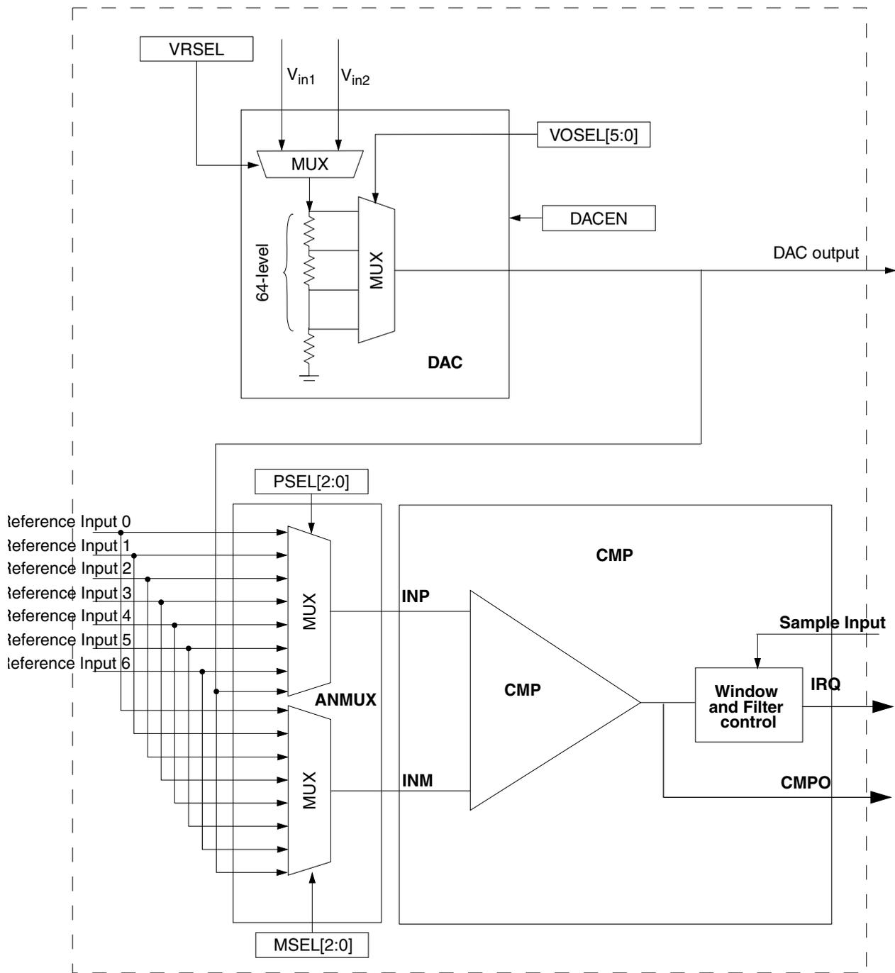
Figure 38-1. CMP, DAC and ANMUX Blocks Diagram
