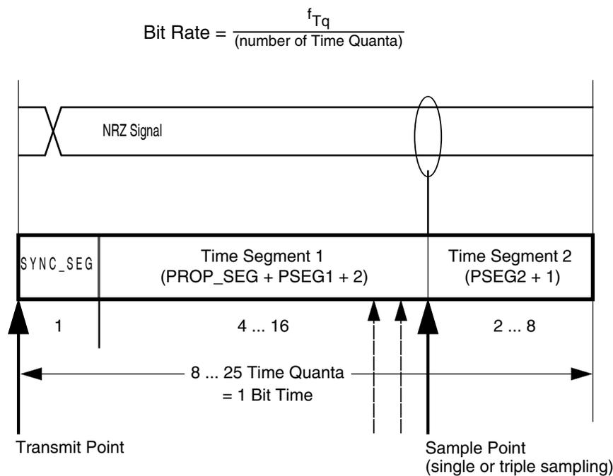
**Figure 52-105. Segments within the Bit Time**
