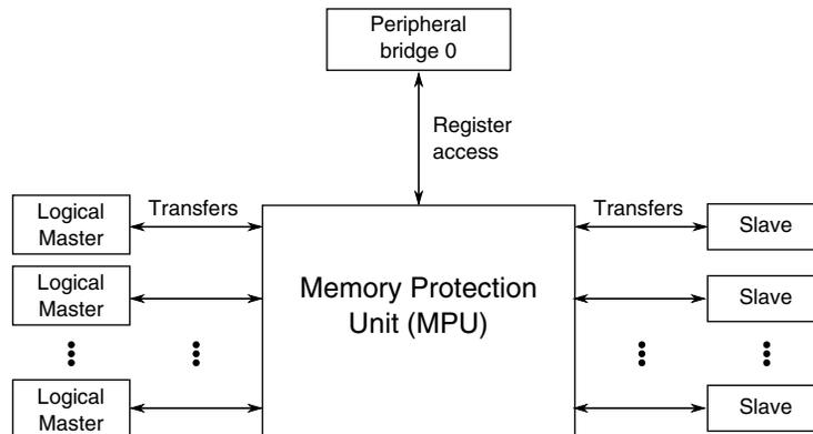
**Figure 3-12. Memory Protection Unit configuration**
