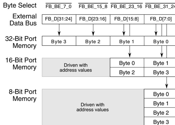
Figure 33-24. Connections for External Memory Port Sizes ( $\text{CSCR}_n[\text{BLS}] = 1$ )
