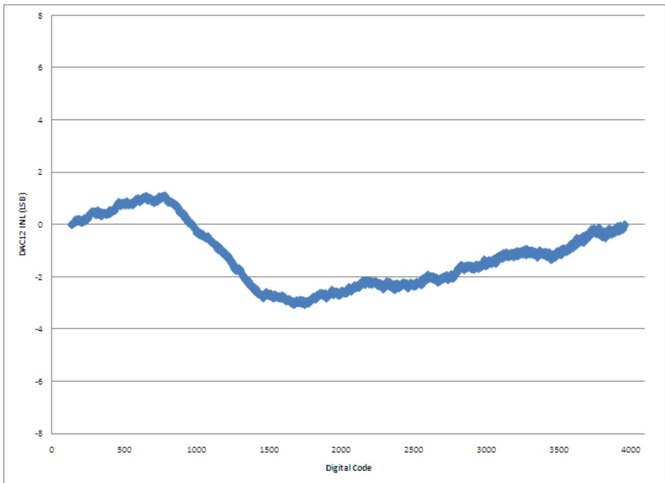
**Figure 18. Typical INL error vs. digital code**
