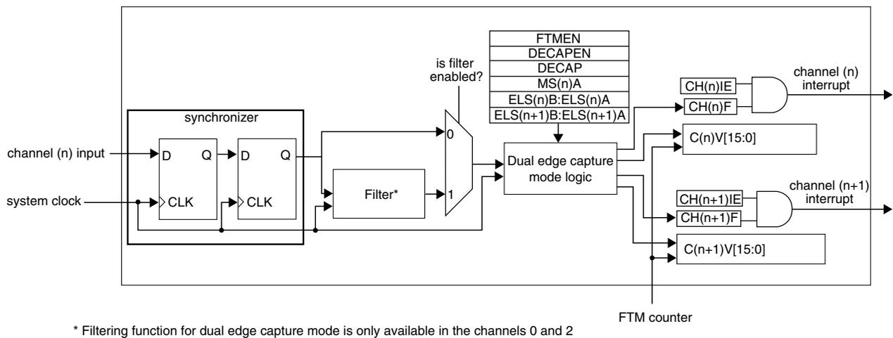
Figure 42-285. Dual Edge Capture Mode Block Diagram
