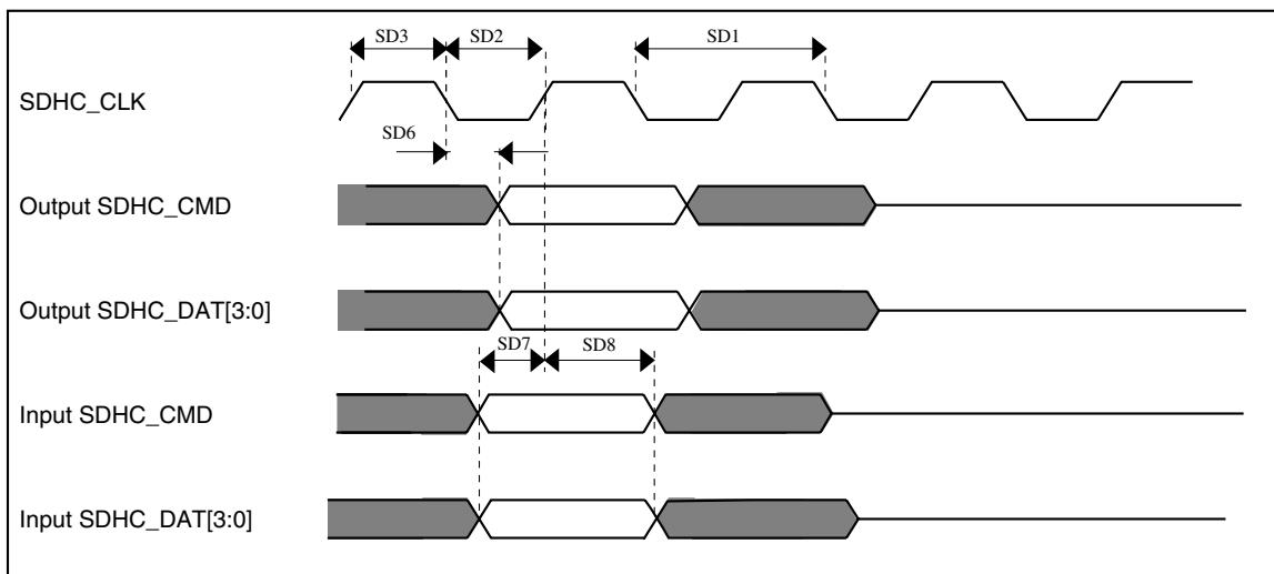
**Figure 27. SDHC timing**
