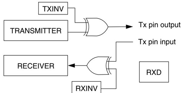
**Figure 59-24. Single-wire operation (C1[LOOPS] = 1, C1[RSRC] = 1)**
