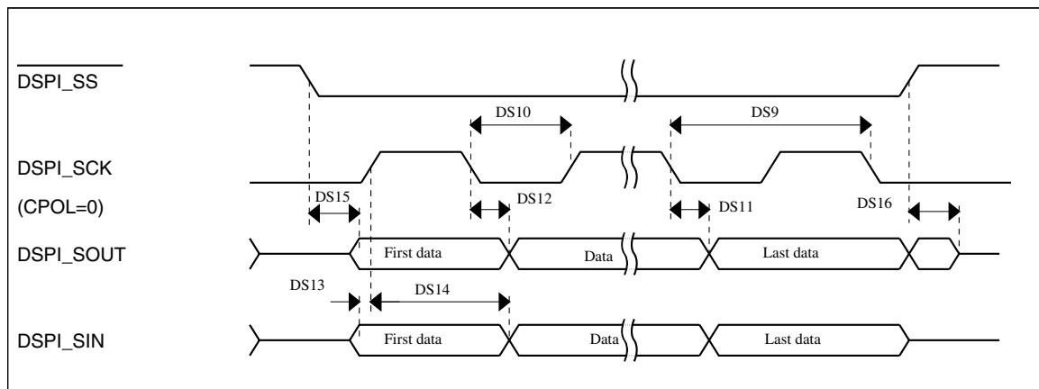
Figure 25. DSPI classic SPI timing — slave mode
