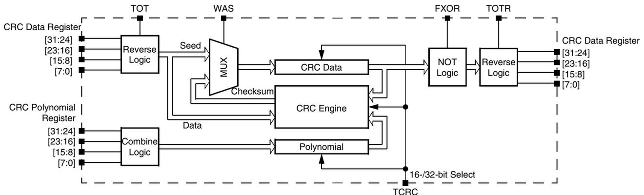
Figure 34-1. Programmable cyclic redundancy check (CRC) block diagram
