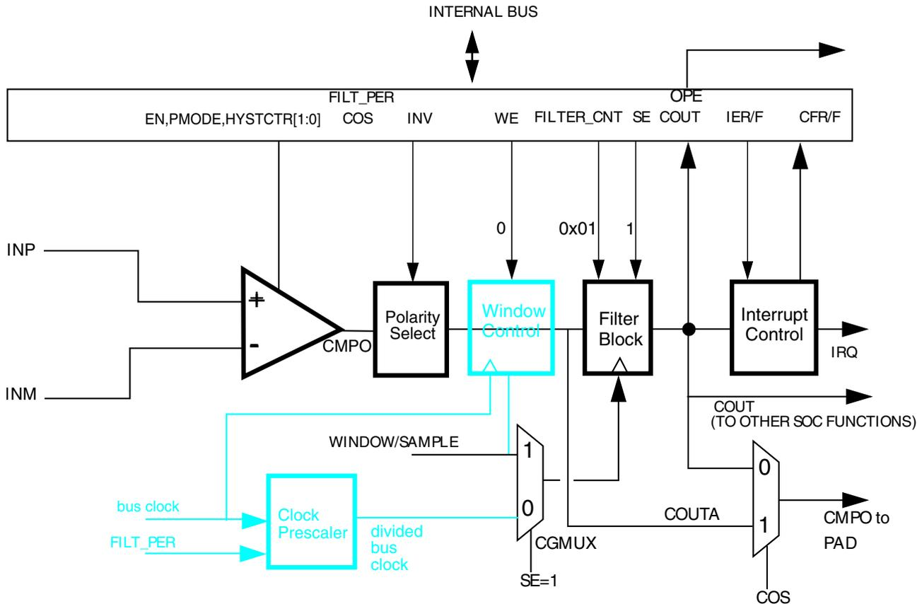
**Figure 38-34. Sampled, Non-Filtered (# 3A): Sampling point externally driven**
