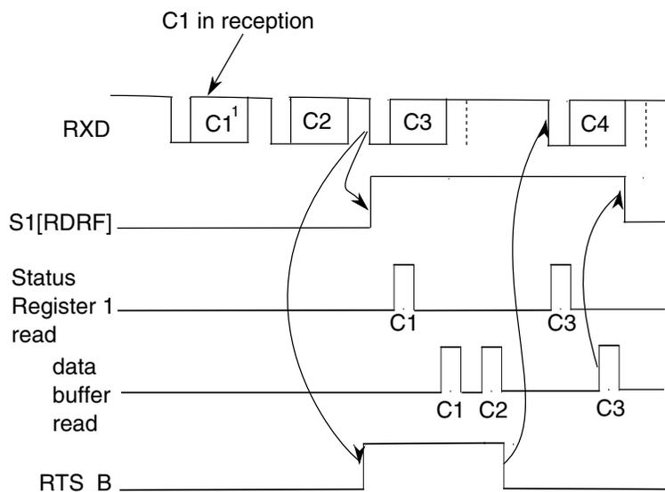
Figure 55-345. Receiver hardware flow control timing diagram
