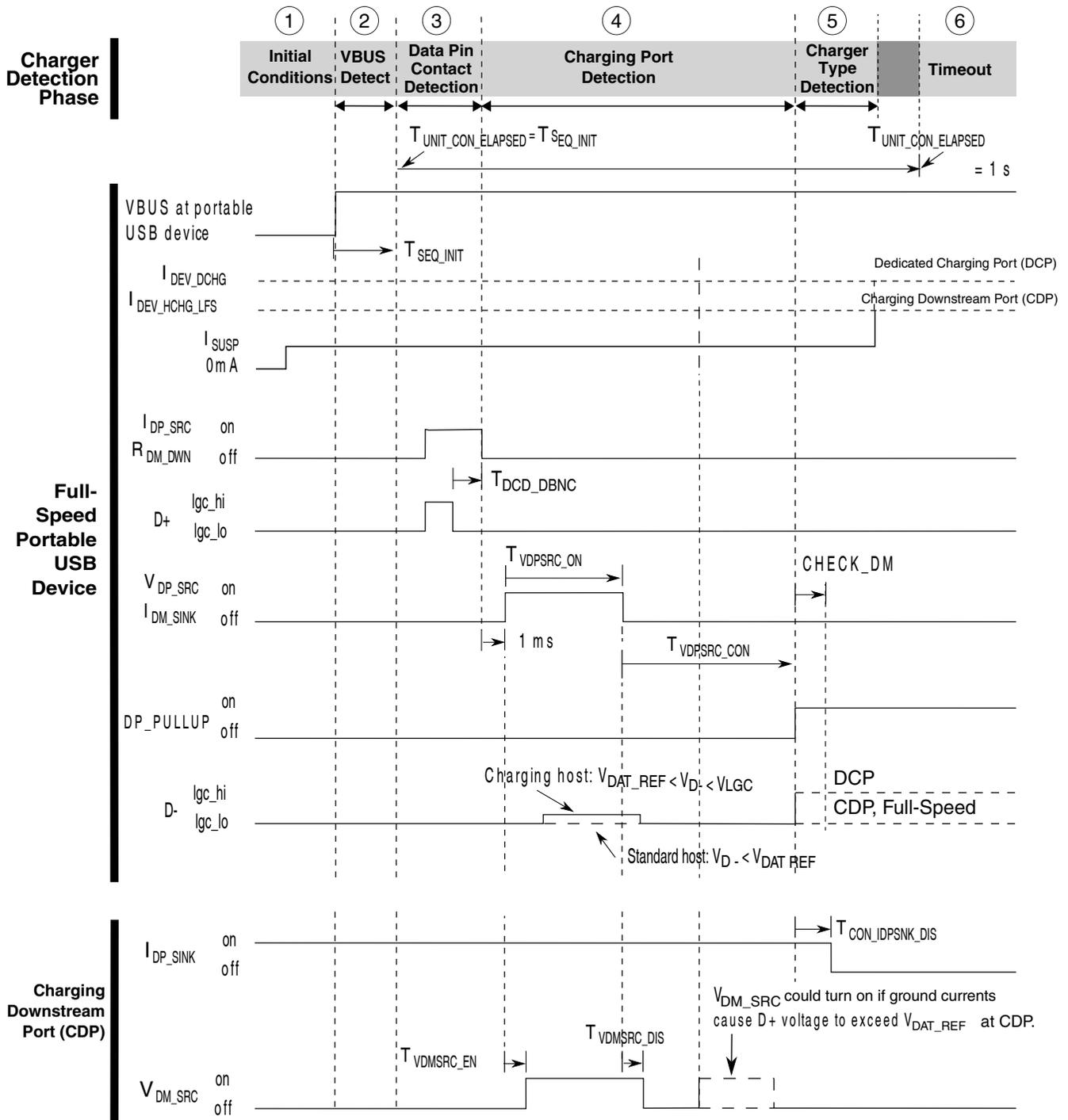
Figure 52-4. Full speed charger detection timing for BC1.1
