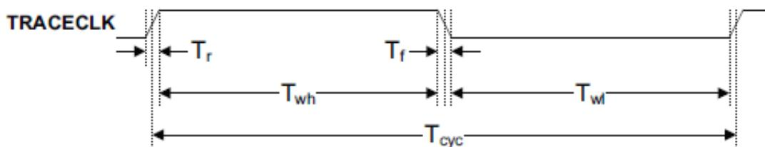
Figure 3. TRACE\_CLKOUT specifications
