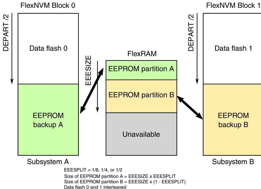
**Figure 32-15. FlexRAM to FlexNVM Memory Mapping for EEPROM**
