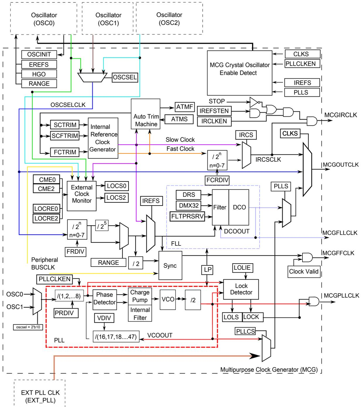
Figure 27-1. Multipurpose Clock Generator (MCG) block diagram
