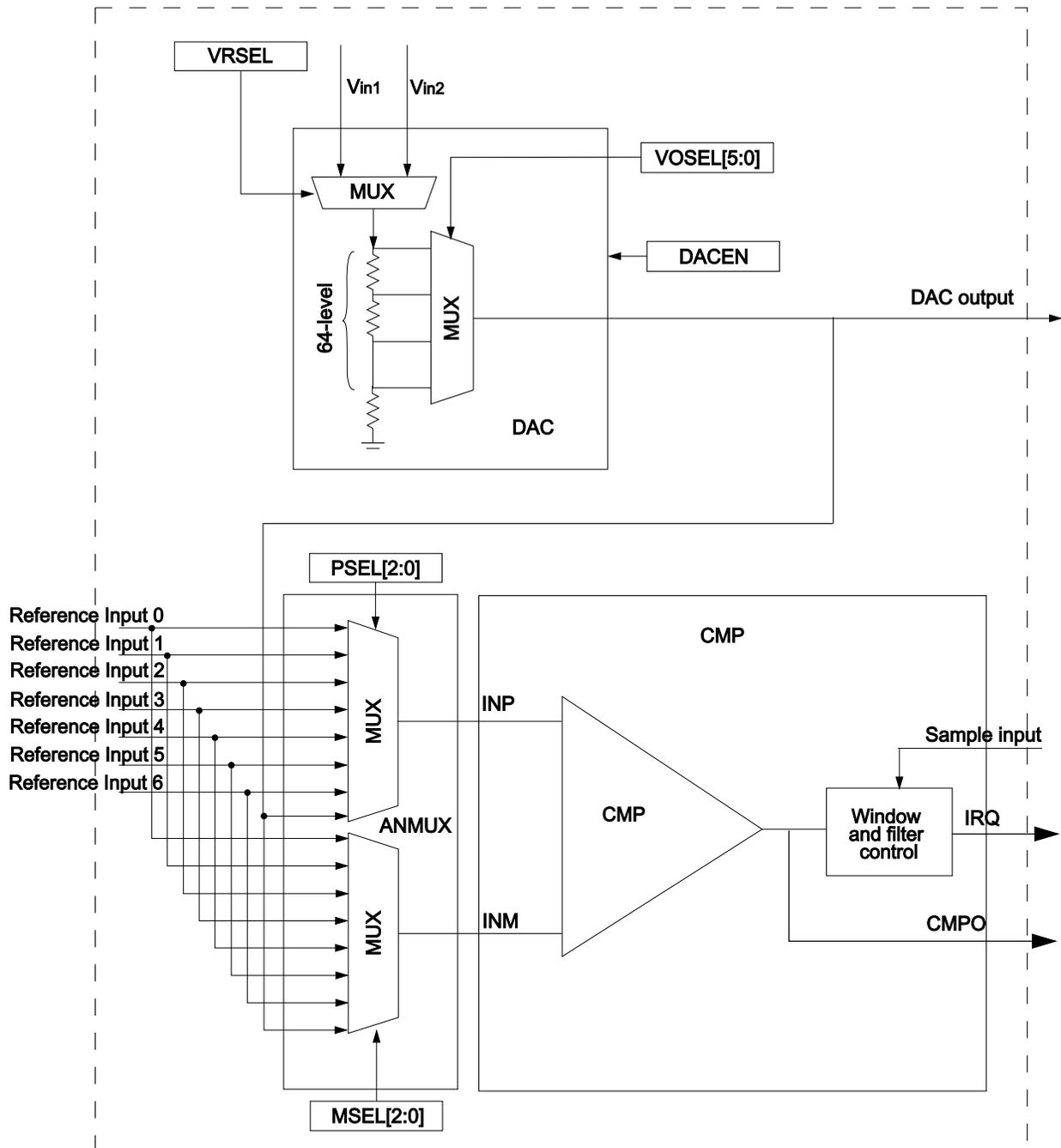
Figure 40-1. CMP, DAC and ANMUX block diagram
