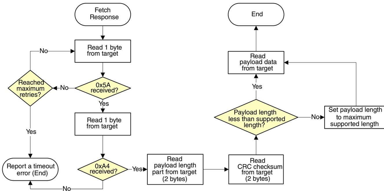
Figure 14-20. Host reads response from target via I2C
