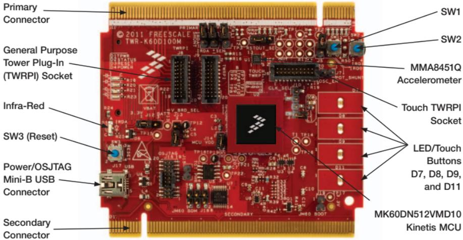
Figure 1: Front side of TWR-K60D100M module.
