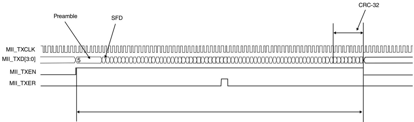
**Figure 50-23. MII transmit operation — errored frame**
