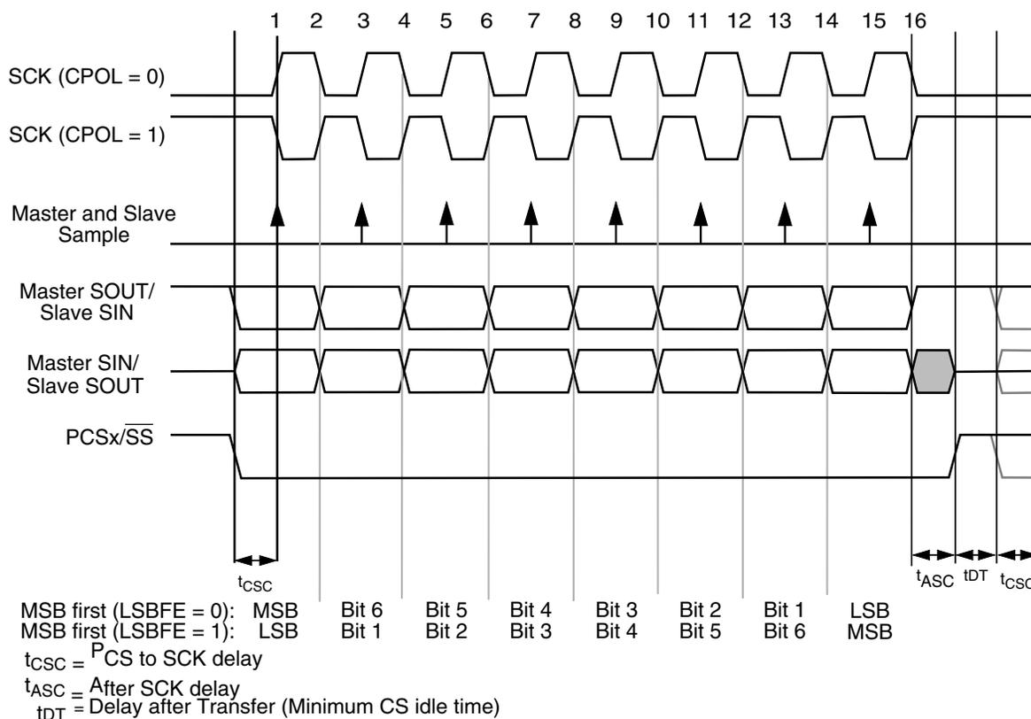
**Figure 53-94. DSPI Transfer Timing Diagram (MTFE=0, CPHA=0, FMSZ=8)**
