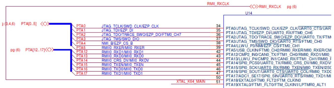
Figure 7. MCU receives RMI0 clock from Micrel Ethernet PHY
