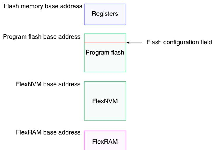
**Figure 3-23. Flash memory map for devices containing FlexNVM**
