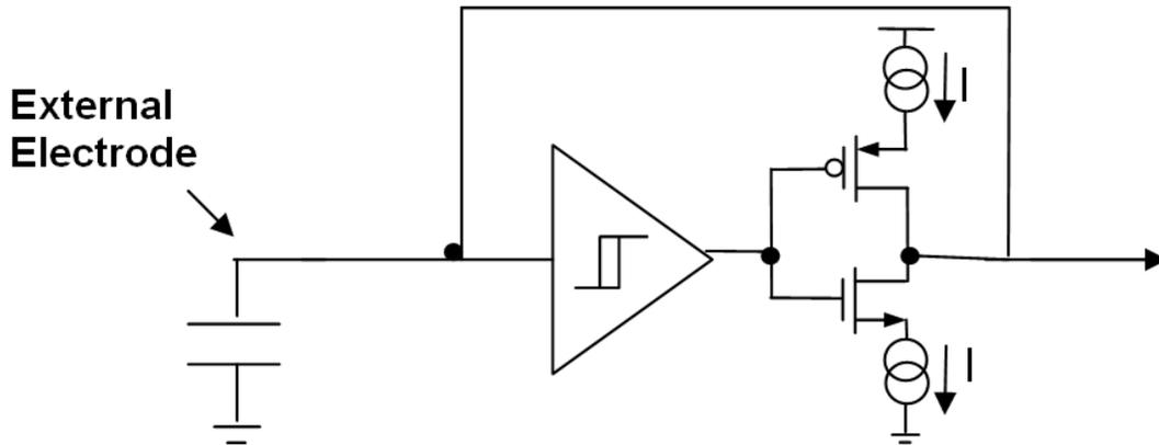
**Figure 59-33. TSI electrode oscillator circuit**
