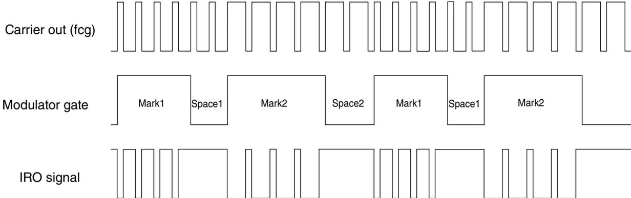
**Figure 48-6. Example: CMT output in FSK mode**
