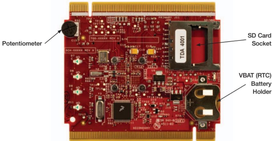
Figure 2: Back side of TWR-K60D100M module.
