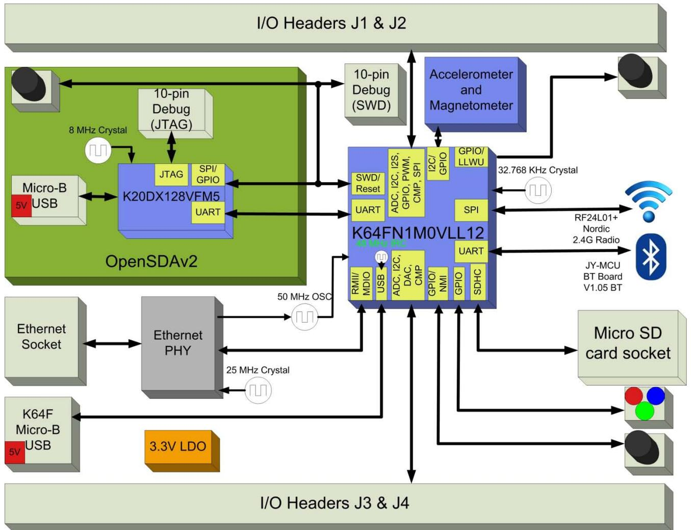
Figure 1. FRDM-K64F block diagram
