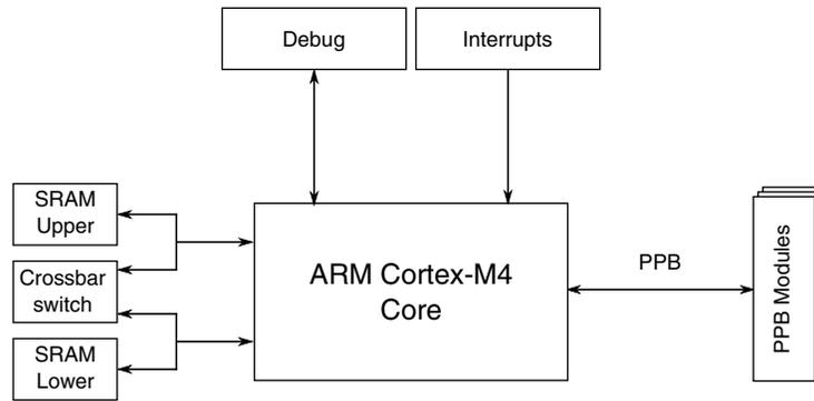
Figure 3-1. Core configuration
