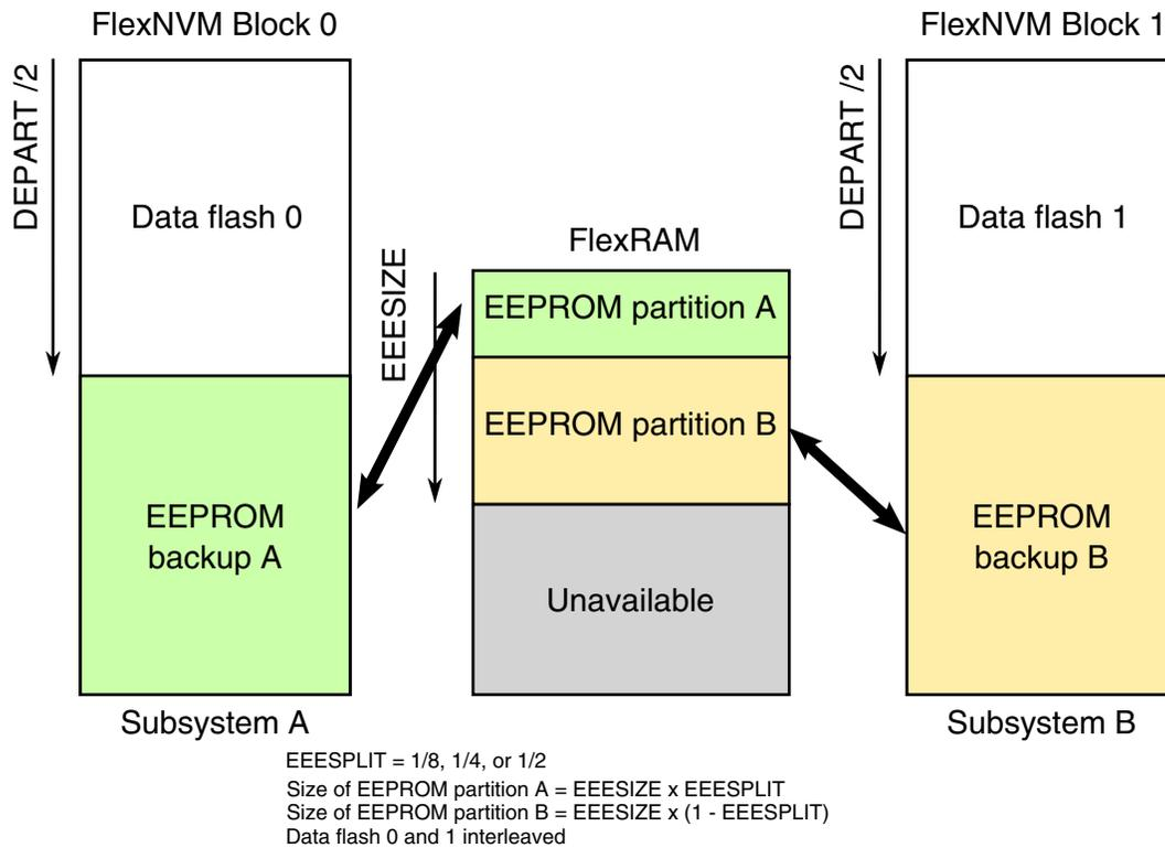
**Figure 30-32. FlexRAM to FlexNVM Memory Mapping for EEPROM**
