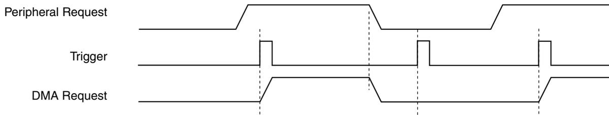
**Figure 21-55. DMA MUX channel triggering: ignored trigger**
