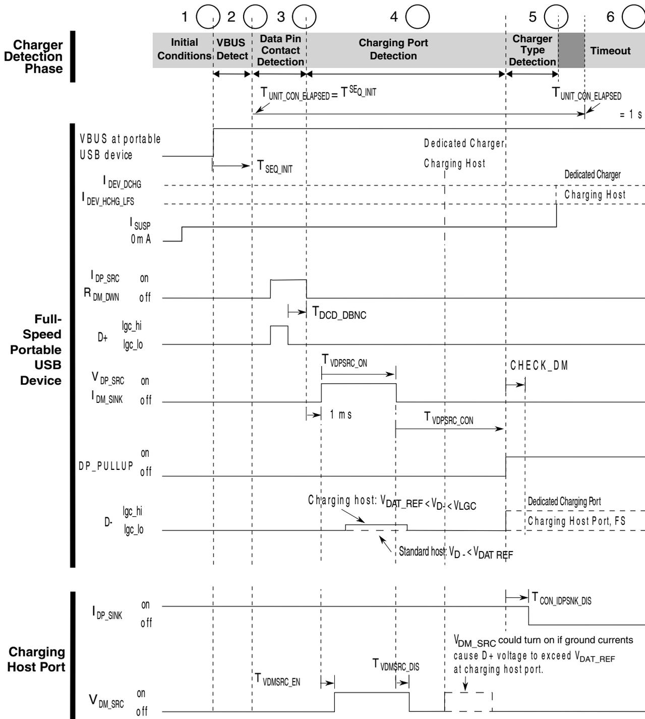
Figure 49-9. Full Speed Charger Detection Timing
