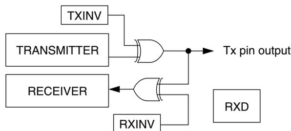
**Figure 59-25. Loop operation (C1[LOOPS] = 1, C1[RSRC] = 0)**
