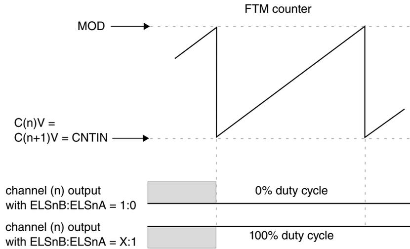
**Figure 45-33. Channel (n) output if  $(C(n)V = C(n+1)V = CNTIN)$**
