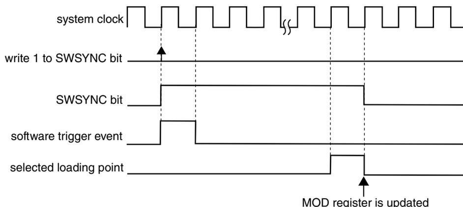
**Figure 45-51. MOD synchronization with (SYNCMODE = 0) and (PWMSYNC = 1)**
