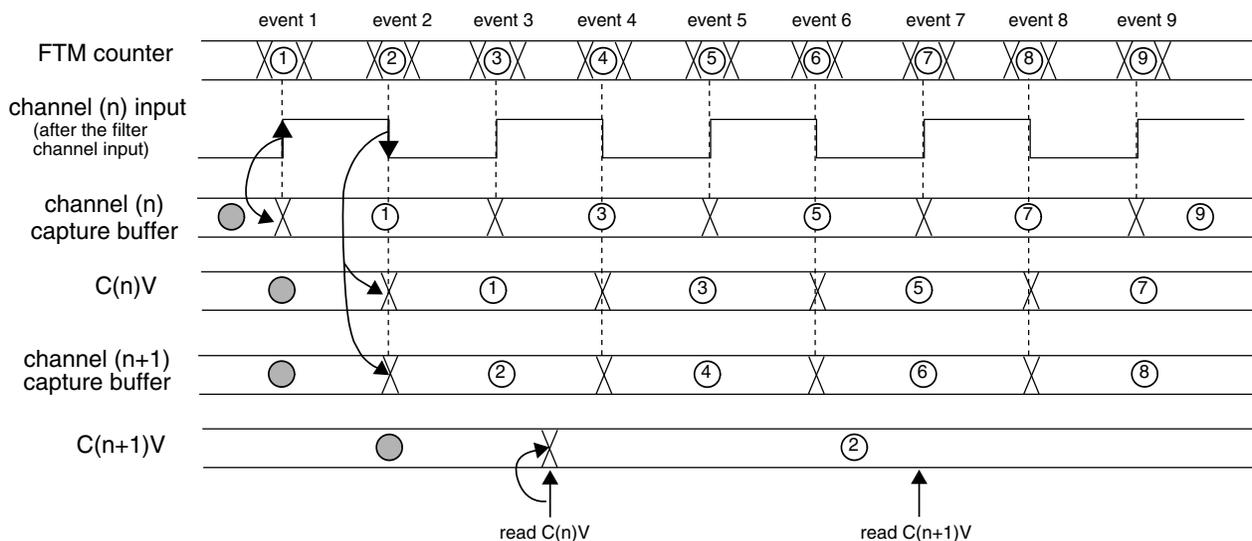
**Figure 42-290. Dual Edge Capture Mode Read Coherency Mechanism**
