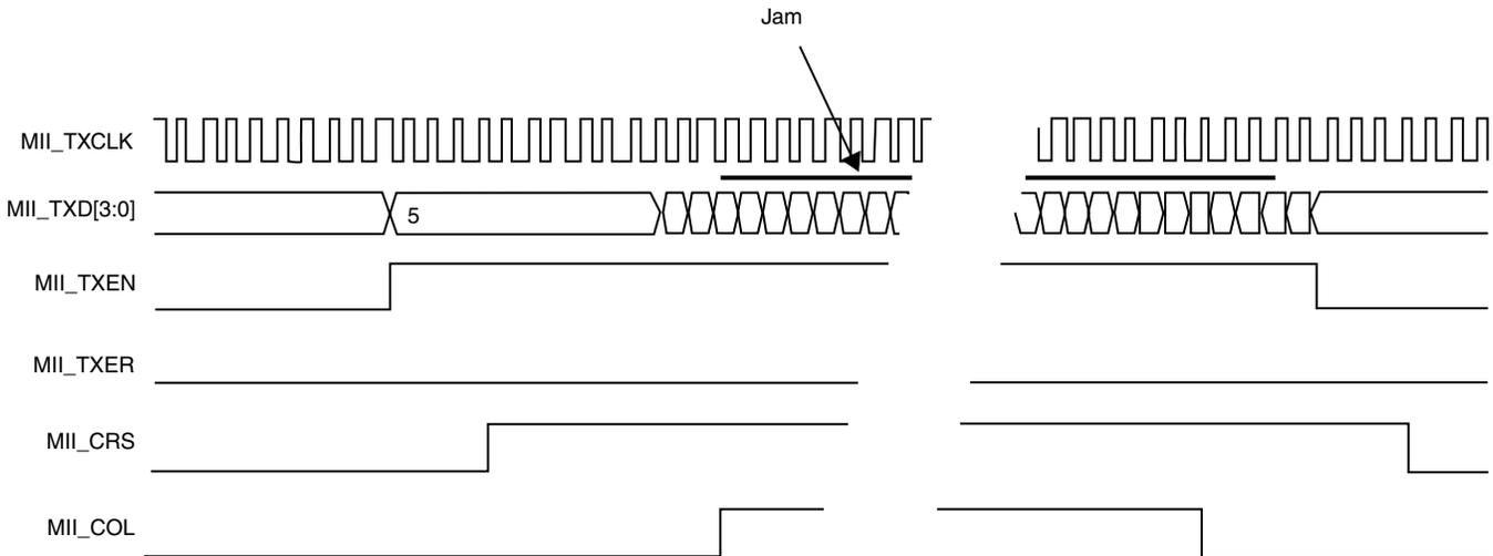
Figure 50-24. MII transmit operation — transmission with collision
