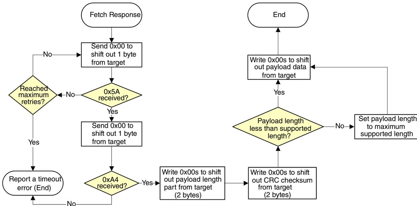
Figure 14-23. Host reads response from target via SPI
