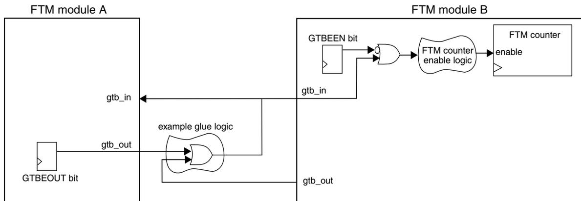
**Figure 45-96. Global time base (GTB) block diagram**
