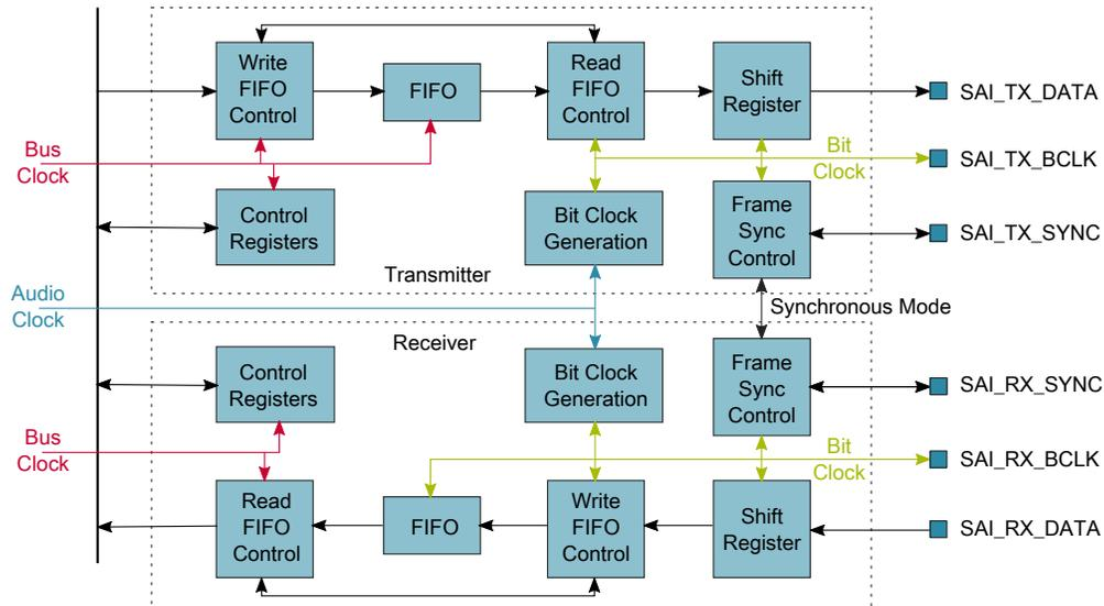
Figure 61-1. I<sup>2</sup>S/SAI block diagram
