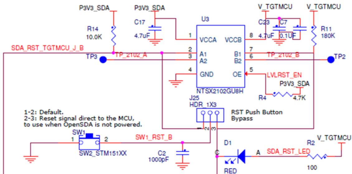
Figure 15. Reset circuit
