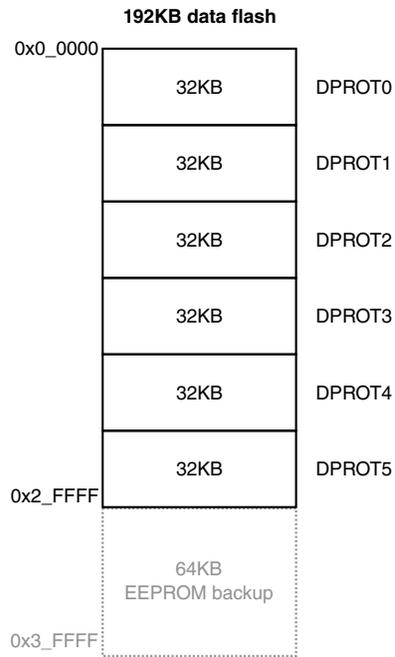
**Figure 32-8. Data flash protection (192KB data flash size)**
