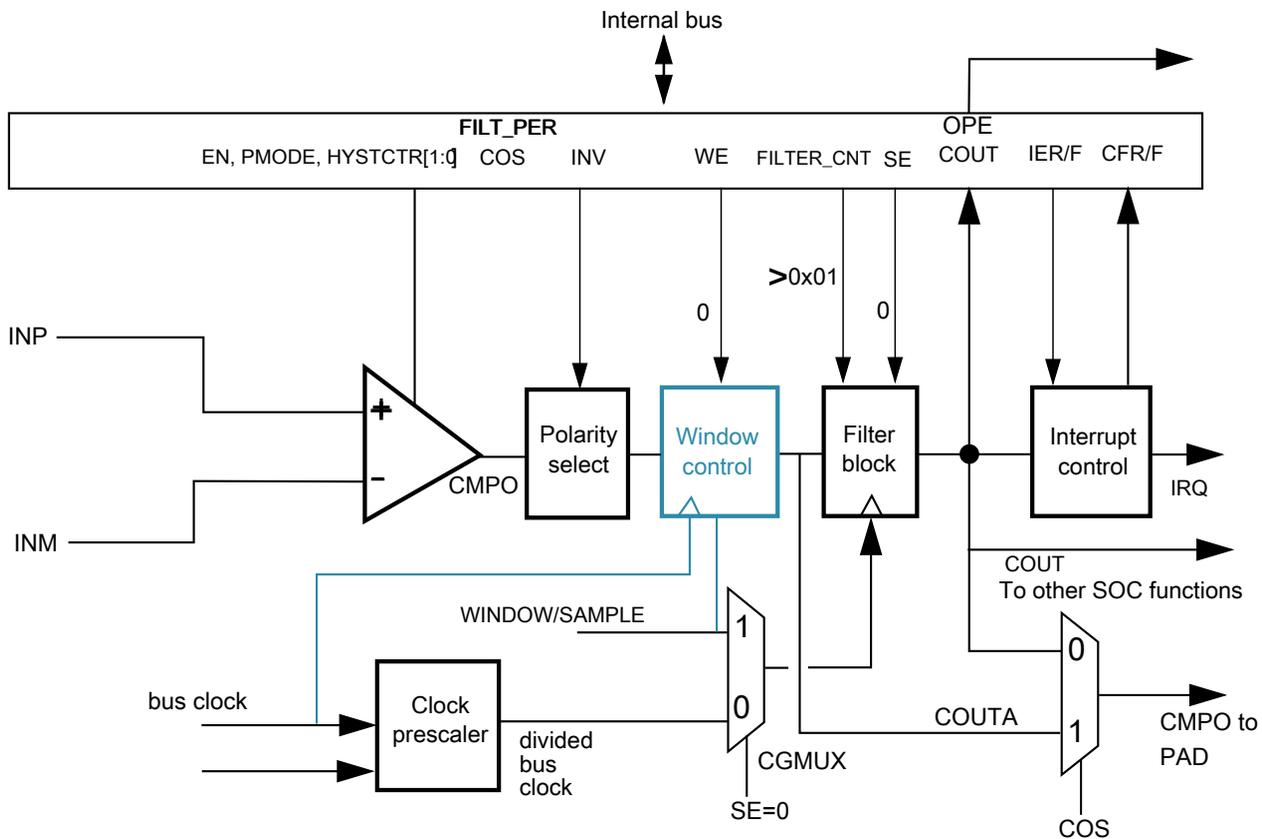
**Figure 40-7. Sampled, Filtered (# 4B): sampling point internally derived**
