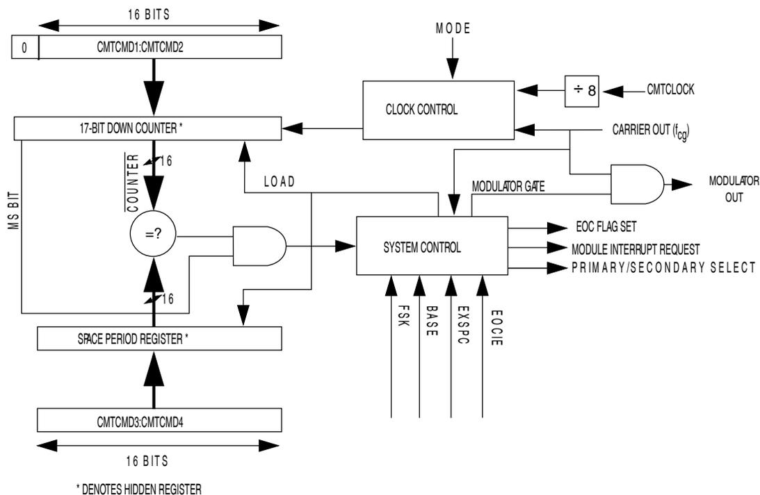
**Figure 45-16. Modulator Block Diagram**
