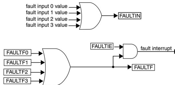
**Figure 45-72. FAULTF and FAULTIN bits and fault interrupt**
