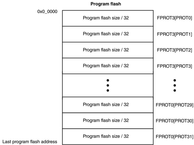
**Figure 32-4. Program flash protection (2MB of program flash)**
