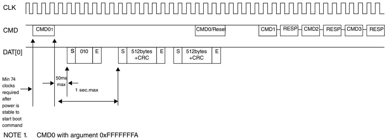
**Figure 60-14. MultiMediaCard state diagram in Alternative Boot mode**
