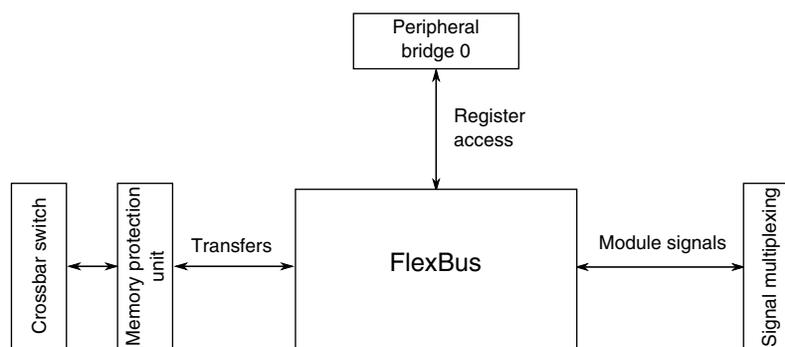
**Figure 3-32. FlexBus configuration**
