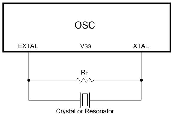
Figure 28-3. Crystal/Ceramic Resonator Connections - Connection 2
