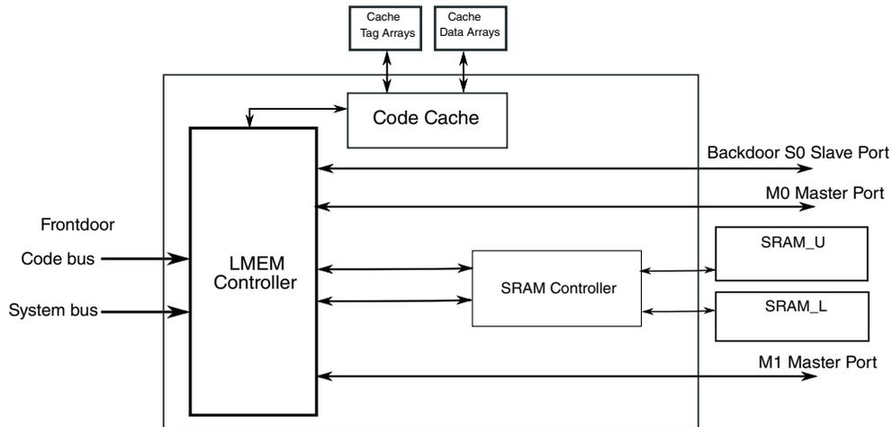
**Figure 30-2. SRAM configuration**
