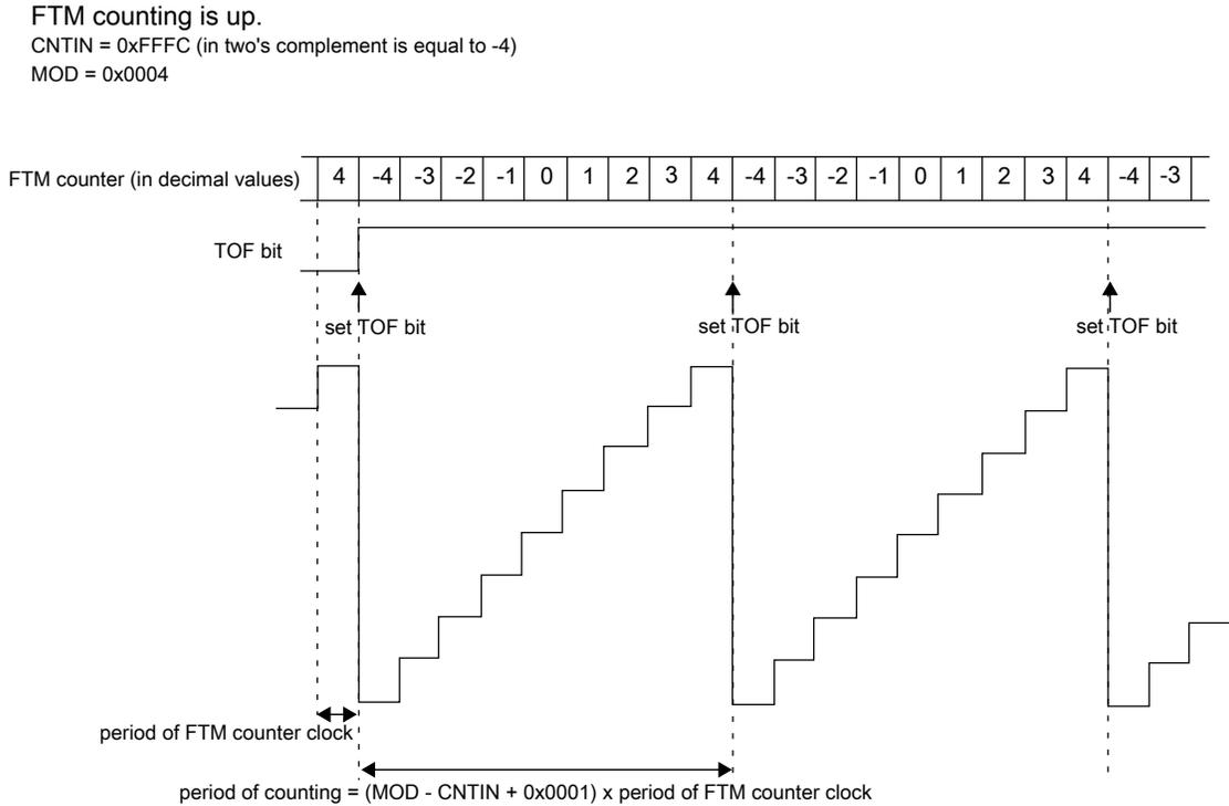
**Figure 45-6. Example of FTM up and signed counting**
