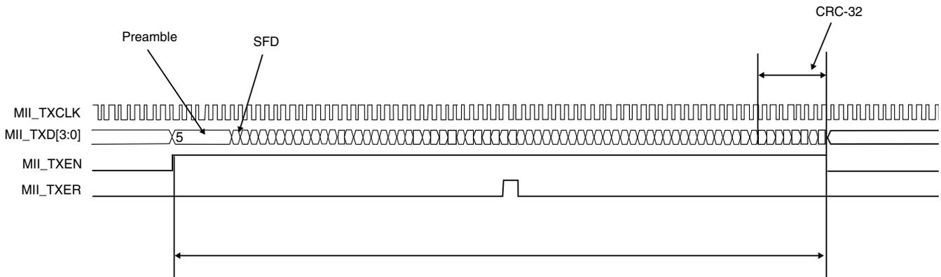
**Figure 47-73. MII Transmit Operation — Errored Frame**
