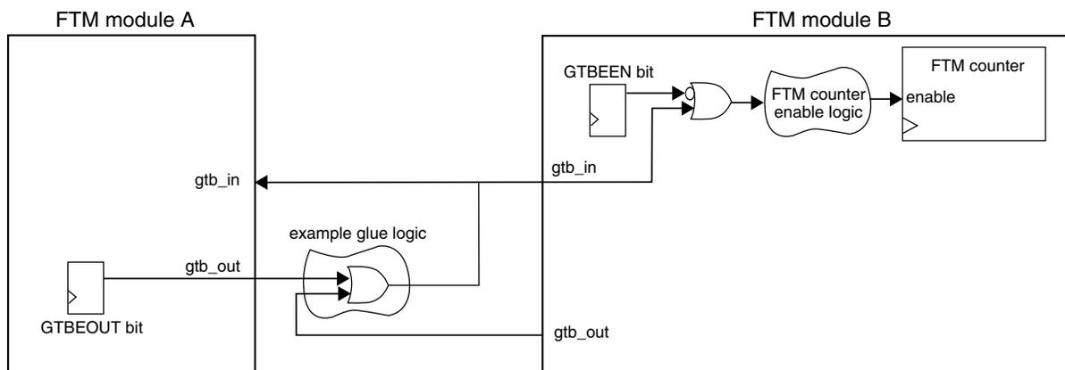
**Figure 42-299. Global Time Base (GTB) Block Diagram**
