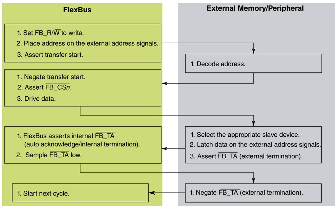
**Figure 34-6. Write-Cycle Flowchart**
