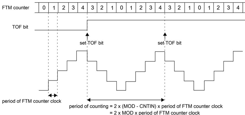
**Figure 45-9. Example of up-down counting when CNTIN = 0x0000**
