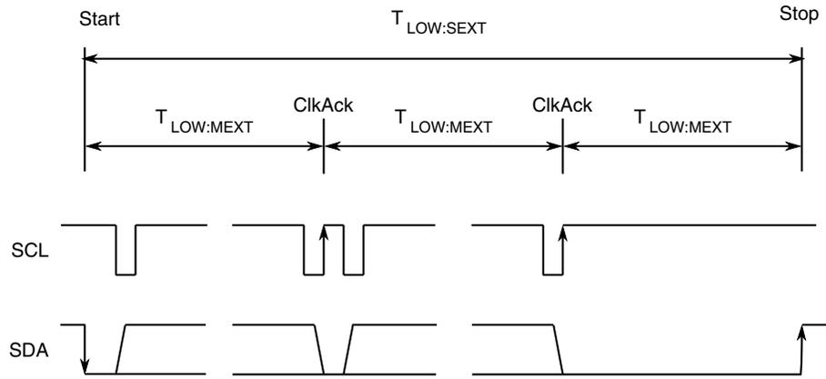
**Figure 54-40. Timeout measurement intervals**
