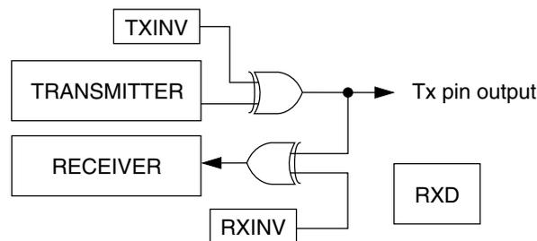
**Figure 55-359. Loop operation (C1[LOOPS] = 1, C1[RSRC] = 0)**
