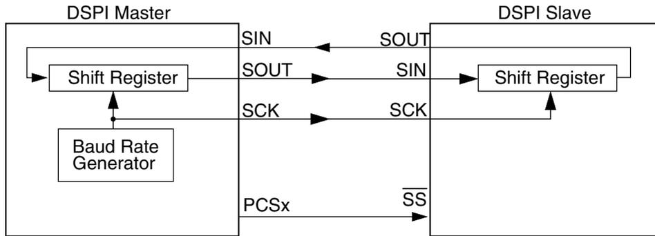
Figure 53-91. SPI Serial Protocol Overview
