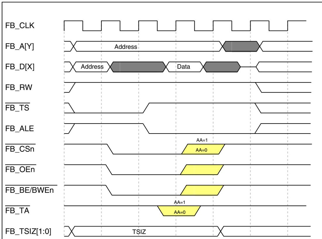
Figure 33-53. Read-Bus Cycle with  $\text{CSCR}_n[\text{EXTS}] = 1$  (One Wait State)
