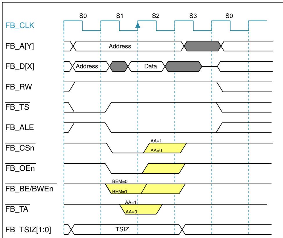
Figure 34-14. Basic Read-Bus Cycle (No Wait States)
