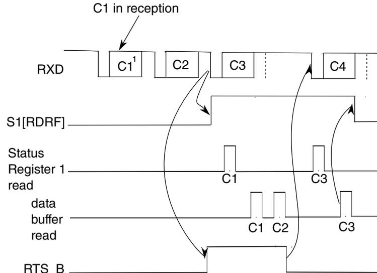
**Figure 59-11. Receiver hardware flow control timing diagram**
