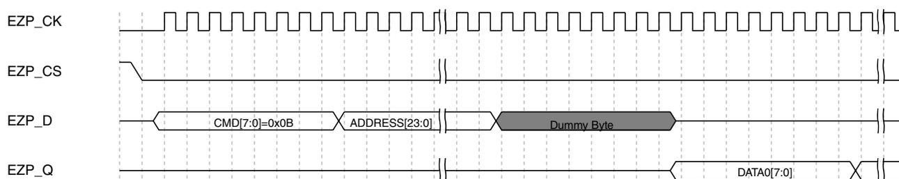
**Figure 33-6. Read Data at High Speed command sequence**
