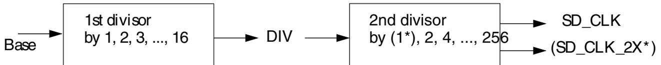
**Figure 60-11. Two stages of the clock divider**
