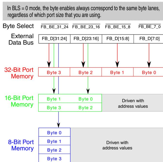
**Figure 34-2. Connections for external memory port sizes (CSCRn[BLS] = 0)**
