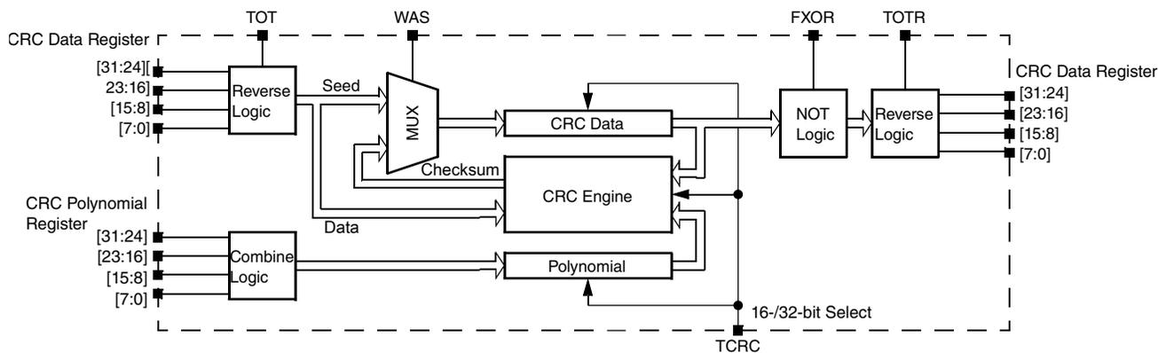
Figure 36-1. Programmable cyclic redundancy check (CRC) block diagram
