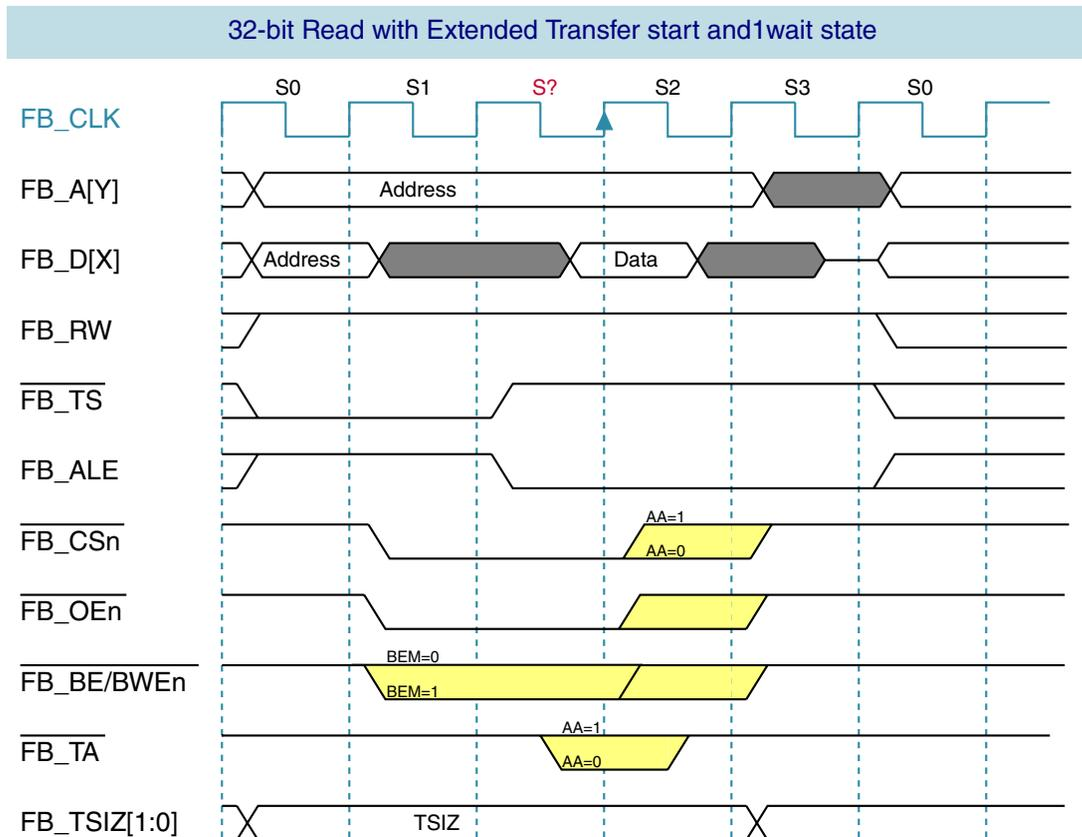
Figure 34-30. Read-Bus Cycle with CSCRn[EXTS] = 1 (One Wait State)
