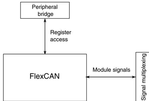
**Figure 3-66. CAN configuration**
