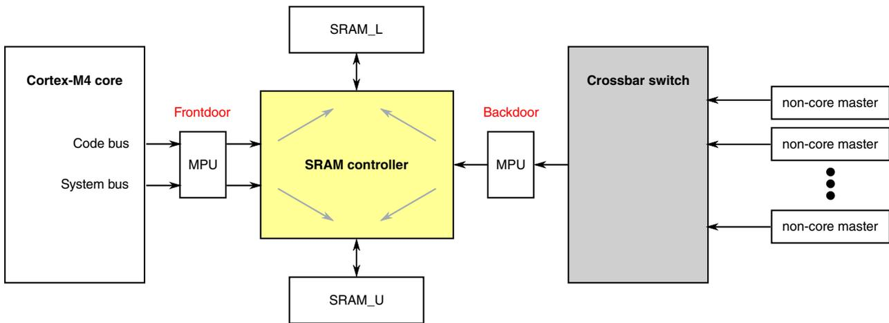
**Figure 4-1. SRAM access diagram**
