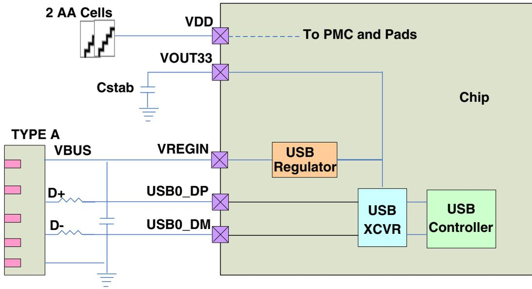
Figure 3-58. USB regulator AA cell usecase
