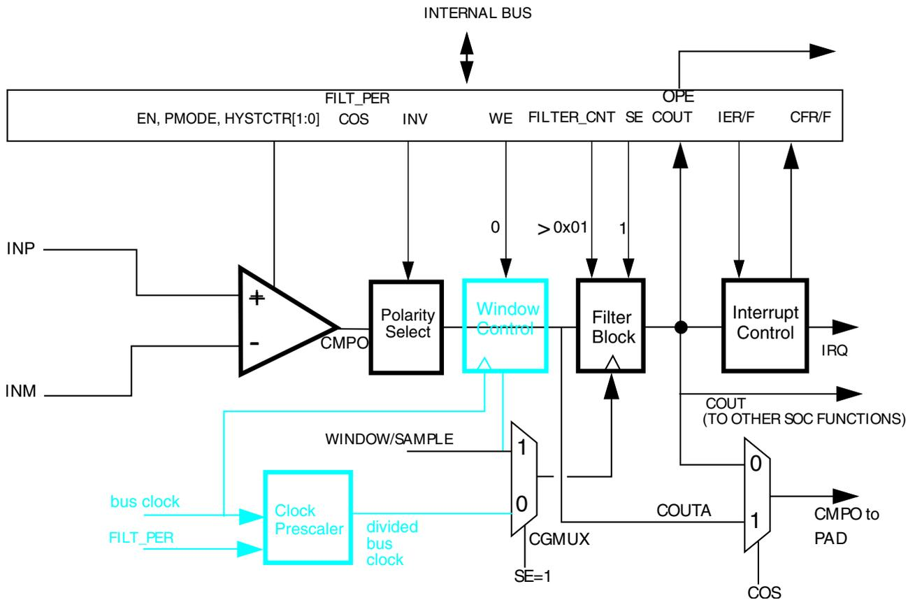
Figure 38-36. Sampled, Filtered (# 4A): Sampling point externally driven
