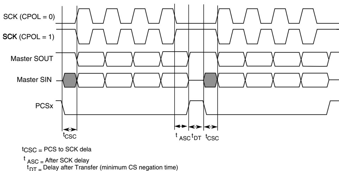
**Figure 53-96. Example of Non-Continuous Format (CPHA=1, CONT=0)**
