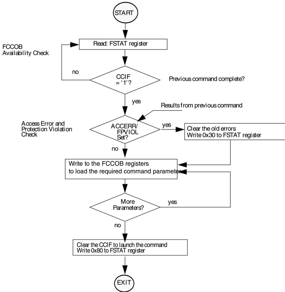
Figure 32-17. Generic Flash Command Write Sequence Flowchart
