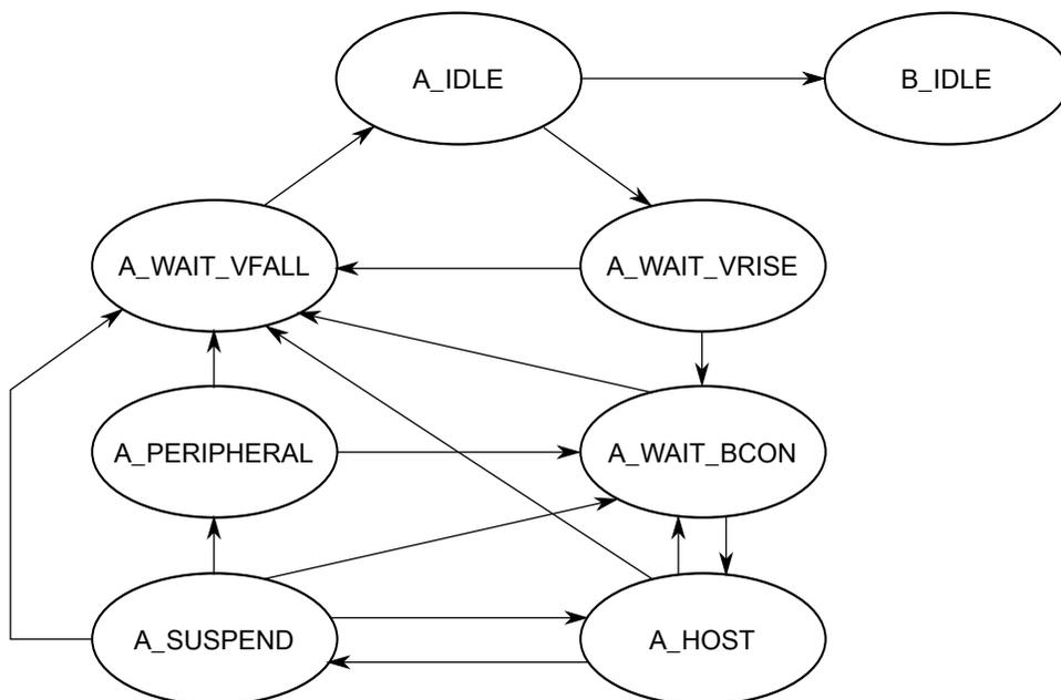
Figure 51-12. Dual role A device flow diagram
