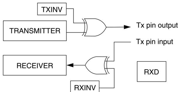
Figure 55-358. Single-wire operation (C1[LOOPS] = 1, C1[RSRC] = 1)
