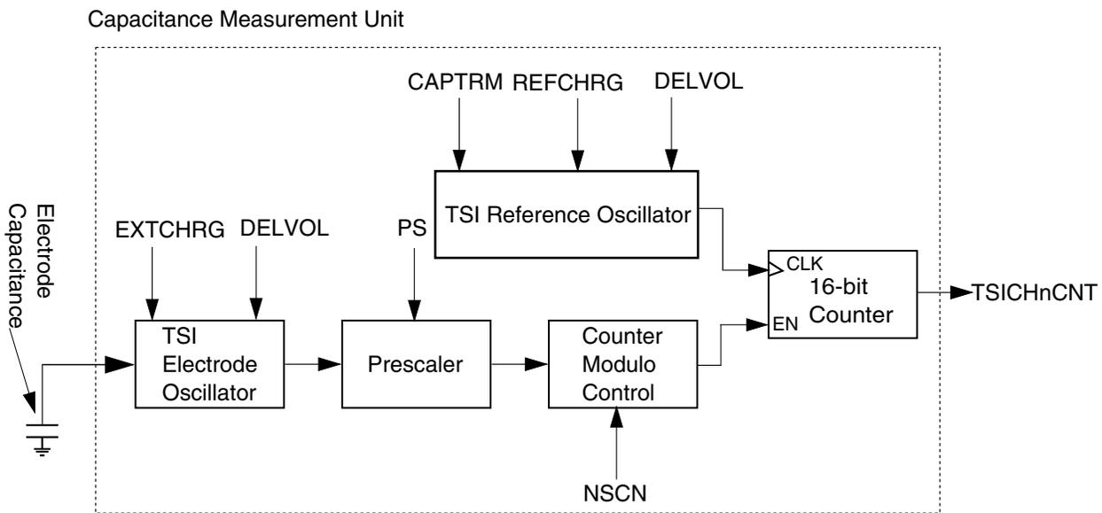
Figure 59-2. TSI capacitance measurement unit block diagram
