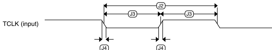
**Figure 5. Test clock input timing**
