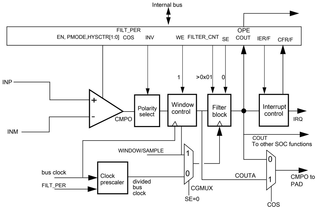
Figure 40-11. Windowed/Filtered mode
