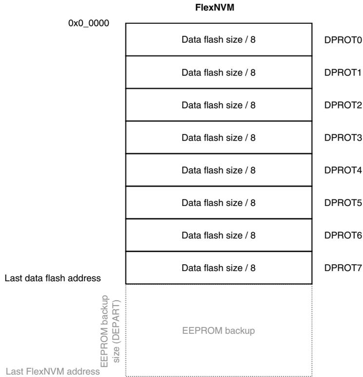
**Figure 30-28. Data flash protection ( $2^n$  data flash sizes)**
