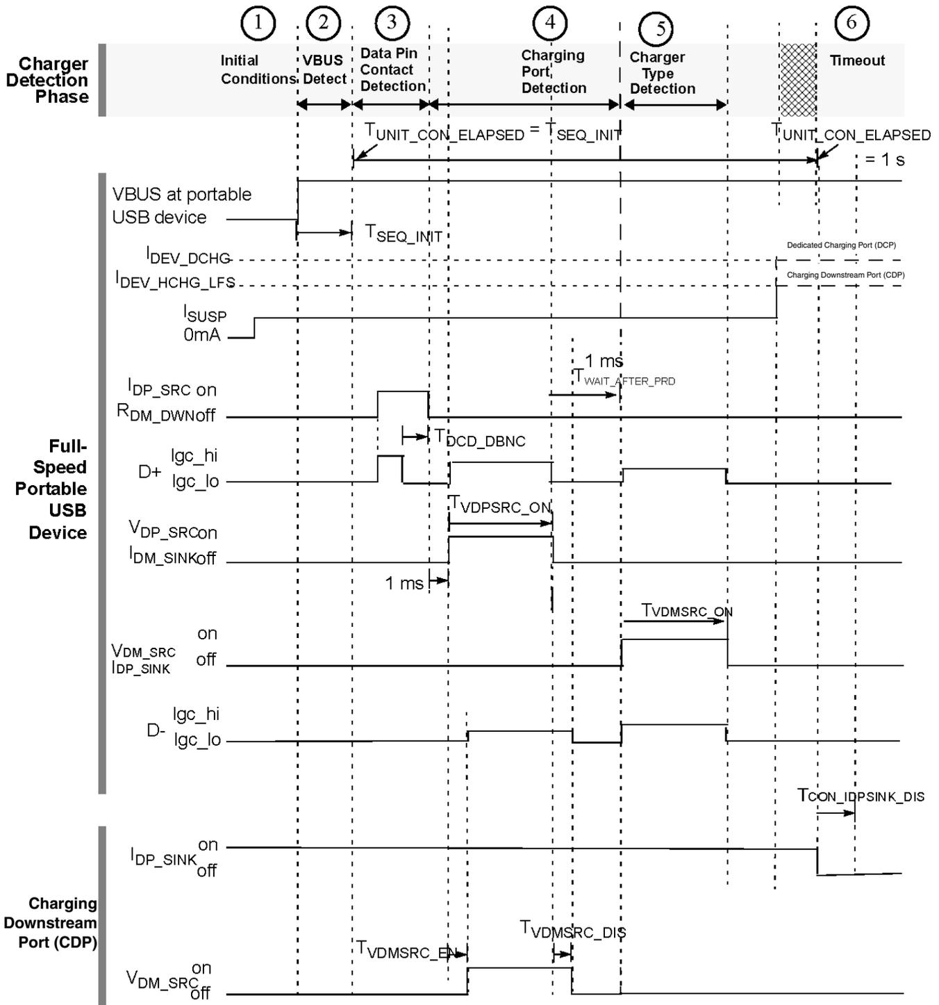
Figure 52-3. Full speed charger detection timing for BC1.2
