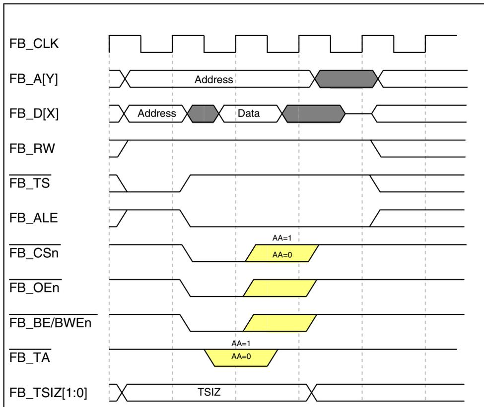
Figure 33-36. Basic Read-Bus Cycle (No Wait States)
