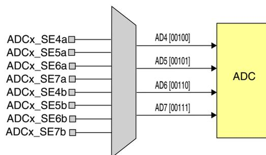
Figure 39-1. ADCx\_SEn channels a and b selection
