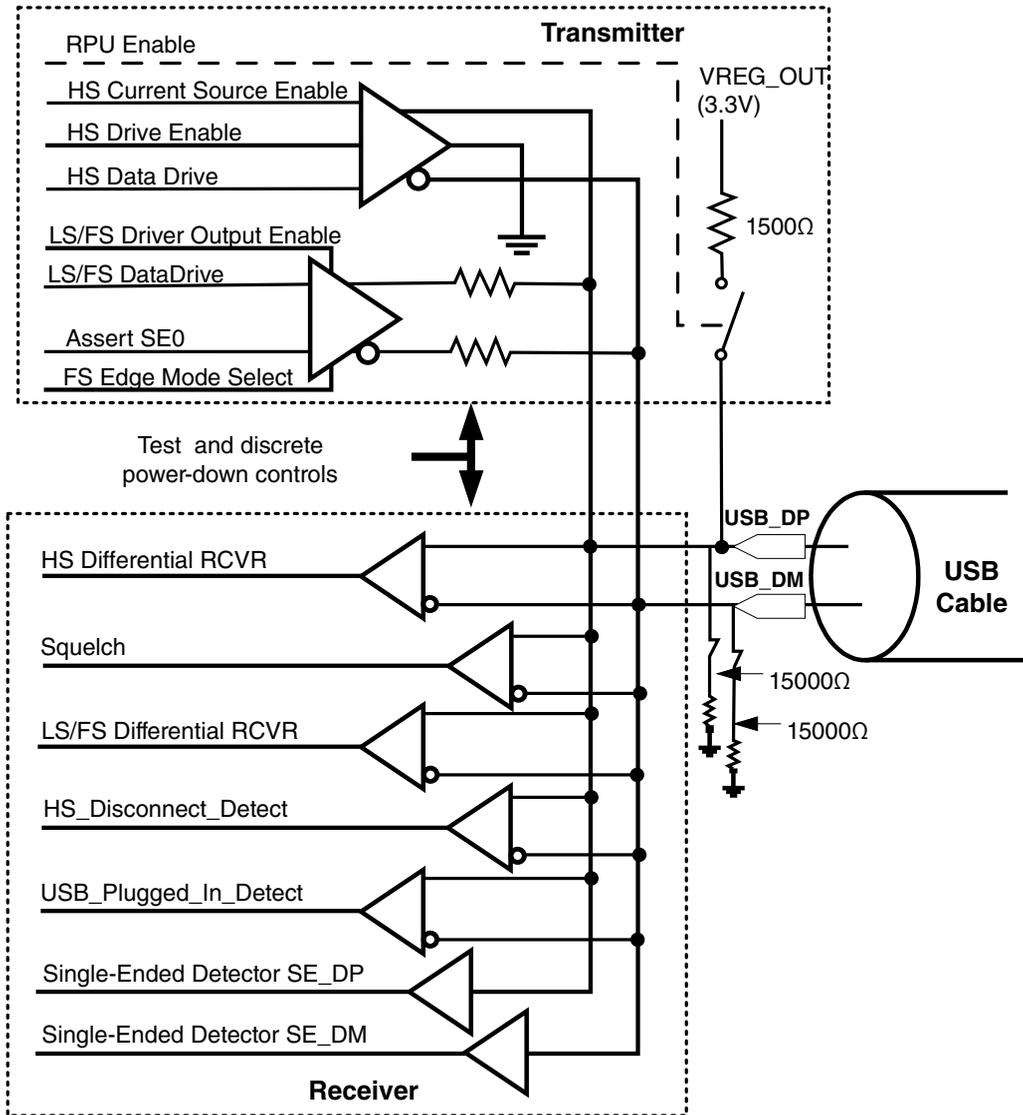
Figure 55-3. USB 2.0 PHY Analog Transceiver Block Diagram
