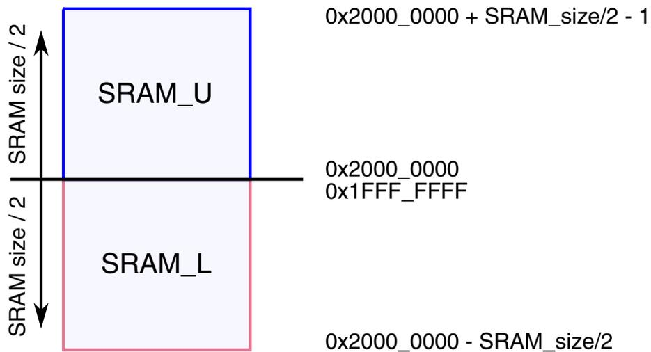
**Figure 28-13. SRAM Arrays**
