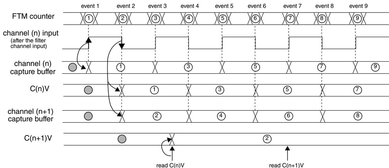
**Figure 45-87. Dual Edge Capture mode read coherency mechanism**
