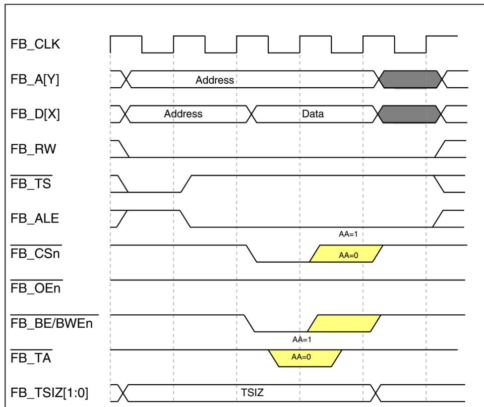
**Figure 33-41. Write-Bus Cycle with Two Clock Address Setup (No Wait States)**
