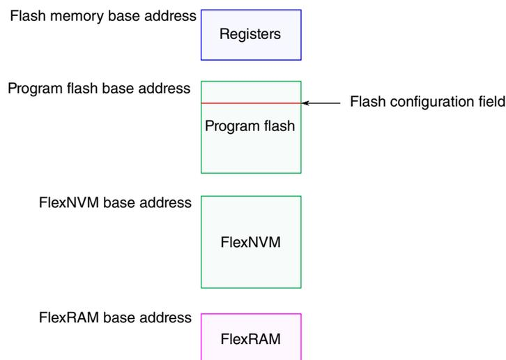
**Figure 5-3. Flash memory map for devices containing FlexNVM**
