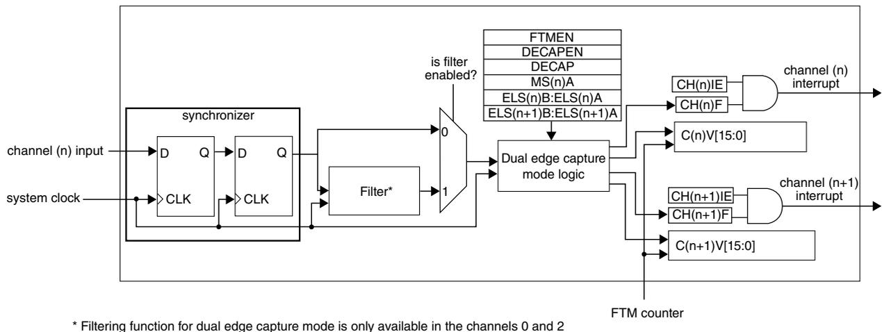
**Figure 45-82. Dual Edge Capture mode block diagram**
