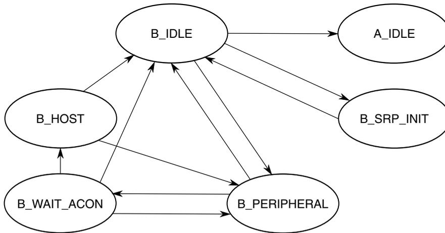
**Figure 51-13. Dual role B device flow diagram**
