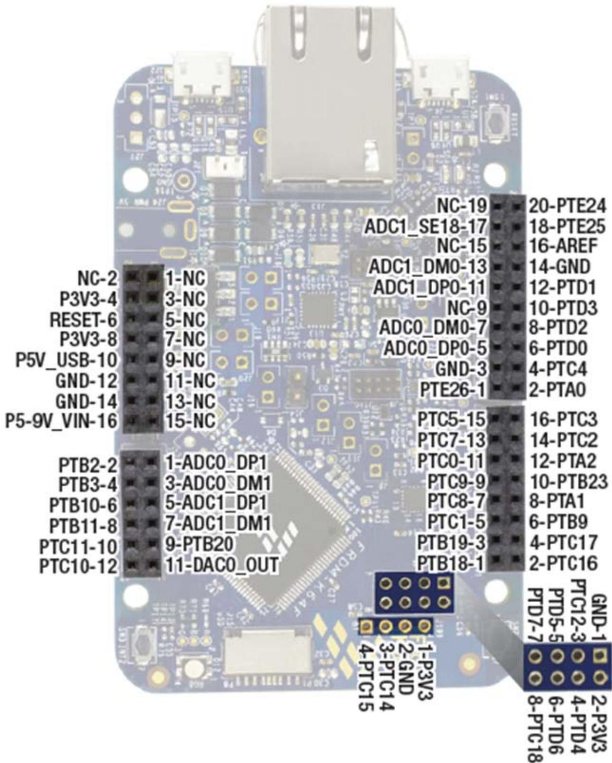
Figure 18. FRDM-K64F pinout
