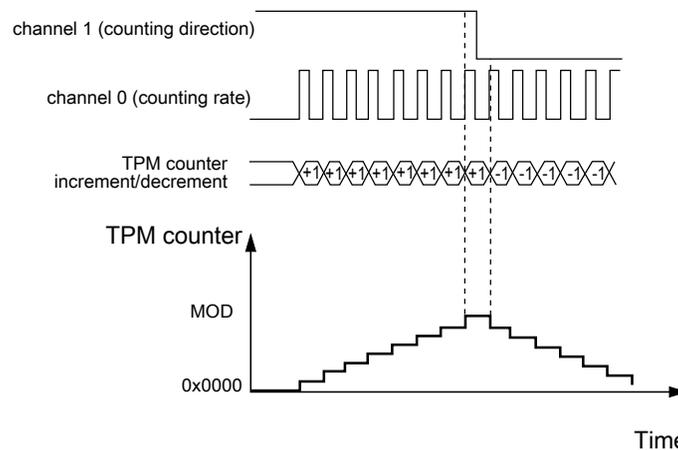
**Figure 43-28. Quadrature Decoder – Count and Direction Encoding mode**
