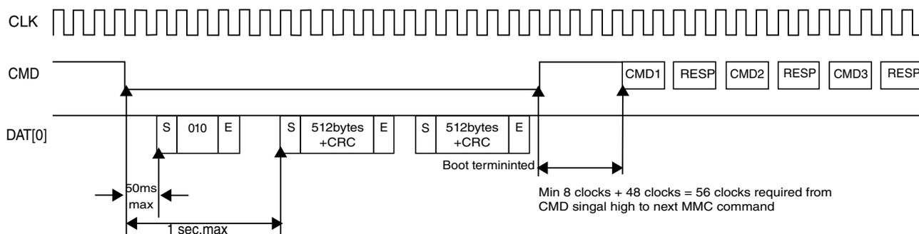
**Figure 60-13. Multimediacard state diagram in Normal Boot mode**
