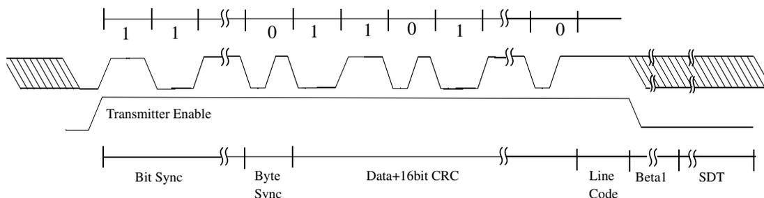
**Figure 55-337. Frame format with differential manchester encoding**
