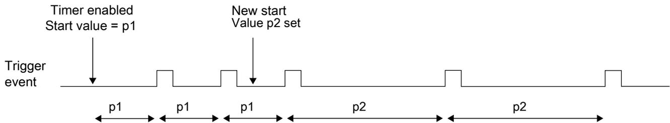
Figure 46-4. Dynamically setting a new load value
