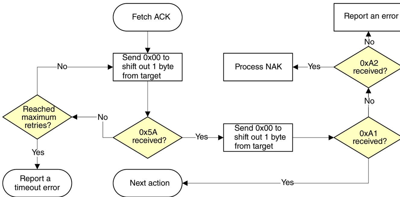
Figure 14-22. Host reads ACK from target via SPI
