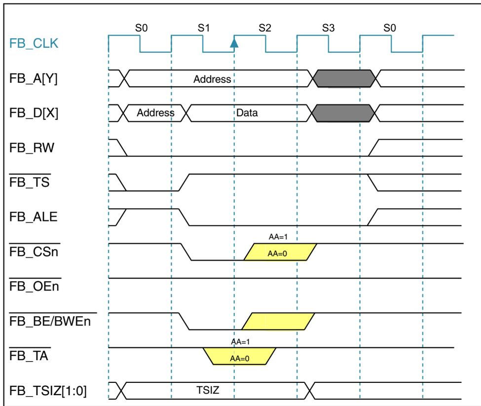
**Figure 34-15. Basic Write-Bus Cycle (No Wait States)**
