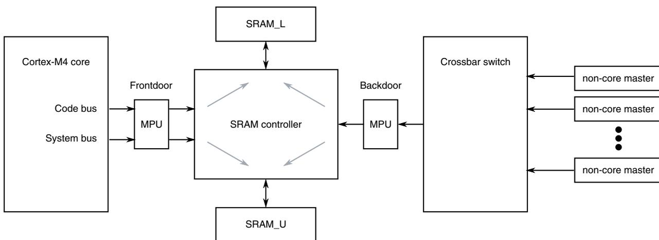
**Figure 3-27. SRAM access diagram**
