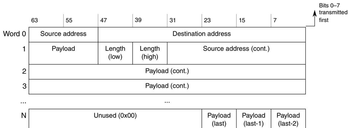
**Figure 50-14. Normal Ethernet frame 64-bit mapping example**
