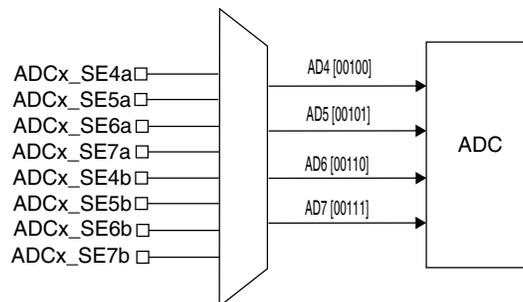
Figure 3-39. ADCx\_SE<sub>n</sub> channels a and b selection
