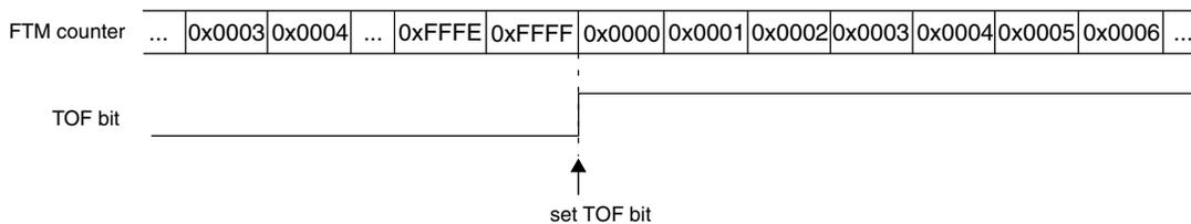
Figure 42-213. Example When the FTM Counter Is a Free Running
