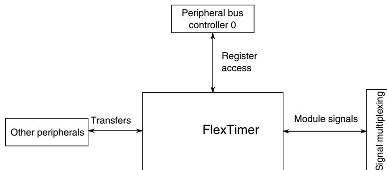
**Figure 3-49. FlexTimer configuration**
