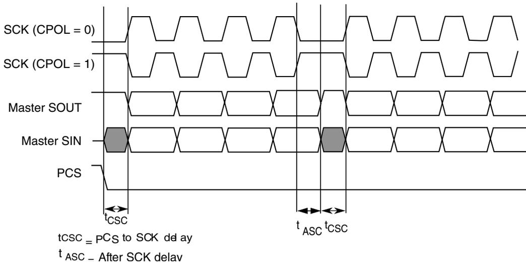
**Figure 57-15. Example of continuous transfer (CPHA=1, CONT=1)**
