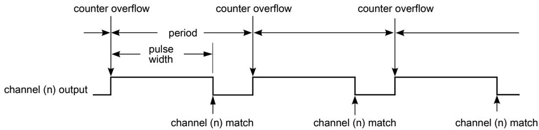
**Figure 43-9. EPWM period and pulse width with  $ELSnB:ELSnA = 1:0$**
