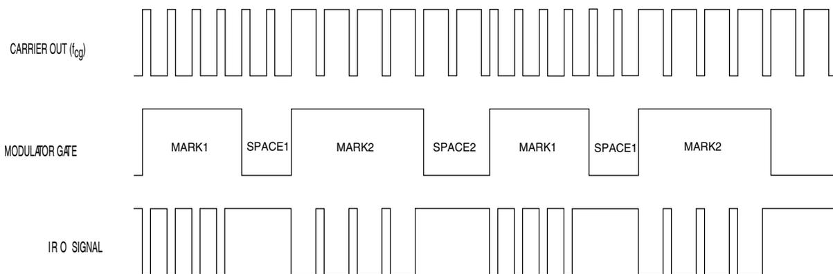
Figure 45-18. Example: CMT Output in FSK Mode
