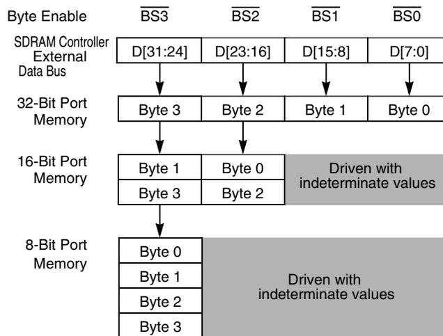
**Figure 35-2. Connections for External Memory Port Sizes**
