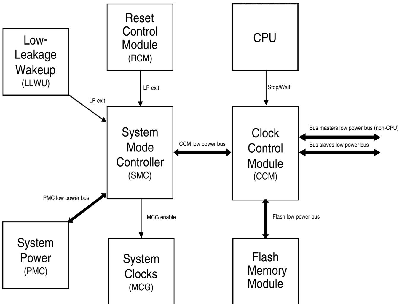
Figure 14-6. Low power system components and connections
