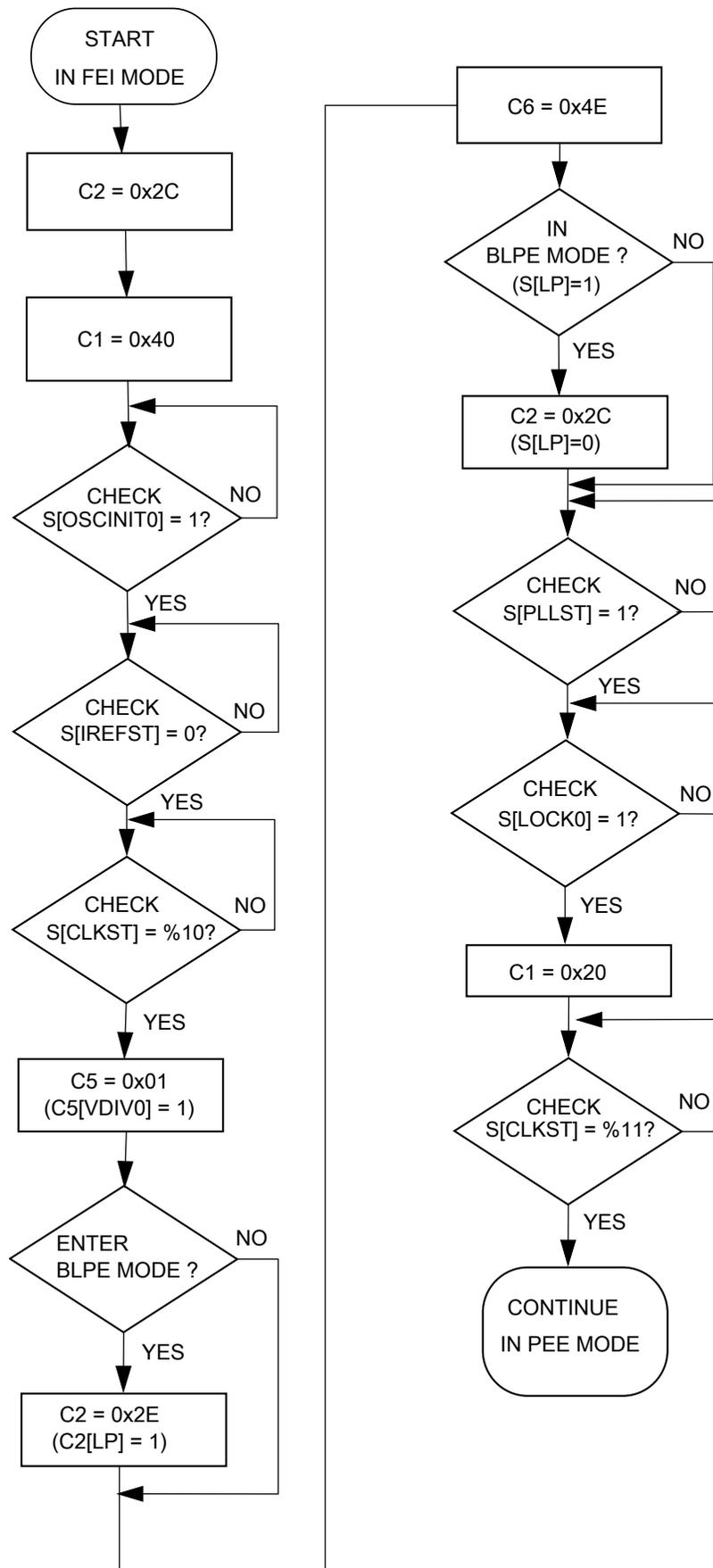
Figure 27-3. Flowchart of FEI to PEE mode transition using an 16 MHz crystal
