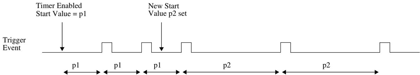
Figure 43-25. Dynamically Setting a New Load Value
