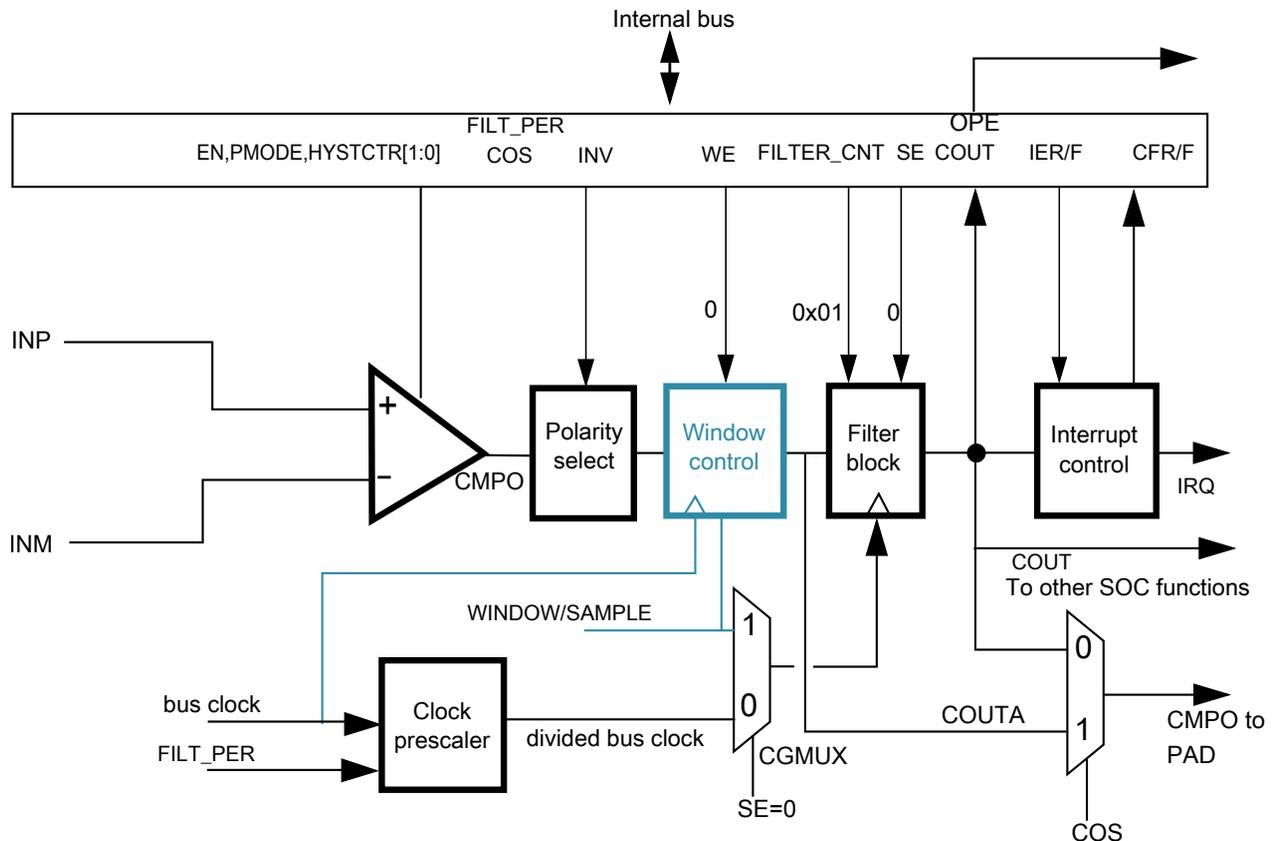
Figure 40-5. Sampled, Non-Filtered (# 3B): sampling interval internally derived
