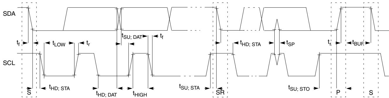
**Figure 26. Timing definition for fast and standard mode devices on the I<sup>2</sup>C bus**
