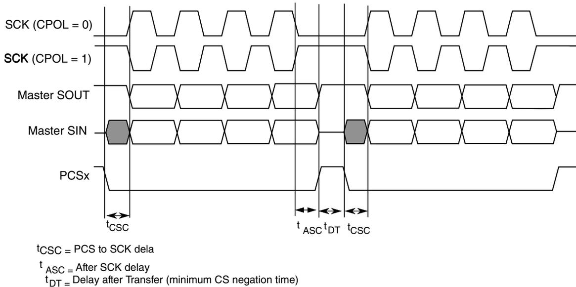
**Figure 57-14. Example of non-continuous format (CPHA=1, CONT=0)**
