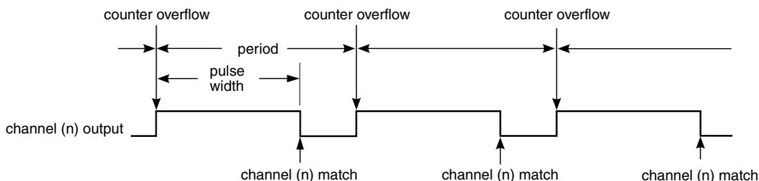
**Figure 45-19. EPWM period and pulse width with ELSnB:ELSnA = 1:0**
