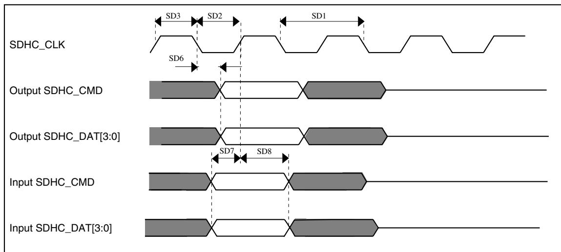
**Figure 27. SDHC timing**
