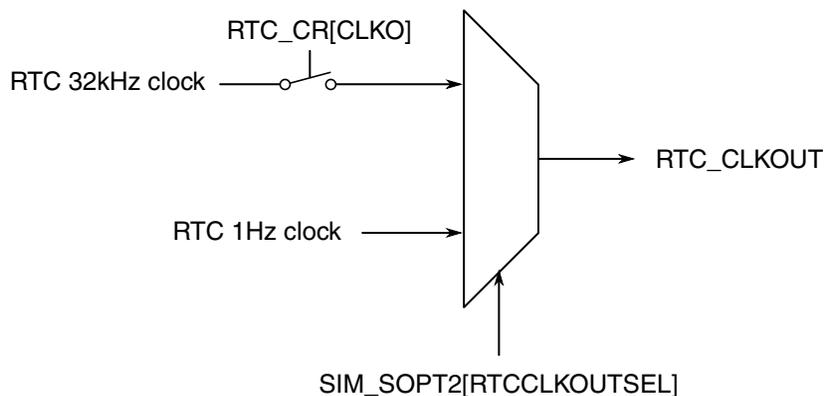
**Figure 49-1. RTC\_CLKOUT generation**
