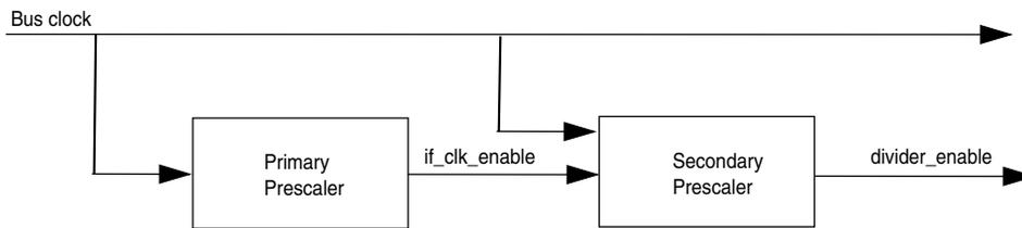
**Figure 45-14. Clock Divider Block Diagram**
