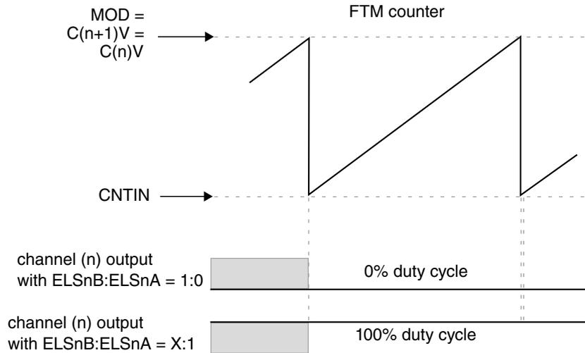
**Figure 45-34. Channel (n) output if  $(C(n)V = C(n+1)V = MOD)$**
