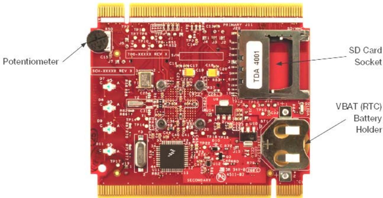
Figure 3. Callouts on back side of the TWR-K60D100M
