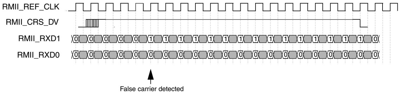
**Figure 50-20. RMII receive operation with false carrier**
