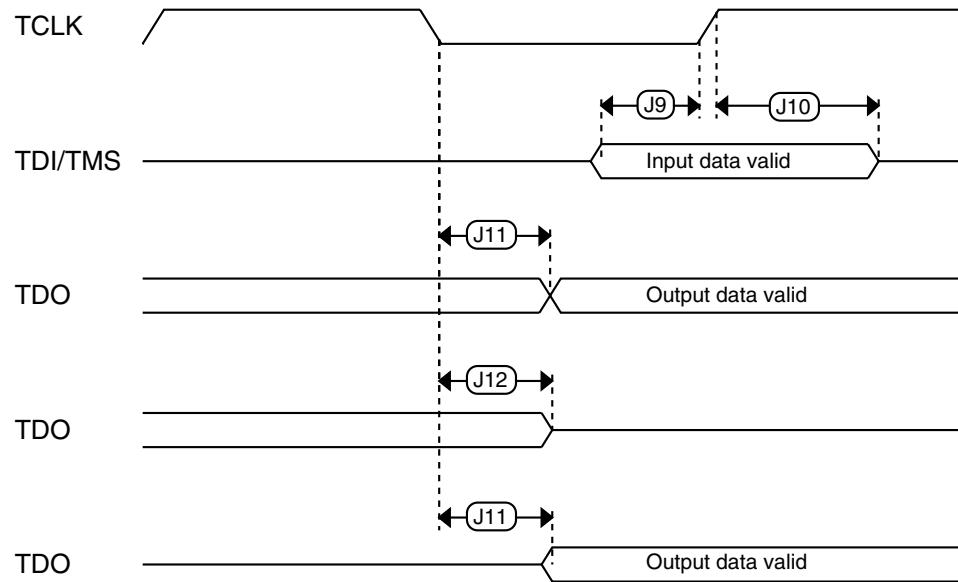
**Figure 7. Test Access Port timing**
