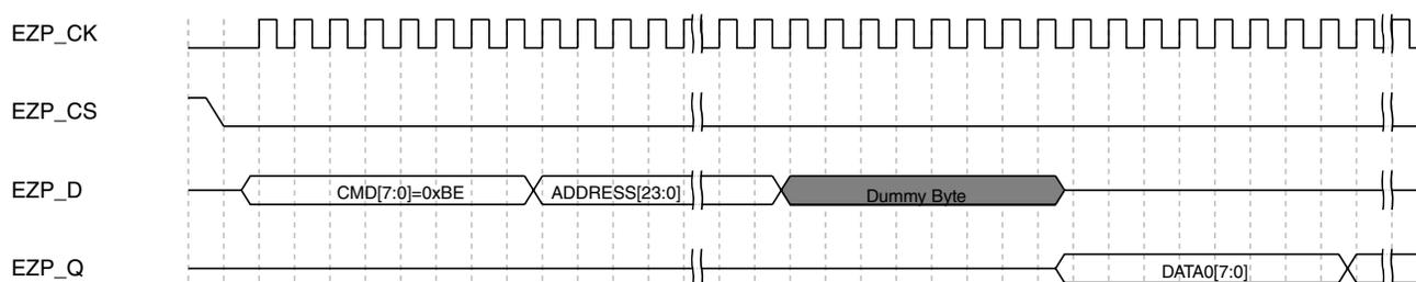
**Figure 33-15. Read FlexRAM at High Speed command sequence**
