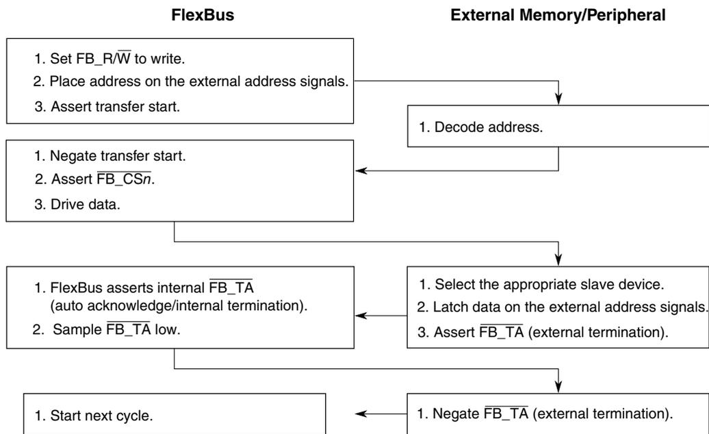
**Figure 33-28. Write-Cycle Flowchart**
