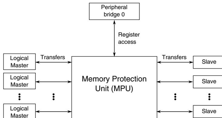
Figure 3-12. Memory Protection Unit configuration
