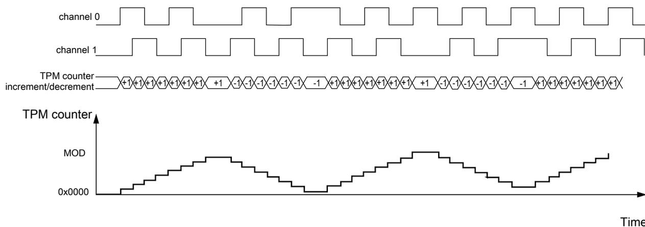
**Figure 43-29. Quadrature Decoder – Phase Encoding mode**
