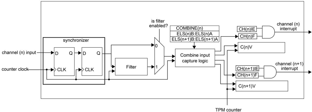
Figure 43-22. Combine Input Capture mode block diagram
