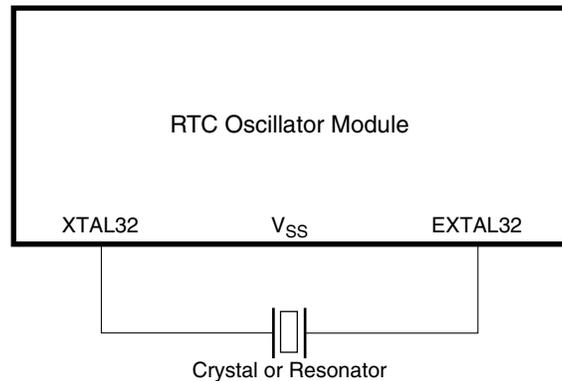
**Figure 27-2. Crystal Connections**
