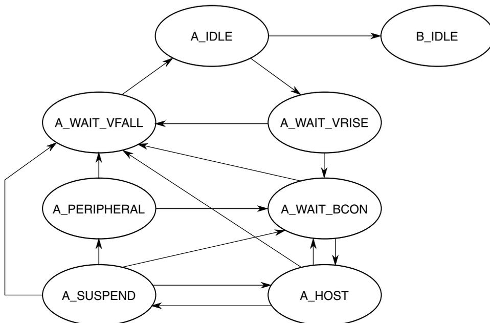
Figure 48-93. Dual Role A Device Flow Diagram
