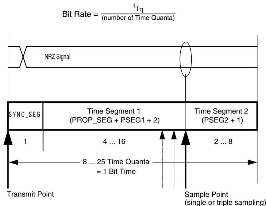
**Figure 52-105. Segments within the Bit Time**
