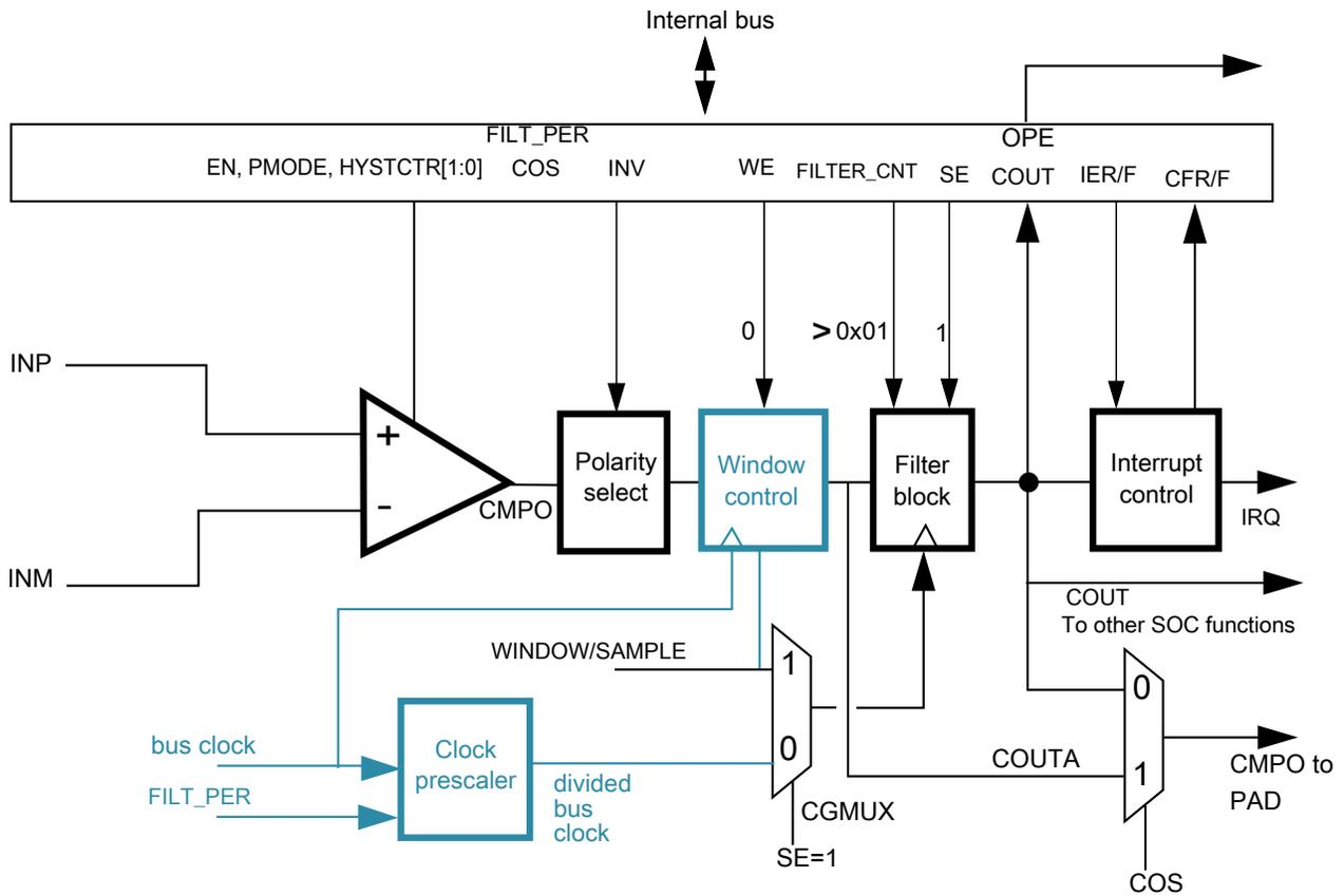
Figure 40-6. Sampled, Filtered (# 4A): sampling point externally driven
