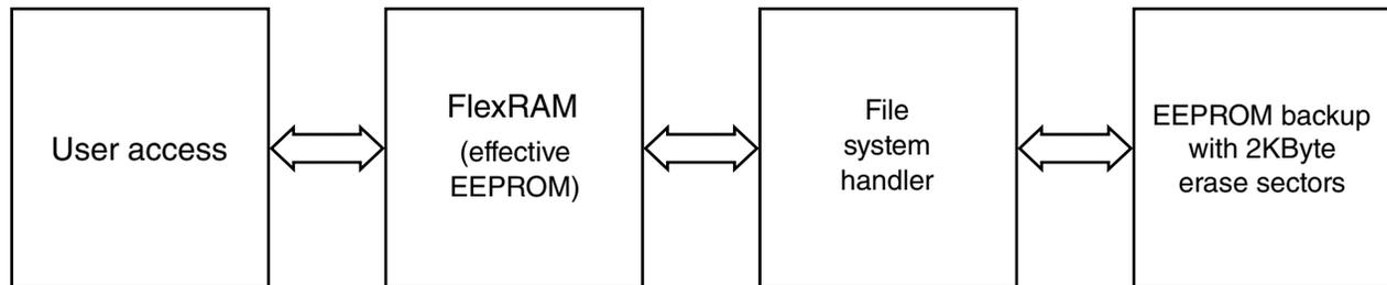
**Figure 32-14. Top Level EEPROM Architecture**
