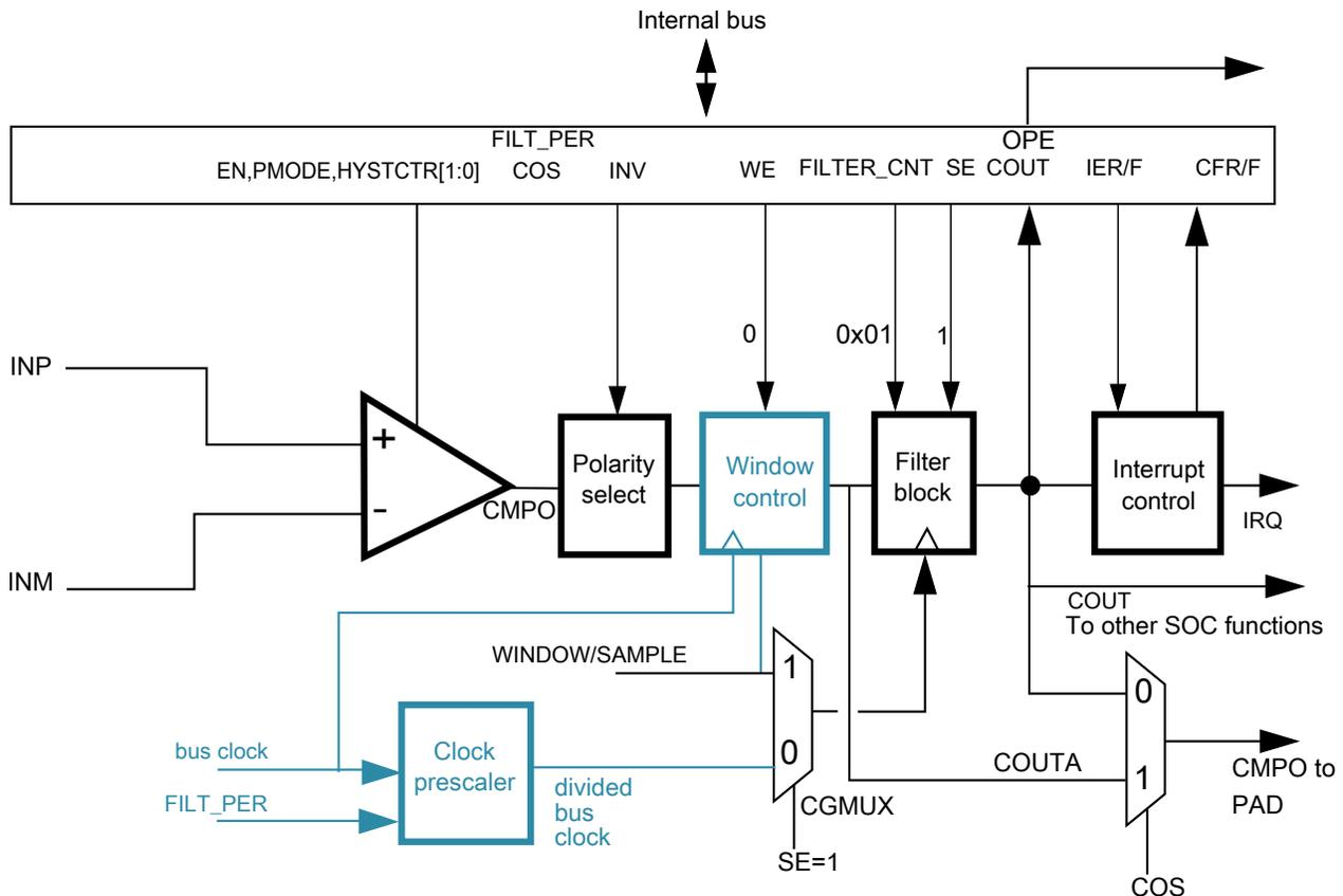
**Figure 40-4. Sampled, Non-Filtered (# 3A): sampling point externally driven**
