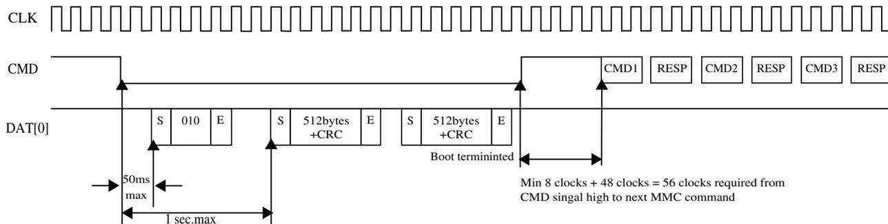
**Figure 56-37. Multimediocard state diagram (normal boot mode)**
