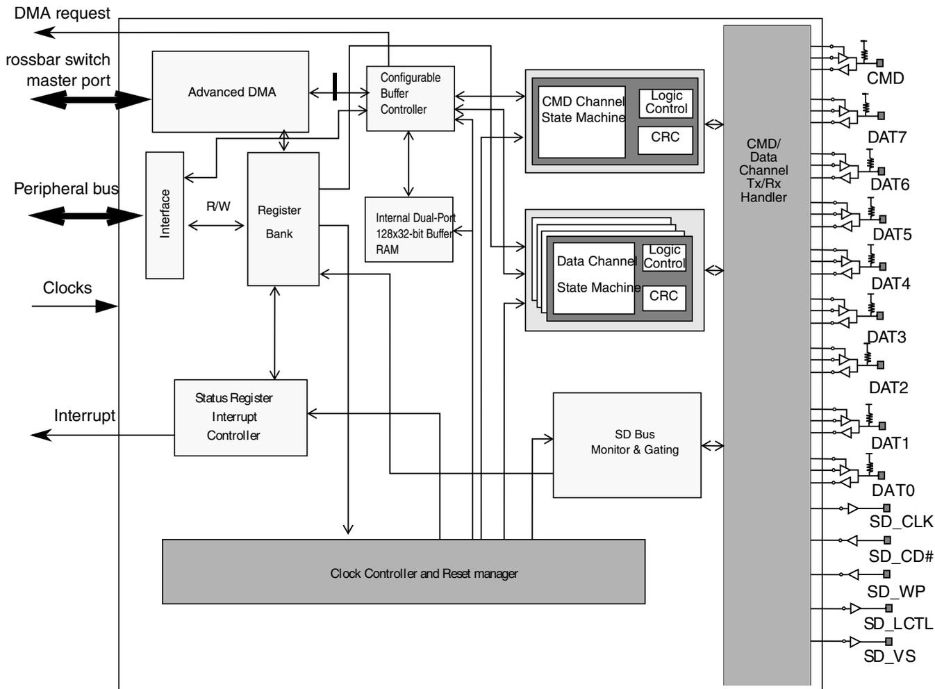
Figure 60-2. Enhanced secure digital host controller block diagram
