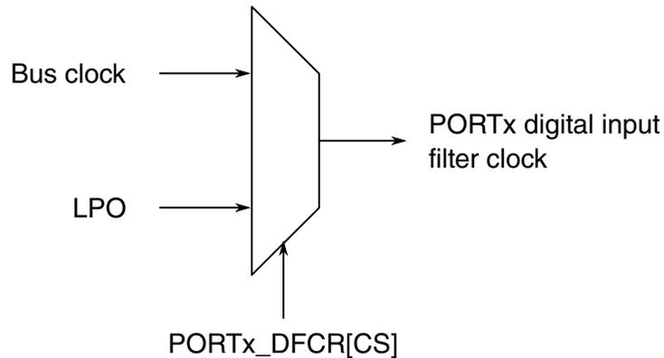
**Figure 6-4. PORTx digital input filter clock generation**
