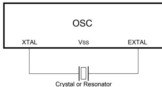
**Figure 28-2. Crystal/Ceramic Resonator Connections - Connection 1**
