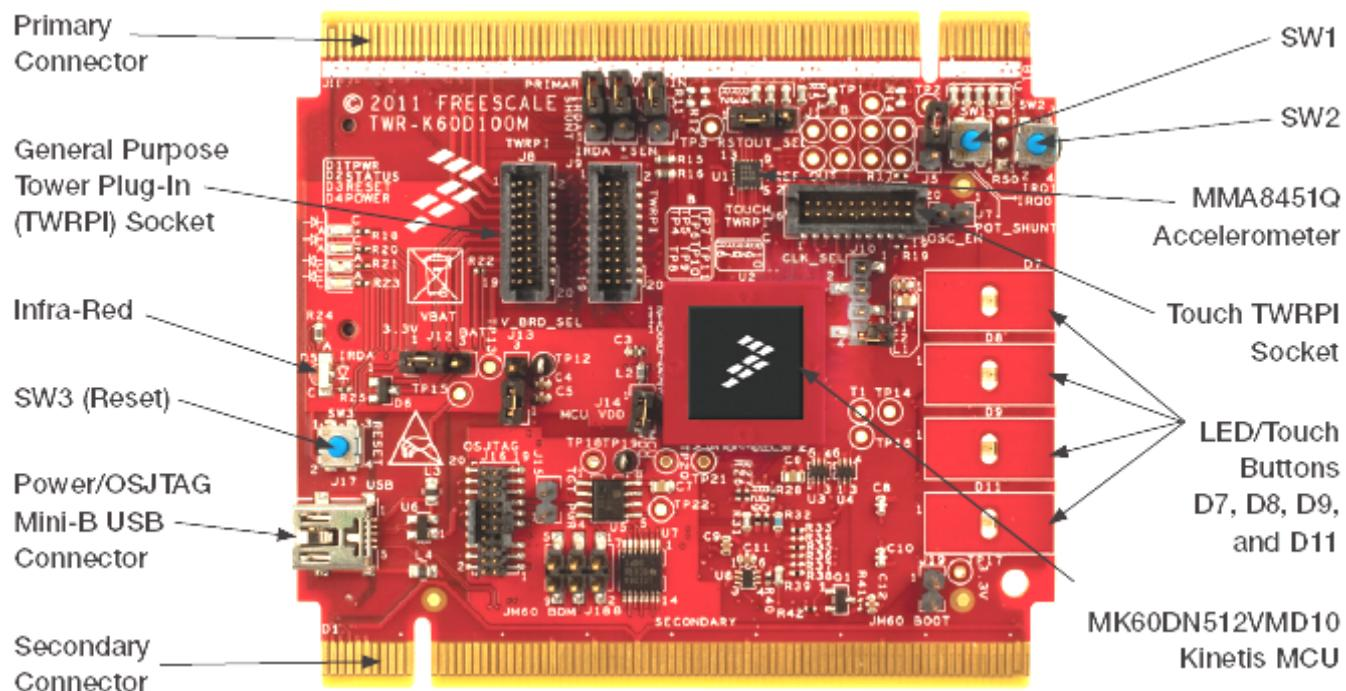
Figure 2. Callouts on front side of the TWR-K60D100M
