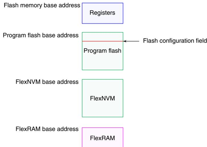
**Figure 4-4. Flash memory map for devices containing FlexNVM**
