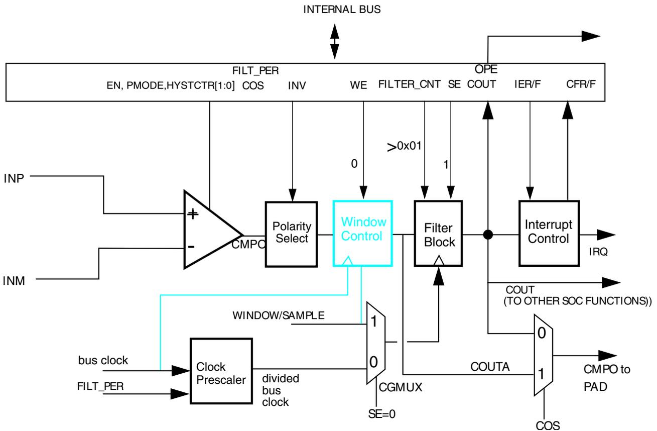
**Figure 38-37. Sampled, Filtered (# 4B): Sampling point internally derived**
