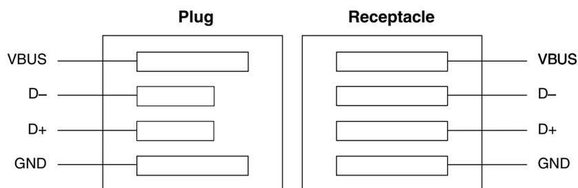
**Figure 52-5. Relative pin positions in USB plugs and receptacles**
