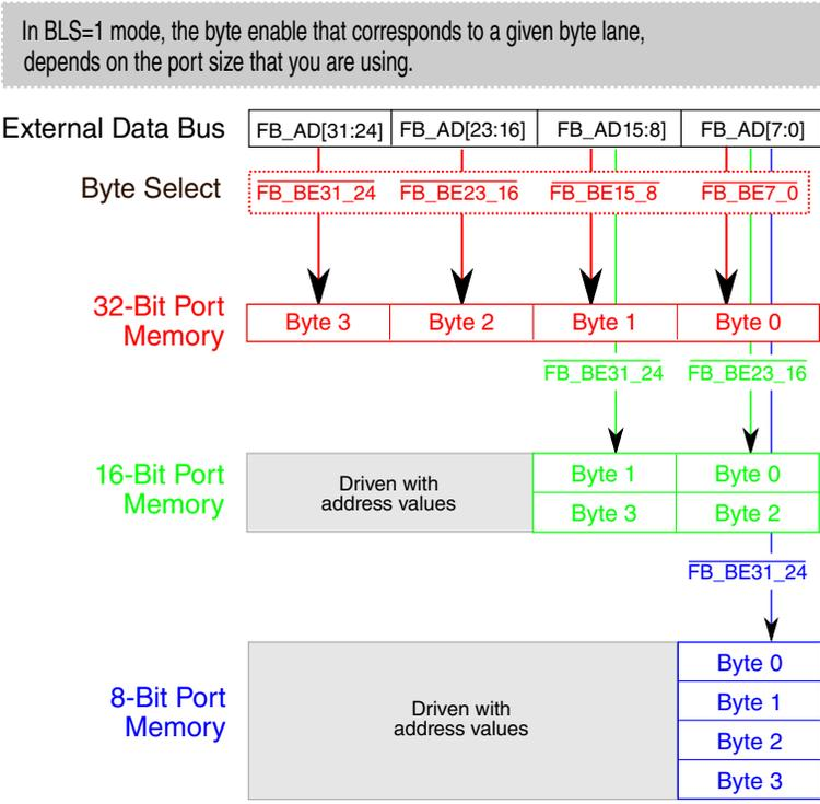
Figure 34-3. Connections for external memory port sizes (CSCRn[BLS] = 1)
