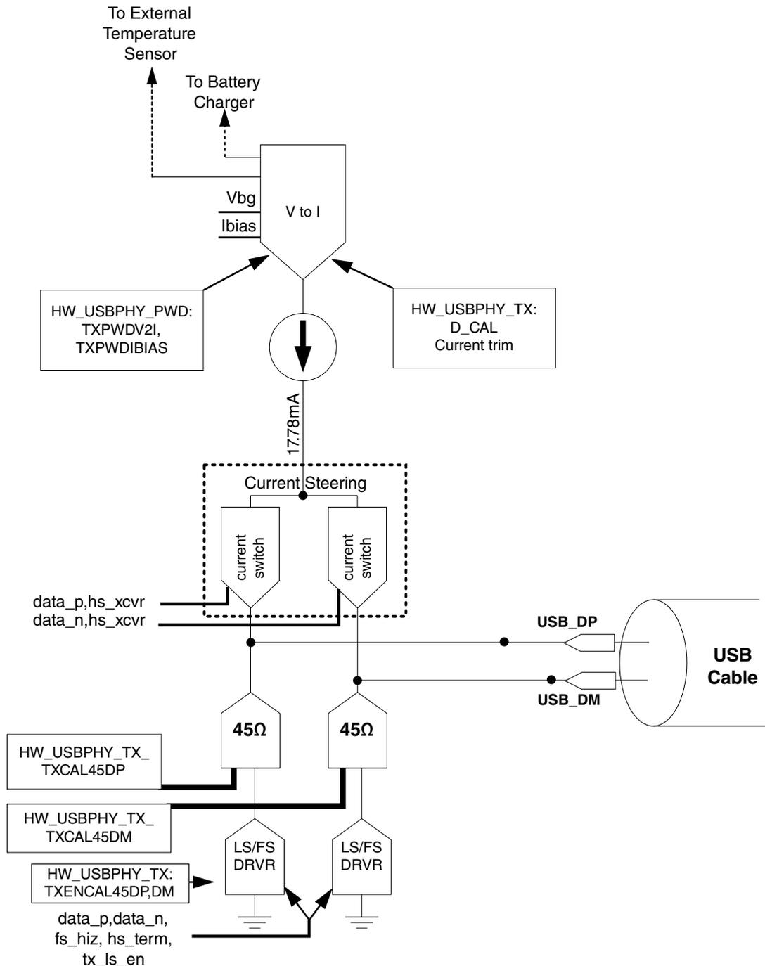
**Figure 55-4. USB 2.0 PHY Transmitter Block Diagram**
