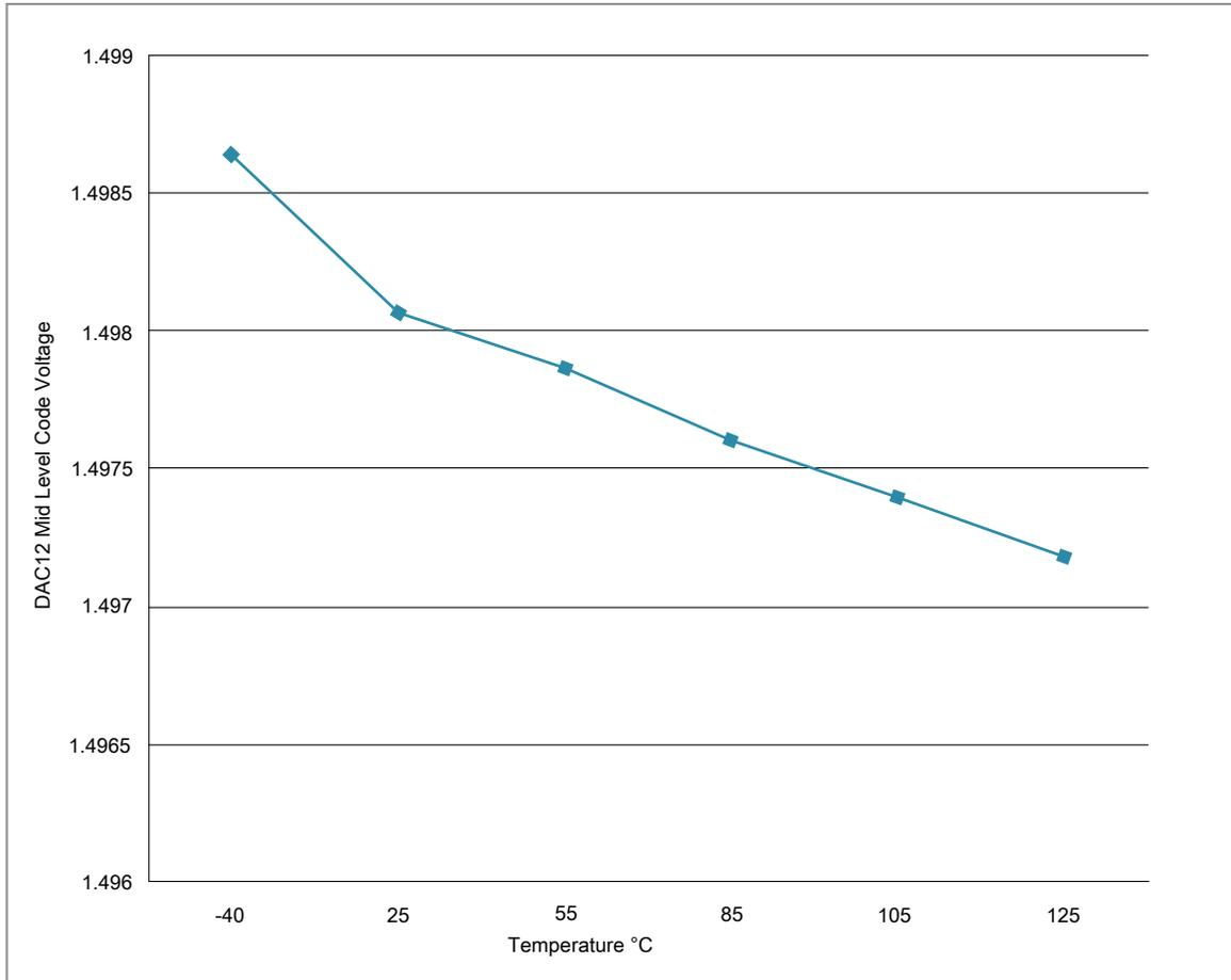
Figure 29. Offset at half scale vs. temperature
