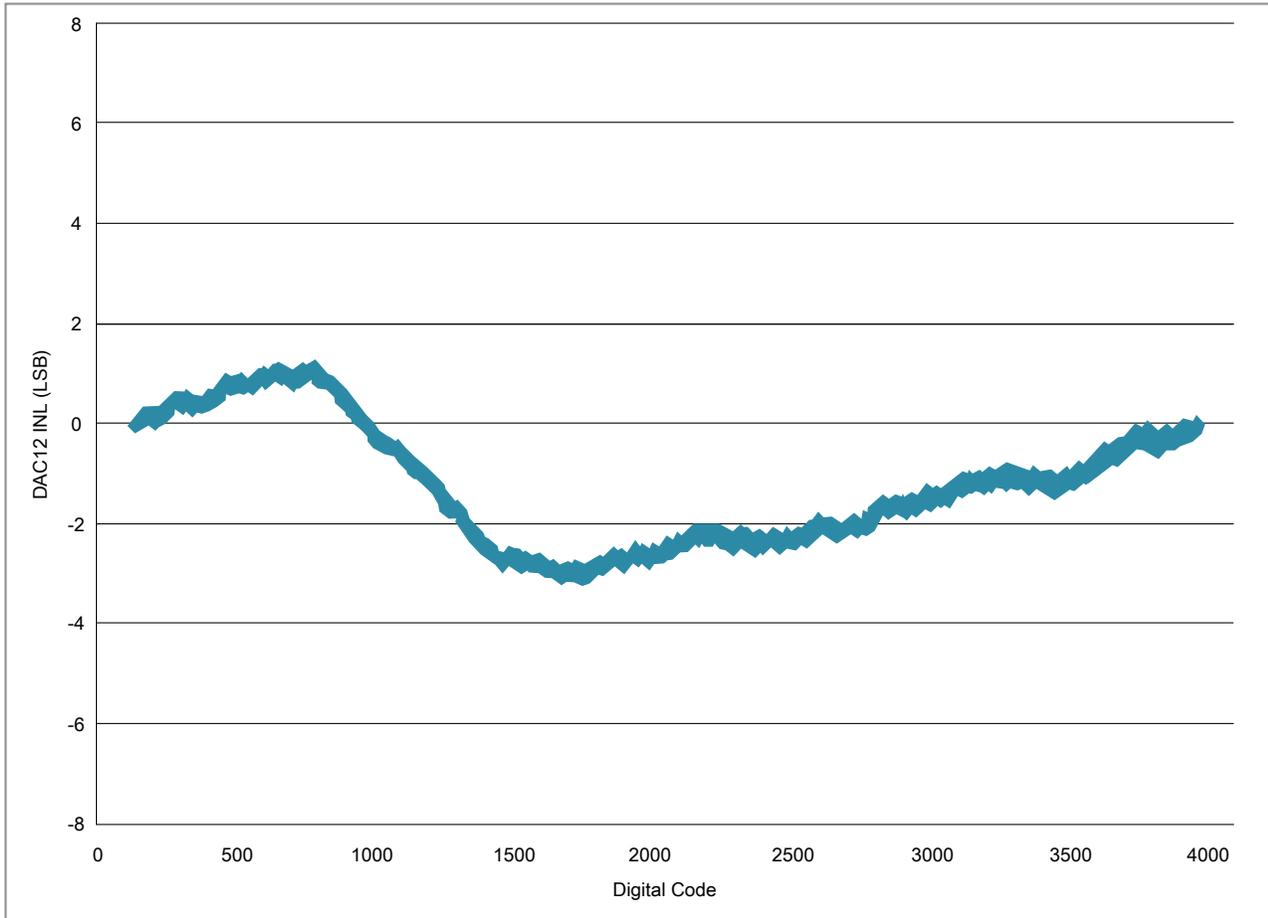
**Figure 28. Typical INL error vs. digital code**
