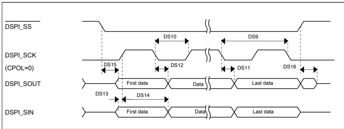
**Figure 37. DSPI classic SPI timing — slave mode**
