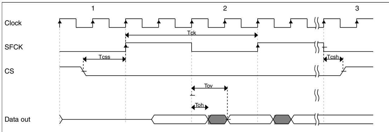
**Figure 17. QuadSPI output timing (DDR mode) diagram**
