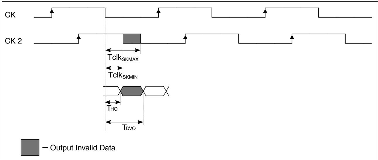
Figure 19. QuadSPI output timing (Hyperflash mode) diagram
