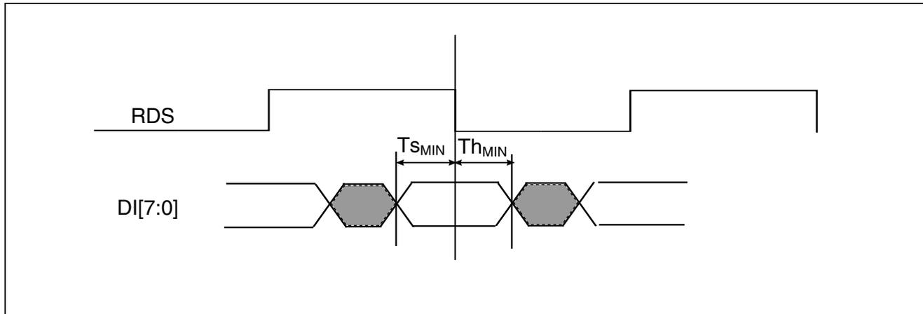
**Figure 18. QuadSPI input timing (Hyperflash mode) diagram**
