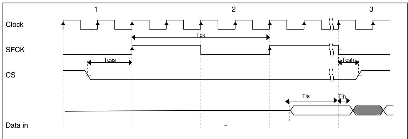
**Figure 14. QuadSPI input timing (SDR mode) diagram**
