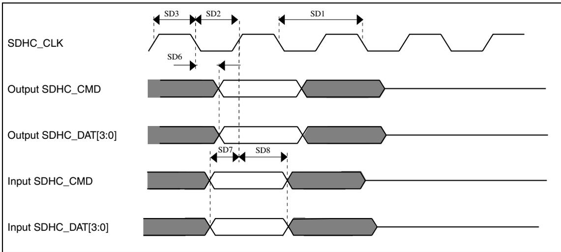
**Figure 38. SDHC timing**
