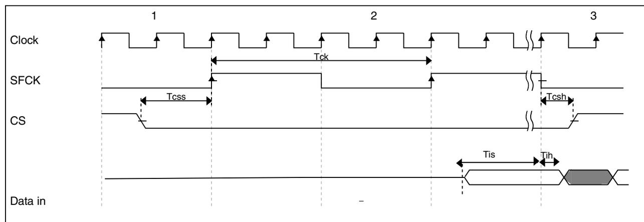
**Figure 14. QuadSPI input timing (SDR mode) diagram**
