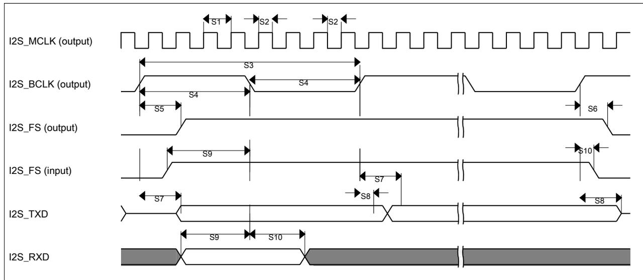
**Figure 39. I<sup>2</sup>S timing — master mode**
