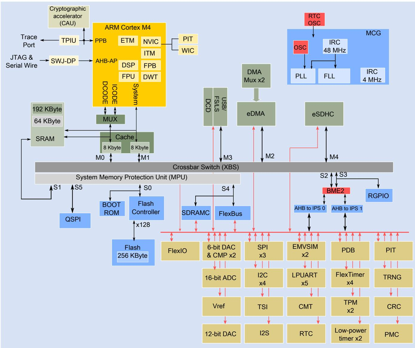
Figure 1. K80 Block Diagram
