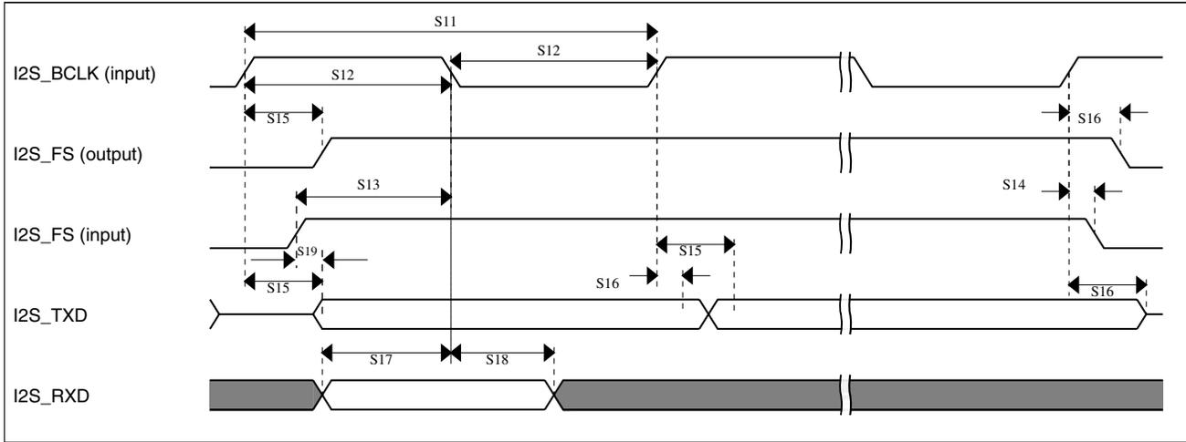
Figure 40. I<sup>2</sup>S timing — slave modes
