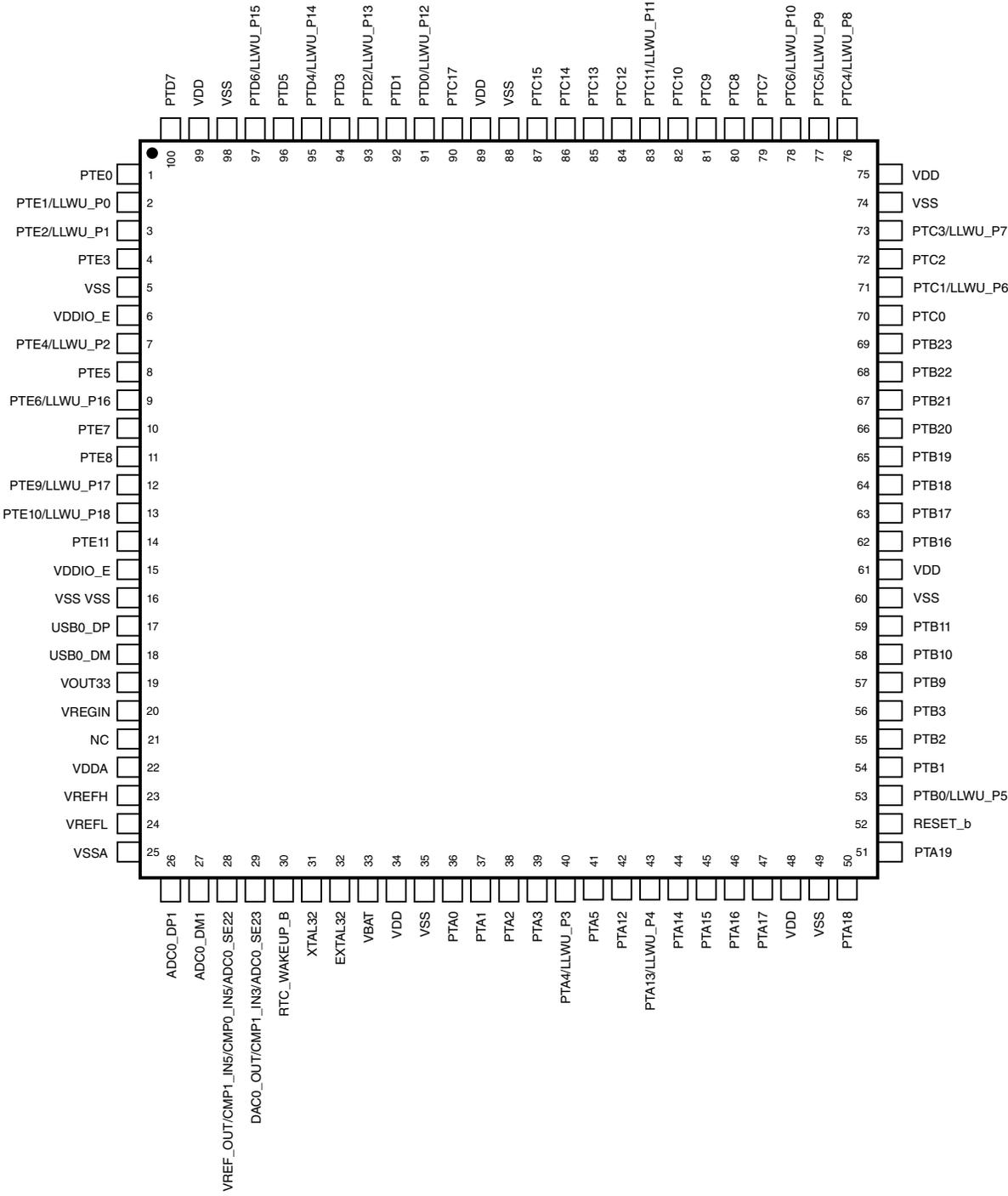
Figure 45. K82 100 LQFP Pinout Diagram
