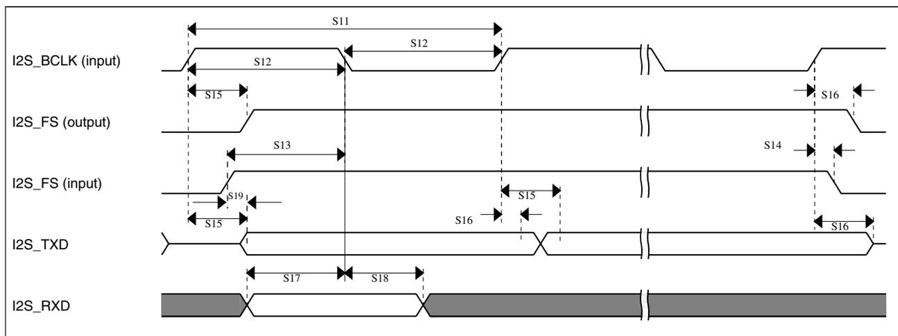
Figure 40. I<sup>2</sup>S timing — slave modes
