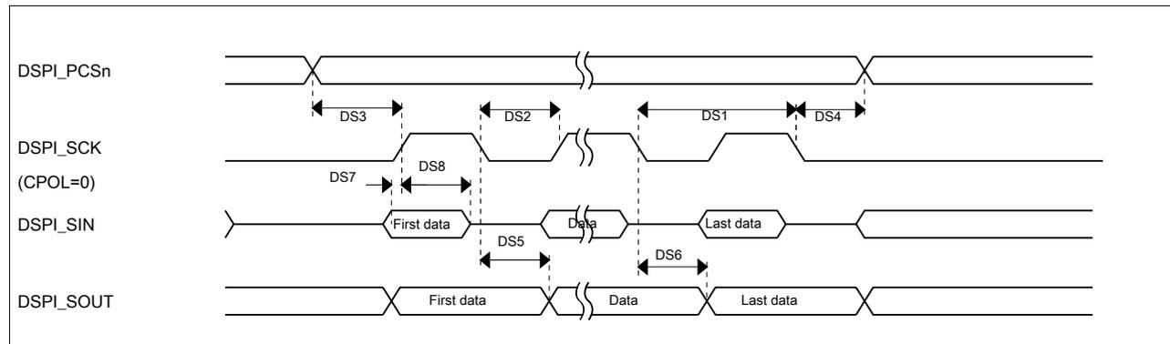
**Figure 36. DSPI classic SPI timing — master mode**
