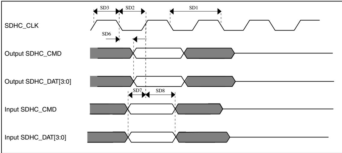
**Figure 38. SDHC timing**
