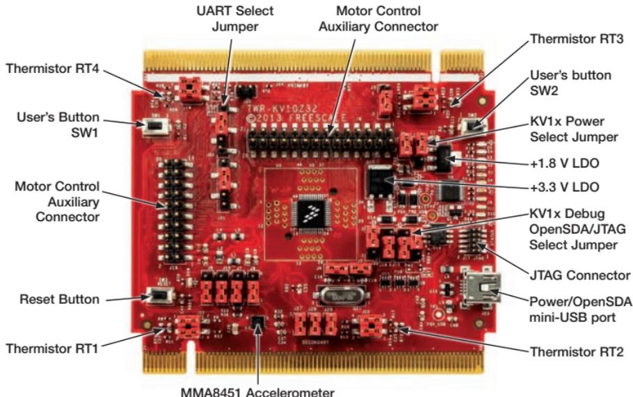
Figure 1: Front side of TWR-KV10Z32
