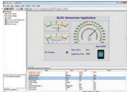
In the Project Options, set the COM port affected as the OpenSDA -CDC Serial Port (info available in Device Manager) and set the baud rate/speed to 9600 bps (check the option Do not Open Port at Startup to avoid error messages at FreeMASTER startup).
