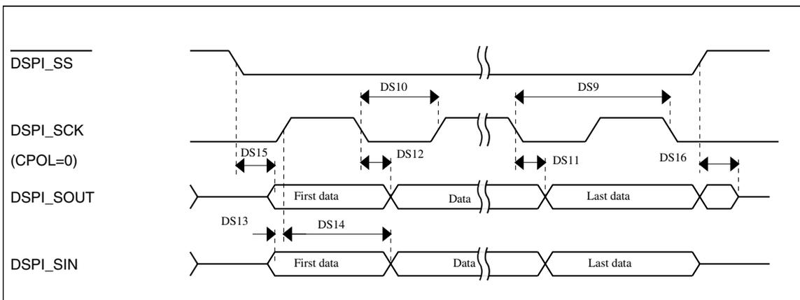
Figure 18. DSPI classic SPI timing — slave mode
