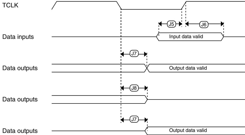
Figure 6. Boundary scan (JTAG) timing
