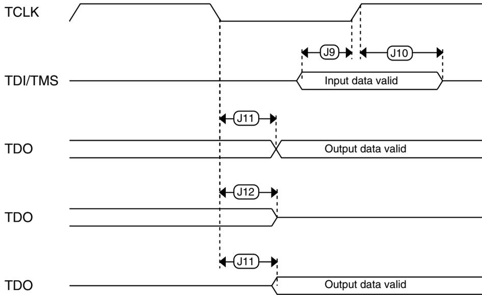
Figure 7. Test Access Port timing
