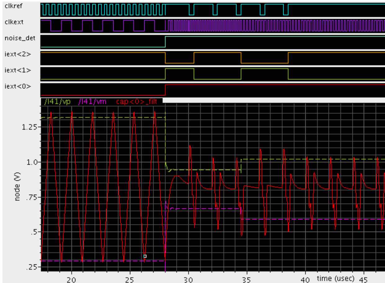
Figure 35-16. TSI noise detection mode waveform
