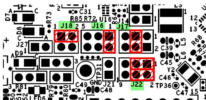
**Figure 10. Bypass headers**
