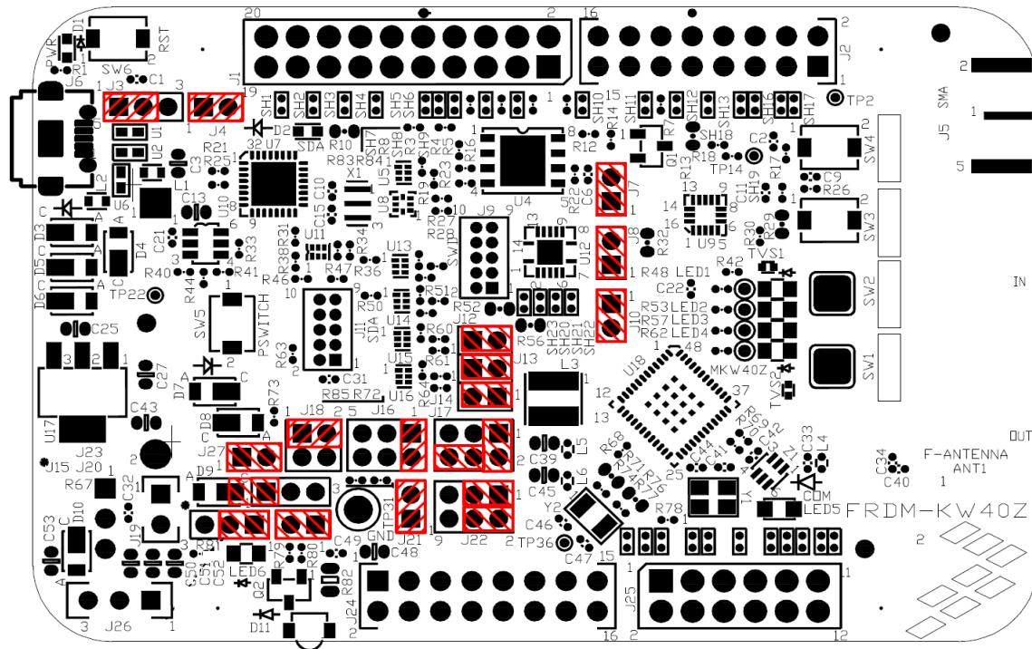
Figure 3. FRDM-KW40Z board with IO headers locations
