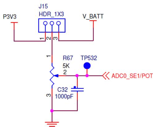
Figure 17. Potentiometer circuit
