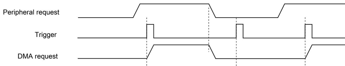
**Figure 18-4. DMAMUX channel triggering: ignored trigger**
