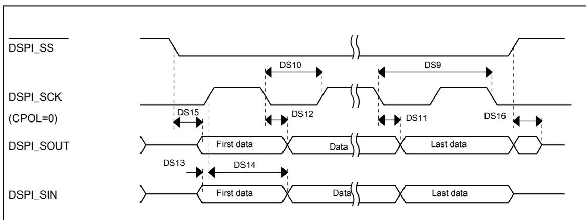
**Figure 13. DSPI classic SPI timing — slave mode**
