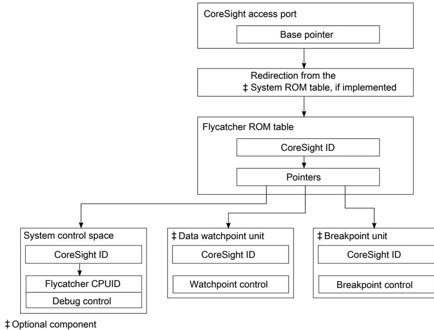
**Figure 15-3. CoreSight discovery process**
