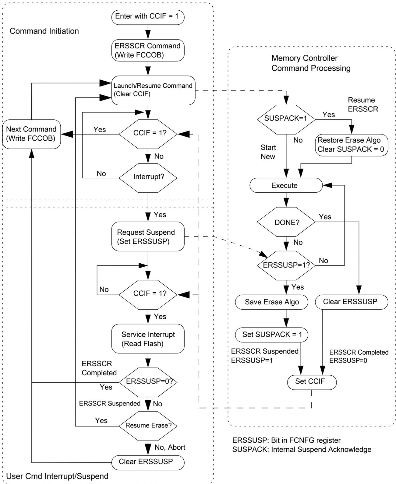
Figure 23-4. Suspend and Resume of Erase Flash Sector Operation
