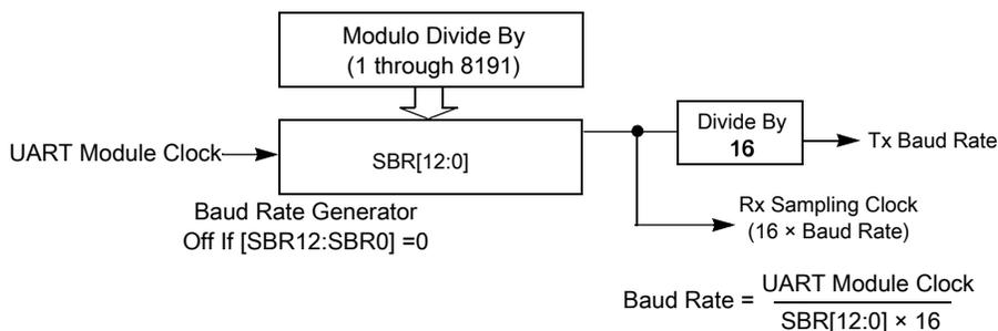
Figure 33-3. UART baud rate generation
