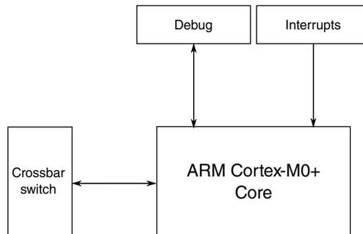
Figure 1-1. Core configuration
