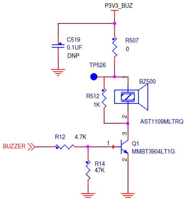
Figure 16. Buzzer circuit
