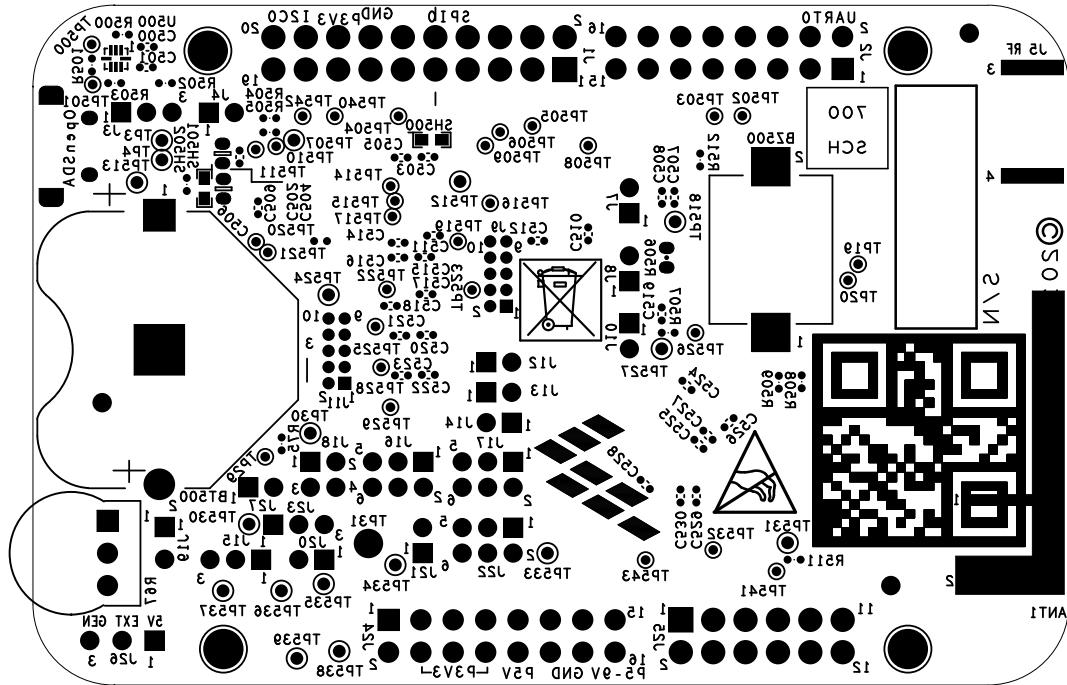
Figure 23. FRDM-KW40Z development board test points
