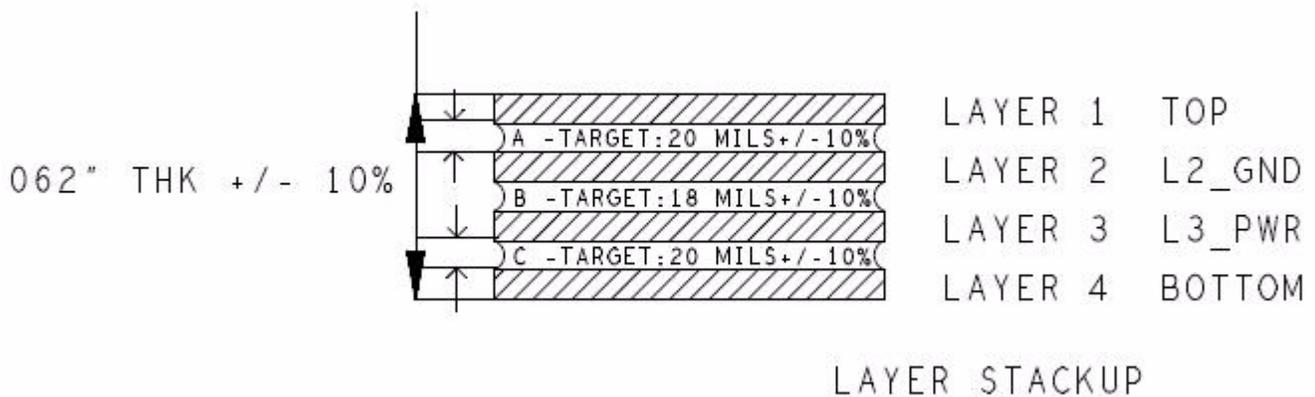
**Figure 4-1. TWR-KW2x PCB Stackup Cross-Section (Four Layer)**
