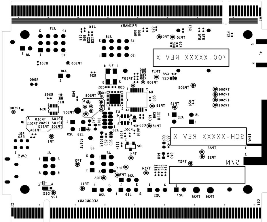
Figure 3-11. TWR-KW24D512 Reference Board PCB Test Points
