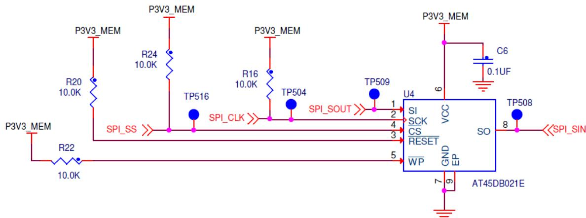
Figure 14. AT45DB021E 2-Mbit (256 Kbyte) serial flash memory circuit
