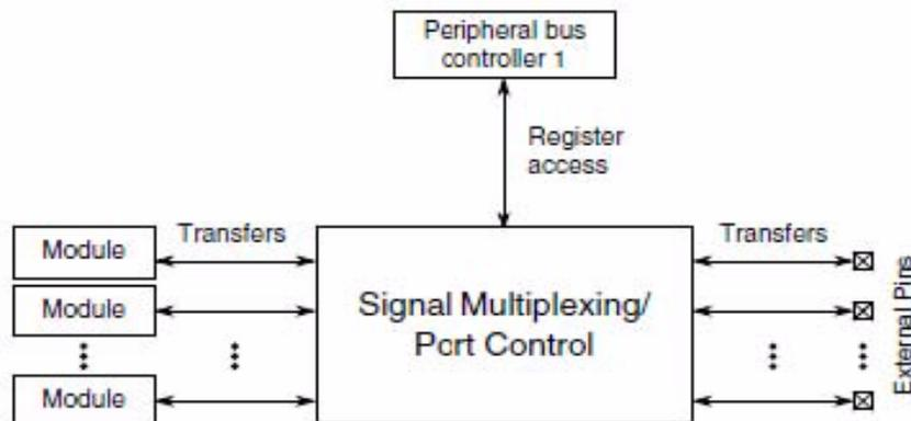
Figure 3-1. Signal Multiplexing Integration
