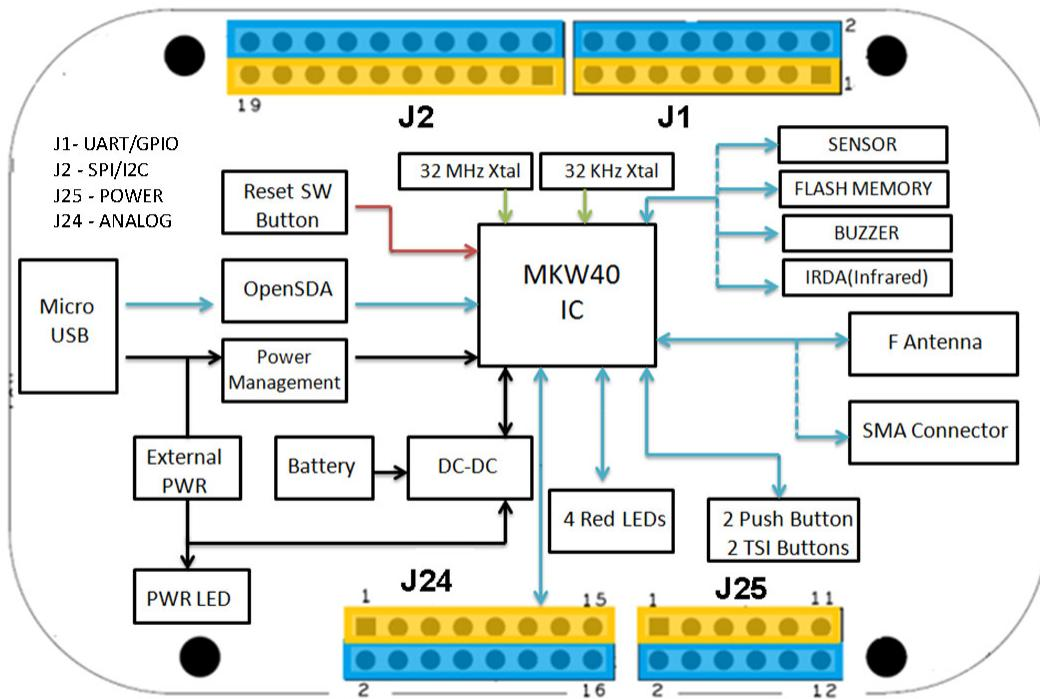
**Figure 5. FRDM-KW40Z board functional block diagram**
