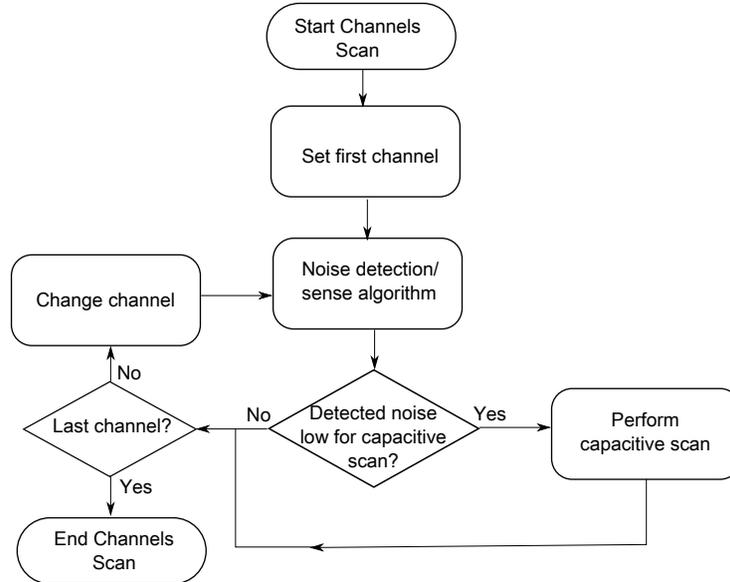
**Figure 35-8. Detection of touch with noise sense and normal capacitive sense flow chart**
