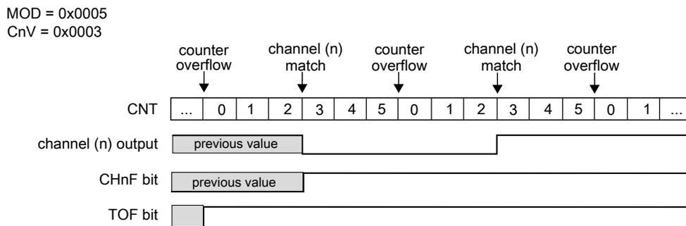
**Figure 27-6. Example of the output compare mode when the match toggles the channel output**
