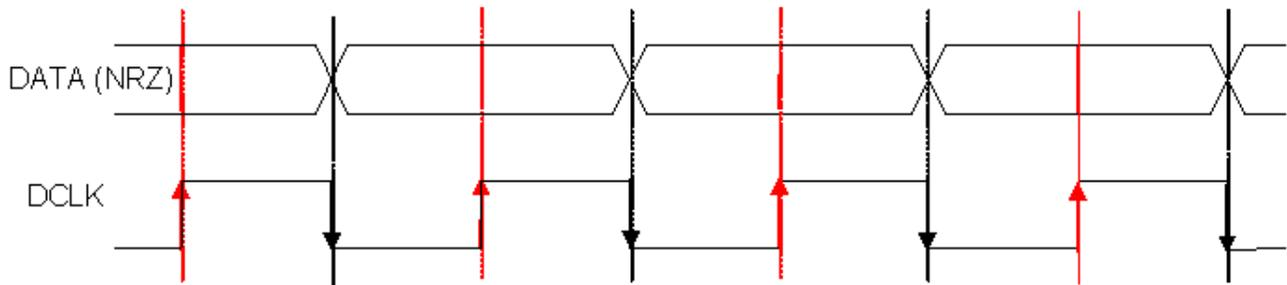
Figure 7-8. RX Processing in Continuous Mode
