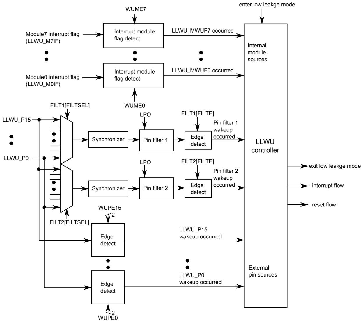
Figure 11-1. LLWU block diagram
