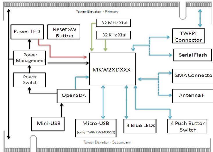
Figure 2-2. Simplified KW24D512-TWR Block Diagram
