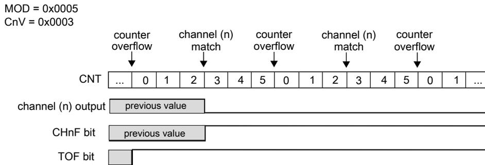
**Figure 27-7. Example of the output compare mode when the match clears the channel output**
