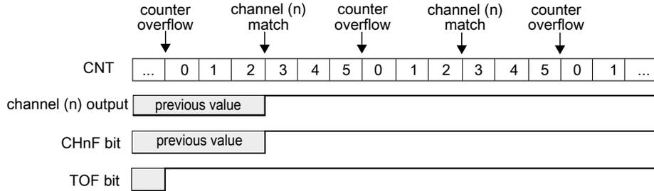
**Figure 27-8. Example of the output compare mode when the match sets the channel output**
