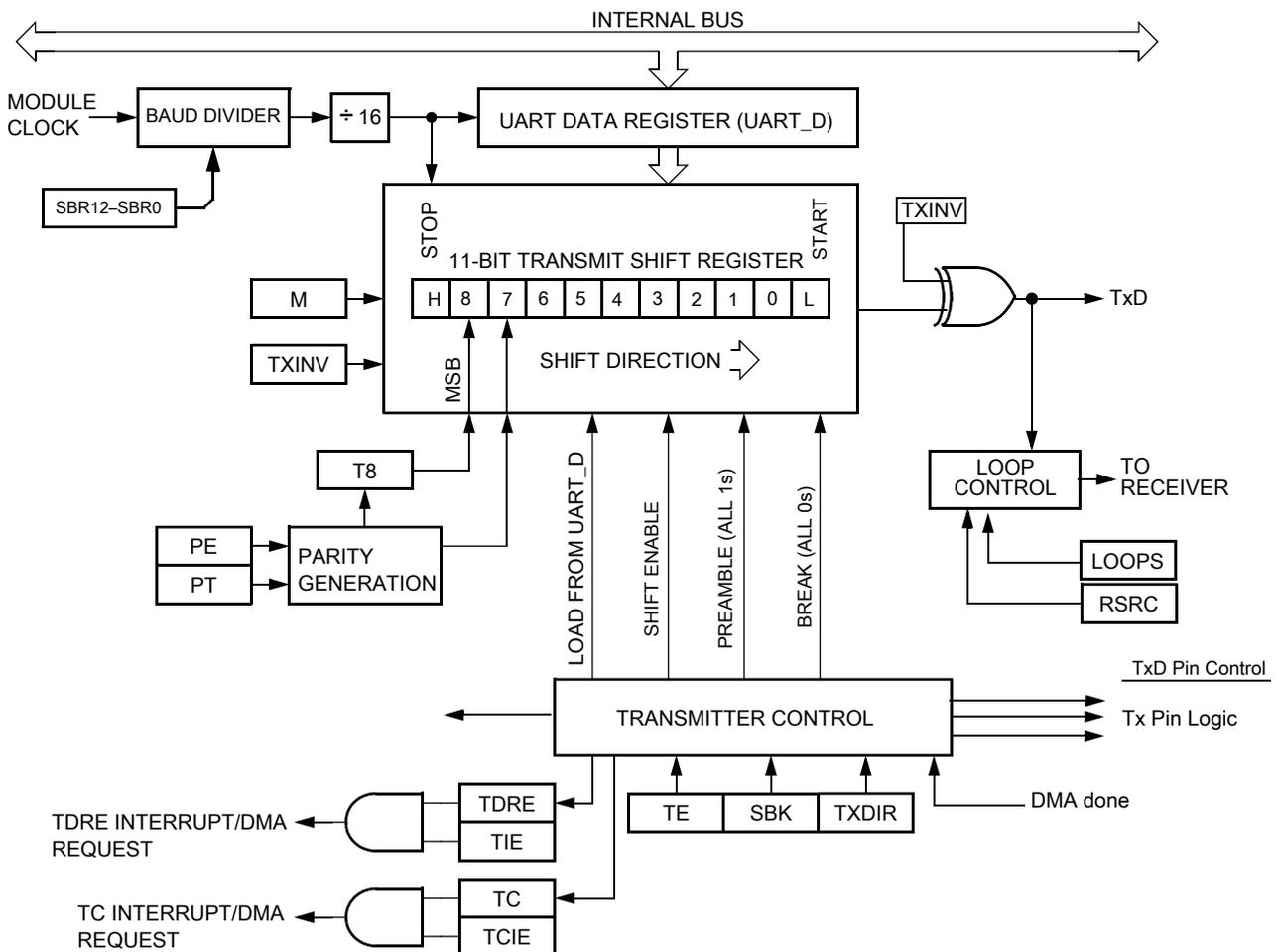
**Figure 33-1. UART transmitter block diagram**
