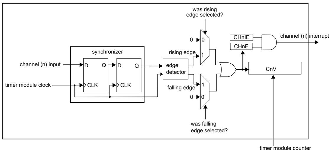
Figure 27-5. Input capture mode
