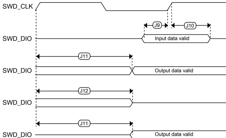
**Figure 6. Serial wire data timing**
