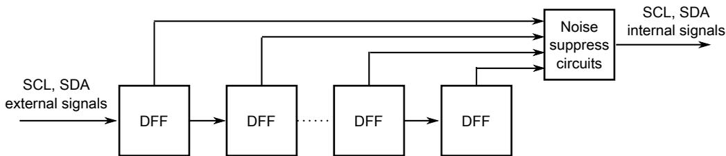
Figure 36-5. Programmable input glitch filter diagram
