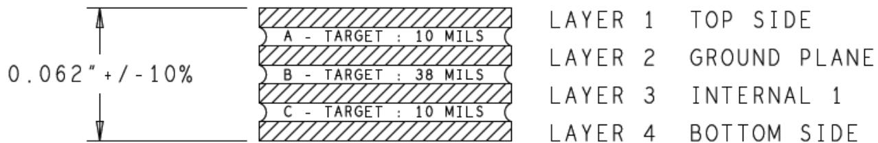
**Figure 26. FRDM-KW40Z PCB layer stackup cross-section (four layer)**
