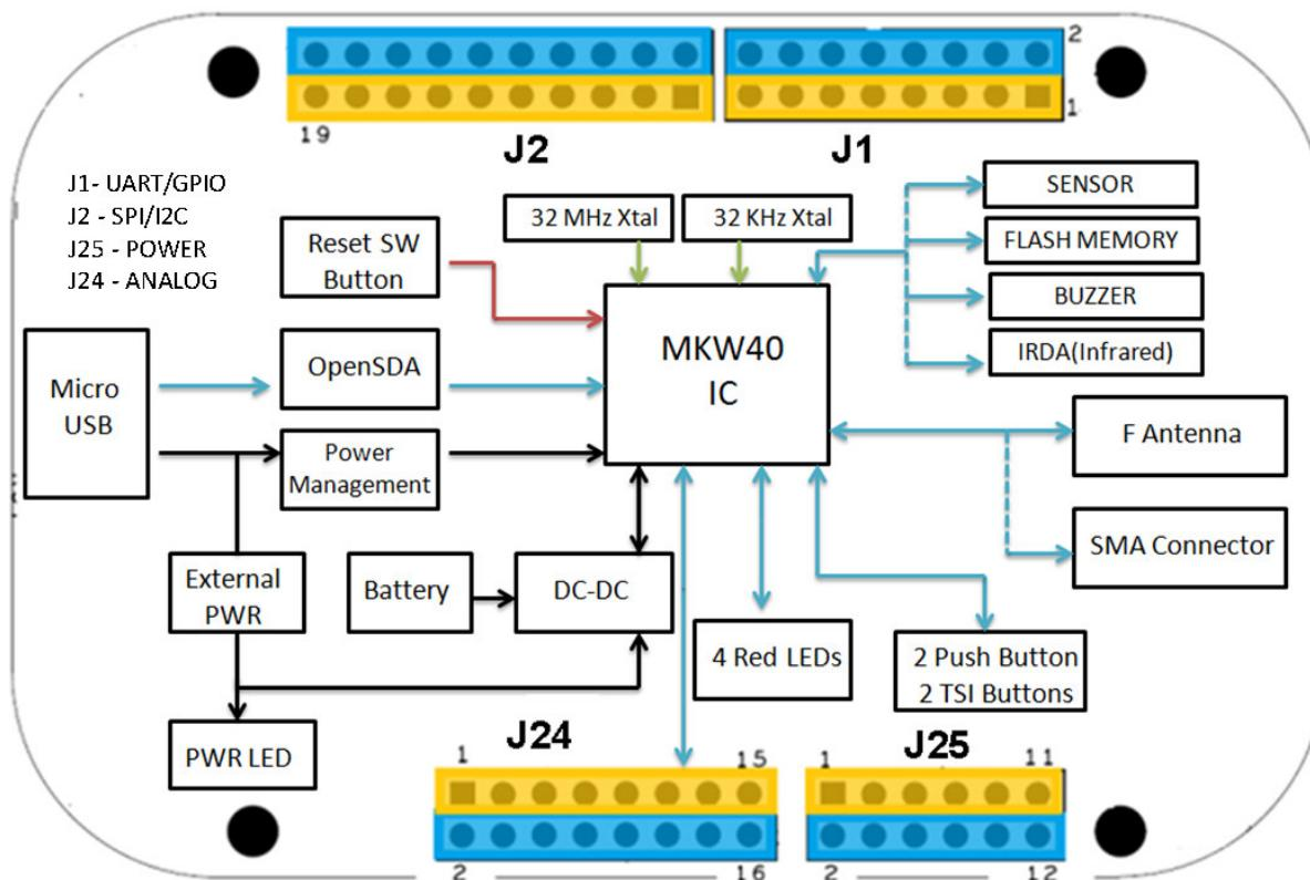
Figure 2. FRDM-KW40Z simplified block diagram
