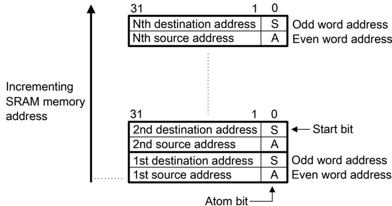
**Figure 15-2. MTB execution trace storage format**
