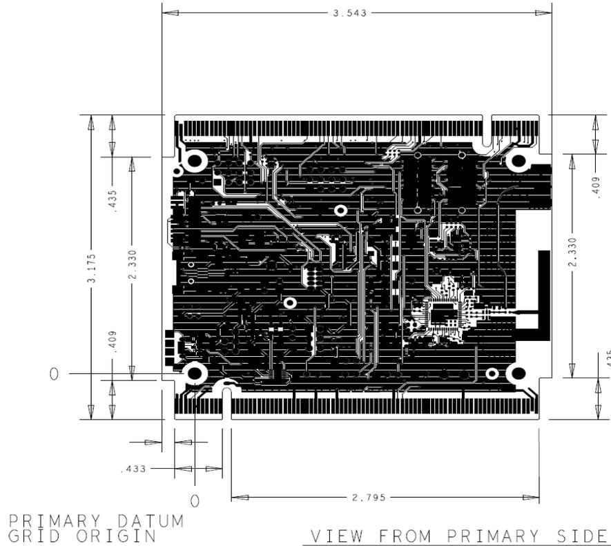
Figure 3-2. TWR-KW2x Top Side (Component Side) Footprint
