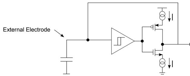
**Figure 35-2. TSI electrode oscillator circuit**
