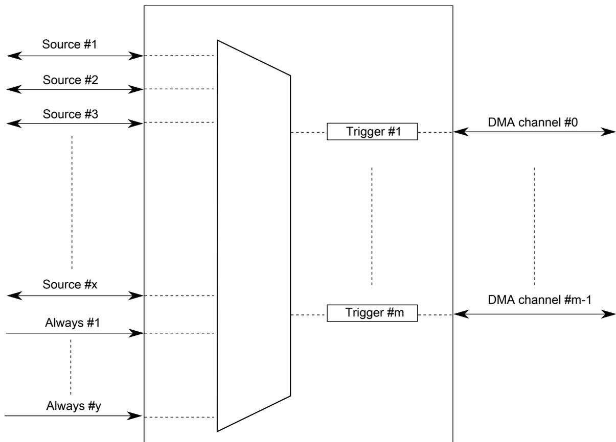
**Figure 18-2. DMAMUX triggered channels**
