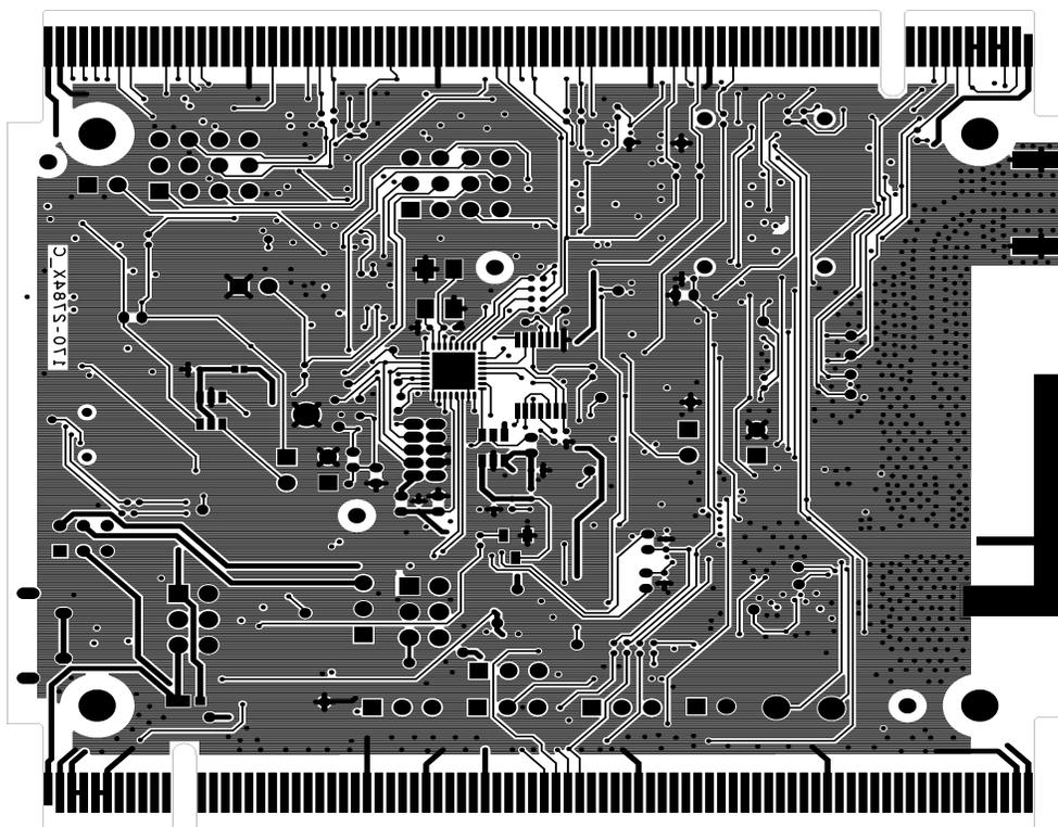
Figure 3-13. TWR-KW24D512 Reference Board PCB Layout (Bottom View)
