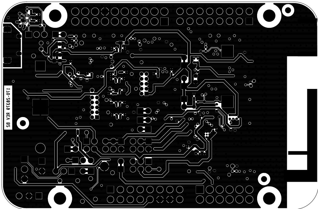
Figure 25. FRDM-KW40Z development board layout (bottom view)
