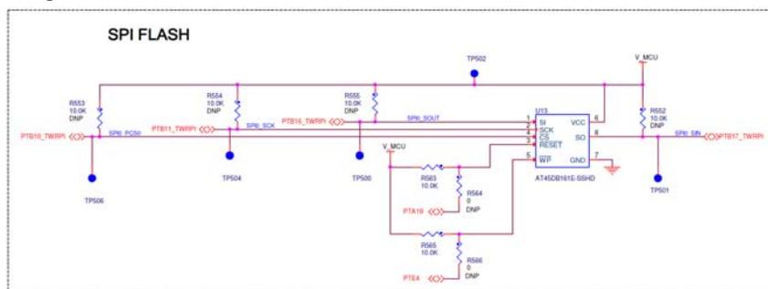
Figure 3-8. AT45DB161E-SSHD 16Mbit (2 Mbyte) Serial FLASH memory
