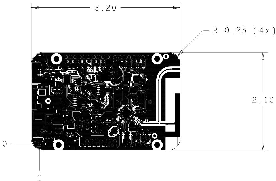
Figure 4. FRDM-KW40Z board dimensions
