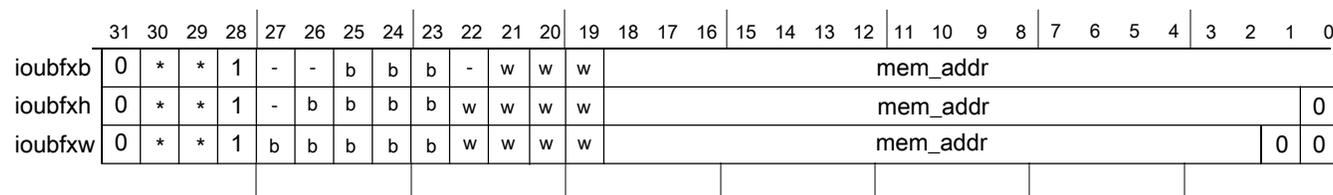
**Figure 13-11. Decorated load address: unsigned bit field extract**
