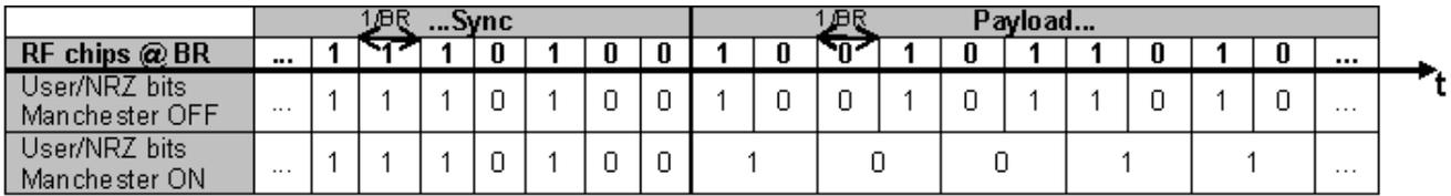
Figure 7-14. Manchester Encoding/Decoding
