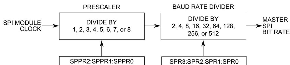
Figure 31-8. SPI baud rate generation
