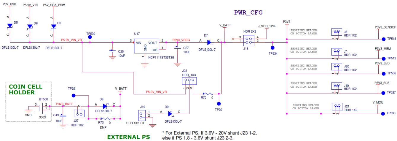
Figure 9. FRDM-KW40Z board's power management circuit
