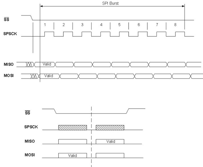
**Figure 8-3. Transceiver SPI Read Single Access Timing Diagram**
