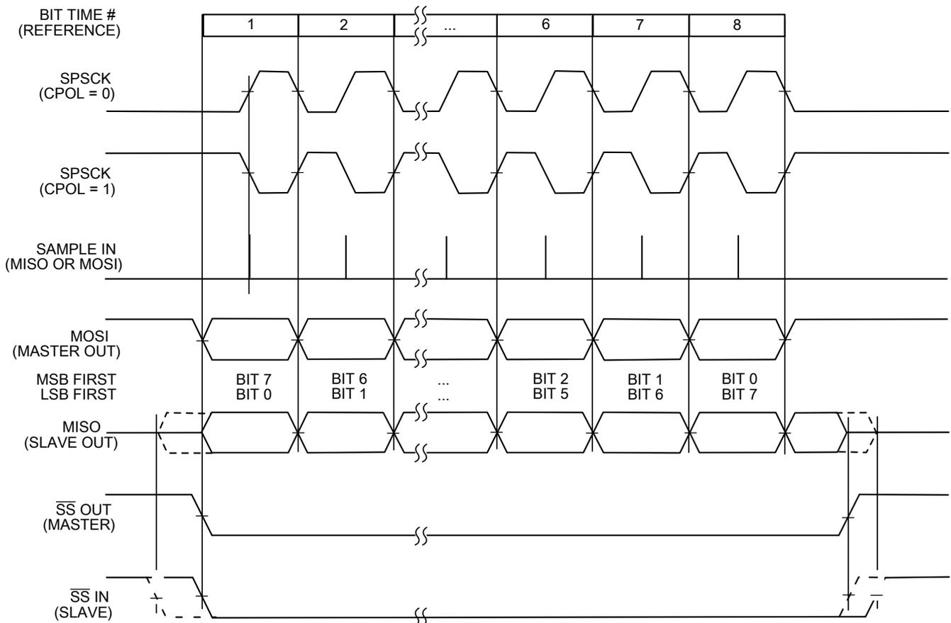
**Figure 31-7. SPI clock formats (CPHA = 0)**
