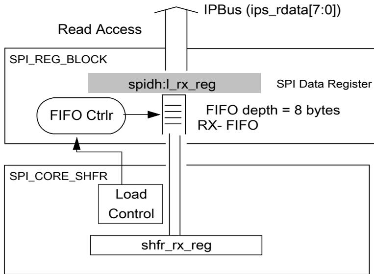
**Figure 31-3. SPIH:L read side structural overview in FIFO mode**
