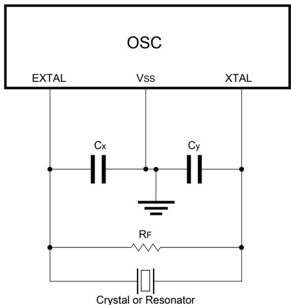
Figure 21-4. Crystal/Ceramic Resonator Connections - Connection 3
