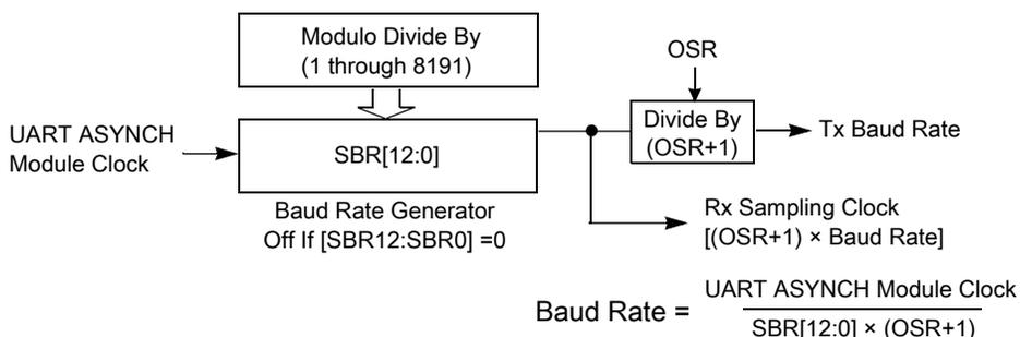
Figure 32-3. UART baud rate generation
