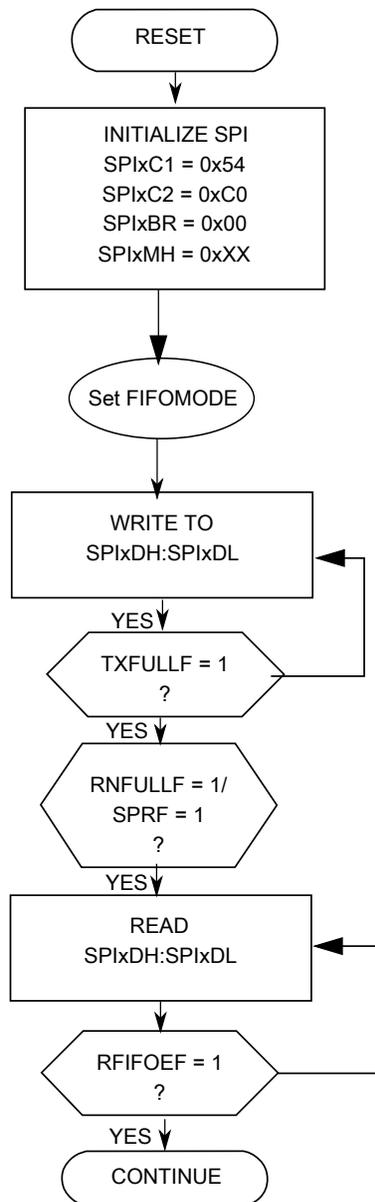
**Figure 31-10. Initialization Flowchart Example for SPI Master Device in 16-bit Mode for FIFOMODE = 1**
