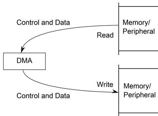
**Figure 19-2. Dual-Address Transfer**
