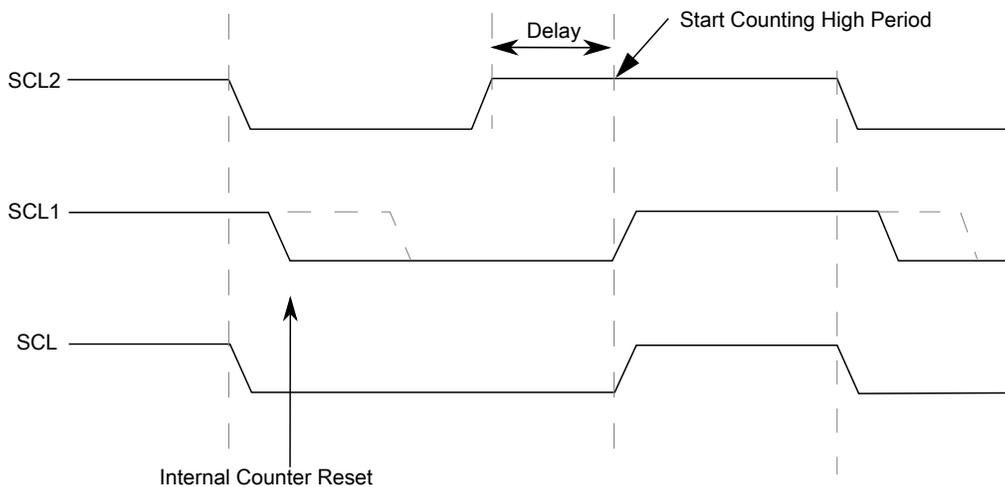
**Figure 36-3. I2C clock synchronization**
