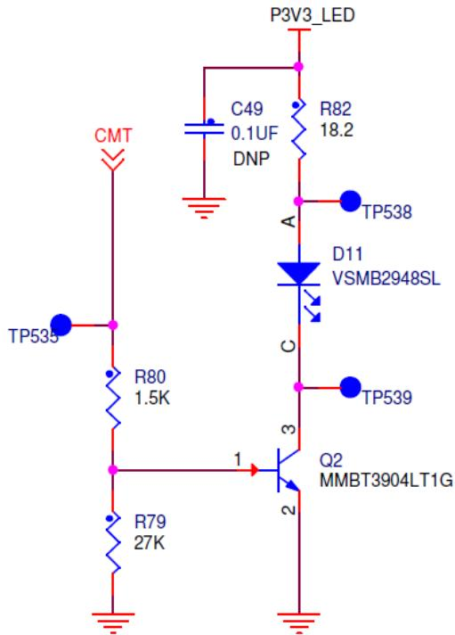
Figure 18. IR transmitter circuit
