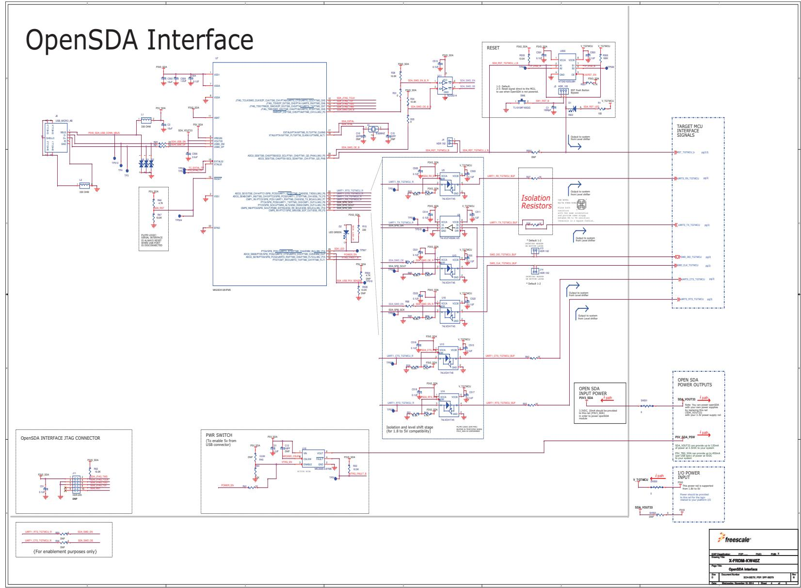
Figure 20. FRDM-KW40Z board schematic rev. B (sheet 2 of 3)
