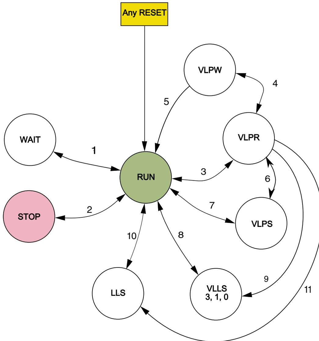
**Figure 9-1. Power mode state diagram**
