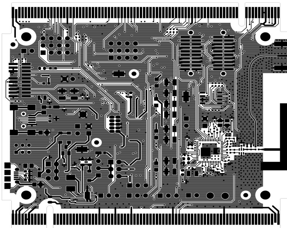
Figure 3-12. TWR-KW24D512 Reference Board PCB Layout (Top View)
