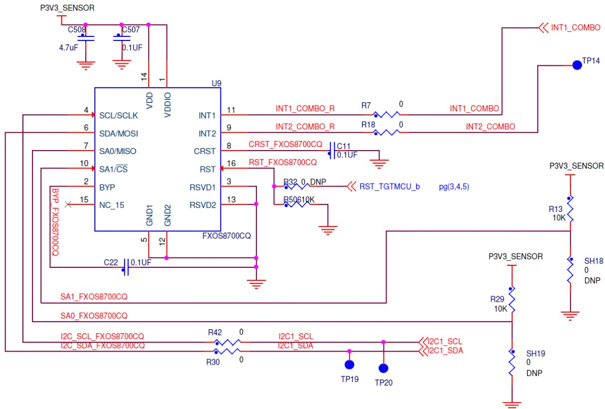
**Figure 15. FXOS8700CQ combo sensor circuit**
