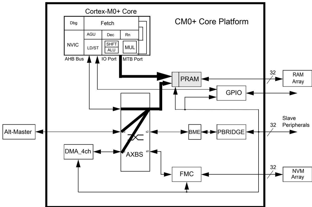
**Figure 15-1. Generic Cortex-M0+ core platform block diagram**
