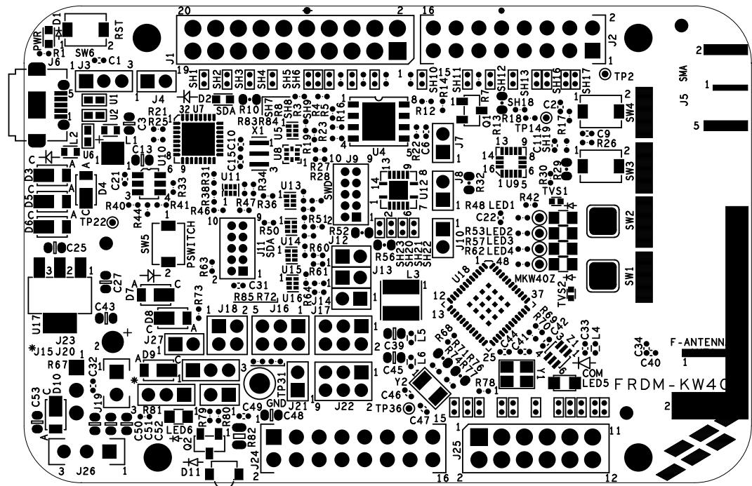
Figure 22. FRDM-KW40Z development board component location (top view)
