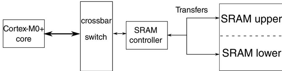
Figure 1-19. SRAM configuration
