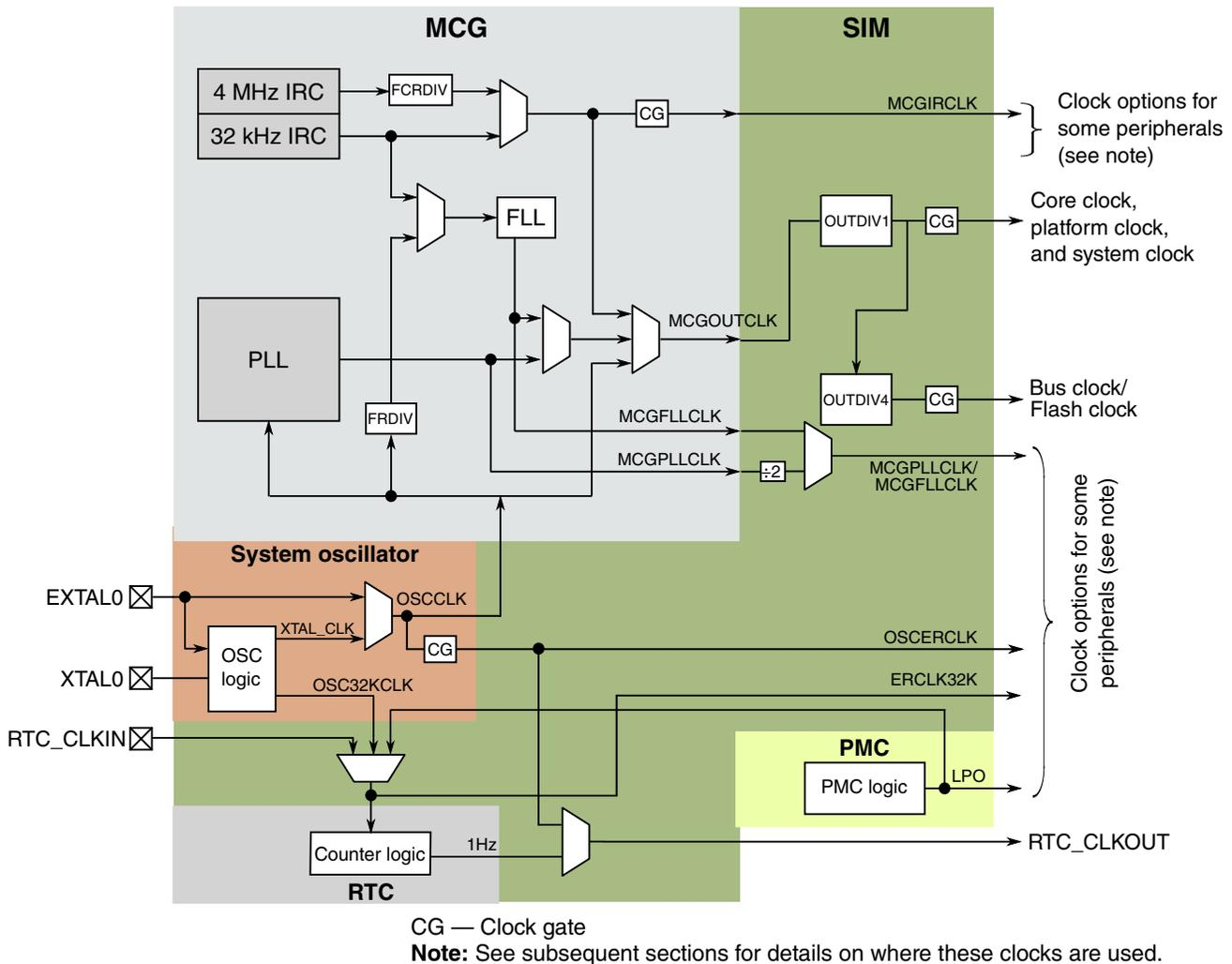
Figure 3-1. Clocking diagram
