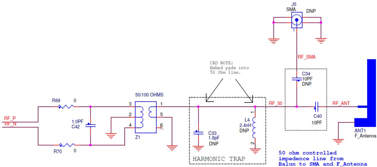
**Figure 6. FRDM-KW40Z board's RF circuitry**
