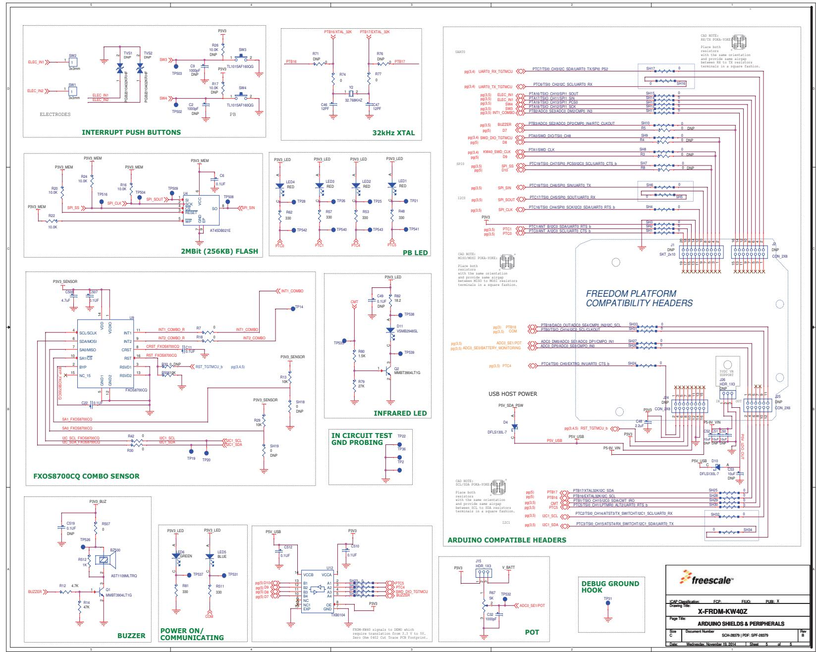
Figure 21. FRDM-KW40Z board schematic rev. B (sheet 3 of 3)
