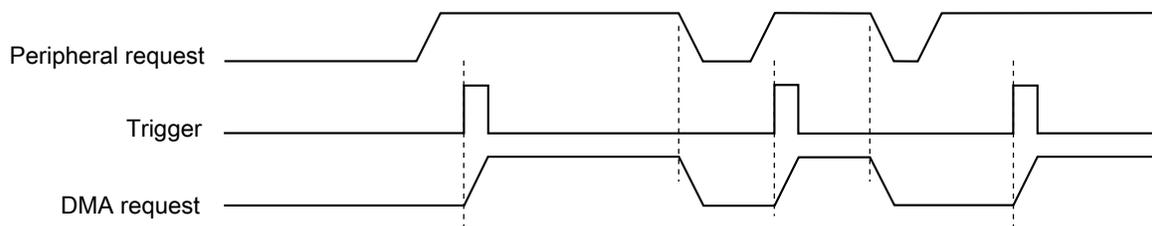
**Figure 18-3. DMAMUX channel triggering: normal operation**
