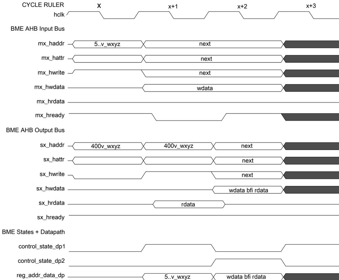
**Figure 13-2. Decorated store: bit field insert timing diagram**
