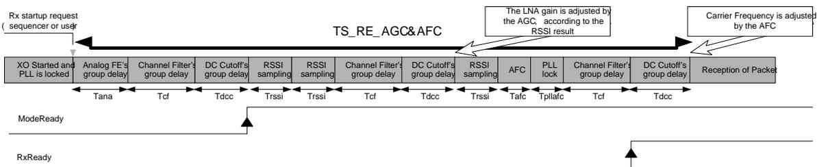
Figure 6-4. RX Startup - AGC and AFC
