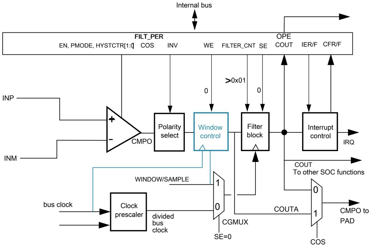
**Figure 25-5. Sampled, Filtered (# 4B): sampling point internally derived**
