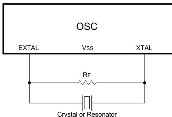
**Figure 21-3. Crystal/Ceramic Resonator Connections - Connection 2****NOTE**
