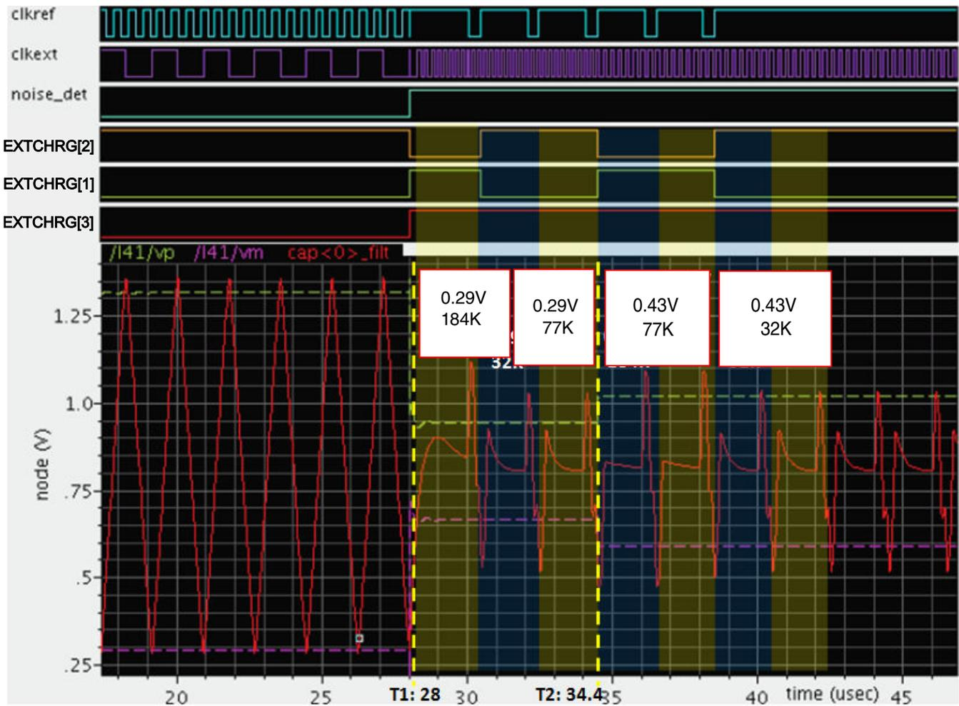
Figure 35-9. TSI noise detection mode waveform
