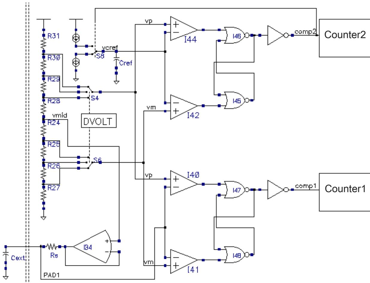
**Figure 35-6. TSI circuit in noise detection mode**
