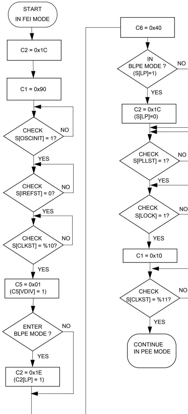
Figure 20-3. Flowchart of FEI to PEE mode transition using an 4 MHz crystal
