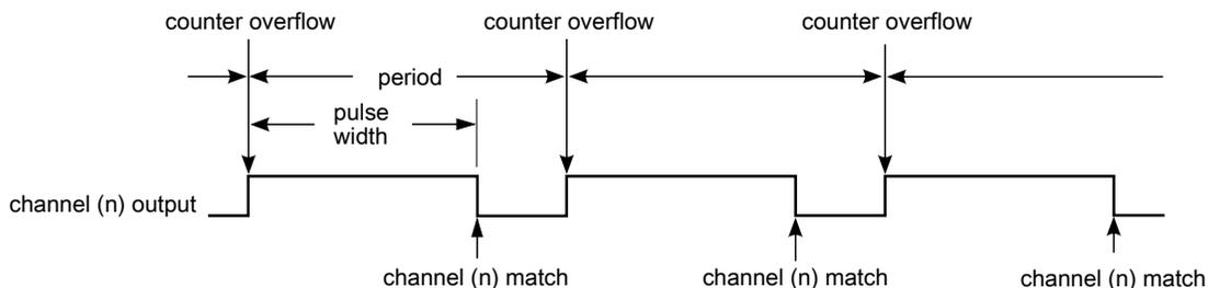
**Figure 27-9. EPWM period and pulse width with ELSnB:ELSnA = 1:0**
