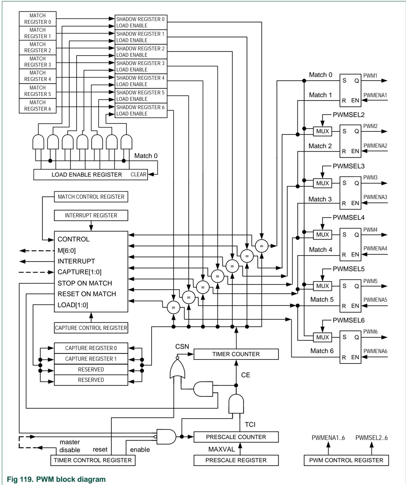
Fig 119. PWM block diagram
