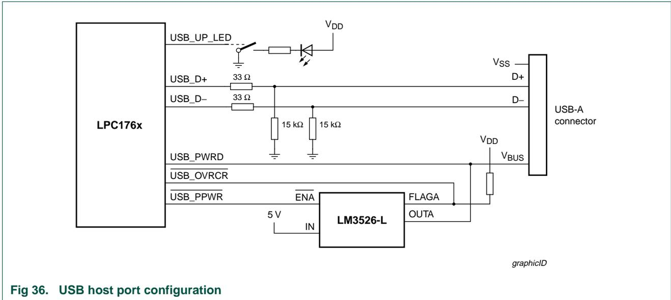
Fig 36. USB host port configuration
