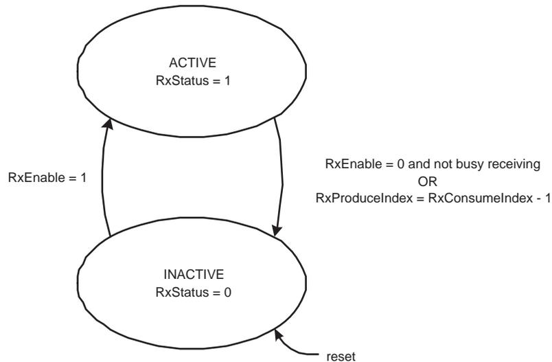
**Fig 25. Receive Active/Inactive state machine**
