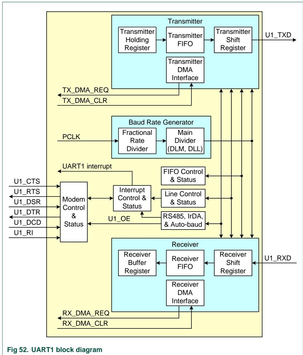
Fig 52. UART1 block diagram
