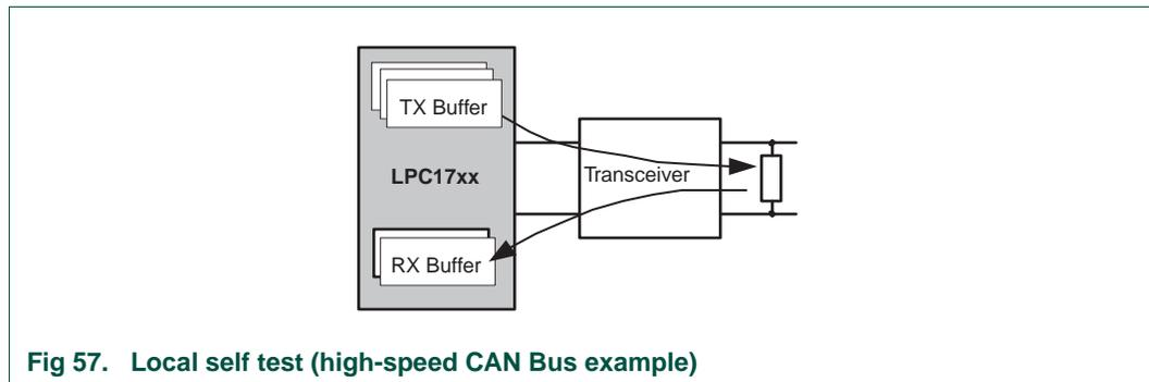
Fig 57. Local self test (high-speed CAN Bus example)
