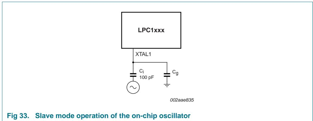
Fig 33. Slave mode operation of the on-chip oscillator
