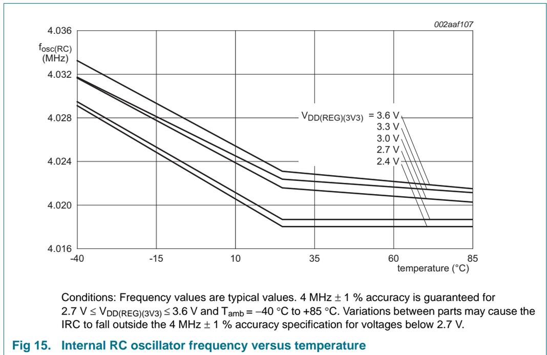
Fig 15. Internal RC oscillator frequency versus temperature
