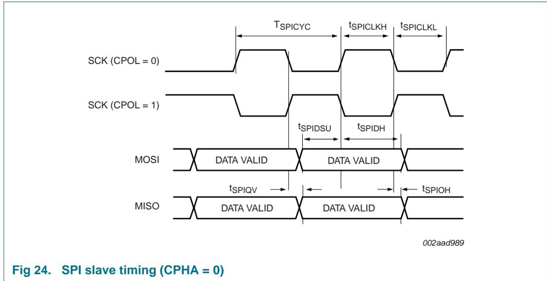
Fig 24. SPI slave timing (CPHA = 0)
