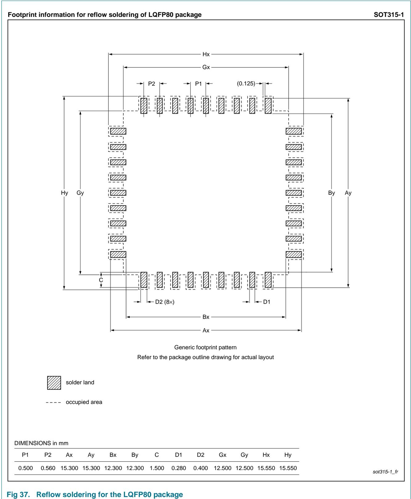
Fig 37. Reflow soldering for the LQFP80 package
