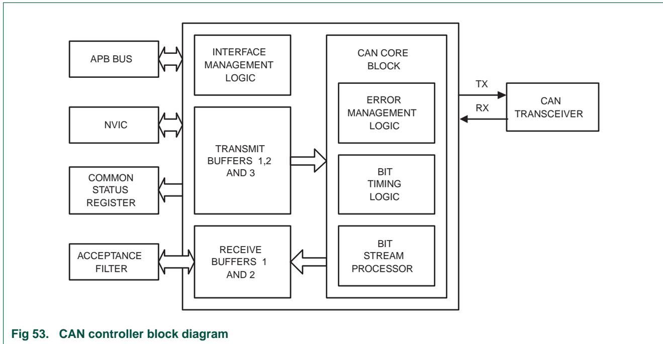
Fig 53. CAN controller block diagram
