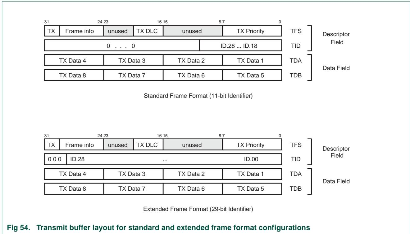
Fig 54. Transmit buffer layout for standard and extended frame format configurations
