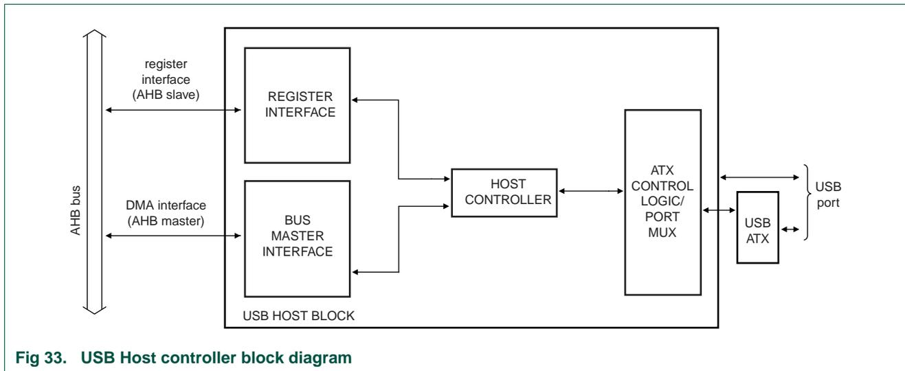
Fig 33. USB Host controller block diagram
