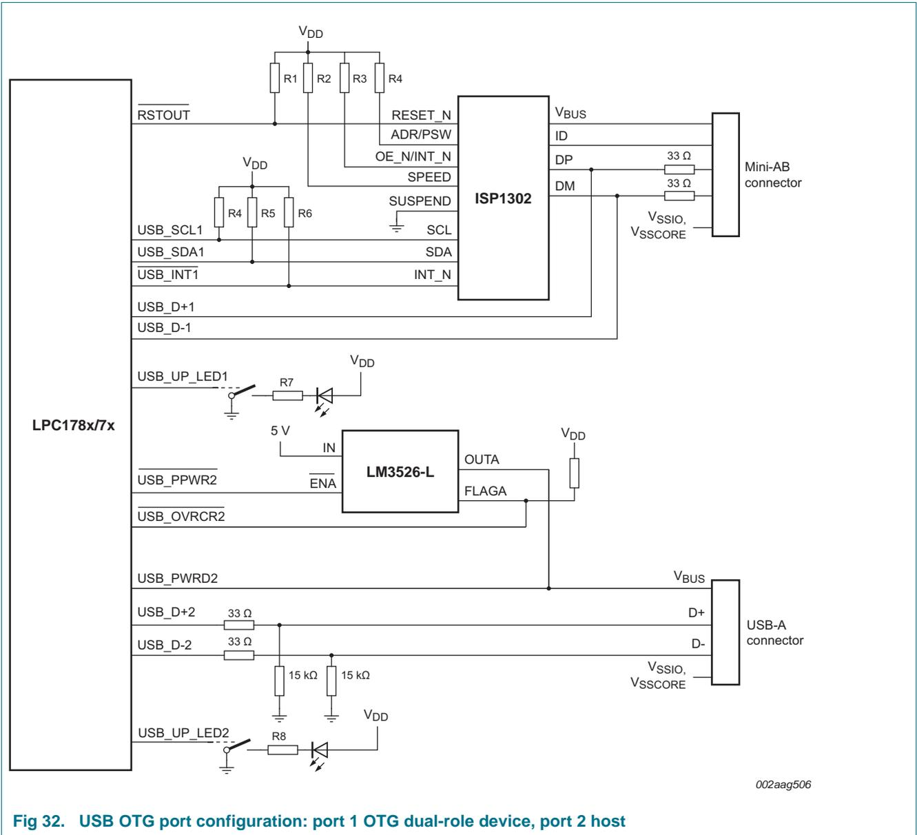
Fig 32. USB OTG port configuration: port 1 OTG dual-role device, port 2 host
