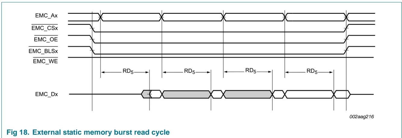
Fig 18. External static memory burst read cycle
