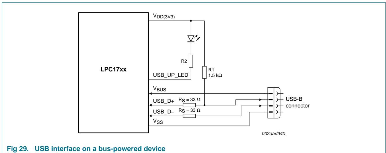
Fig 29. USB interface on a bus-powered device
