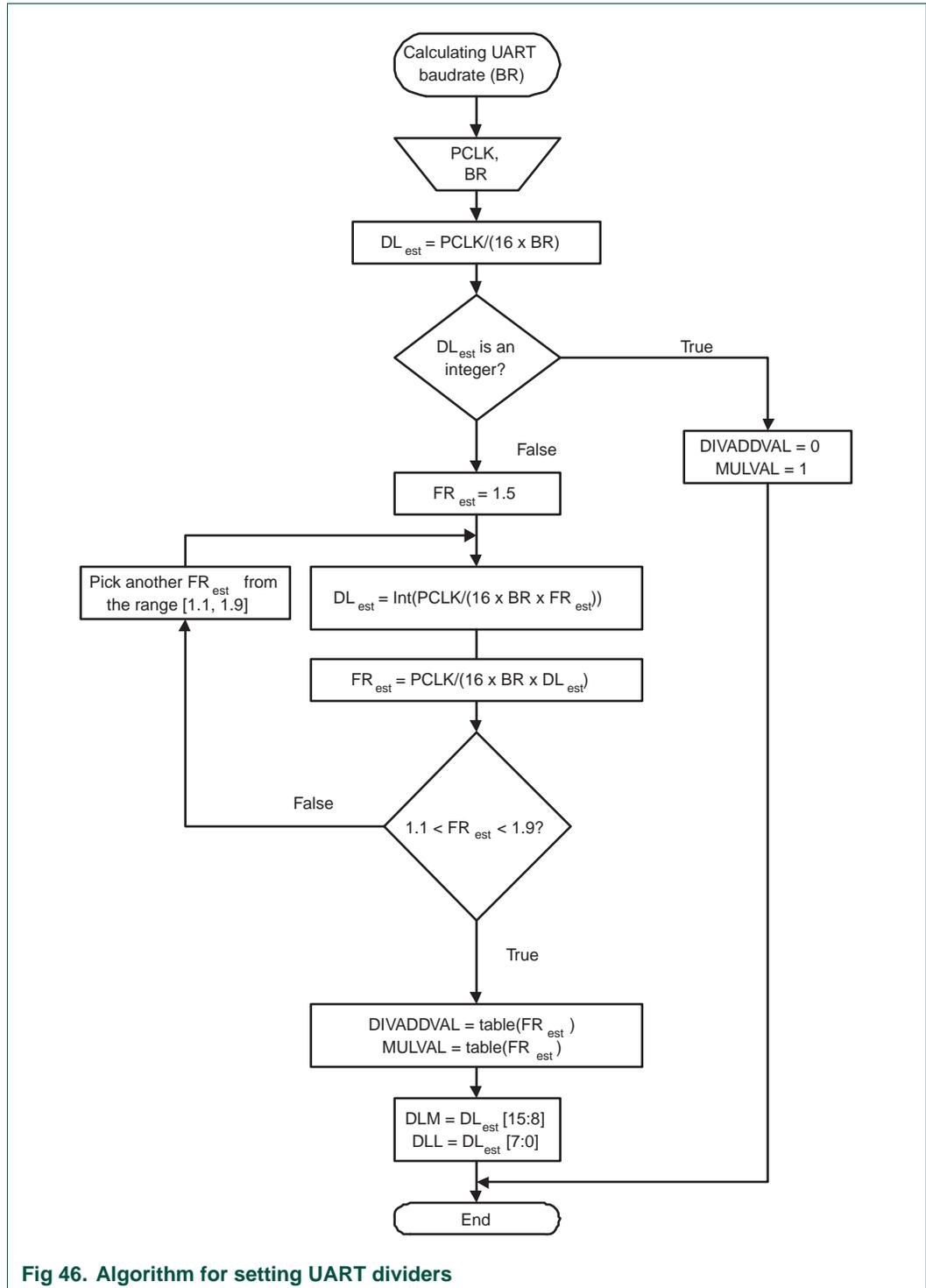
Fig 46. Algorithm for setting UART dividers
