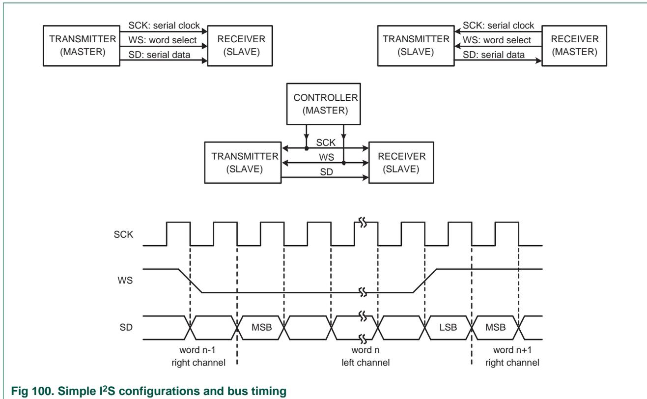
Fig 100. Simple I<sup>2</sup>S configurations and bus timing
