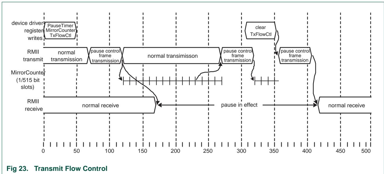
Fig 23. Transmit Flow Control
