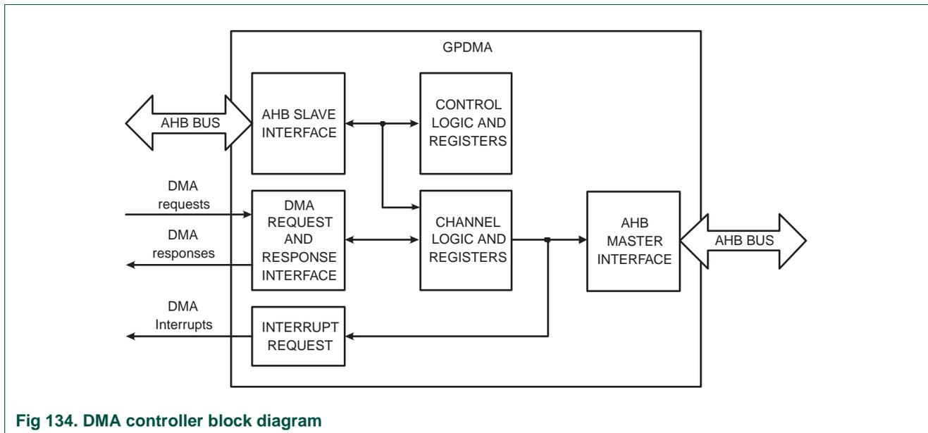
Fig 134. DMA controller block diagram
