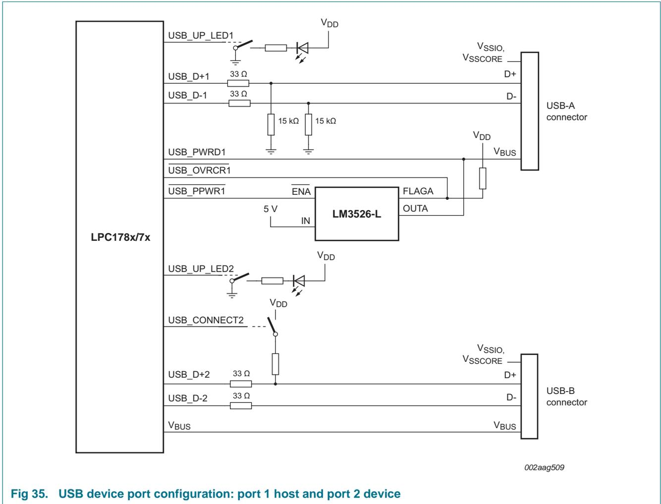
Fig 35. USB device port configuration: port 1 host and port 2 device
