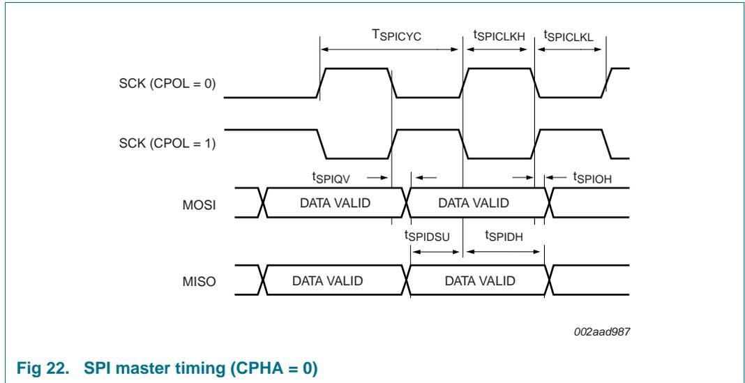
**Fig 22. SPI master timing (CPHA = 0)**
