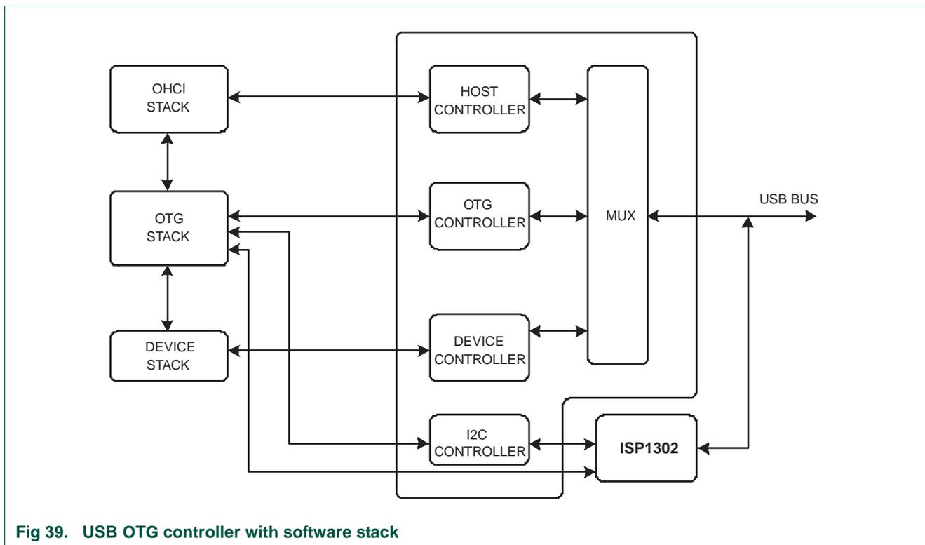
Fig 39. USB OTG controller with software stack
