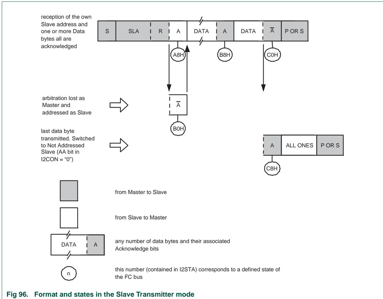
Fig 96. Format and states in the Slave Transmitter mode
