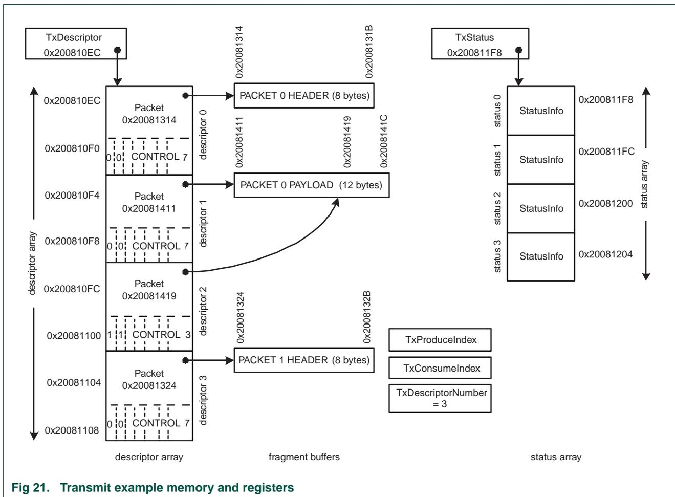
**Fig 21. Transmit example memory and registers**
