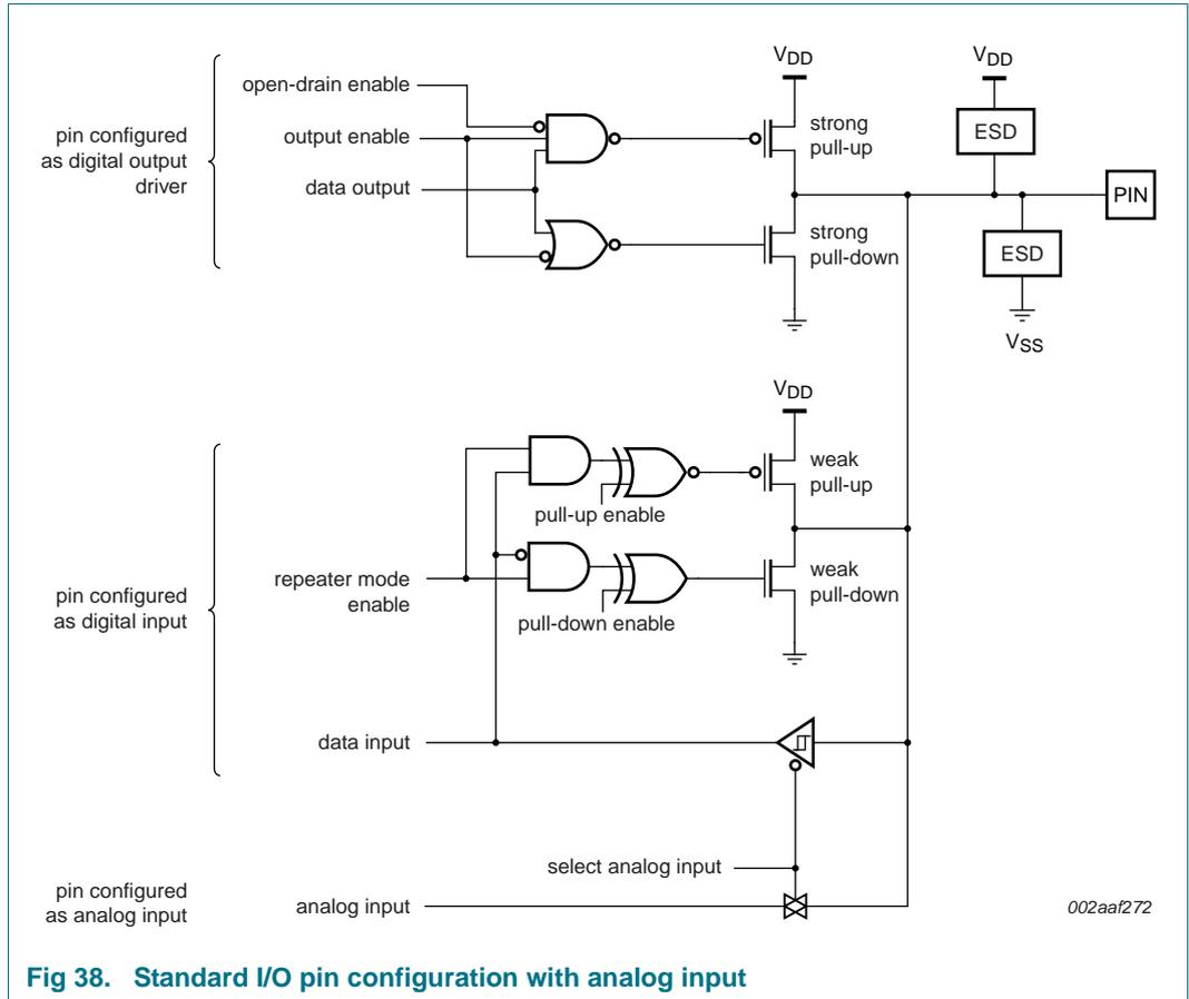
Fig 38. Standard I/O pin configuration with analog input
