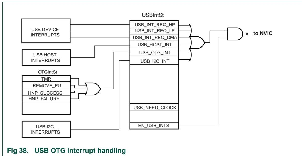
Fig 38. USB OTG interrupt handling
