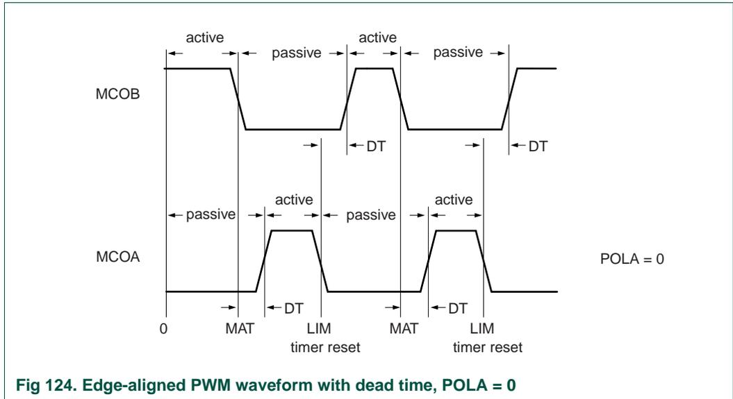
Fig 124. Edge-aligned PWM waveform with dead time, POLA = 0
