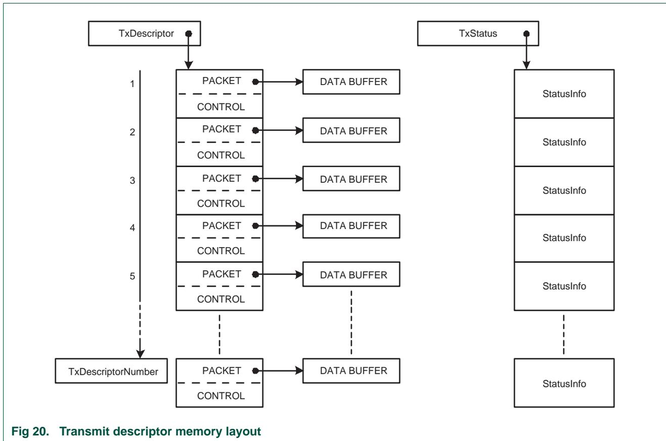
Fig 20. Transmit descriptor memory layout
