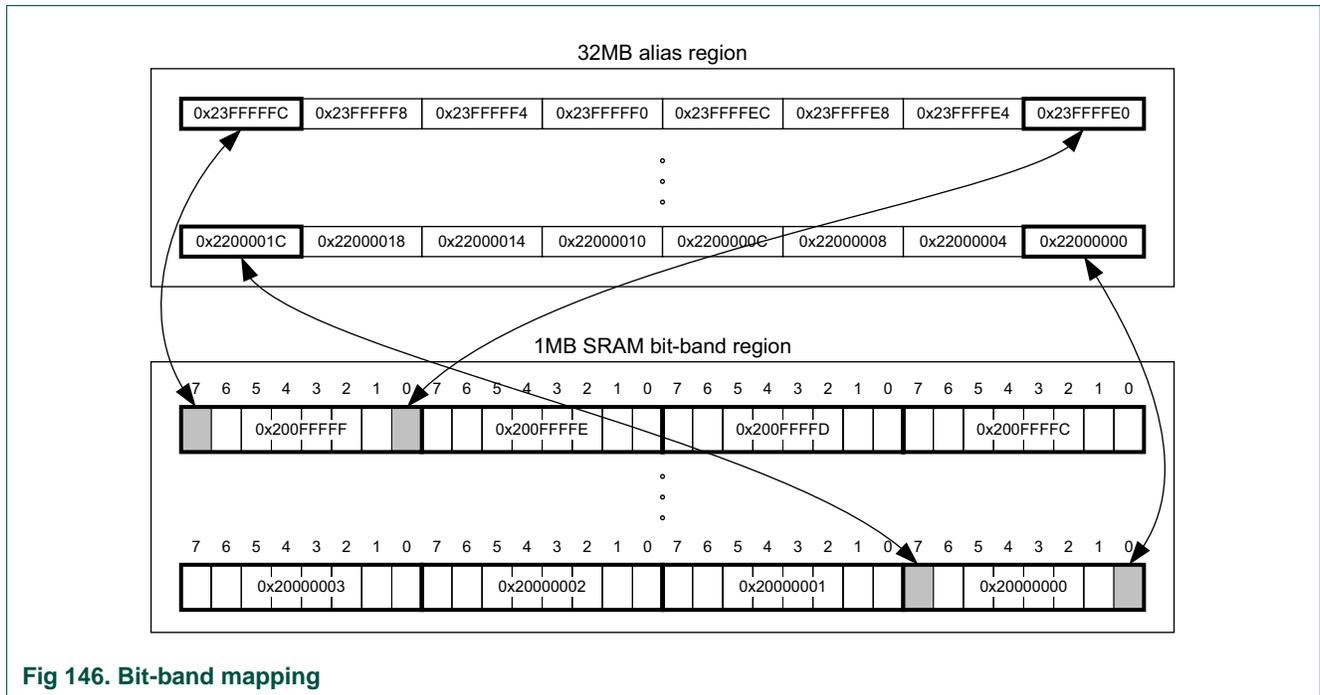
Fig 146. Bit-band mapping
