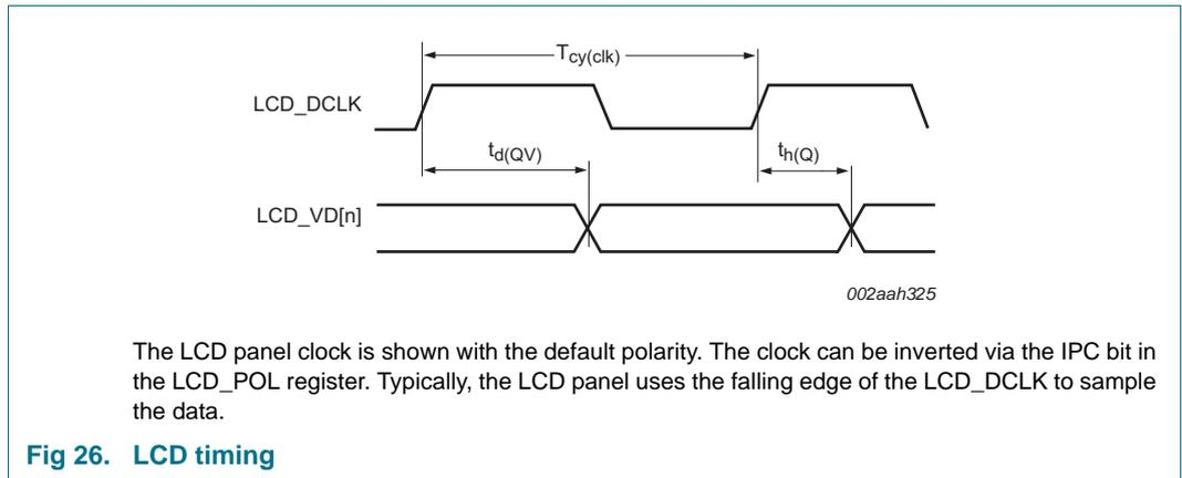
Fig 26. LCD timing
