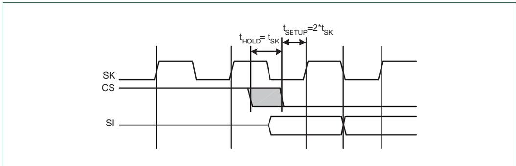
Fig 83. Microwire frame format setup and hold details
