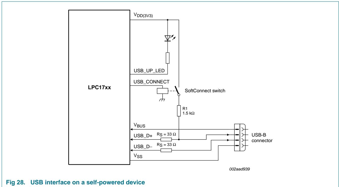
Fig 28. USB interface on a self-powered device
