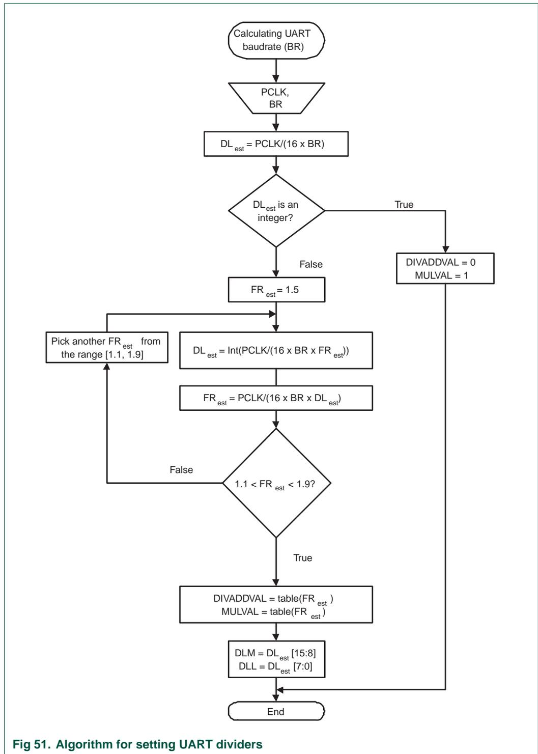
Fig 51. Algorithm for setting UART dividers
