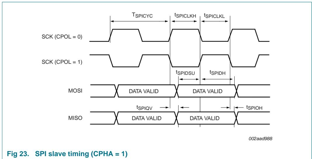
**Fig 23. SPI slave timing (CPHA = 1)**
