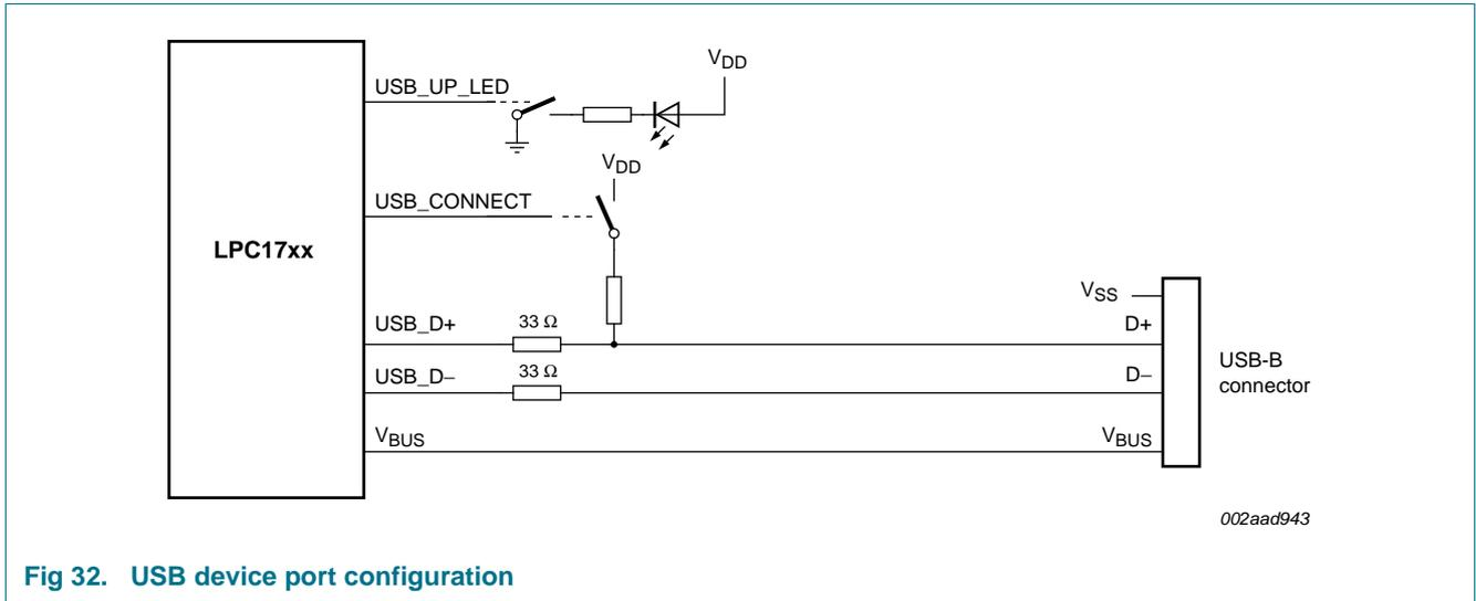
Fig 32. USB device port configuration
