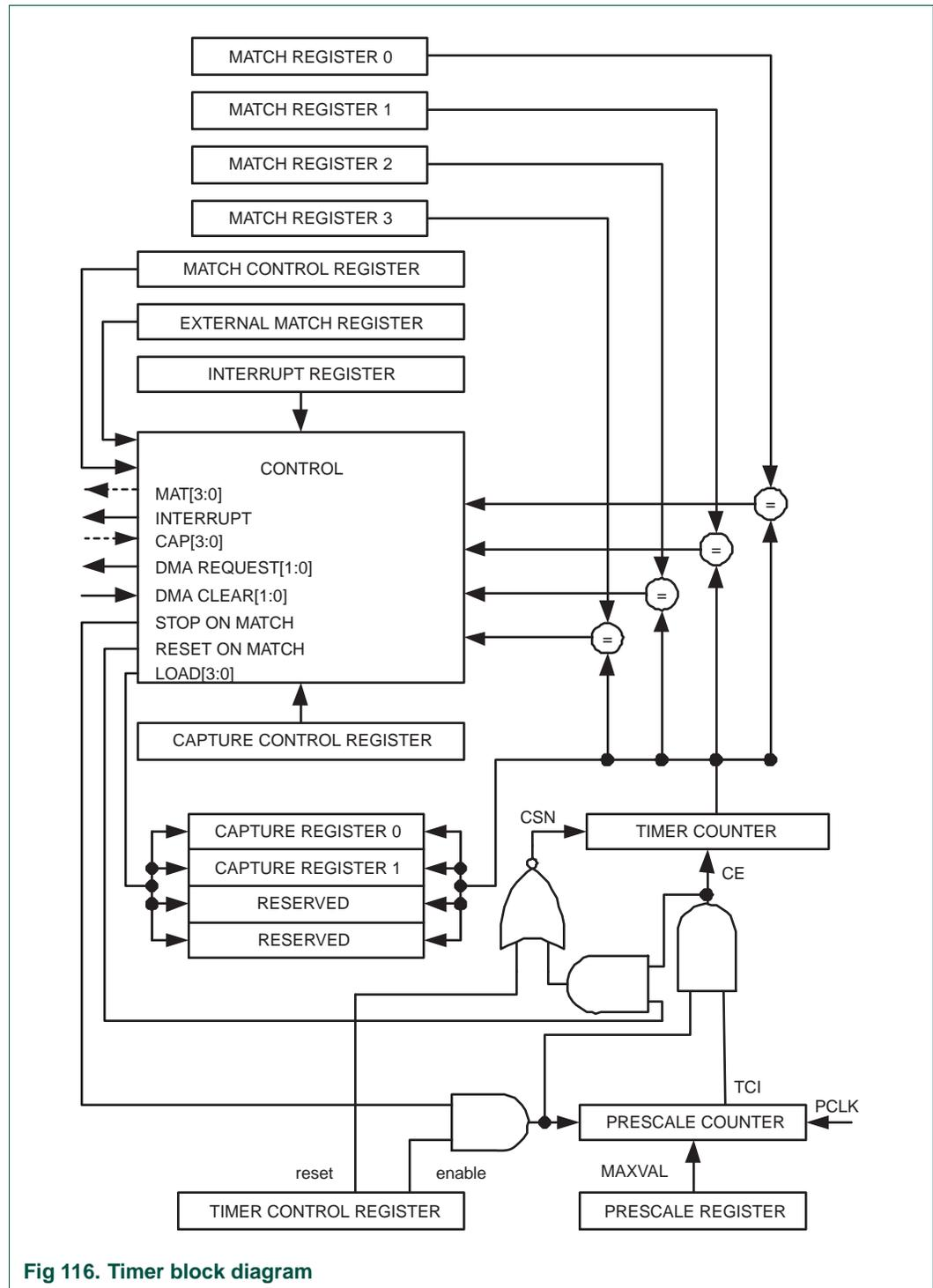
Fig 116. Timer block diagram
