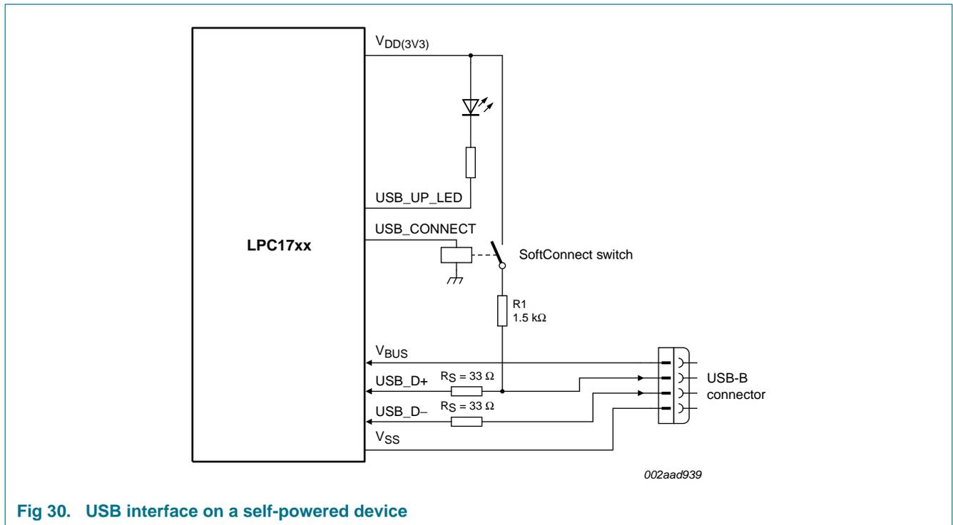
Fig 30. USB interface on a self-powered device
