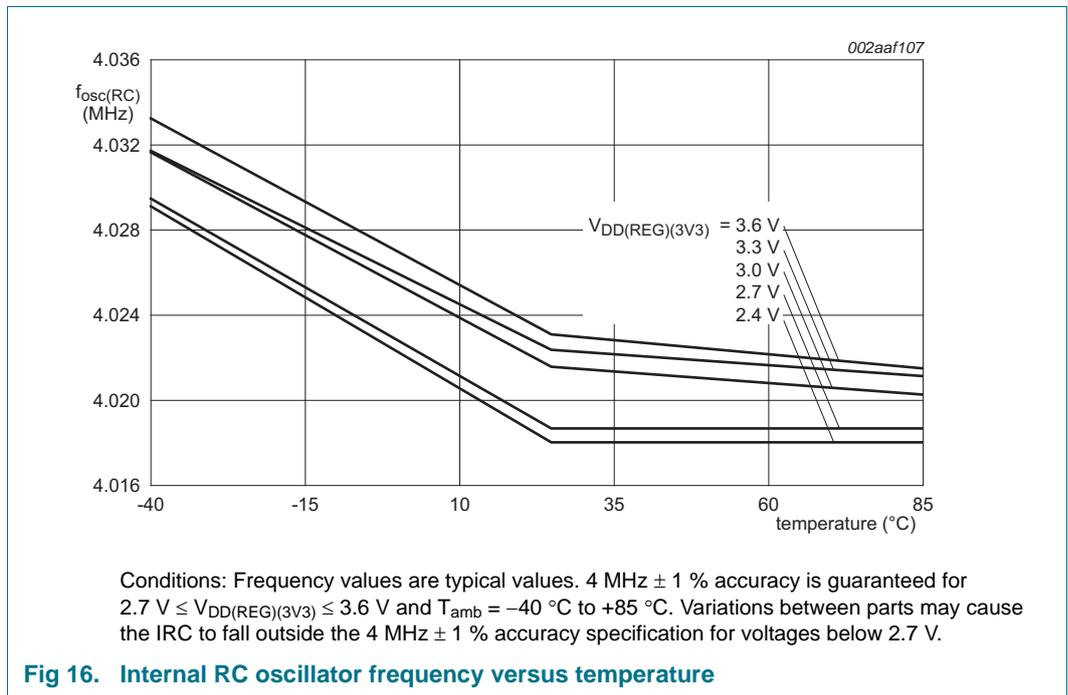
Fig 16. Internal RC oscillator frequency versus temperature
