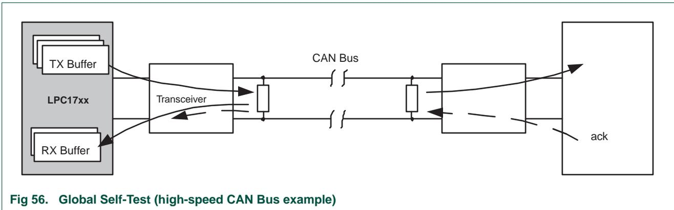
Fig 56. Global Self-Test (high-speed CAN Bus example)
