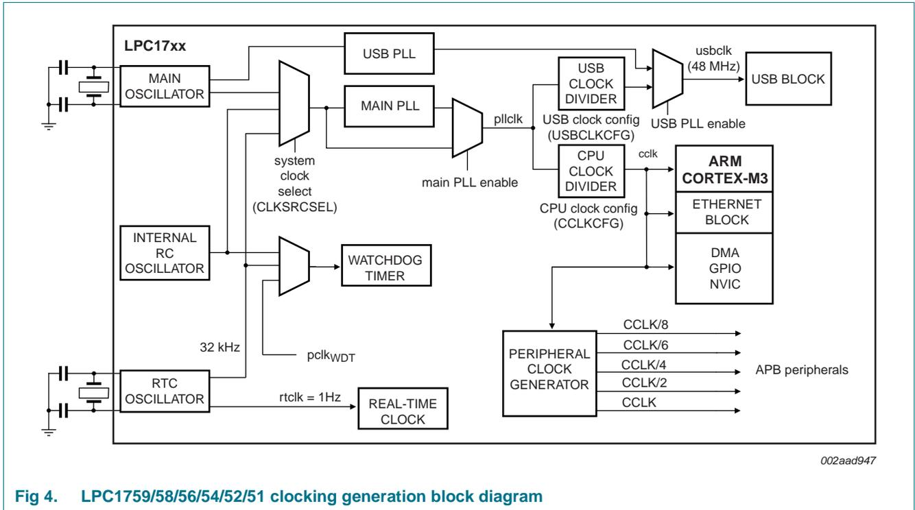
Fig 4. LPC1759/58/56/54/52/51 clocking generation block diagram
