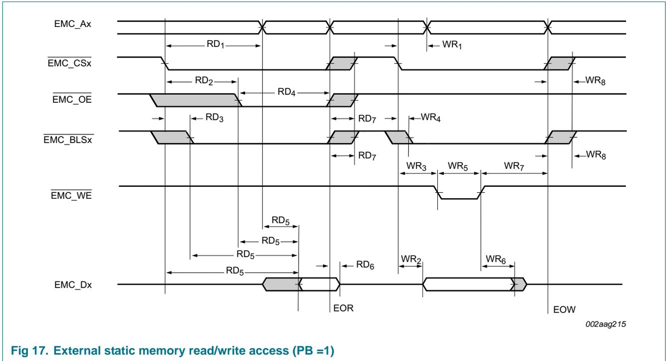
Fig 17. External static memory read/write access (PB =1)
