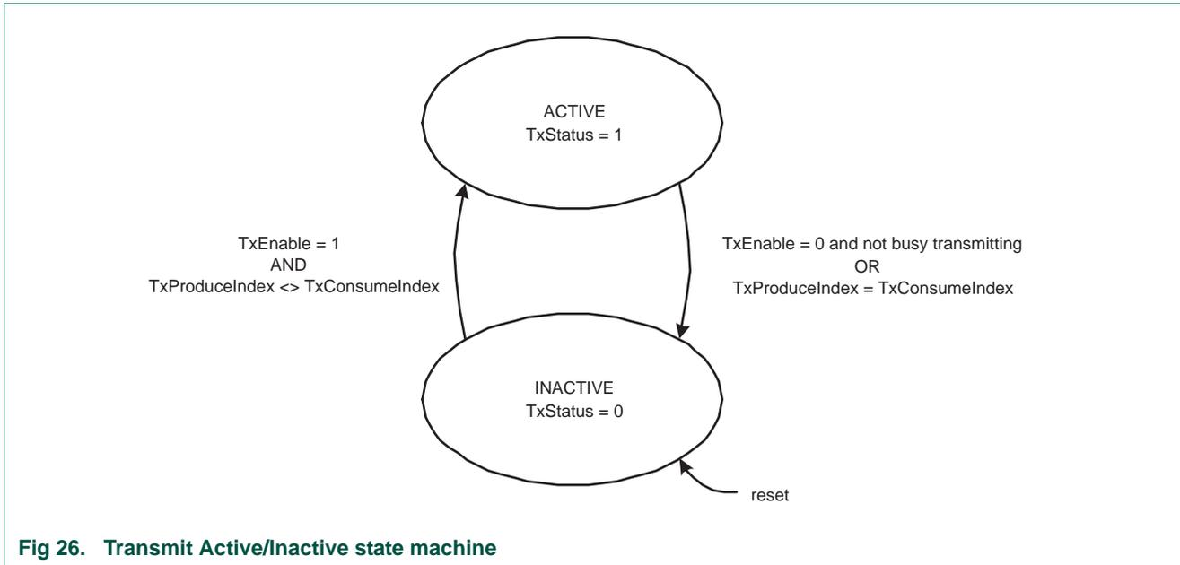
**Fig 26. Transmit Active/Inactive state machine**
