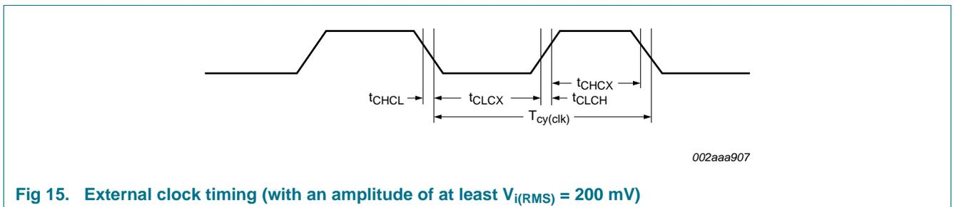
**Fig 15. External clock timing (with an amplitude of at least  $V_{i(RMS)} = 200\text{ mV}$ )**
