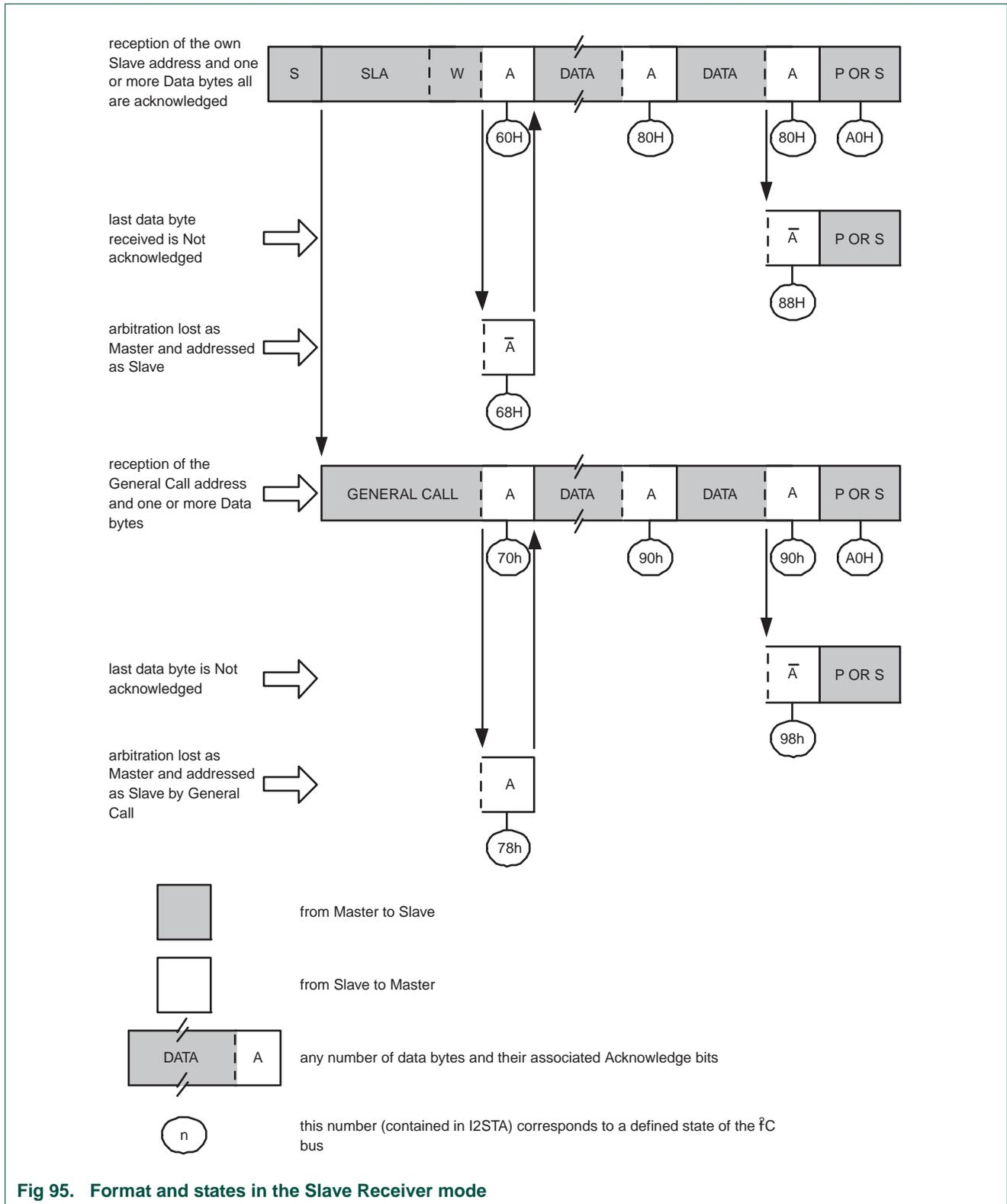
Fig 95. Format and states in the Slave Receiver mode
