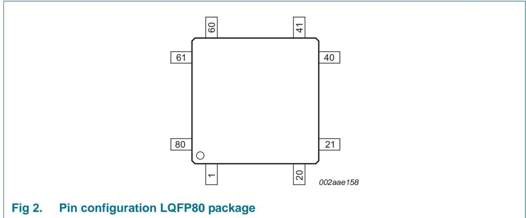
Fig 2. Pin configuration LQFP80 package
