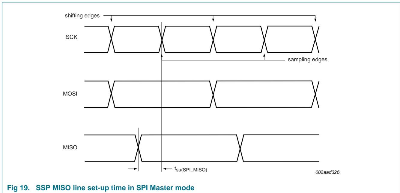
**Fig 19. SSP MISO line set-up time in SPI Master mode**
