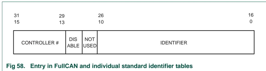
**Fig 58. Entry in FullCAN and individual standard identifier tables**
