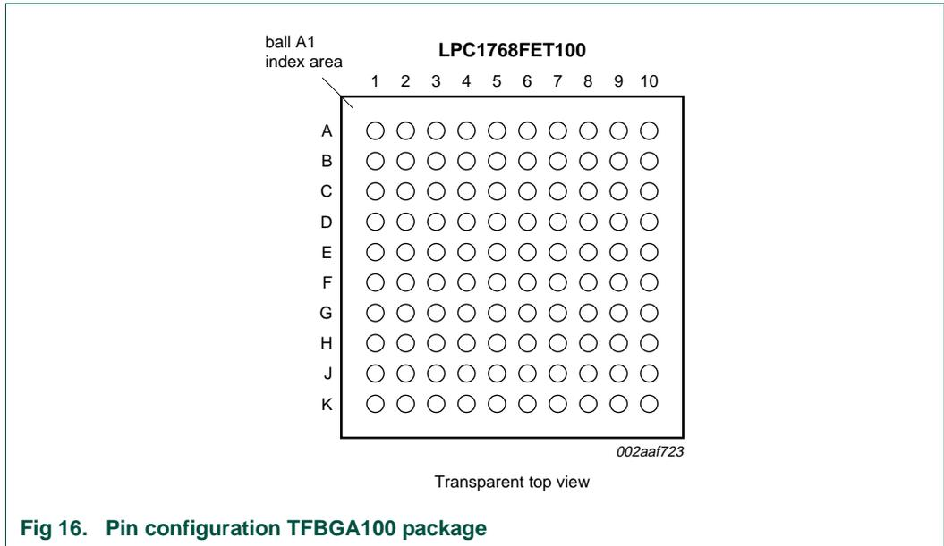
Fig 16. Pin configuration TFBGA100 package
