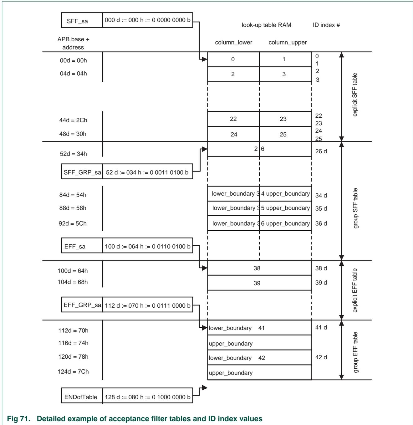
Fig 71. Detailed example of acceptance filter tables and ID index values
