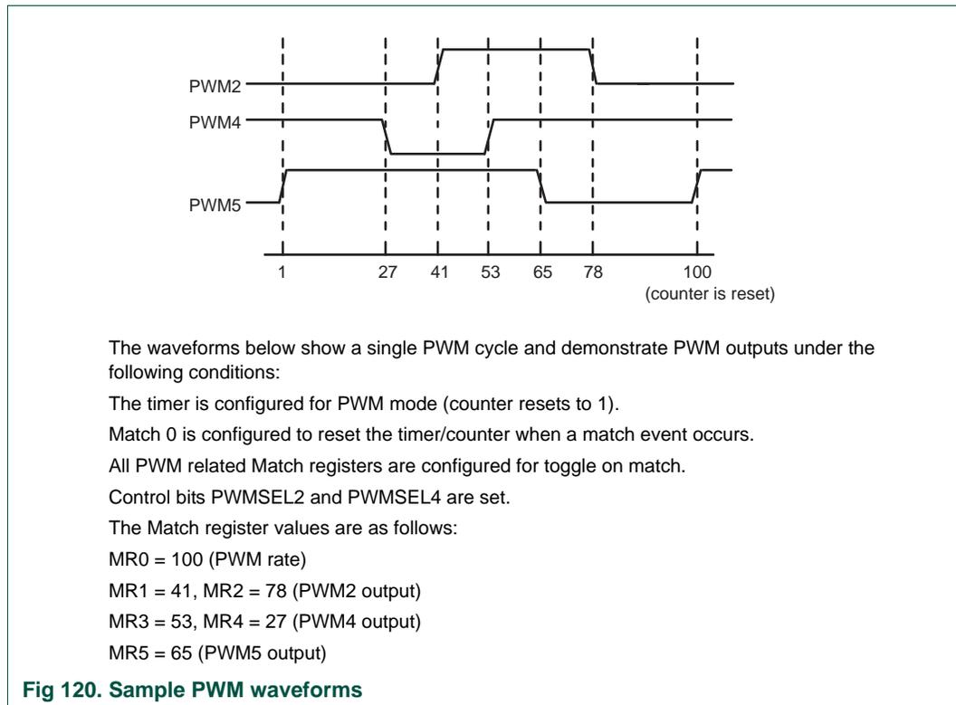
**Fig 120. Sample PWM waveforms**
