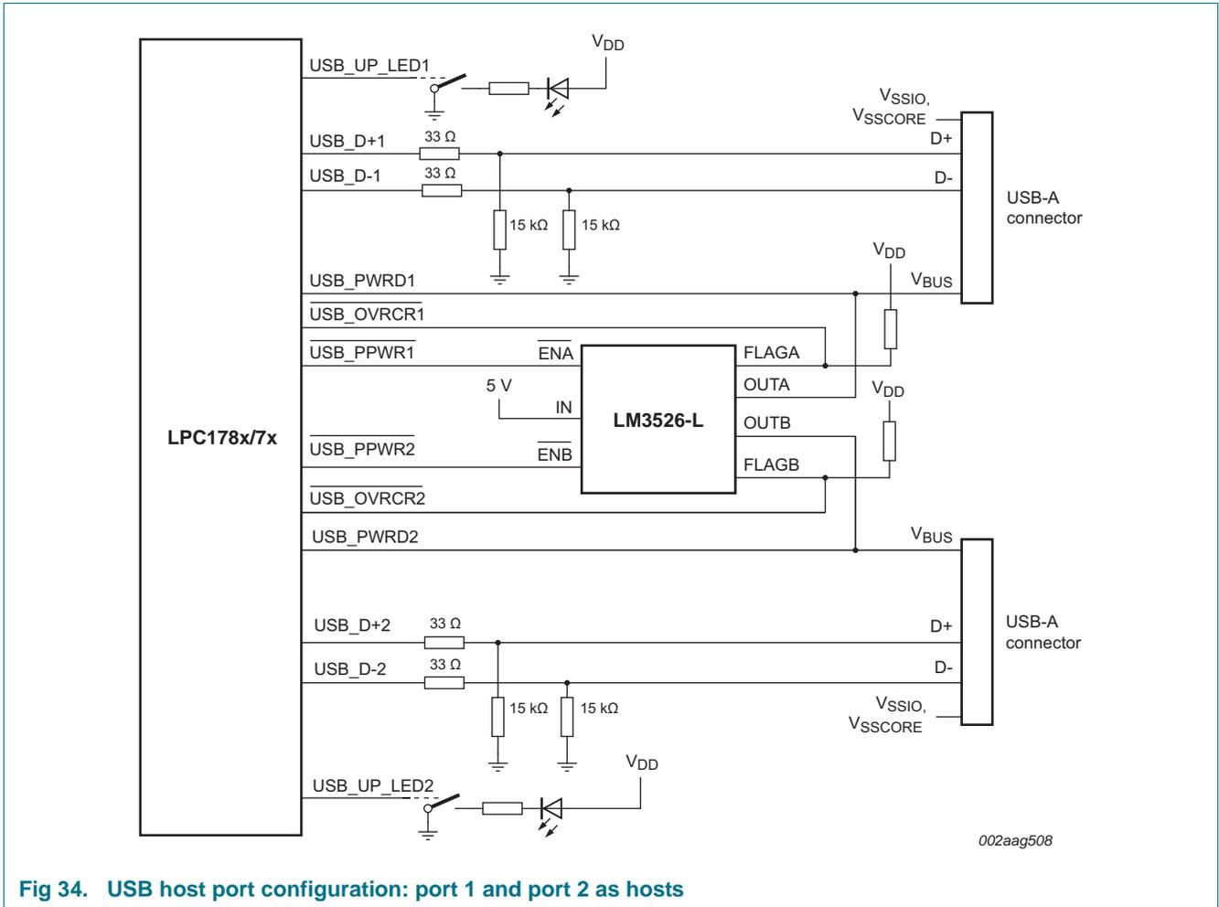
Fig 34. USB host port configuration: port 1 and port 2 as hosts
