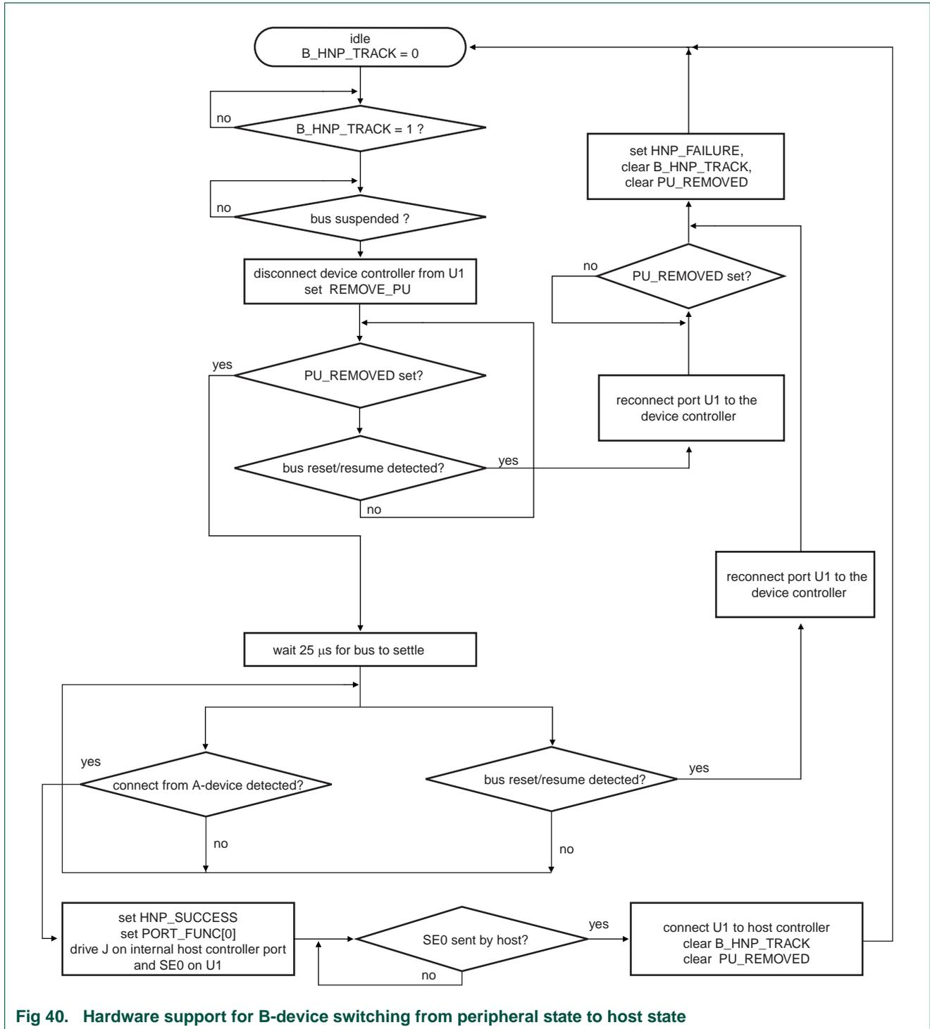
Fig 40. Hardware support for B-device switching from peripheral state to host state
