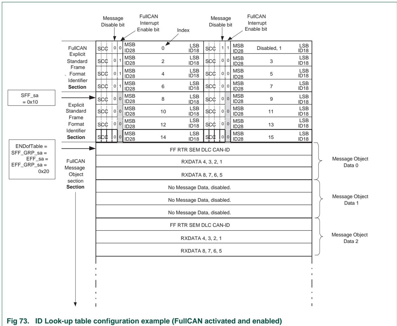
Fig 73. ID Look-up table configuration example (FullCAN activated and enabled)
