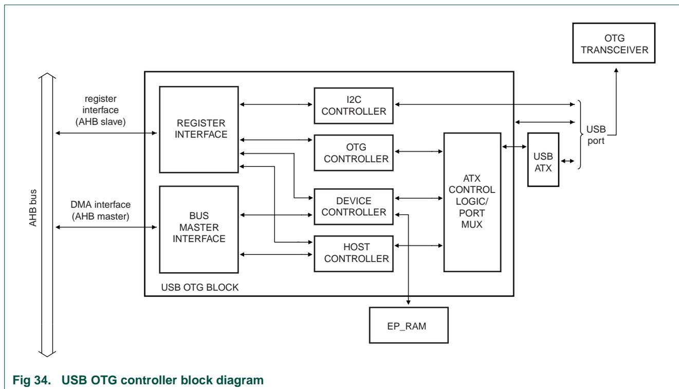
Fig 34. USB OTG controller block diagram
