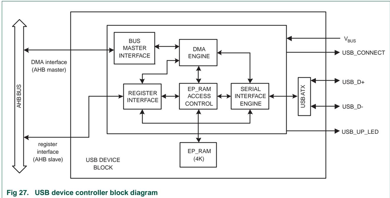
Fig 27. USB device controller block diagram
