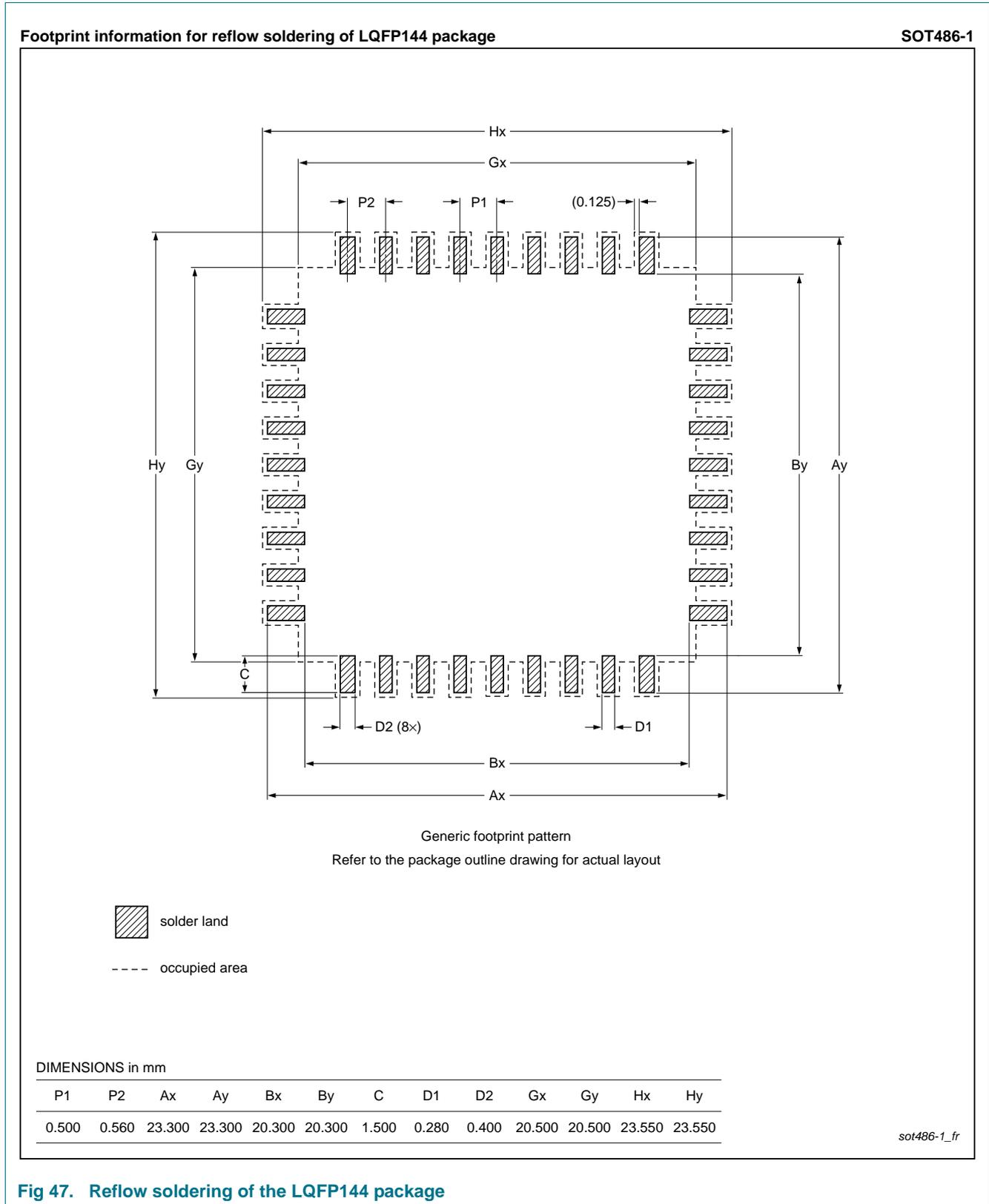
**Fig 47. Reflow soldering of the LQFP144 package**
