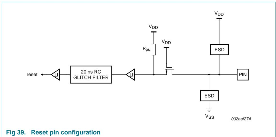
Fig 39. Reset pin configuration
