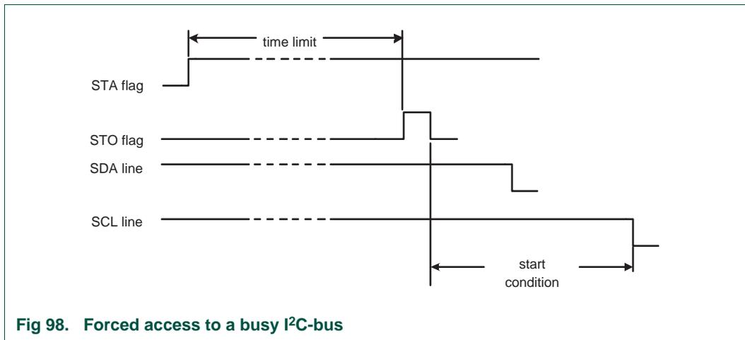
**Fig 98. Forced access to a busy I<sup>2</sup>C-bus**
