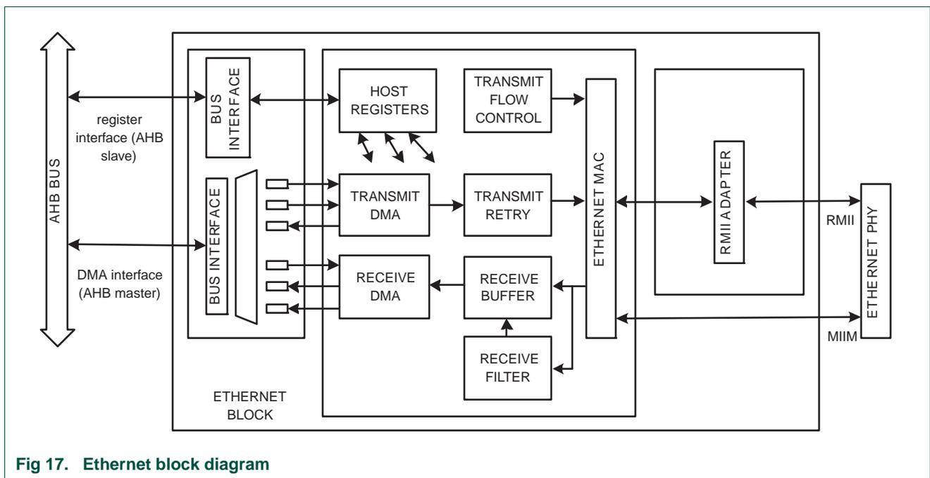
Fig 17. Ethernet block diagram
