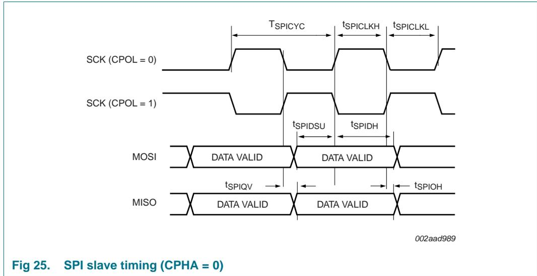
Fig 25. SPI slave timing (CPHA = 0)
