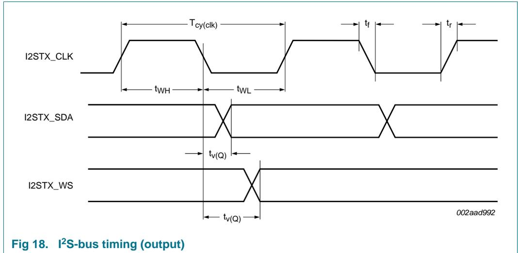
**Fig 18. I<sup>2</sup>S-bus timing (output)**
