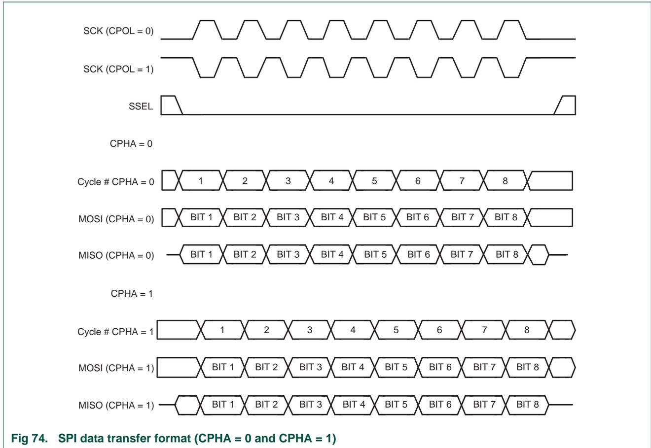
**Fig 74. SPI data transfer format (CPHA = 0 and CPHA = 1)**
