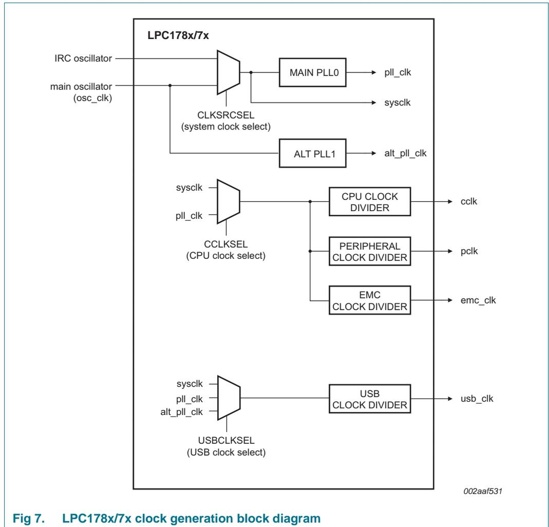
Fig 7. LPC178x/7x clock generation block diagram
