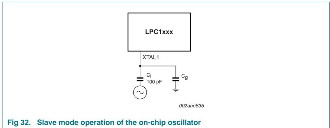
Fig 32. Slave mode operation of the on-chip oscillator
