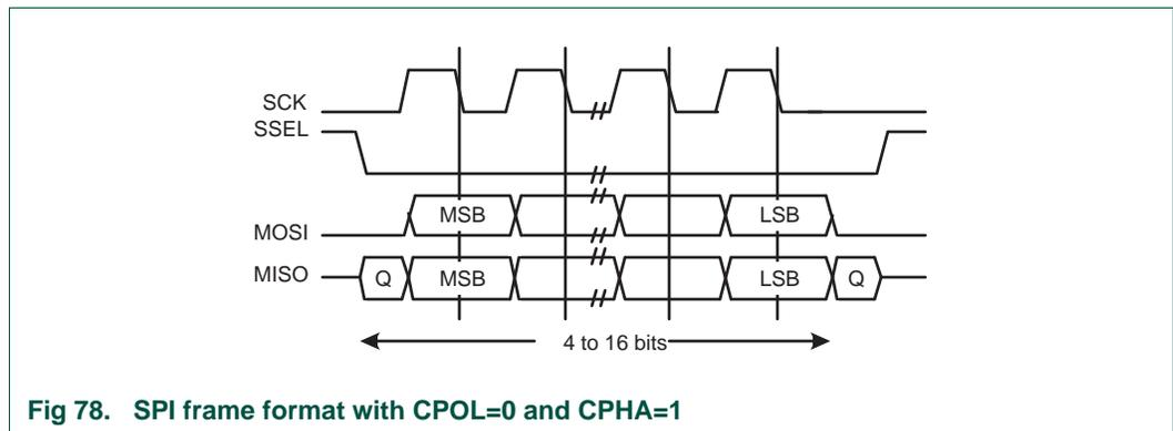
**Fig 78. SPI frame format with CPOL=0 and CPHA=1**
