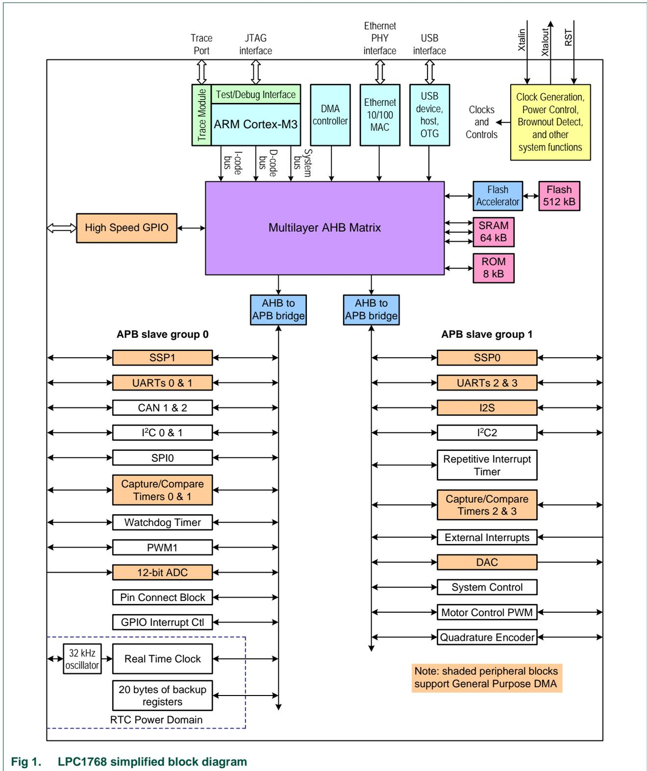
Fig 1. LPC1768 simplified block diagram
