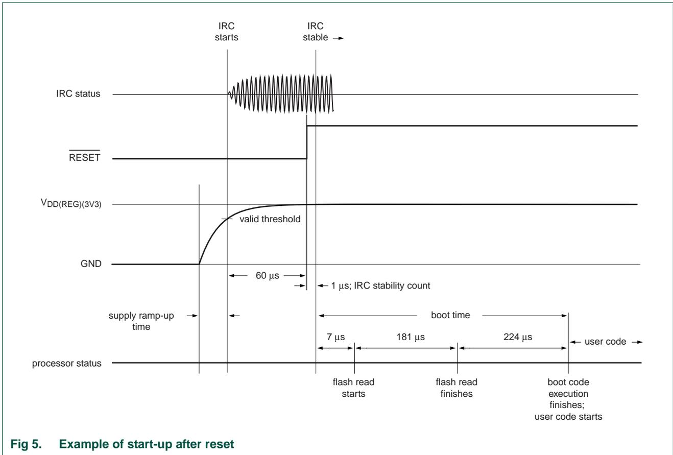
Fig 5. Example of start-up after reset
