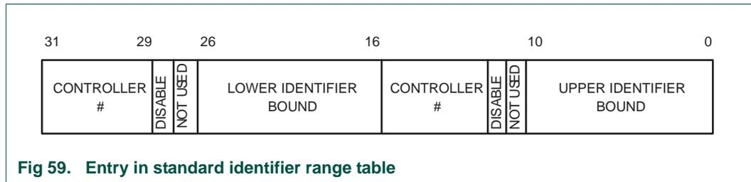
**Fig 59. Entry in standard identifier range table**
