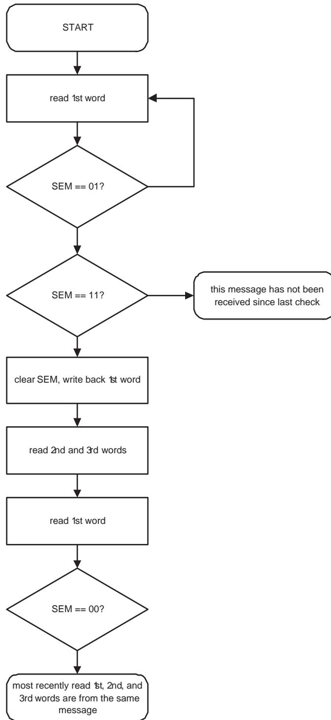
Fig 62. Semaphore procedure for reading an auto-stored message
