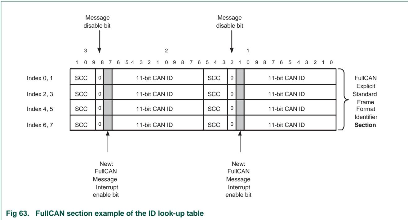
Fig 63. FullCAN section example of the ID look-up table
