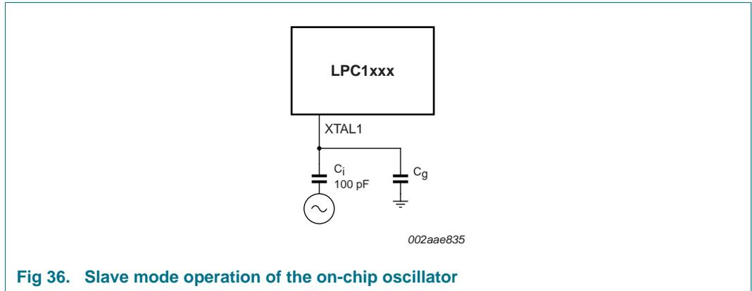
Fig 36. Slave mode operation of the on-chip oscillator
