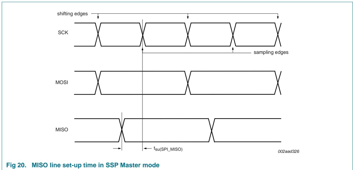
**Fig 20. MISO line set-up time in SSP Master mode**
