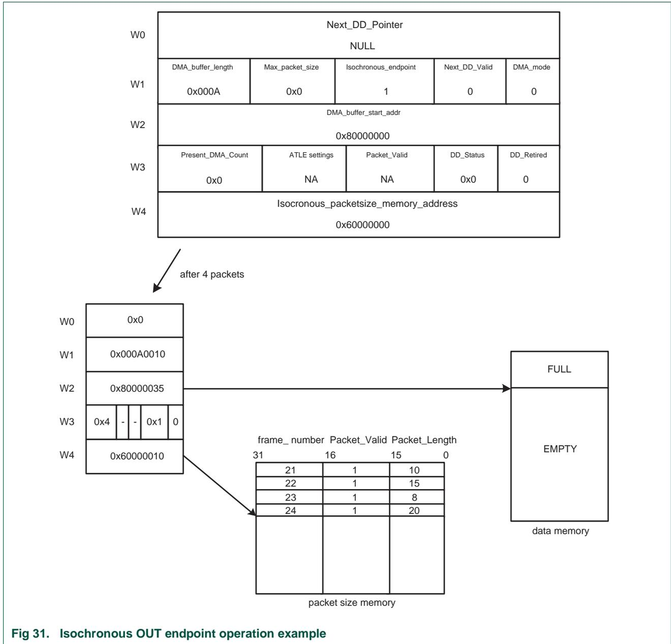
Fig 31. Isochronous OUT endpoint operation example
