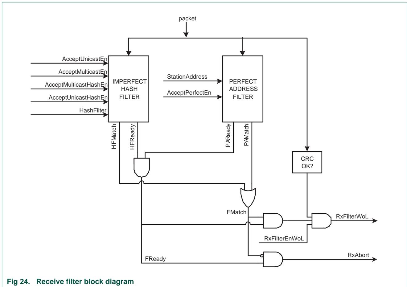
Fig 24. Receive filter block diagram
