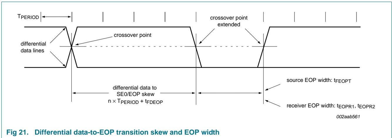
**Fig 21. Differential data-to-EOP transition skew and EOP width**
