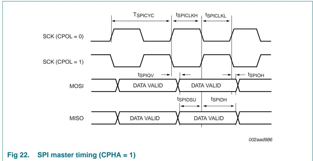
Fig 22. SPI master timing (CPHA = 1)
