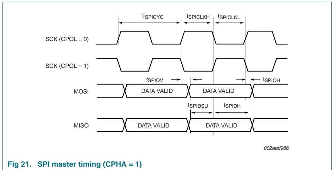
Fig 21. SPI master timing (CPHA = 1)
