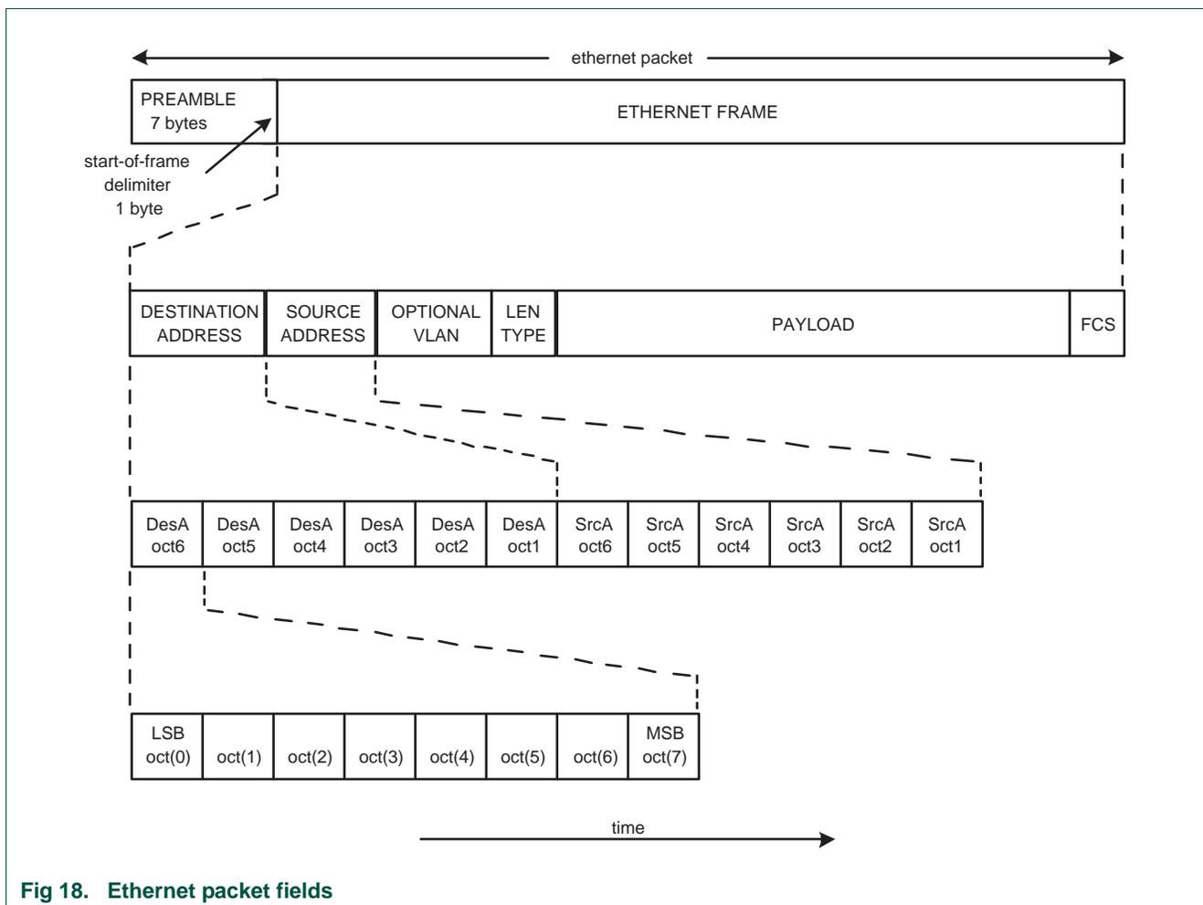
Fig 18. Ethernet packet fields
