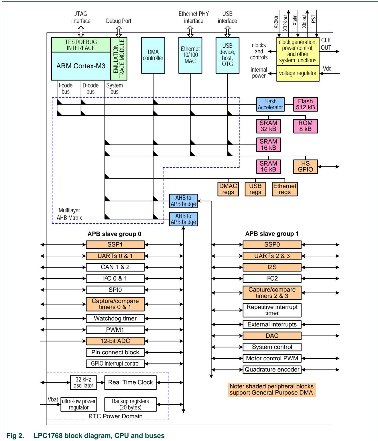
Fig 2. LPC1768 block diagram, CPU and buses
