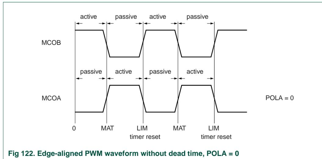
Fig 122. Edge-aligned PWM waveform without dead time, POLA = 0
