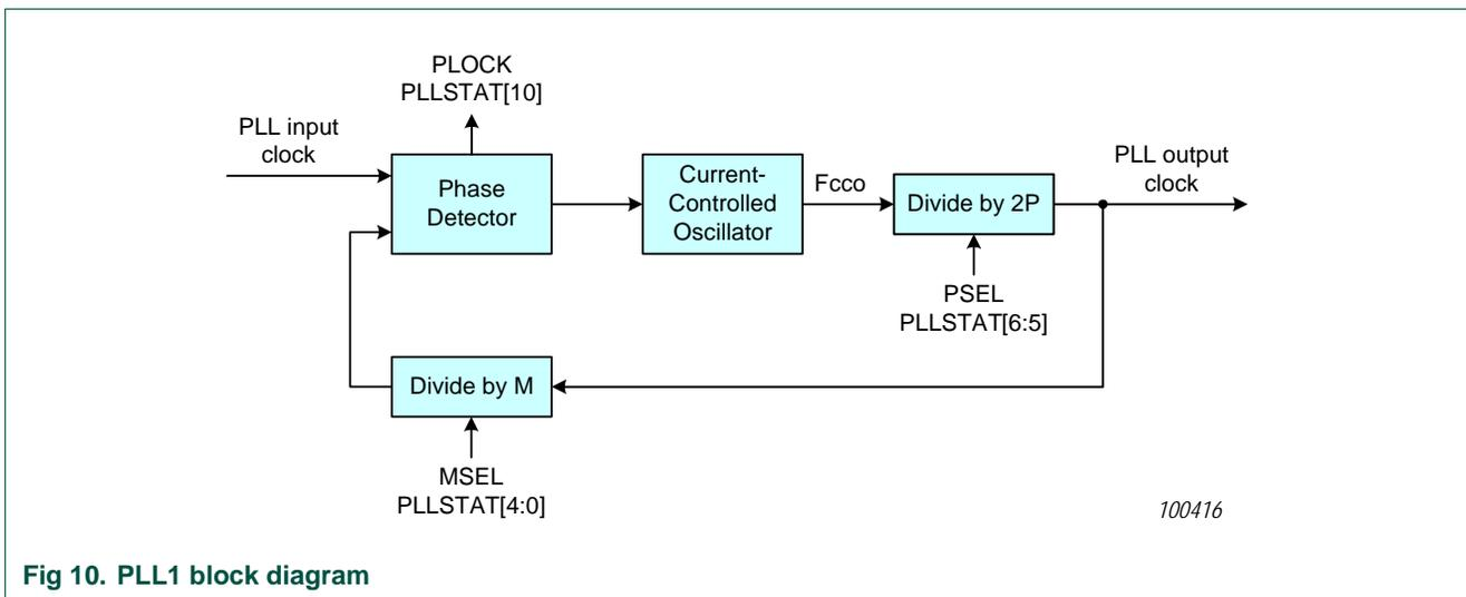
Fig 10. PLL1 block diagram
