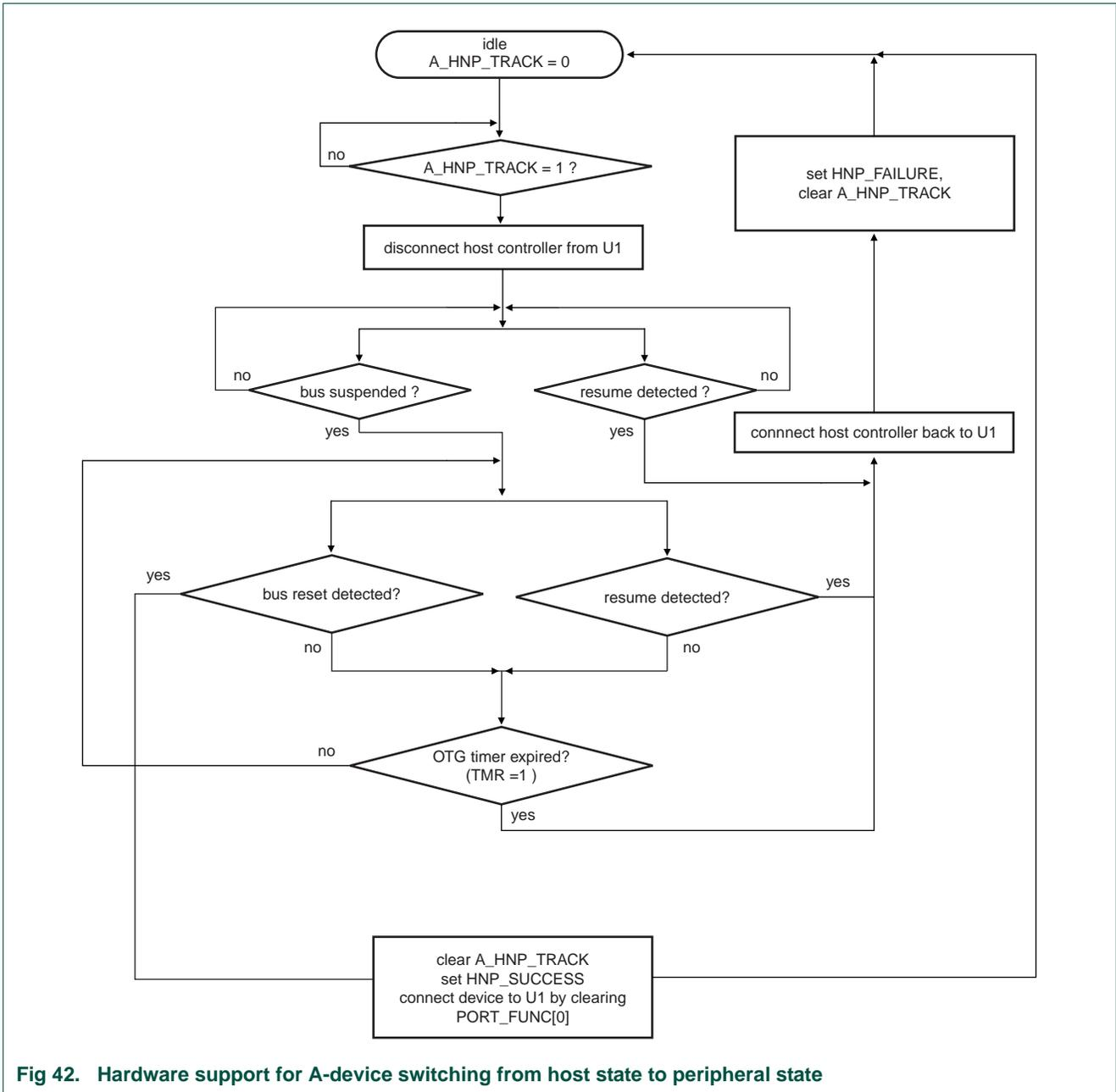
Fig 42. Hardware support for A-device switching from host state to peripheral state
