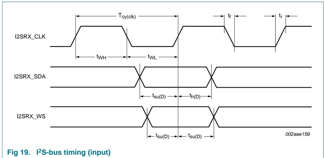
**Fig 19. I<sup>2</sup>S-bus timing (input)**
