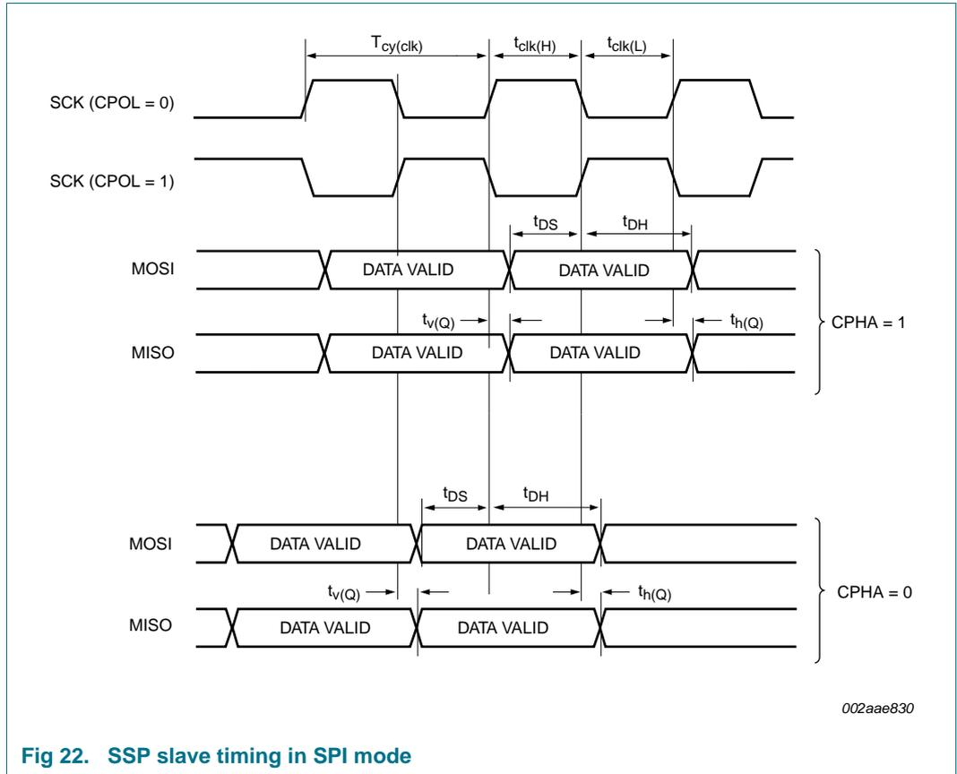
Fig 22. SSP slave timing in SPI mode
