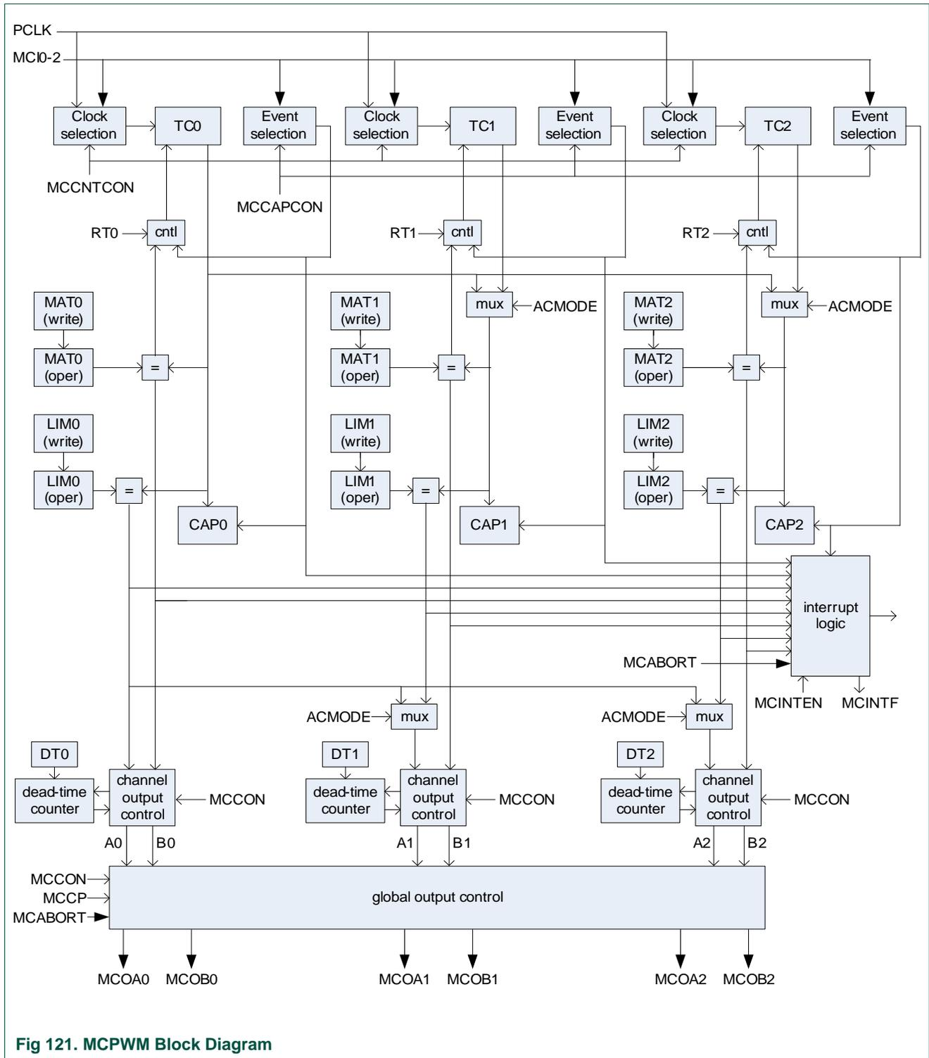
Fig 121. MCPWM Block Diagram
