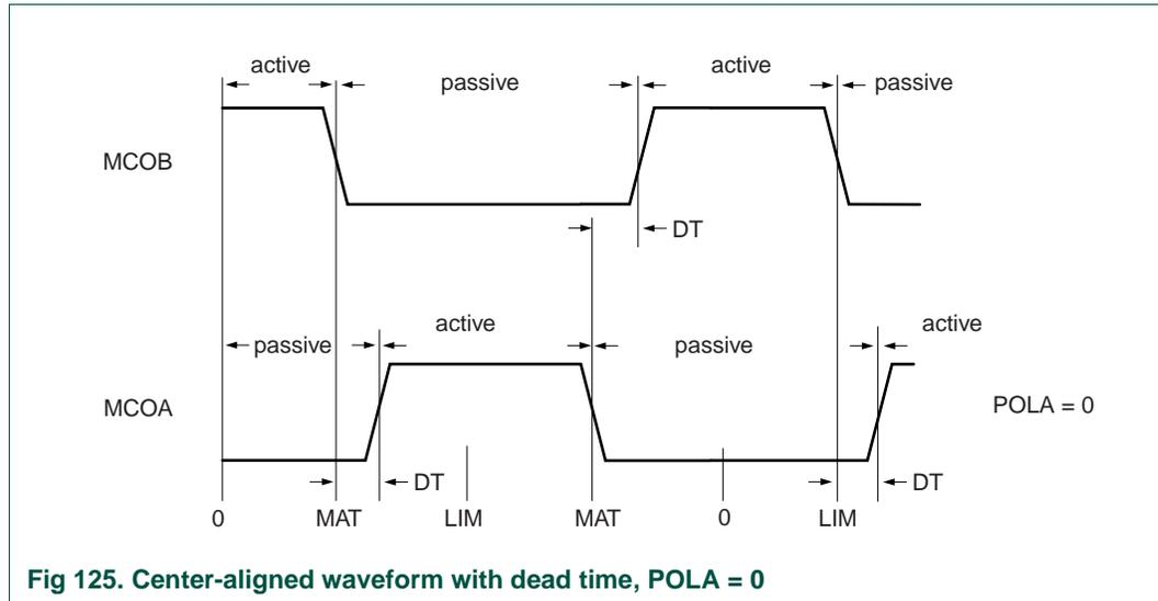
Fig 125. Center-aligned waveform with dead time, POLA = 0
