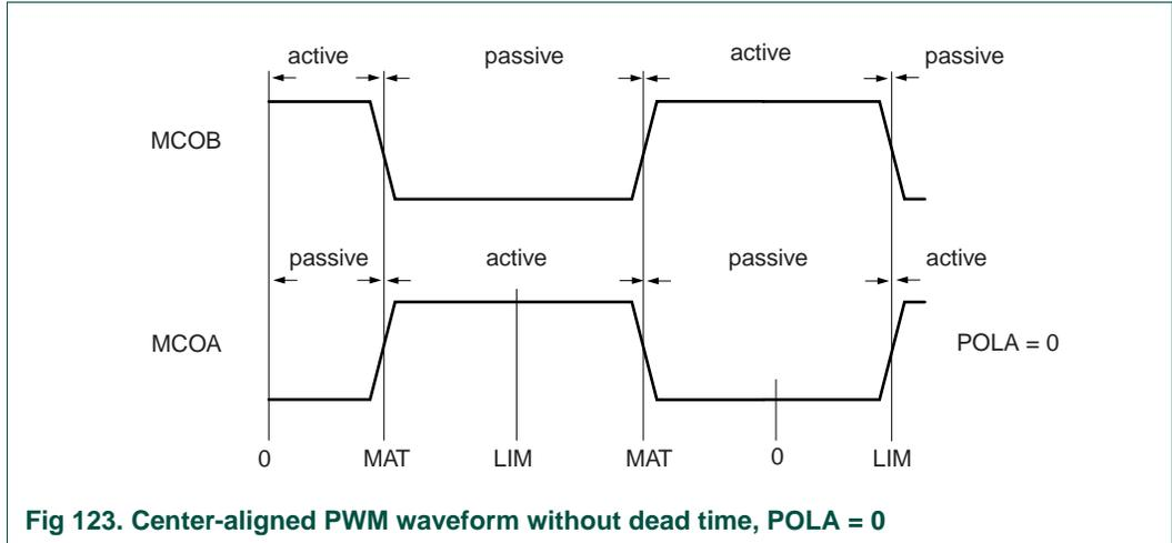
Fig 123. Center-aligned PWM waveform without dead time, POLA = 0
