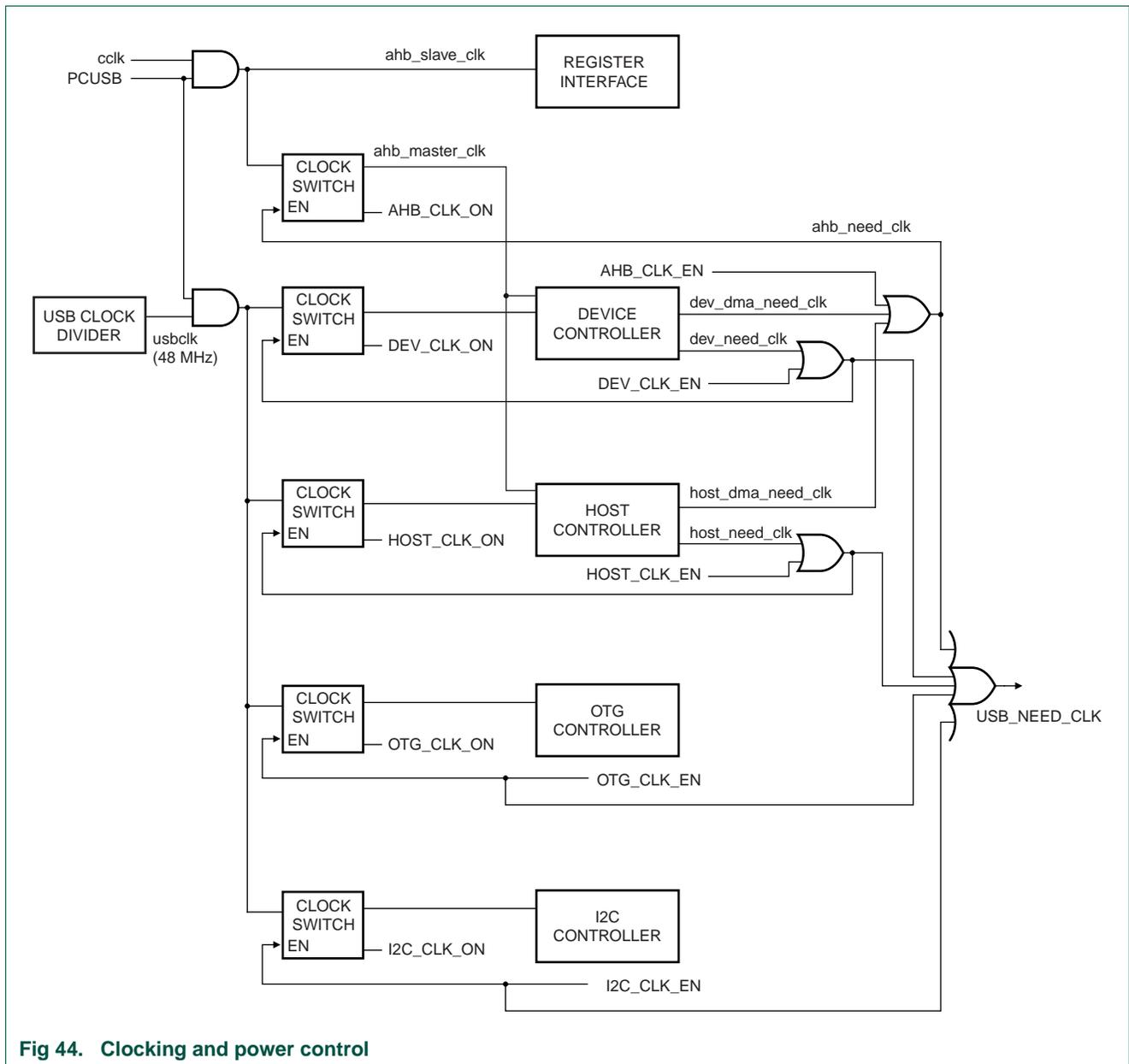
Fig 44. Clocking and power control
