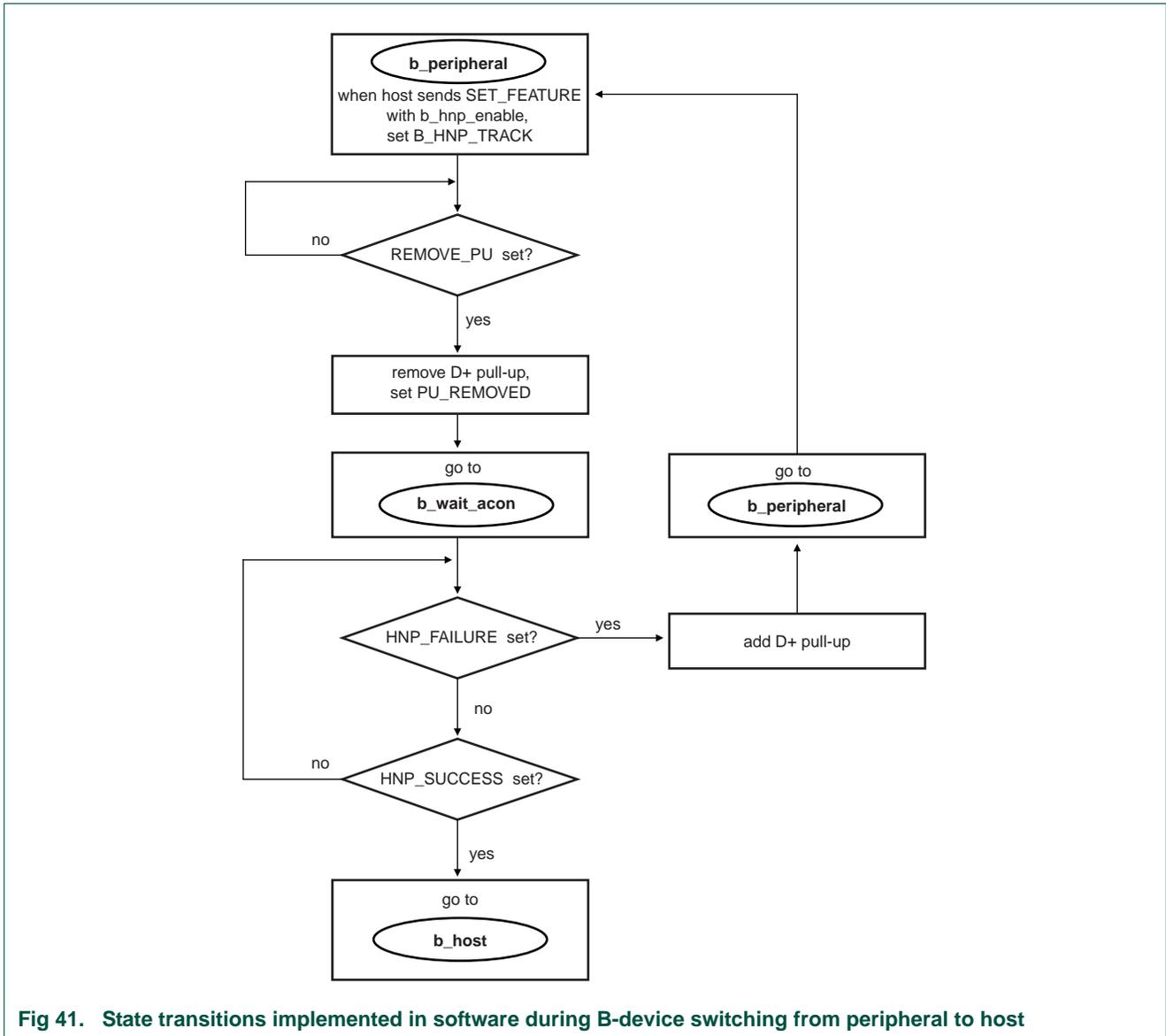
Fig 41. State transitions implemented in software during B-device switching from peripheral to host
