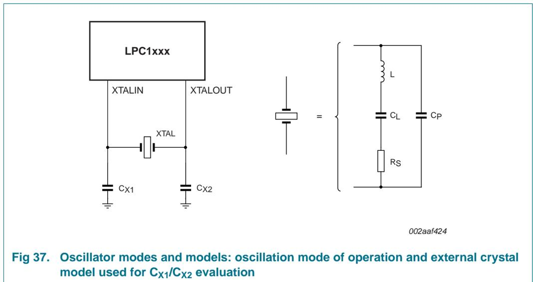
Fig 37. Oscillator modes and models: oscillation mode of operation and external crystal model used for  $C_{X1}/C_{X2}$  evaluation
