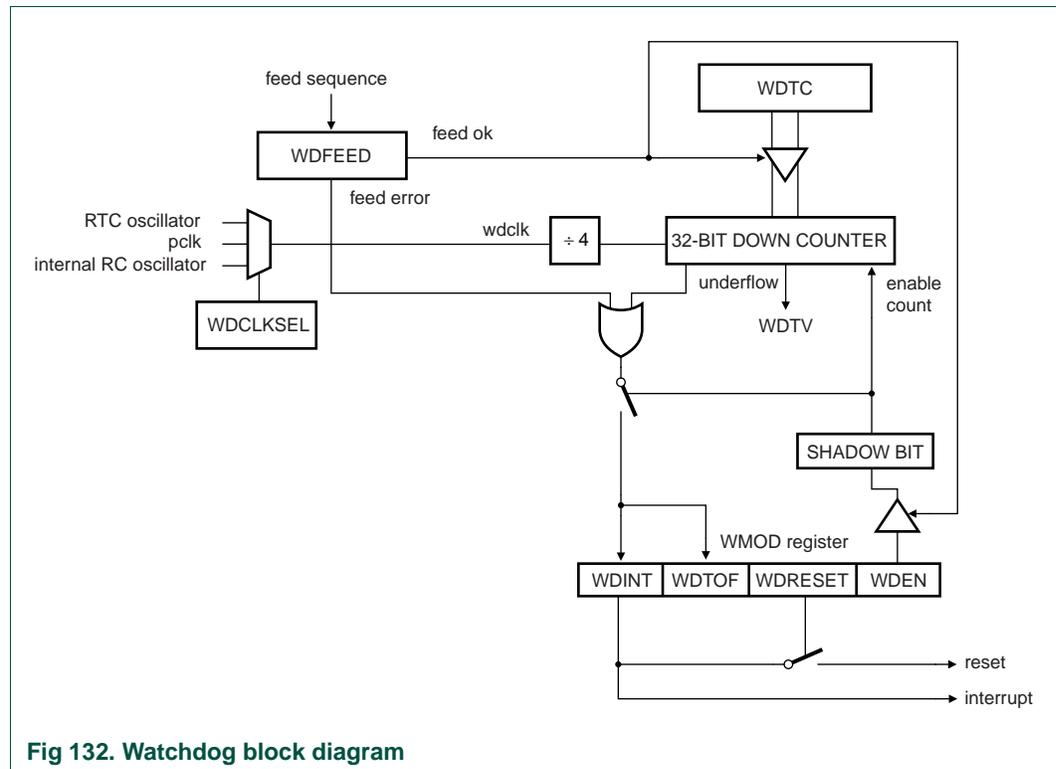
Fig 132. Watchdog block diagram
