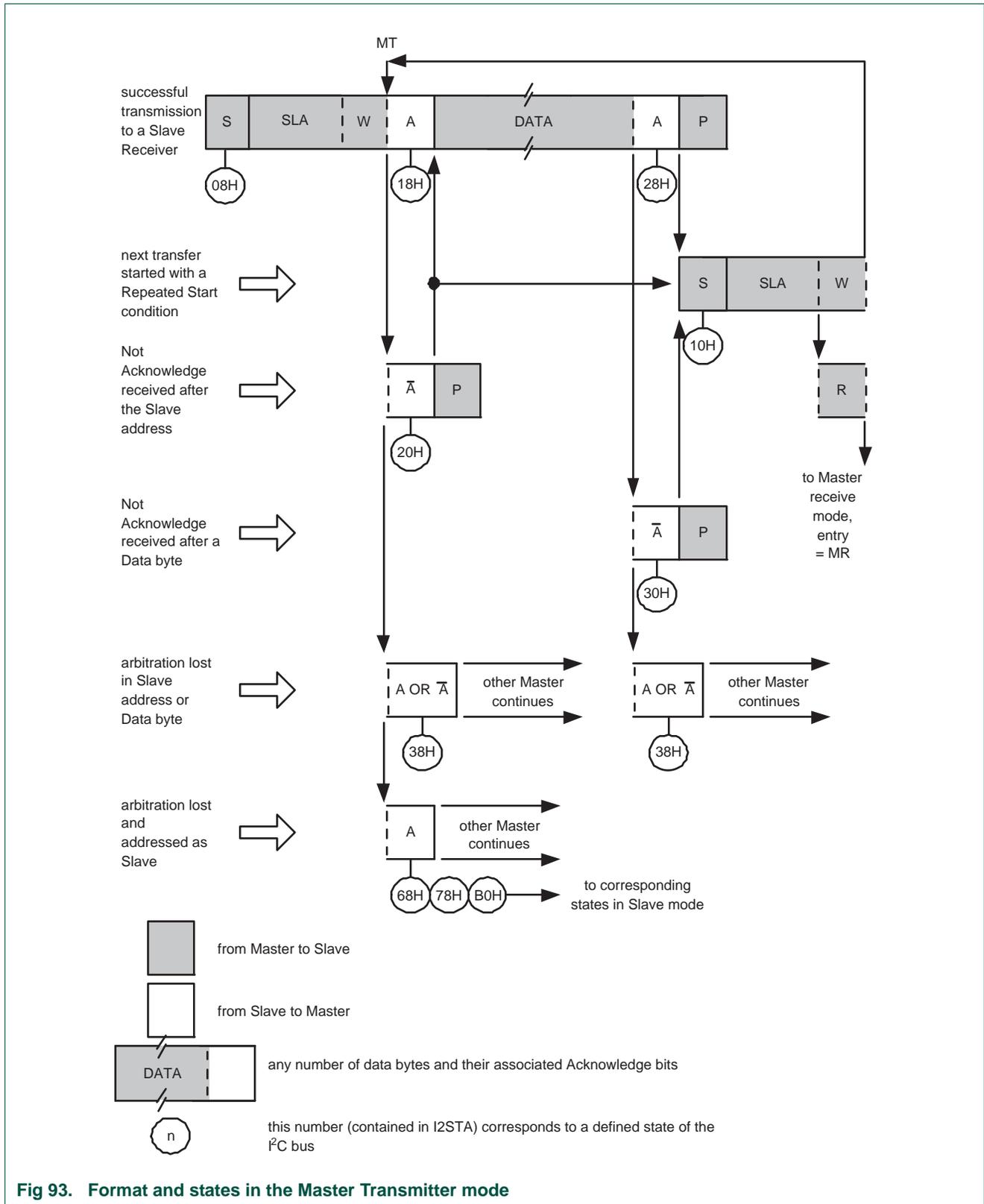
Fig 93. Format and states in the Master Transmitter mode
