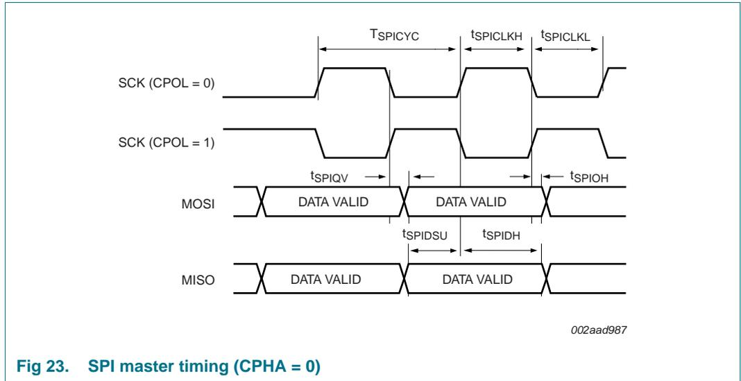
Fig 23. SPI master timing (CPHA = 0)
