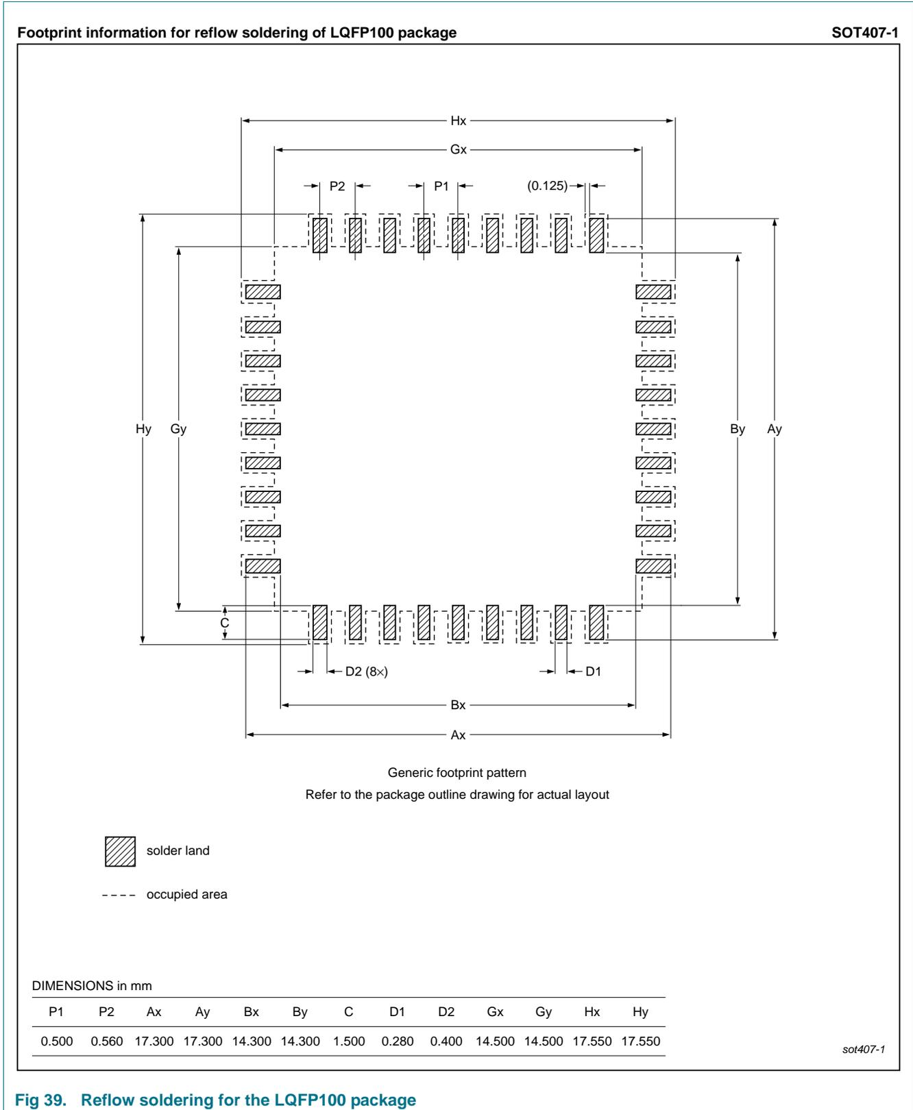
Fig 39. Reflow soldering for the LQFP100 package
