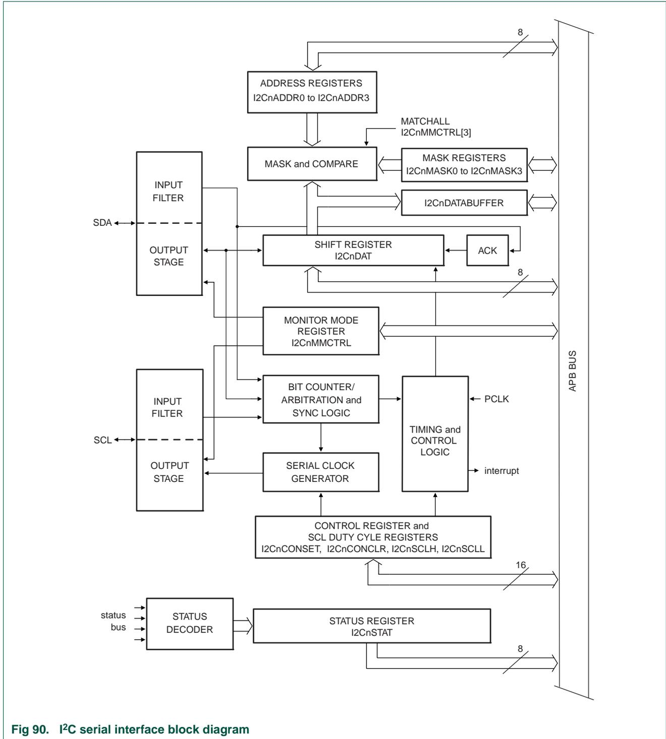
Fig 90. I<sup>2</sup>C serial interface block diagram
