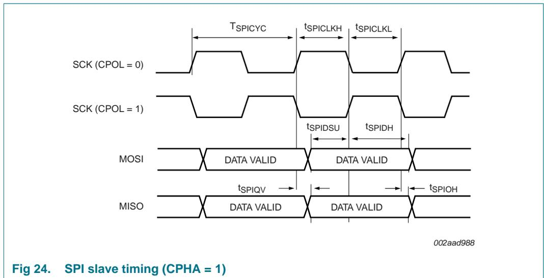
Fig 24. SPI slave timing (CPHA = 1)
