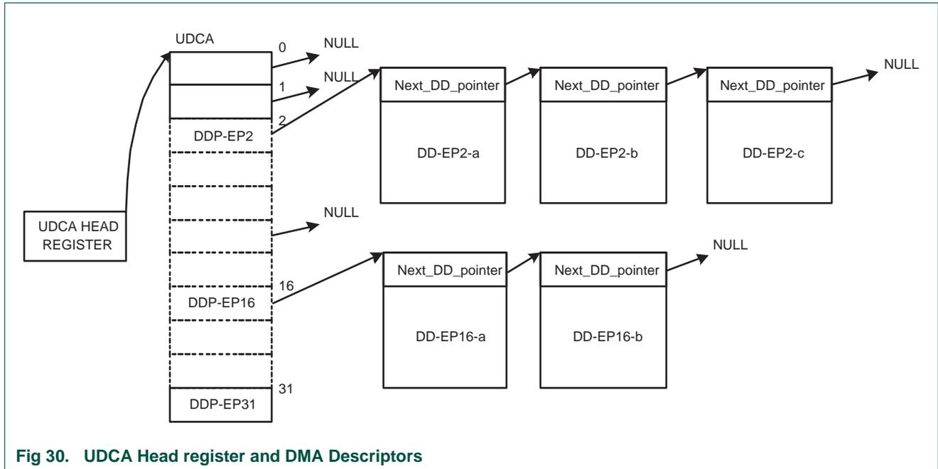
Fig 30. UDCA Head register and DMA Descriptors
