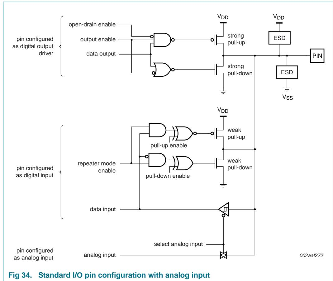
Fig 34. Standard I/O pin configuration with analog input
