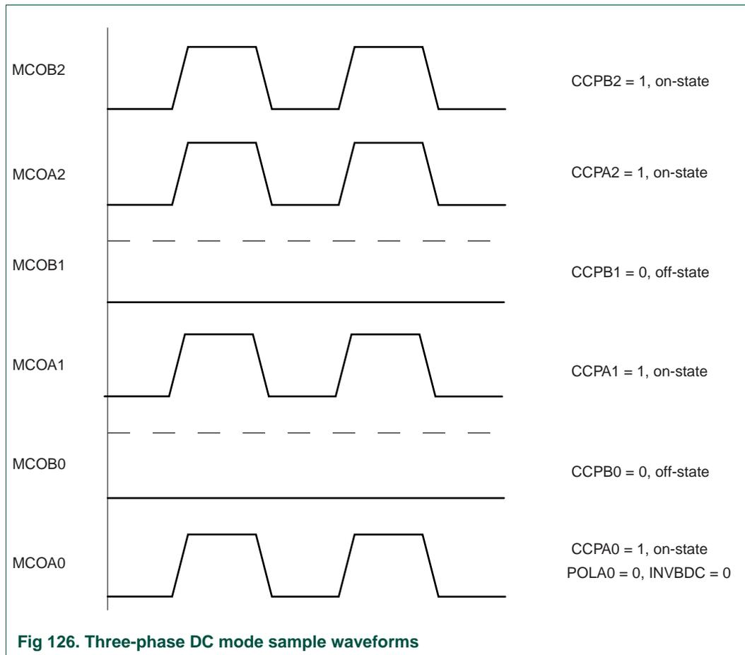
Fig 126. Three-phase DC mode sample waveforms
