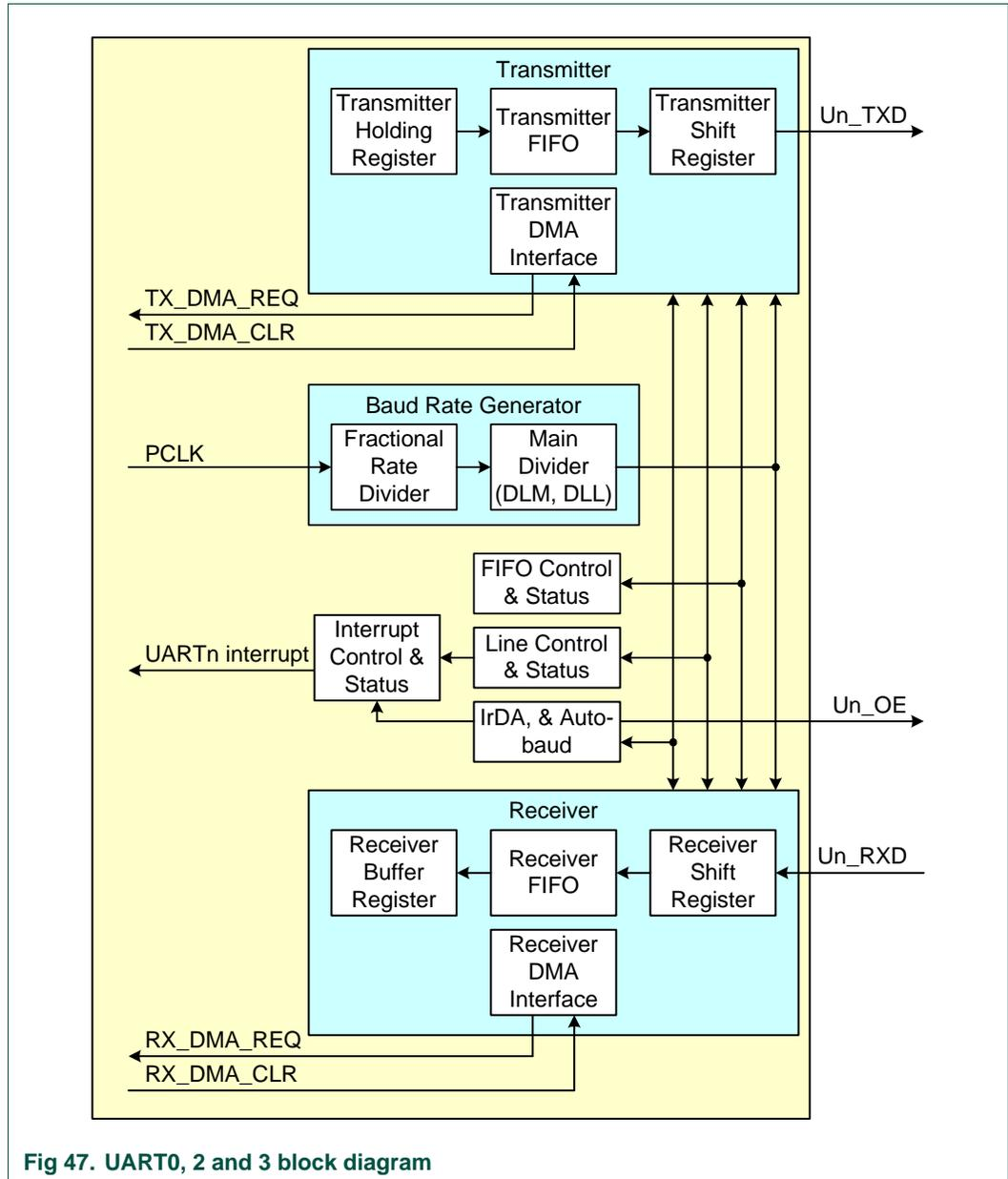
Fig 47. UART0, 2 and 3 block diagram
