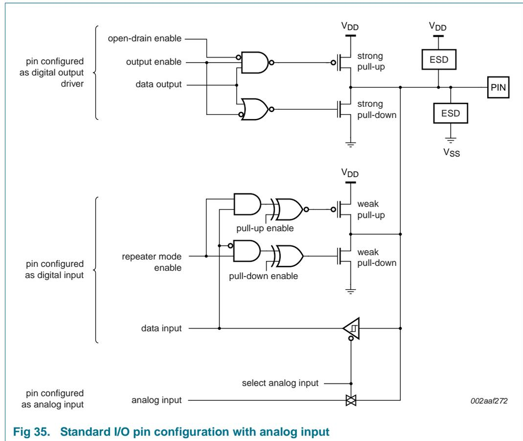
Fig 35. Standard I/O pin configuration with analog input
