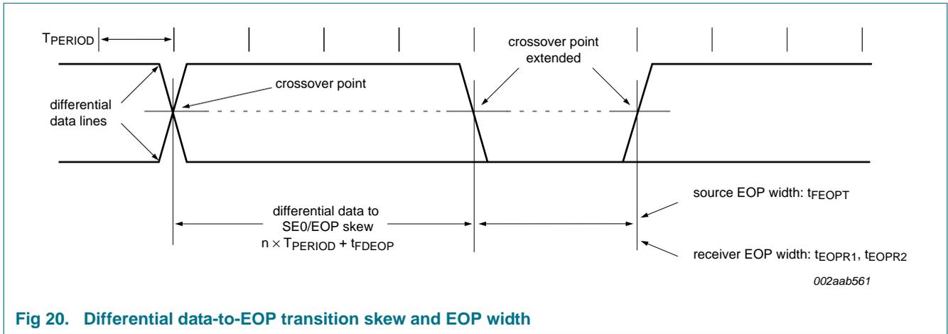
Fig 20. Differential data-to-EOP transition skew and EOP width
