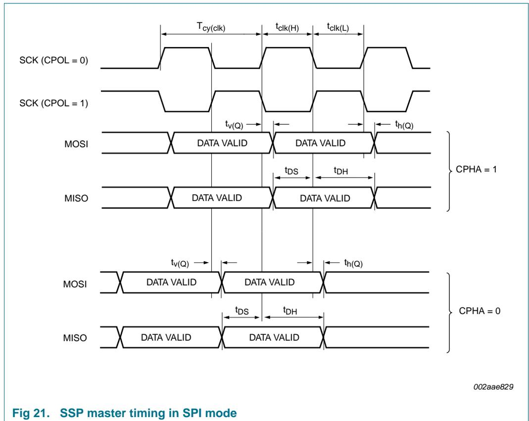
**Fig 21. SSP master timing in SPI mode**
