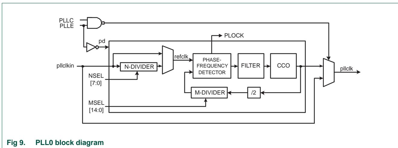
**Fig 9. PLL0 block diagram**
