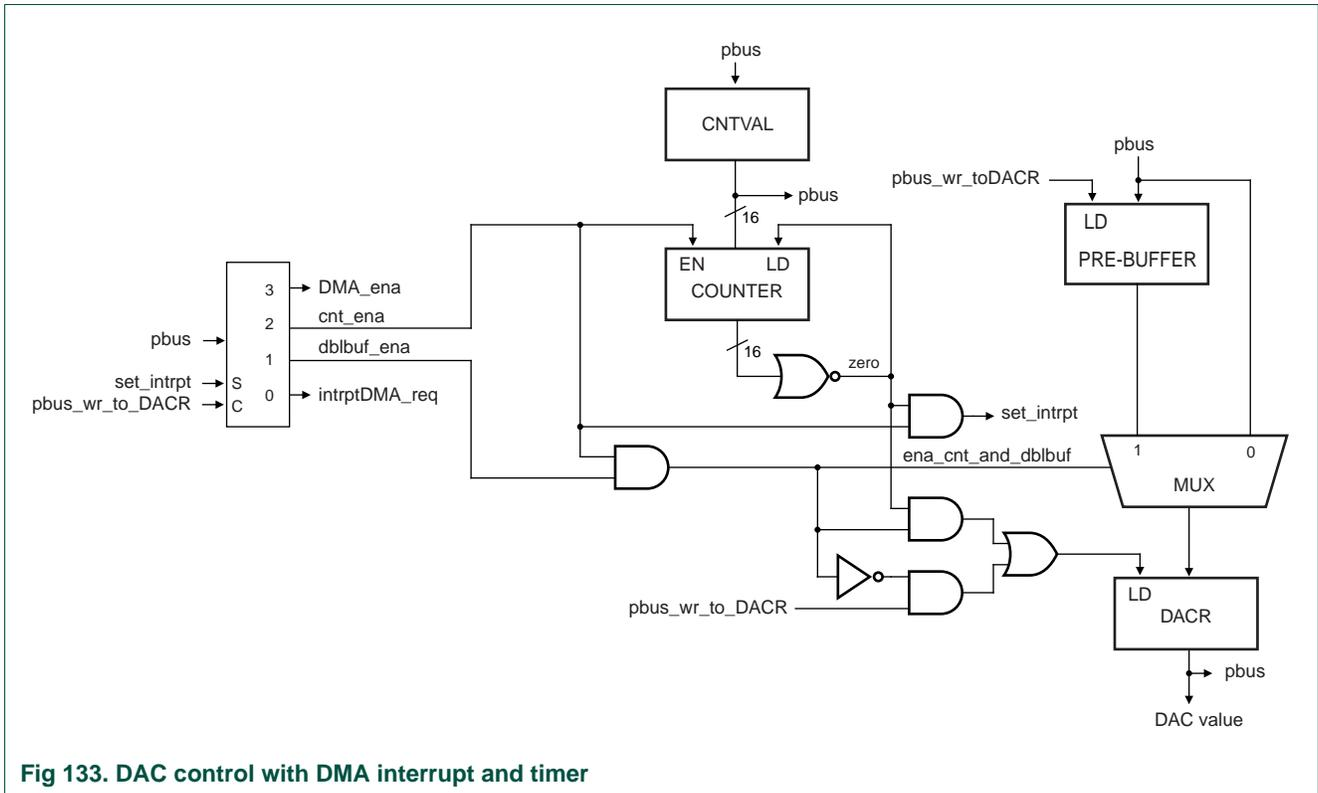
Fig 133. DAC control with DMA interrupt and timer
