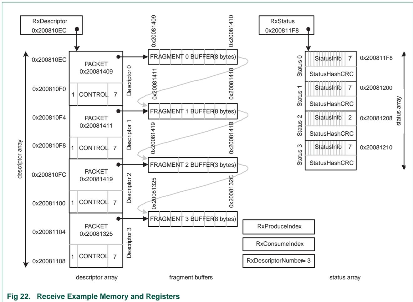
Fig 22. Receive Example Memory and Registers
