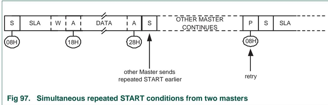
**Fig 97. Simultaneous repeated START conditions from two masters**
