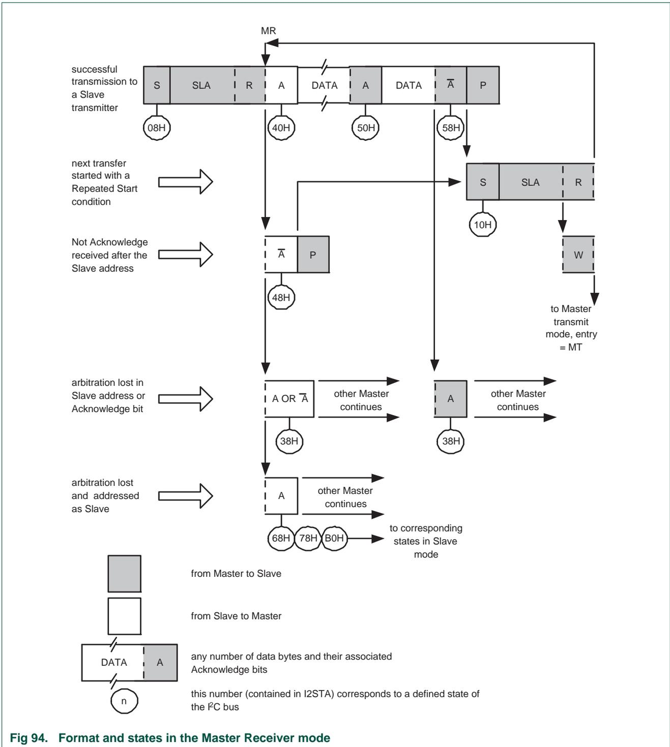
Fig 94. Format and states in the Master Receiver mode
