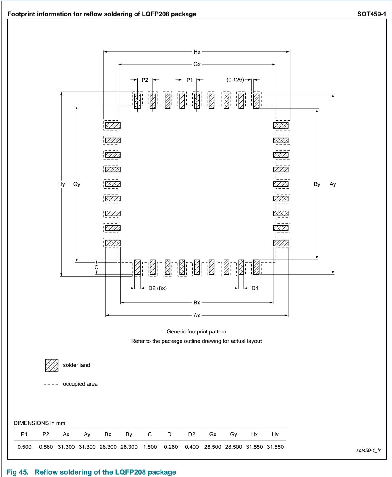
Fig 45. Reflow soldering of the LQFP208 package
