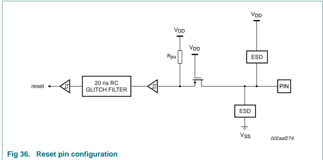
Fig 36. Reset pin configuration
