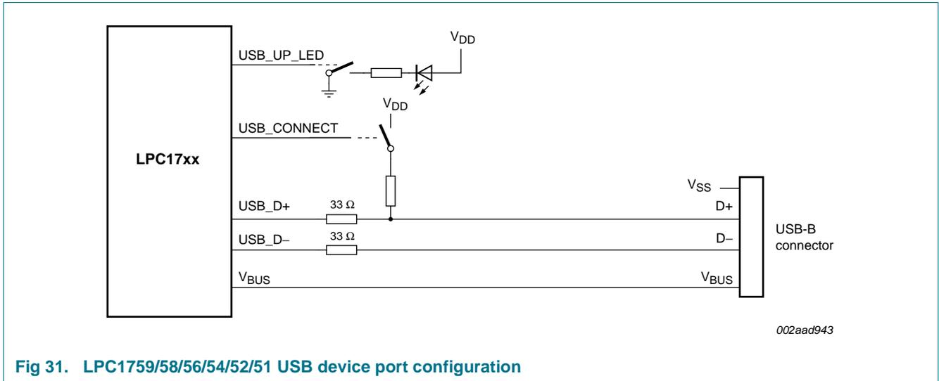
Fig 31. LPC1759/58/56/54/52/51 USB device port configuration
