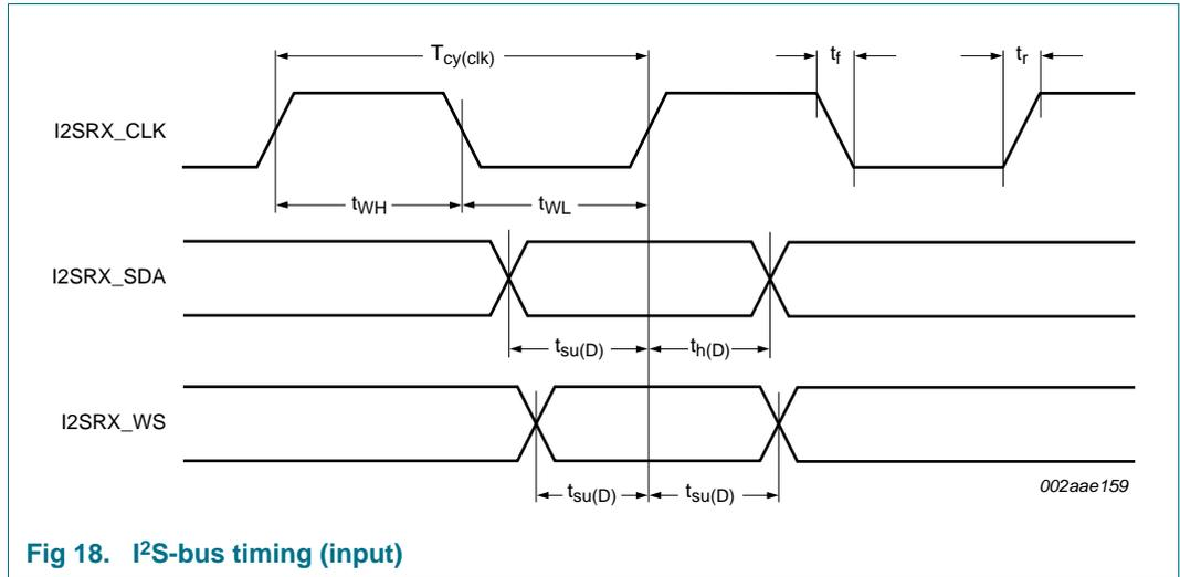
Fig 18. I<sup>2</sup>S-bus timing (input)
