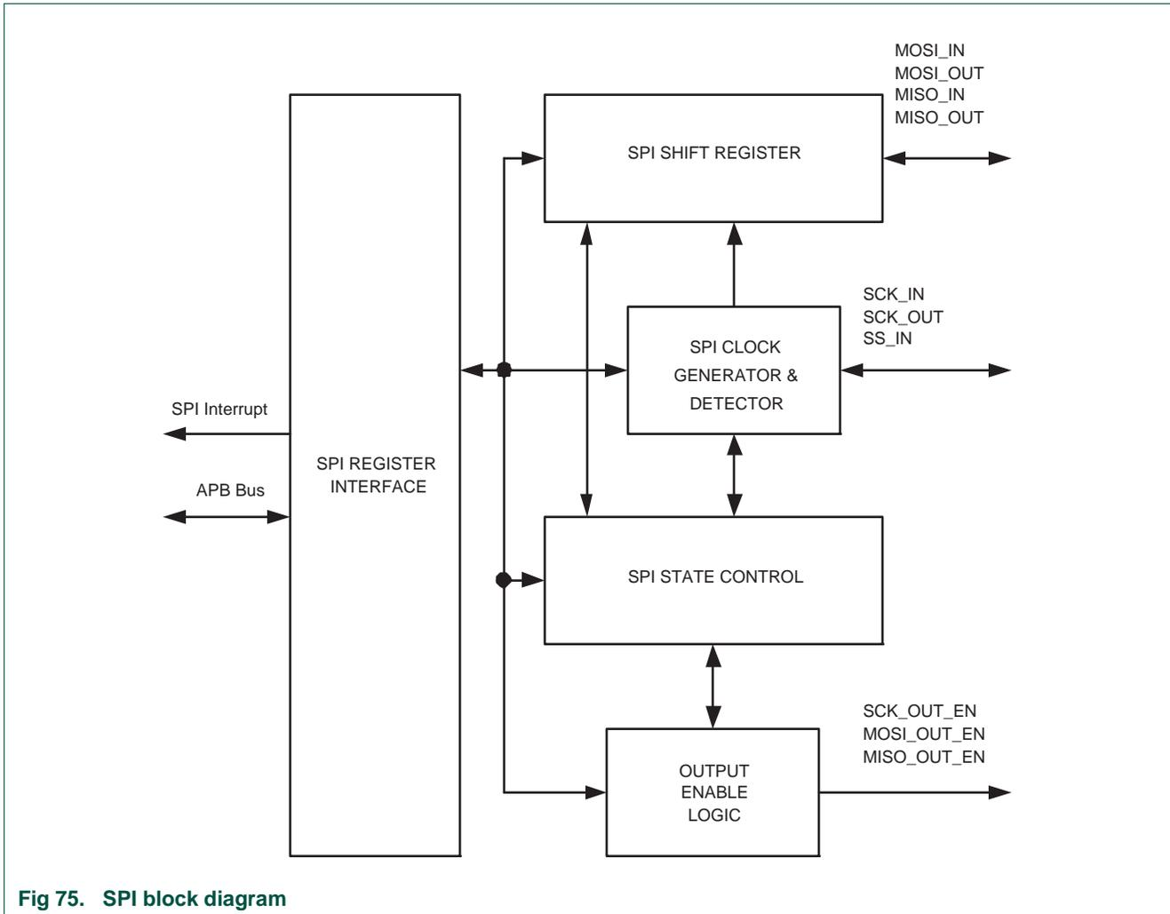
Fig 75. SPI block diagram
