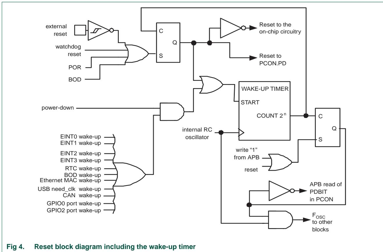
Fig 4. Reset block diagram including the wake-up timer
