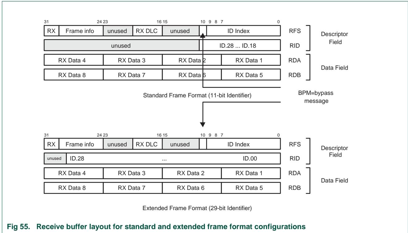
Fig 55. Receive buffer layout for standard and extended frame format configurations
