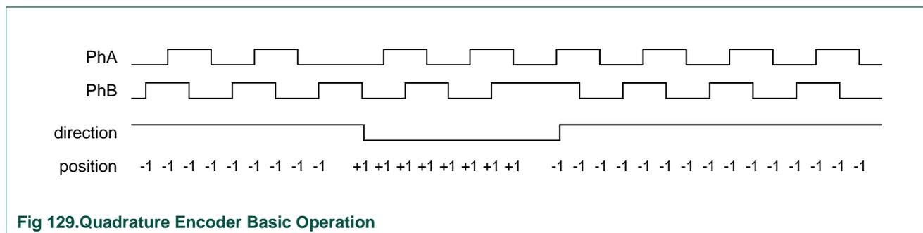
**Fig 129. Quadrature Encoder Basic Operation**
