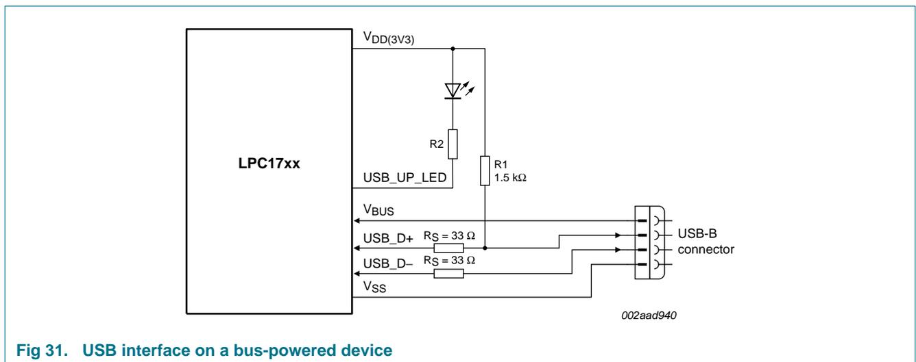
Fig 31. USB interface on a bus-powered device
