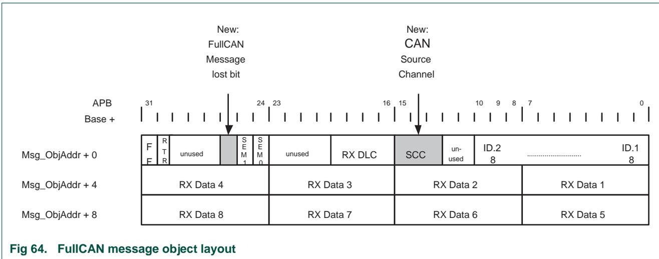
Fig 64. FullCAN message object layout
