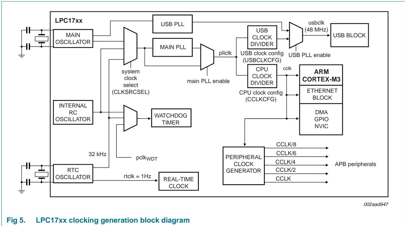
Fig 5. LPC17xx clocking generation block diagram
