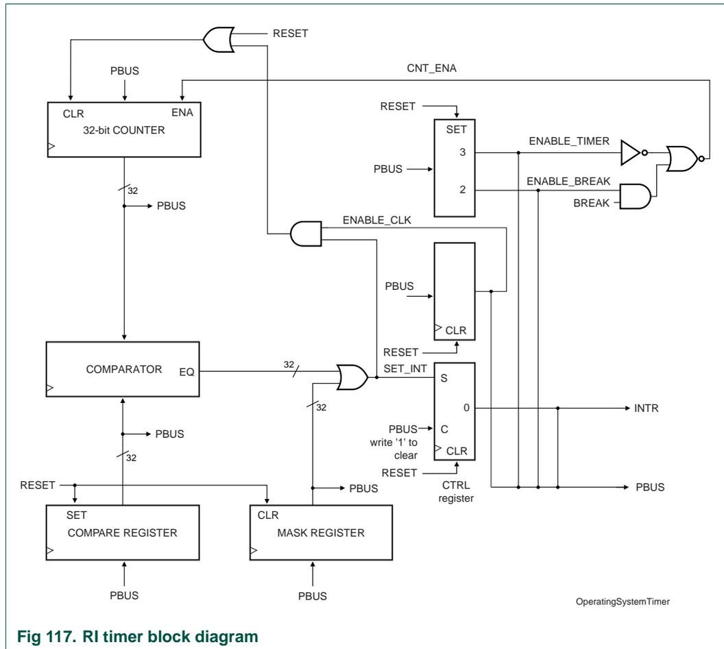
Fig 117. RIT timer block diagram
