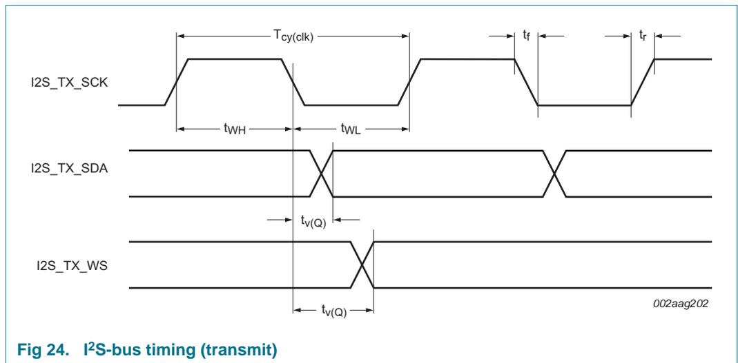
**Fig 24. I<sup>2</sup>S-bus timing (transmit)**
