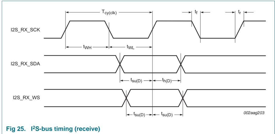
Fig 25. I2S-bus timing (receive)
