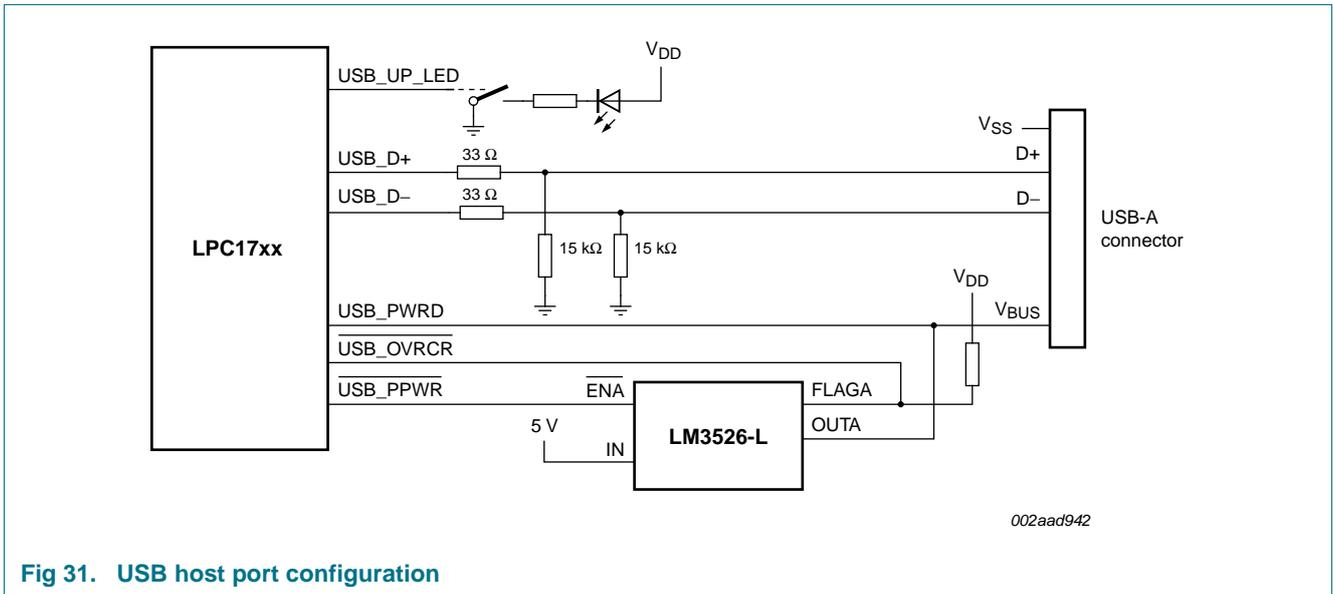
Fig 31. USB host port configuration
