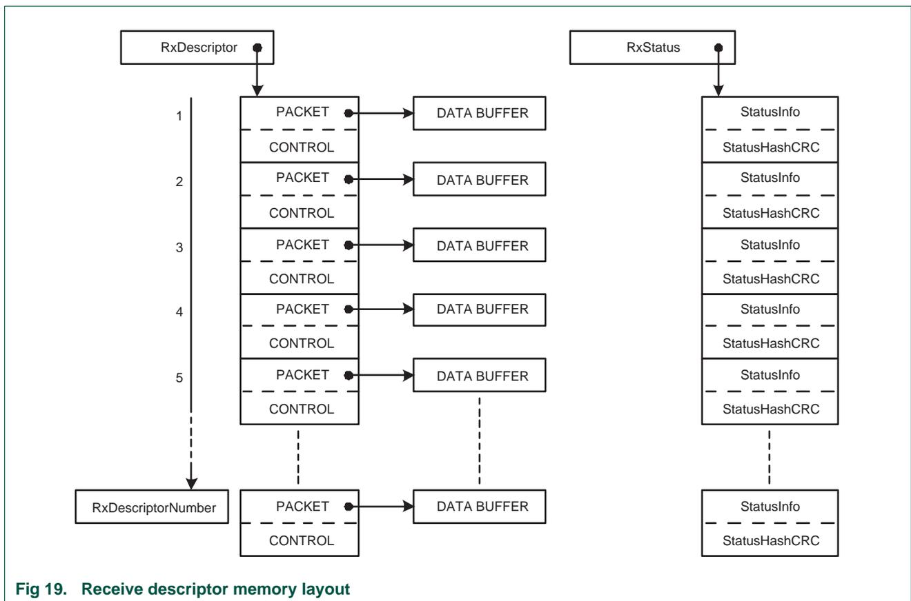
Fig 19. Receive descriptor memory layout
