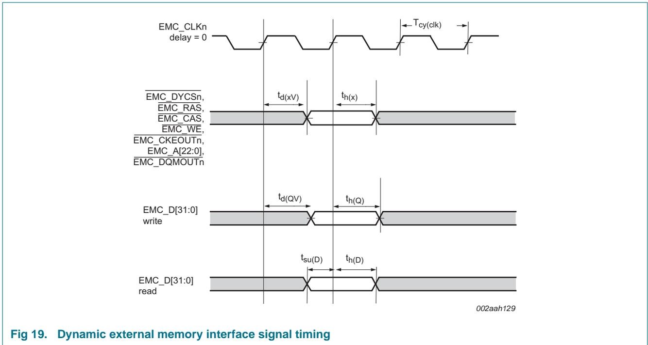
Fig 19. Dynamic external memory interface signal timing
