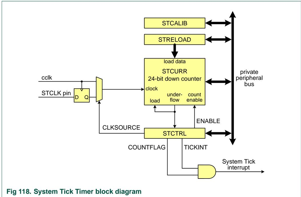
Fig 118. System Tick Timer block diagram
