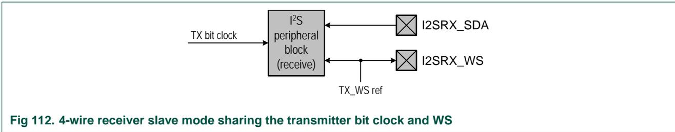
Fig 112. 4-wire receiver slave mode sharing the transmitter bit clock and WS
