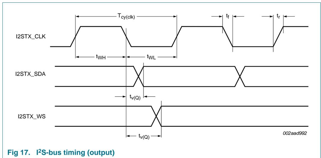
Fig 17. I<sup>2</sup>S-bus timing (output)
