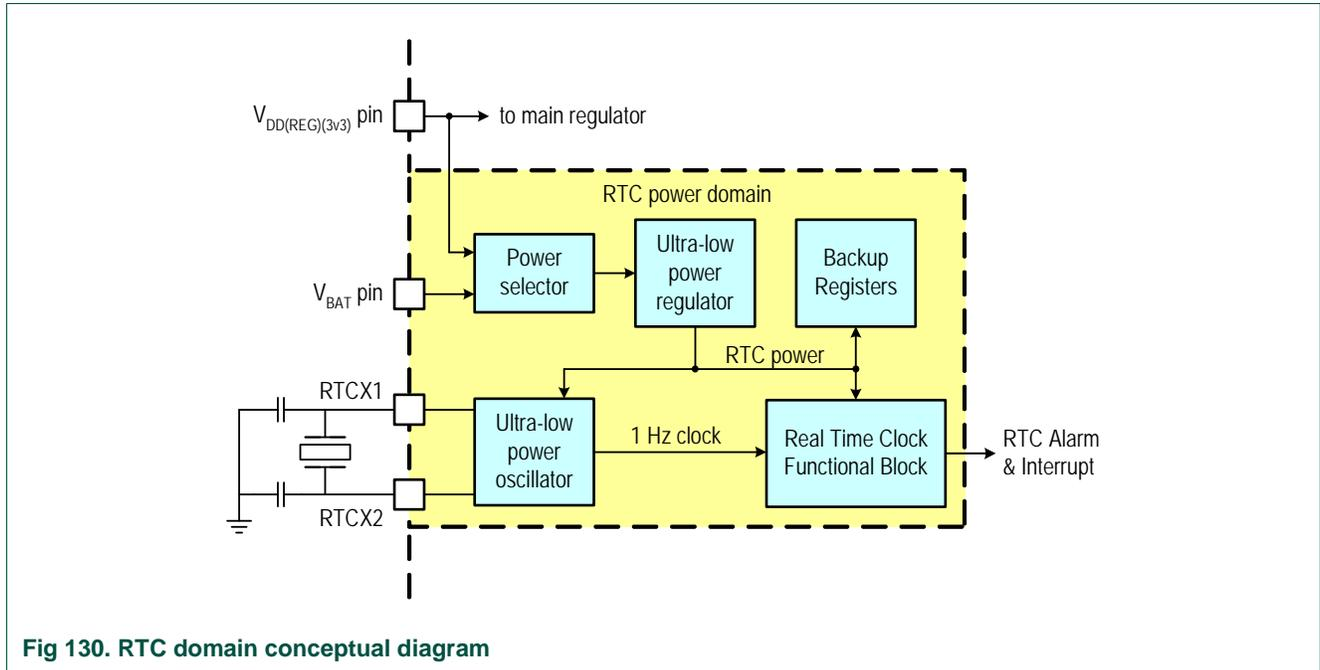
Fig 130. RTC domain conceptual diagram
