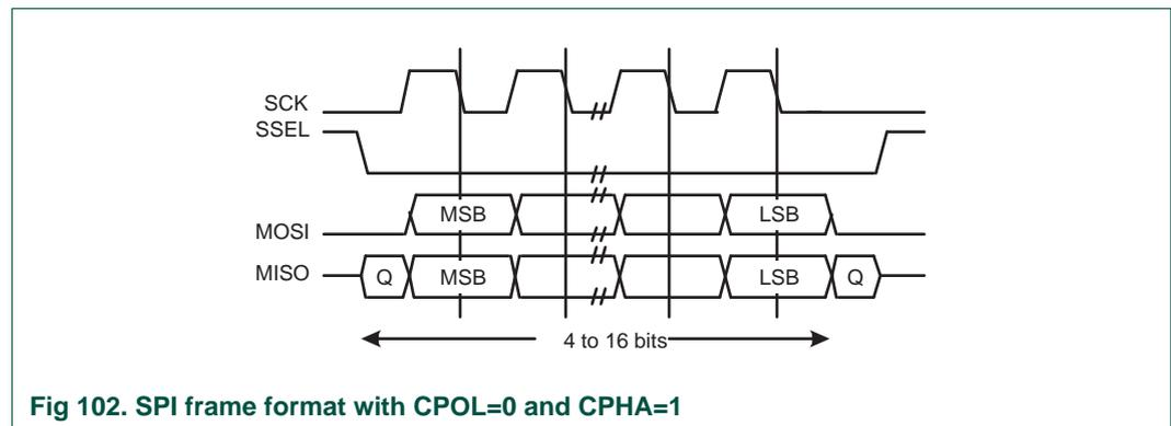
**Fig 102. SPI frame format with CPOL=0 and CPHA=1**
