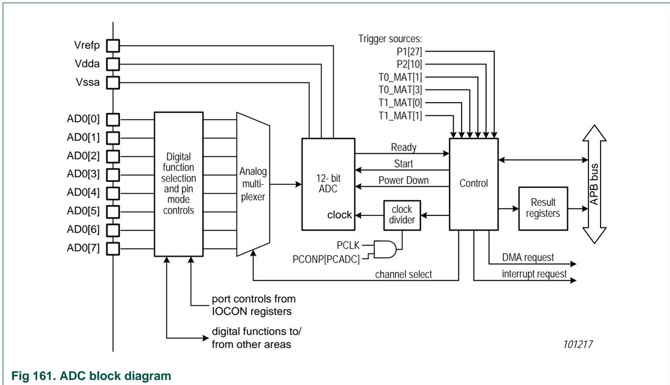
Fig 161. ADC block diagram
