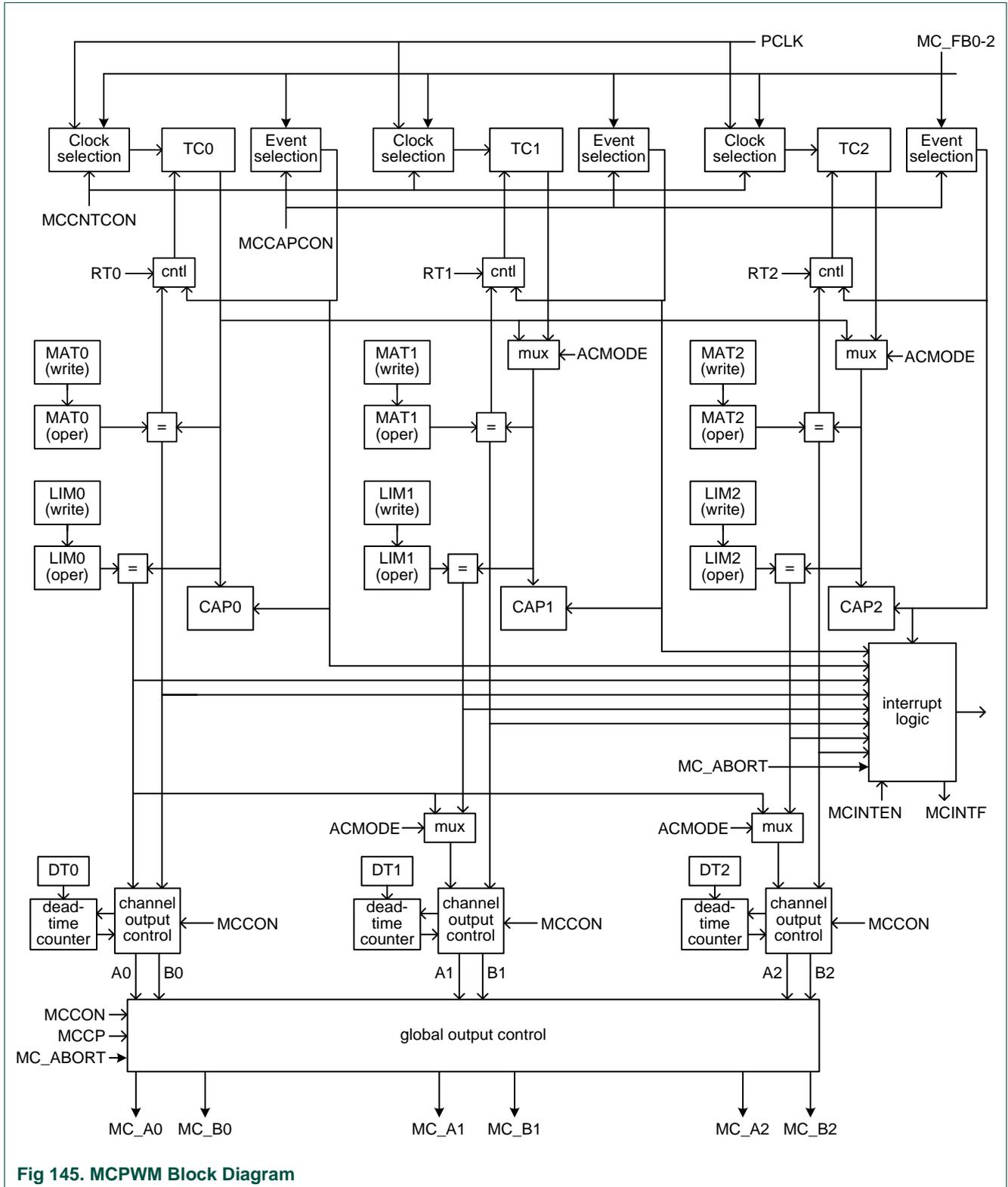
Fig 145. MCPWM Block Diagram
