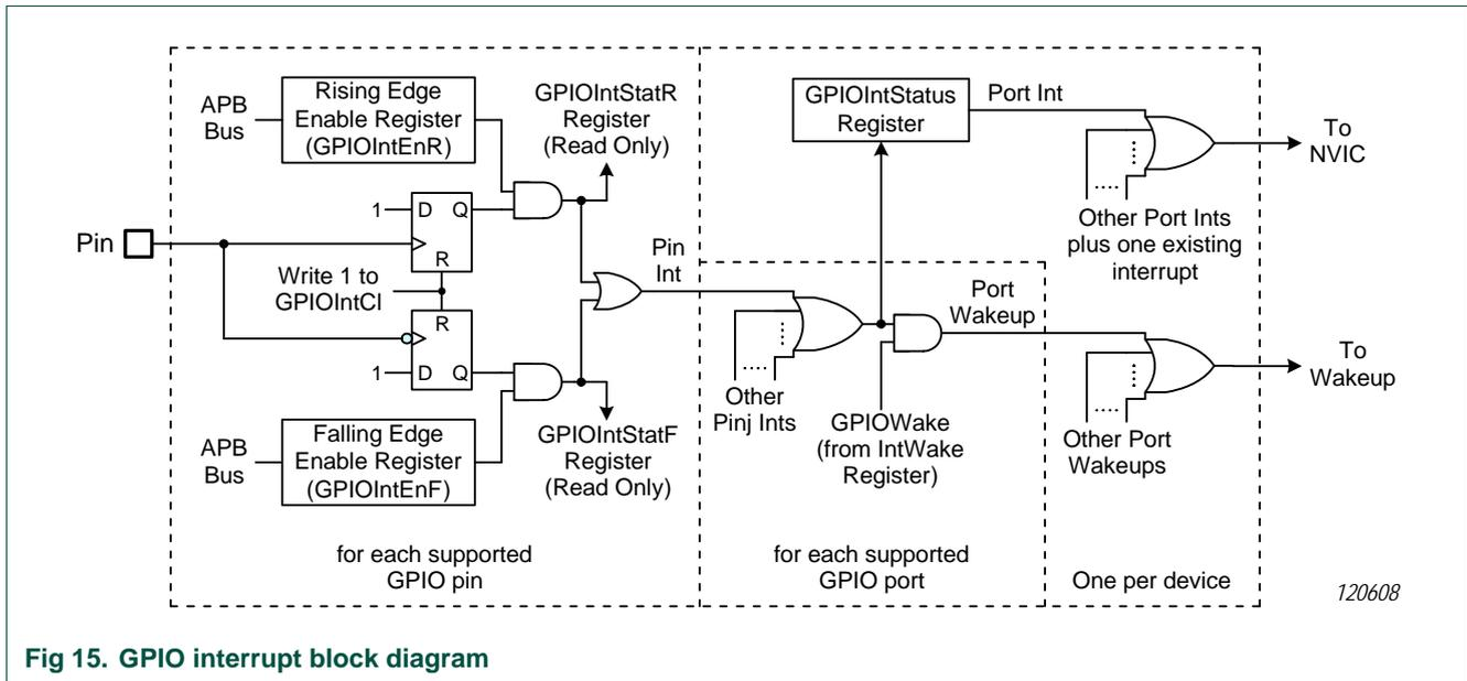
Fig 15. GPIO interrupt block diagram
