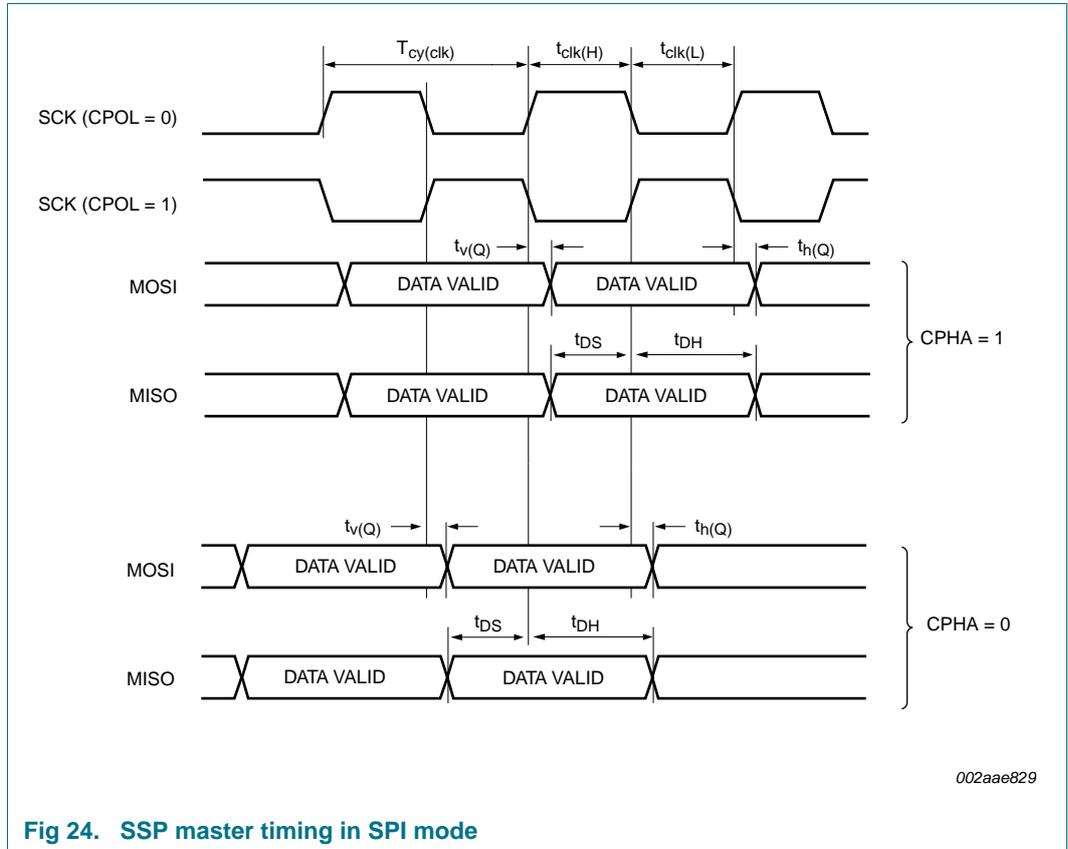
Fig 24. SSP master timing in SPI mode
