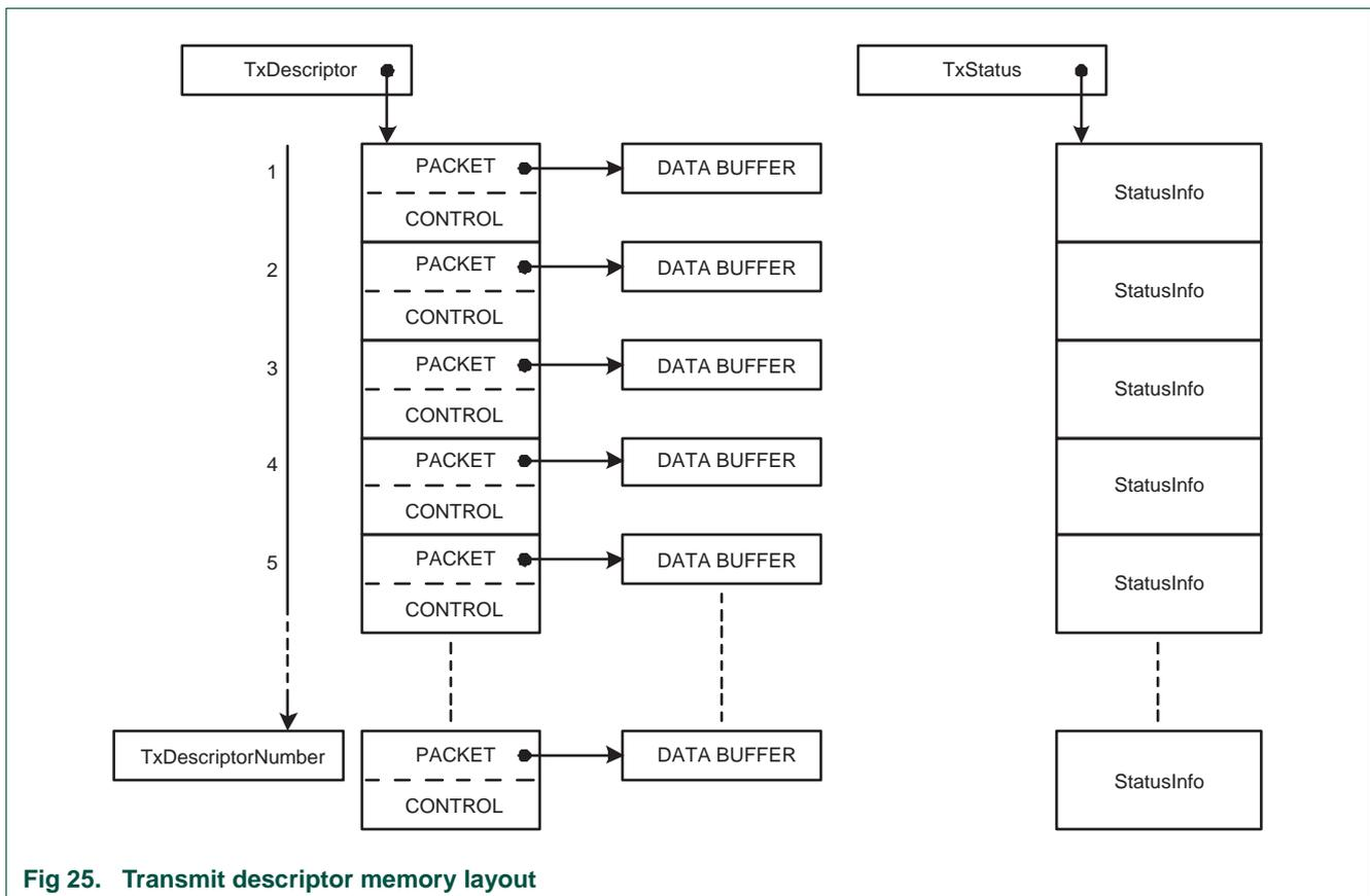
Fig 25. Transmit descriptor memory layout
