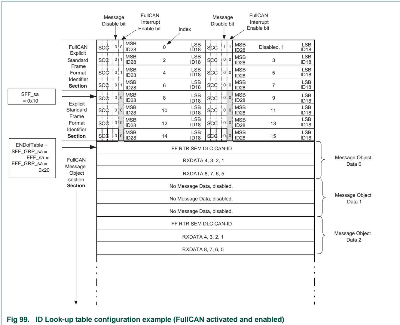
Fig 99. ID Look-up table configuration example (FullCAN activated and enabled)
