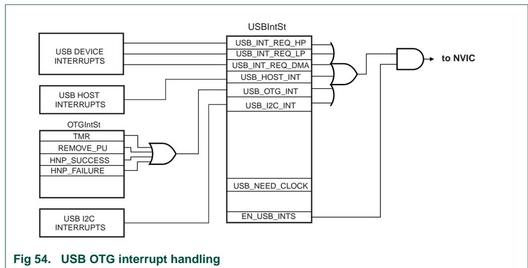
Fig 54. USB OTG interrupt handling
