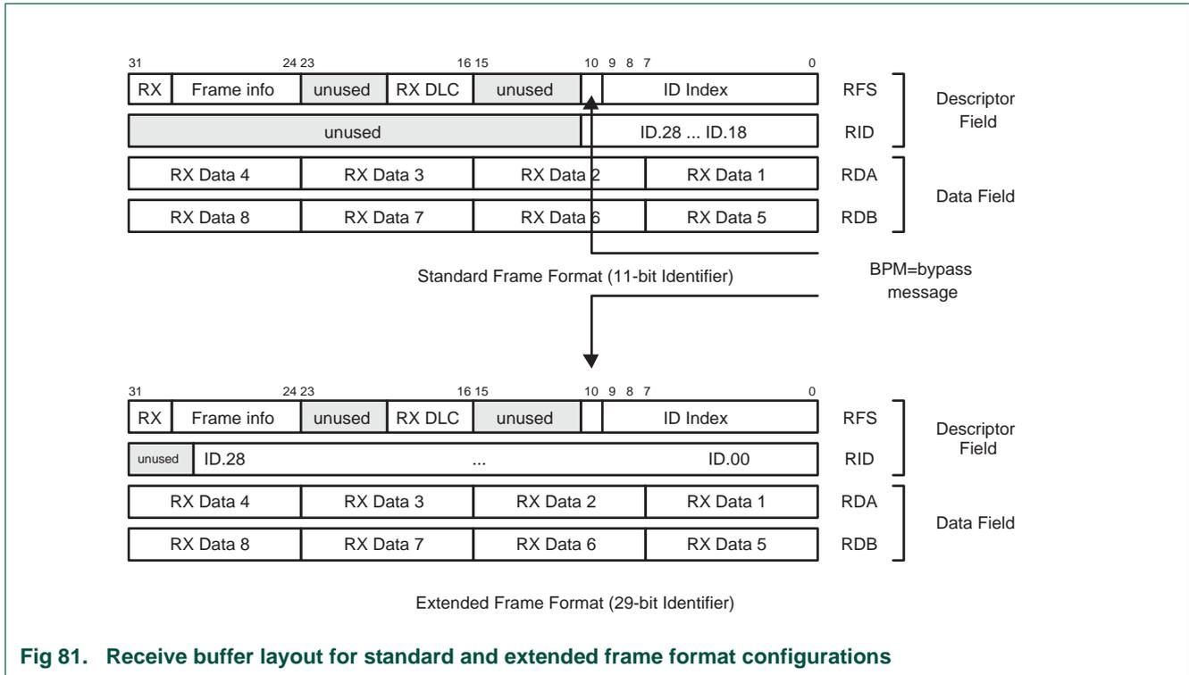
Fig 81. Receive buffer layout for standard and extended frame format configurations
