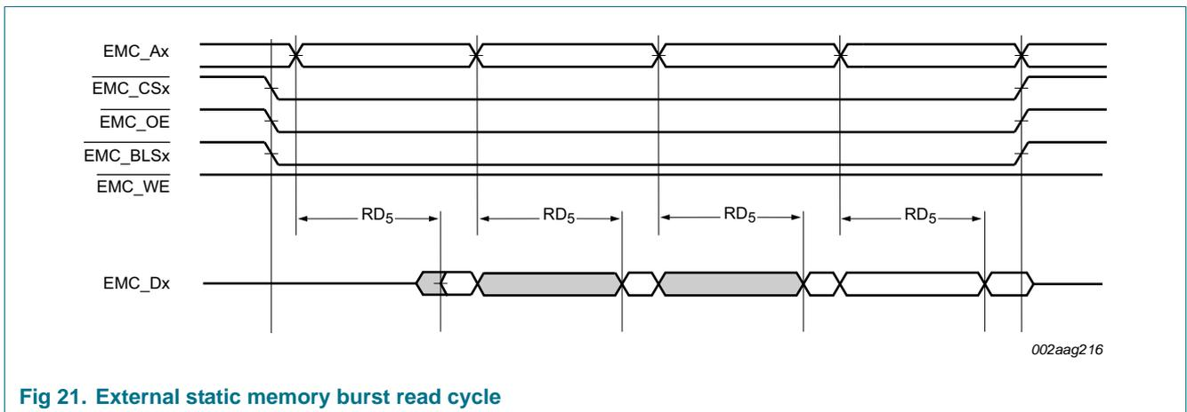
Fig 21. External static memory burst read cycle
