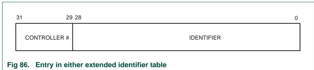
**Fig 86. Entry in either extended identifier table**
