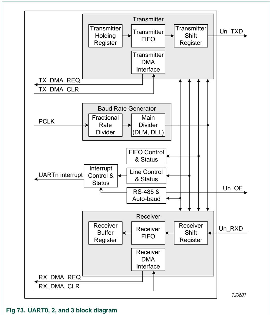
Fig 73. UART0, 2, and 3 block diagram
