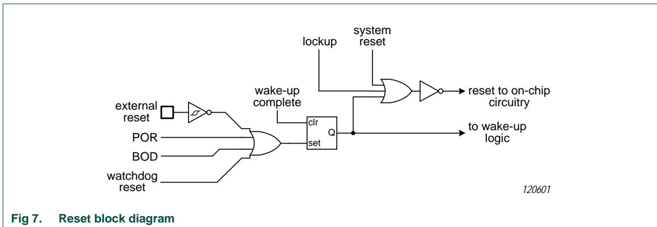
**Fig 7. Reset block diagram**
