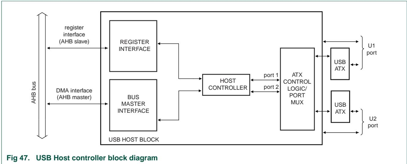
**Fig 47. USB Host controller block diagram**
