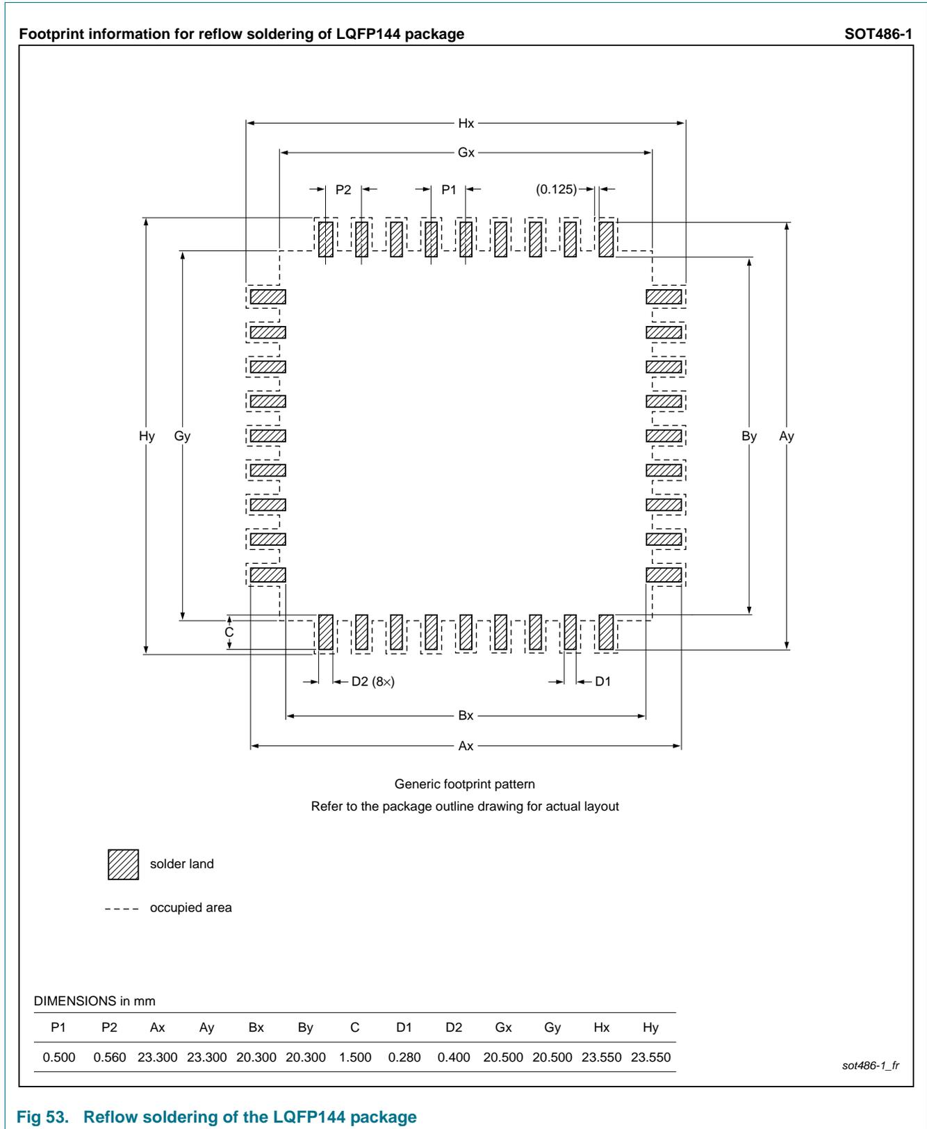
**Fig 53. Reflow soldering of the LQFP144 package**
