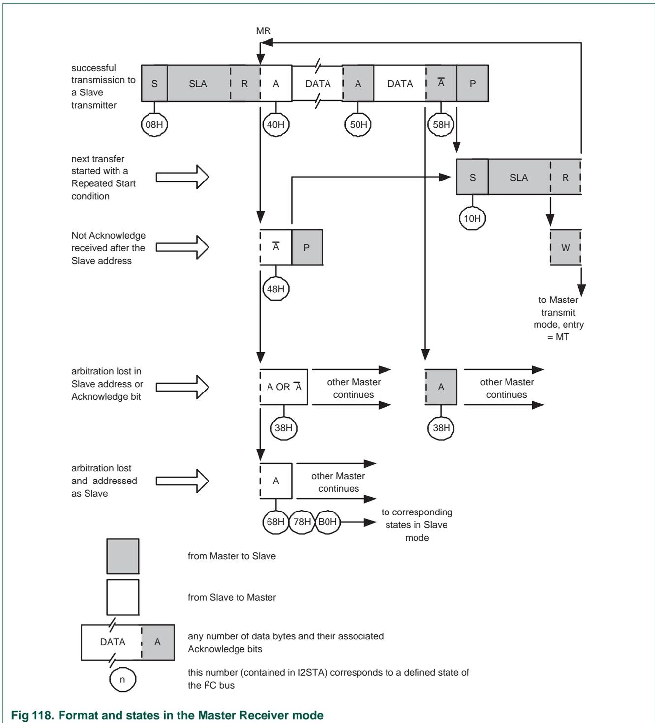
Fig 118. Format and states in the Master Receiver mode
