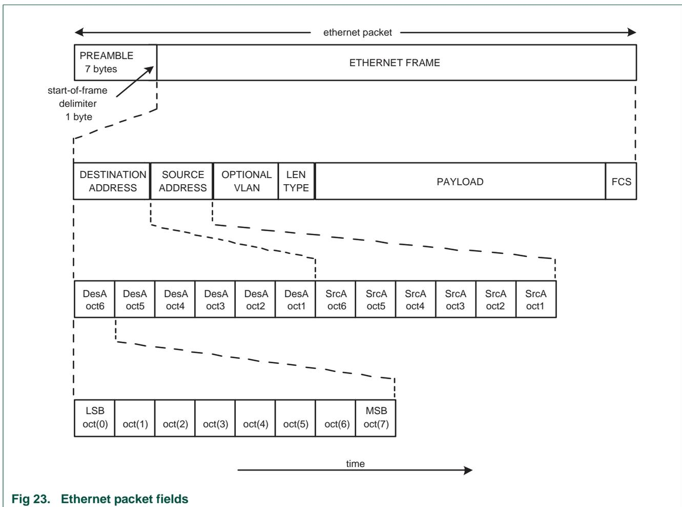
Fig 23. Ethernet packet fields
