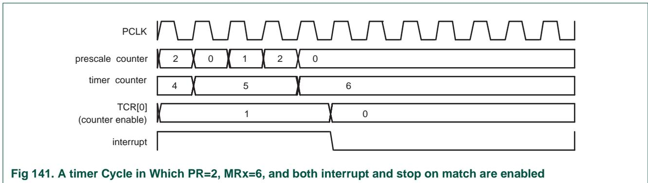
Fig 141. A timer Cycle in Which PR=2, MRx=6, and both interrupt and stop on match are enabled
