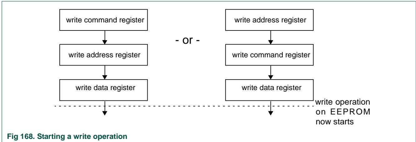
**Fig 168. Starting a write operation**
