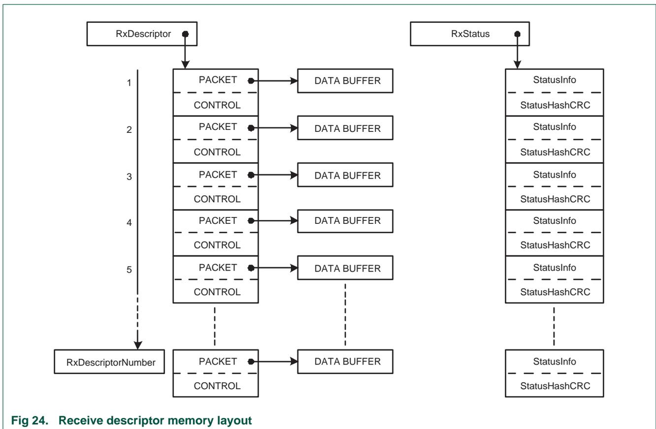
Fig 24. Receive descriptor memory layout
