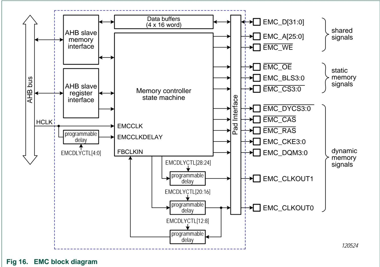
Fig 16. EMC block diagram
