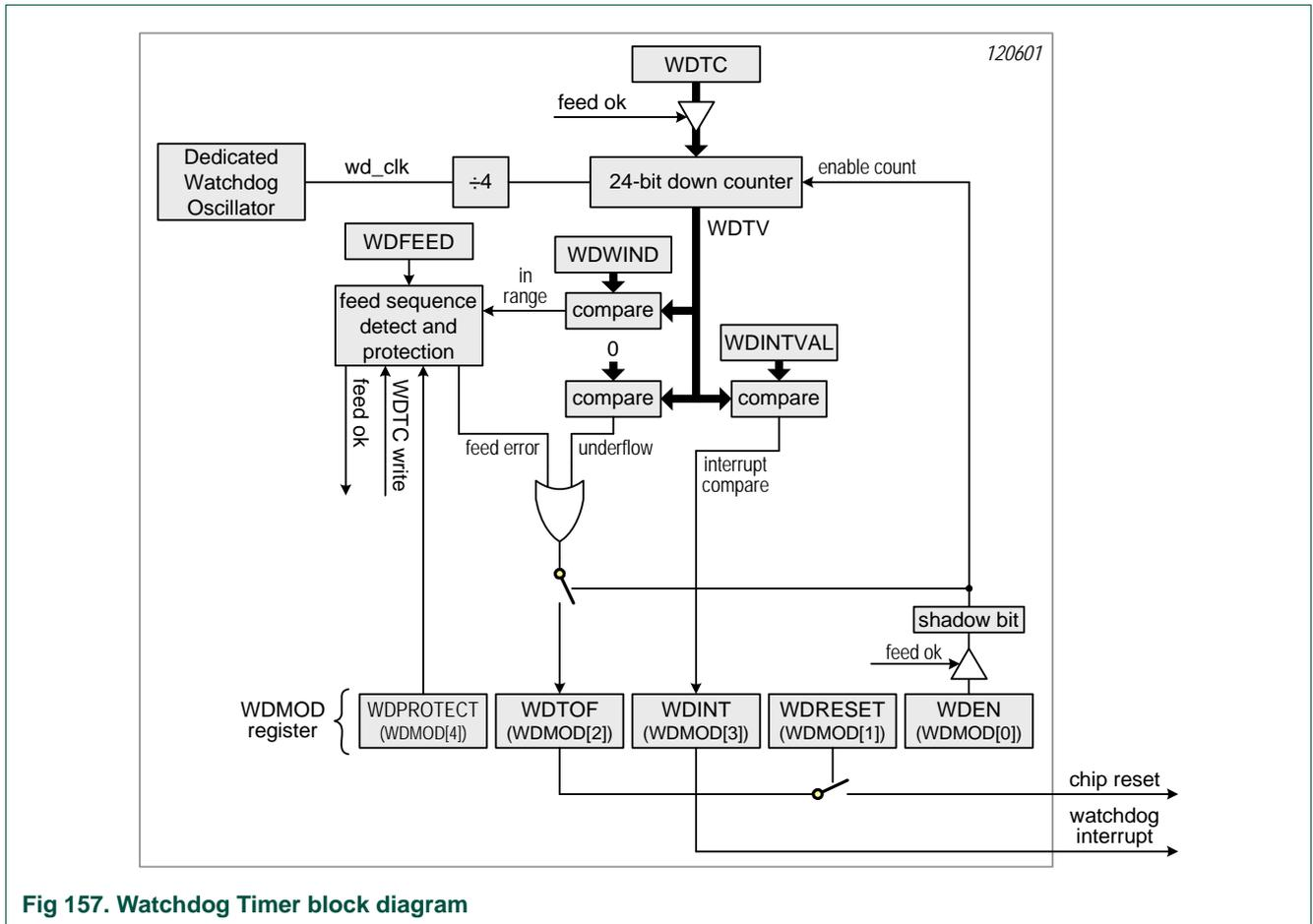
Fig 157. Watchdog Timer block diagram
