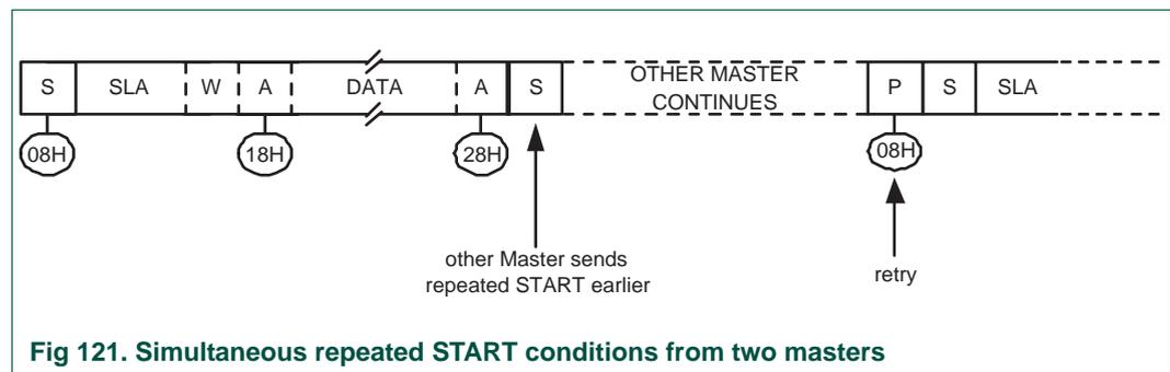
**Fig 121. Simultaneous repeated START conditions from two masters**
