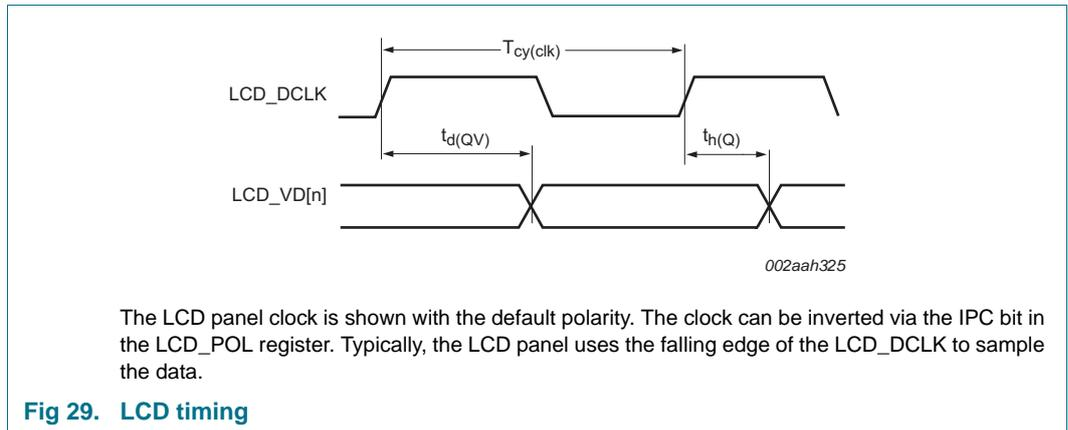
Fig 29. LCD timing
