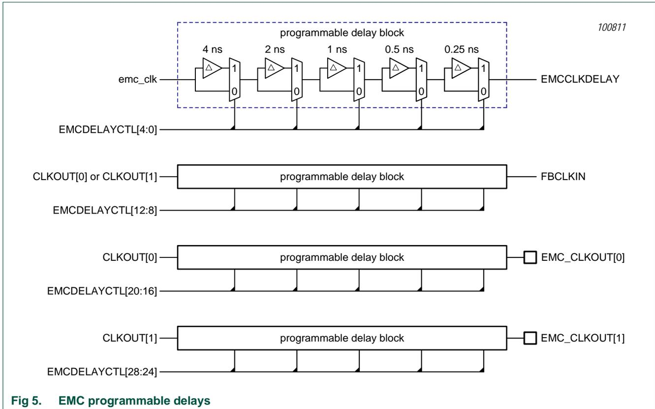
Fig 5. EMC programmable delays
