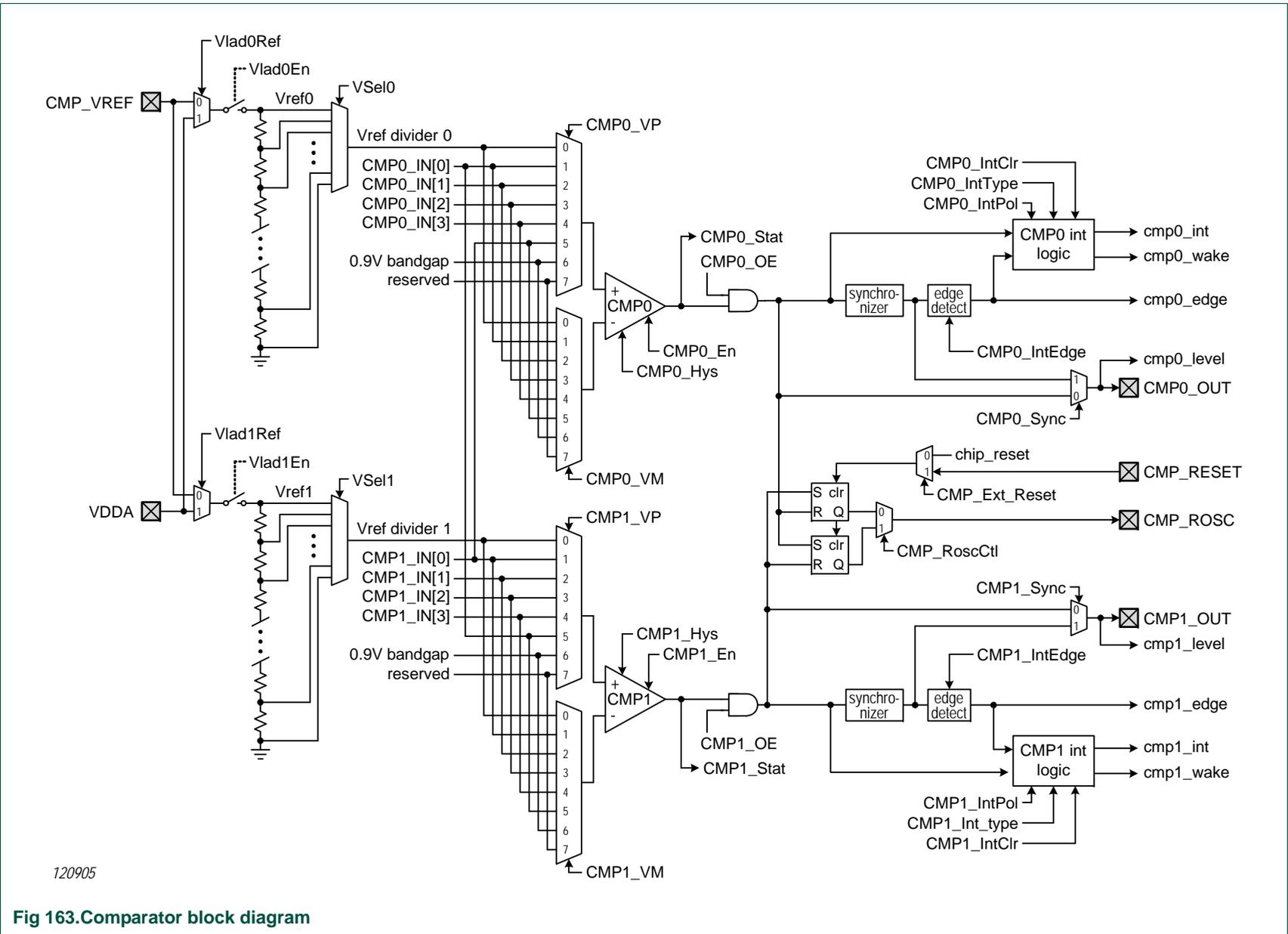
Fig 163. Comparator block diagram
