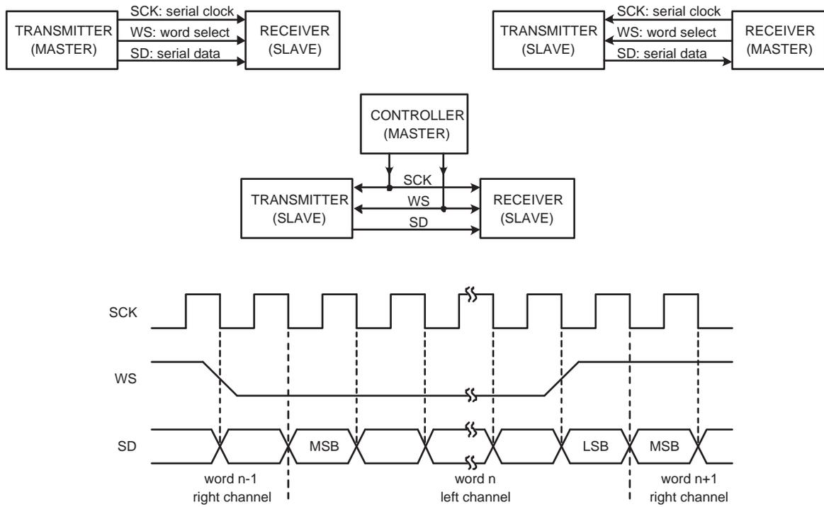
Fig 124. Simple I<sup>2</sup>S configurations and bus timing
