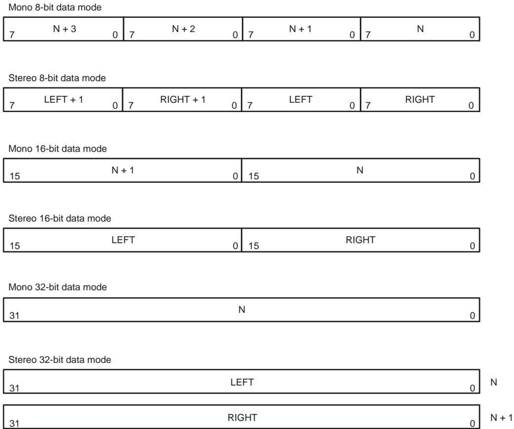
Fig 138. FIFO contents for various I<sup>2</sup>S modes
