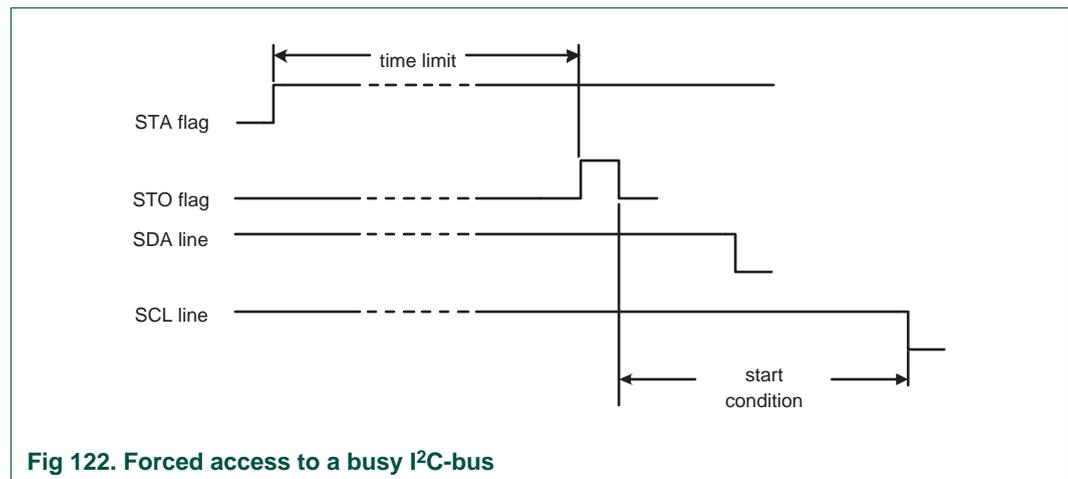
**Fig 122. Forced access to a busy I<sup>2</sup>C-bus**
