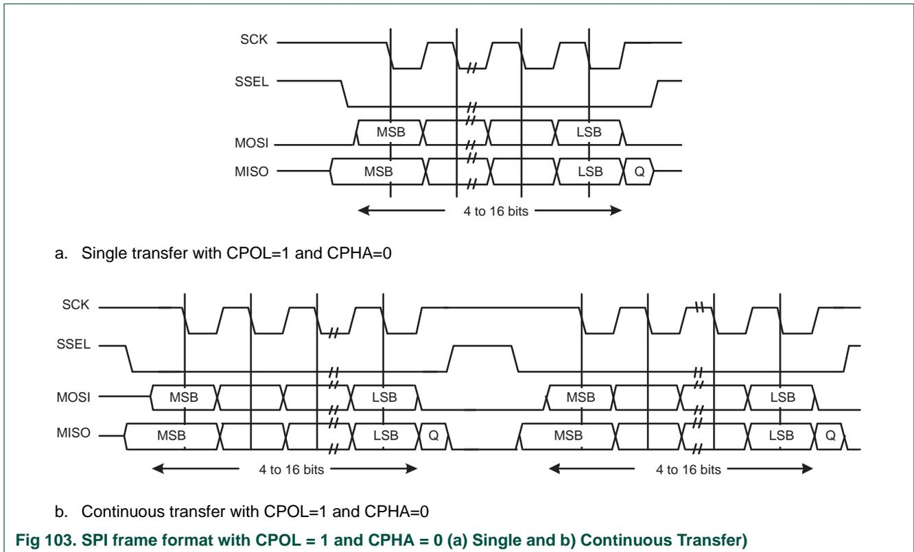
**Fig 103. SPI frame format with CPOL = 1 and CPHA = 0 (a) Single and b) Continuous Transfer)**
