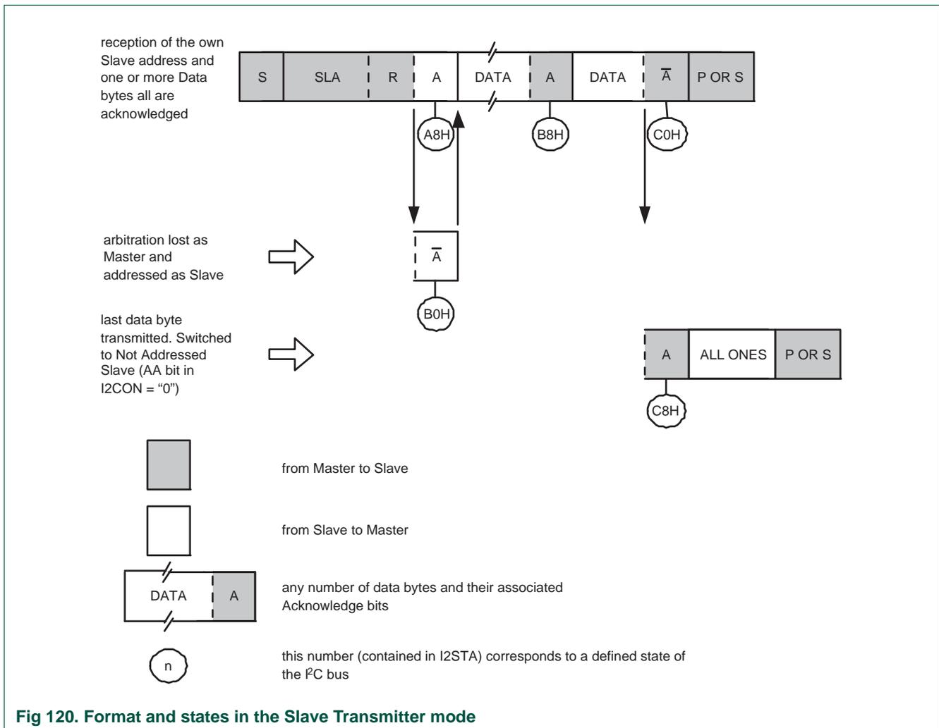
Fig 120. Format and states in the Slave Transmitter mode
