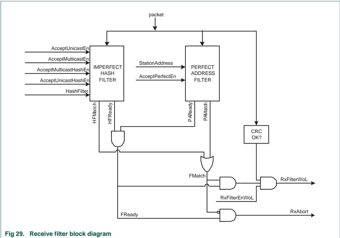
Fig 29. Receive filter block diagram
