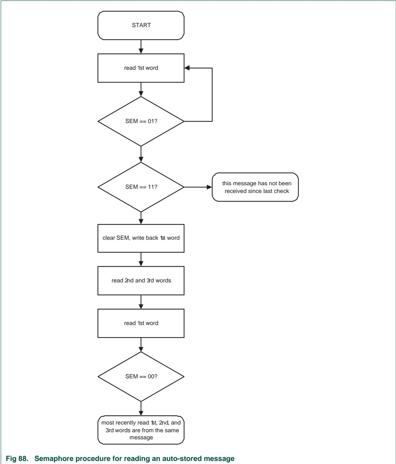
Fig 88. Semaphore procedure for reading an auto-stored message
