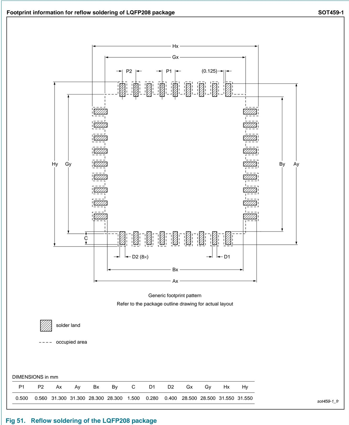
Fig 51. Reflow soldering of the LQFP208 package
