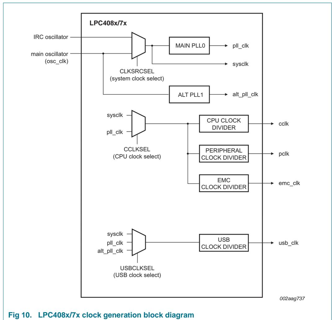
Fig 10. LPC408x/7x clock generation block diagram
