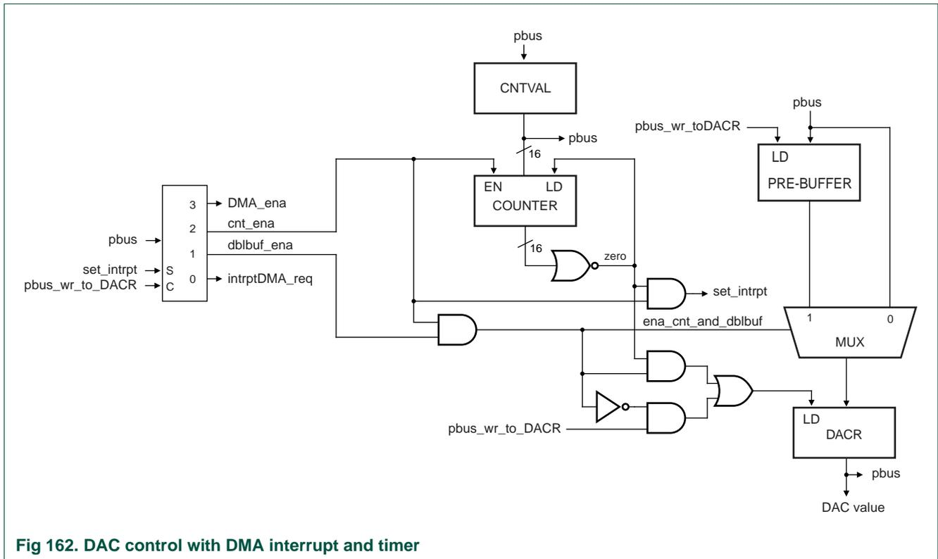
Fig 162. DAC control with DMA interrupt and timer
