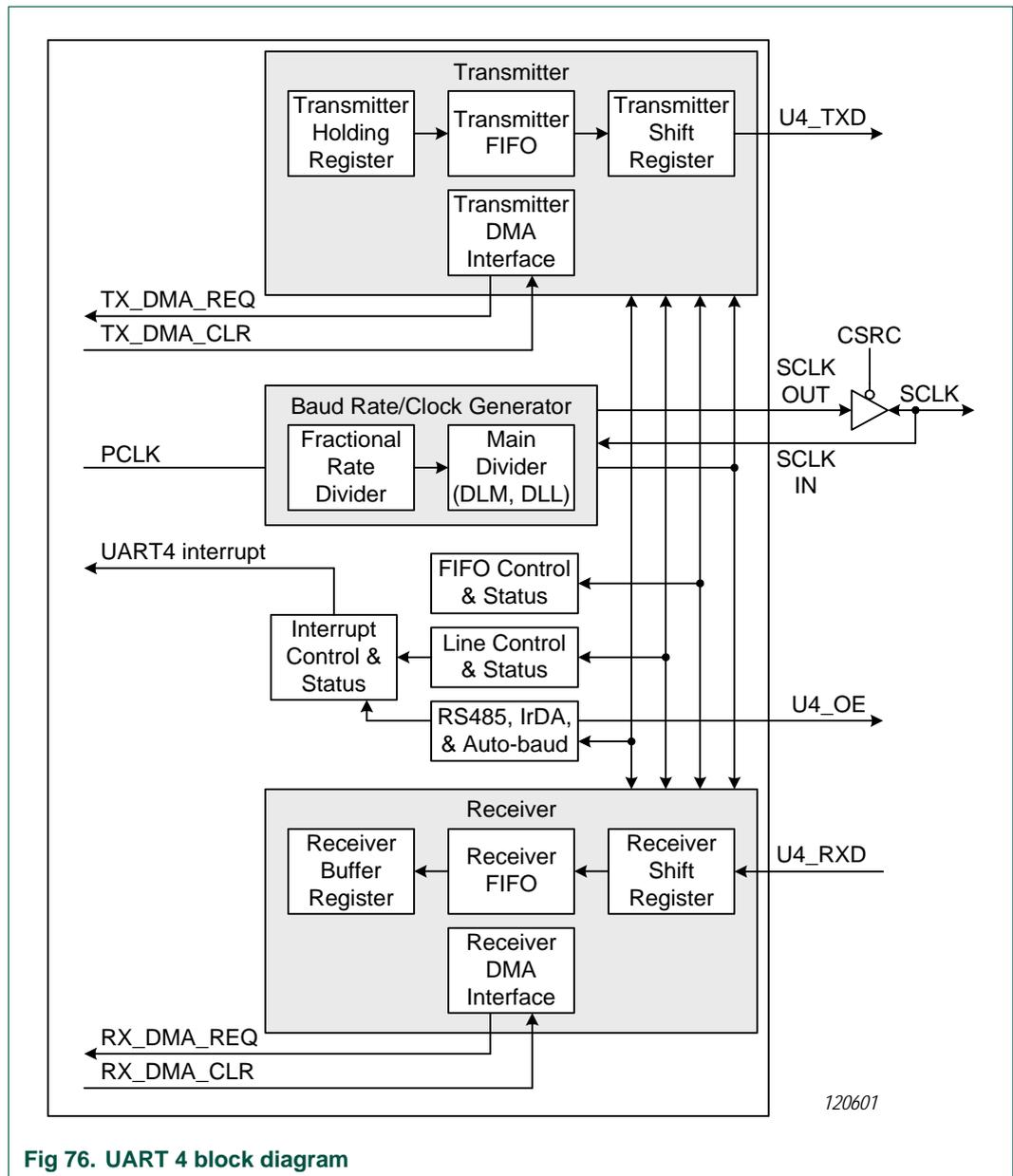
Fig 76. UART 4 block diagram
