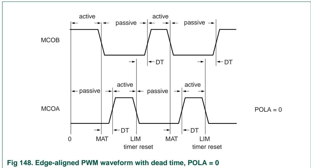
Fig 148. Edge-aligned PWM waveform with dead time, POLA = 0
