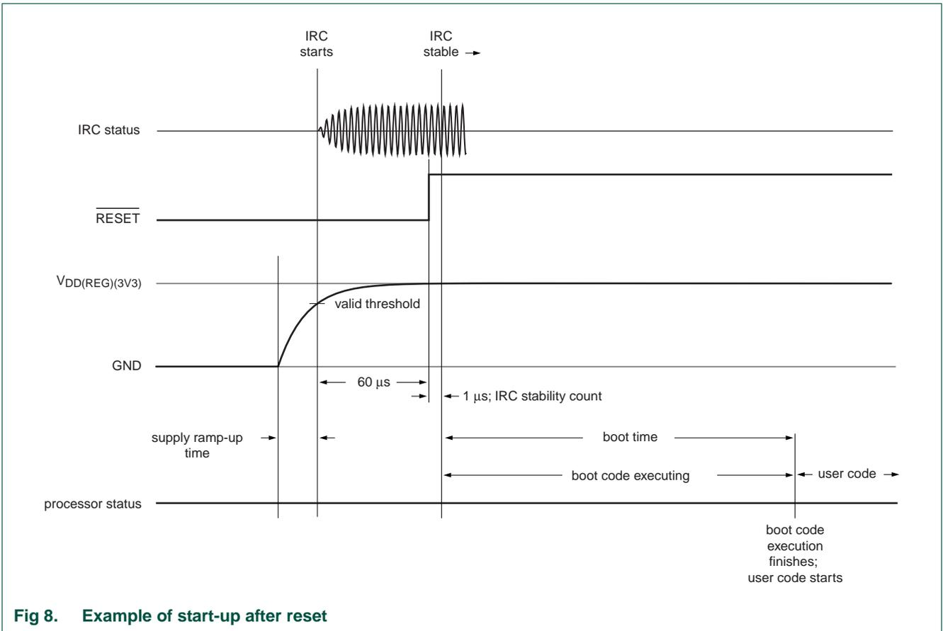
Fig 8. Example of start-up after reset
