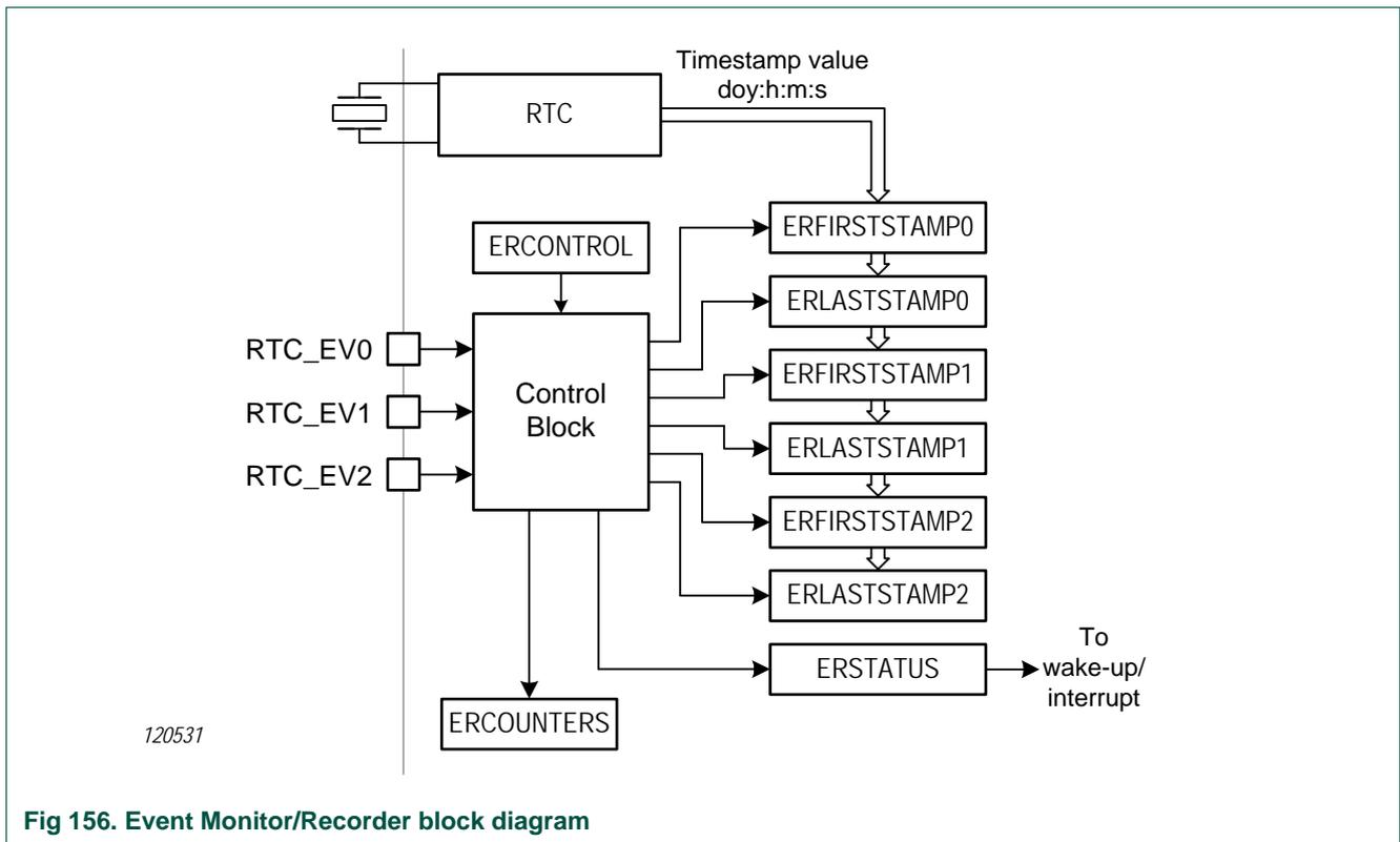
Fig 156. Event Monitor/Recorder block diagram
