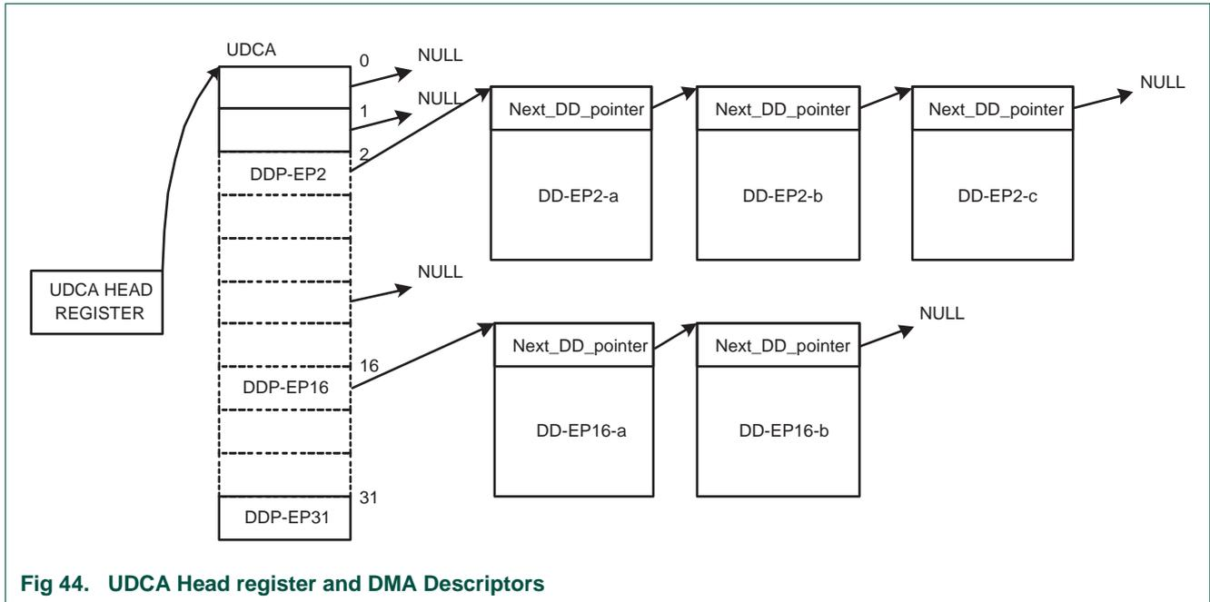
Fig 44. UDCA Head register and DMA Descriptors
