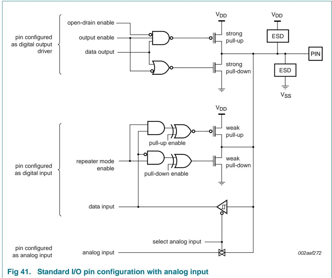
Fig 41. Standard I/O pin configuration with analog input
