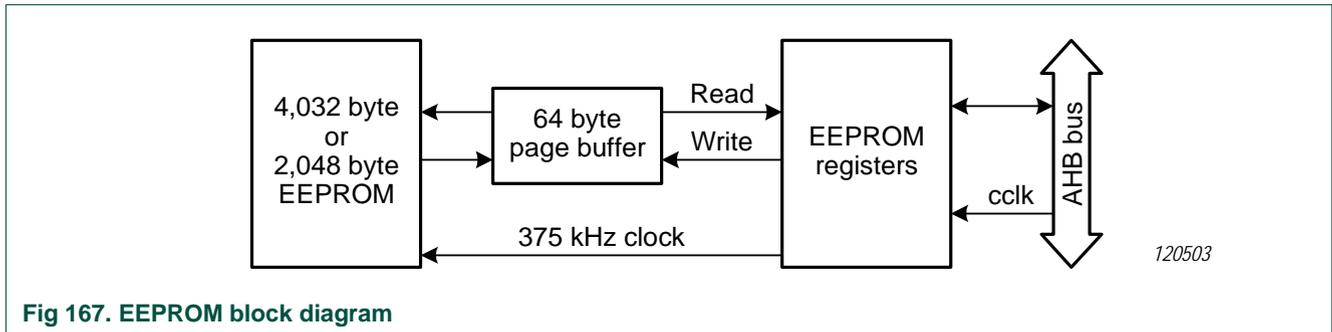
Fig 167. EEPROM block diagram
