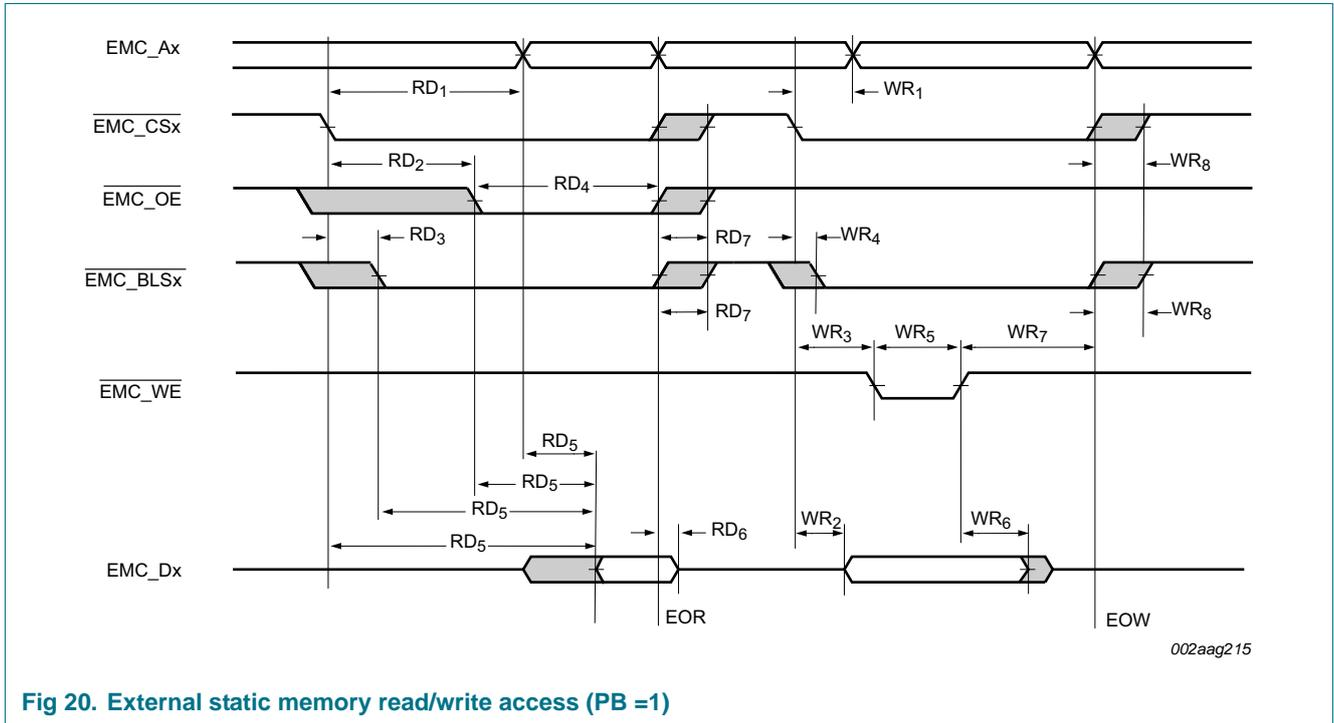
Fig 20. External static memory read/write access (PB =1)
