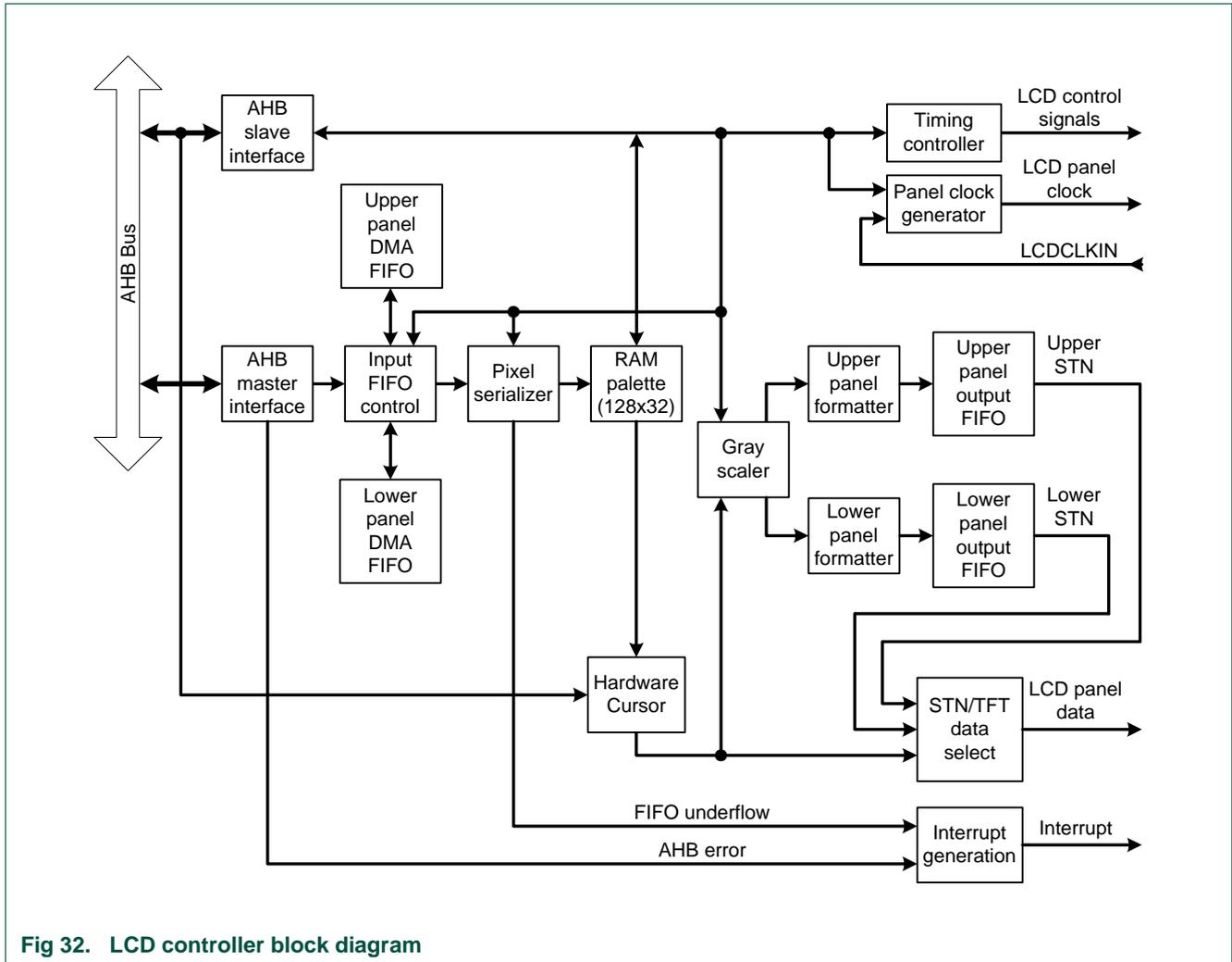
Fig 32. LCD controller block diagram
