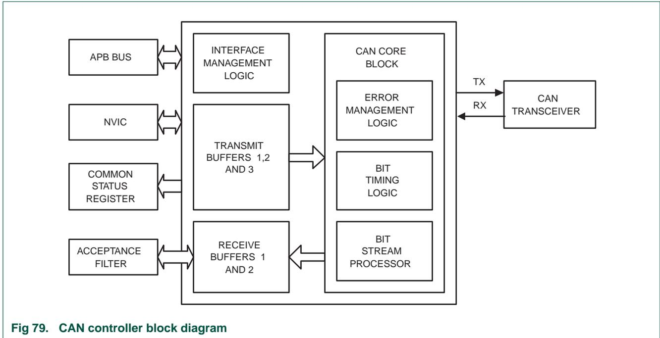
Fig 79. CAN controller block diagram
