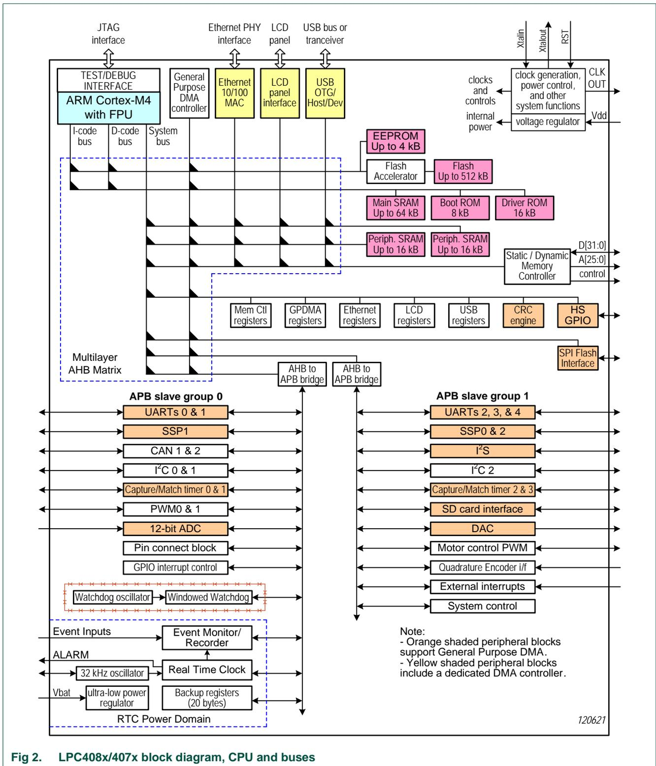
Fig 2. LPC408x/407x block diagram, CPU and buses
