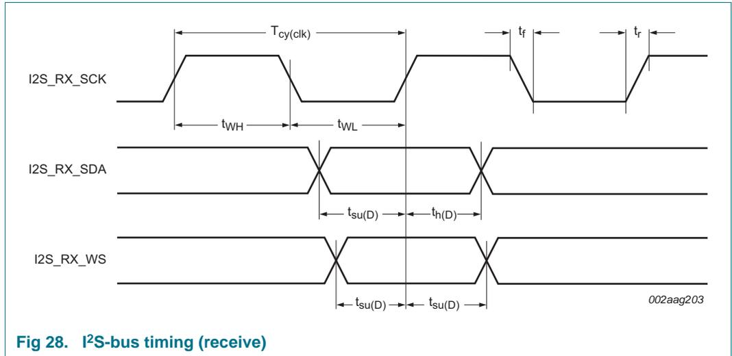
Fig 28. I2S-bus timing (receive)
