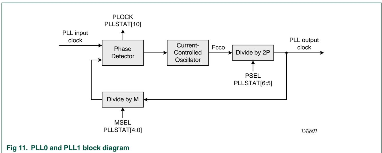
**Fig 11. PLL0 and PLL1 block diagram**
