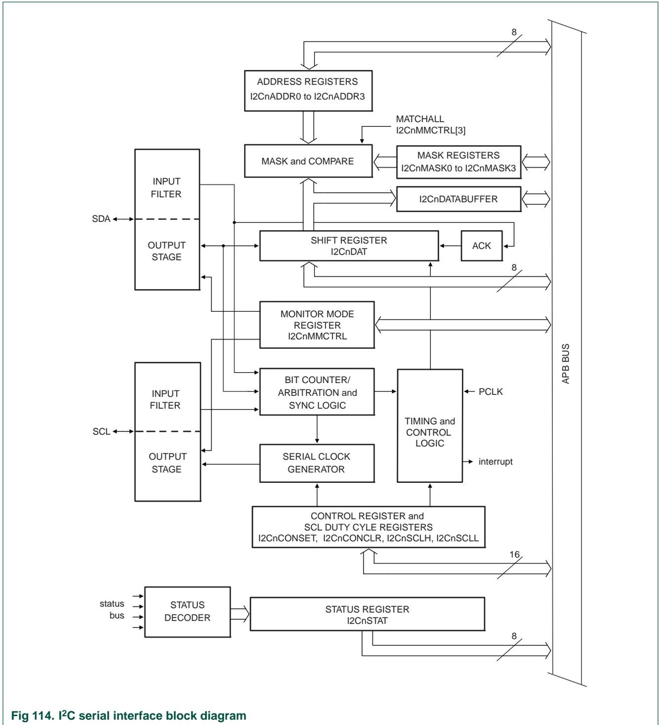
Fig 114. I2C serial interface block diagram
