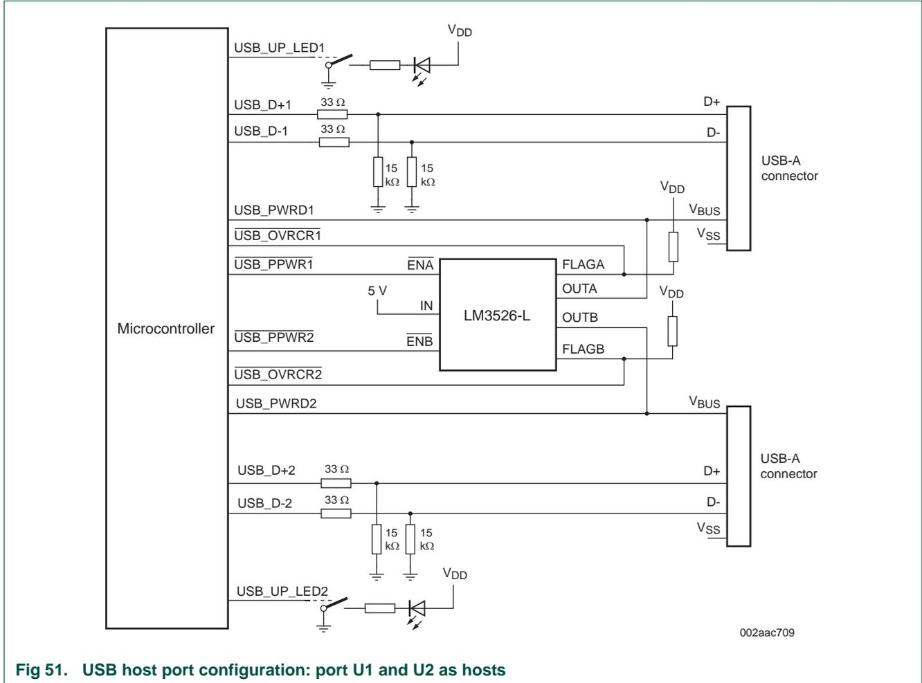
Fig 51. USB host port configuration: port U1 and U2 as hosts
