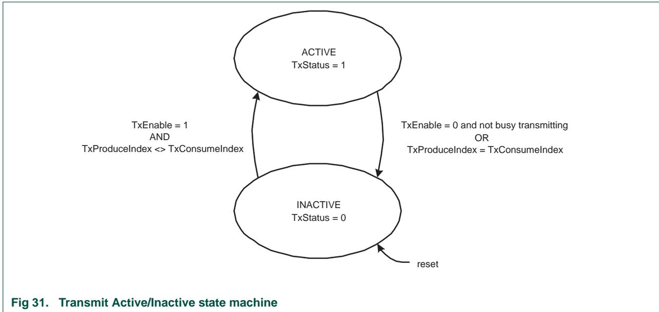
Fig 31. Transmit Active/Inactive state machine
