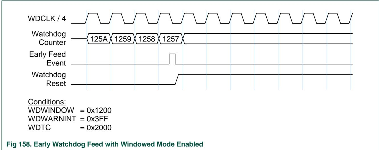
**Fig 158. Early Watchdog Feed with Windowed Mode Enabled**
