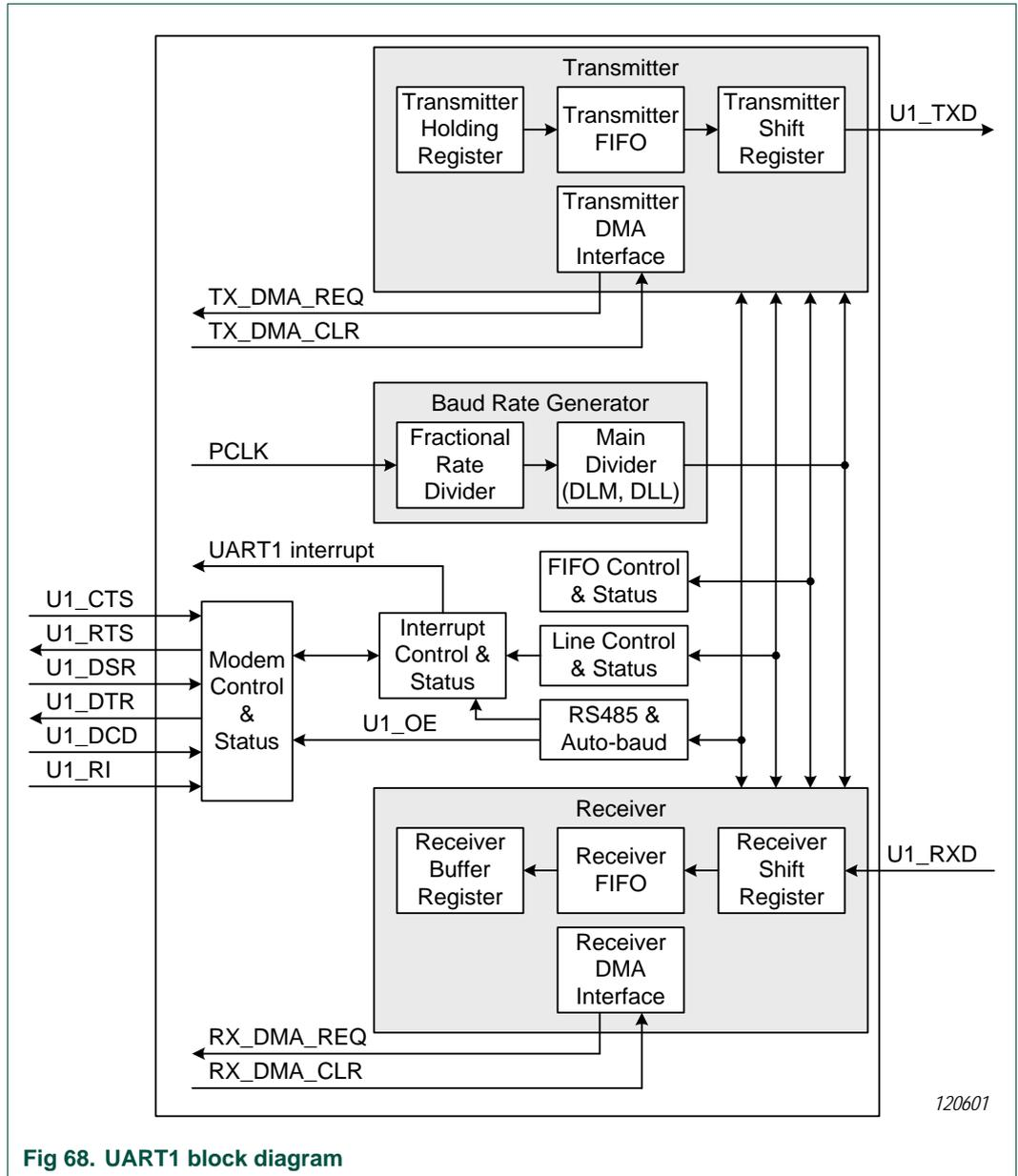
Fig 68. UART1 block diagram
