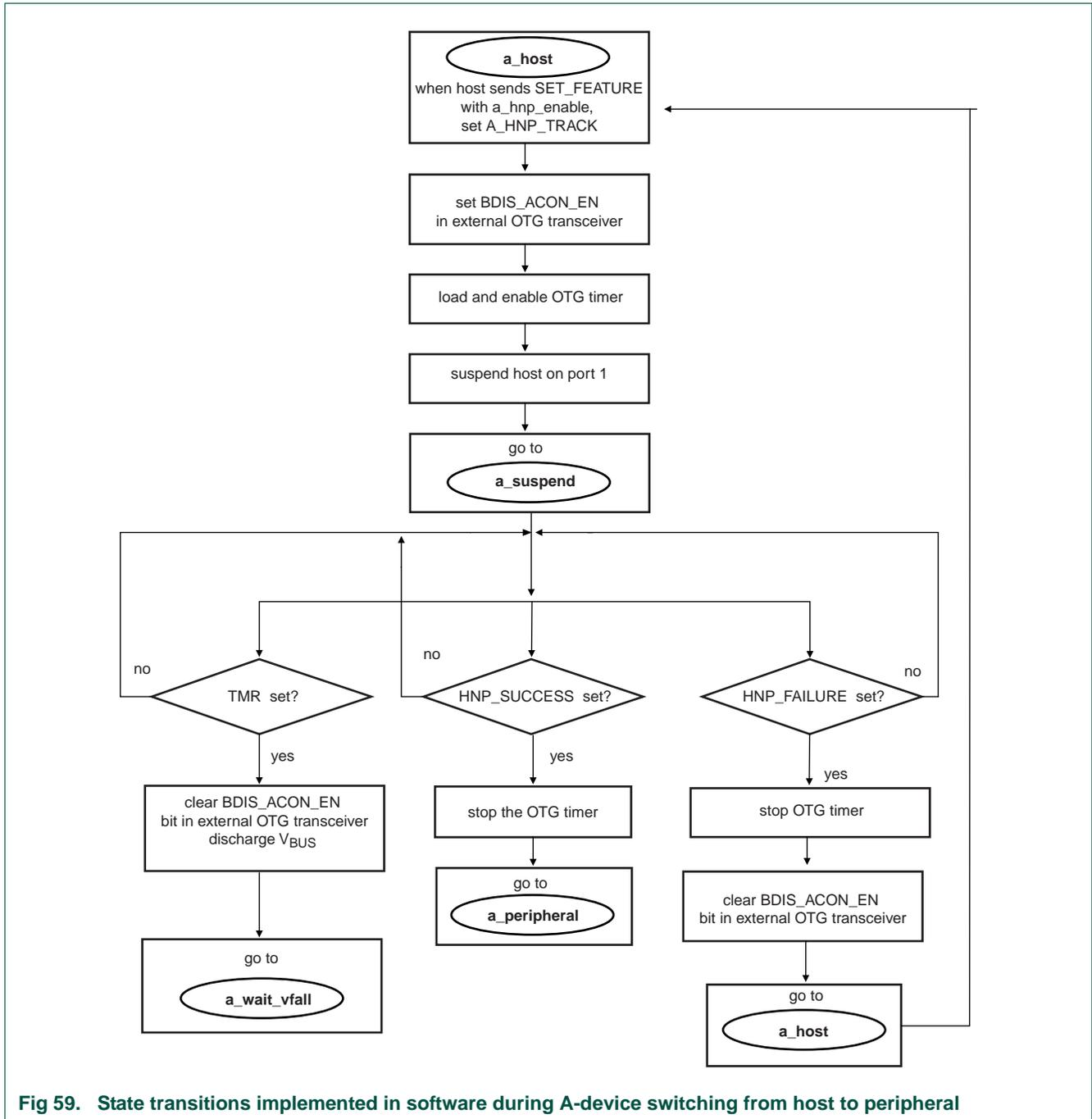
Fig 59. State transitions implemented in software during A-device switching from host to peripheral
