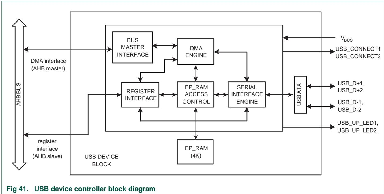
Fig 41. USB device controller block diagram
