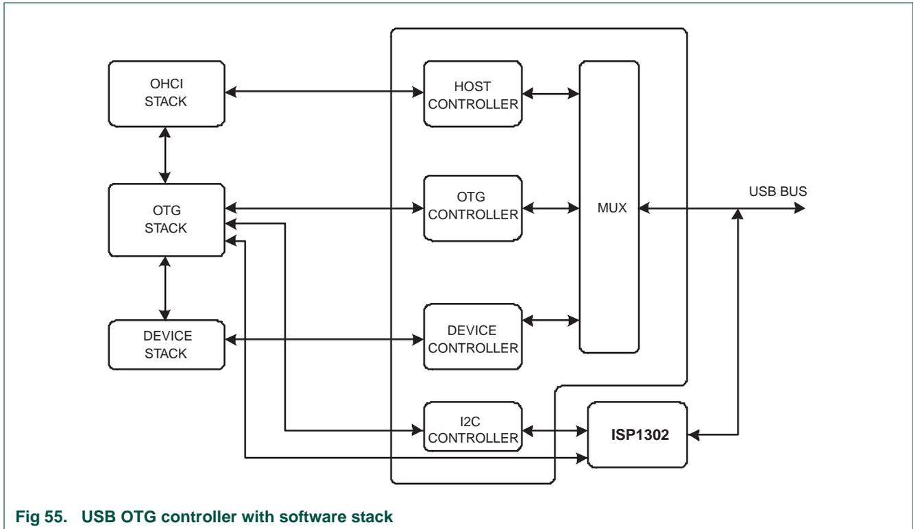
Fig 55. USB OTG controller with software stack
