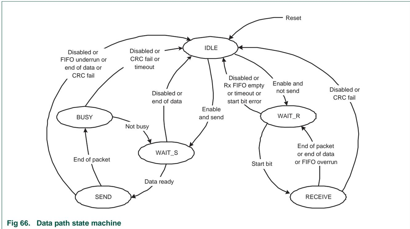
**Fig 66. Data path state machine**
