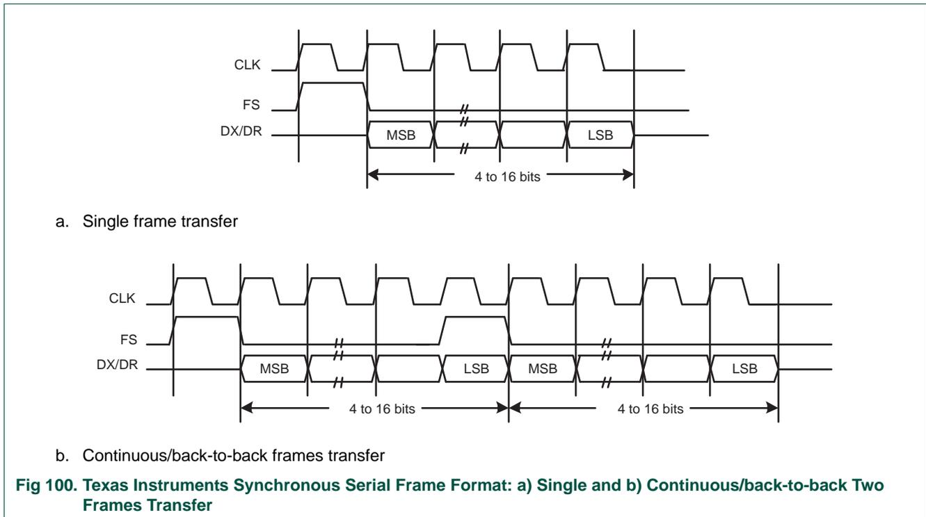
**Fig 100. Texas Instruments Synchronous Serial Frame Format: a) Single and b) Continuous/back-to-back Two Frames Transfer**
