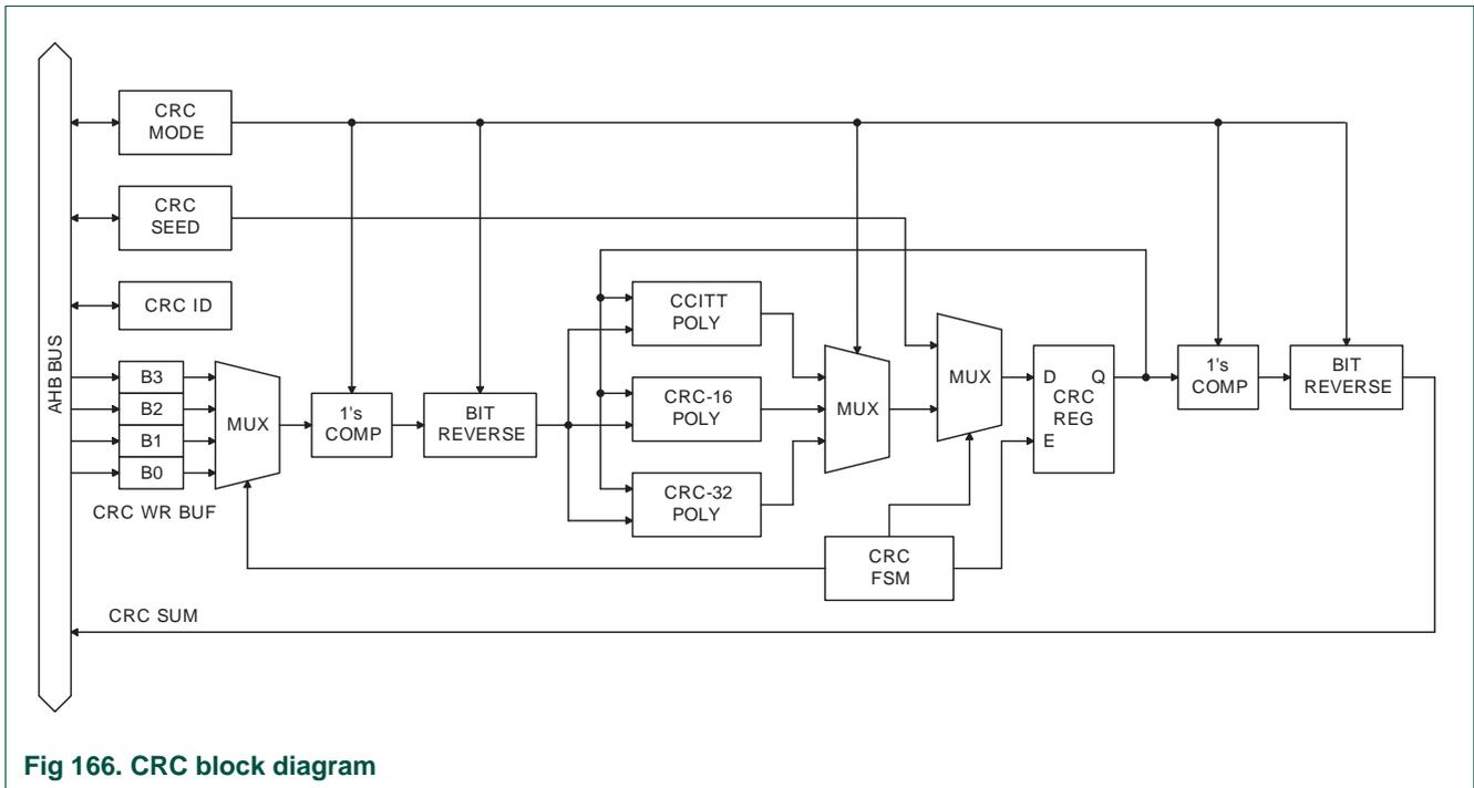
Fig 166. CRC block diagram
