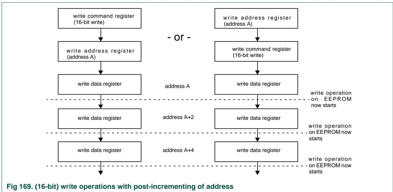
**Fig 169. (16-bit) write operations with post-incrementing of address**
