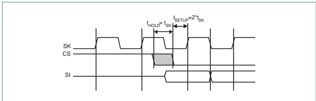
Fig 107. Microwire frame format setup and hold details
