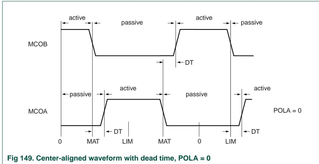
Fig 149. Center-aligned waveform with dead time, POLA = 0
