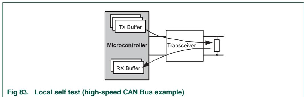
**Fig 83. Local self test (high-speed CAN Bus example)**
