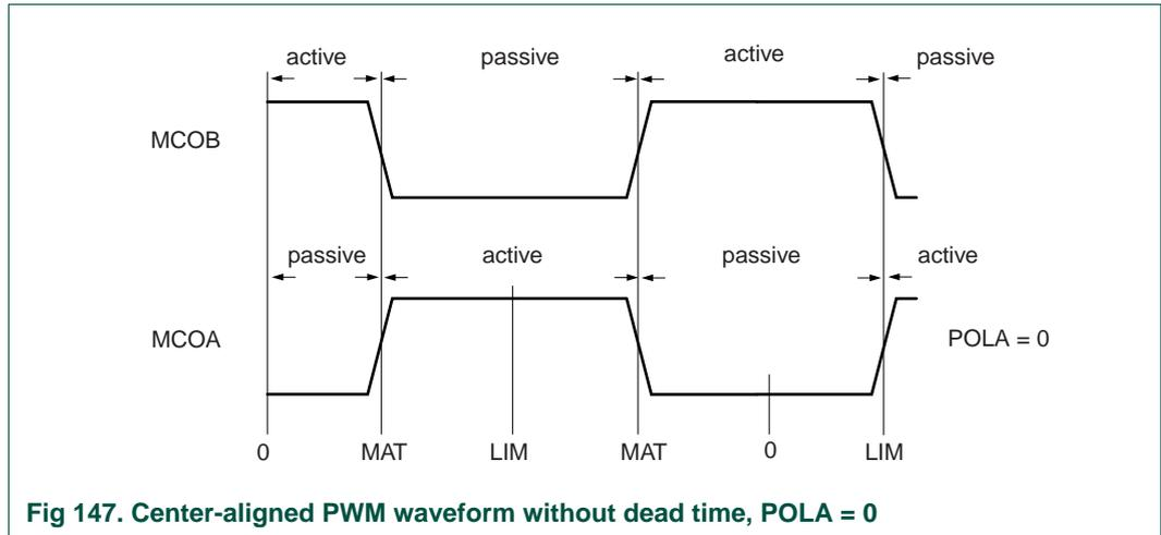
Fig 147. Center-aligned PWM waveform without dead time, POLA = 0
