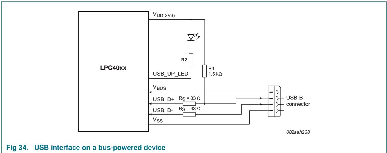
Fig 34. USB interface on a bus-powered device
