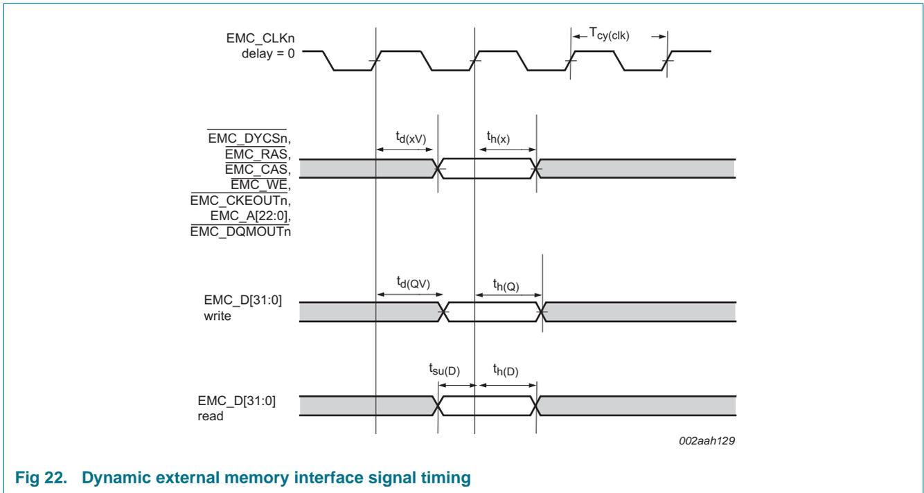
Fig 22. Dynamic external memory interface signal timing
