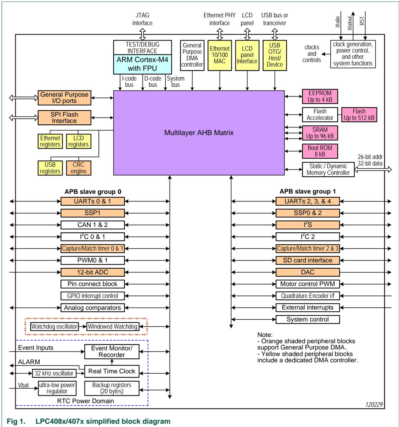
Fig 1. LPC408x/407x simplified block diagram
