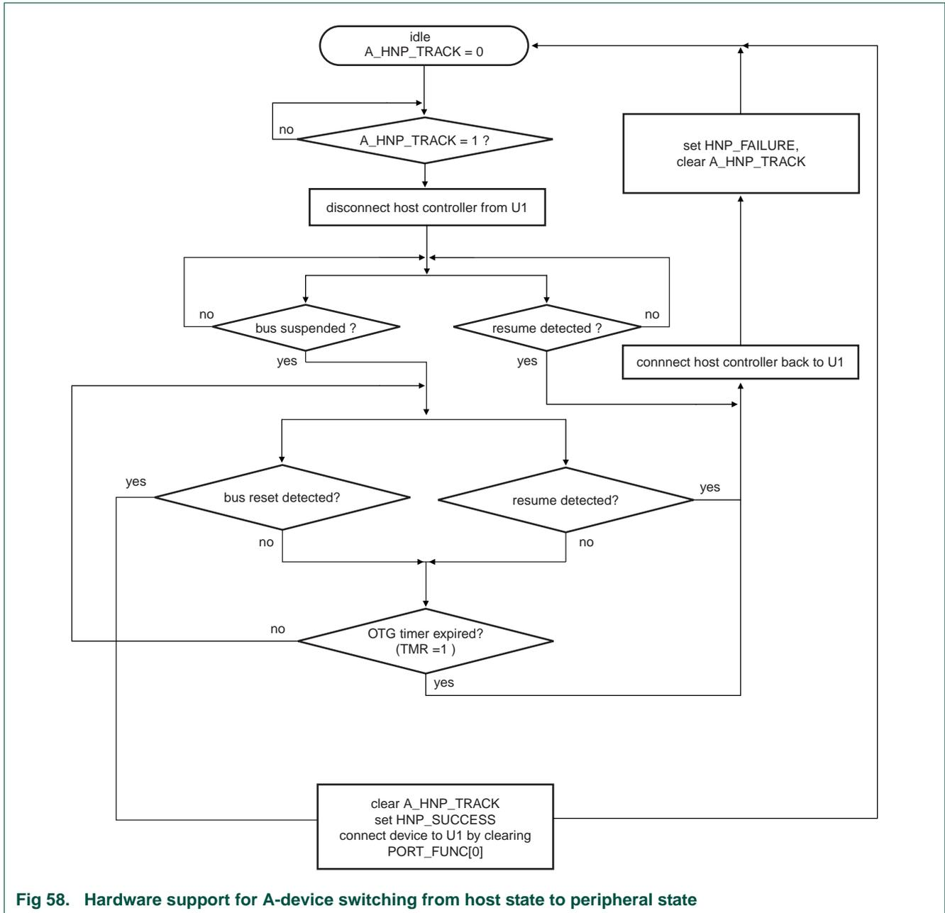
Fig 58. Hardware support for A-device switching from host state to peripheral state
