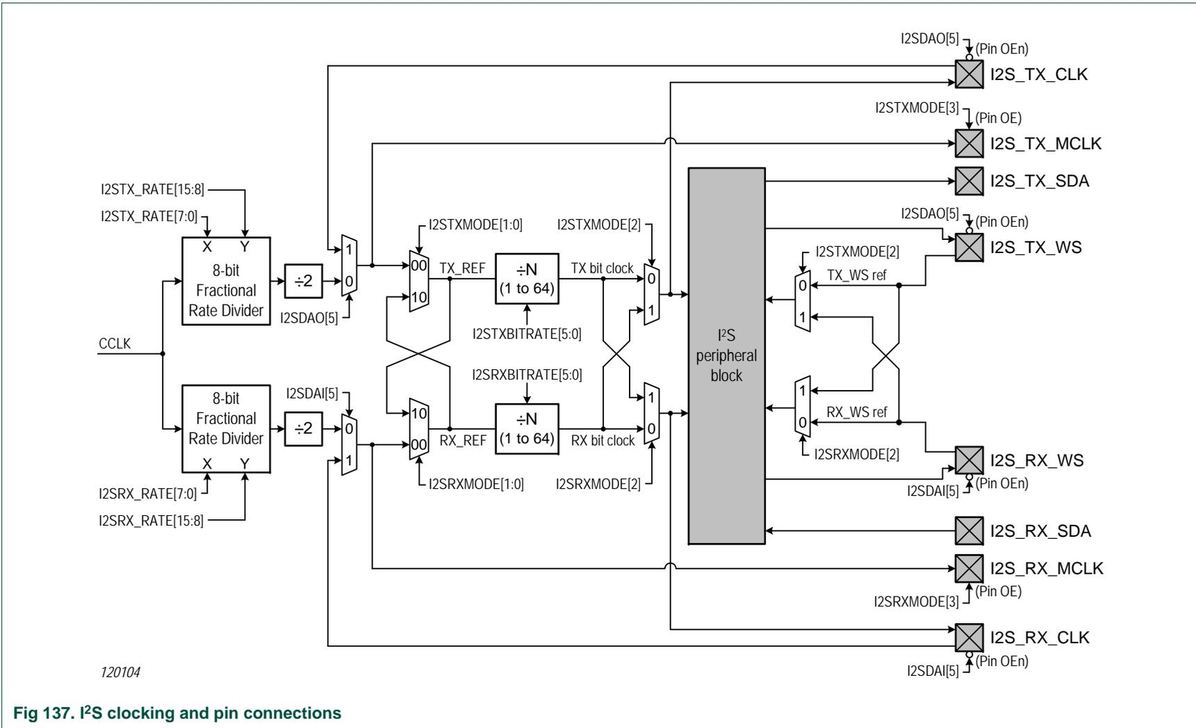
Fig 137. I<sup>2</sup>S clocking and pin connections
