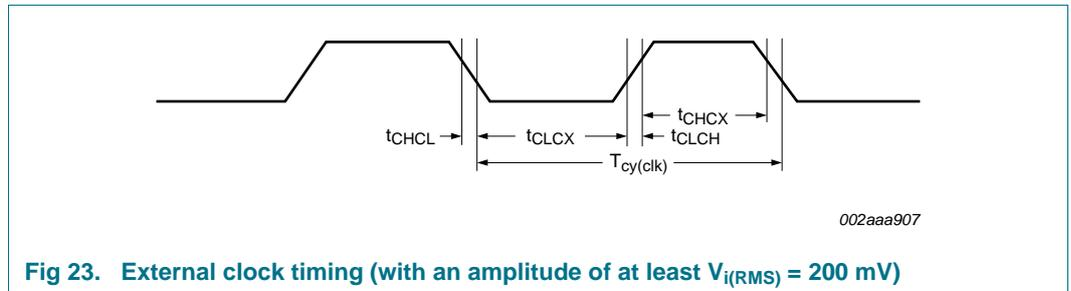
**Fig 23. External clock timing (with an amplitude of at least  $V_{i(RMS)} = 200\text{ mV}$ )**
