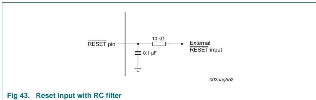
Fig 43. Reset input with RC filter
