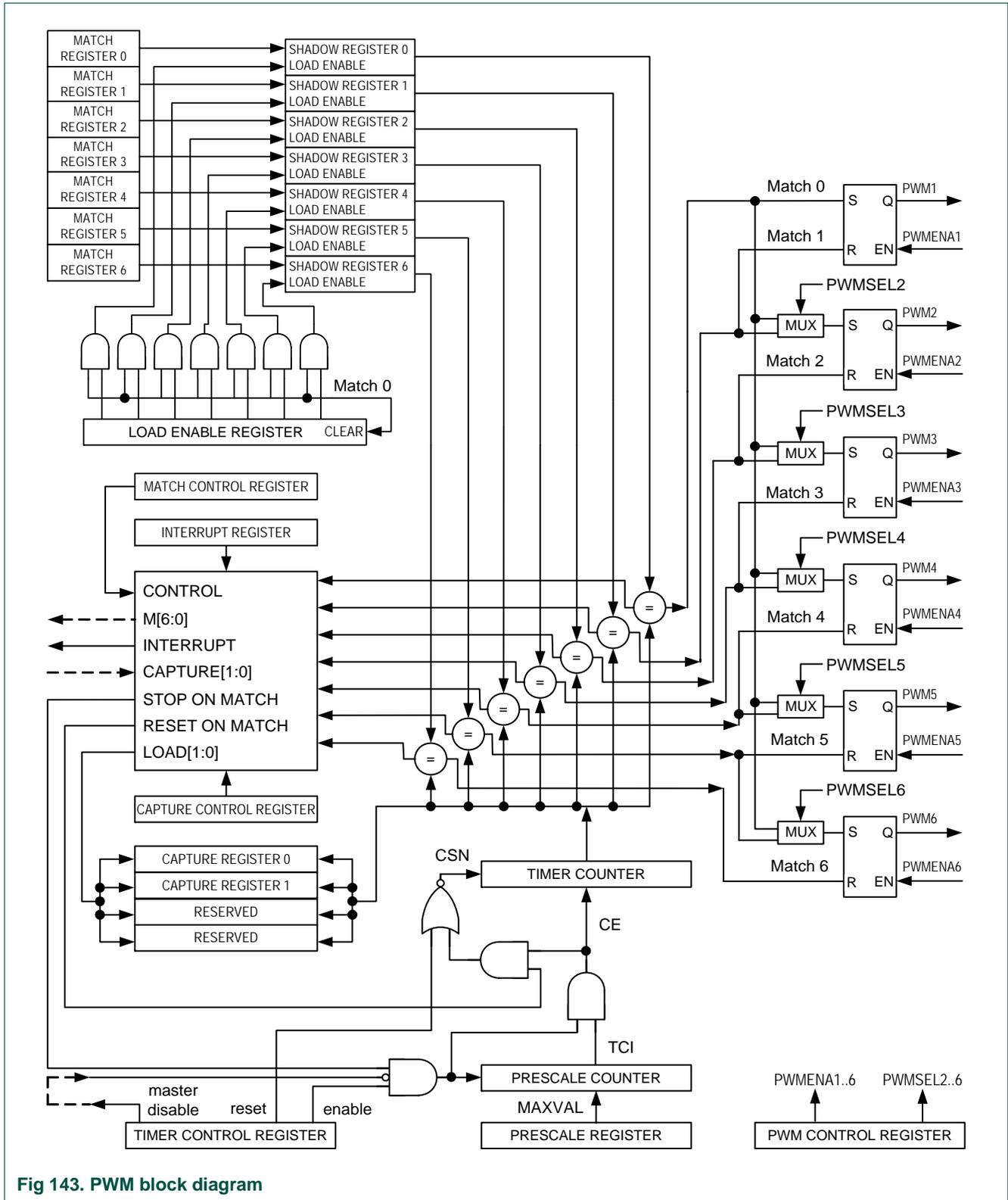
Fig 143. PWM block diagram
