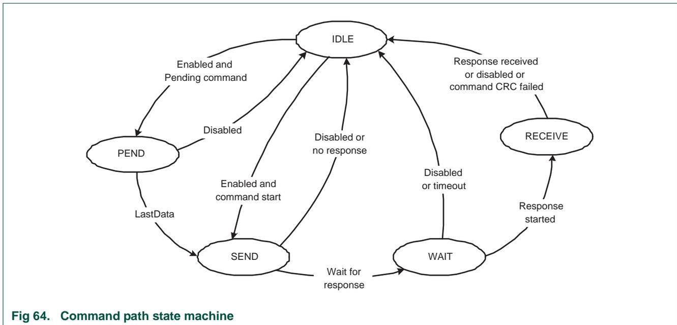
**Fig 64. Command path state machine**
