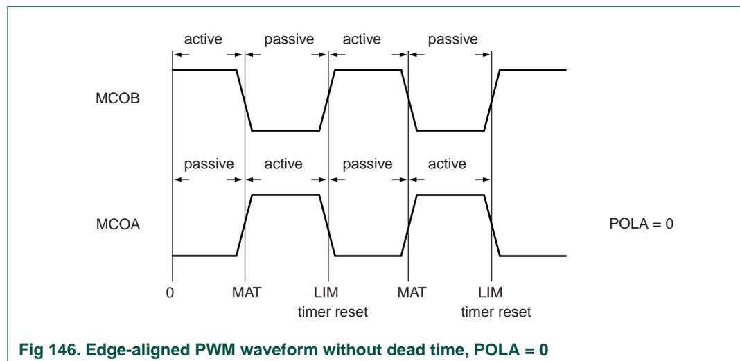
Fig 146. Edge-aligned PWM waveform without dead time, POLA = 0
