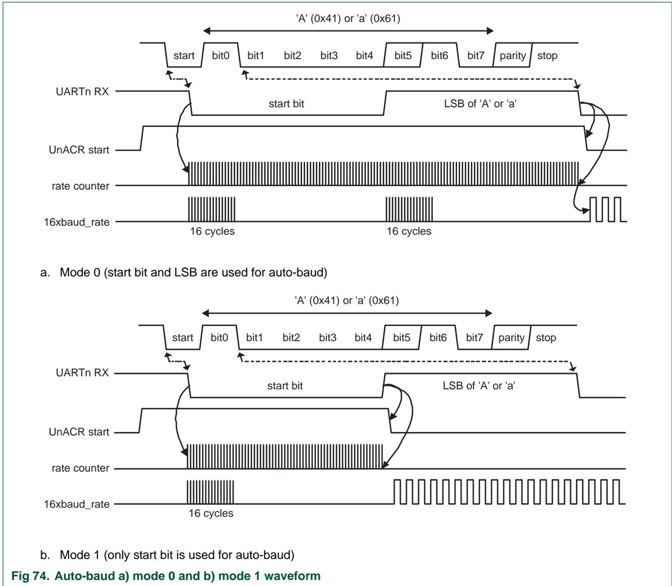
Fig 74. Auto-baud a) mode 0 and b) mode 1 waveform
