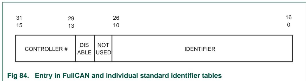
**Fig 84. Entry in FullCAN and individual standard identifier tables**
