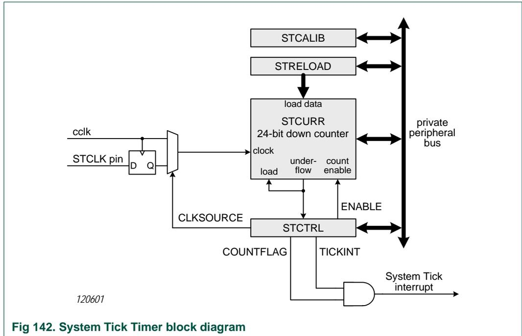
Fig 142. System Tick Timer block diagram
