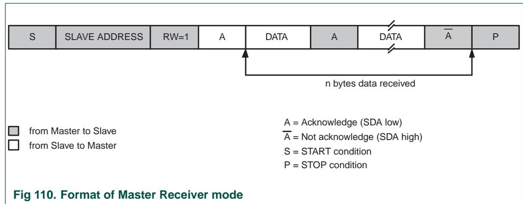
Fig 110. Format of Master Receiver mode
