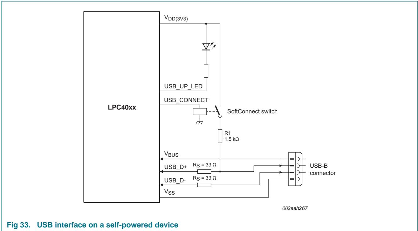
Fig 33. USB interface on a self-powered device
