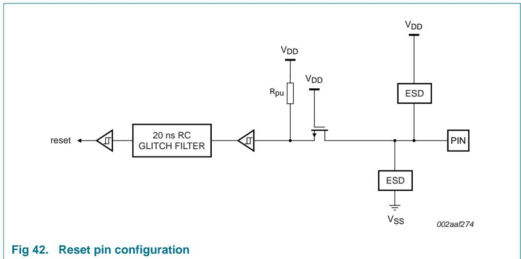
Fig 42. Reset pin configuration
