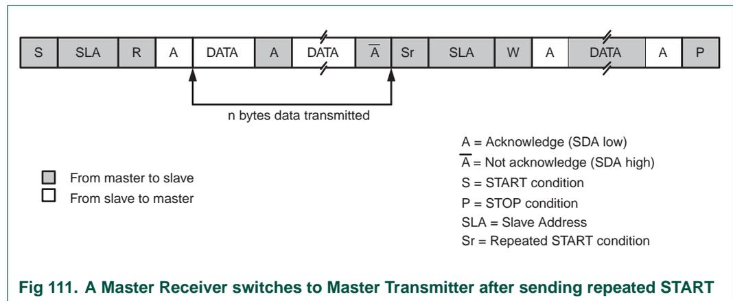
Fig 111. A Master Receiver switches to Master Transmitter after sending repeated START
