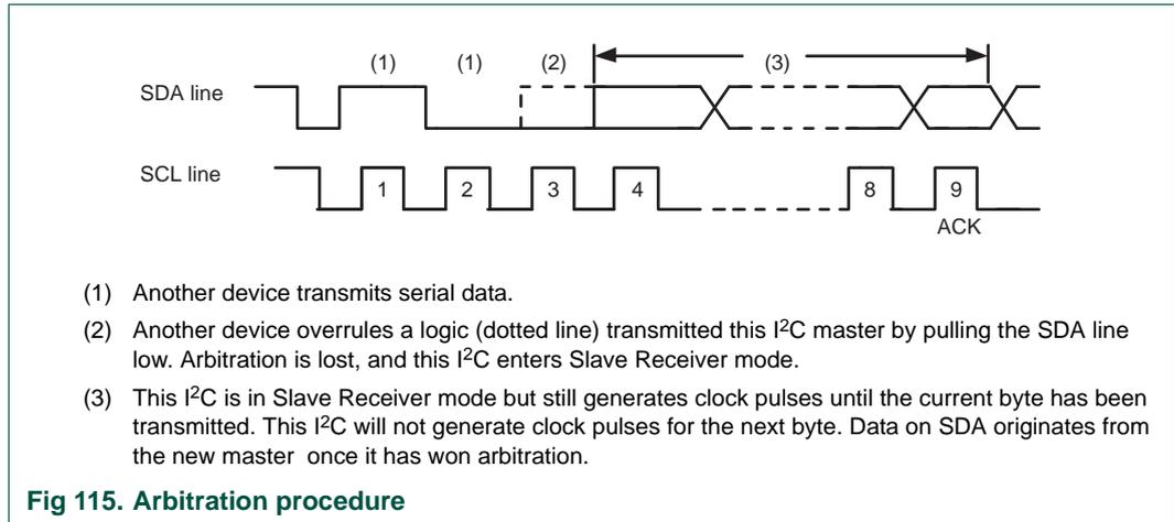
The synchronization logic will synchronize the serial clock generator with the clock pulses on the SCL line from another device. If two or more master devices generate clock pulses, the “mark” duration is determined by the device that generates the shortest “marks,” and the “space” duration is determined by the device that generates the longest “spaces”. [Figure 116](#) shows the synchronization procedure.
