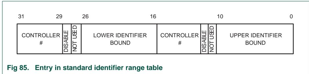
**Fig 85. Entry in standard identifier range table**
