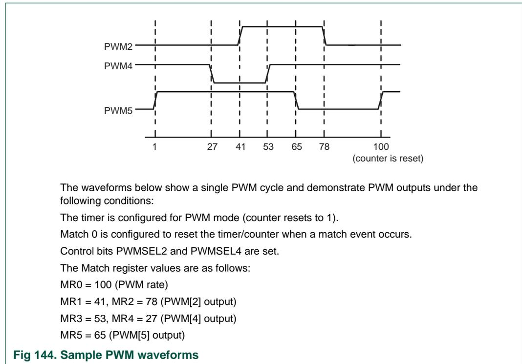
Fig 144. Sample PWM waveforms
