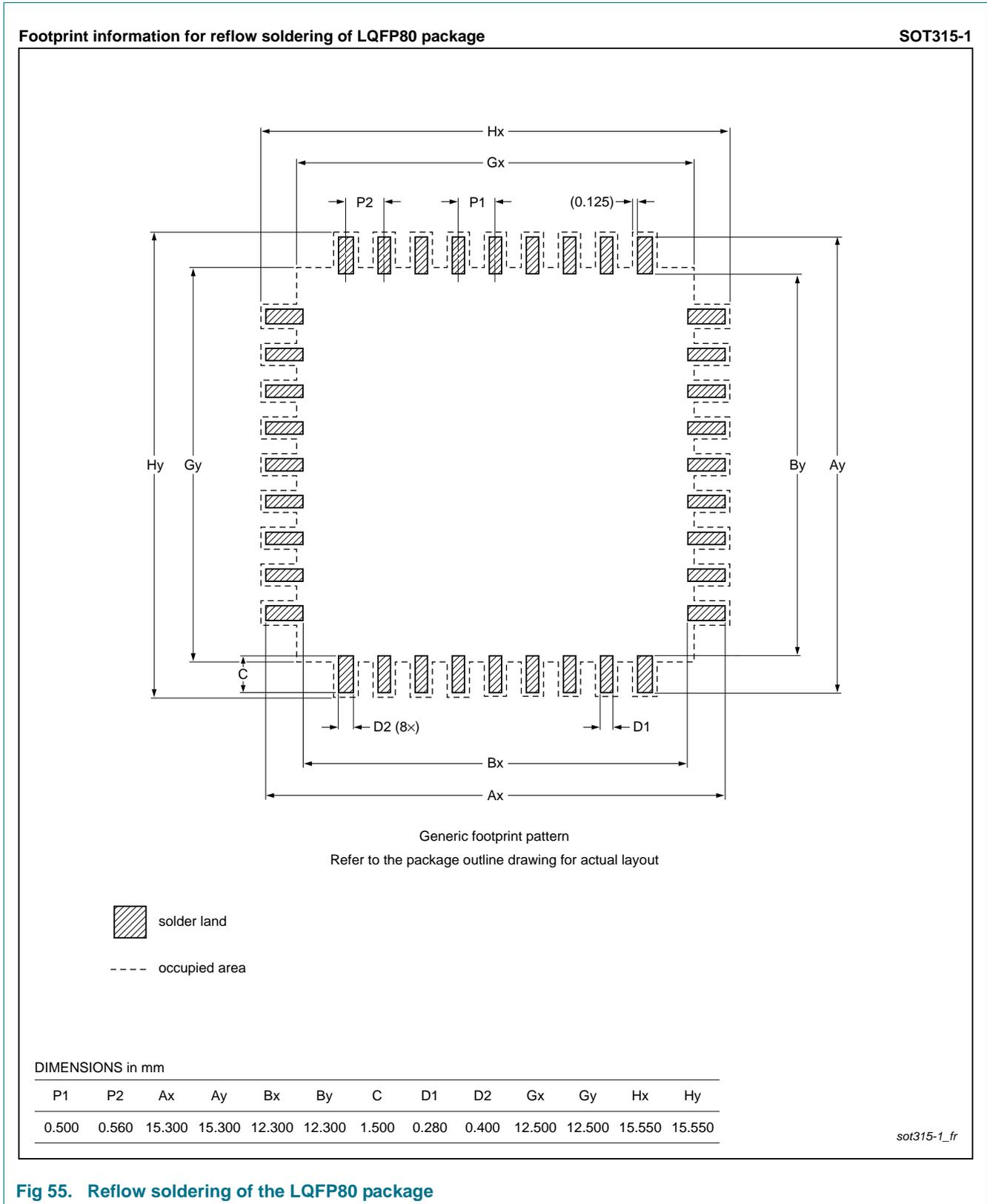
**Fig 55. Reflow soldering of the LQFP80 package**
