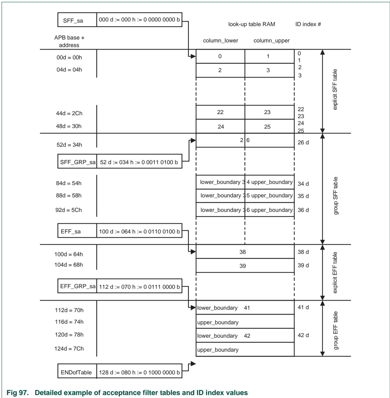
Fig 97. Detailed example of acceptance filter tables and ID index values
