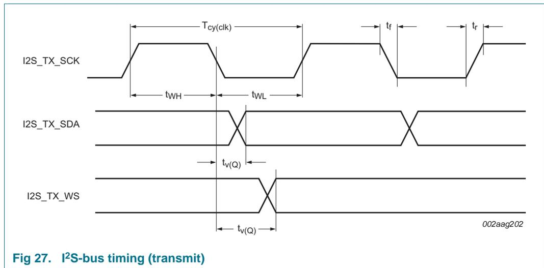
**Fig 27. I<sup>2</sup>S-bus timing (transmit)**
