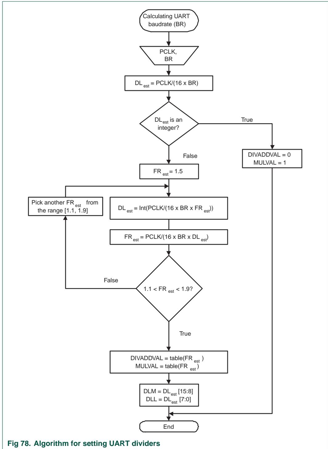
Fig 78. Algorithm for setting UART dividers
