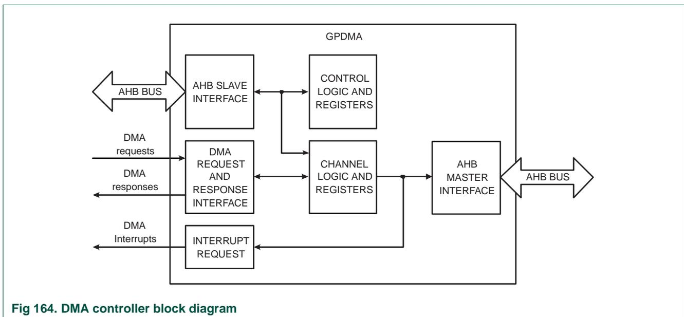
Fig 164. DMA controller block diagram
