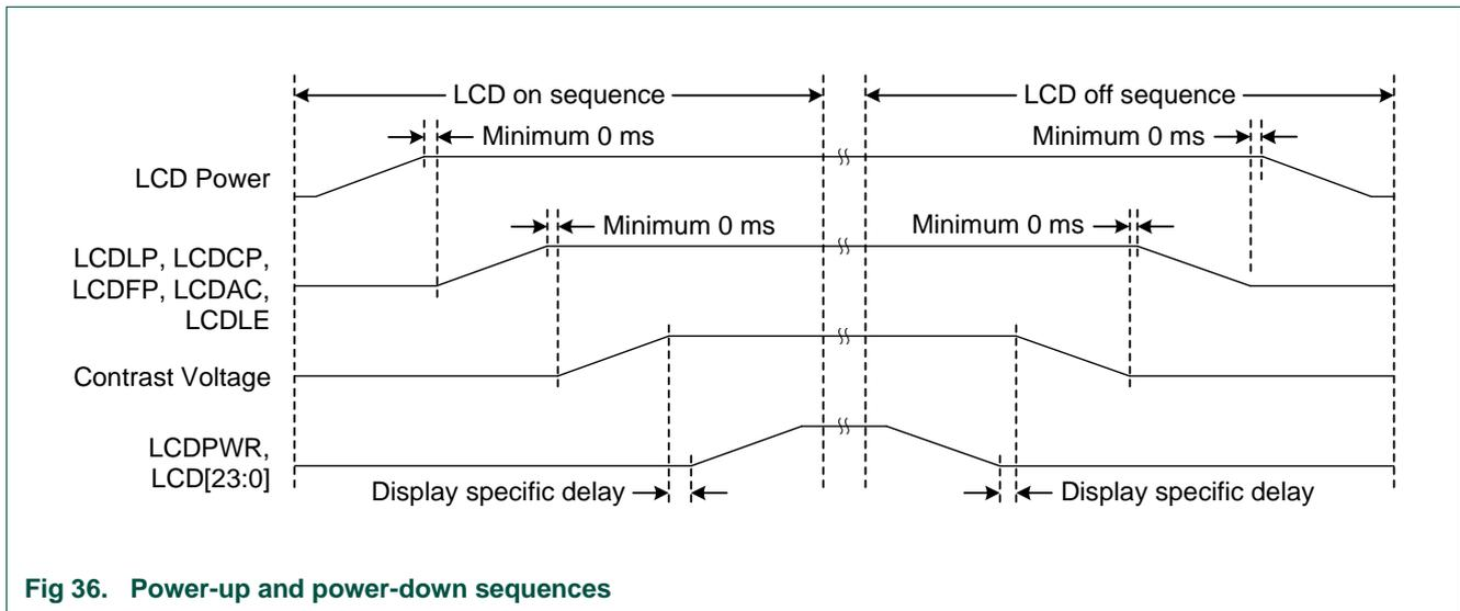
Fig 36. Power-up and power-down sequences
