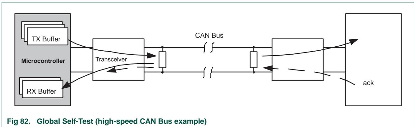
**Fig 82. Global Self-Test (high-speed CAN Bus example)**
