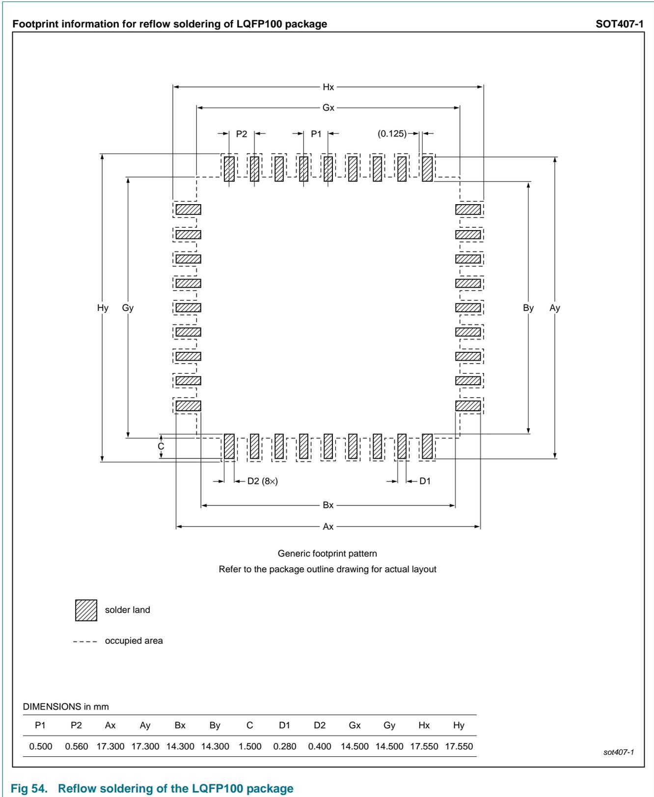
**Fig 54. Reflow soldering of the LQFP100 package**
