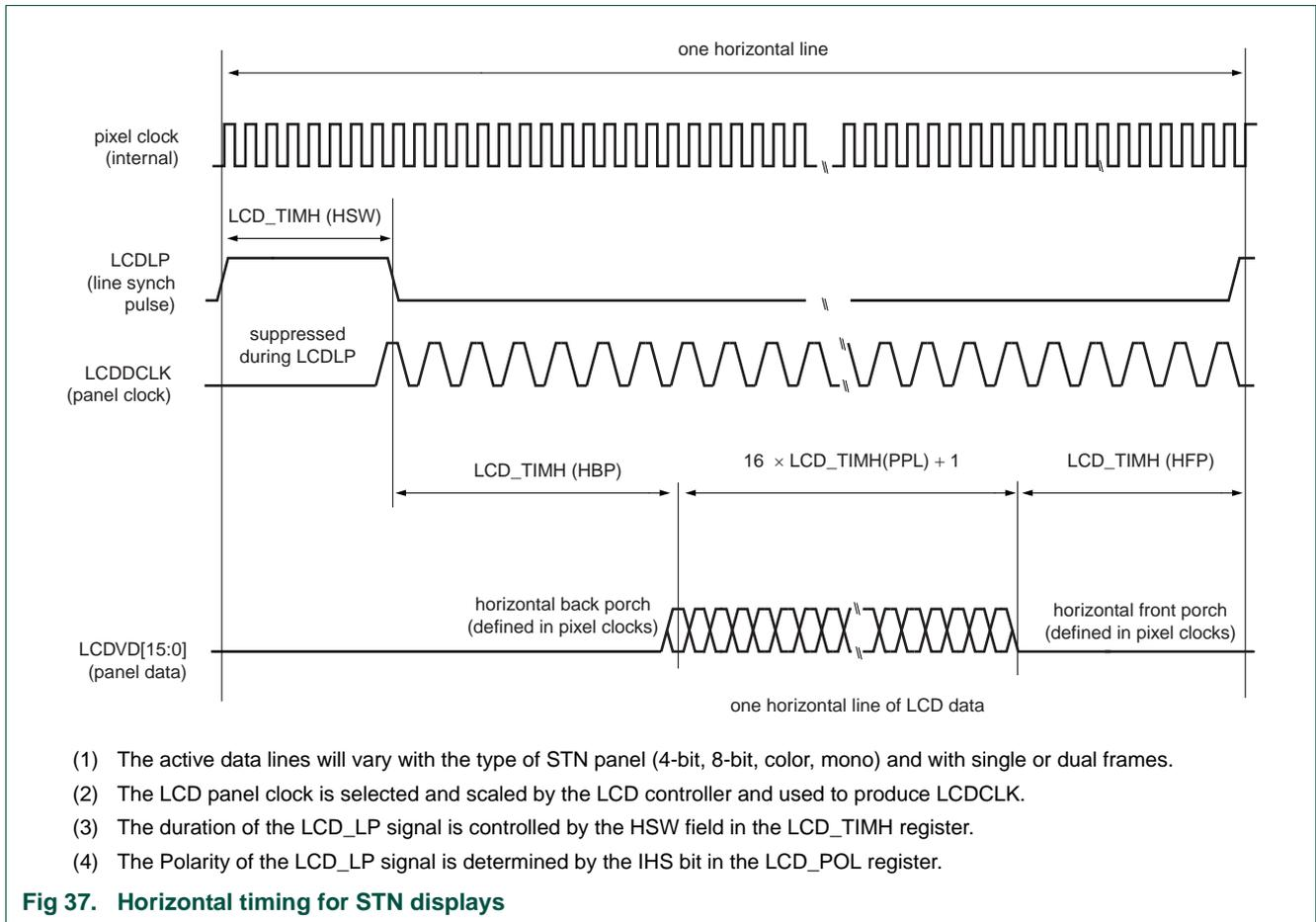
**Fig 37. Horizontal timing for STN displays**
