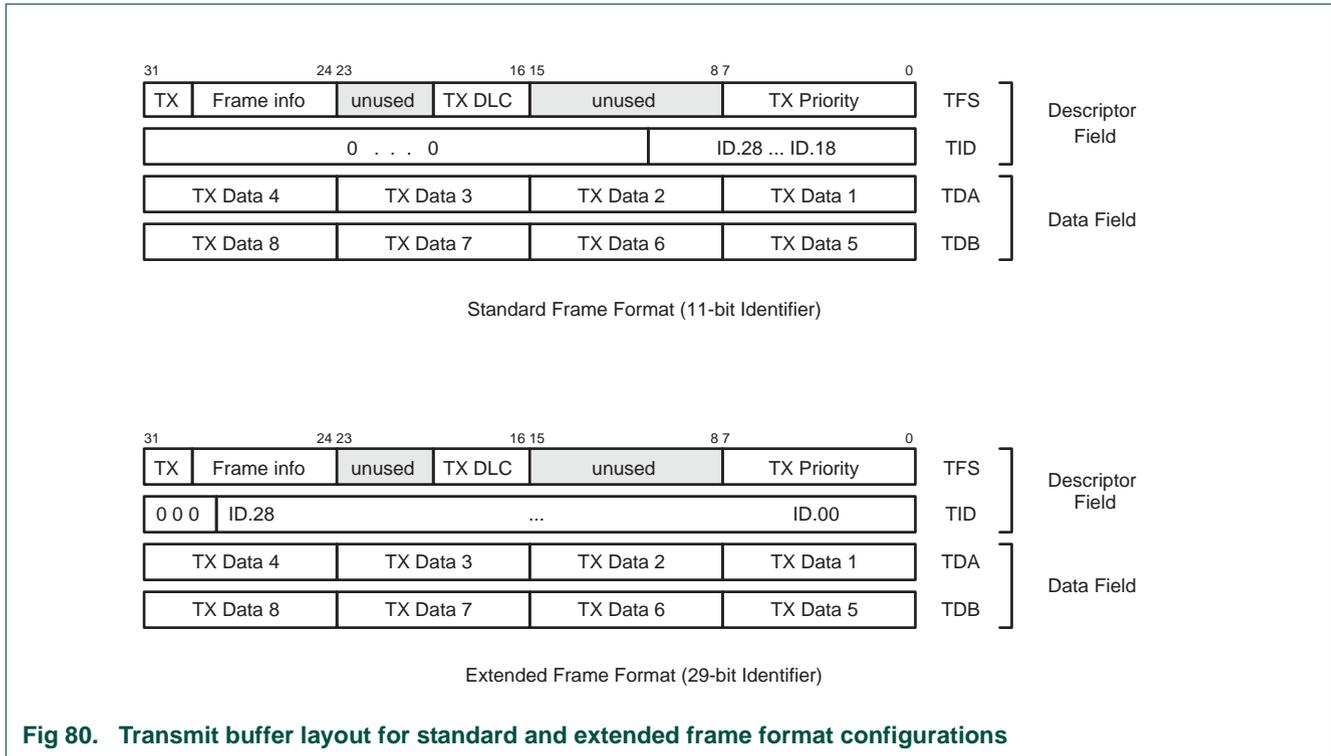
Fig 80. Transmit buffer layout for standard and extended frame format configurations
