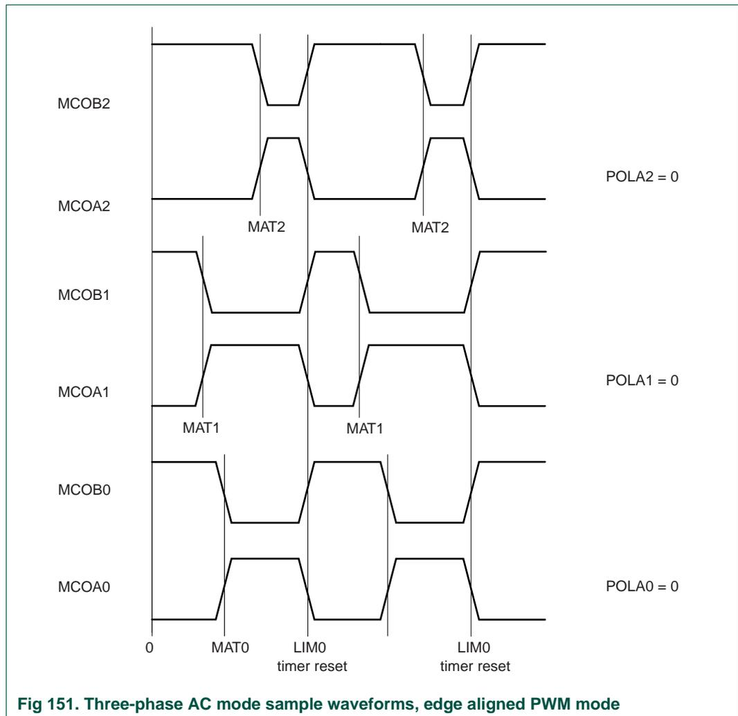
Fig 151. Three-phase AC mode sample waveforms, edge aligned PWM mode
