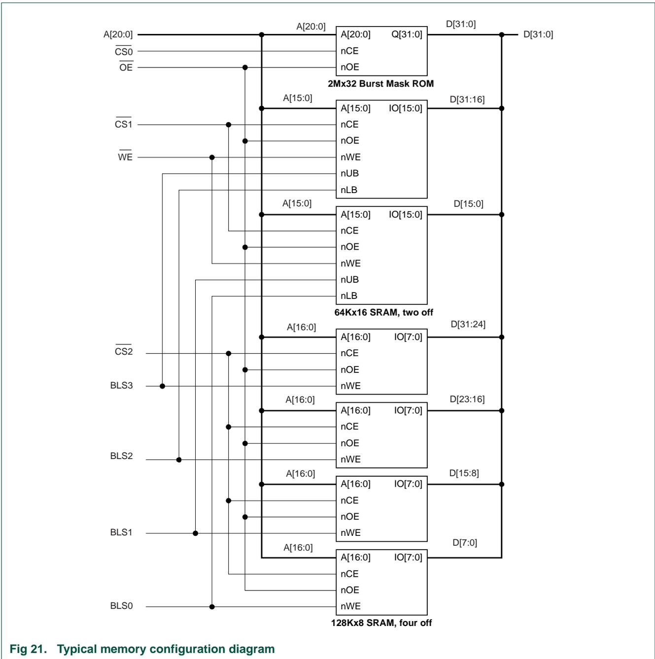
Fig 21. Typical memory configuration diagram
