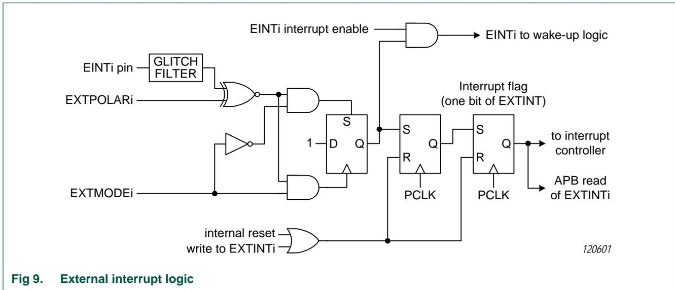
Fig 9. External interrupt logic
