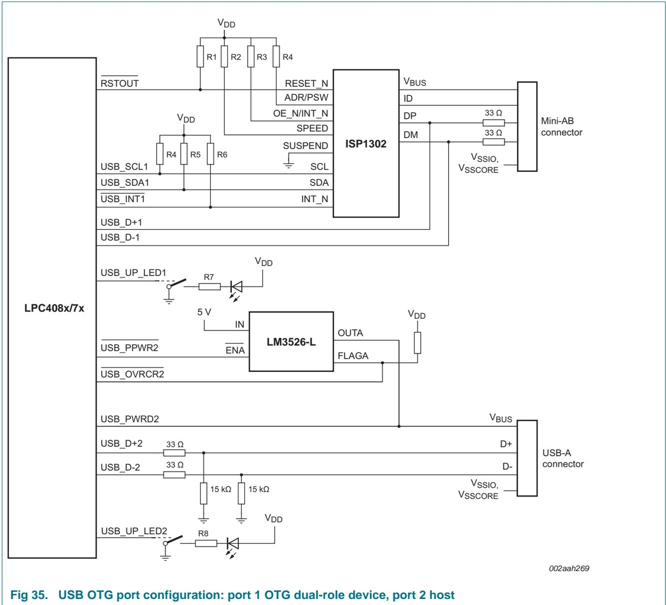
Fig 35. USB OTG port configuration: port 1 OTG dual-role device, port 2 host
