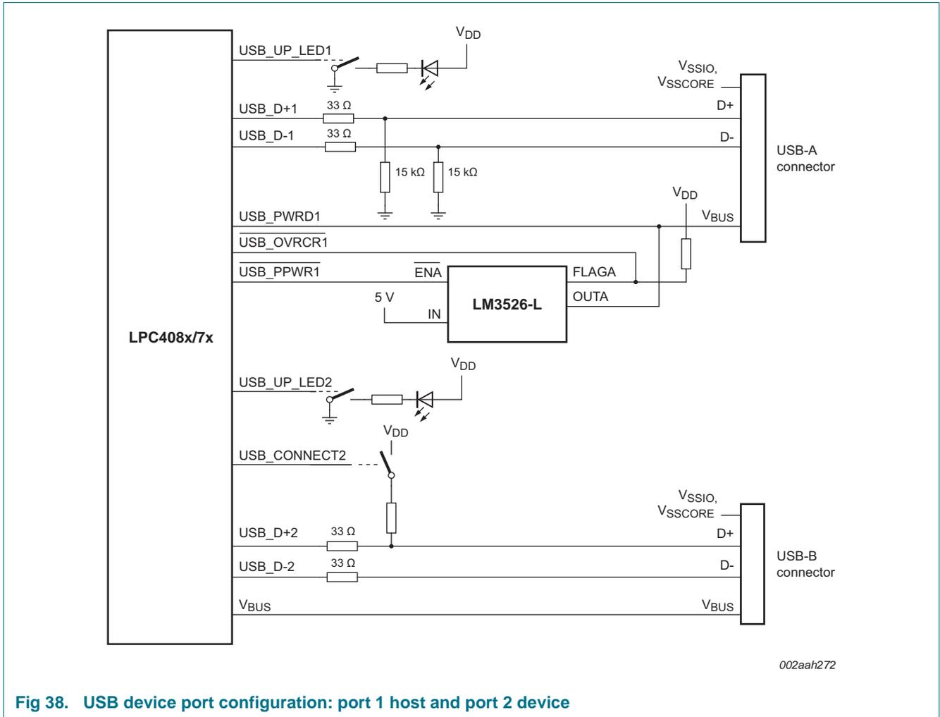
Fig 38. USB device port configuration: port 1 host and port 2 device
