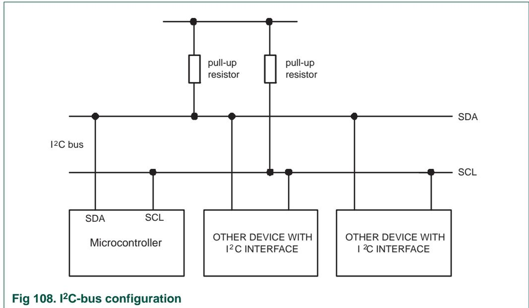
Fig 108. I<sup>2</sup>C-bus configuration
