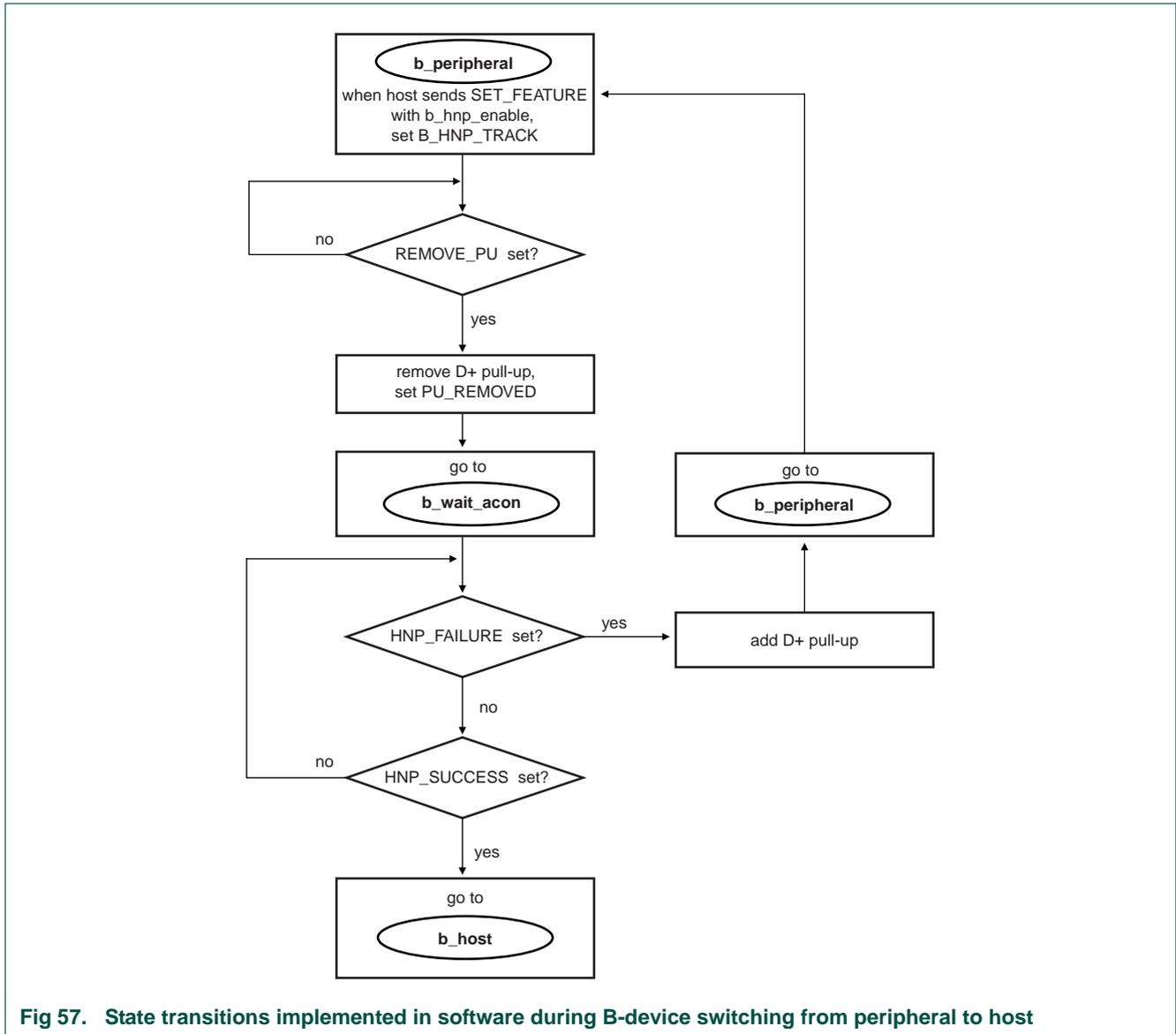
Fig 57. State transitions implemented in software during B-device switching from peripheral to host
