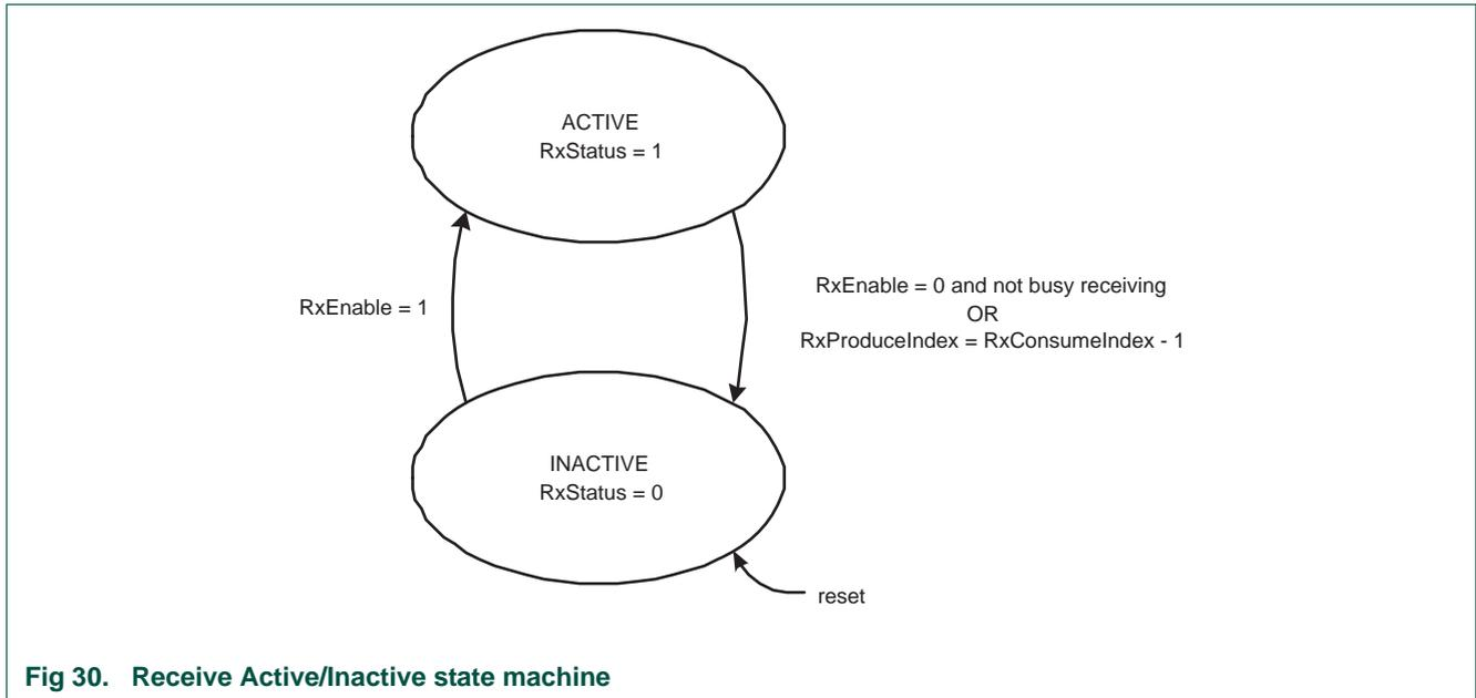
**Fig 30. Receive Active/Inactive state machine**
