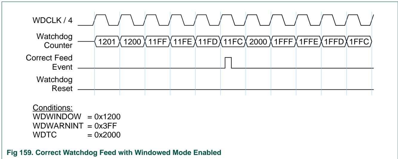
**Fig 159. Correct Watchdog Feed with Windowed Mode Enabled**
