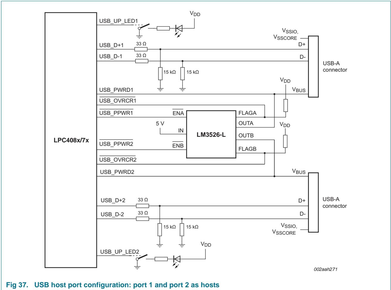
Fig 37. USB host port configuration: port 1 and port 2 as hosts
