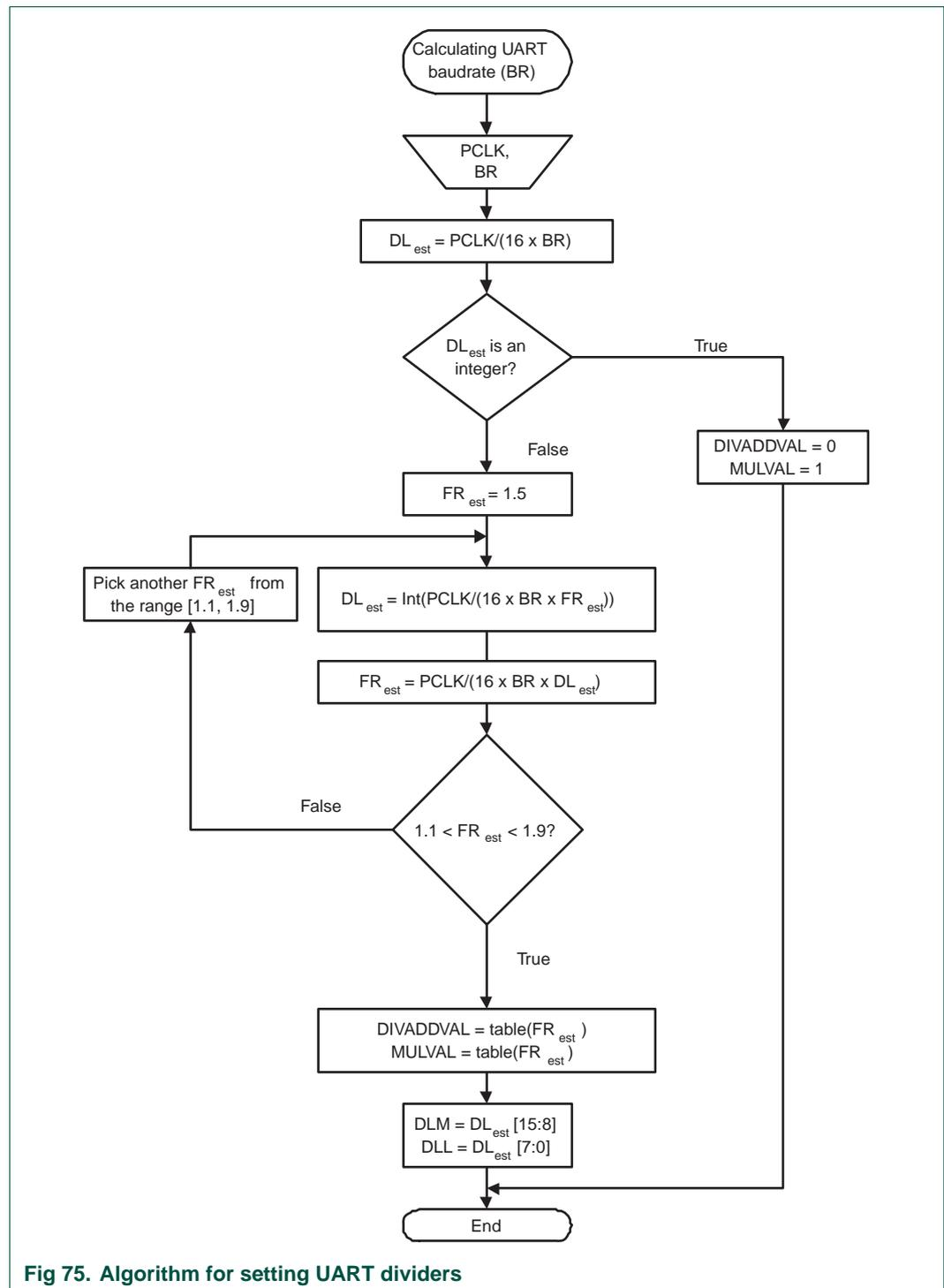
Fig 75. Algorithm for setting UART dividers
