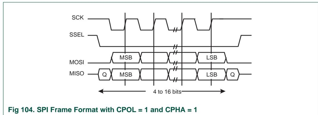
**Fig 104. SPI Frame Format with CPOL = 1 and CPHA = 1**
