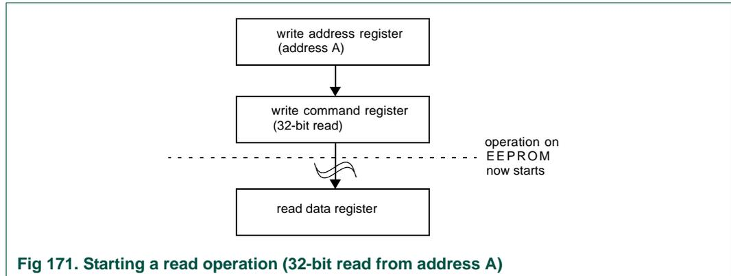
**Fig 171. Starting a read operation (32-bit read from address A)**
