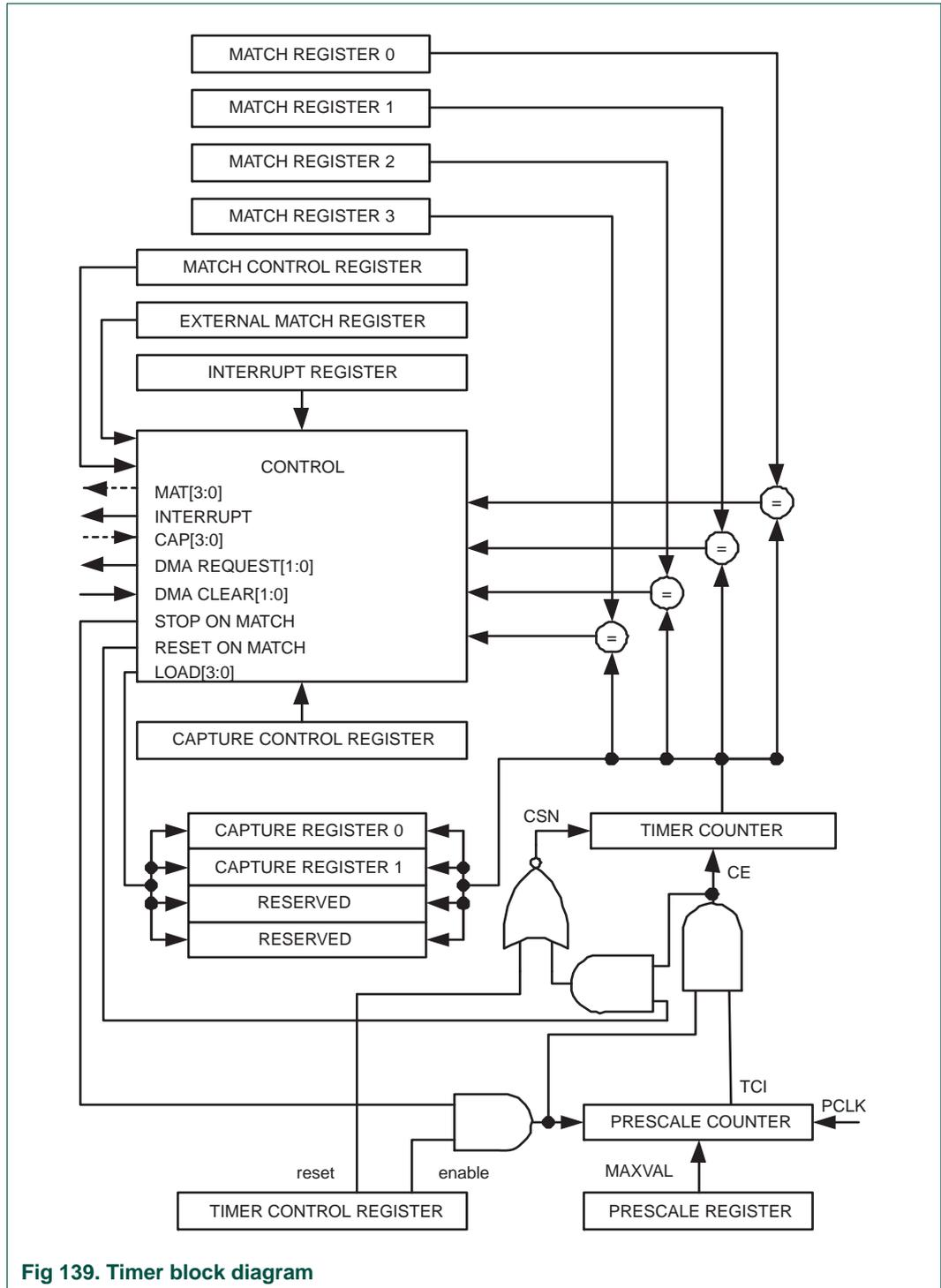
Fig 139. Timer block diagram
