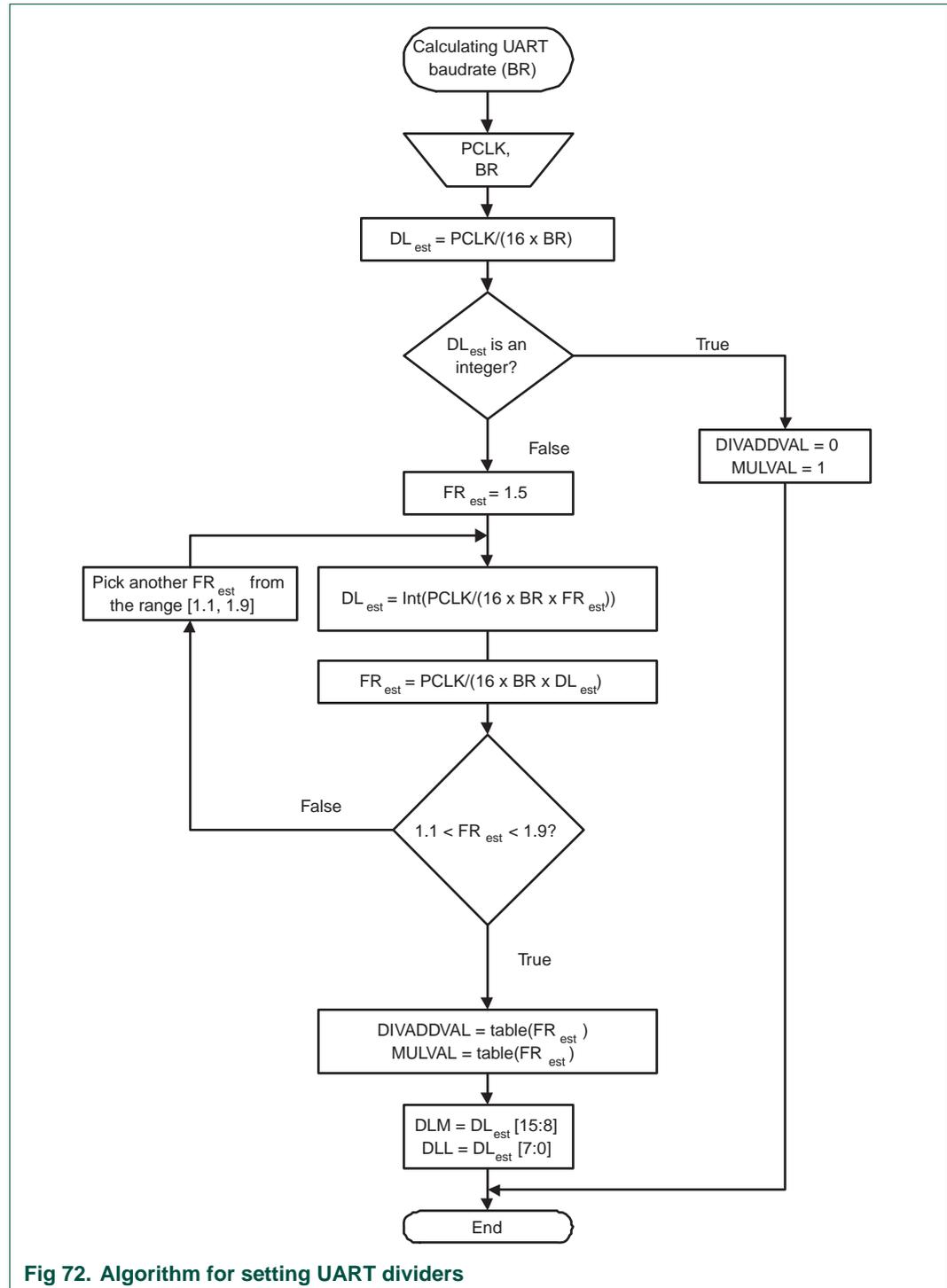
Fig 72. Algorithm for setting UART dividers
