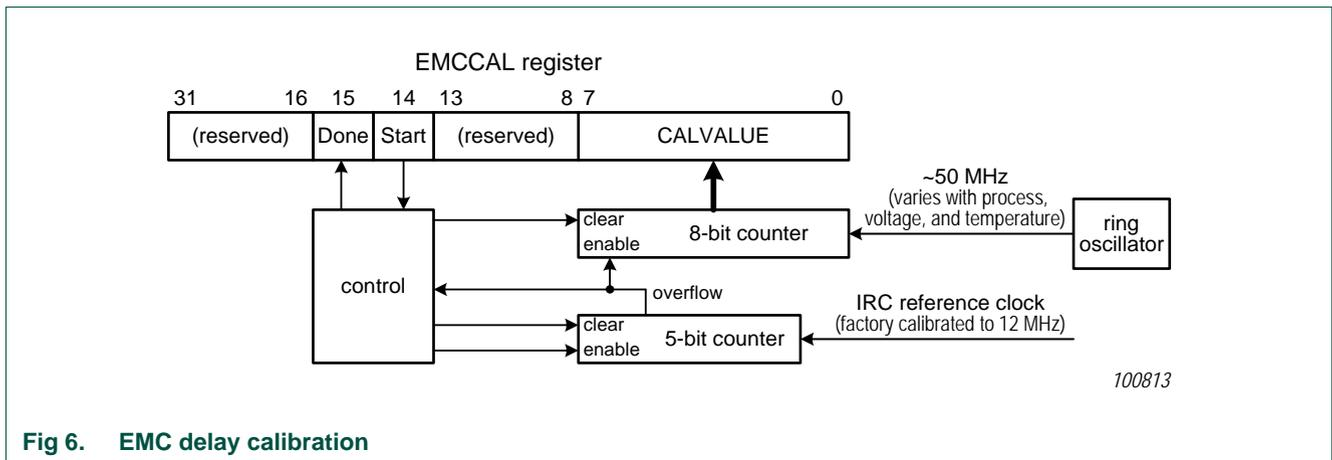
**Fig 6. EMC delay calibration**
