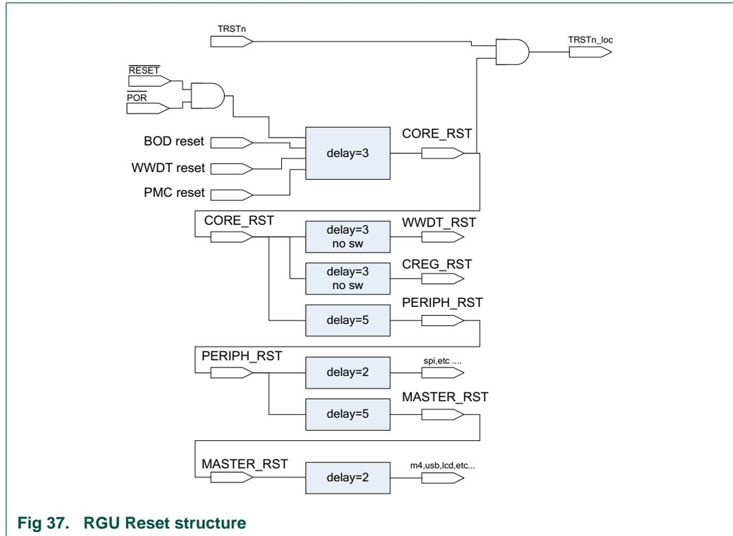
Fig 37. RGU Reset structure
