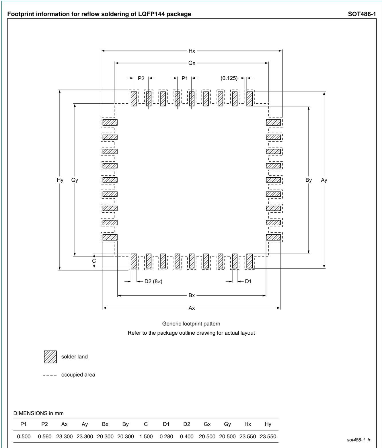
Fig 57. Reflow soldering of the LQFP144 package
