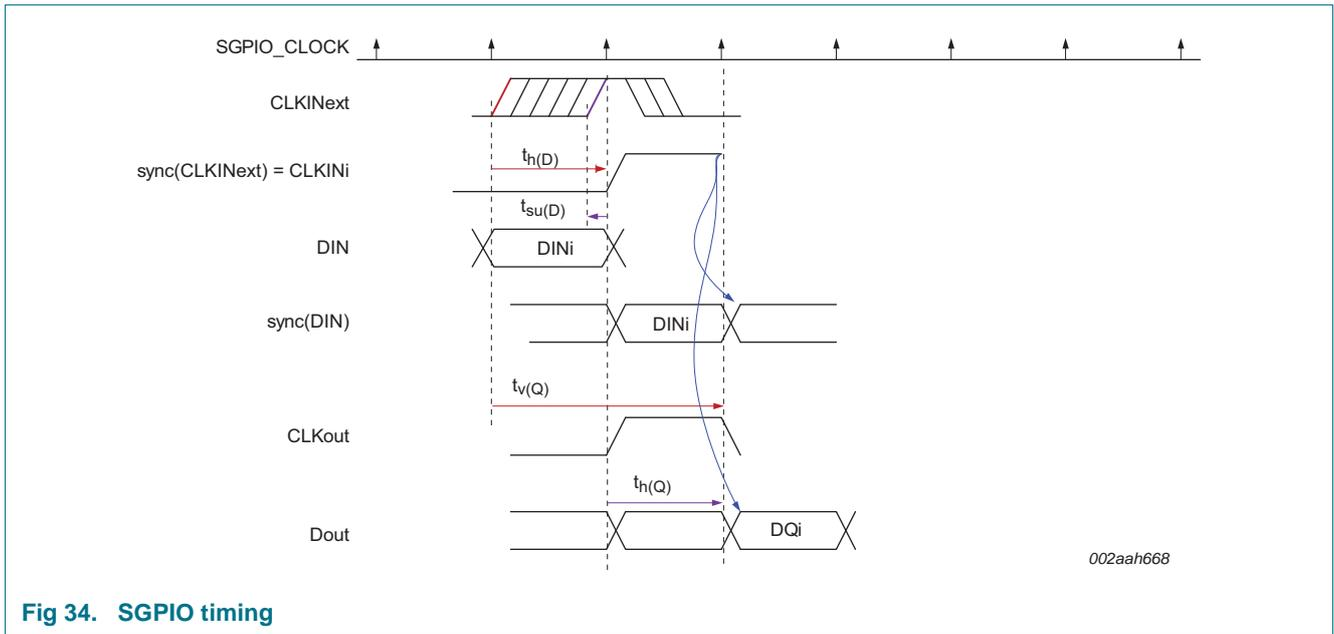
**Fig 34. SGPIO timing**
