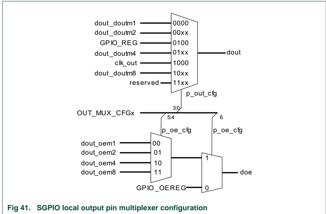
Fig 41. SGPIO local output pin multiplexer configuration
