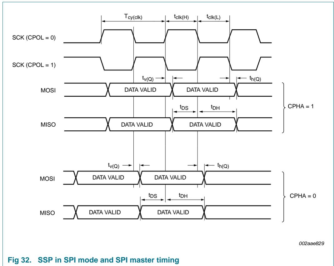
Fig 32. SSP in SPI mode and SPI master timing
