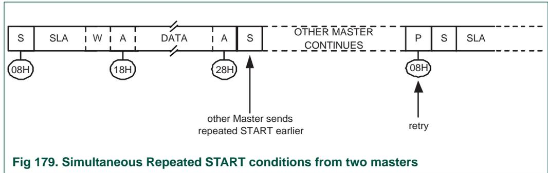
Fig 179. Simultaneous Repeated START conditions from two masters
