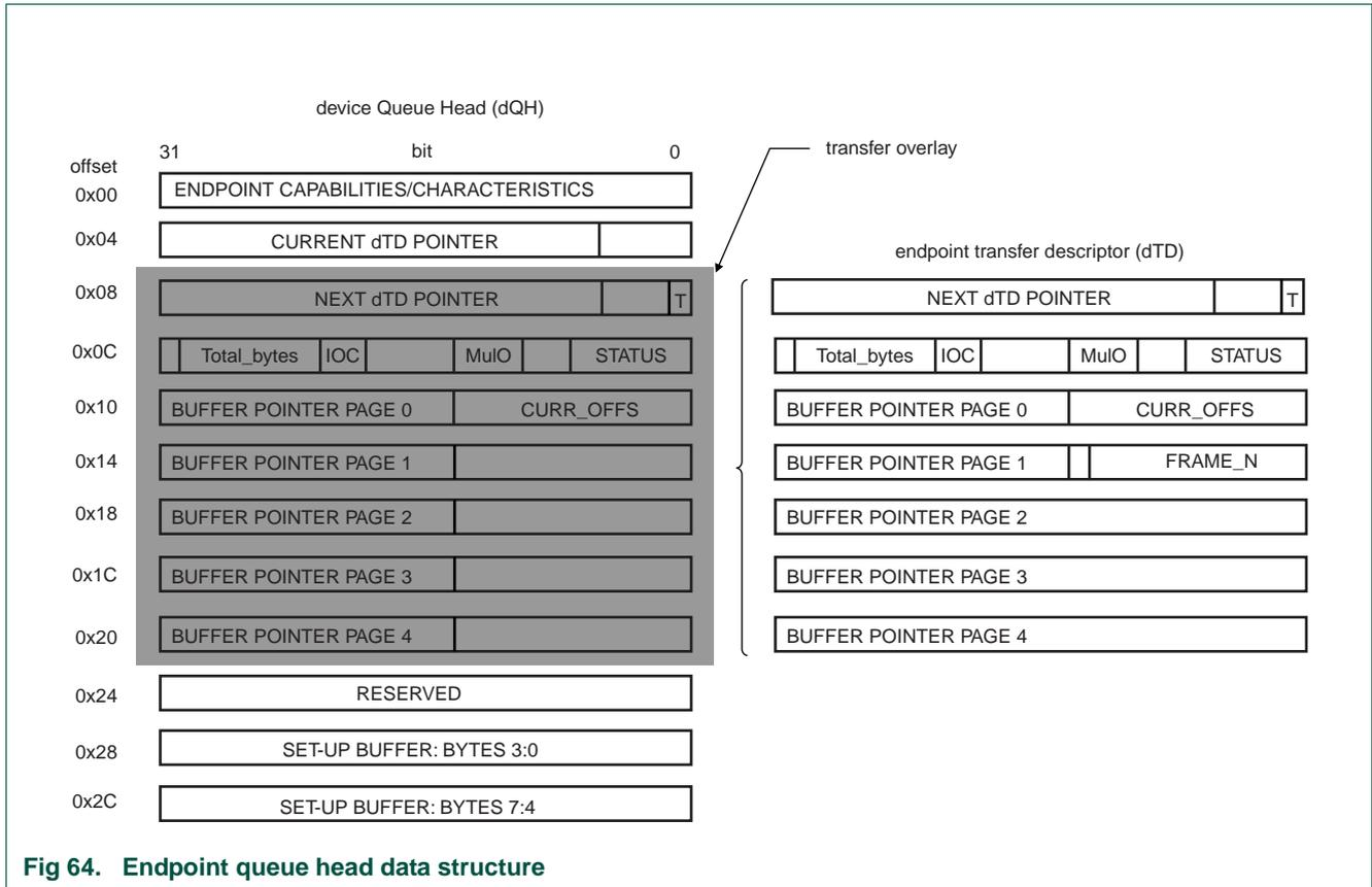
Fig 64. Endpoint queue head data structure
