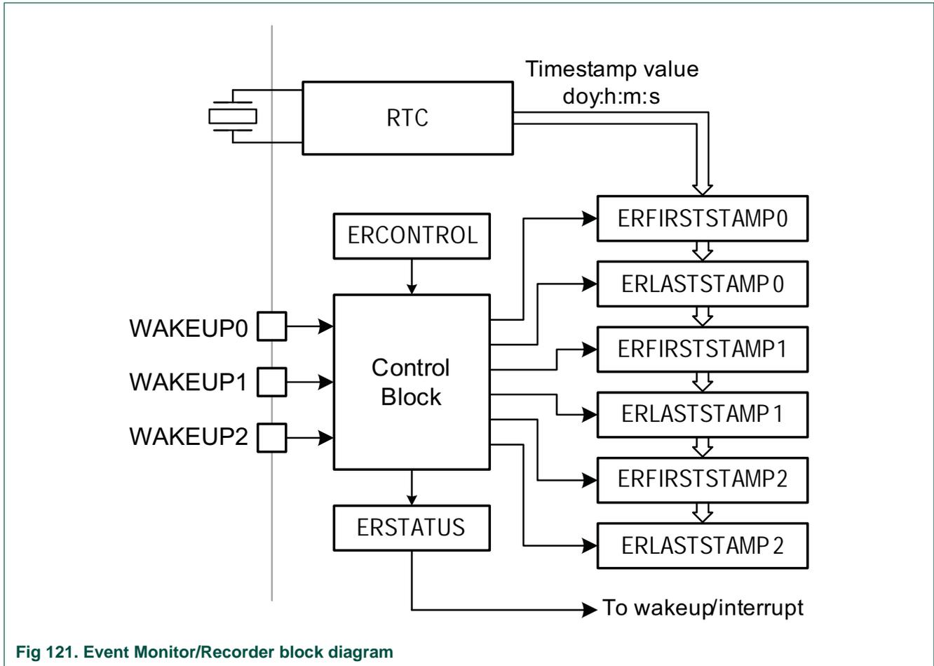
Fig 121. Event Monitor/Recorder block diagram
