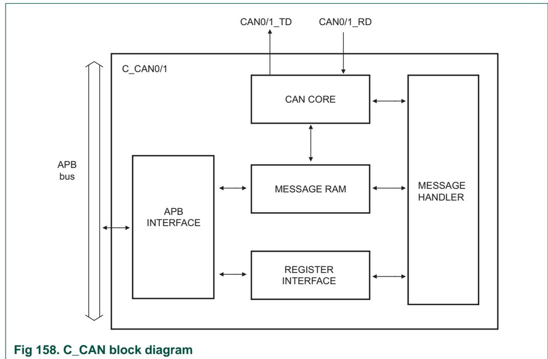
Fig 158. C\_CAN block diagram
