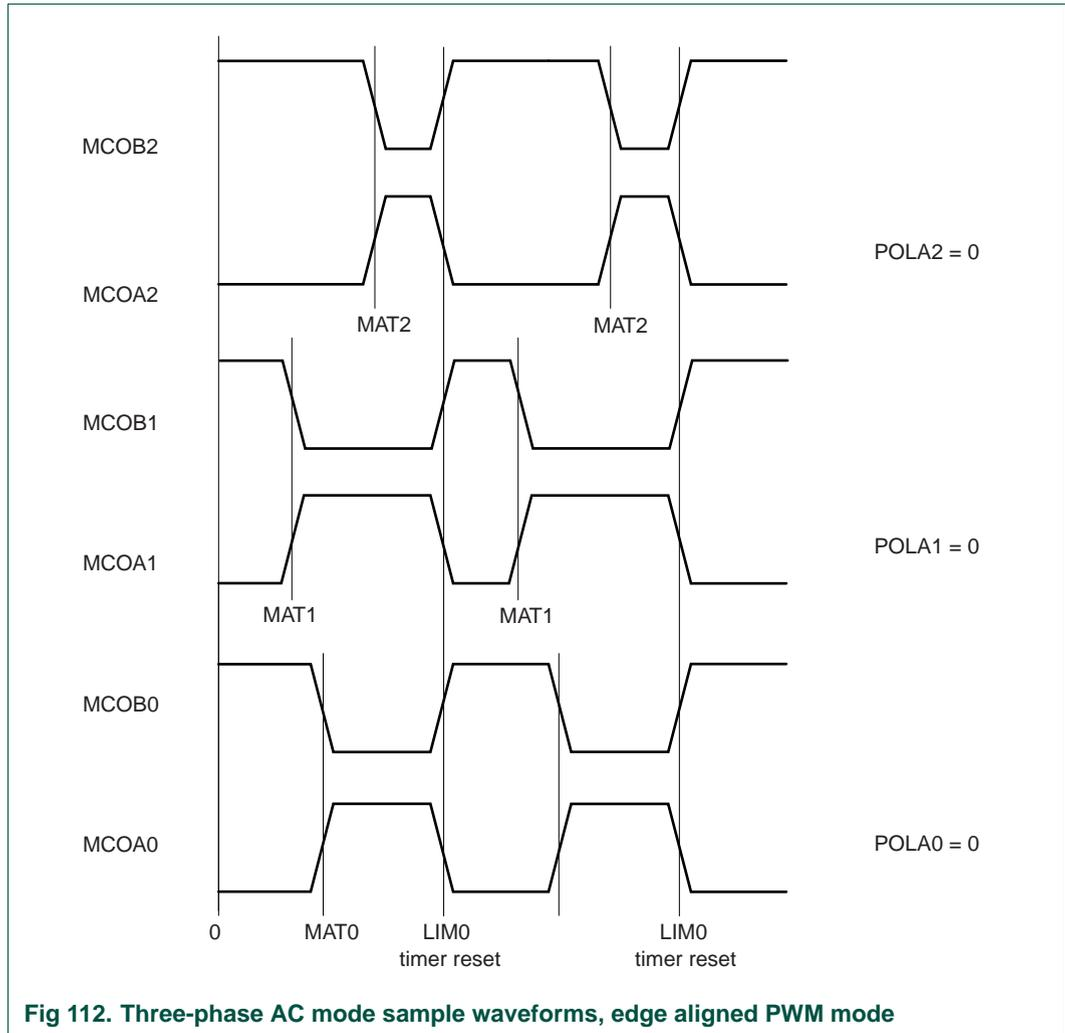
Fig 112. Three-phase AC mode sample waveforms, edge aligned PWM mode
