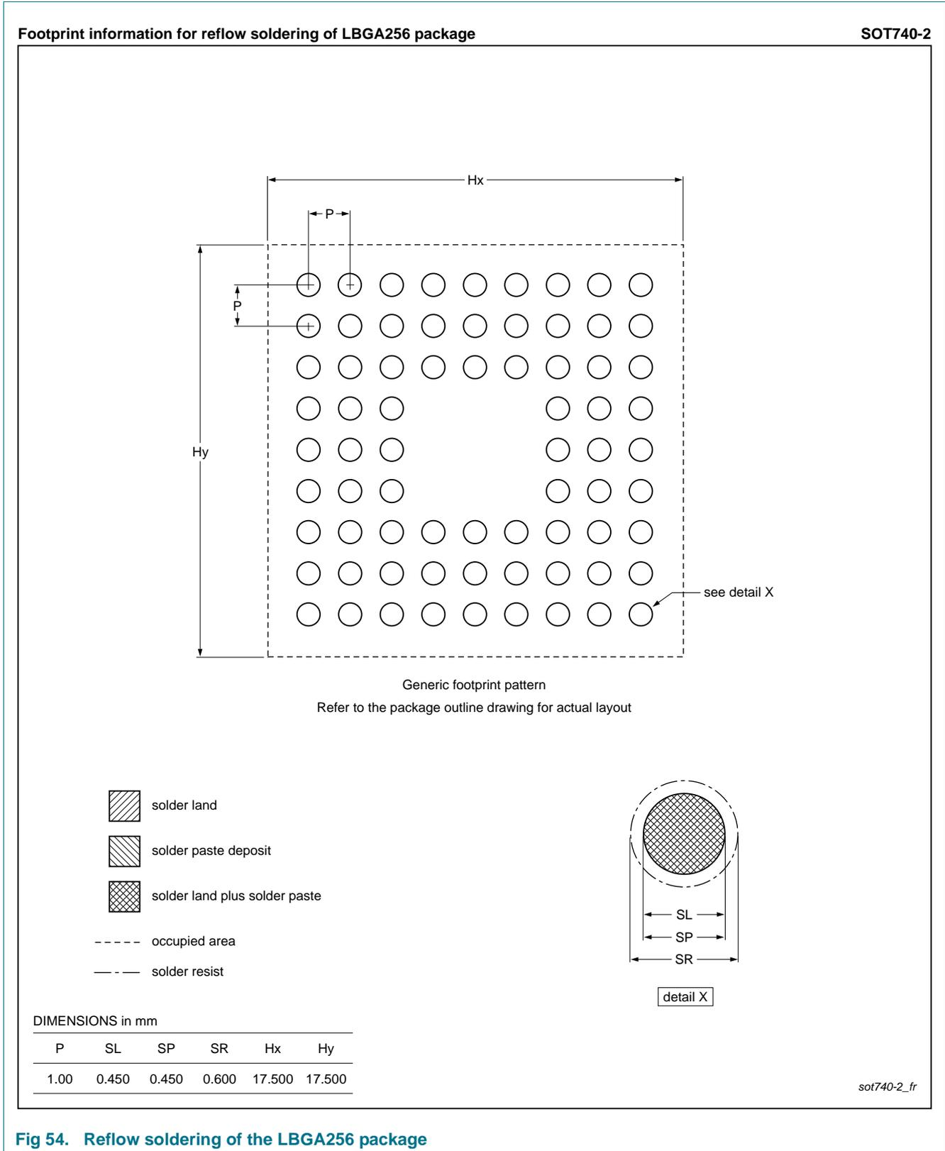
Fig 54. Reflow soldering of the LPGA256 package
