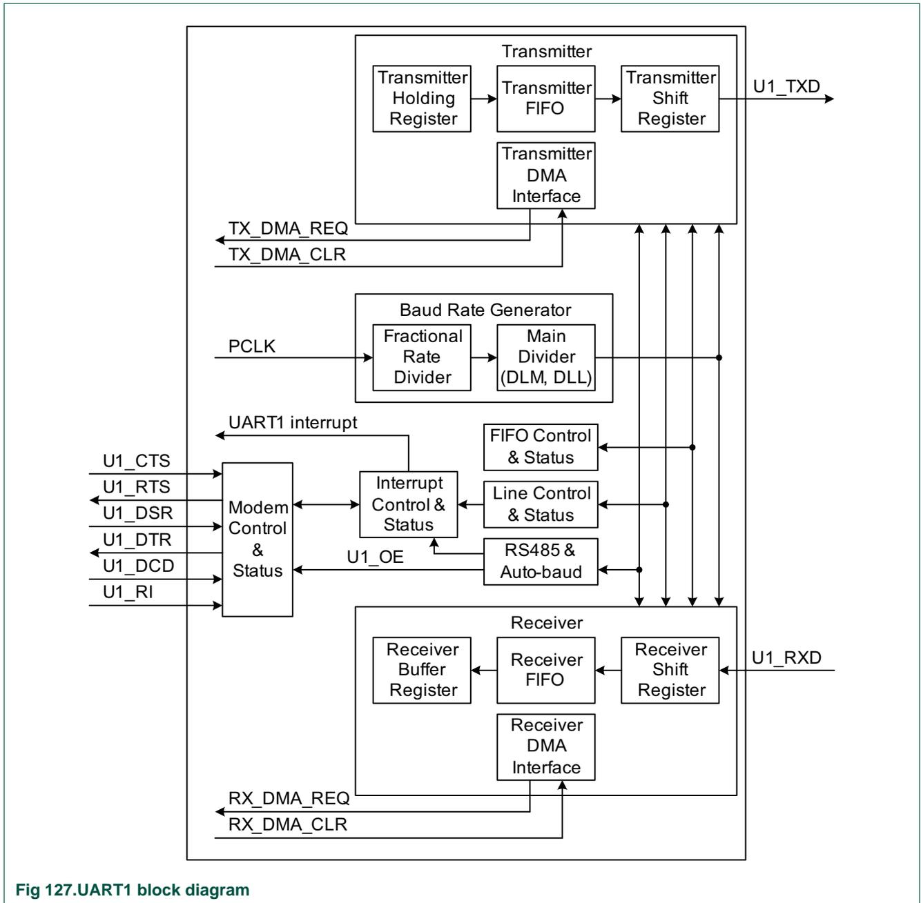
Fig 127. UART1 block diagram
