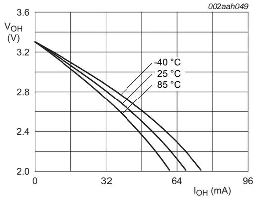
Conditions:  $V_{DD(REG)(3V3)} = V_{DD(IO)} = 3.3$  V; high-drive; EHD = 0x2.
