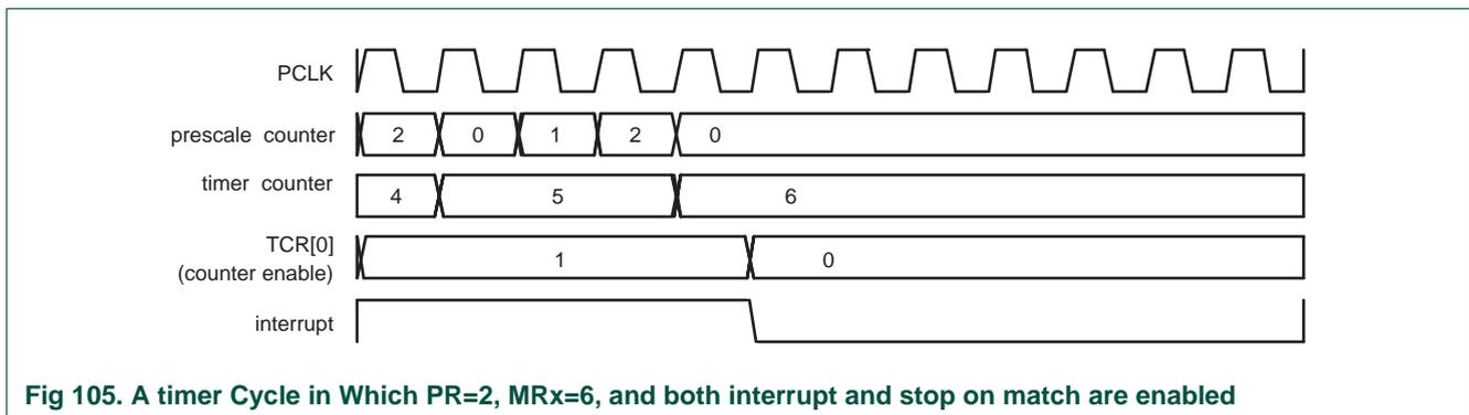
**Fig 105. A timer Cycle in Which PR=2, MRx=6, and both interrupt and stop on match are enabled**
