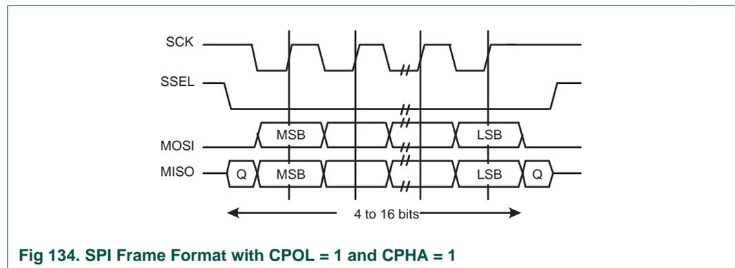
**Fig 134. SPI Frame Format with CPOL = 1 and CPHA = 1**
