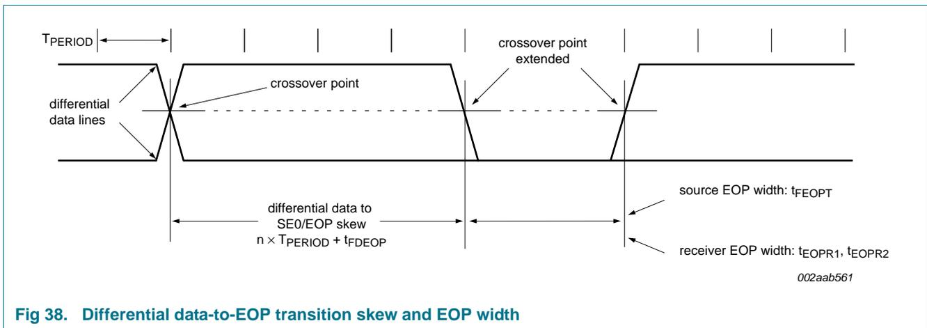
Fig 38. Differential data-to-EOP transition skew and EOP width
