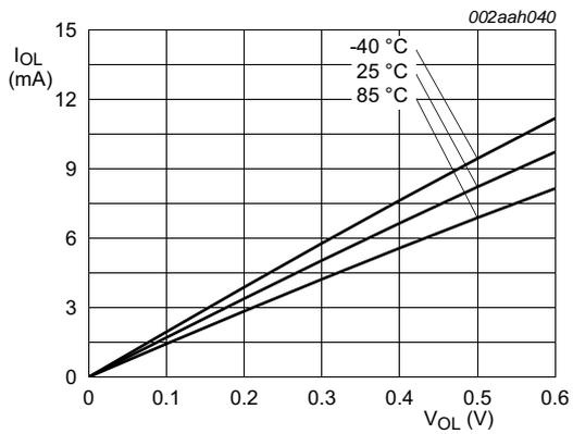
Conditions:  $V_{DD(REG)(3V3)} = V_{DD(IO)} = 3.3$  V; normal-drive; EHD = 0x0.
