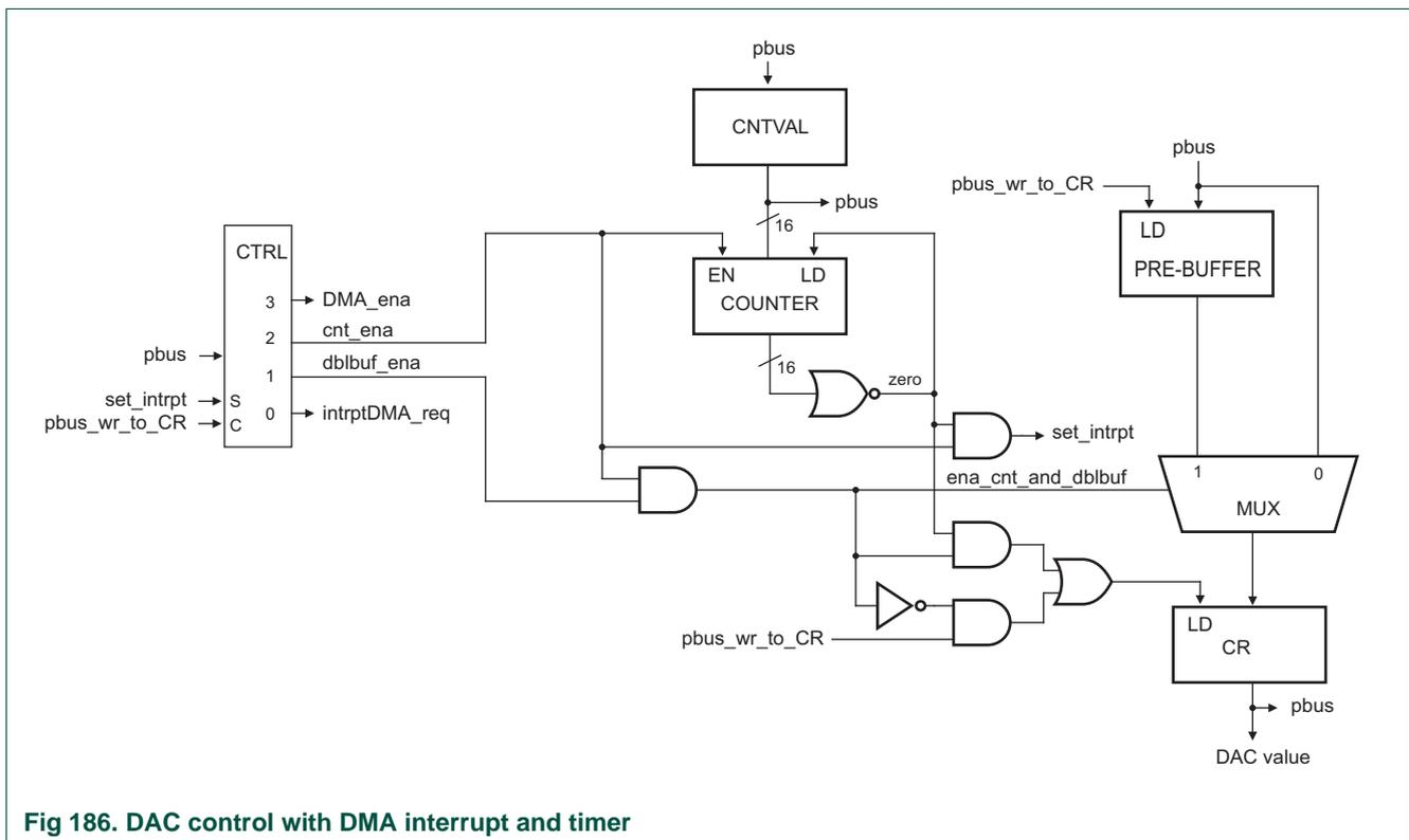
Fig 186. DAC control with DMA interrupt and timer
