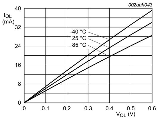
Conditions:  $V_{DD(REG)(3V3)} = V_{DD(IO)} = 3.3$  V; high-drive; EHD = 0x2.
