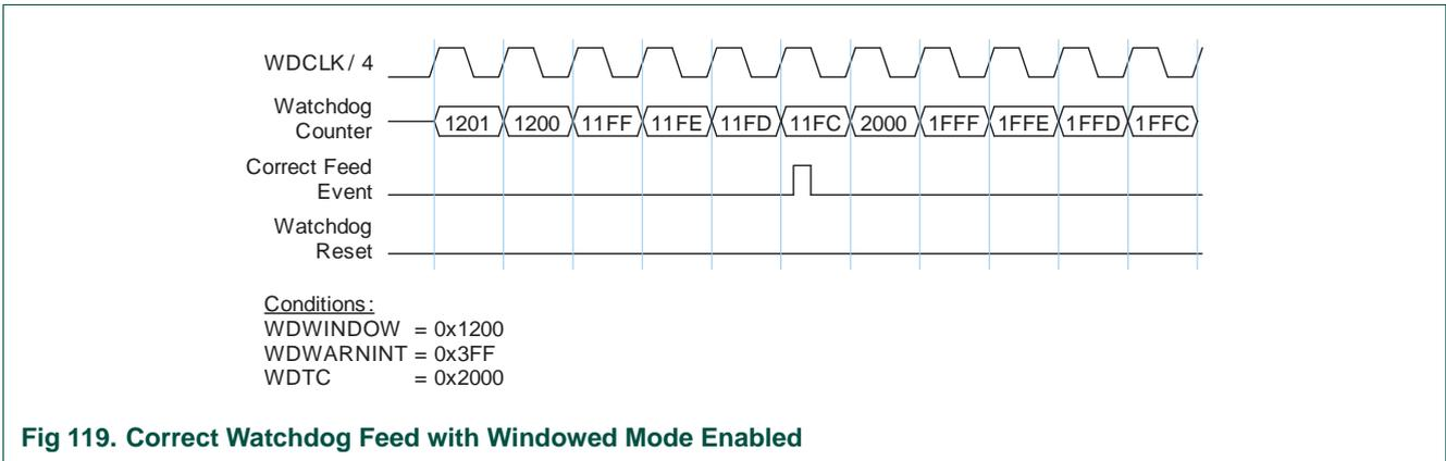
Fig 119. Correct Watchdog Feed with Windowed Mode Enabled
