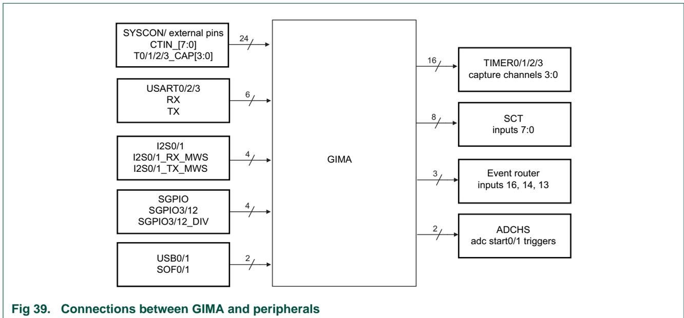
Fig 39. Connections between GIMA and peripherals
