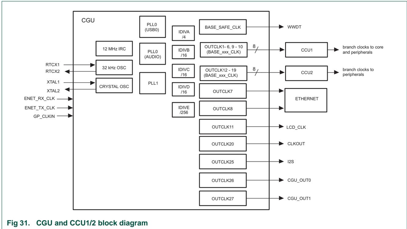
Fig 31. CGU and CCU1/2 block diagram
