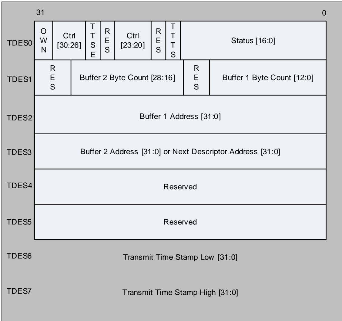
**Fig 83. Transmitter descriptor fields**
