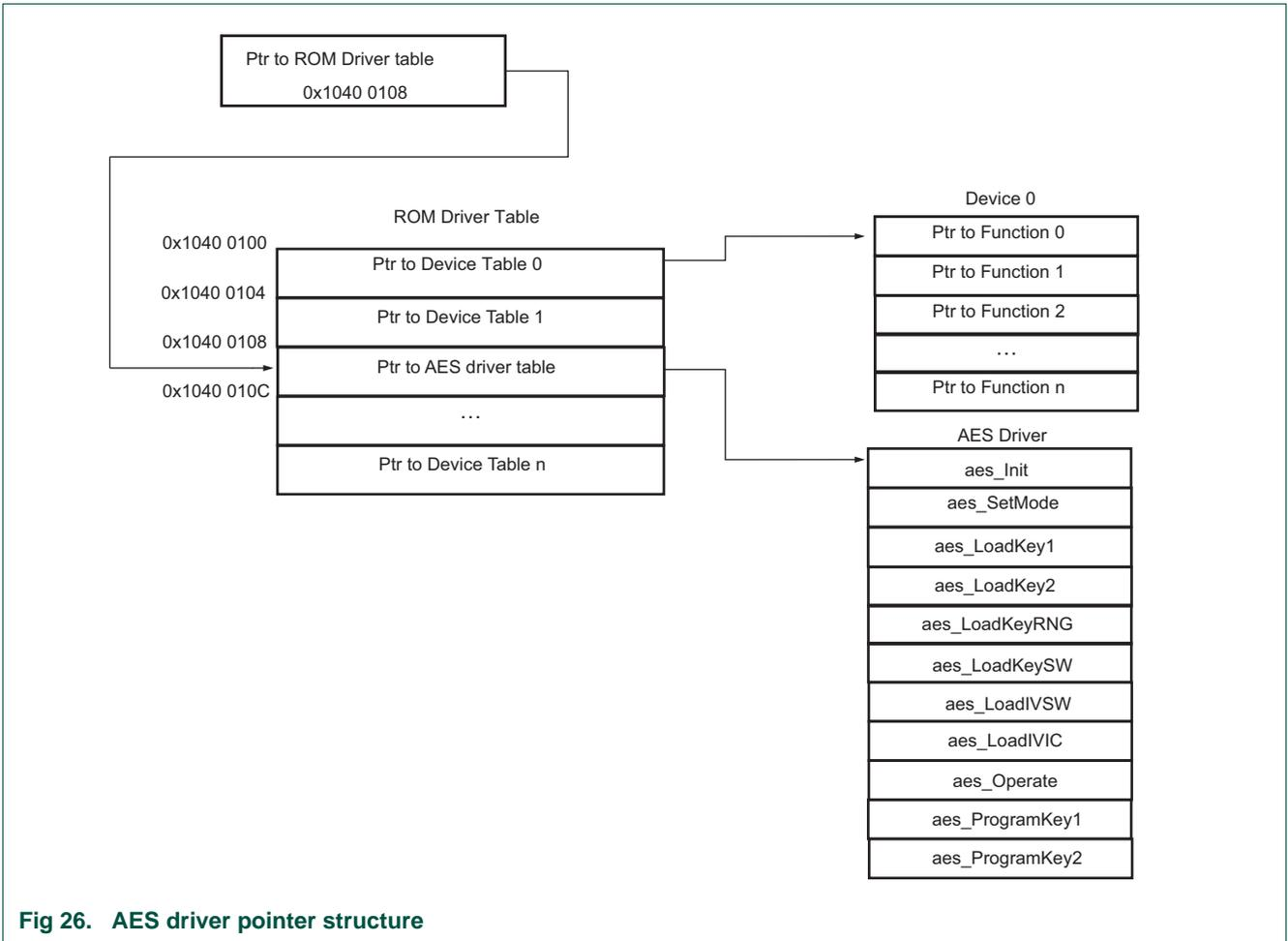
Fig 26. AES driver pointer structure
