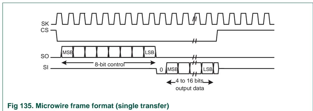
Fig 135. Microwire frame format (single transfer)
