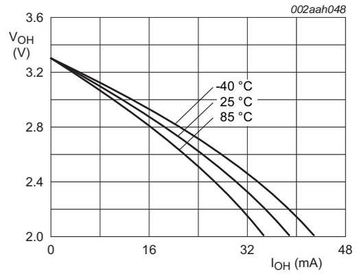
Conditions:  $V_{DD(REG)(3V3)} = V_{DD(IO)} = 3.3$  V; medium-drive; EHD = 0x1.
