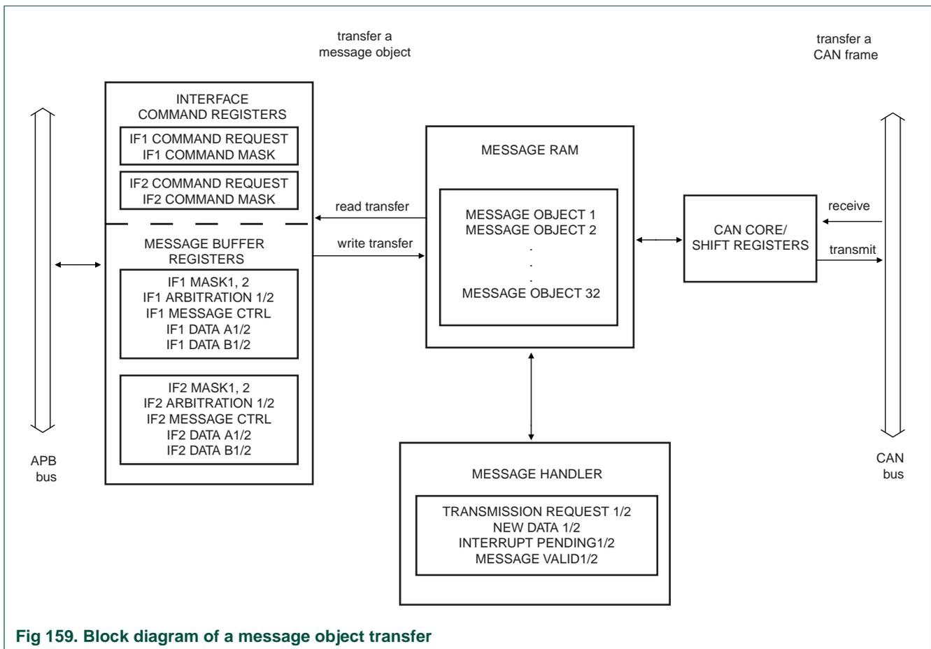
Fig 159. Block diagram of a message object transfer
