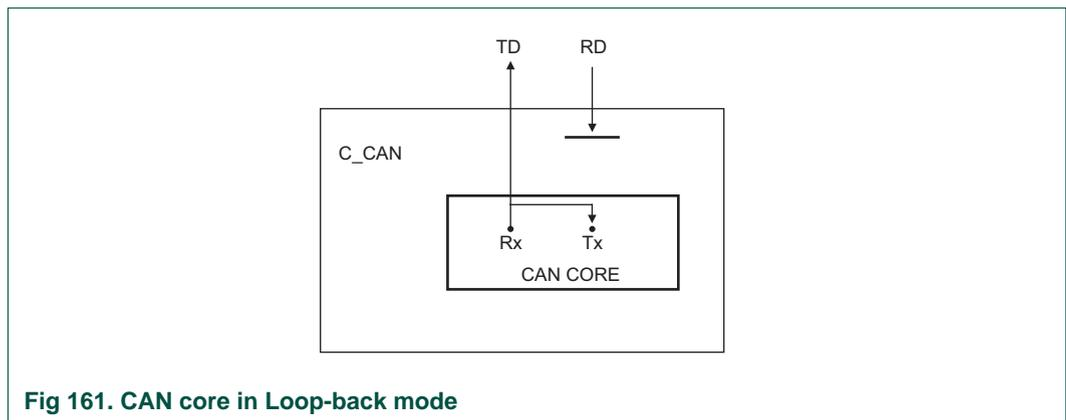
Fig 161. CAN core in Loop-back mode
