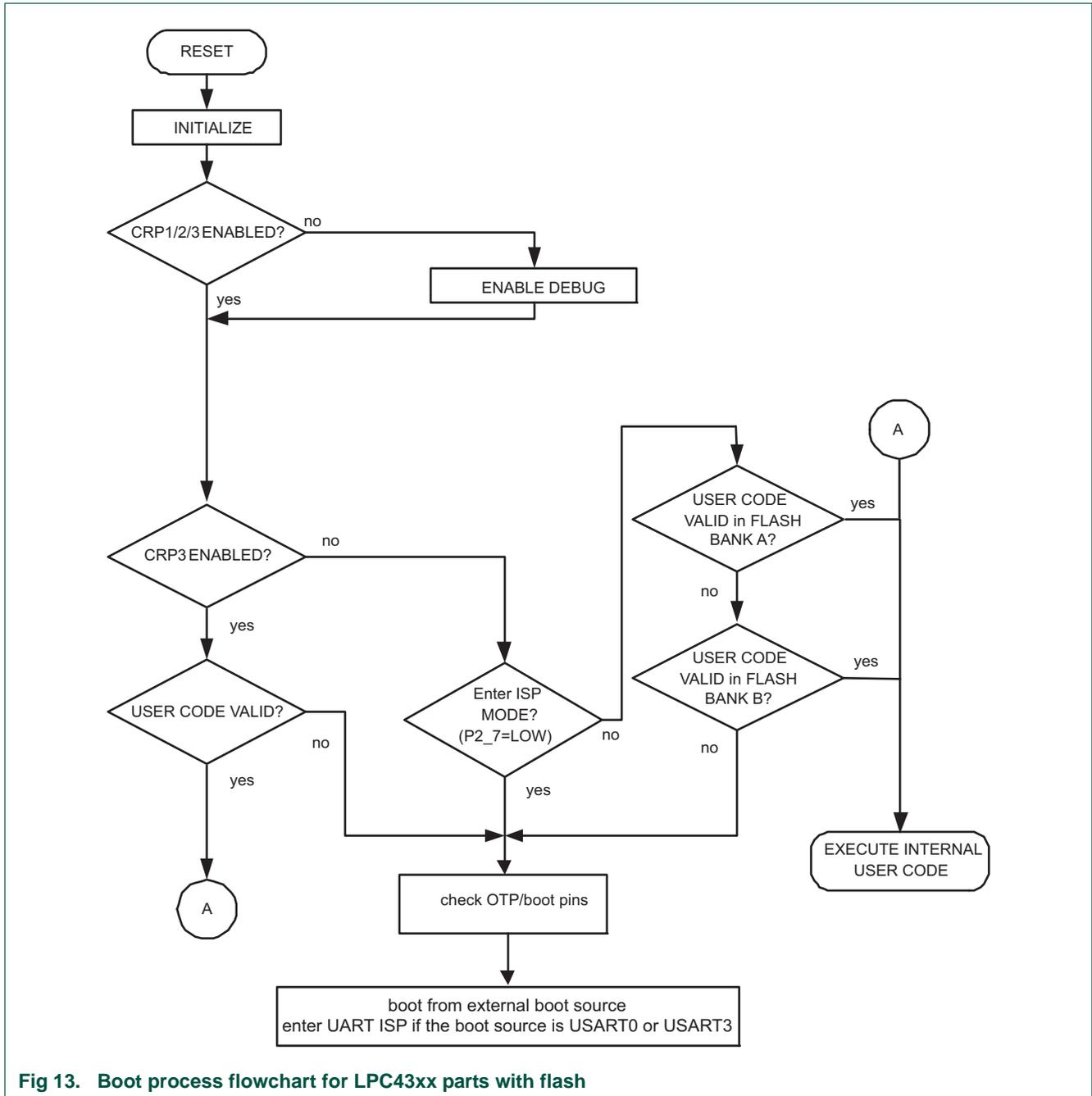
Fig 13. Boot process flowchart for LPC43xx parts with flash
