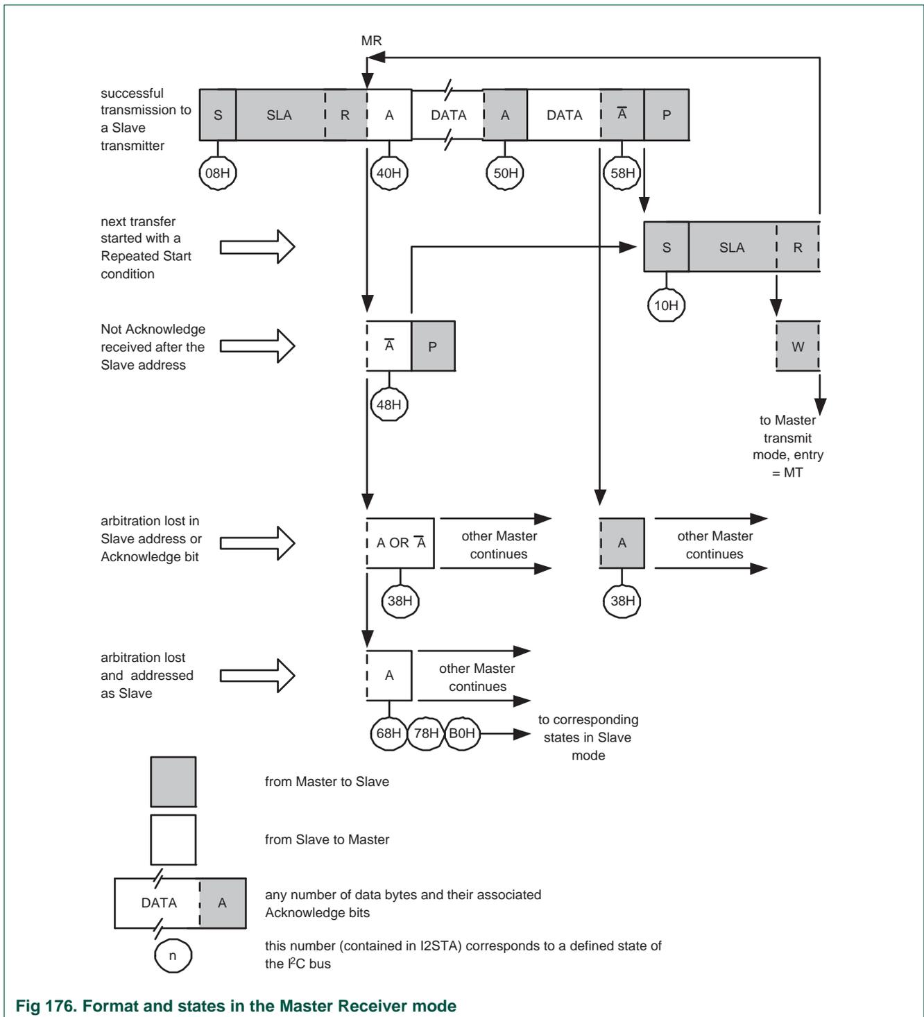
Fig 176. Format and states in the Master Receiver mode
