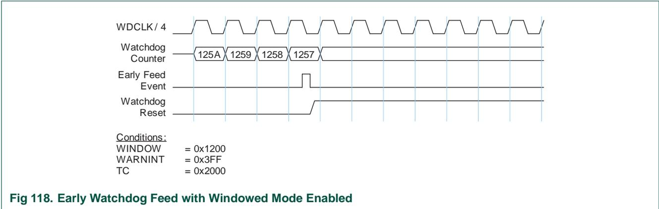
Fig 118. Early Watchdog Feed with Windowed Mode Enabled
