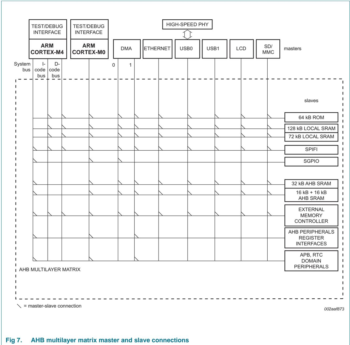
Fig 7. AHB multilayer matrix master and slave connections
