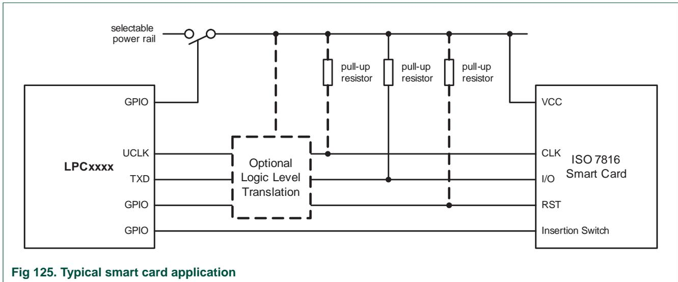
Fig 125. Typical smart card application
