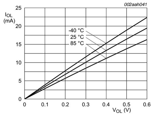
Conditions:  $V_{DD(REG)(3V3)} = V_{DD(IO)} = 3.3$  V; medium-drive; EHD = 0x1.
