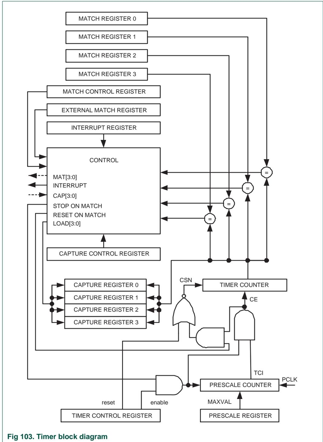
Fig 103. Timer block diagram
