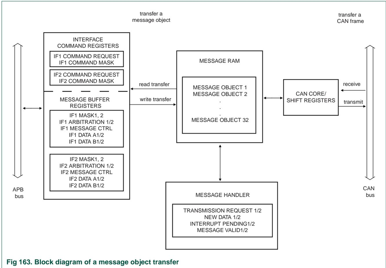
Fig 163. Block diagram of a message object transfer
