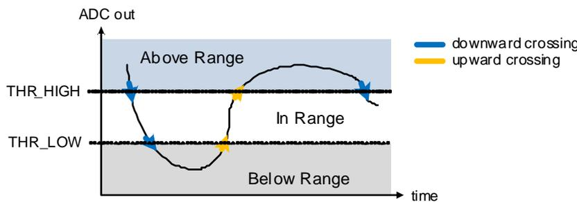
**Fig 185. Threshold detection**
