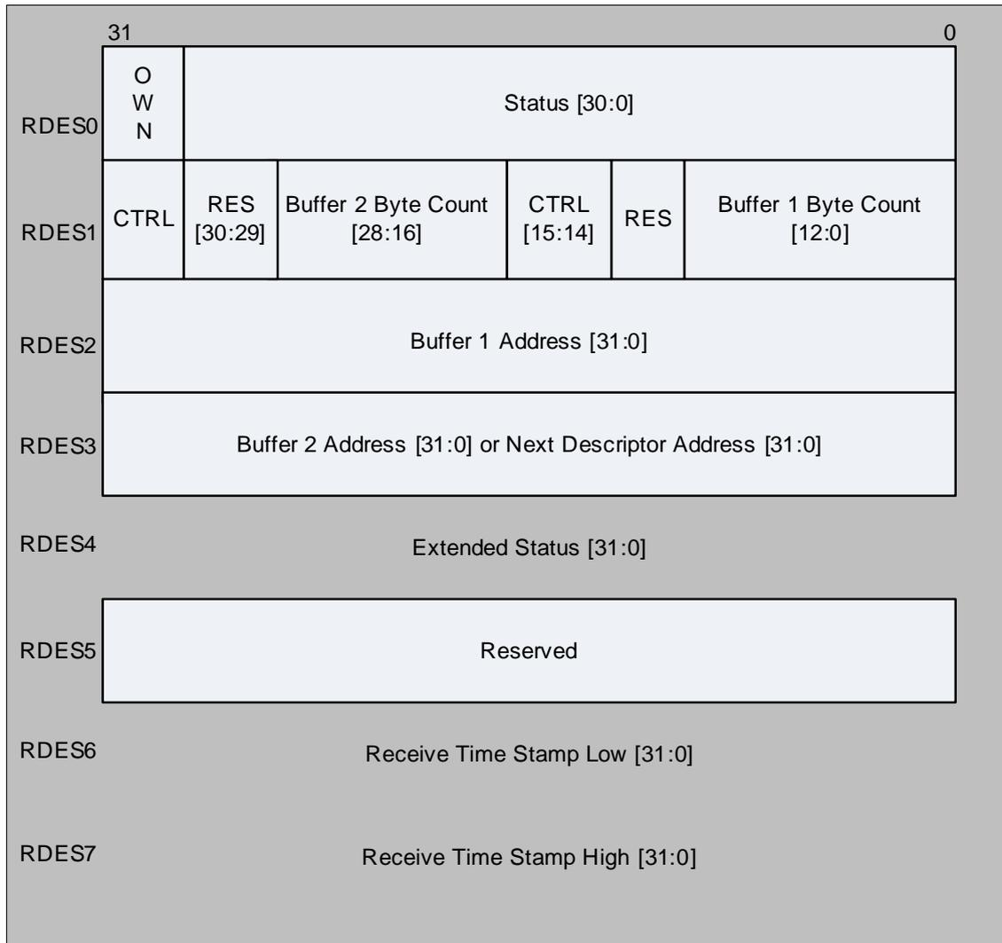
**Fig 85. Receive descriptor fields (alternate configuration)**
