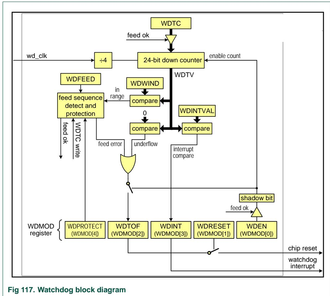
Fig 117. Watchdog block diagram
