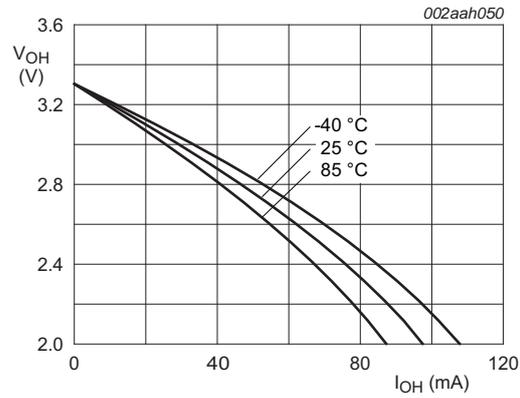
Conditions:  $V_{DD(REG)(3V3)} = V_{DD(IO)} = 3.3$  V; ultra high-drive; EHD = 0x3.
