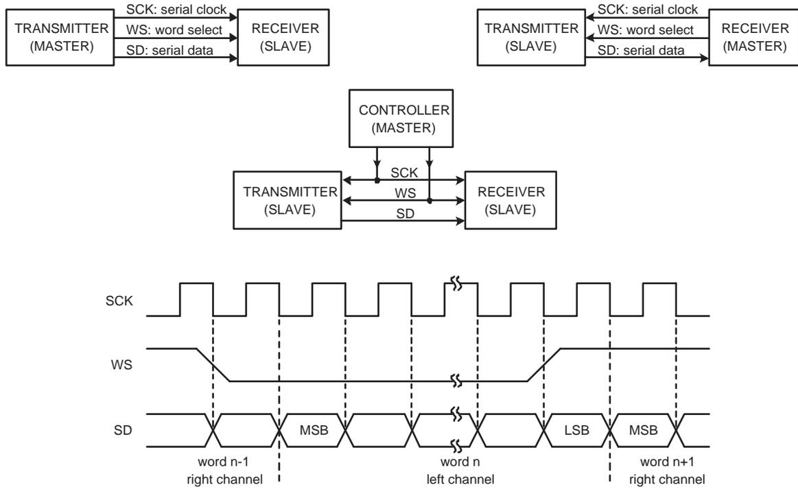
Fig 141. Simple I2S configurations and bus timing
