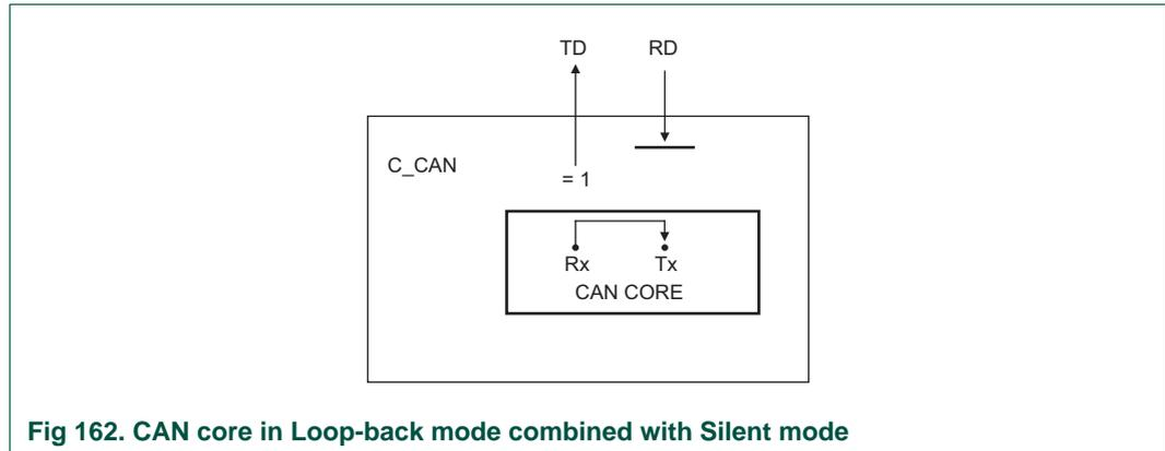
Fig 162. CAN core in Loop-back mode combined with Silent mode
