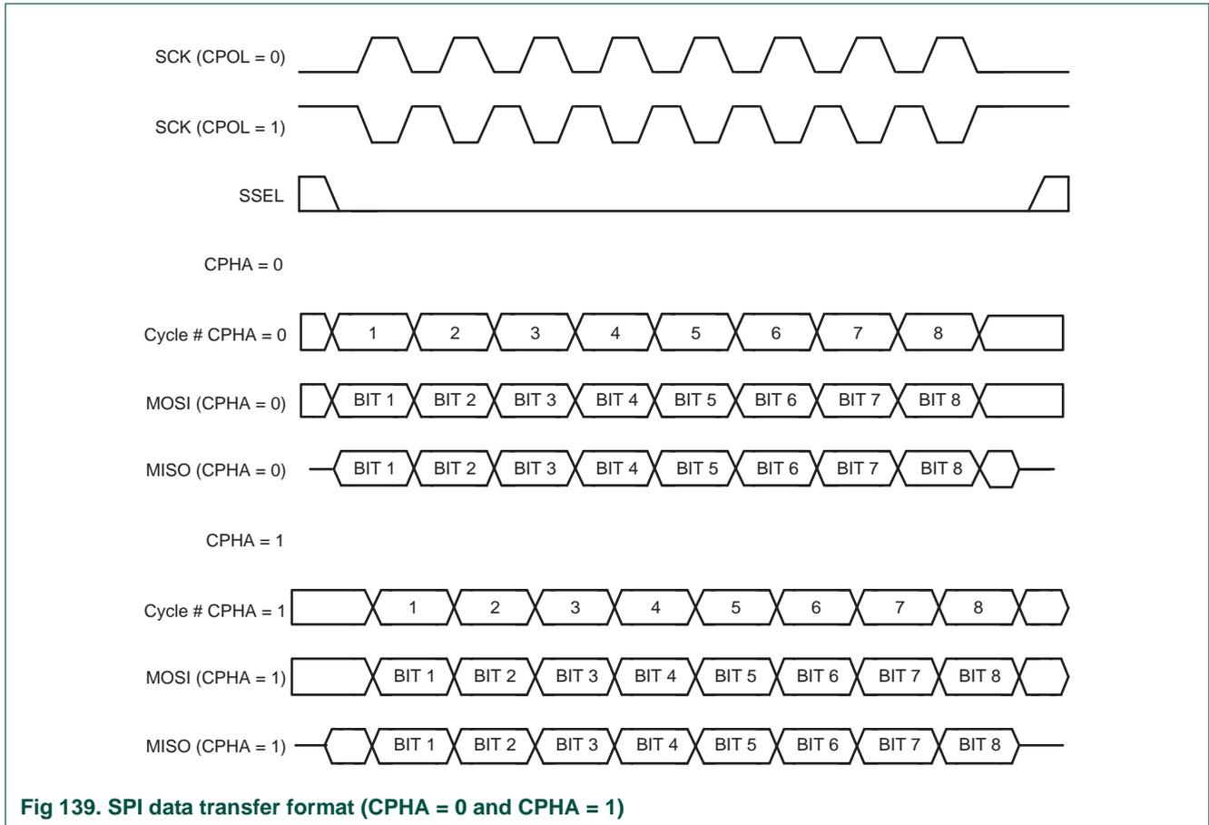
Fig 139. SPI data transfer format (CPHA = 0 and CPHA = 1)
