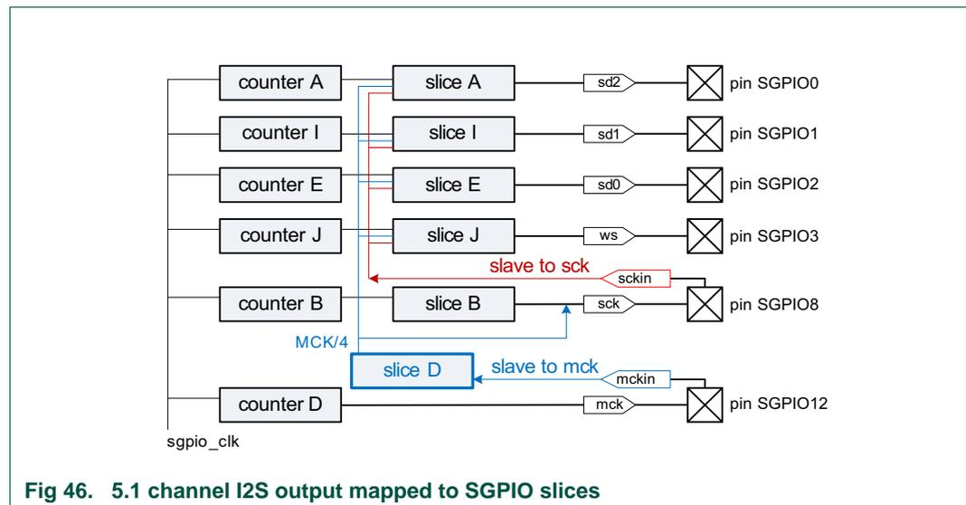
**Fig 46. 5.1 channel I2S output mapped to SGPIO slices**
