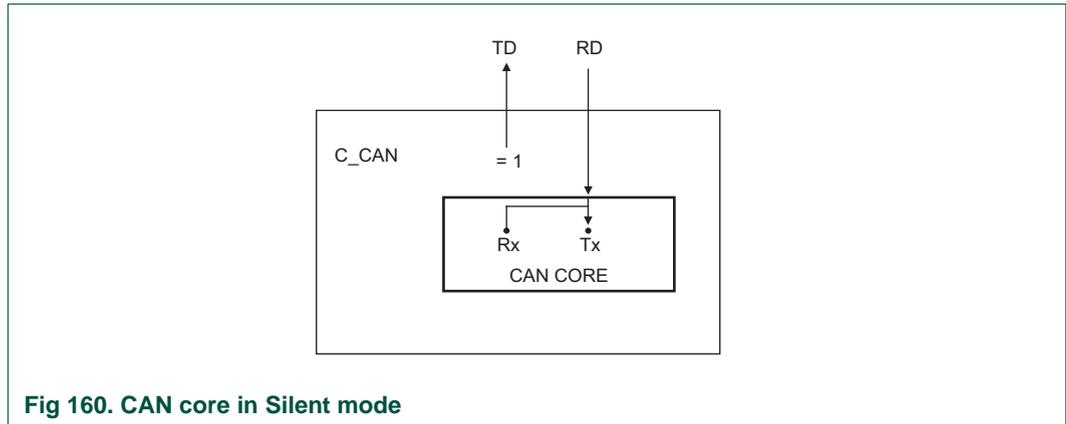
Fig 160. CAN core in Silent mode
