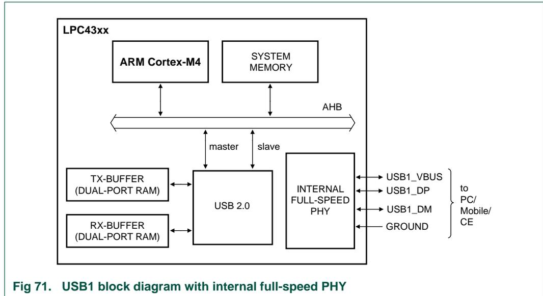
Fig 71. USB1 block diagram with internal full-speed PHY
