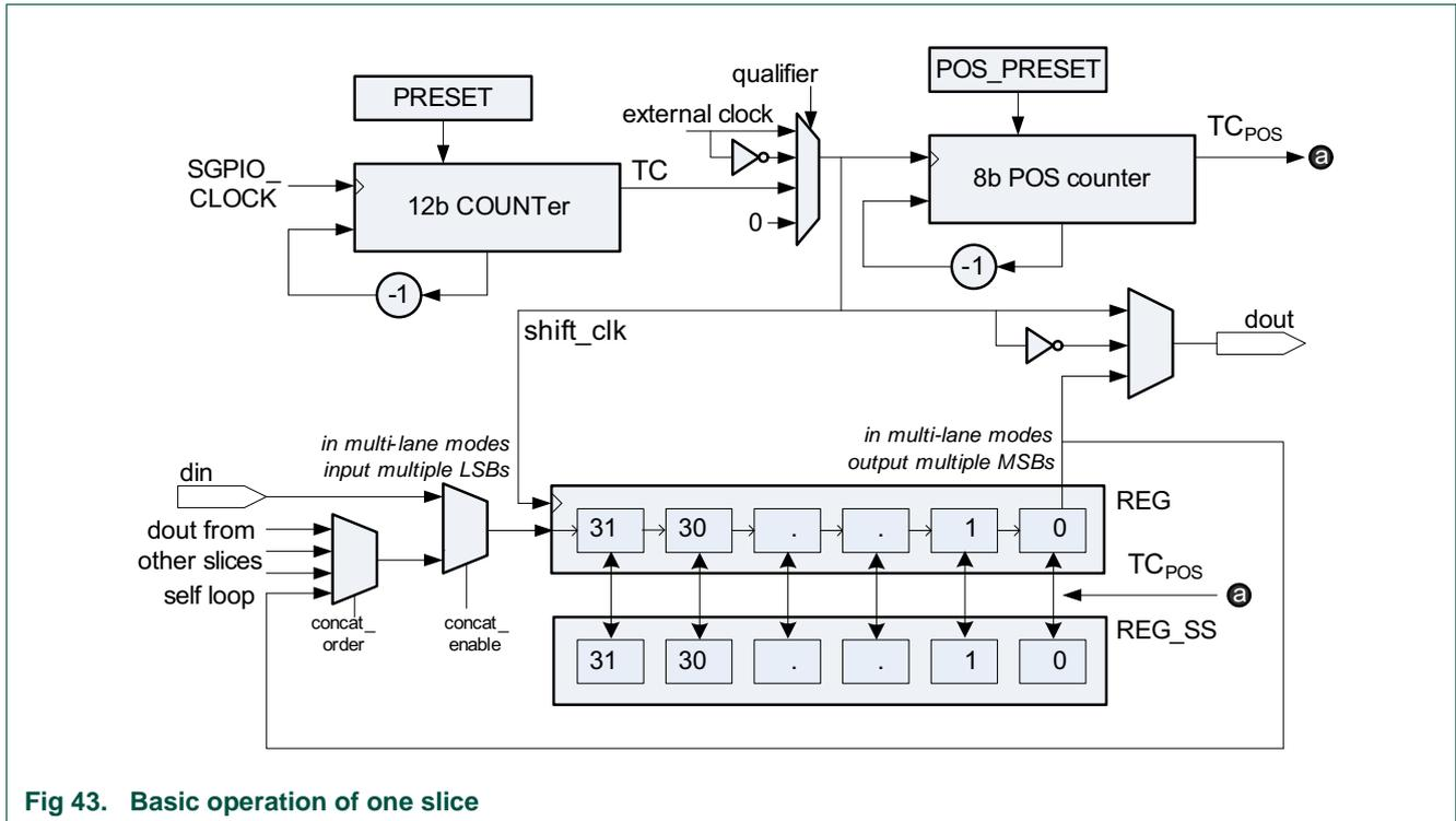
Fig 43. Basic operation of one slice
