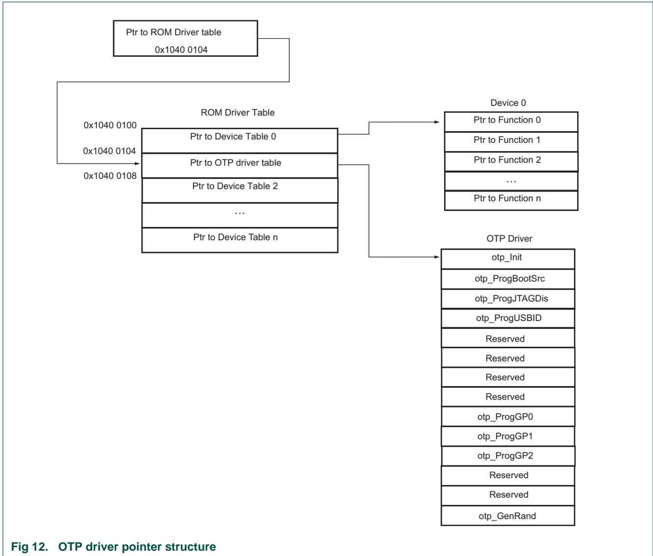
Fig 12. OTP driver pointer structure
