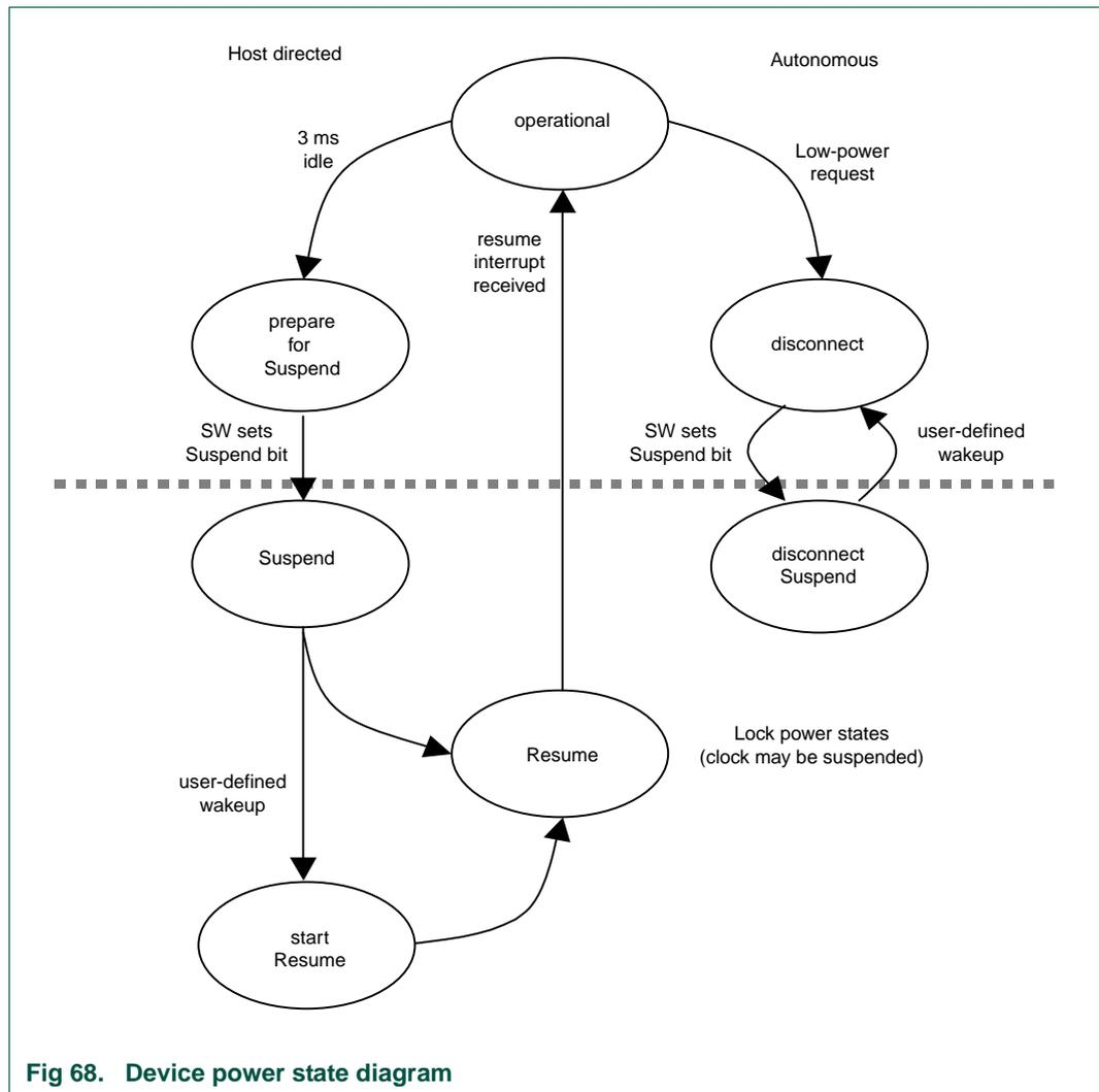
Fig 68. Device power state diagram
