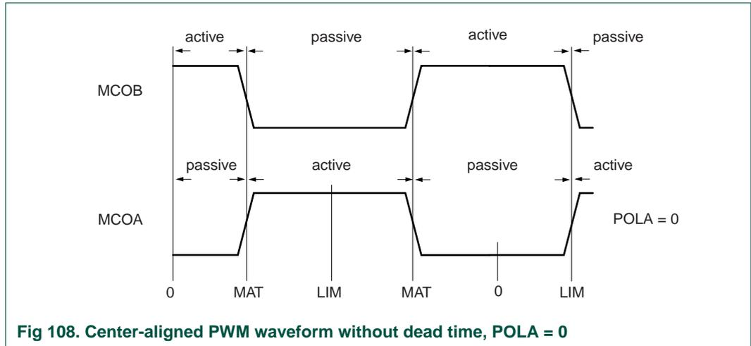
Fig 108. Center-aligned PWM waveform without dead time, POLA = 0
