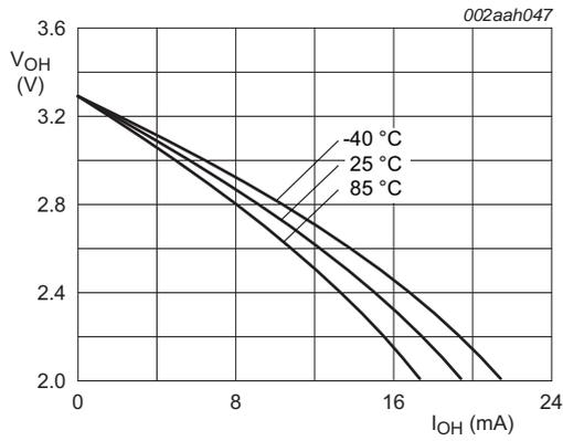
Conditions:  $V_{DD(REG)(3V3)} = V_{DD(IO)} = 3.3$  V; normal-drive; EHD = 0x0.
