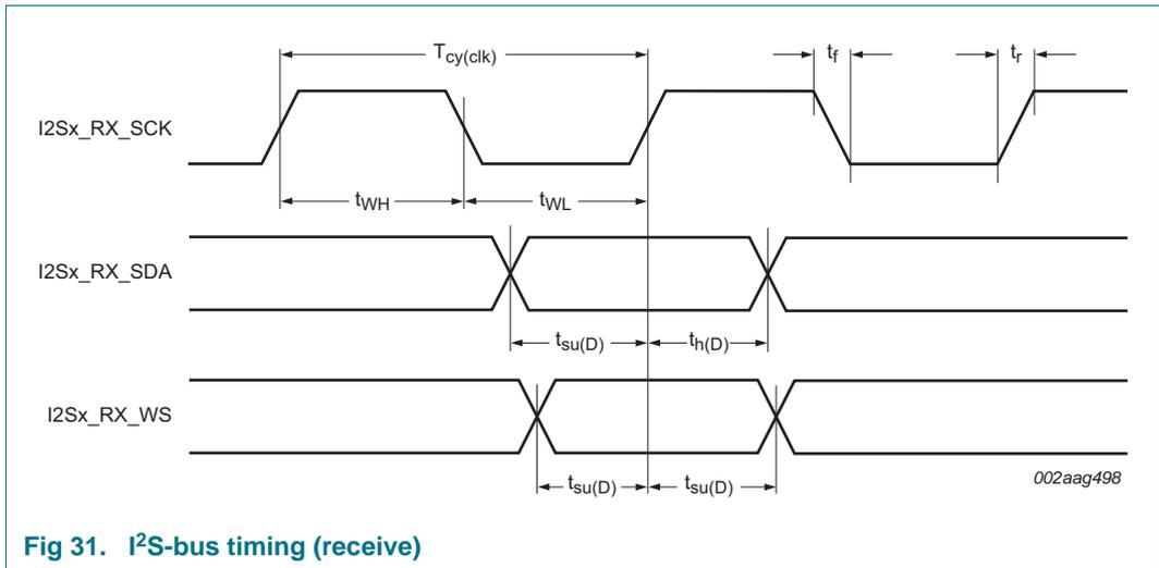
Fig 31. I<sup>2</sup>S-bus timing (receive)
