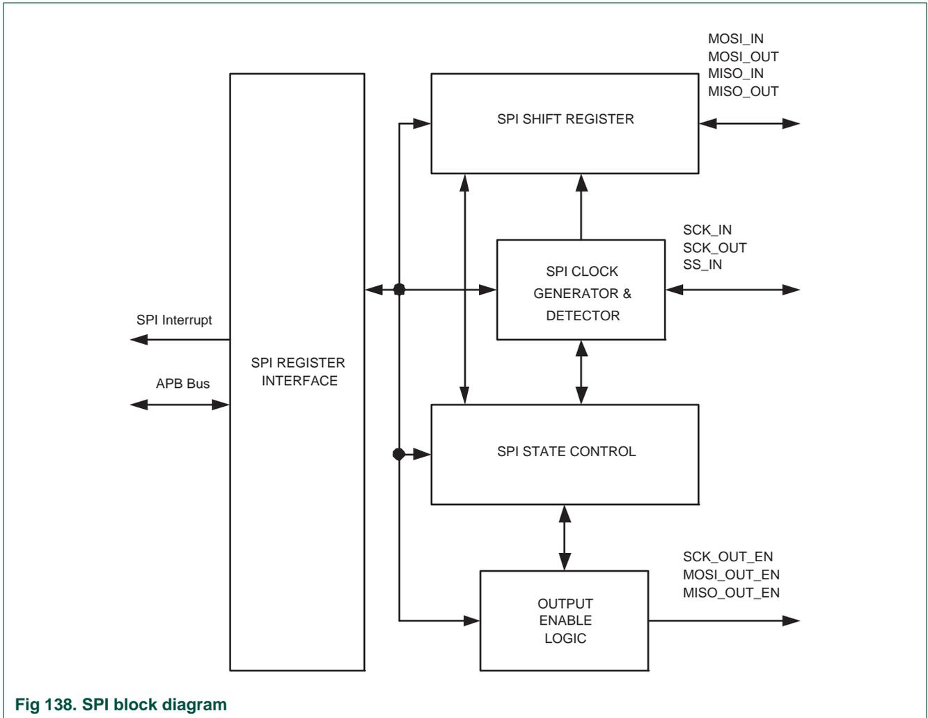
Fig 138. SPI block diagram
