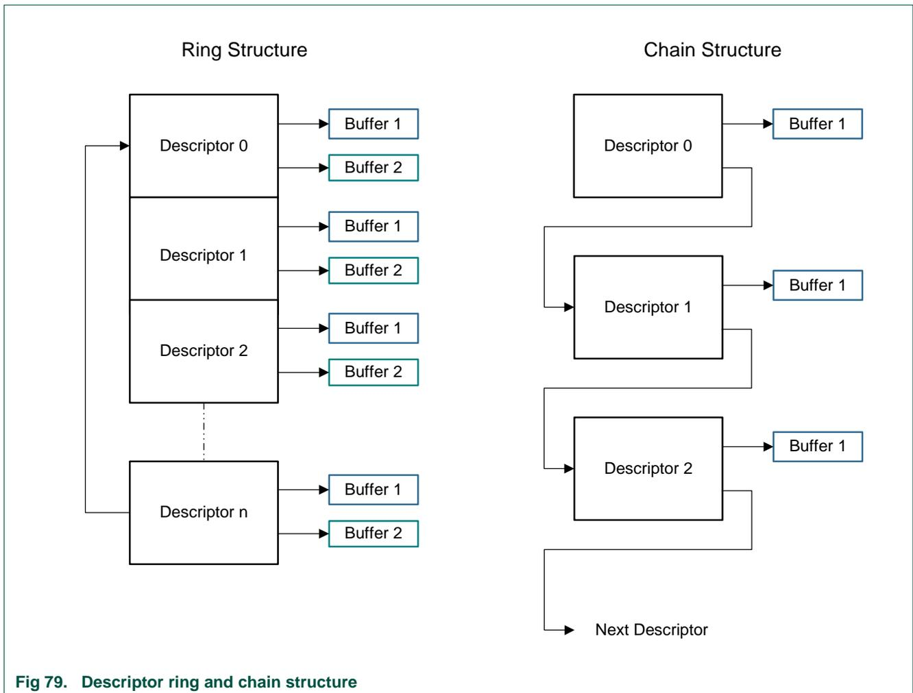
Fig 79. Descriptor ring and chain structure
