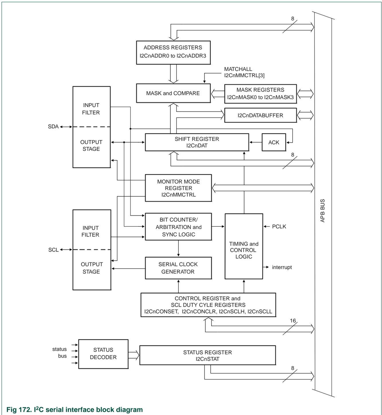
Fig 172. I<sup>2</sup>C serial interface block diagram
