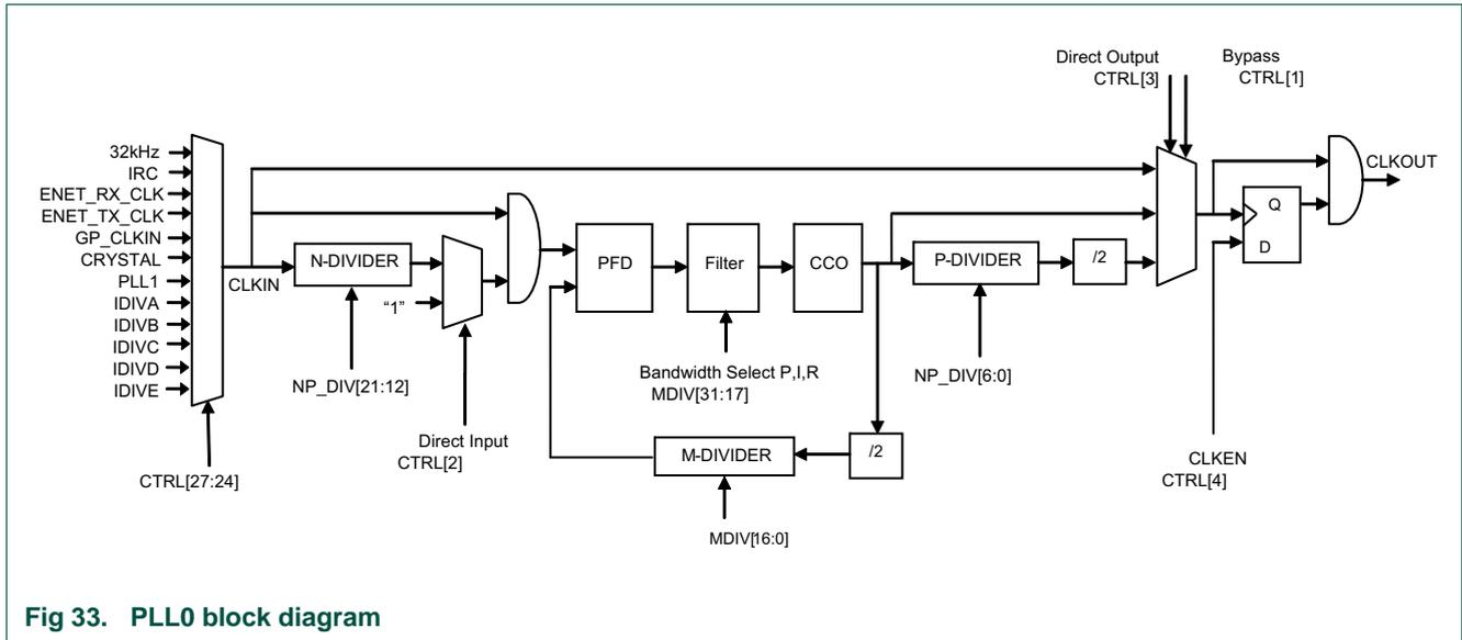
Fig 33. PLL0 block diagram
