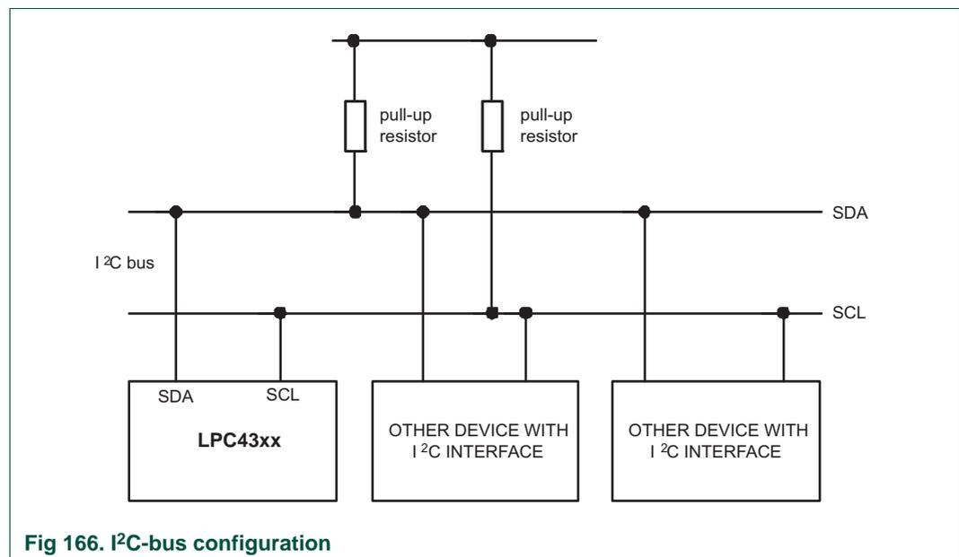
Fig 166. I<sup>2</sup>C-bus configuration
