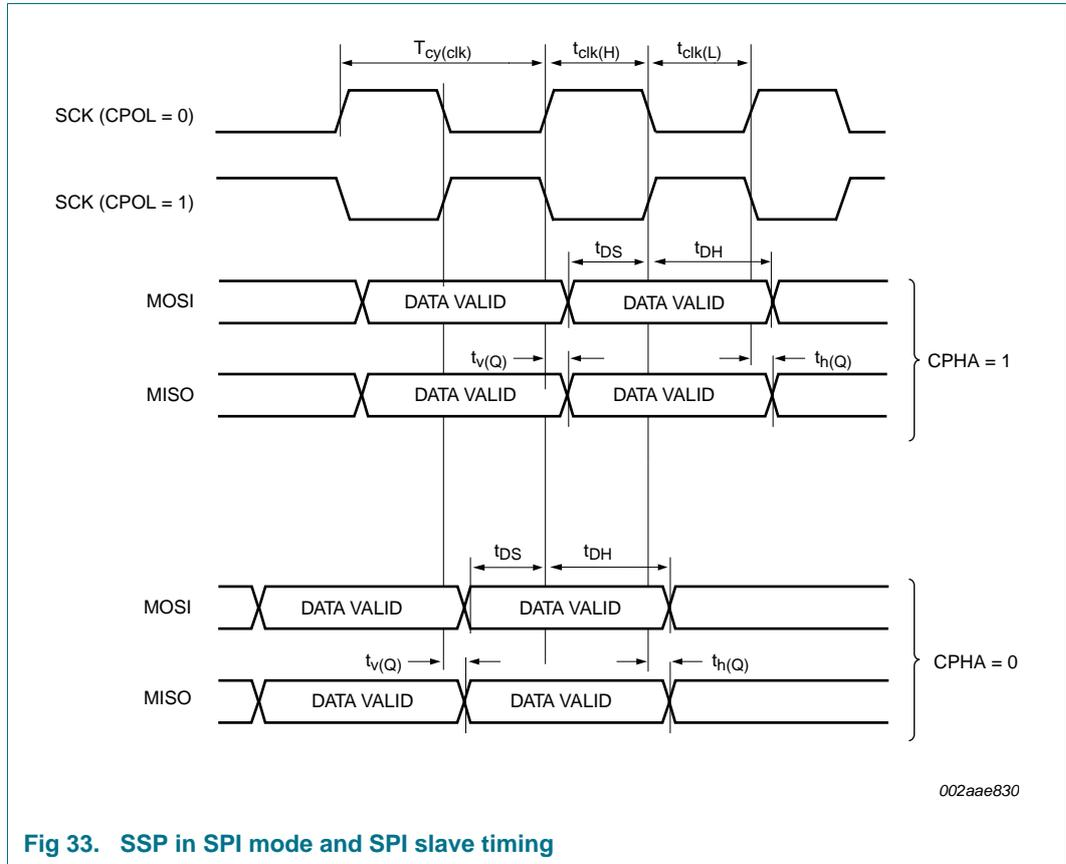
Fig 33. SSP in SPI mode and SPI slave timing
