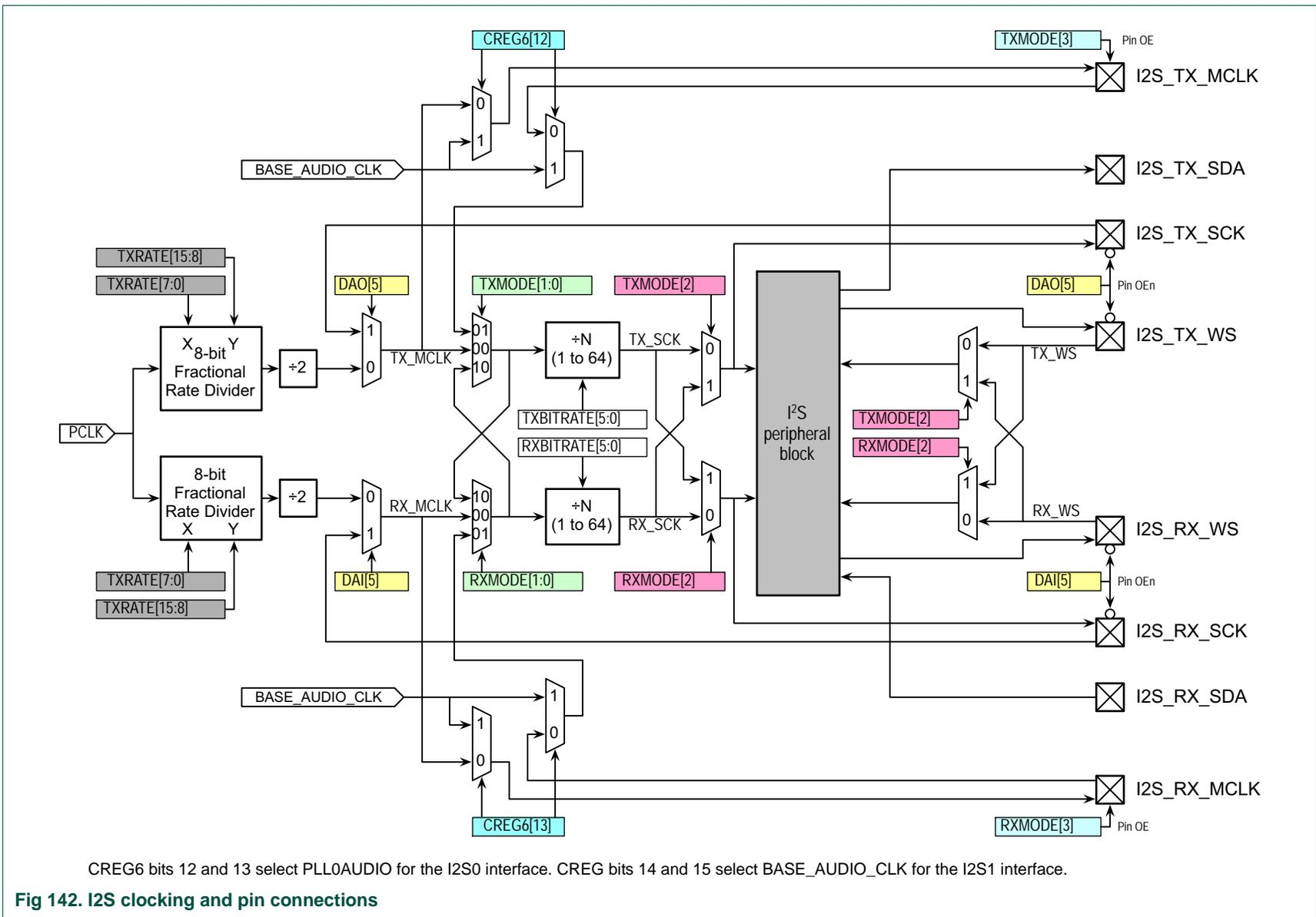
CREG6 bits 12 and 13 select PLL0AUDIO for the I2S0 interface. CREG bits 14 and 15 select BASE\_AUDIO\_CLK for the I2S1 interface.
