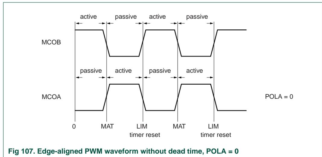
Fig 107. Edge-aligned PWM waveform without dead time, POLA = 0
