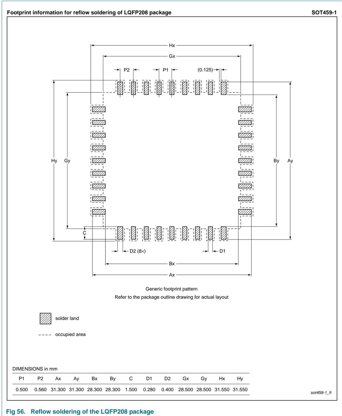
**Fig 56. Reflow soldering of the LQFP208 package**
