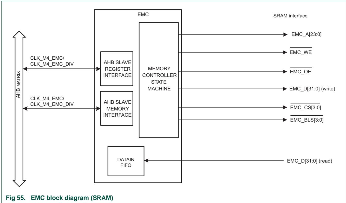
Fig 55. EMC block diagram (SRAM)
