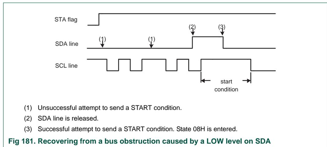
**Fig 181. Recovering from a bus obstruction caused by a LOW level on SDA**
