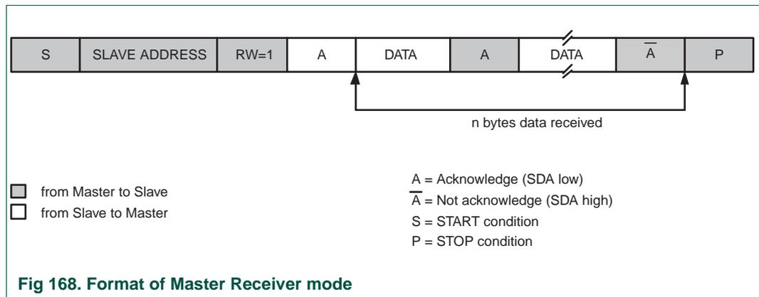
After a Repeated START condition, I<sup>2</sup>C may switch to the master transmitter mode.
