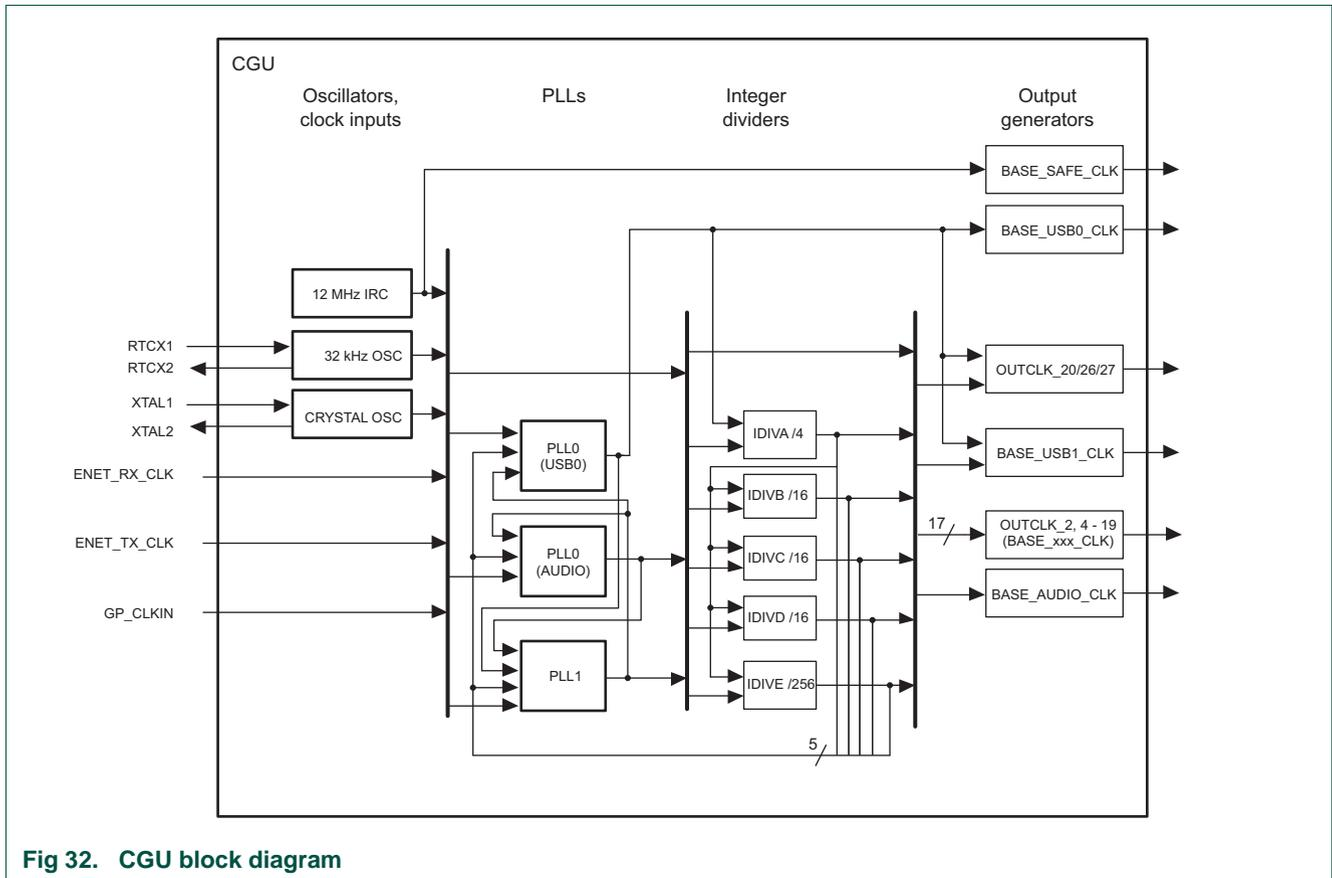
Fig 32. CGU block diagram
