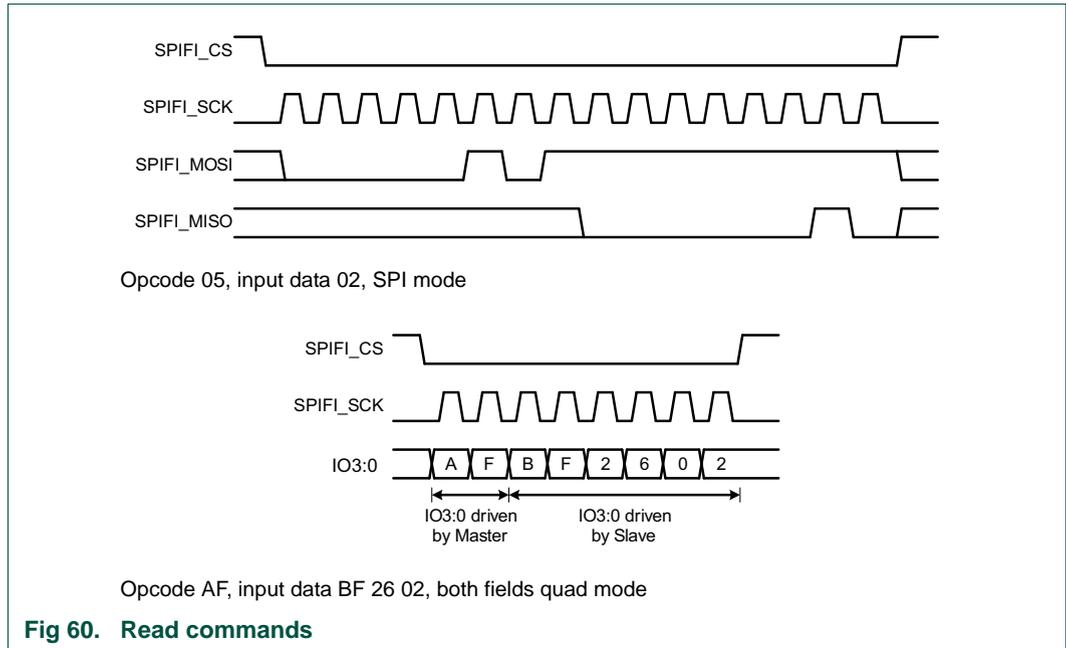
In quad mode, the IO3:0 lines are driven by the SPIFI in opcode, address, intermediate and output data fields, and driven by the flash memory in input data fields. In address fields the more significant bytes are sent first.
