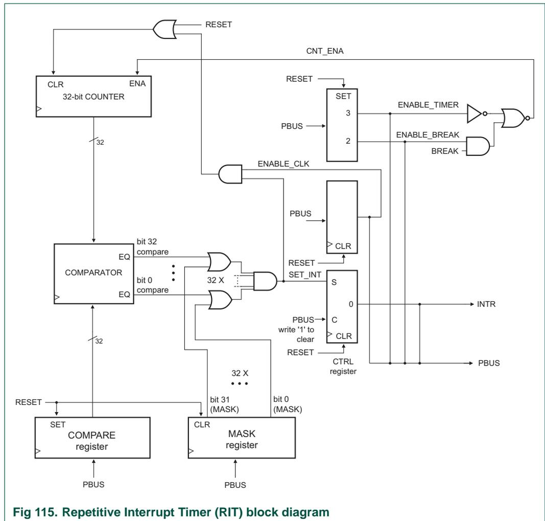
Fig 115. Repetitive Interrupt Timer (RIT) block diagram
