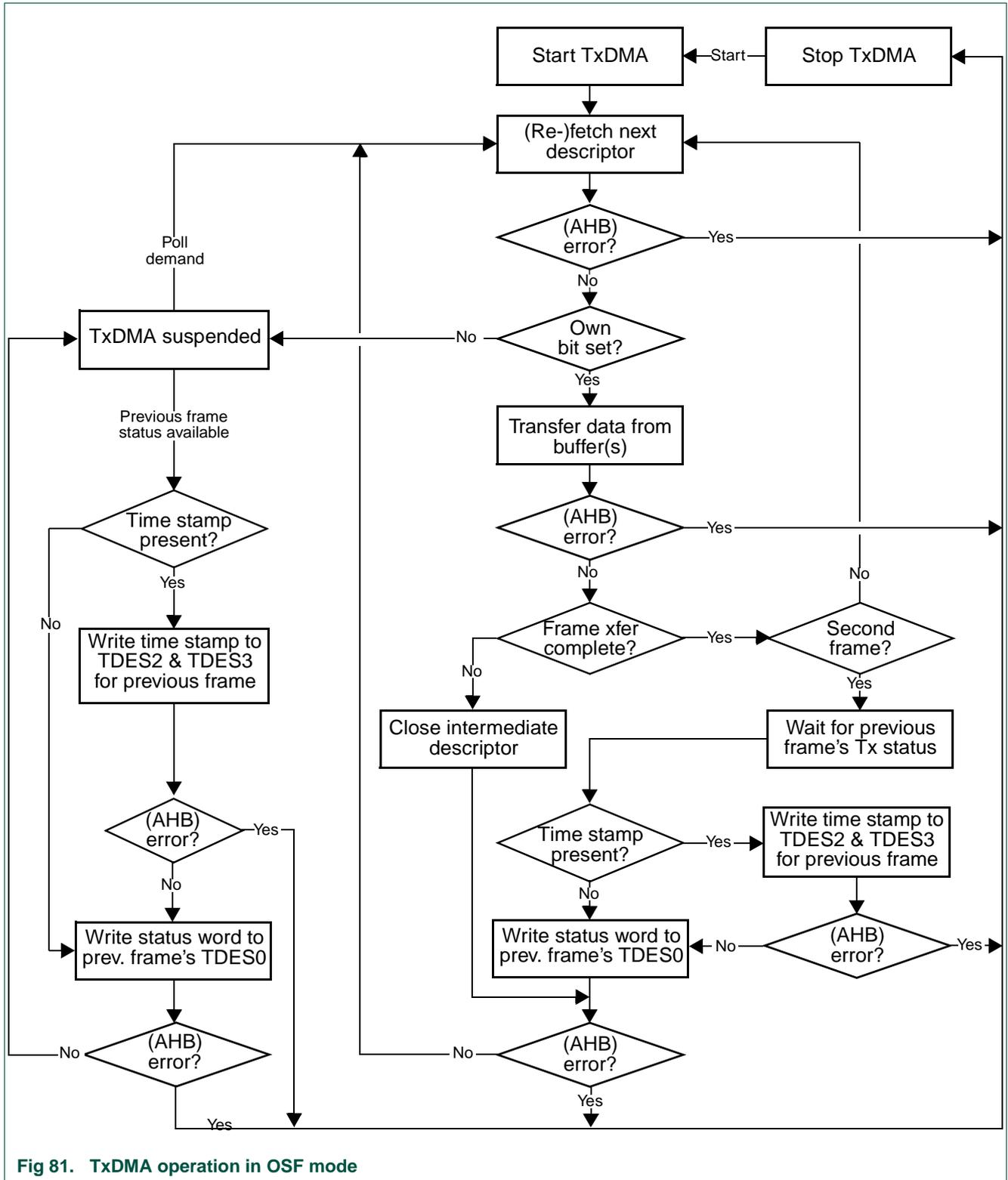
Fig 81. TxDMA operation in OSF mode
