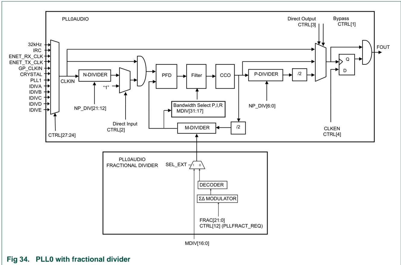
Fig 34. PLL0 with fractional divider
