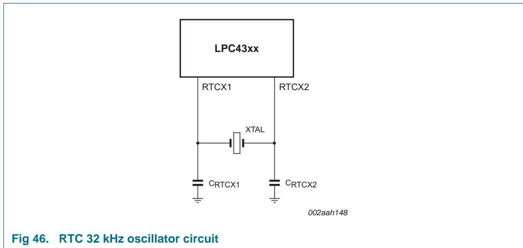
Fig 46. RTC 32 kHz oscillator circuit
