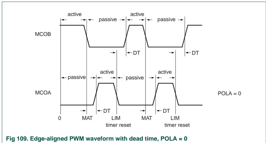
Fig 109. Edge-aligned PWM waveform with dead time, POLA = 0
