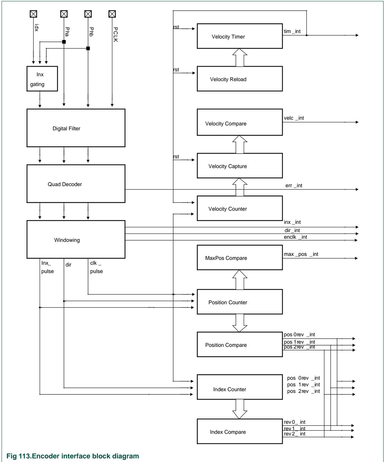
Fig 113. Encoder interface block diagram
