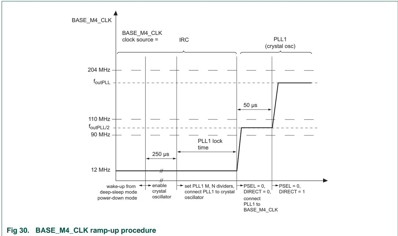
Fig 30. BASE\_M4\_CLK ramp-up procedure
