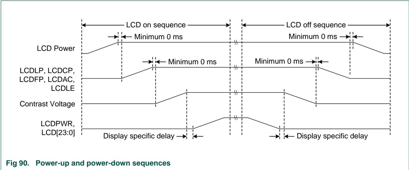
Fig 90. Power-up and power-down sequences
