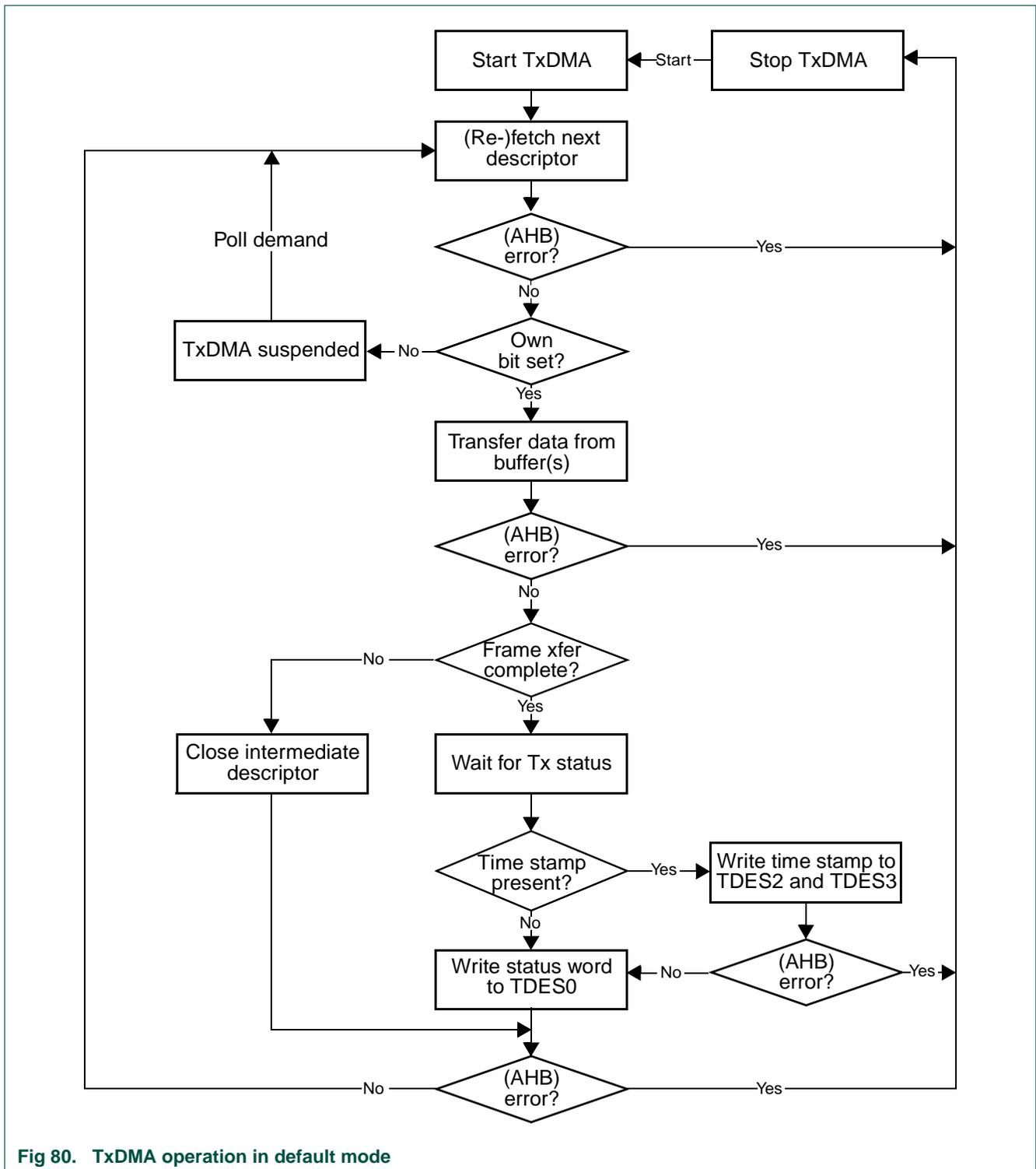
Fig 80. TxDMA operation in default mode
