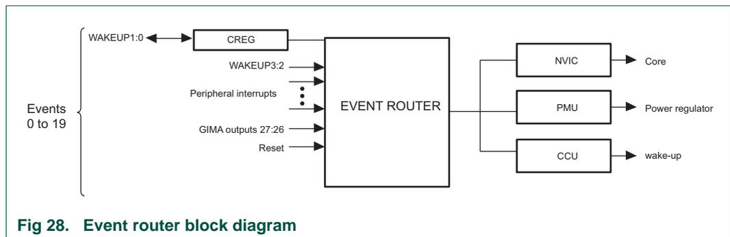
Fig 28. Event router block diagram
