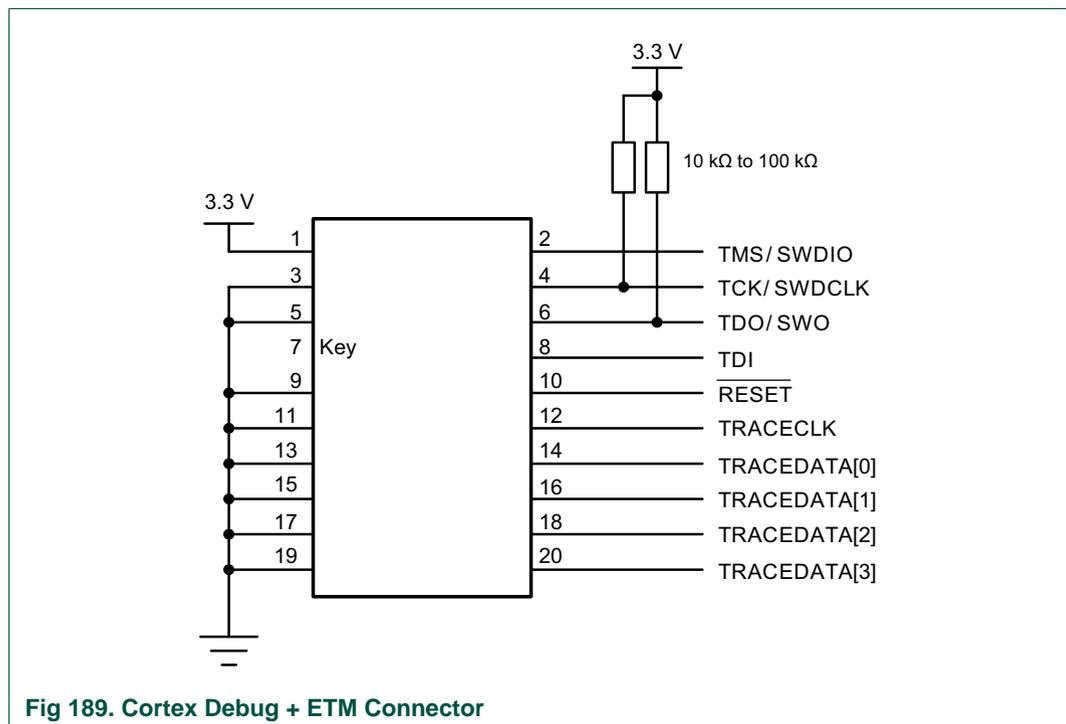
Fig 189. Cortex Debug + ETM Connector
