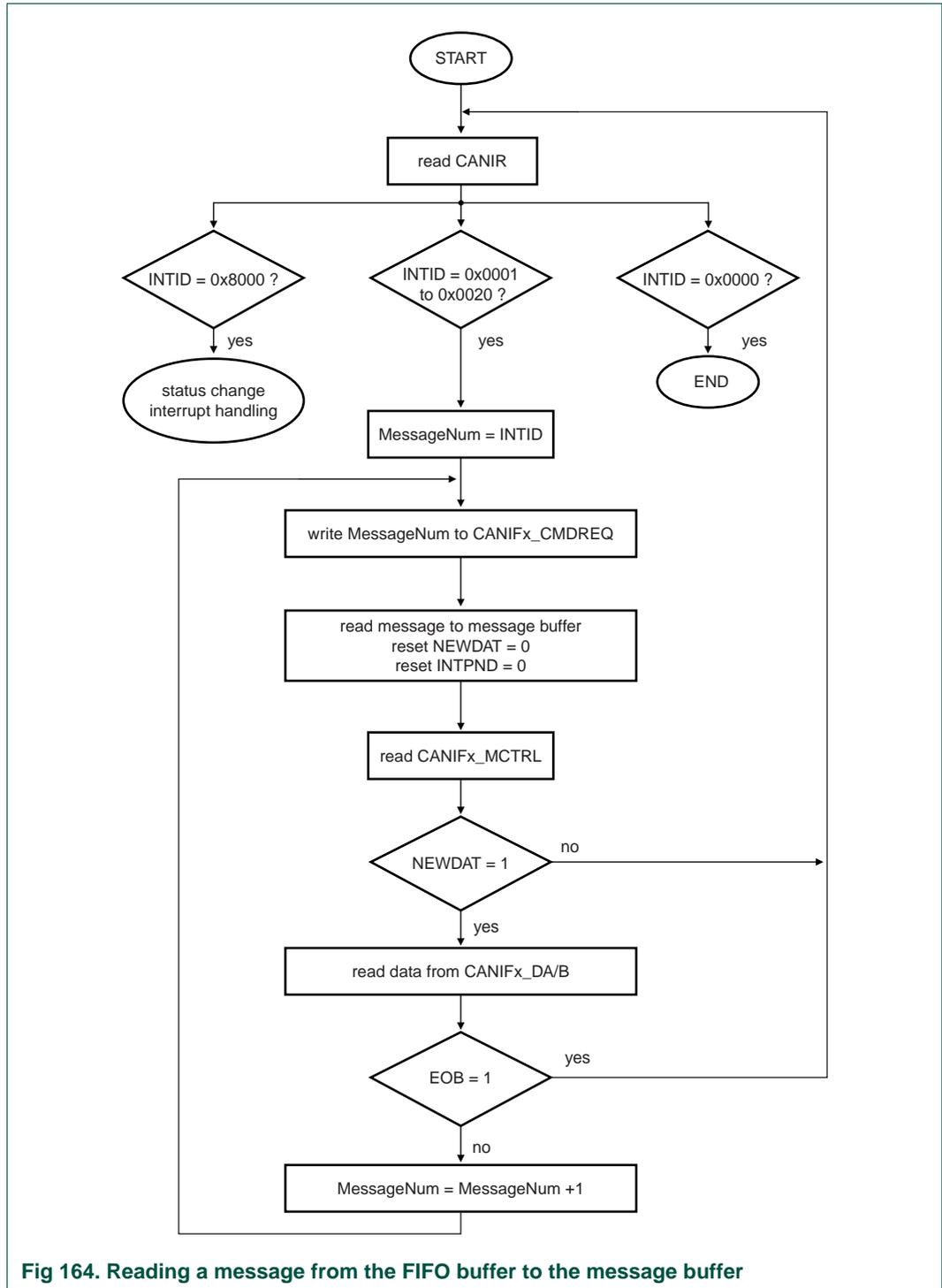
Fig 164. Reading a message from the FIFO buffer to the message buffer
