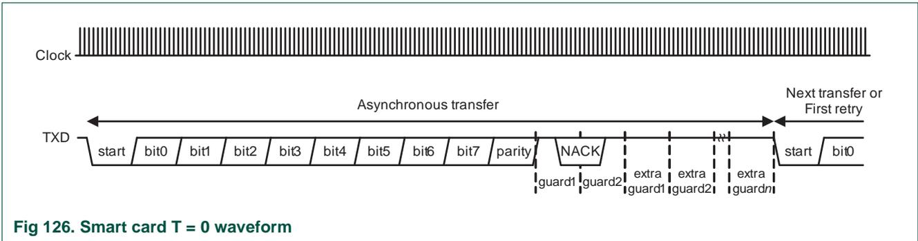
Fig 126. Smart card T = 0 waveform
