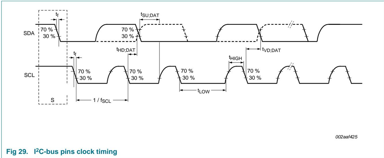
Fig 29. I<sup>2</sup>C-bus pins clock timing
