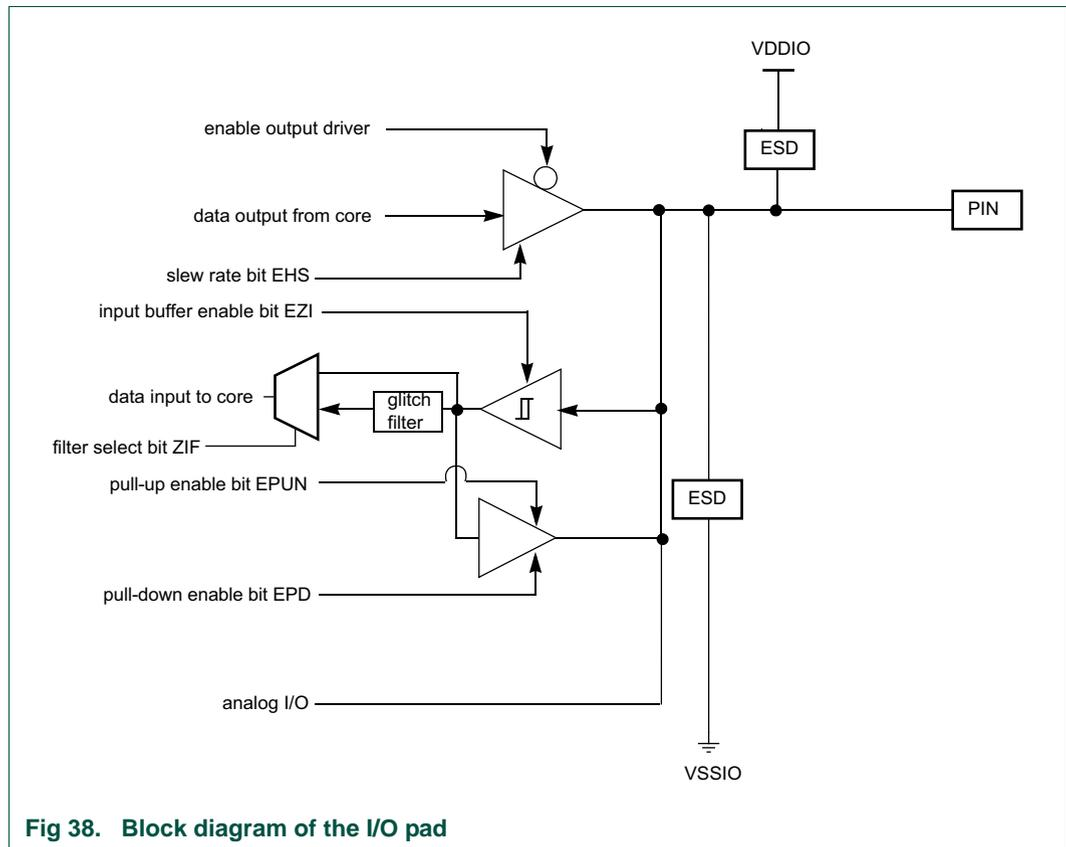
Fig 38. Block diagram of the I/O pad
