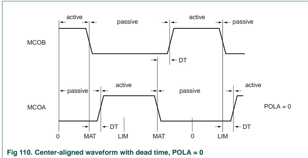
Fig 110. Center-aligned waveform with dead time, POLA = 0
