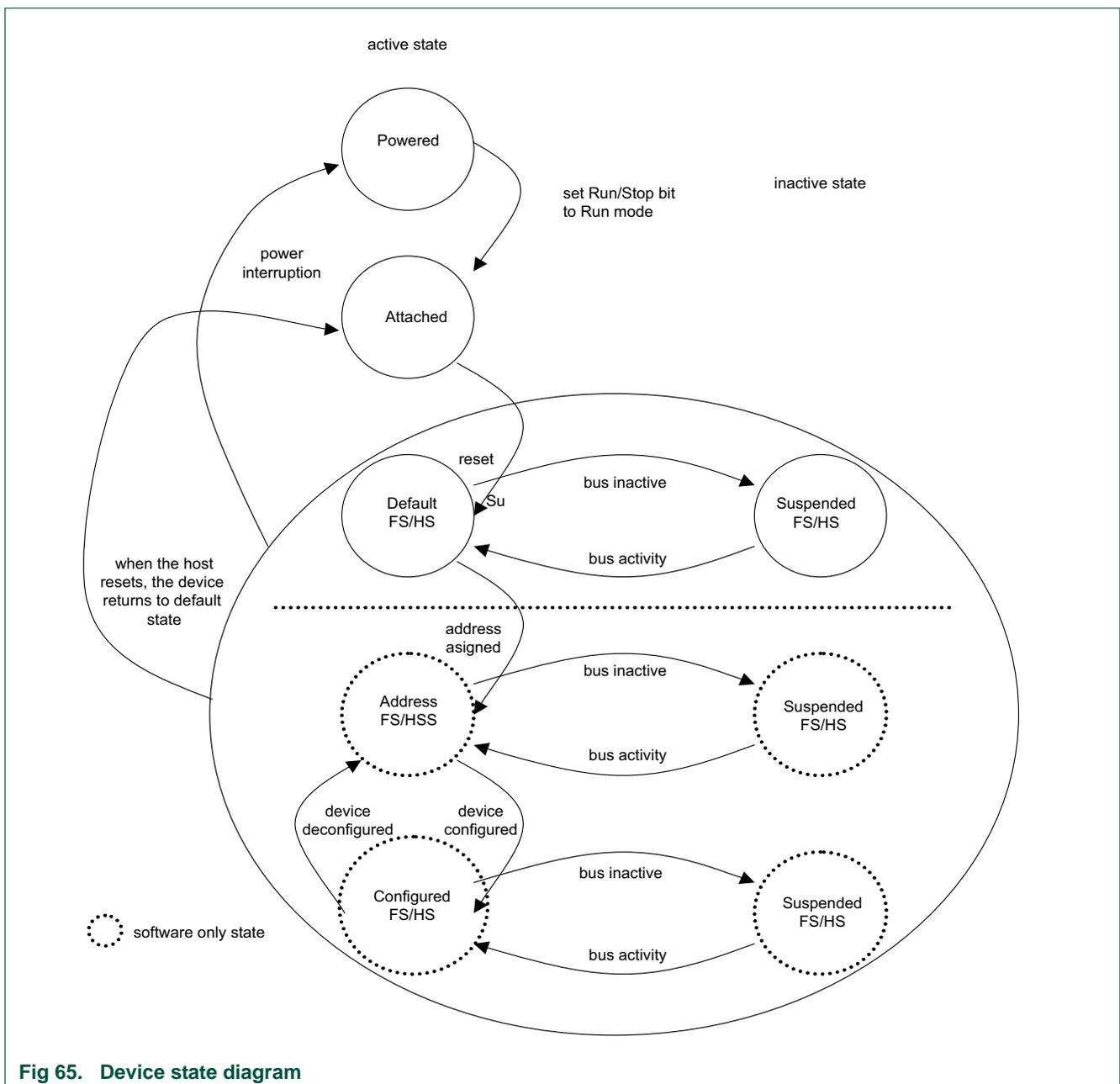
Fig 65. Device state diagram
