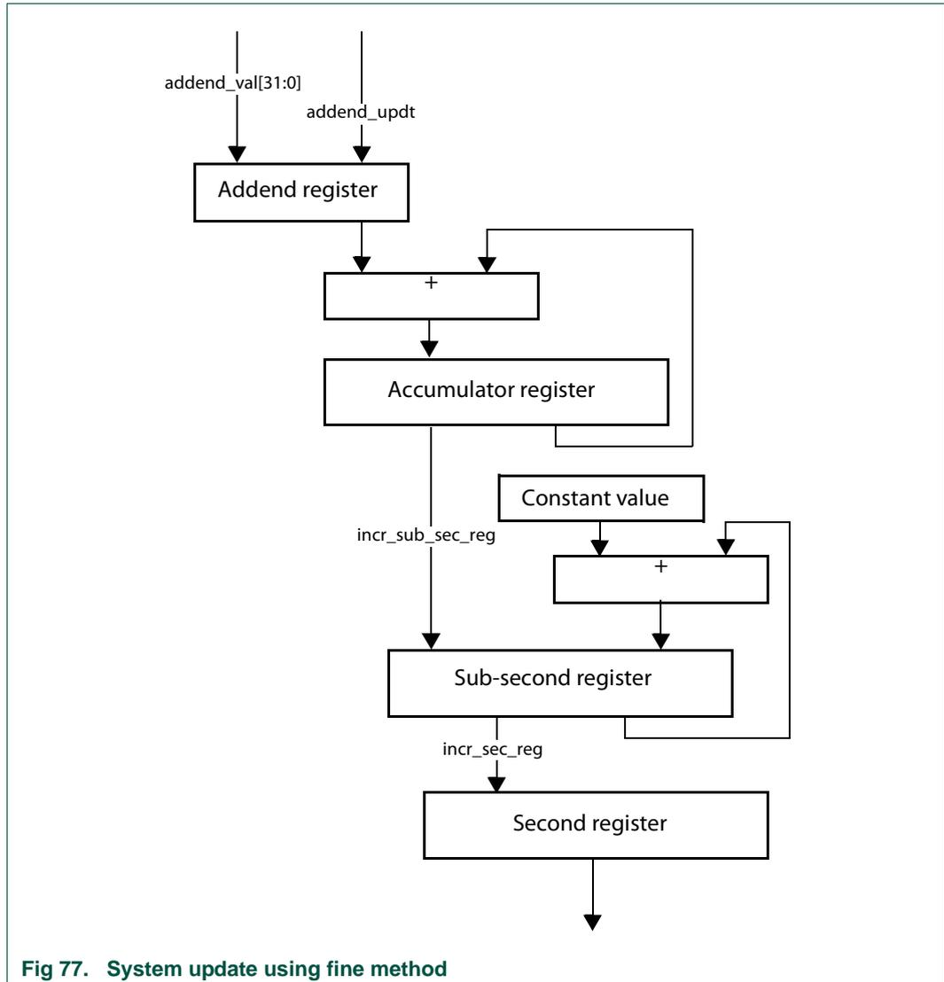
**Fig 77. System update using fine method**
