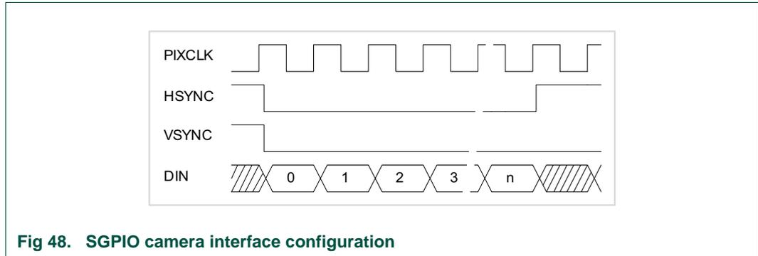
Fig 48. SGPIO camera interface configuration
