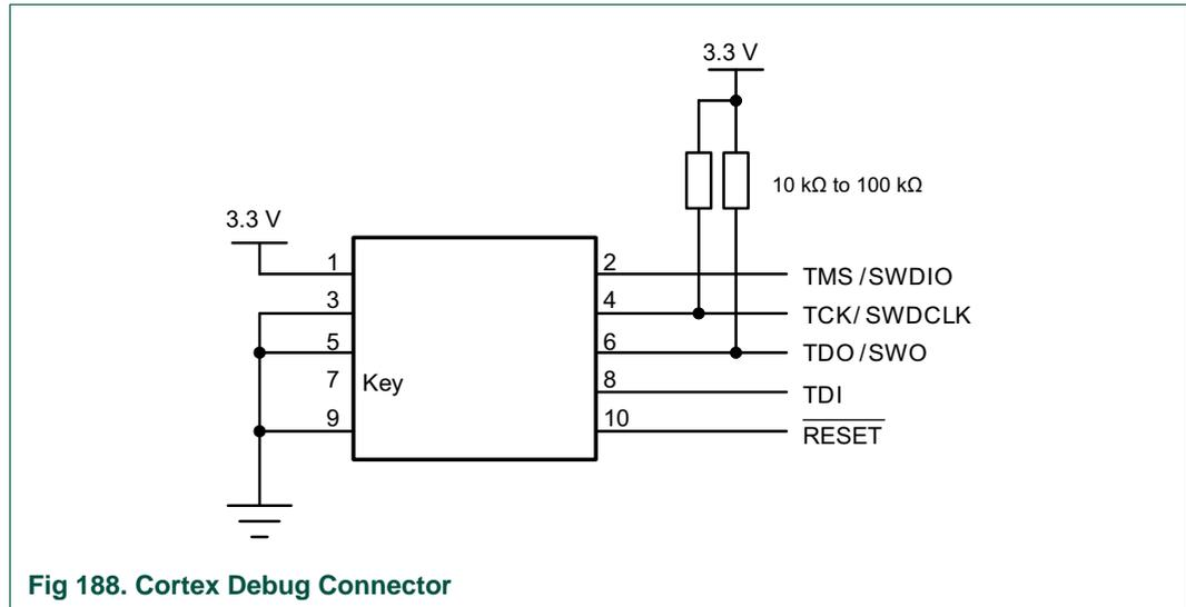
Fig 188. Cortex Debug Connector
