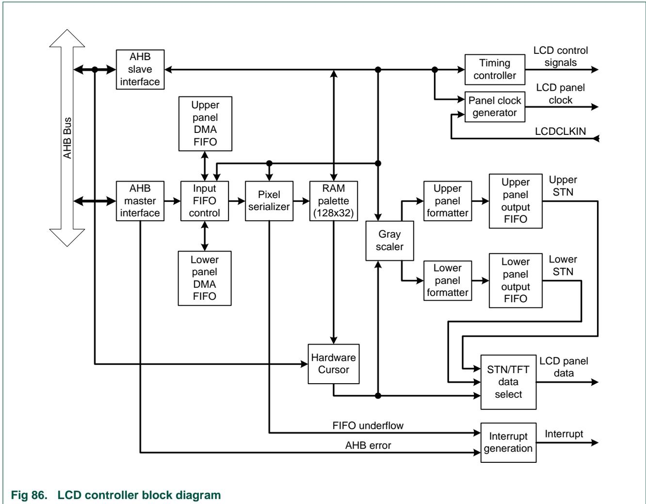
Fig 86. LCD controller block diagram
