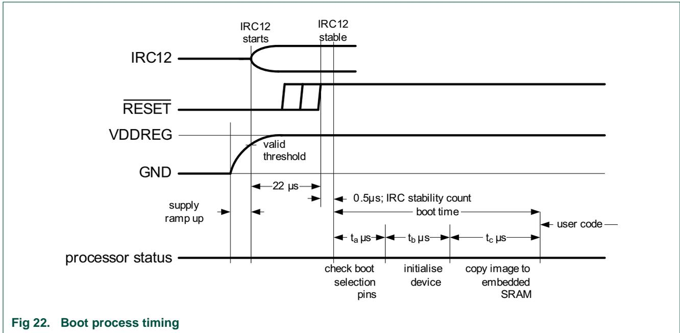
Fig 22. Boot process timing
