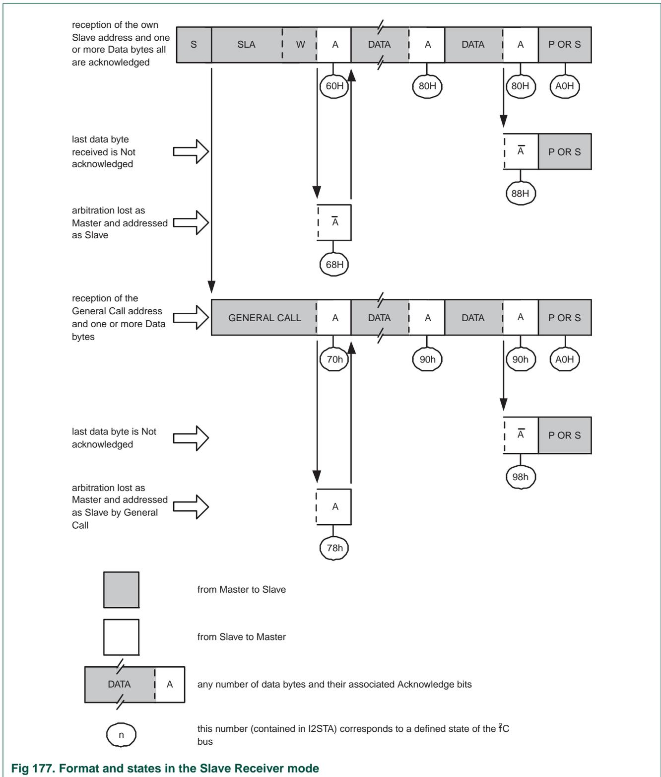
Fig 177. Format and states in the Slave Receiver mode
