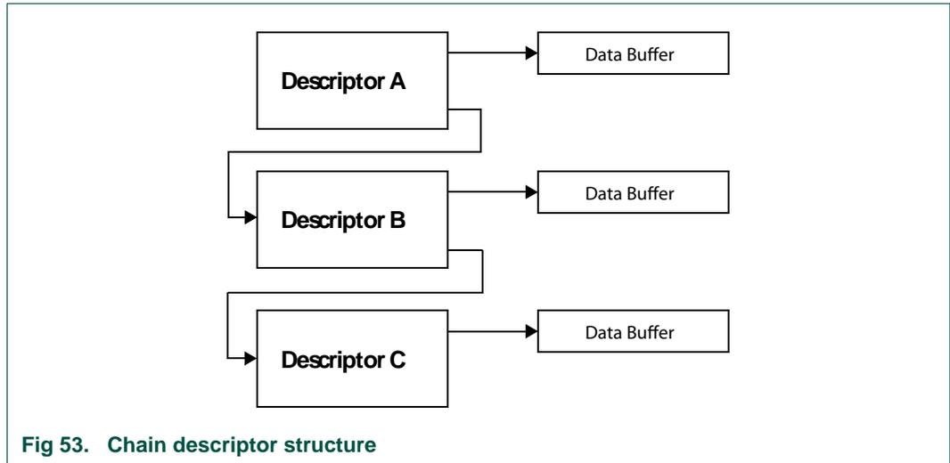
Fig 53. Chain descriptor structure
