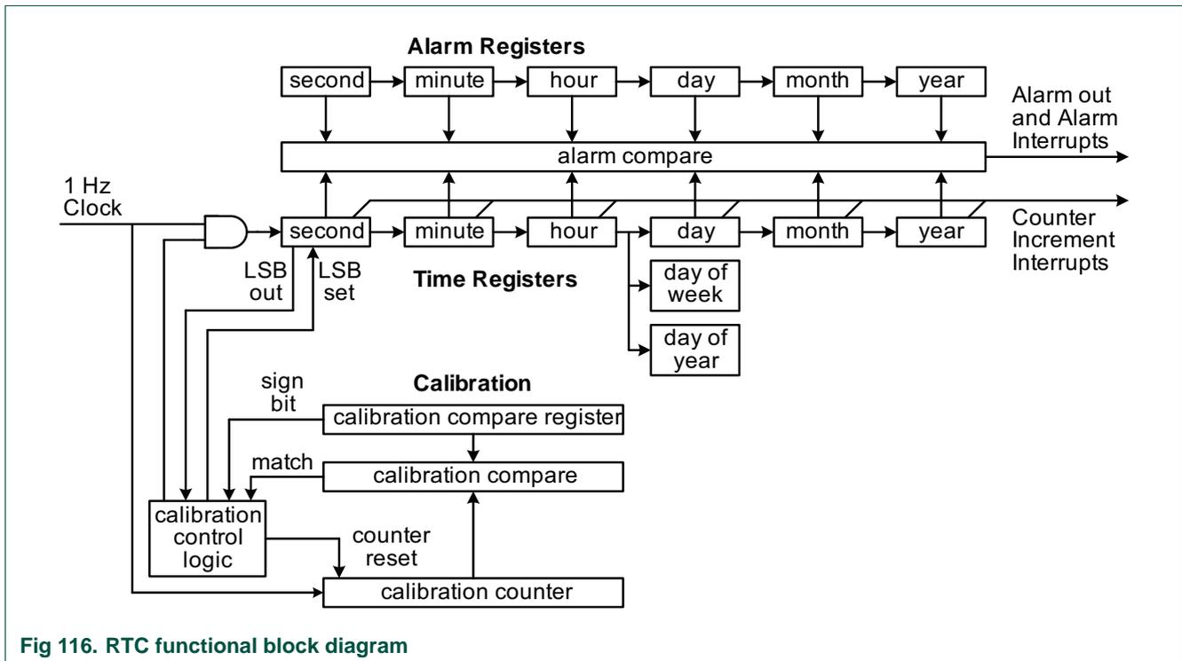
Fig 116. RTC functional block diagram
