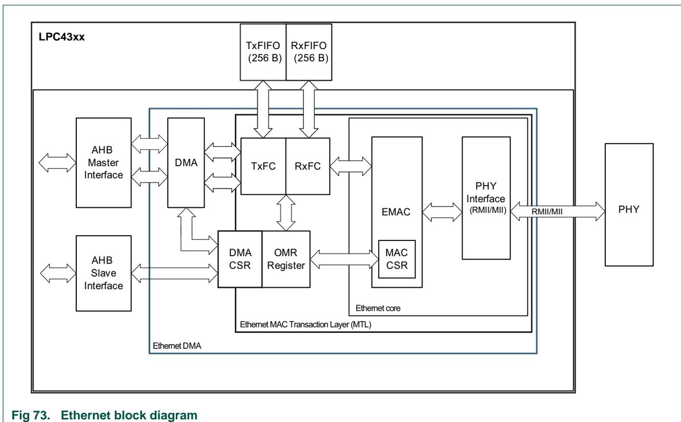
Fig 73. Ethernet block diagram
