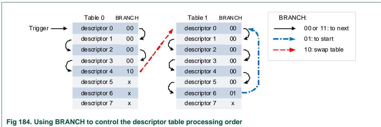
Fig 184. Using BRANCH to control the descriptor table processing order
