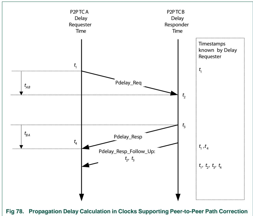
**Fig 78. Propagation Delay Calculation in Clocks Supporting Peer-to-Peer Path Correction**
