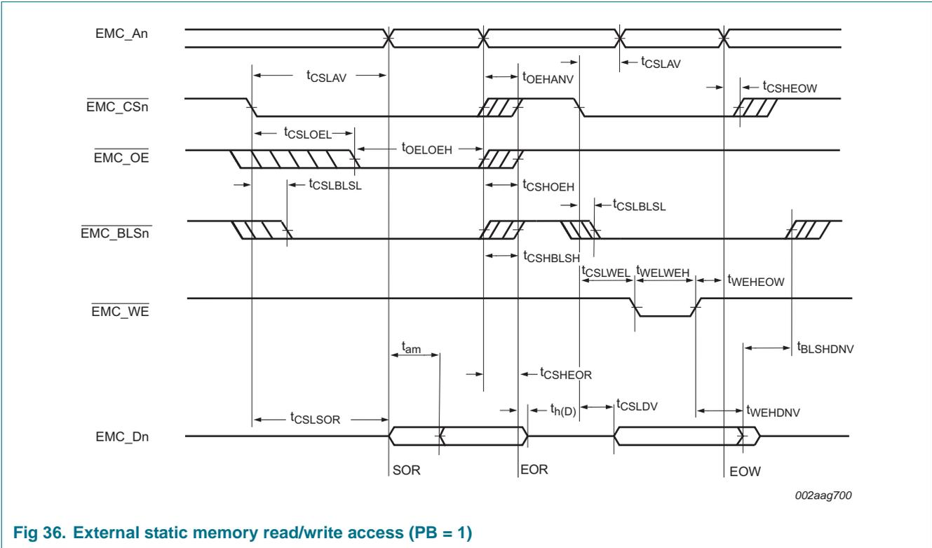
Fig 36. External static memory read/write access (PB = 1)
