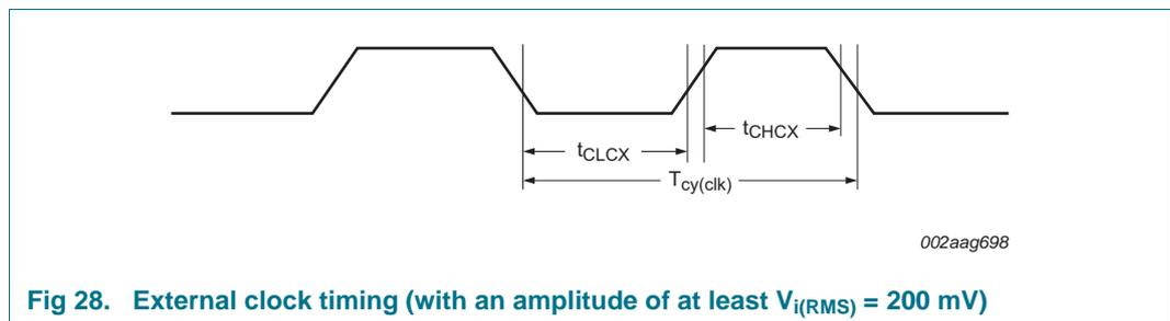
**Fig 28. External clock timing (with an amplitude of at least  $V_{i(RMS)} = 200\text{ mV}$ )**
