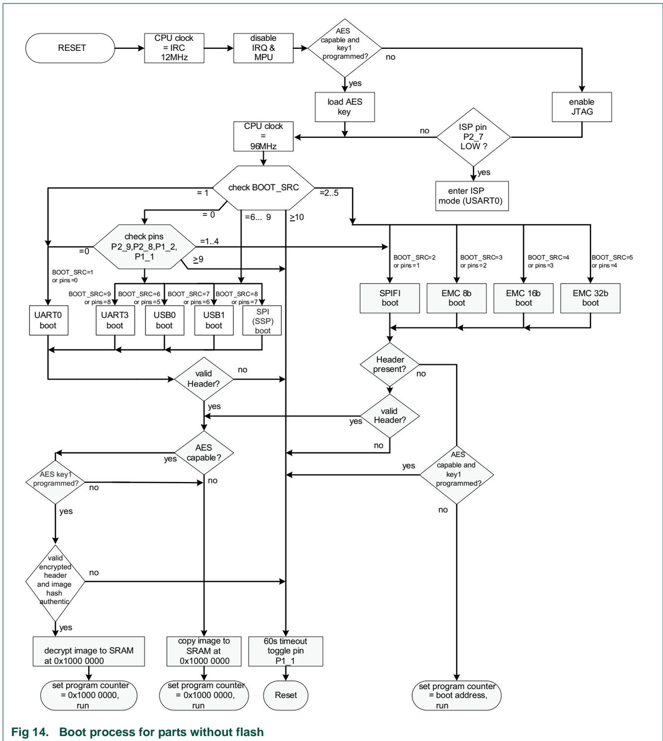
Fig 14. Boot process for parts without flash
