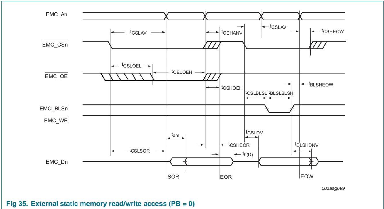
**Fig 35. External static memory read/write access (PB = 0)**
