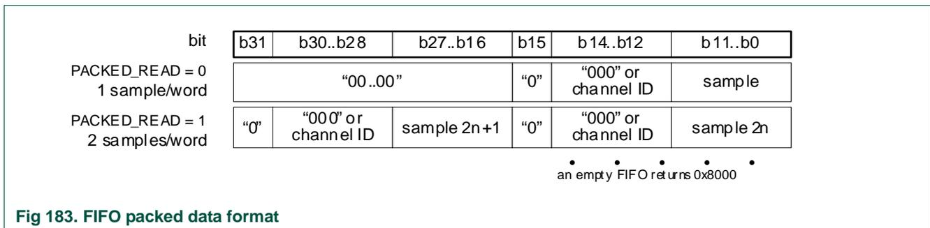
Fig 183. FIFO packed data format
