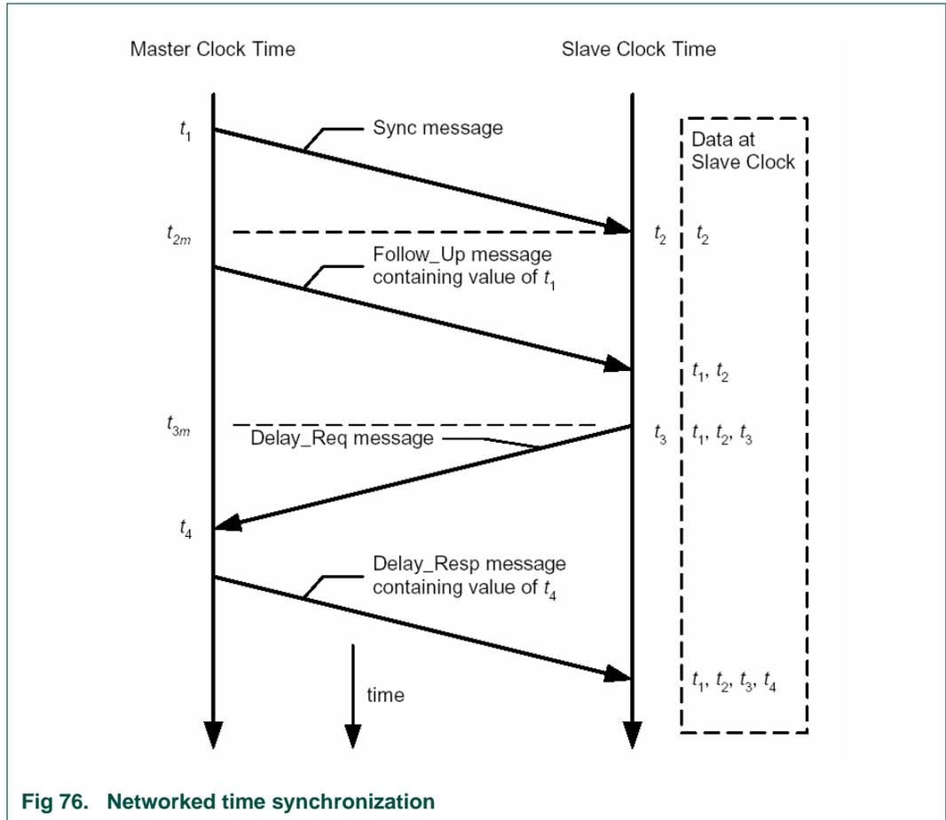
**Fig 76. Networked time synchronization**
