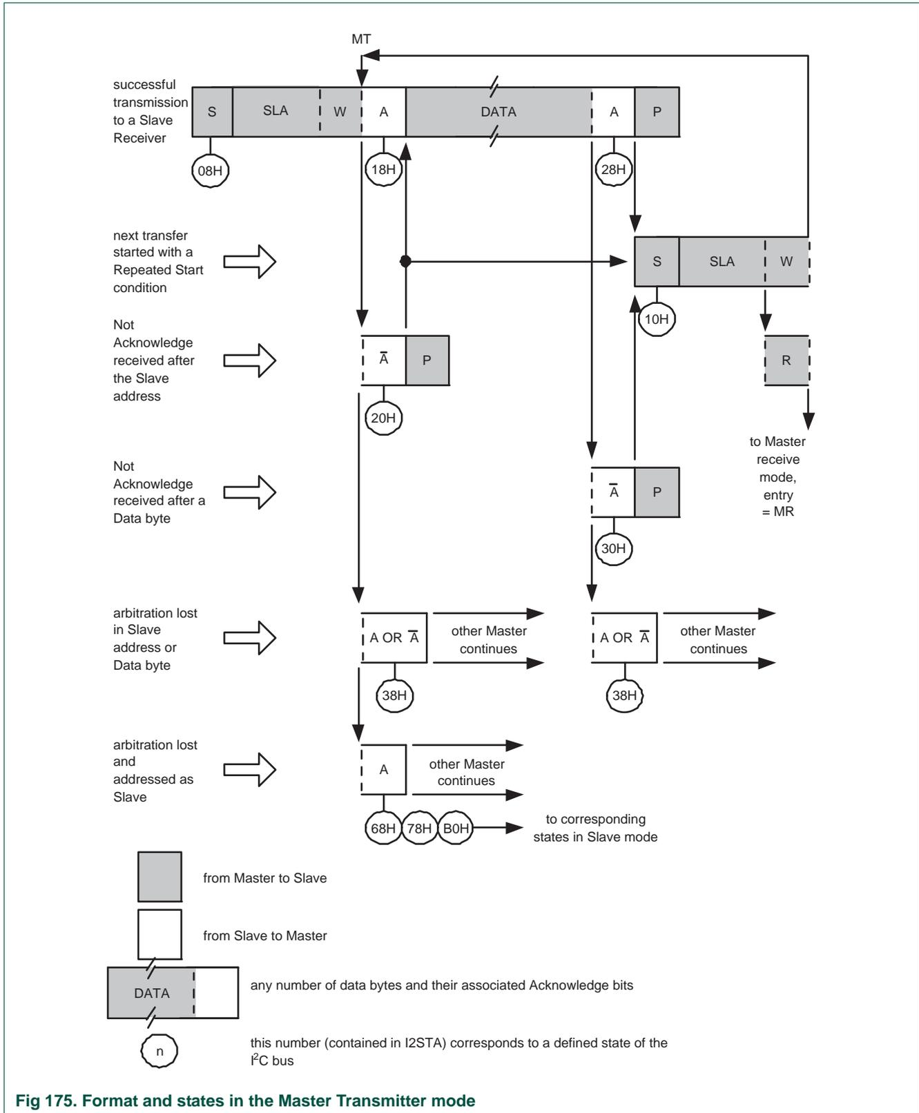
Fig 175. Format and states in the Master Transmitter mode
