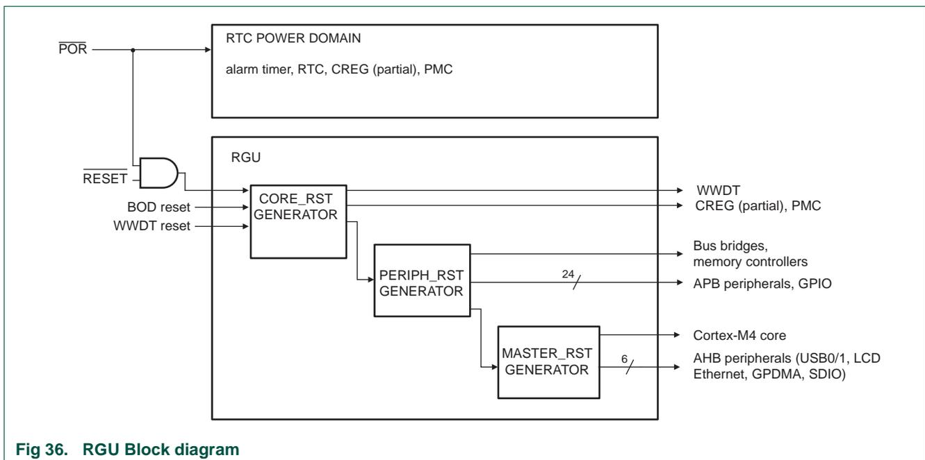
**Fig 36. RGU Block diagram**
