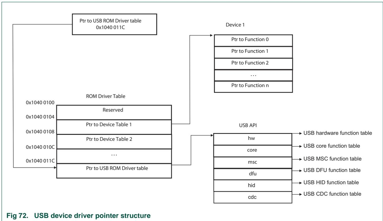
Fig 72. USB device driver pointer structure
