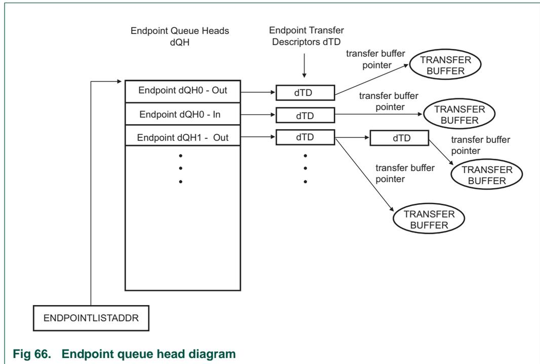
Fig 66. Endpoint queue head diagram
