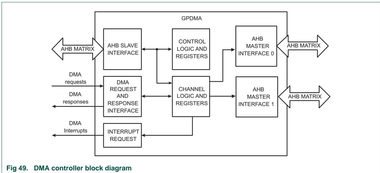
Fig 49. DMA controller block diagram
