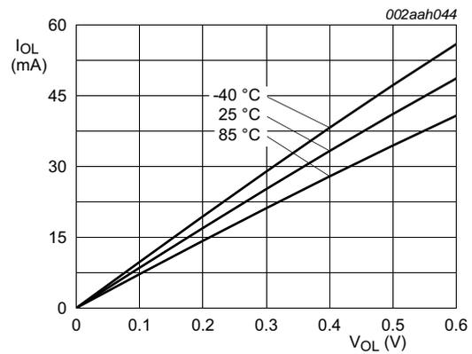
Conditions:  $V_{DD(REG)(3V3)} = V_{DD(IO)} = 3.3$  V; ultra high-drive; EHD = 0x3.
