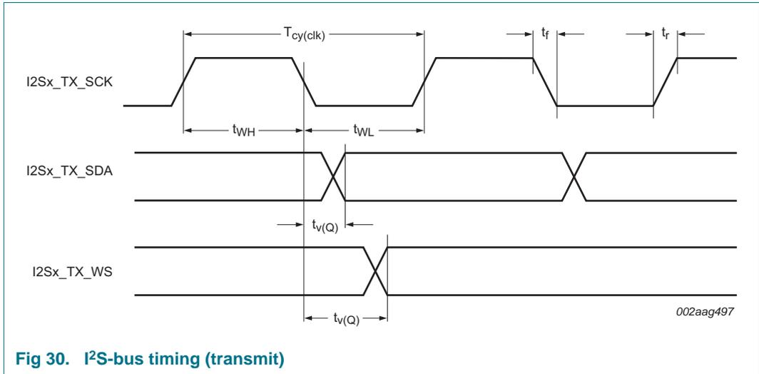
Fig 30. I<sup>2</sup>S-bus timing (transmit)
