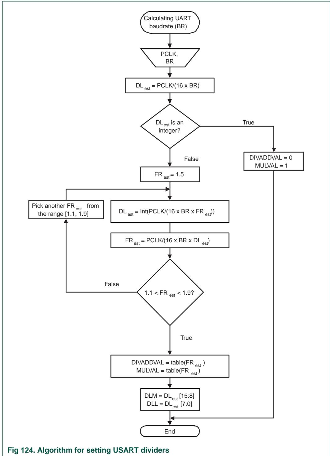
Fig 124. Algorithm for setting USART dividers
