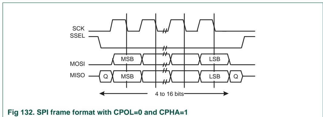
Fig 132. SPI frame format with CPOL=0 and CPHA=1
