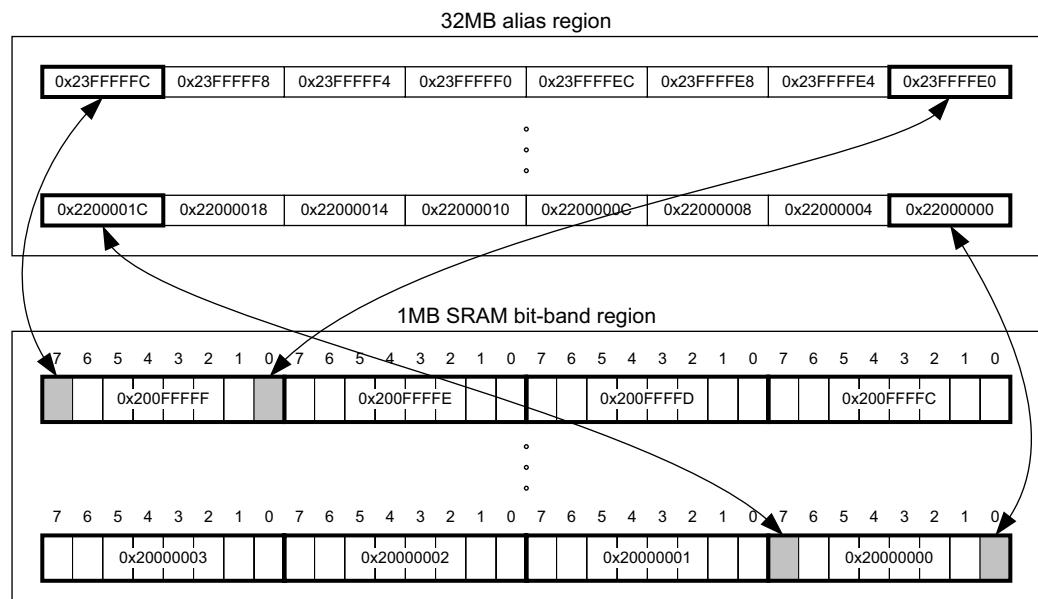
**Figure 2-1 Bit-band mapping**
