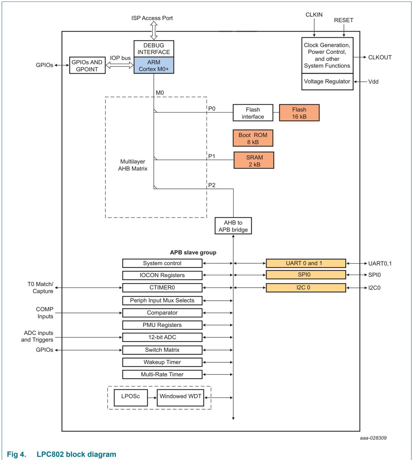
Fig 4. LPC802 block diagram
