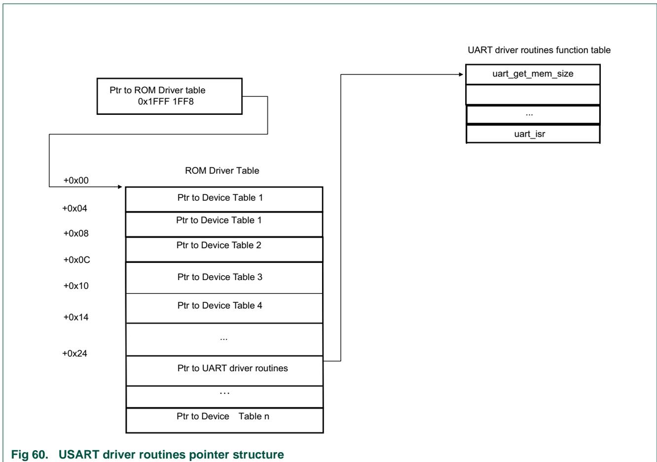
Fig 60. USART driver routines pointer structure
