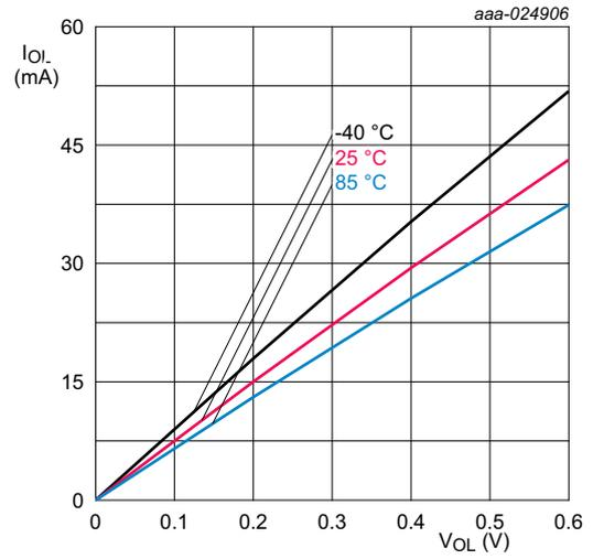
Conditions:  $V_{DD} = 3.3$  V; on pins PIO0\_10 and PIO0\_11.
