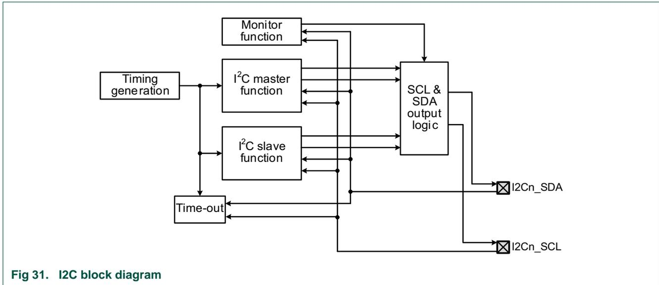
Fig 31. I2C block diagram
