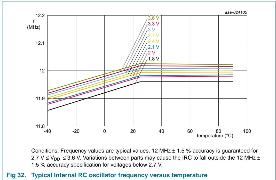
**Fig 32. Typical Internal RC oscillator frequency versus temperature**
