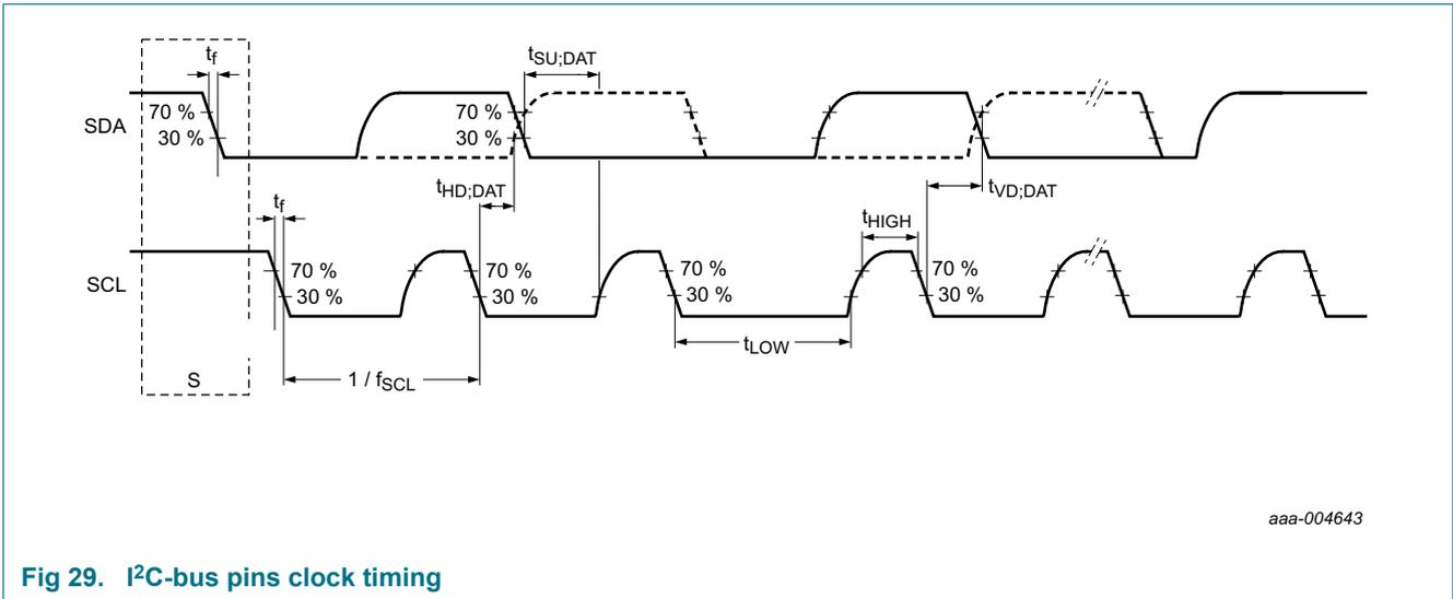
Fig 29. I<sup>2</sup>C-bus pins clock timing
