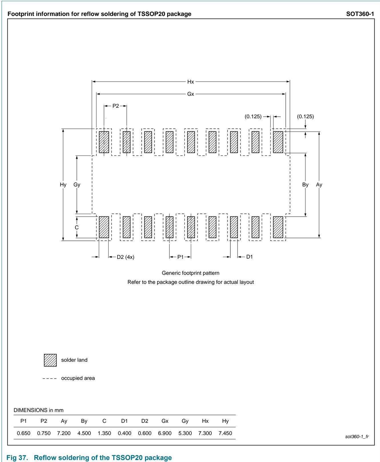
Fig 37. Reflow soldering of the TSSOP20 package
