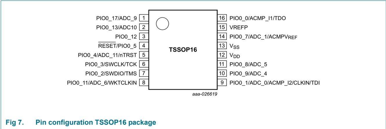
Fig 7. Pin configuration TSSOP16 package
