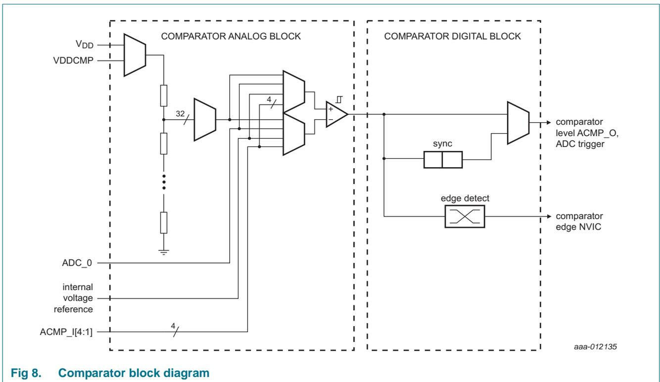
Fig 8. Comparator block diagram
