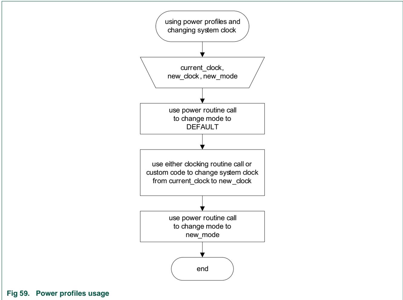
Fig 59. Power profiles usage
