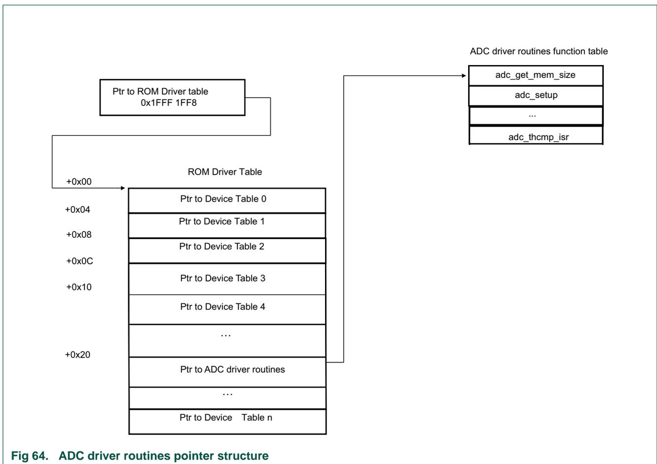
Fig 64. ADC driver routines pointer structure
