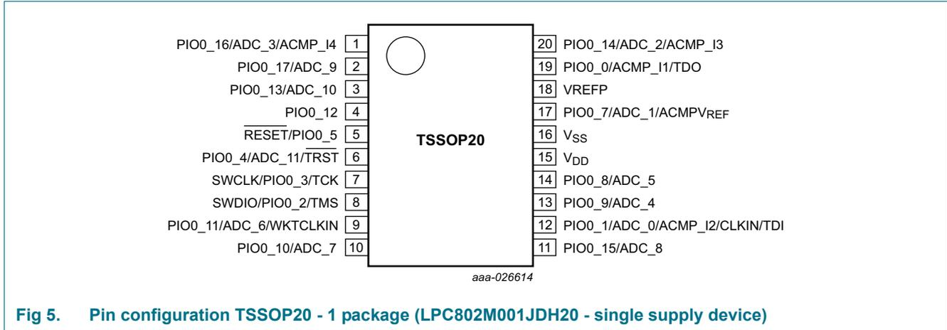
Fig 5. Pin configuration TSSOP20 - 1 package (LPC802M001JDH20 - single supply device)
