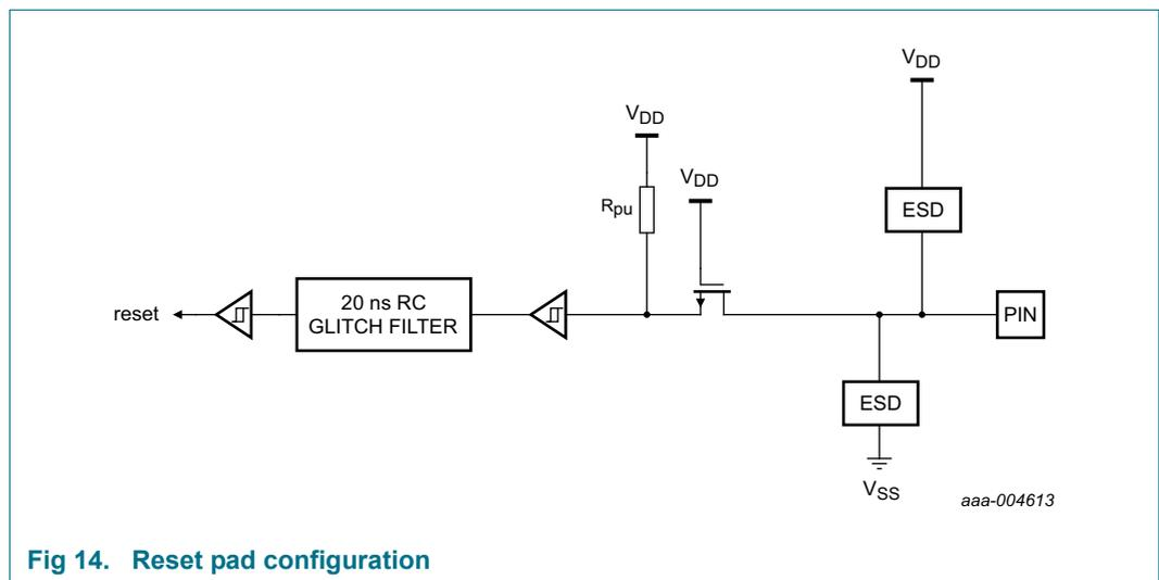
Fig 14. Reset pad configuration
