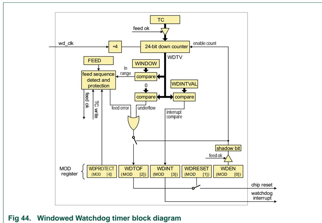
Fig 44. Windowed Watchdog timer block diagram
