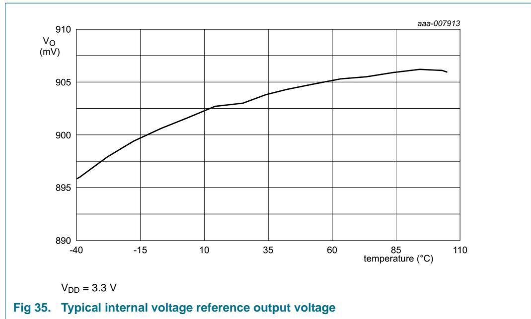
Fig 35. Typical internal voltage reference output voltage
