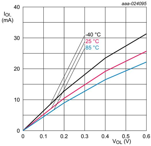
Conditions:  $V_{DD} = 1.8$  V; on pins PIO0\_10 and PIO0\_11.
