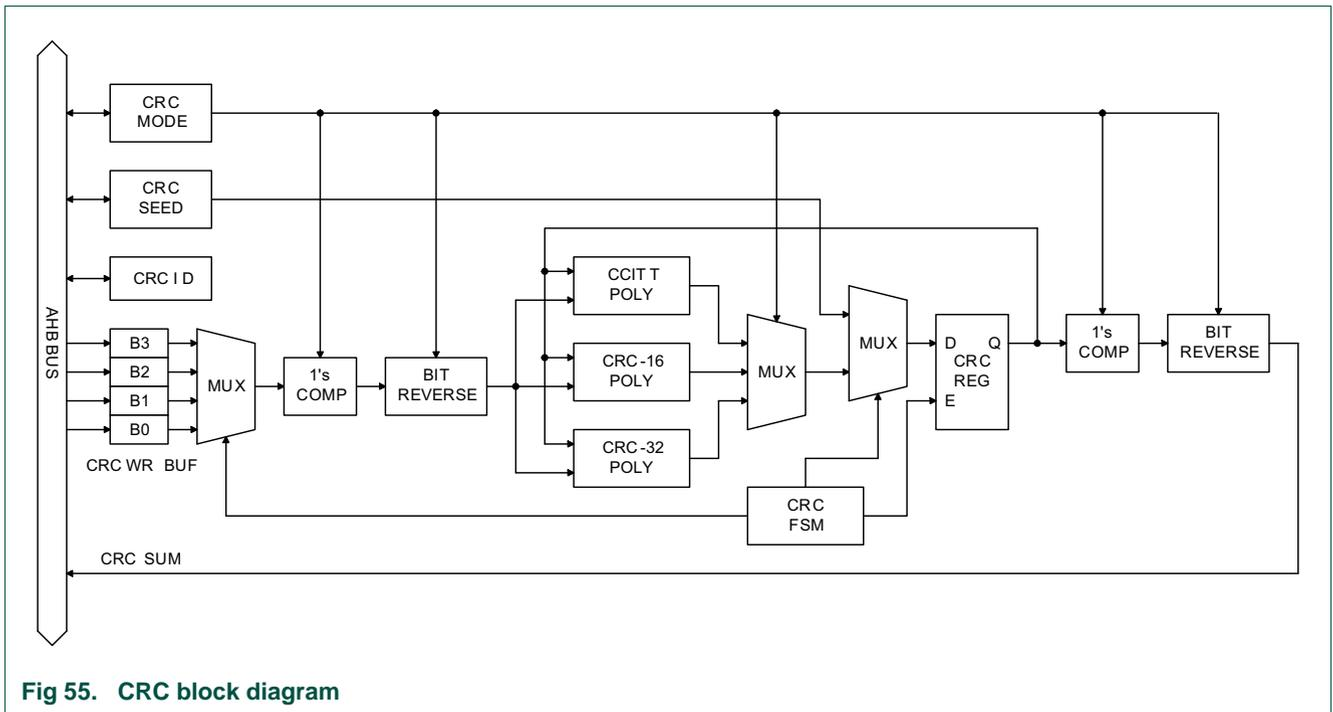
Fig 55. CRC block diagram
