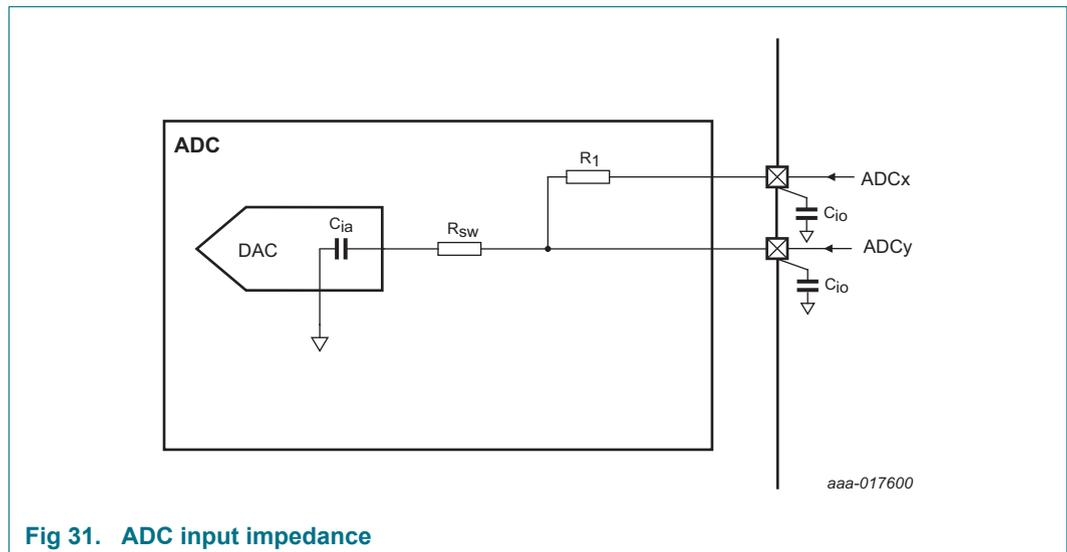
Fig 31. ADC input impedance
