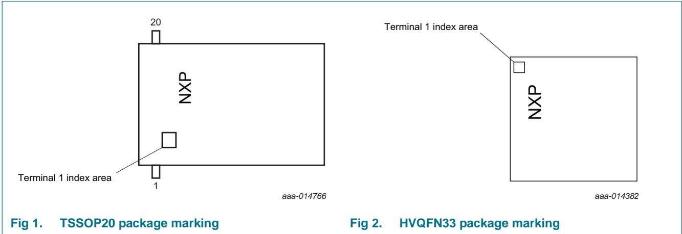
Fig 1. TSSOP20 package marking
