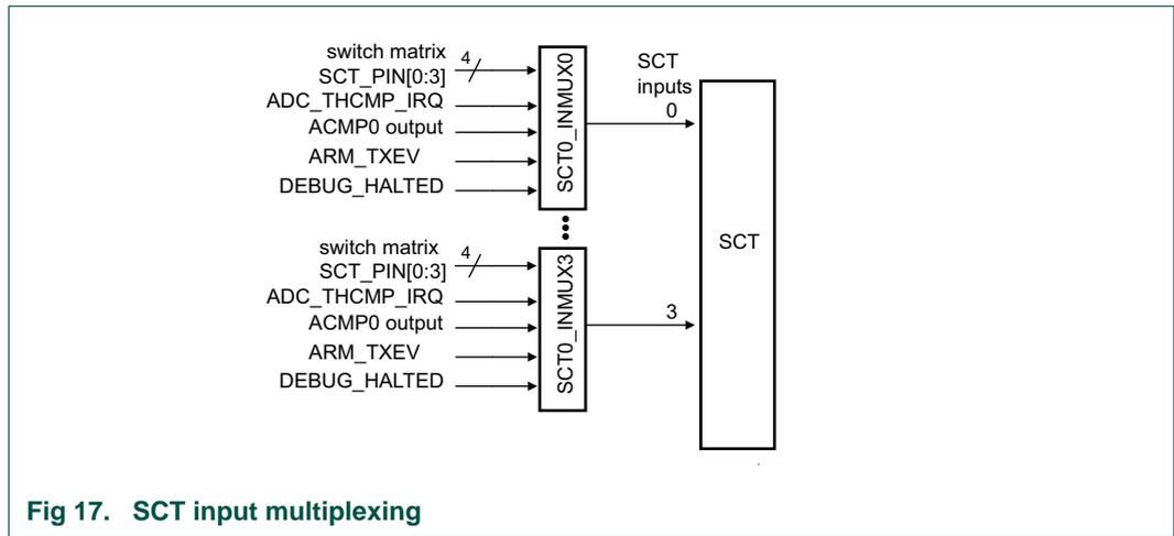
Fig 17. SCT input multiplexing
