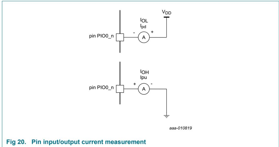
Fig 20. Pin input/output current measurement
