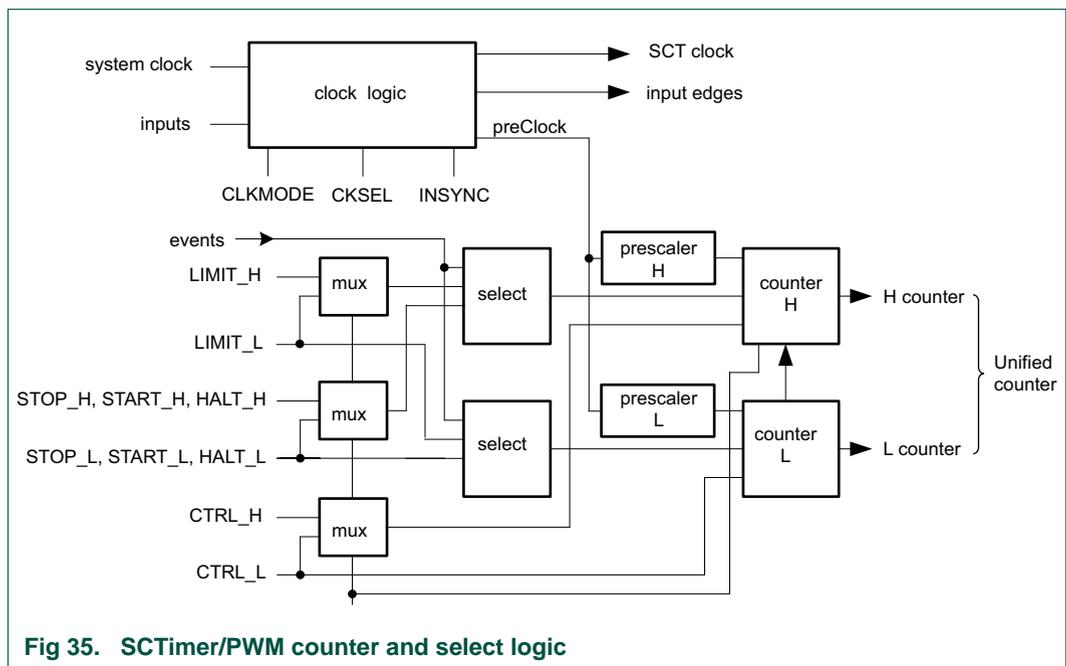
Fig 35. SCTimer/PWM counter and select logic
