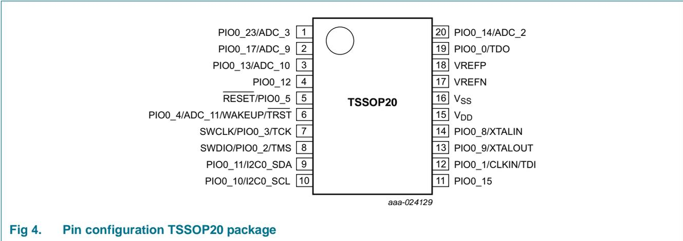
Fig 4. Pin configuration TSSOP20 package
