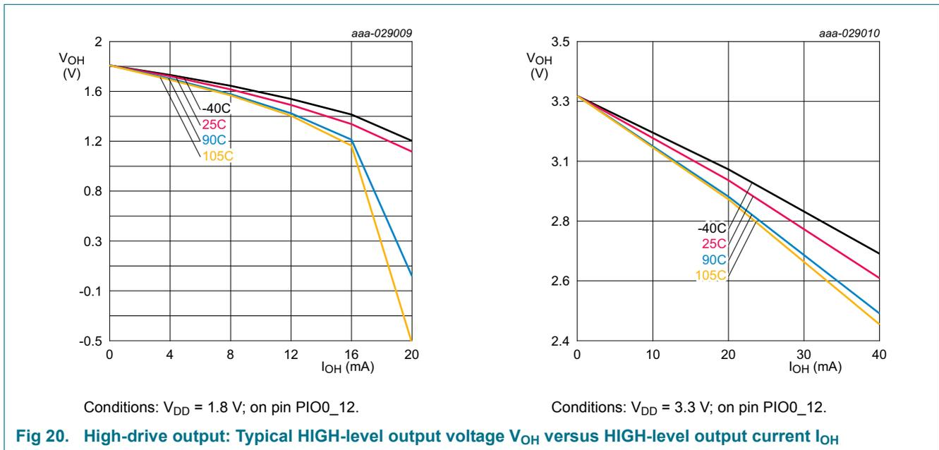
Fig 20. High-drive output: Typical HIGH-level output voltage  $V_{OH}$  versus HIGH-level output current  $I_{OH}$
