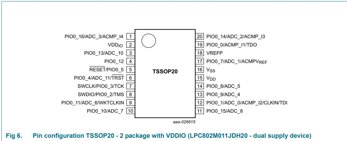
Fig 6. Pin configuration TSSOP20 - 2 package with VDDIO (LPC802M011JDH20 - dual supply device)
