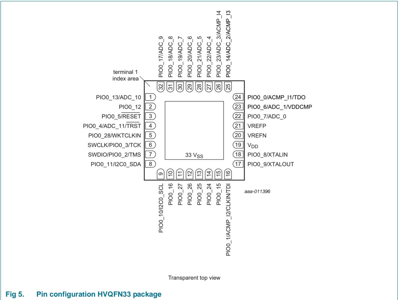
Fig 5. Pin configuration HVQFN33 package
