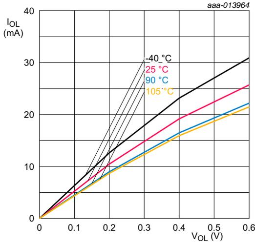
Conditions:  $V_{DD} = 1.8\text{ V}$ ; on pins PIO0\_10 and PIO0\_11.
