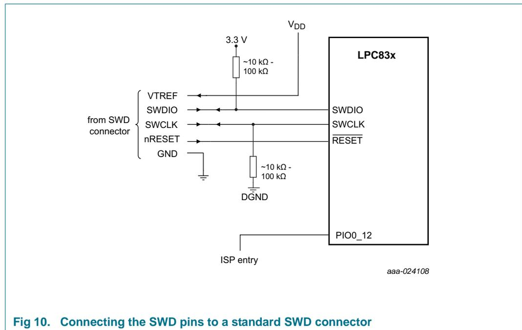
**Fig 10. Connecting the SWD pins to a standard SWD connector**
