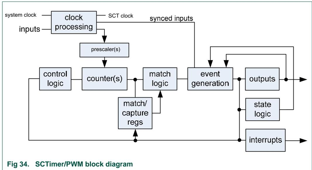
Fig 34. SCTimer/PWM block diagram
