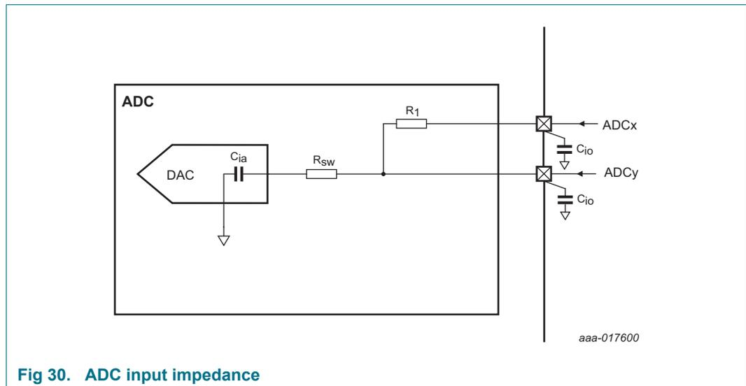
Fig 30. ADC input impedance
