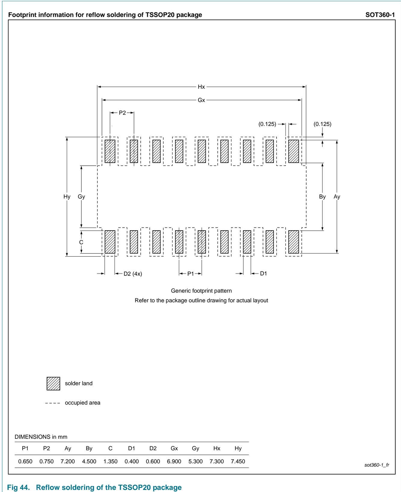
Fig 44. Reflow soldering of the TSSOP20 package
