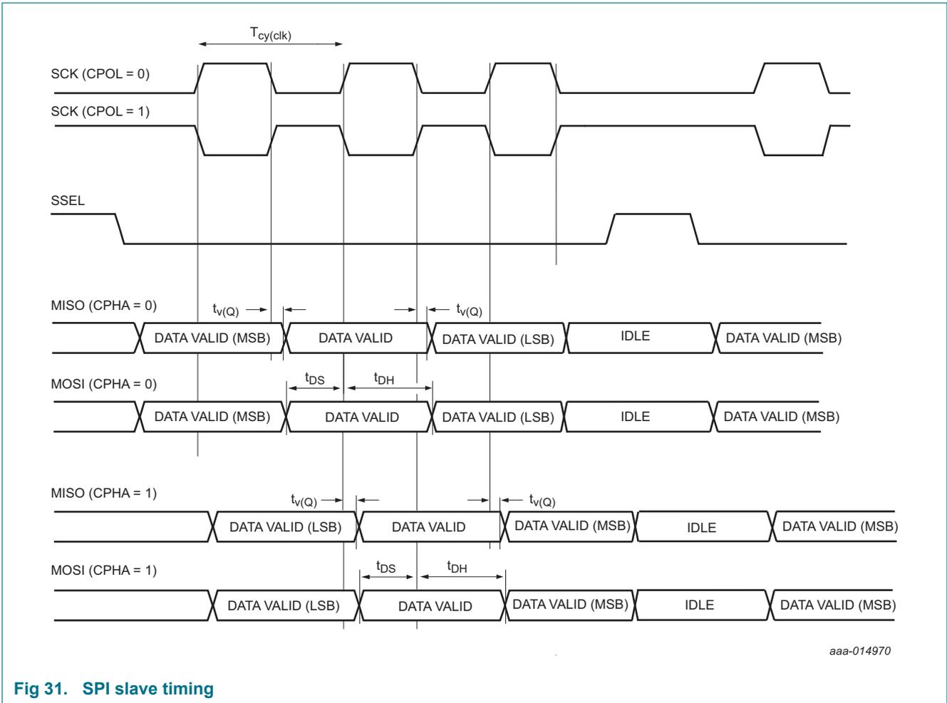
Fig 31. SPI slave timing
