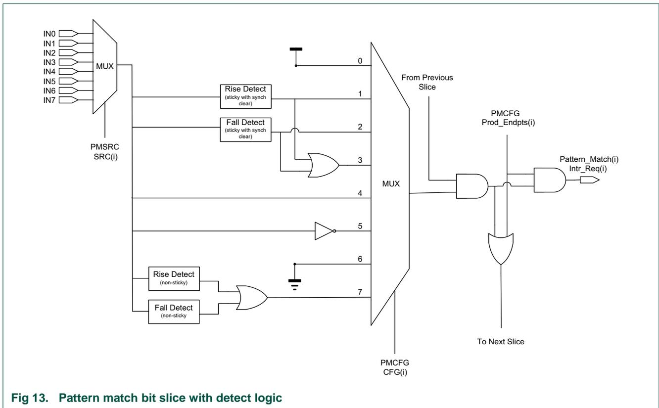
Fig 13. Pattern match bit slice with detect logic
