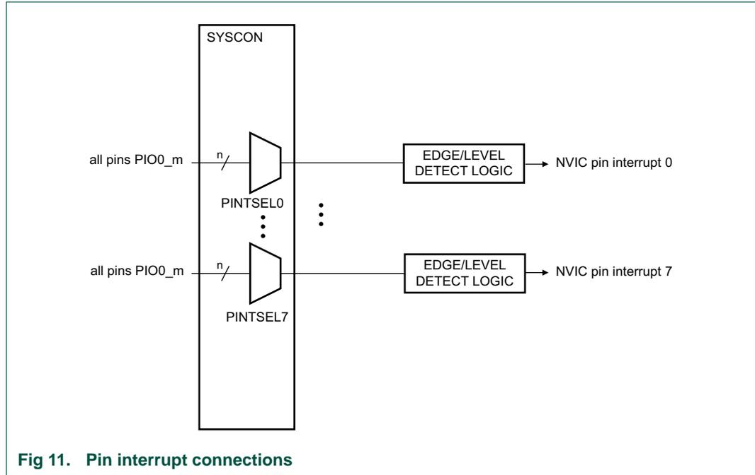
Fig 11. Pin interrupt connections
