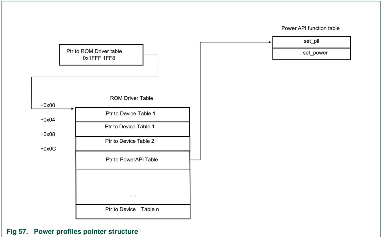
Fig 57. Power profiles pointer structure
