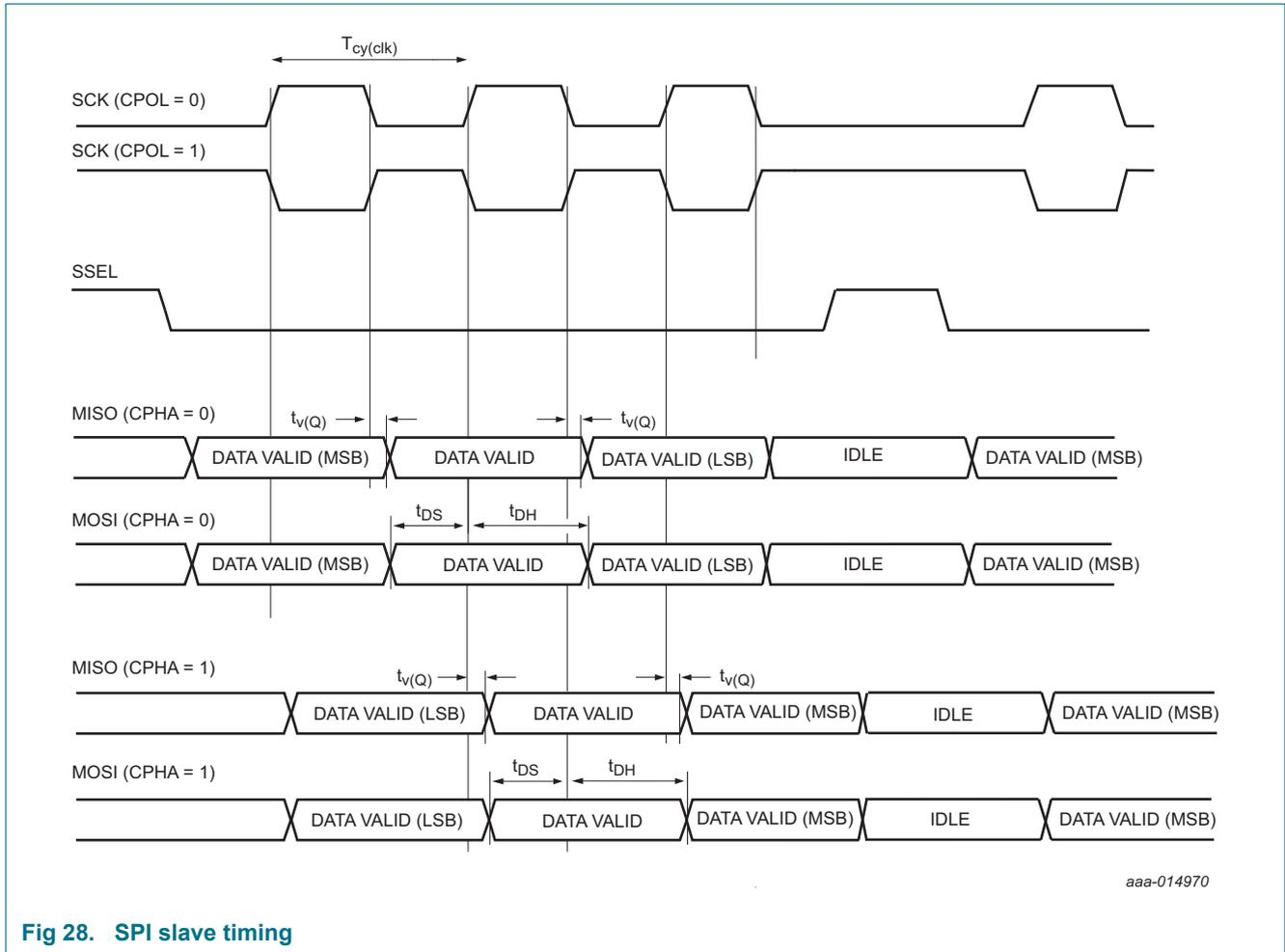
Fig 28. SPI slave timing
