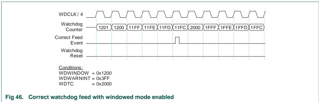
Fig 46. Correct watchdog feed with windowed mode enabled
