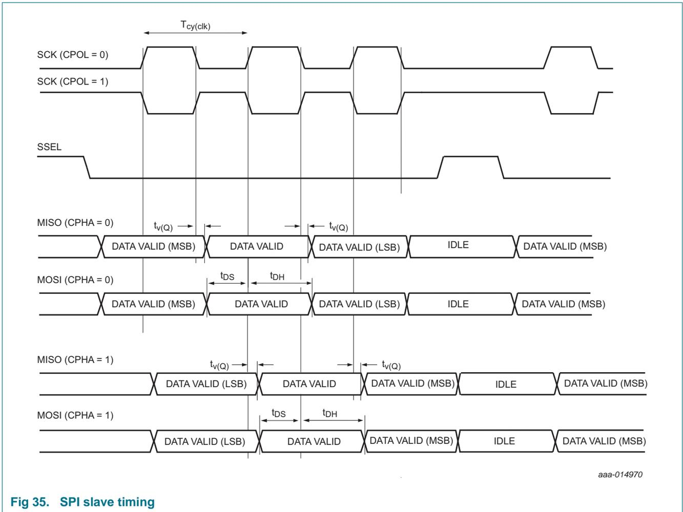
Fig 35. SPI slave timing
