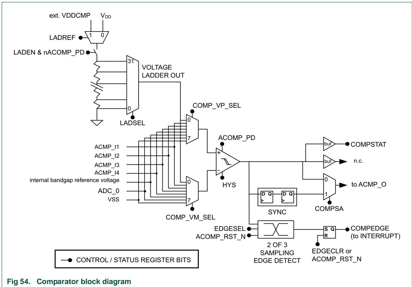
Fig 54. Comparator block diagram
