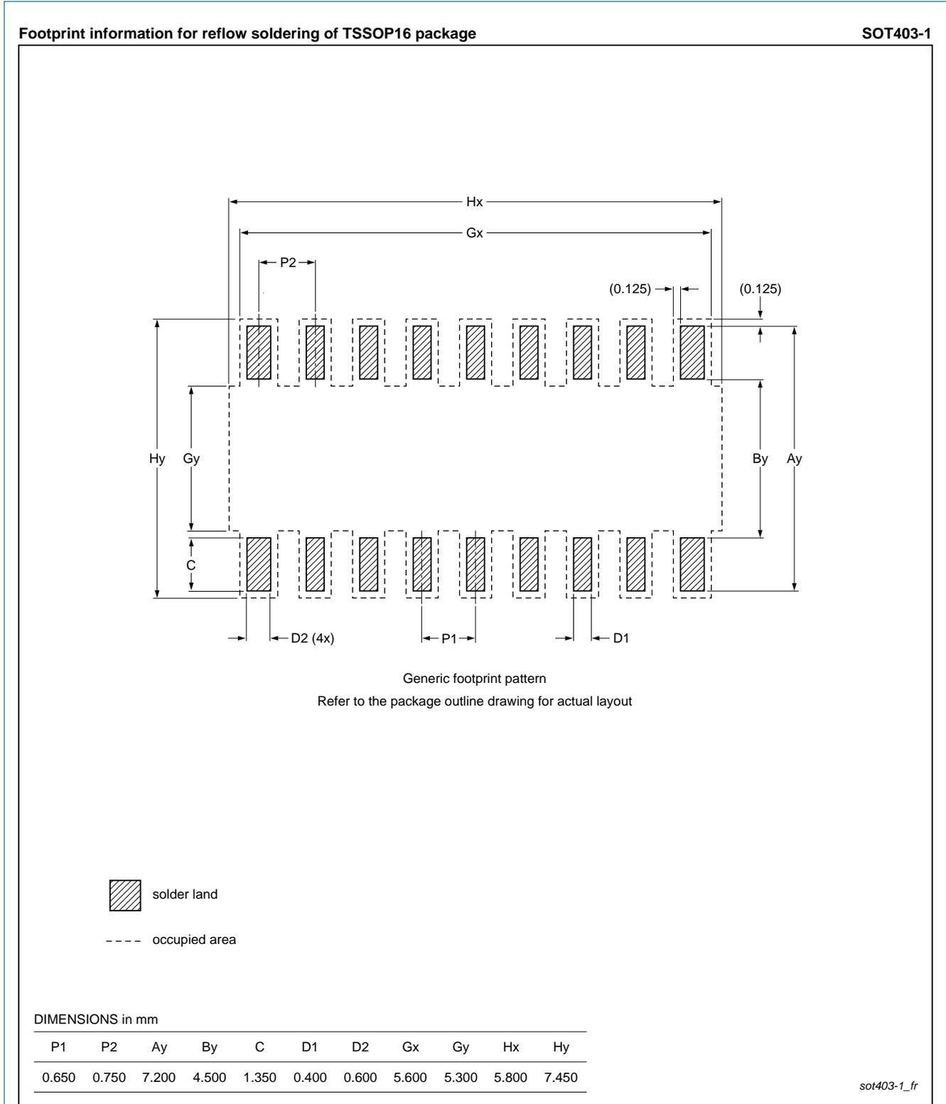
**Fig 40. Reflow soldering of the TSSOP16 package**
