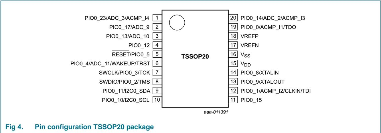
Fig 4. Pin configuration TSSOP20 package
