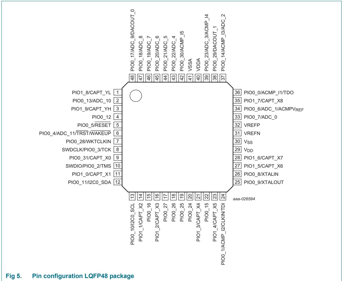
Fig 5. Pin configuration LQFP48 package
