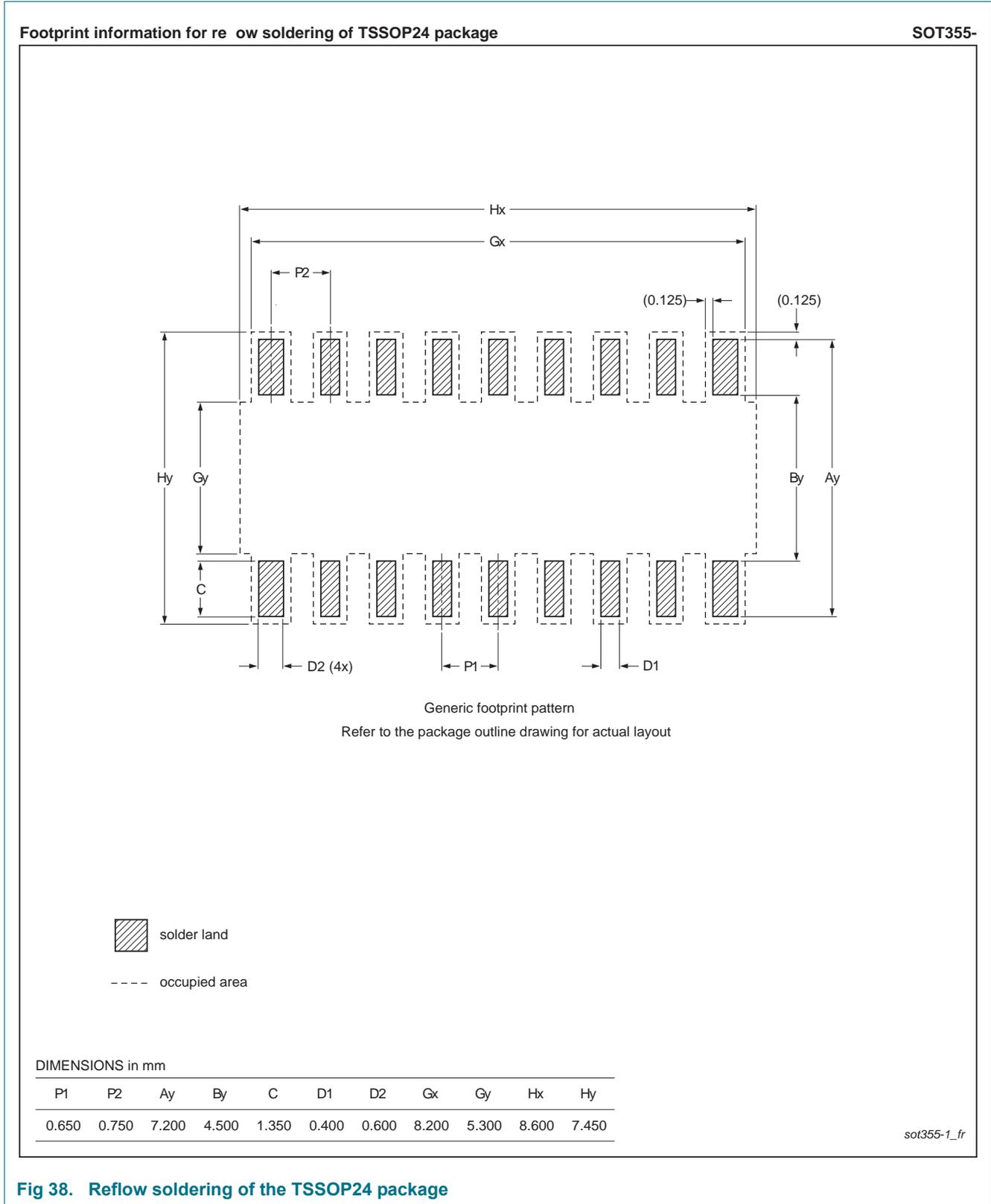
Fig 38. Reflow soldering of the TSSOP24 package
