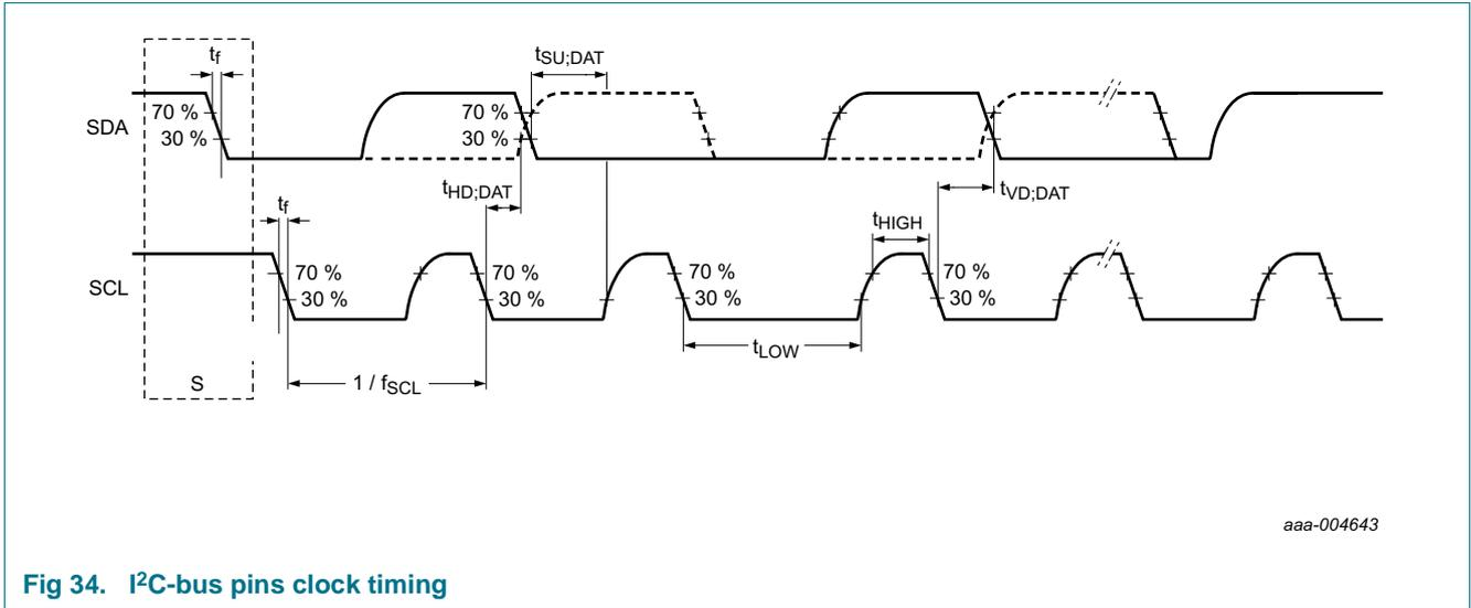
Fig 34. I<sup>2</sup>C-bus pins clock timing
