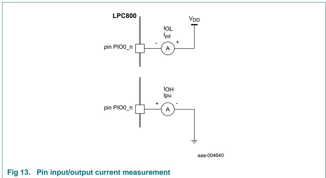
**Fig 13. Pin input/output current measurement**
