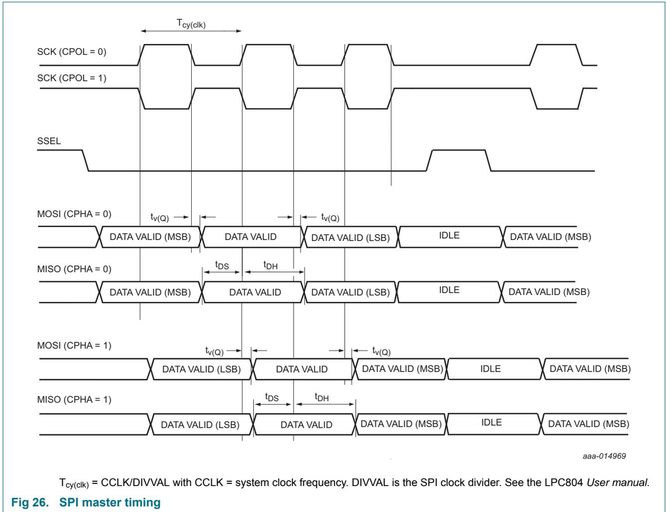
Fig 26. SPI master timing
