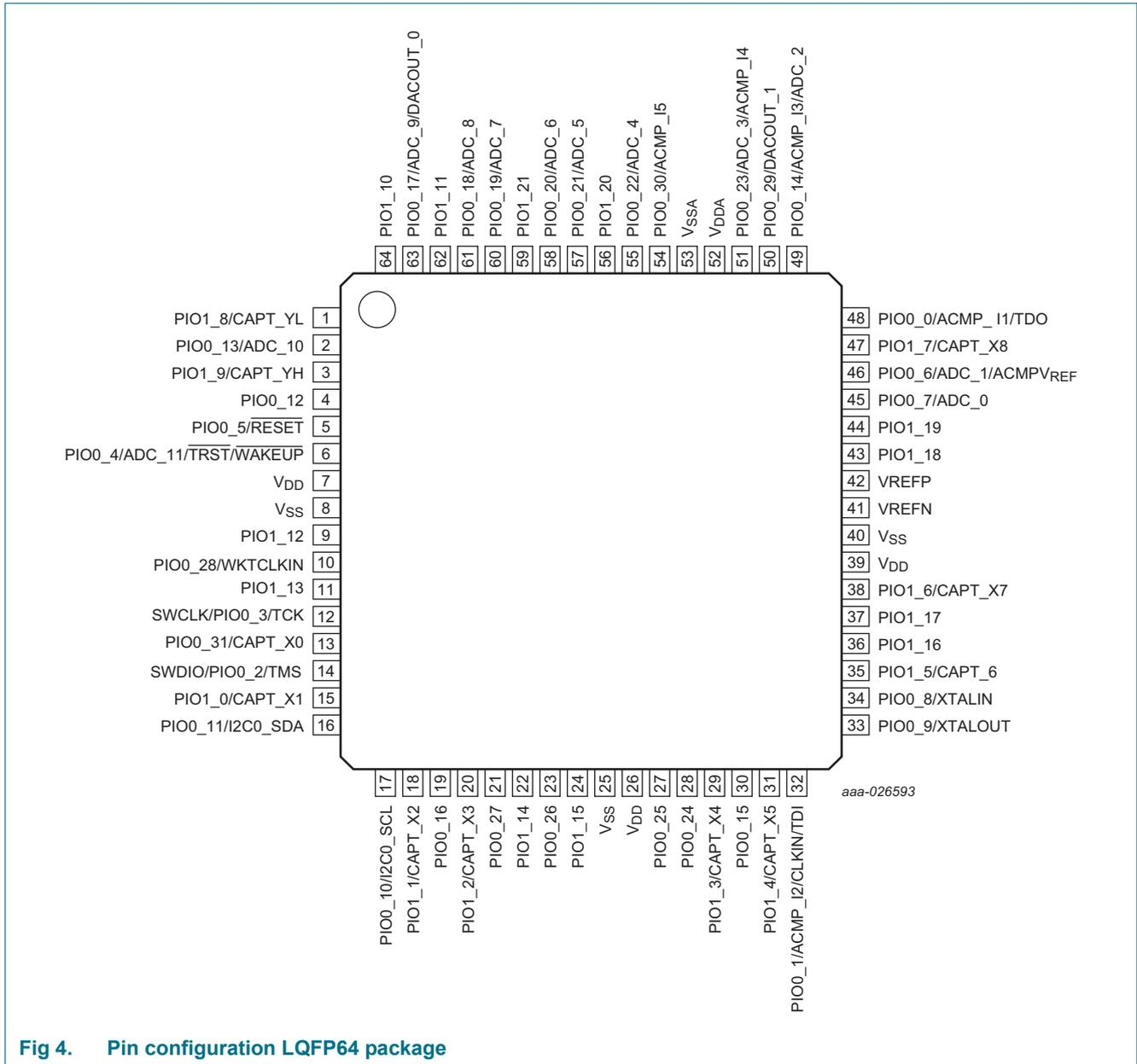
Fig 4. Pin configuration LQFP64 package
