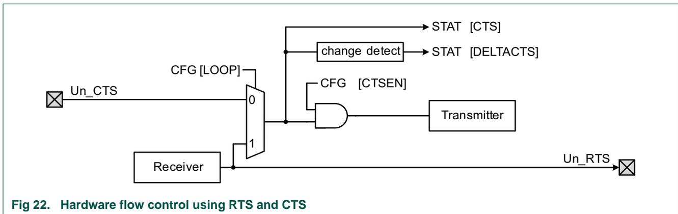
Fig 22. Hardware flow control using RTS and CTS
