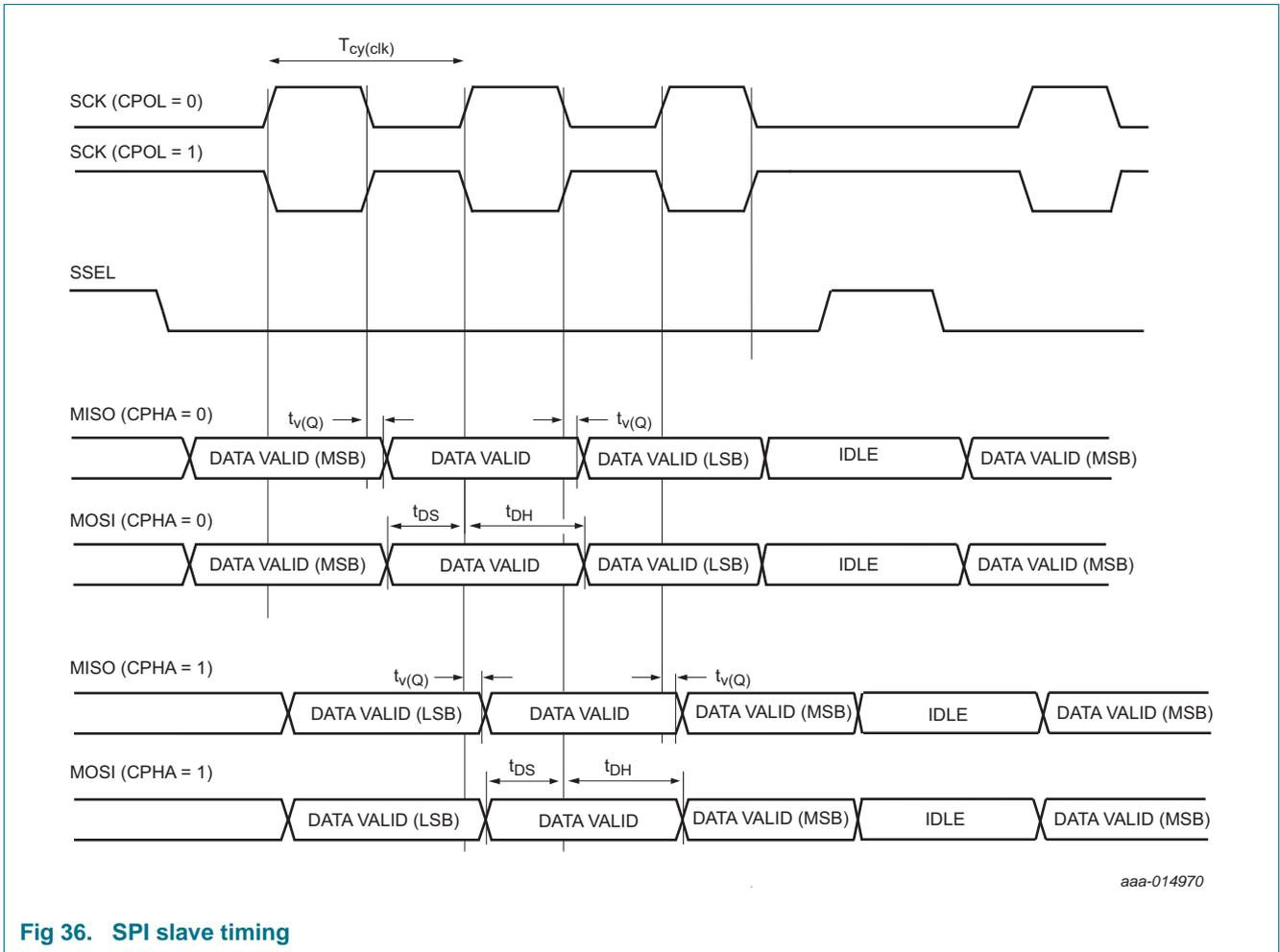
Fig 36. SPI slave timing
