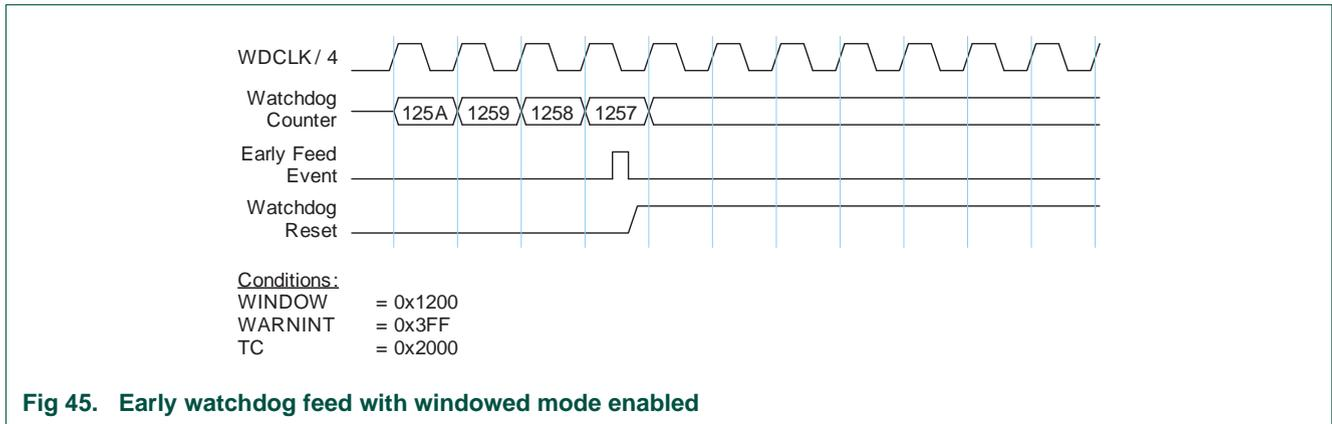
Fig 45. Early watchdog feed with windowed mode enabled
