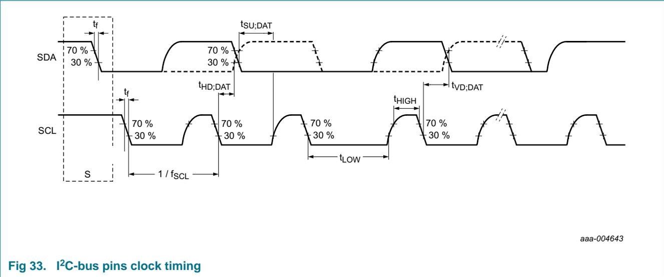
Fig 33. I<sup>2</sup>C-bus pins clock timing
