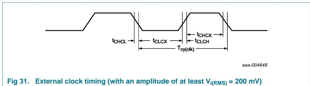
**Fig 31. External clock timing (with an amplitude of at least  $V_{i(RMS)} = 200\text{ mV}$ )**
