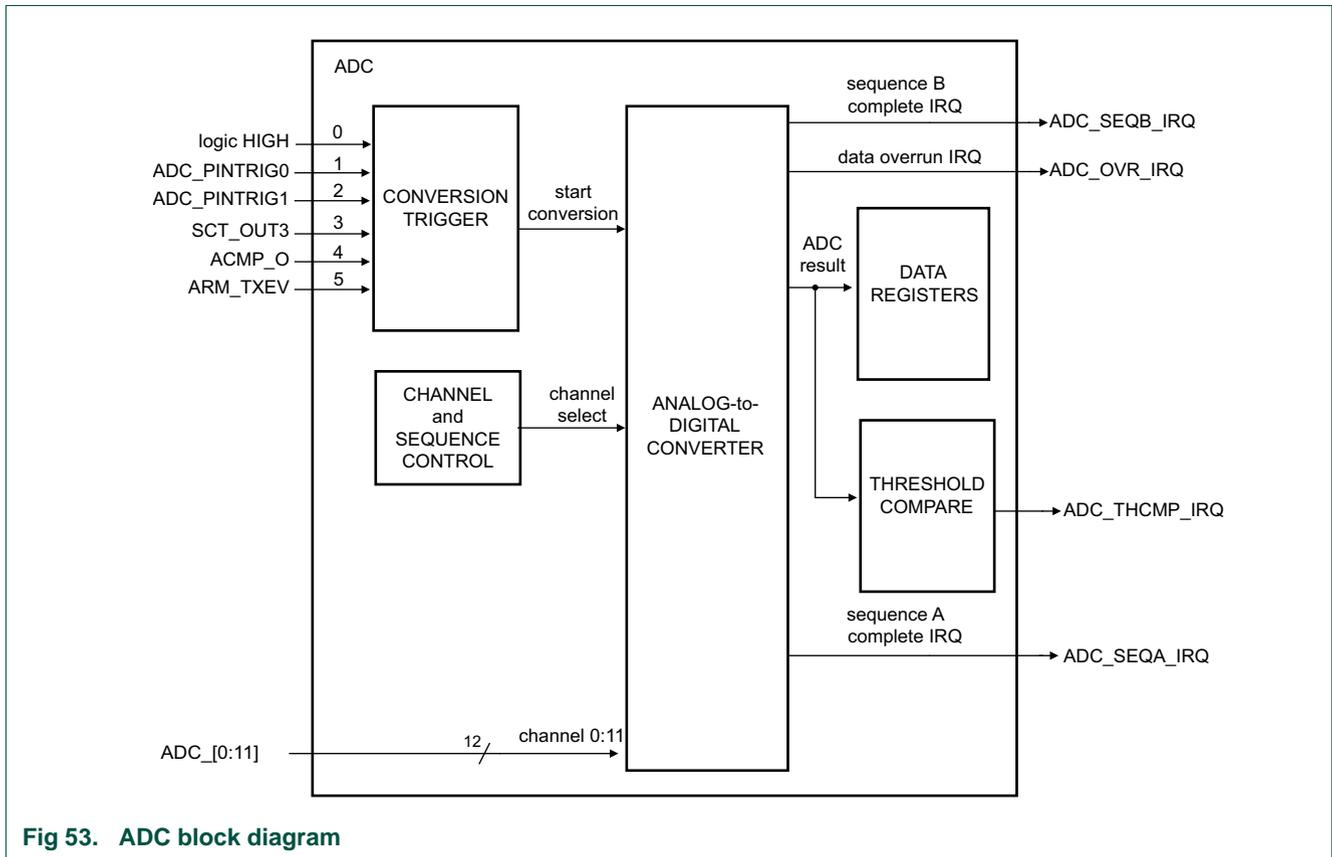
Fig 53. ADC block diagram
