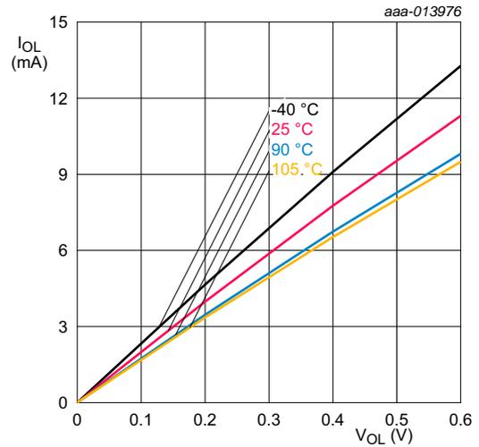
Conditions:  $V_{DD} = 3.3\text{ V}$ ; standard port pins and high-drive pin PIO0\_12.
