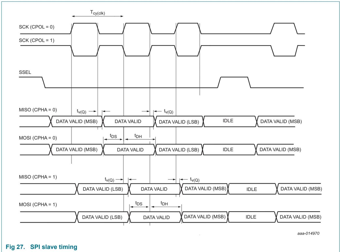
Fig 27. SPI slave timing
