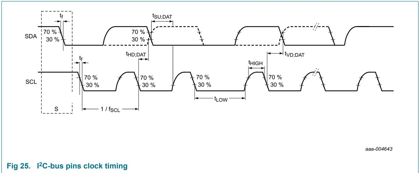
Fig 25. I<sup>2</sup>C-bus pins clock timing
