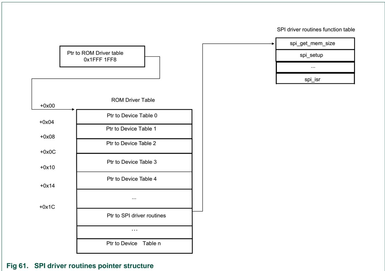
Fig 61. SPI driver routines pointer structure
