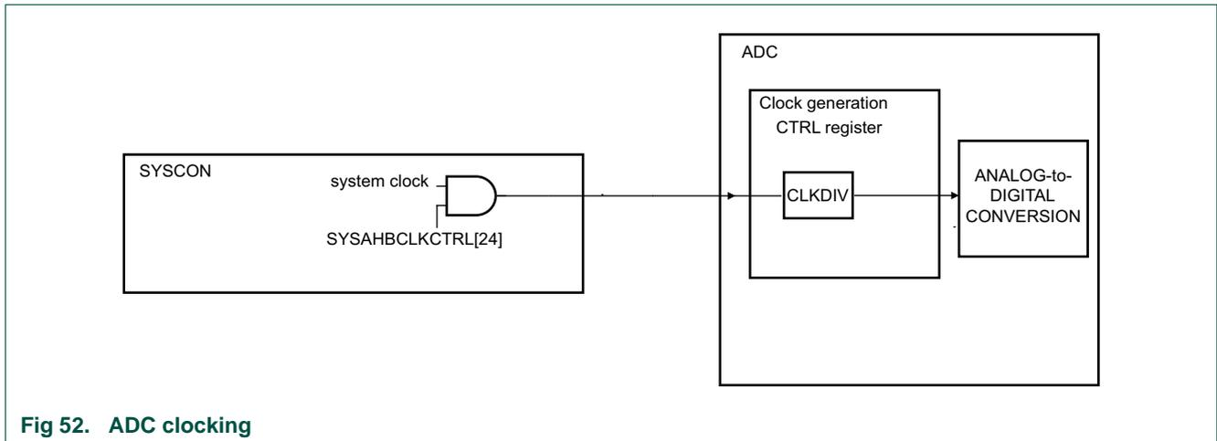
Fig 52. ADC clocking
