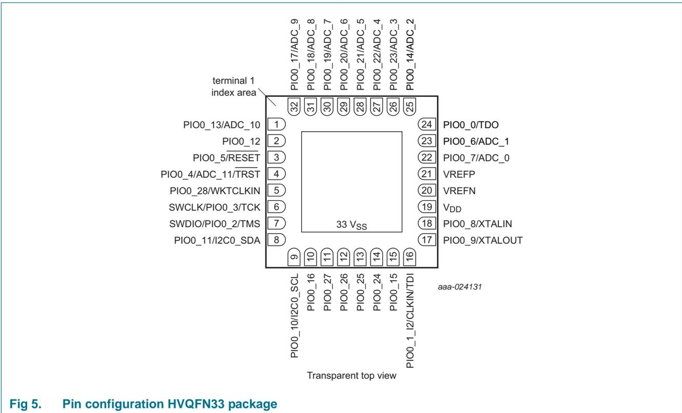
Fig 5. Pin configuration HVQFN33 package
