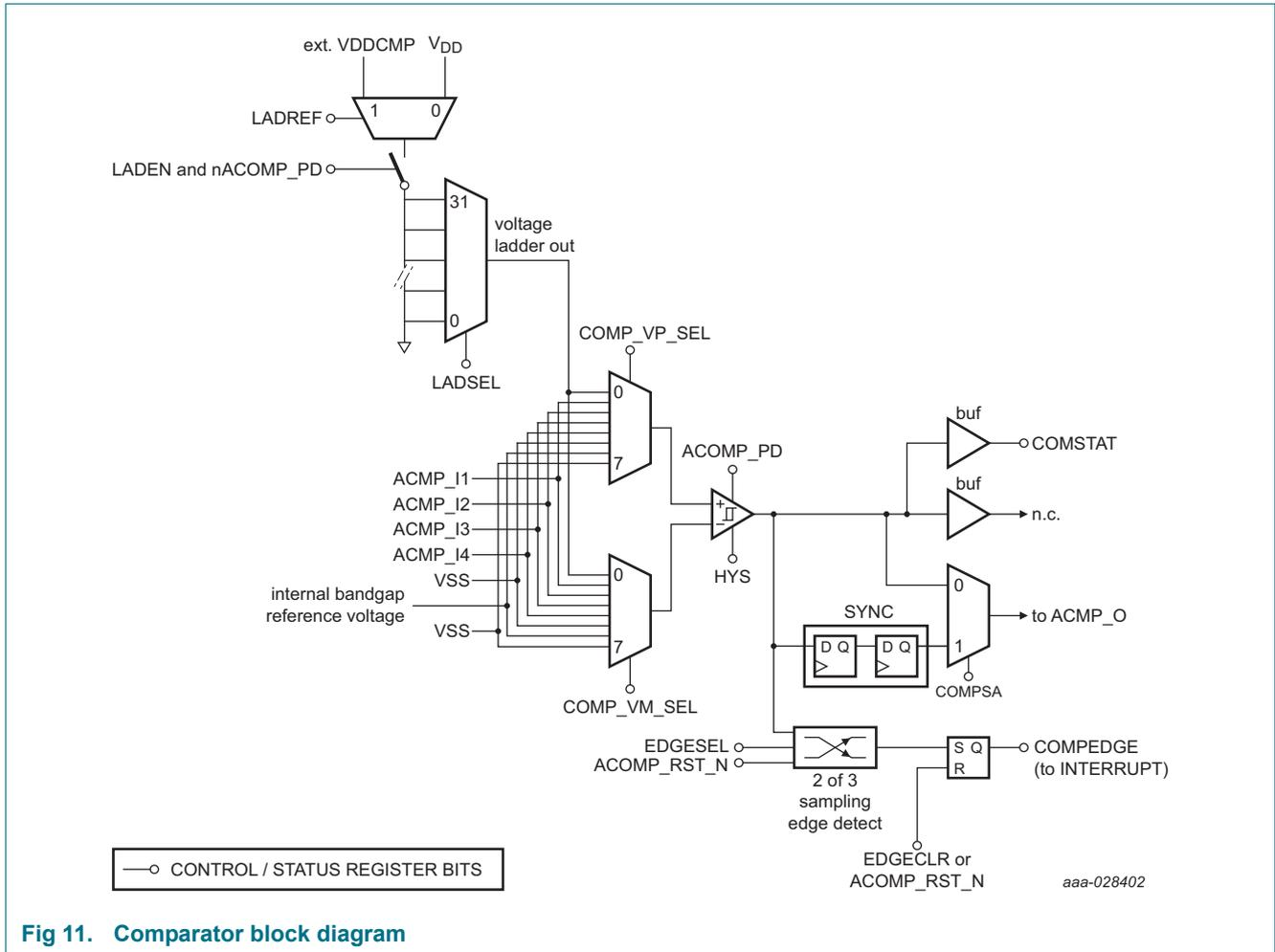
Fig 11. Comparator block diagram
