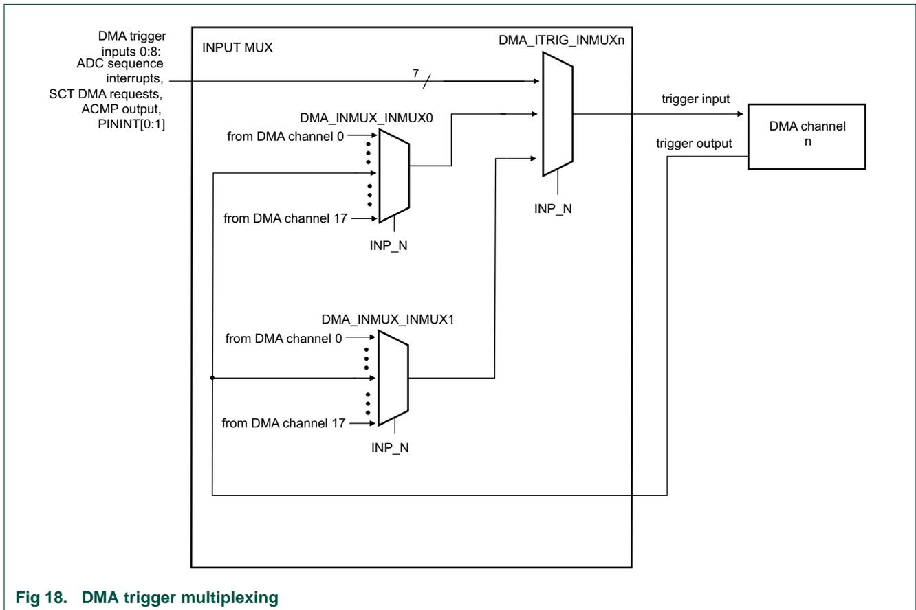
Fig 18. DMA trigger multiplexing
