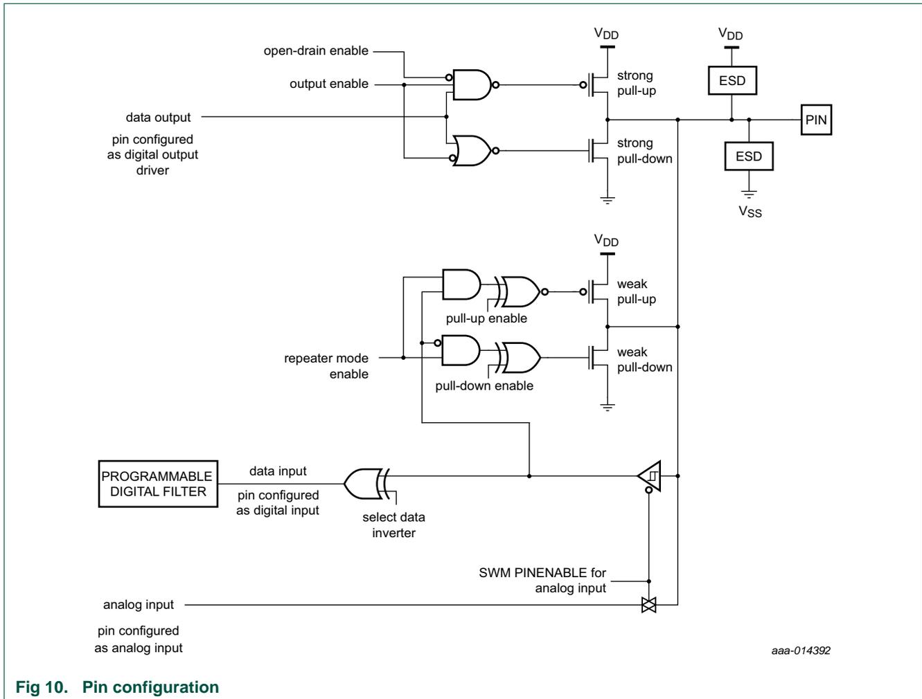
Fig 10. Pin configuration
