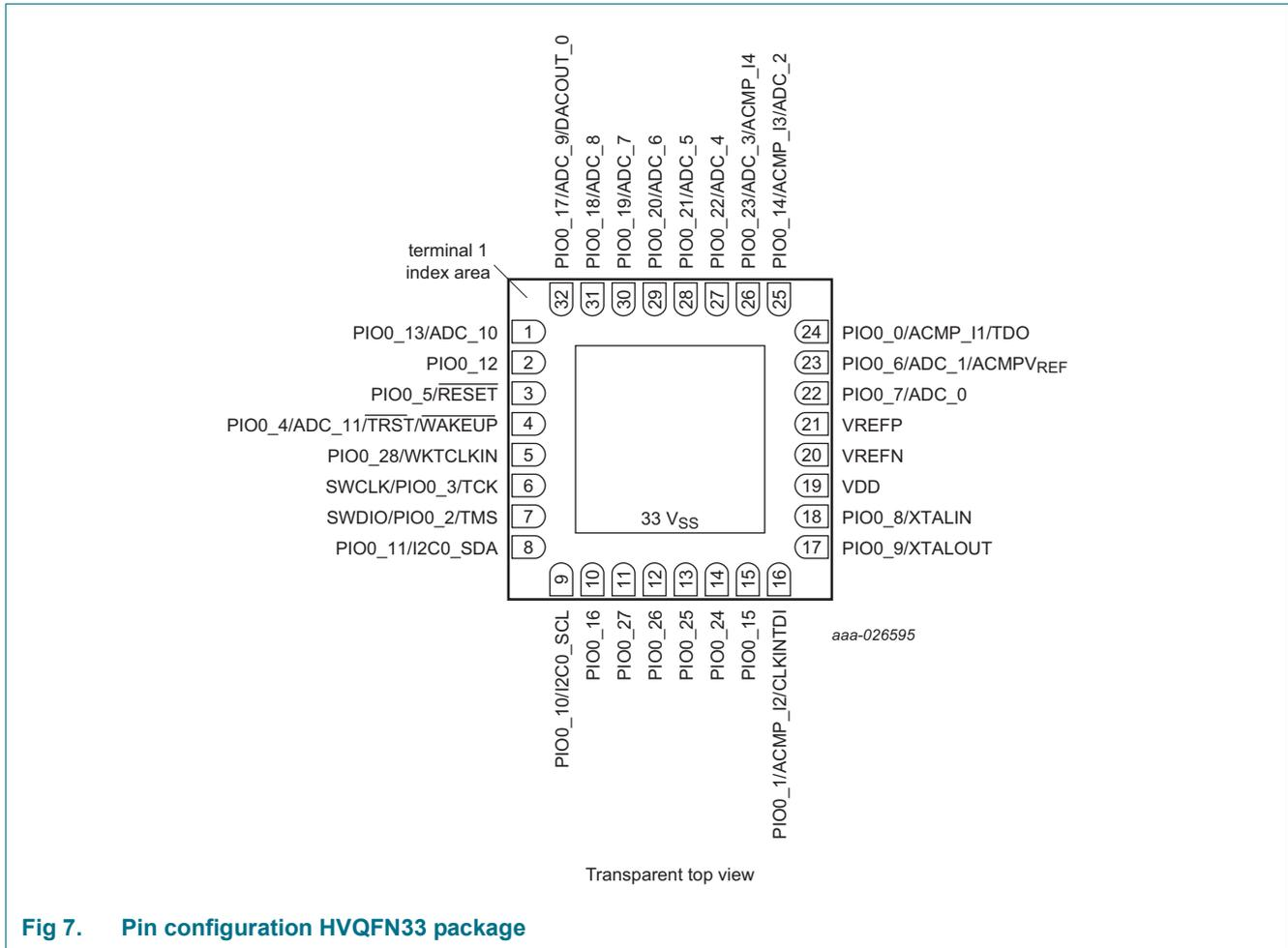
Fig 7. Pin configuration HVQFN33 package
