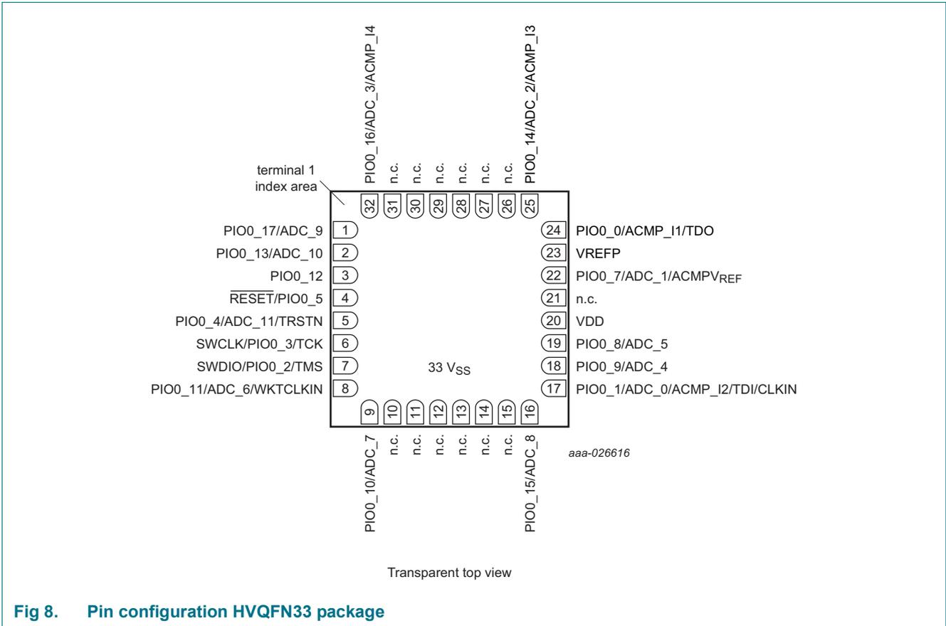
Fig 8. Pin configuration HVQFN33 package
