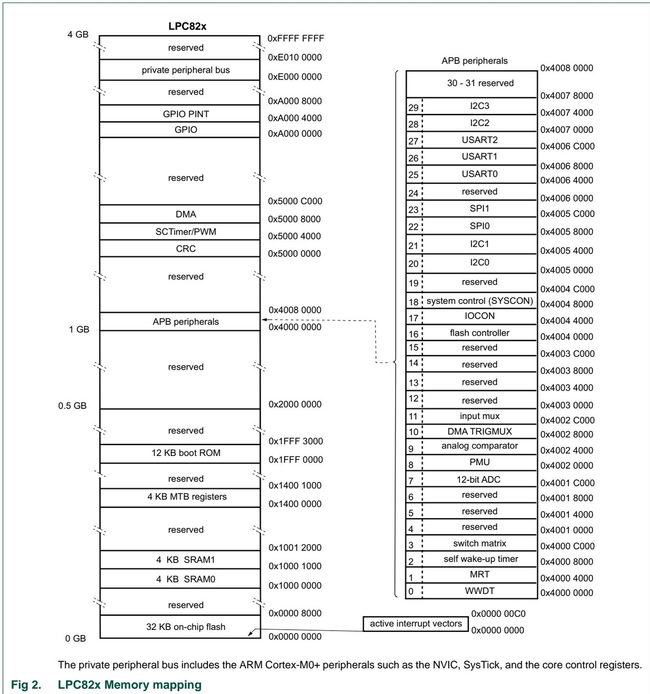
The private peripheral bus includes the ARM Cortex-M0+ peripherals such as the NVIC, SysTick, and the core control registers.
