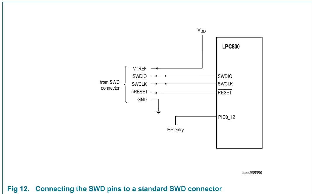
**Fig 12. Connecting the SWD pins to a standard SWD connector**
