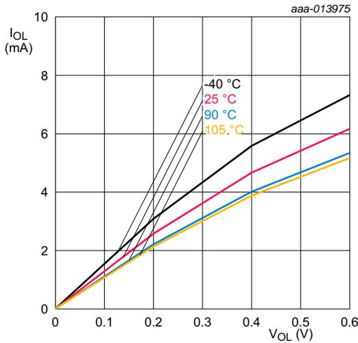
Conditions:  $V_{DD} = 1.8\text{ V}$ ; standard port pins and high-drive pin PIO0\_12.
