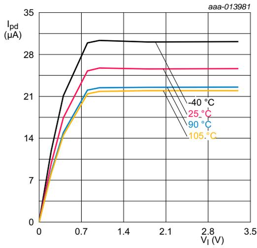
Conditions:  $V_{DD} = 1.8\text{ V}$ ; standard port pins.
