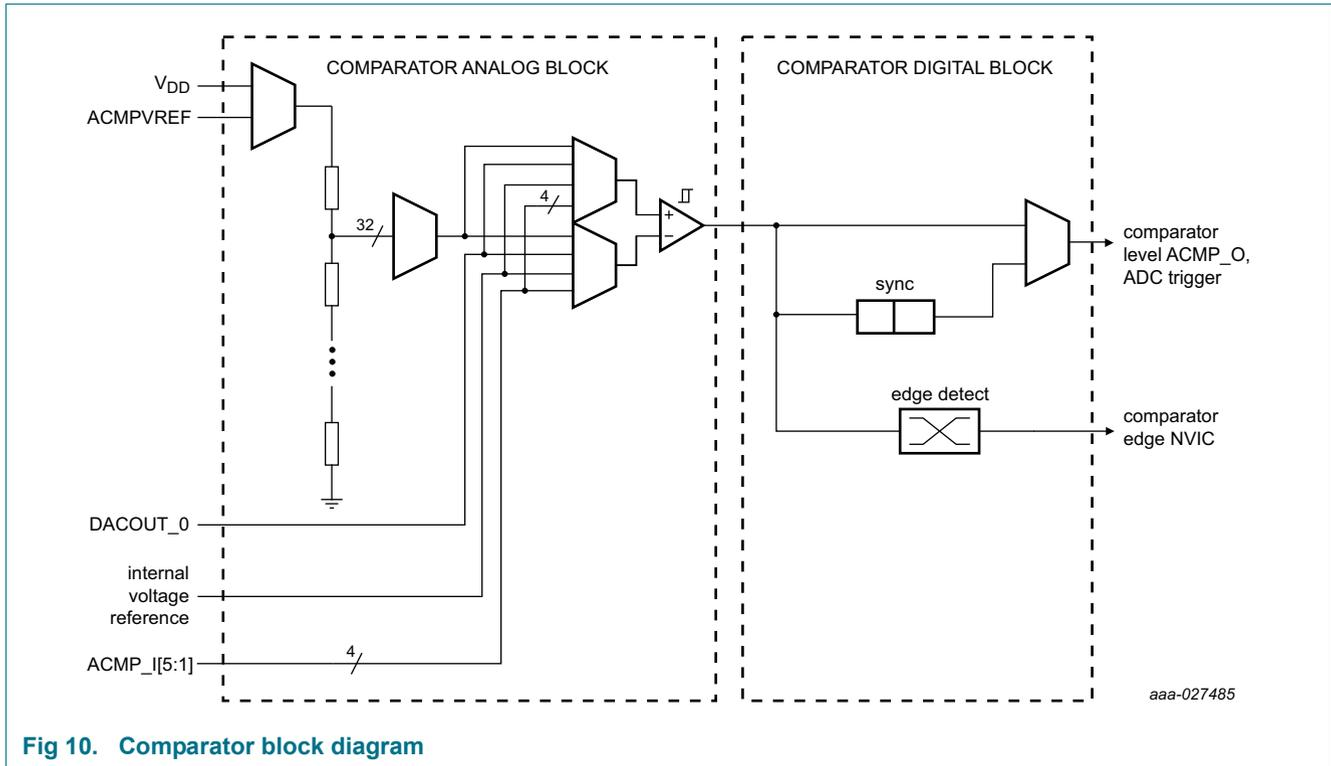
Fig 10. Comparator block diagram
