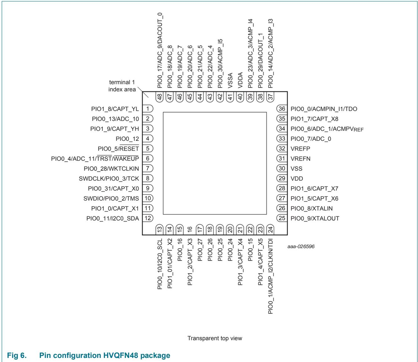
Fig 6. Pin configuration HVQFN48 package
