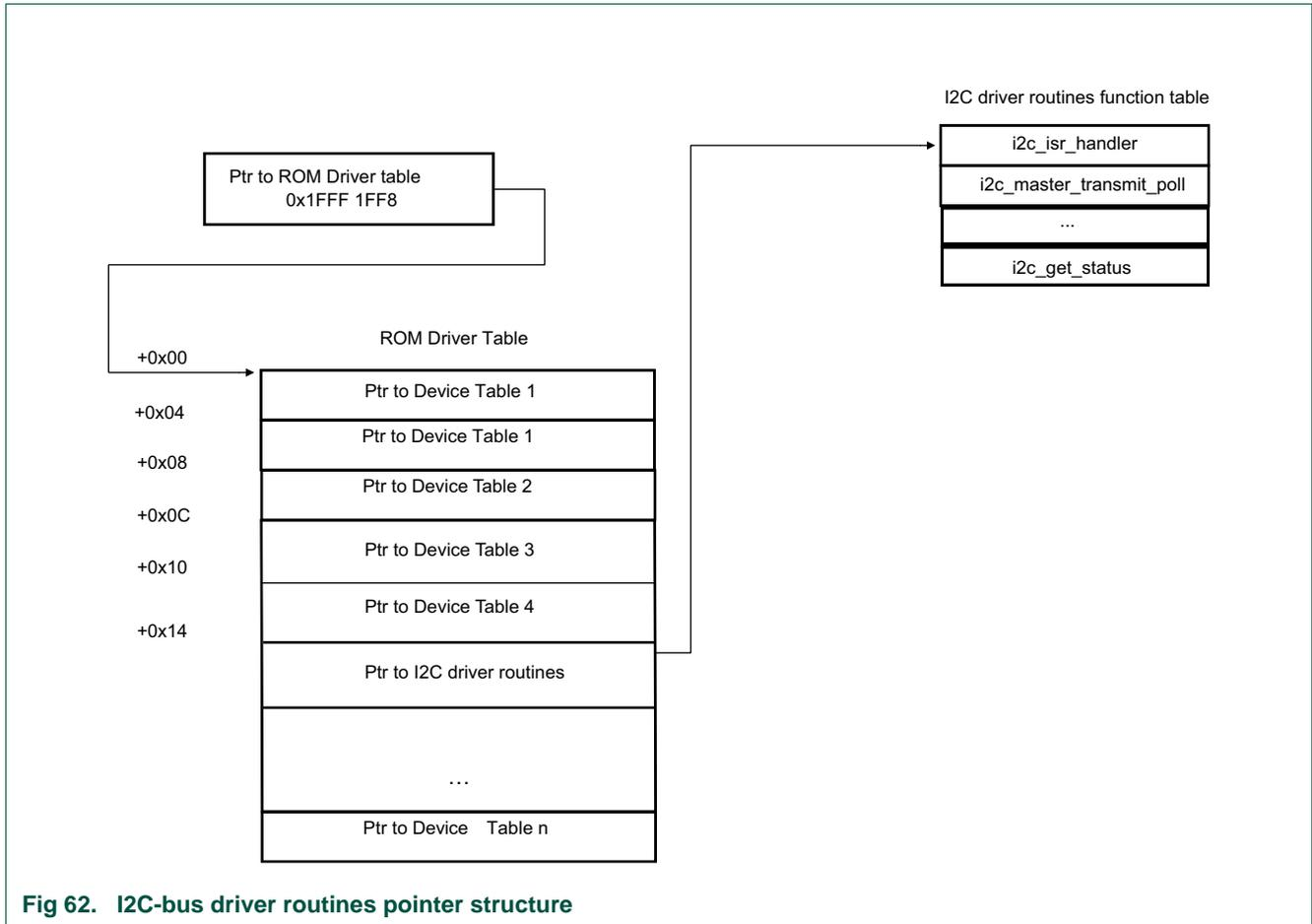
Fig 62. I2C-bus driver routines pointer structure
