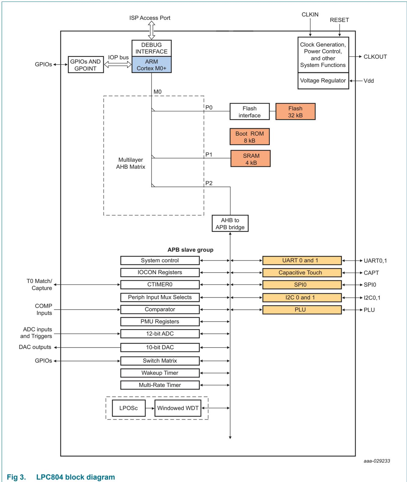
Fig 3. LPC804 block diagram
