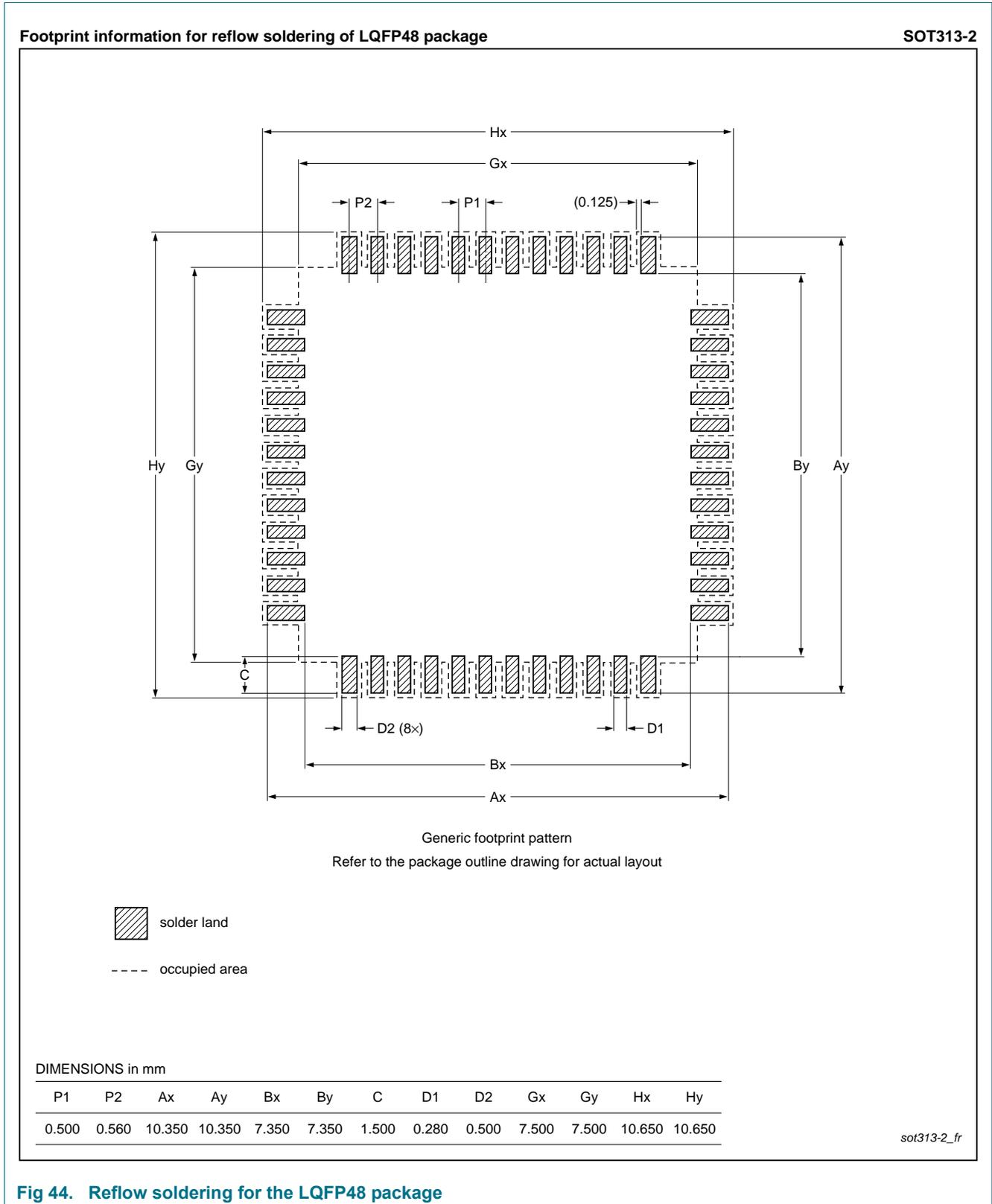
Fig 44. Reflow soldering for the LQFP48 package
