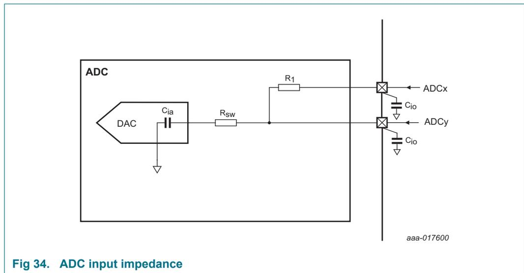
Fig 34. ADC input impedance
