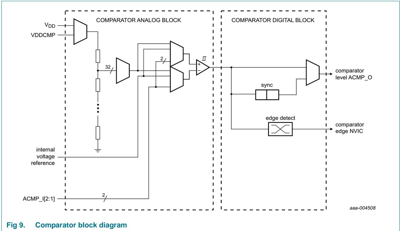
Fig 9. Comparator block diagram
