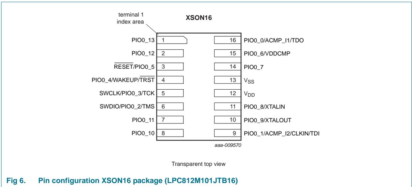
Fig 6. Pin configuration XSON16 package (LPC812M101JT B16)
