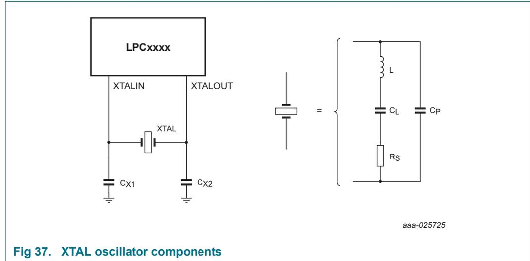
Fig 37. XTAL oscillator components
