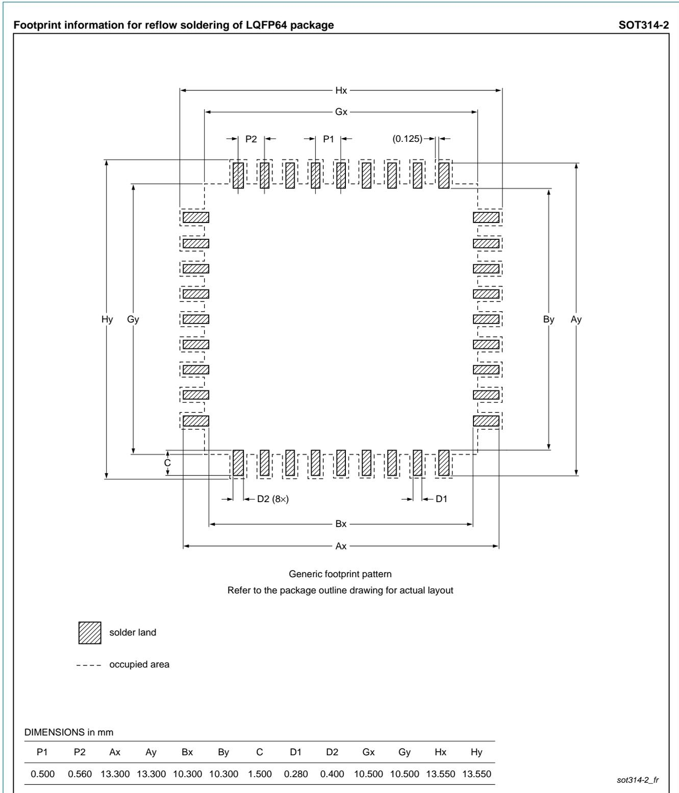
**Fig 45. Reflow soldering for the LQFP64 package**
