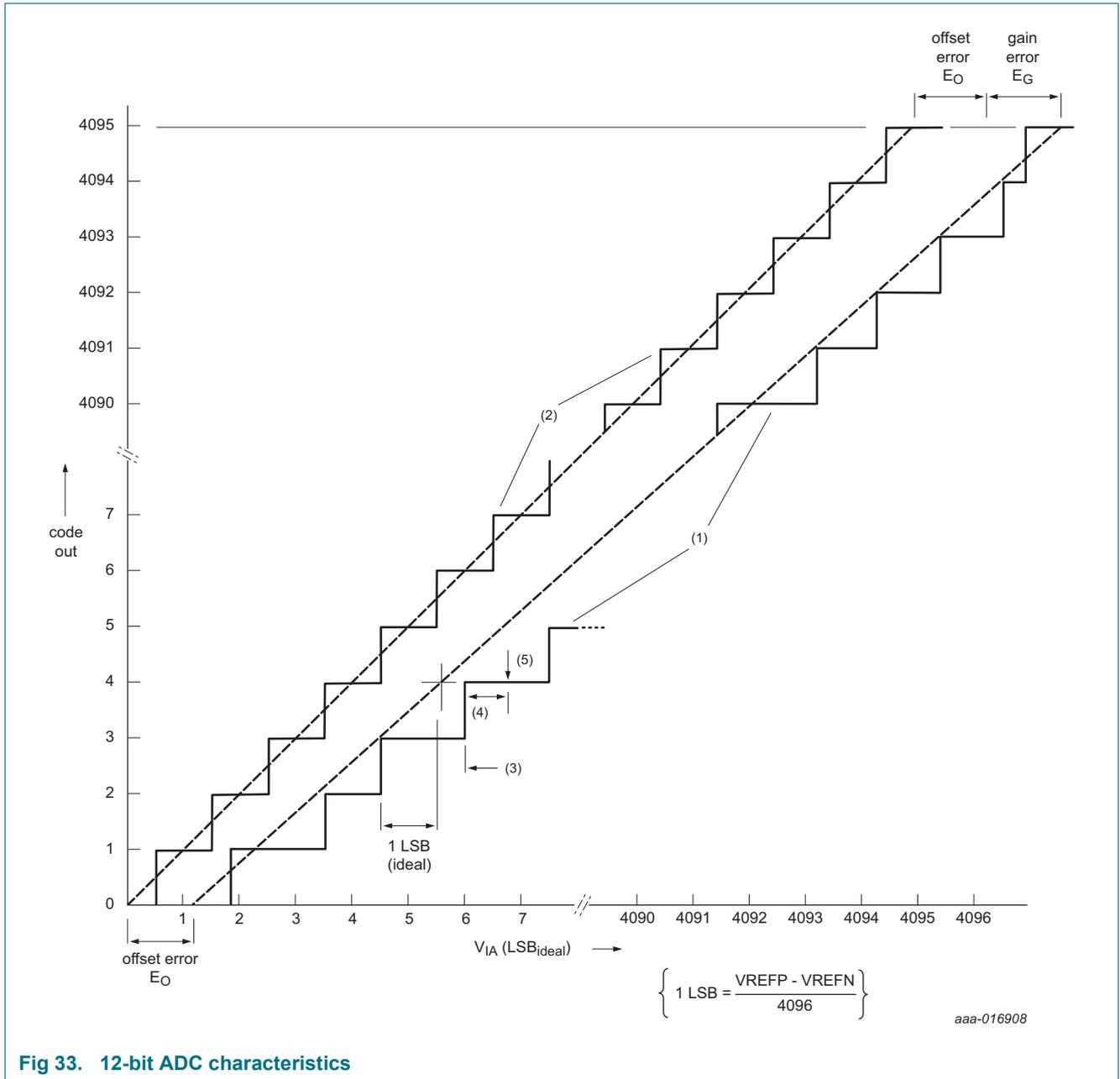
Fig 33. 12-bit ADC characteristics
