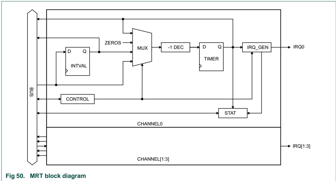
Fig 50. MRT block diagram
