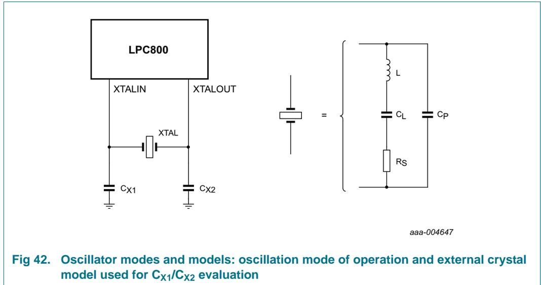
Fig 42. Oscillator modes and models: oscillation mode of operation and external crystal model used for  $C_{X1}/C_{X2}$  evaluation
