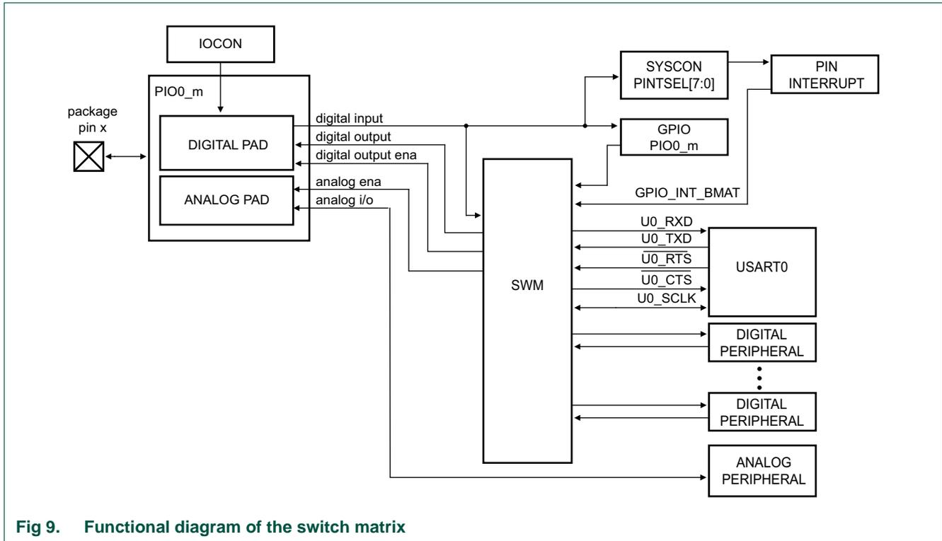
Fig 9. Functional diagram of the switch matrix
