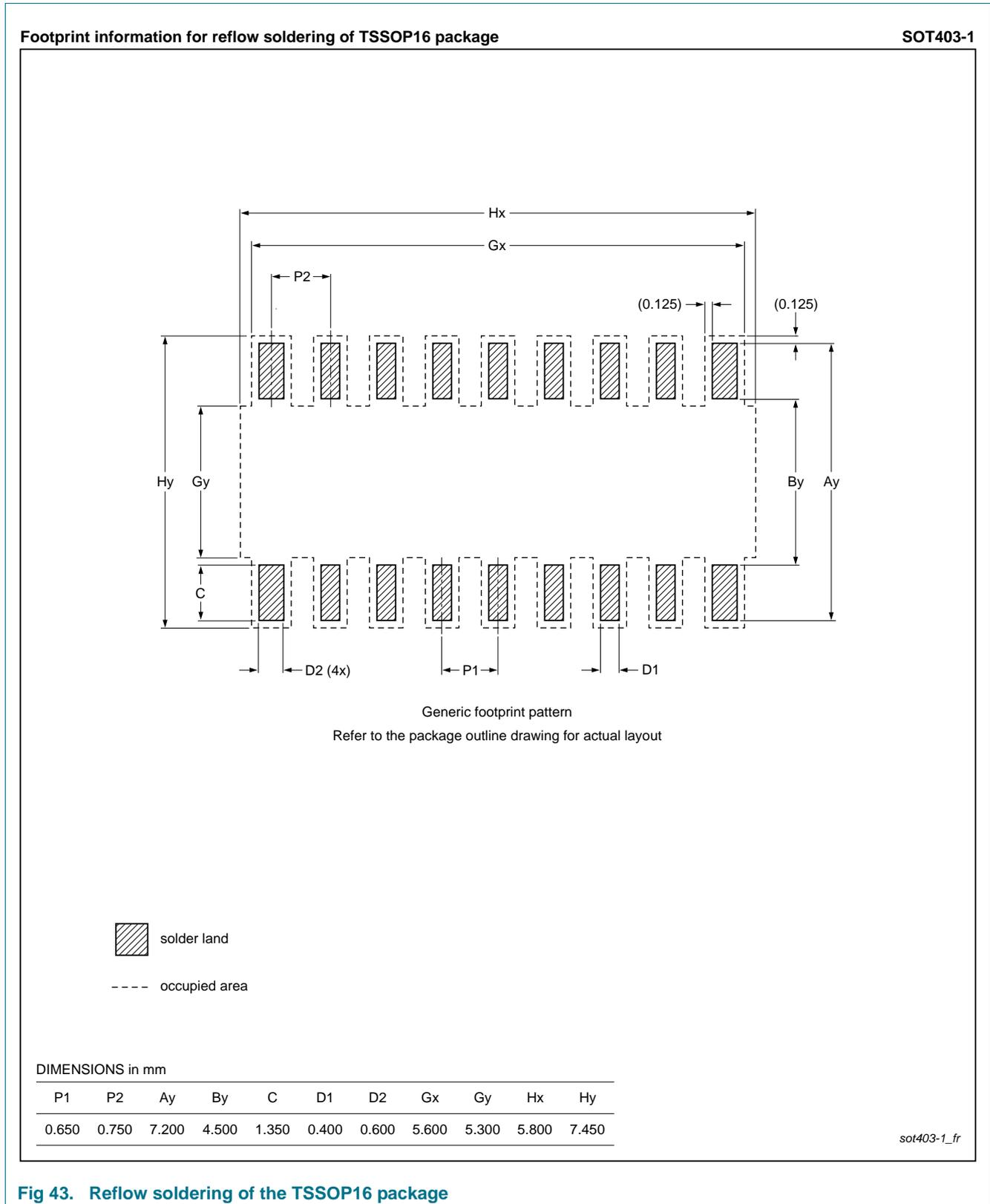
Fig 43. Reflow soldering of the TSSOP16 package
