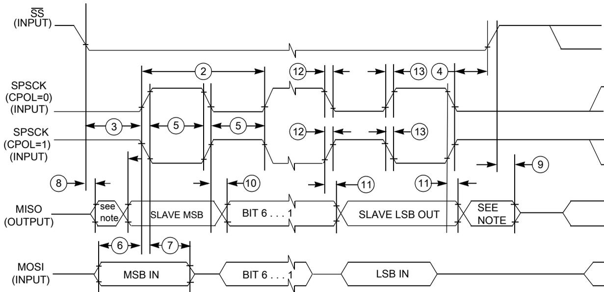
Figure 20. LPSPI slave mode timing (CPHA = 0)
