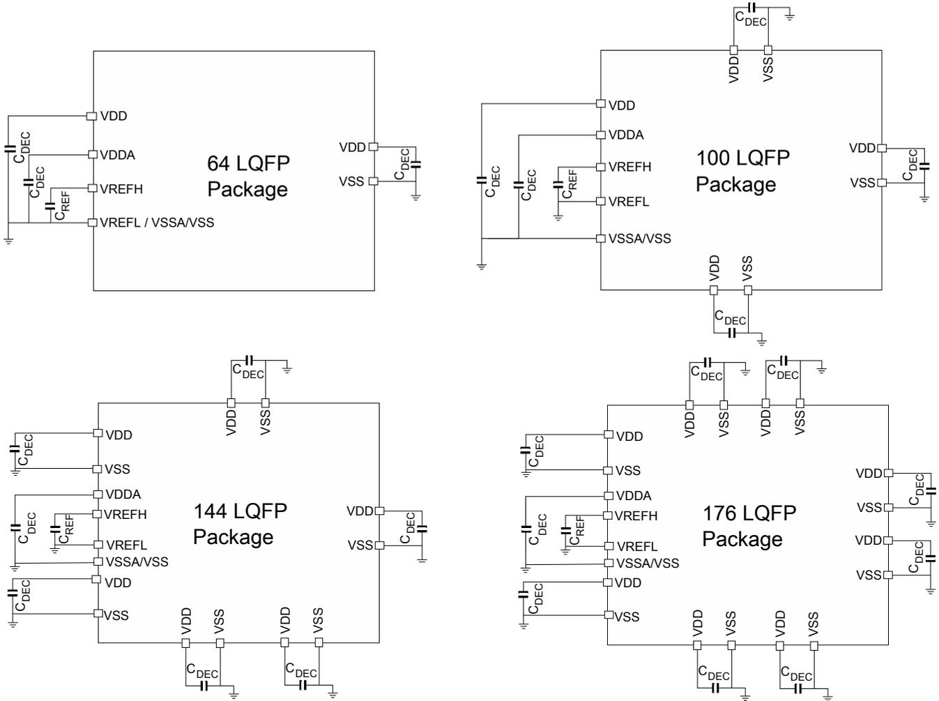
Figure 5. Pinout decoupling
