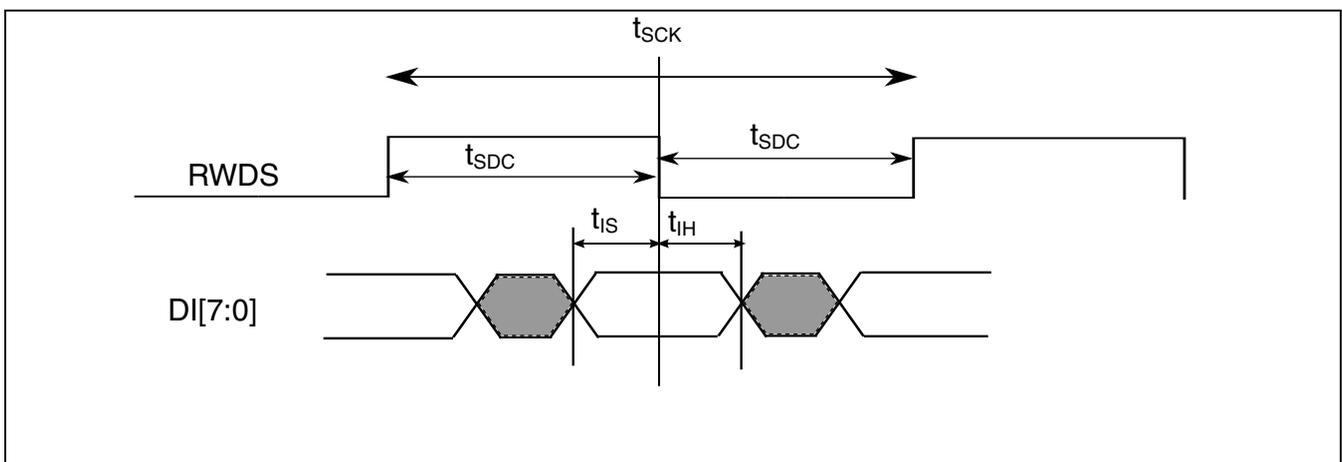
Figure 11. QuadSPI input timing (HyperRAM mode) diagram
