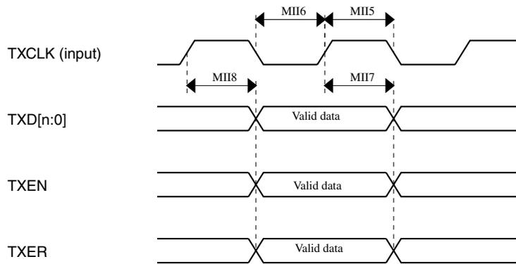
Figure 25. MII transmit signal diagram
