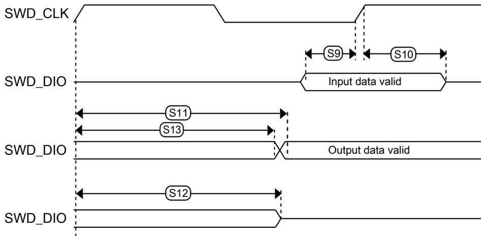
Figure 30. Serial wire data timing
