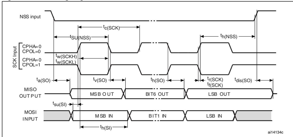
Figure 27. SPI timing diagram - slave mode and CPHA = 1<sup>(1)</sup>
