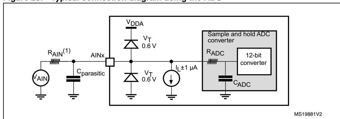
1. Refer to [Table 49: ADC characteristics](#) for the values of  $R_{\text{AIN}}$ ,  $R_{\text{ADC}}$  and  $C_{\text{ADC}}$ .
