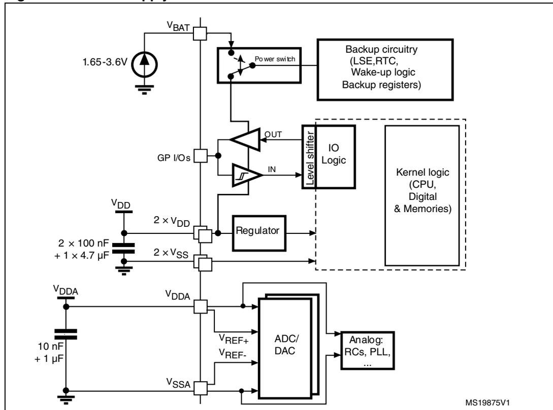
**Caution:** Each power supply pair ( $V_{DD}/V_{SS}$ ,  $V_{DDA}/V_{SSA}$  etc..) must be decoupled with filtering ceramic capacitors as shown above. These capacitors must be placed as close as possible to, or below, the appropriate pins on the underside of the PCB to ensure the good functionality of the device.
