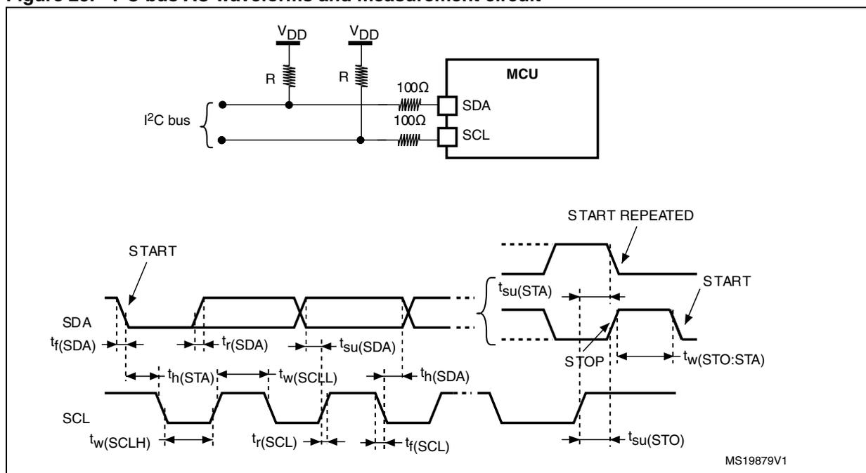
1. Measurement points are done at CMOS levels: 0.3  $V_{DD}$  and 0.7  $V_{DD}$ .
