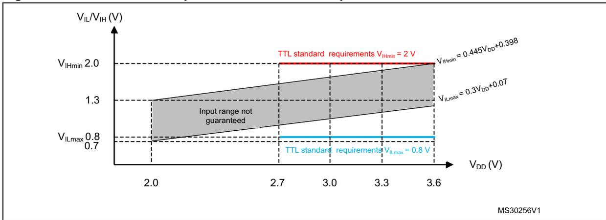
Figure 18. Five volt tolerant (FT and FTf) I/O input characteristics - CMOS port
