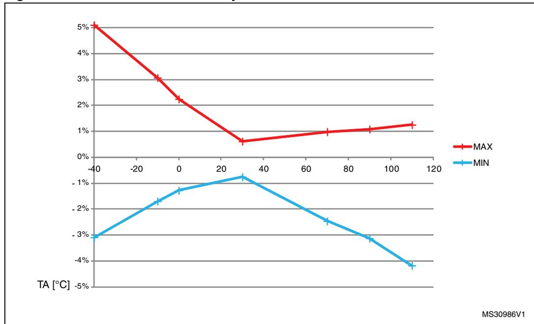
**Low-speed internal (LSI) RC oscillator**
