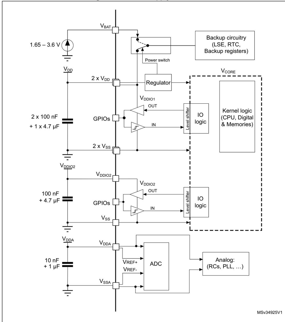
**Caution:** Each power supply pair (V<sub>DD</sub>/V<sub>SS</sub>, V<sub>DDA</sub>/V<sub>SSA</sub> etc.) must be decoupled with filtering ceramic capacitors as shown above. These capacitors must be placed as close as possible to, or below, the appropriate pins on the underside of the PCB to ensure the good functionality of the device.
