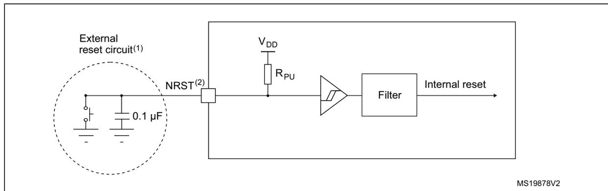
1. The external capacitor protects the device against parasitic resets.
