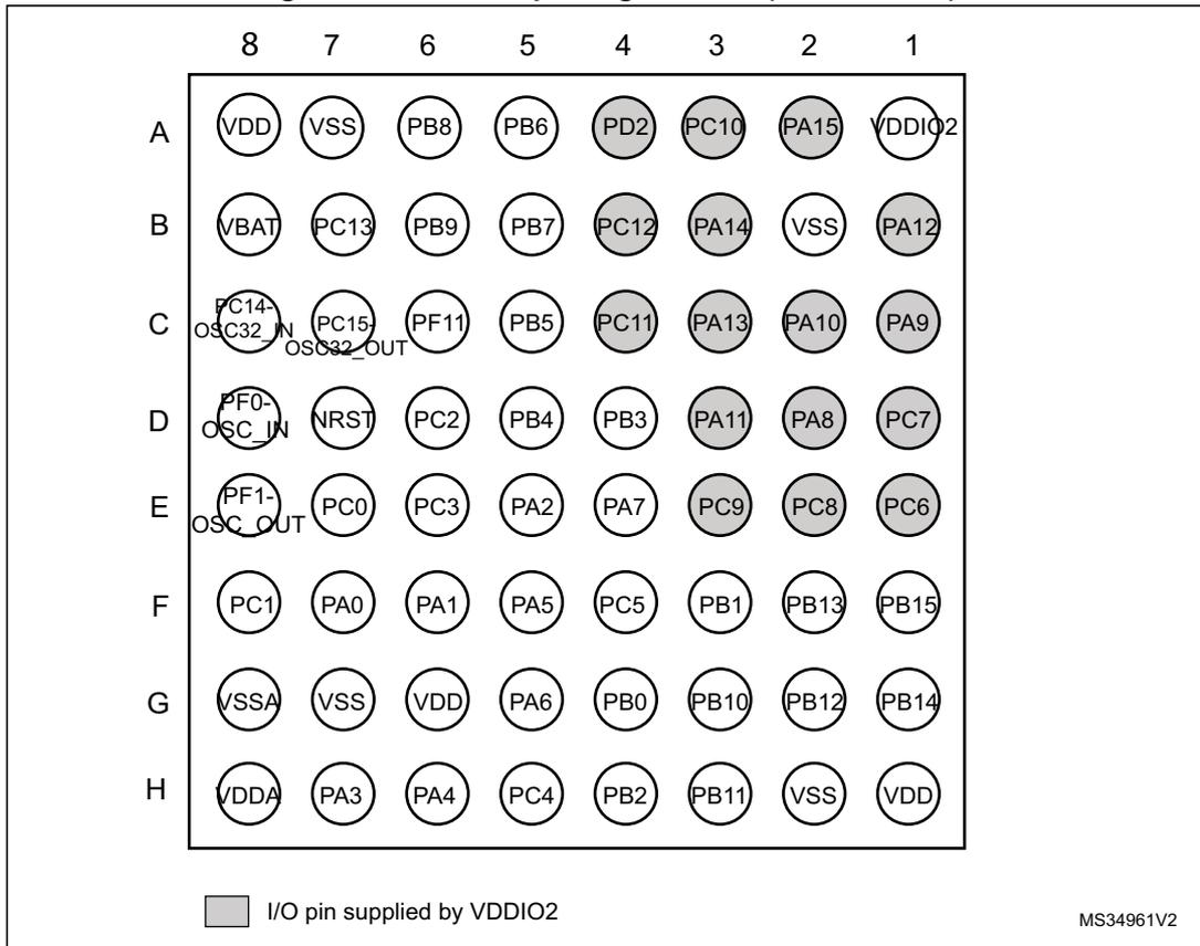
Figure 8. LQFP48 48-pin package pinout (top view)
