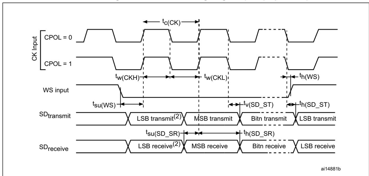
1. Measurement points are done at CMOS levels:  $0.3 \times V_{DDIOx}$  and  $0.7 \times V_{DDIOx}$ .
