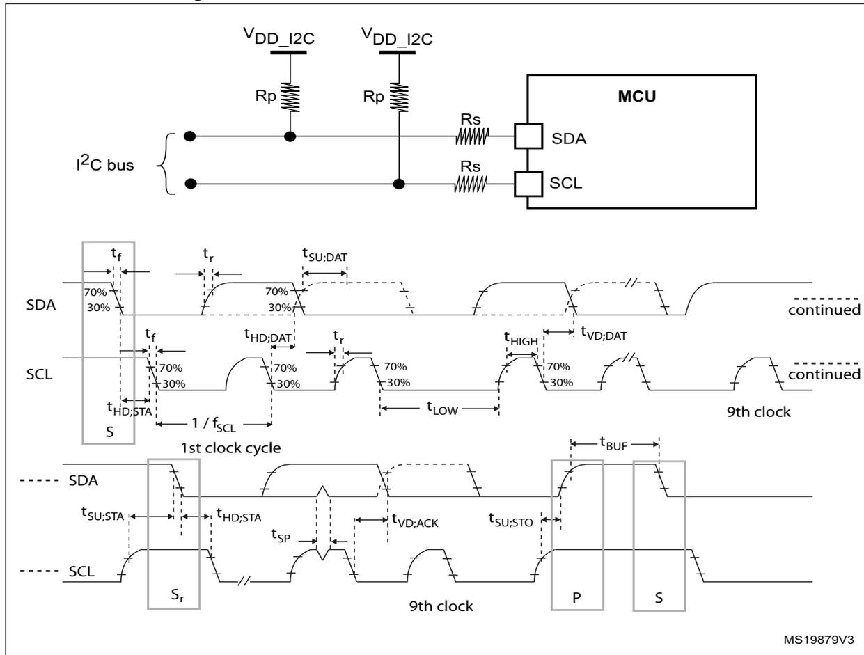
Legend: Rs: Series protection resistors. Rp: Pull-up resistors. V<sub>DD\_I2C</sub>: I<sup>2</sup>C bus supply.
