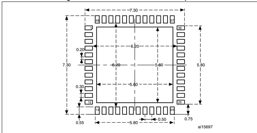
1. Dimensions are in millimeters.
