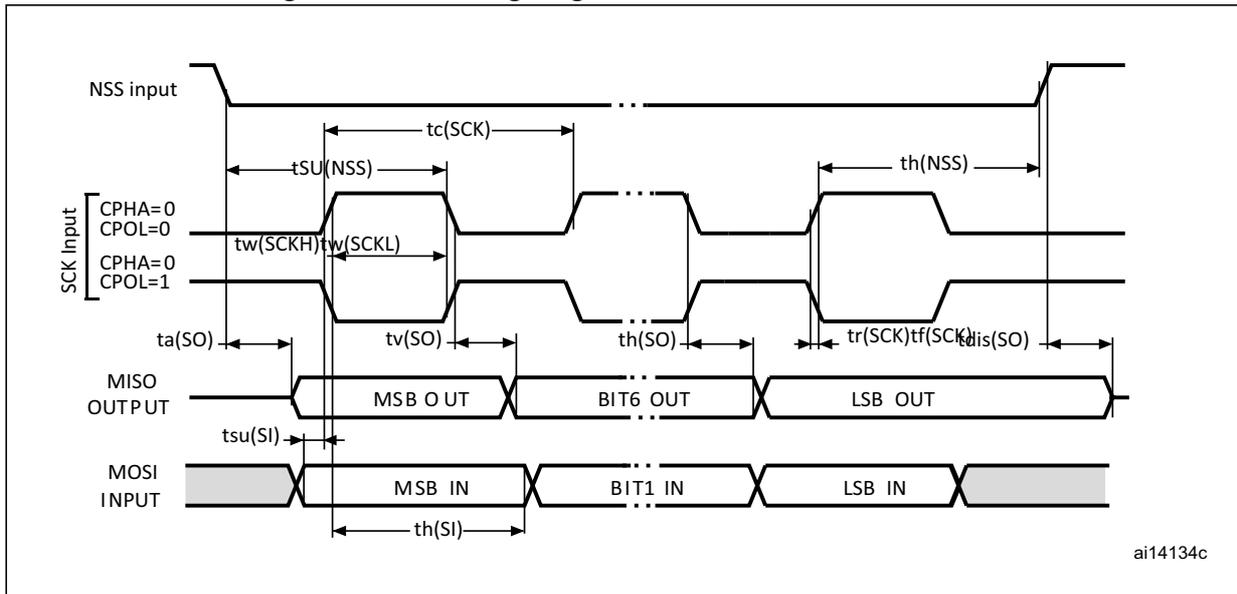
Figure 29. SPI timing diagram - slave mode and CPHA = 1
