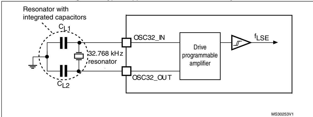
Note: An external resistor is not required between OSC32\_IN and OSC32\_OUT and it is forbidden to add one.
