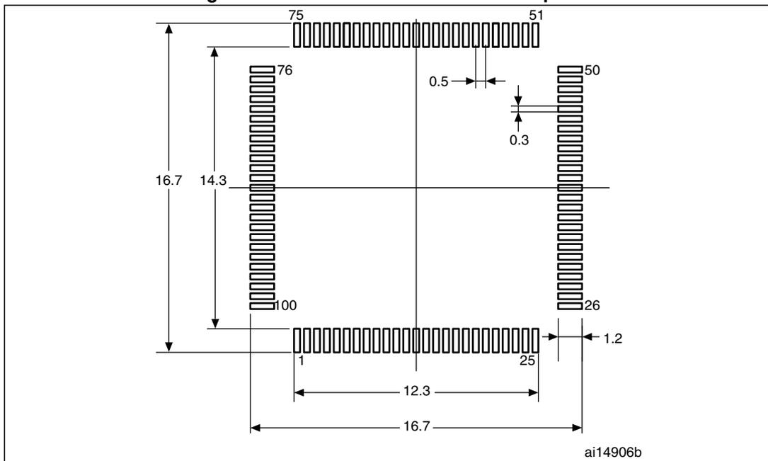
1. Dimensions are in millimeters.
