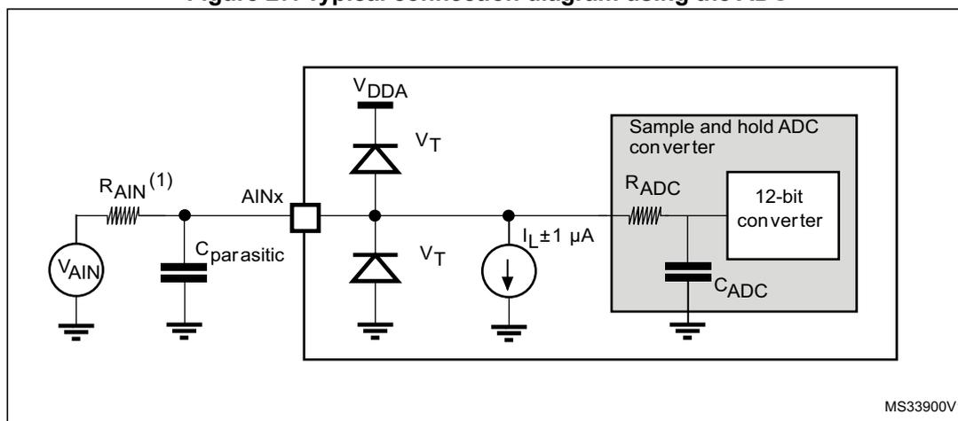
1. Refer to [Table 54: ADC characteristics](#) for the values of  $R_{AIN}$ ,  $R_{ADC}$  and  $C_{ADC}$ .
