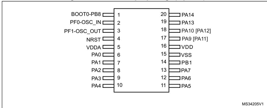
1. Pin pair PA11/12 can be remapped instead of pin pair PA9/10 using the SYSCFG\_CFGR1 register.
