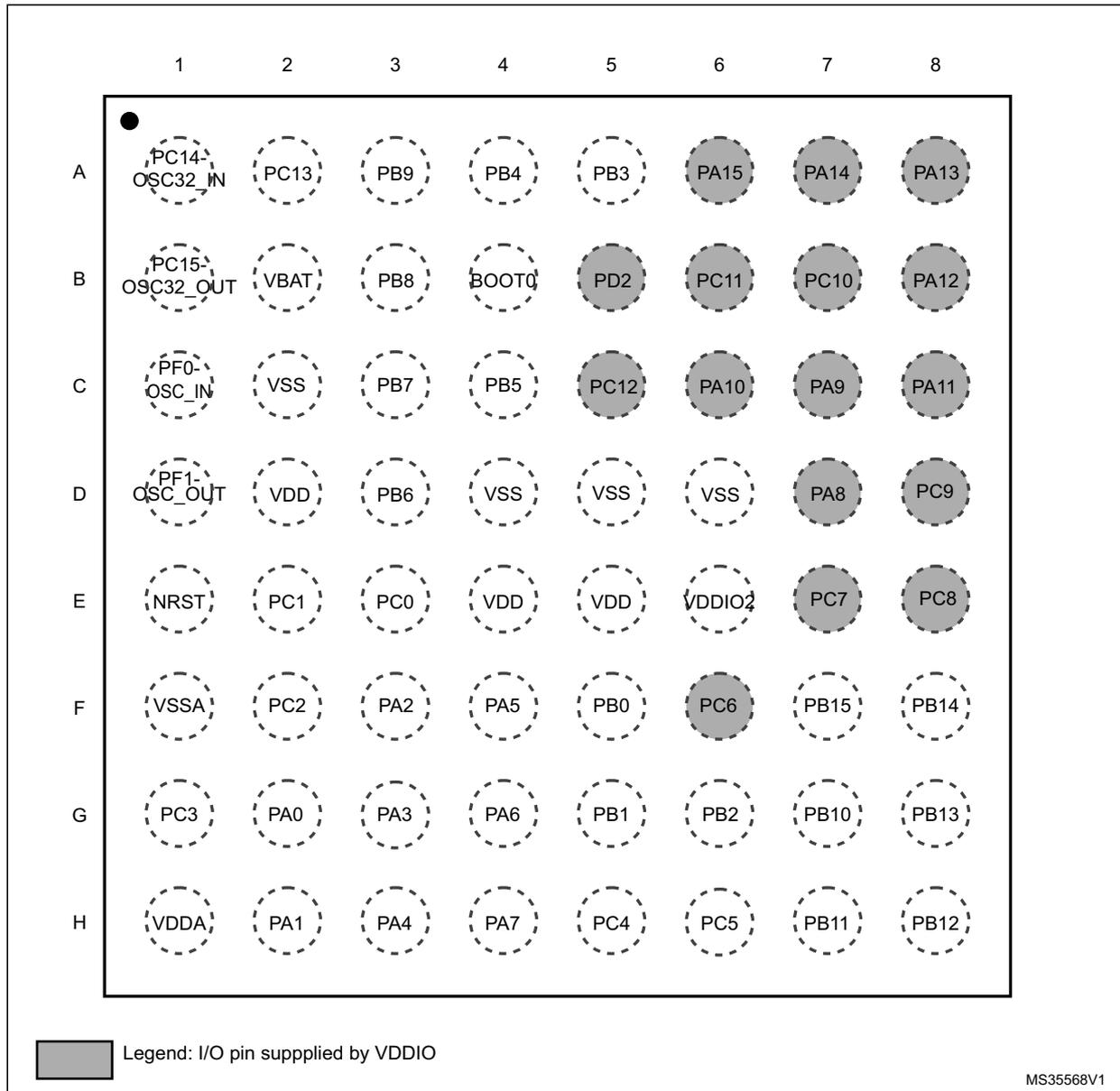
Figure 6. LQFP64 64-pin package pinout (top view)
