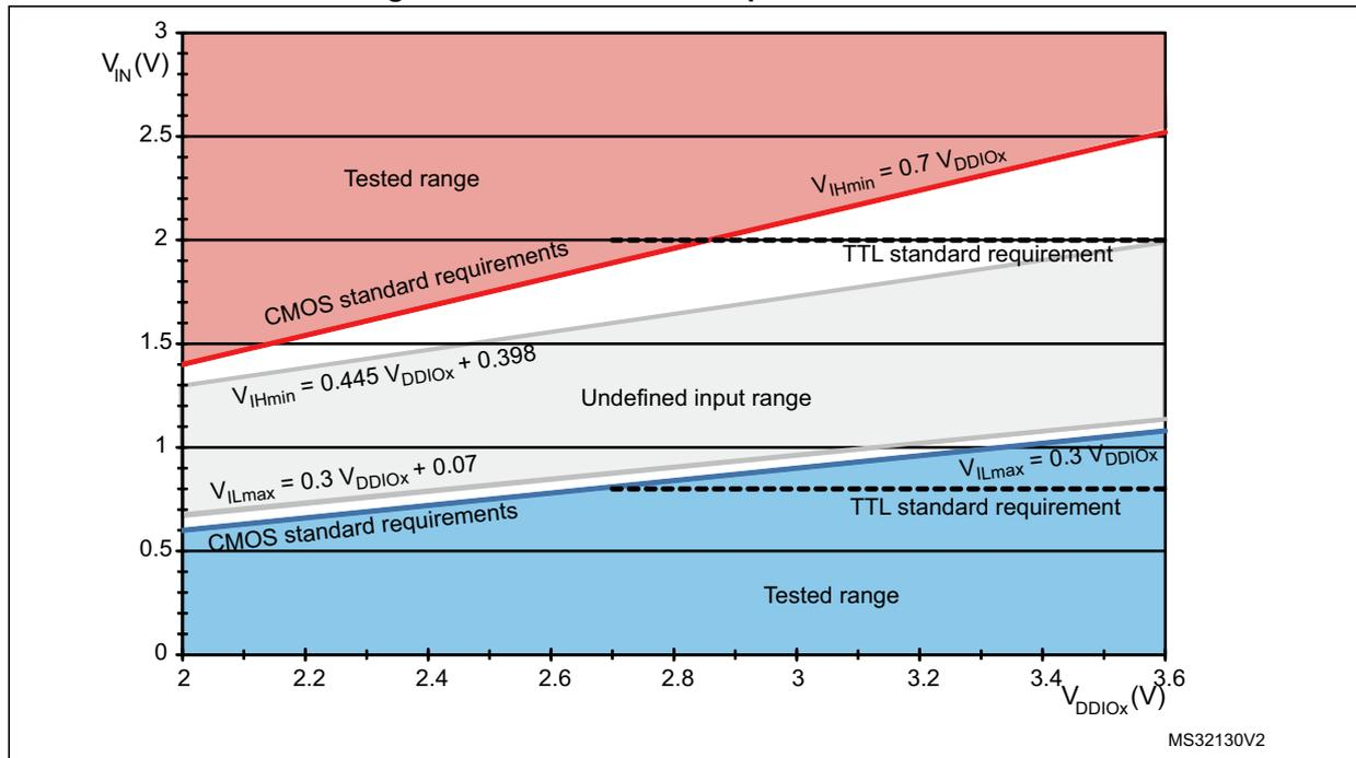
**Figure 22. Five volt tolerant (FT and FTf) I/O input characteristics**
