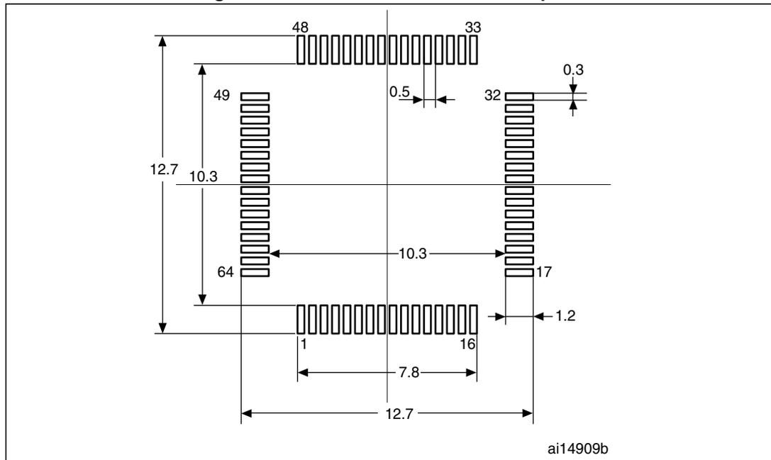
1. Dimensions are in millimeters.
