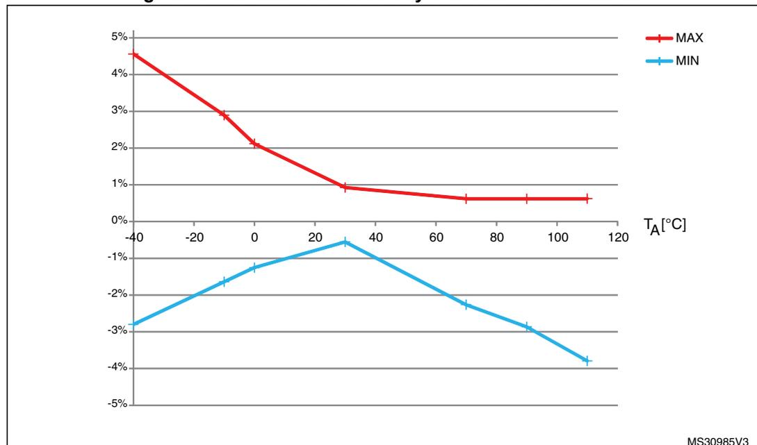
High-speed internal 14 MHz (HSI14) RC oscillator (dedicated to ADC)
