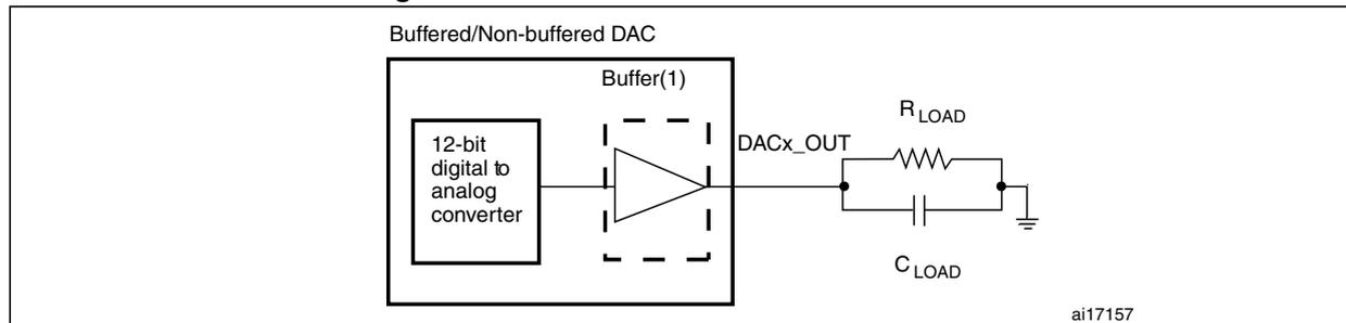
1. The DAC integrates an output buffer that can be used to reduce the output impedance and to drive external loads directly without the use of an external operational amplifier. The buffer can be bypassed by configuring the BOFFx bit in the DAC\_CR register.
