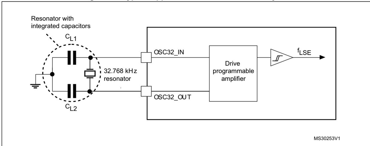
Note: An external resistor is not required between OSC32\_IN and OSC32\_OUT and it is forbidden to add one.
