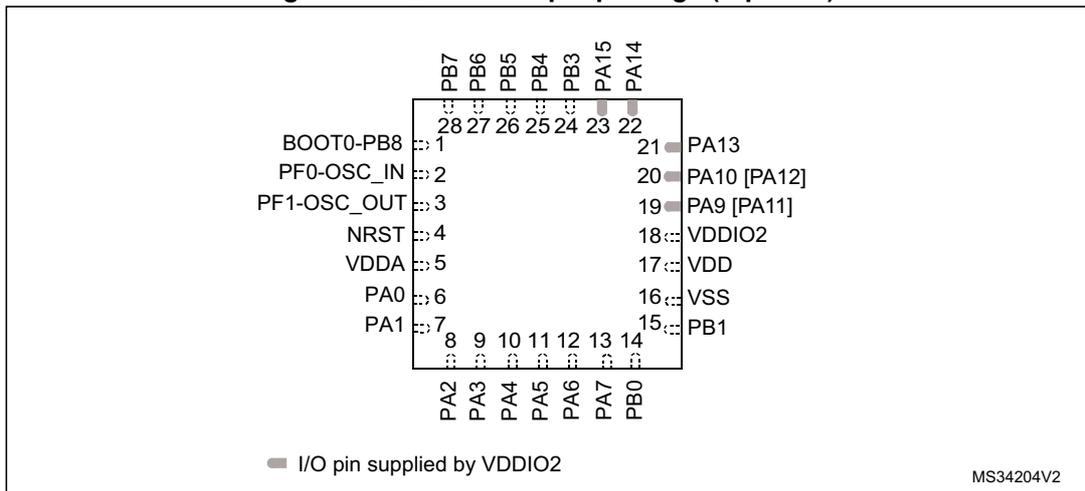
1. Pin pair PA11/12 can be remapped instead of pin pair PA9/10 using the SYSCFG\_CFGR1 register.
