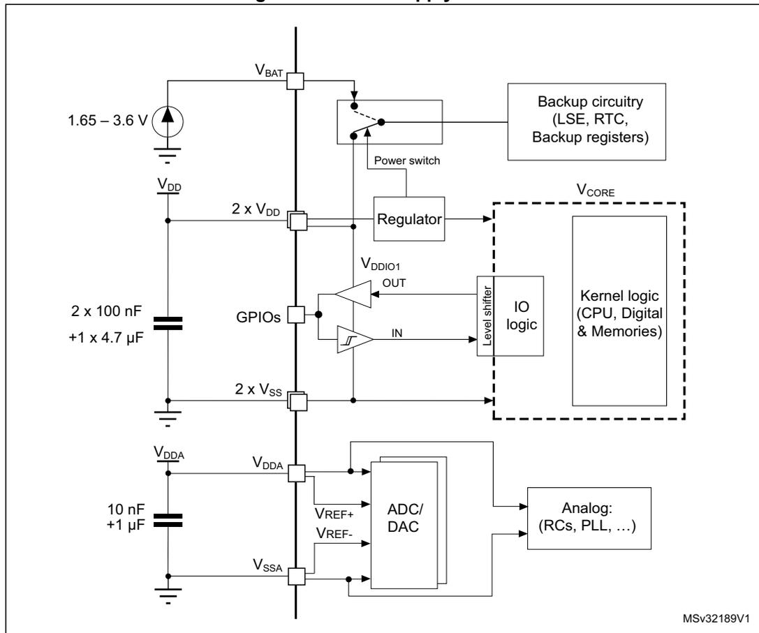
**Caution:** Each power supply pair (V<sub>DD</sub>/V<sub>SS</sub>, V<sub>DDA</sub>/V<sub>SSA</sub> etc.) must be decoupled with filtering ceramic capacitors as shown above. These capacitors must be placed as close as possible to, or below, the appropriate pins on the underside of the PCB to ensure the good functionality of the device.
