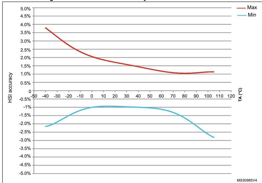
High-speed internal 14 MHz (HSI14) RC oscillator (dedicated to ADC)
