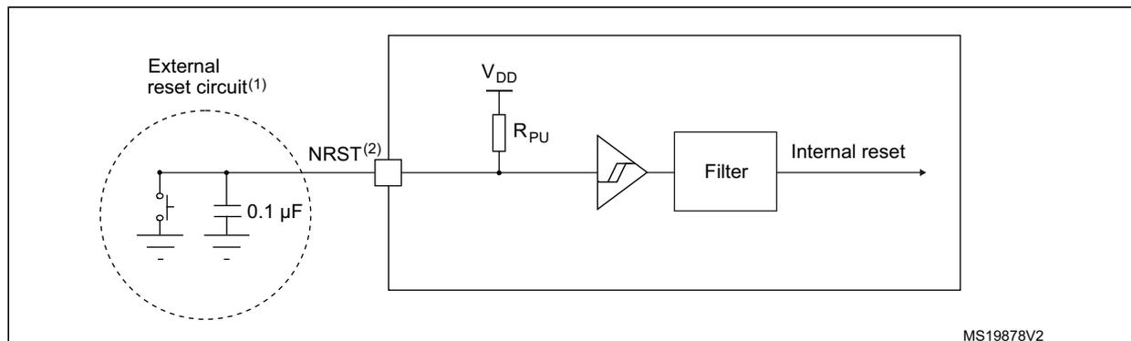
1. The external capacitor protects the device against parasitic resets.
