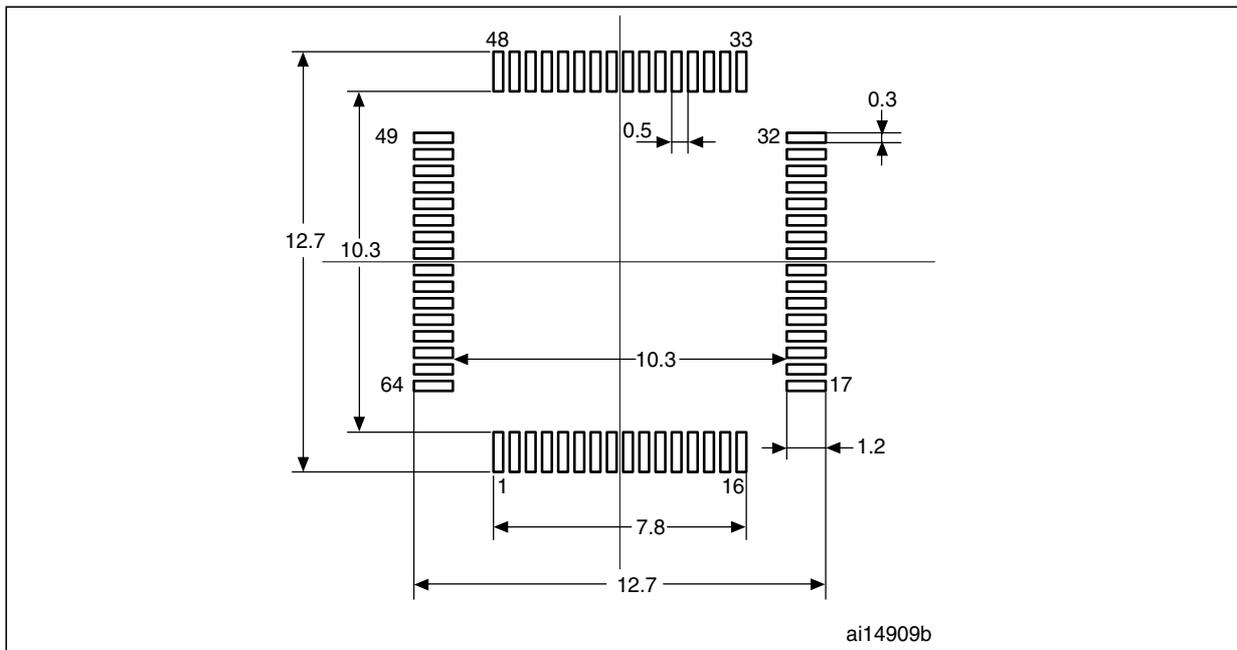
1. Dimensions are in millimeters.
