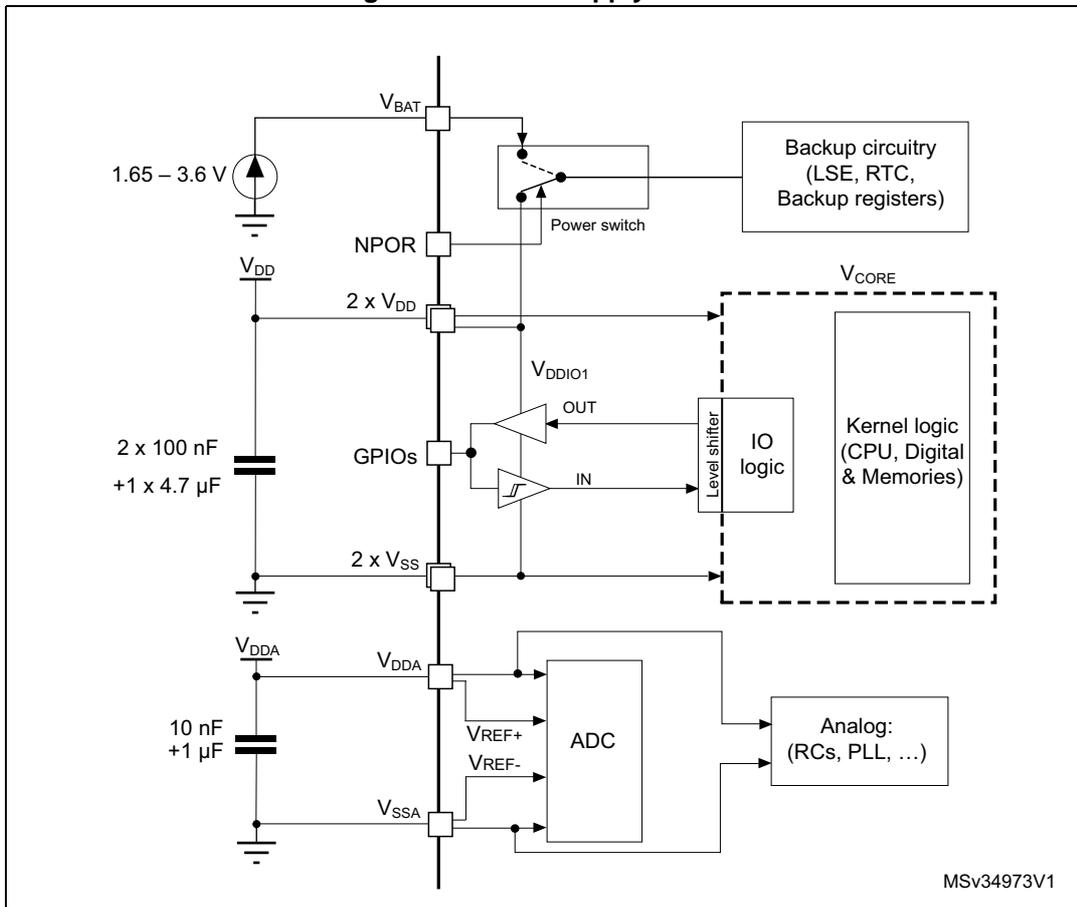
**Caution:** Each power supply pair ( $V_{DD}/V_{SS}$ ,  $V_{DDA}/V_{SSA}$  etc.) must be decoupled with filtering ceramic capacitors as shown above. These capacitors must be placed as close as possible to, or below, the appropriate pins on the underside of the PCB to ensure the good functionality of the device.
