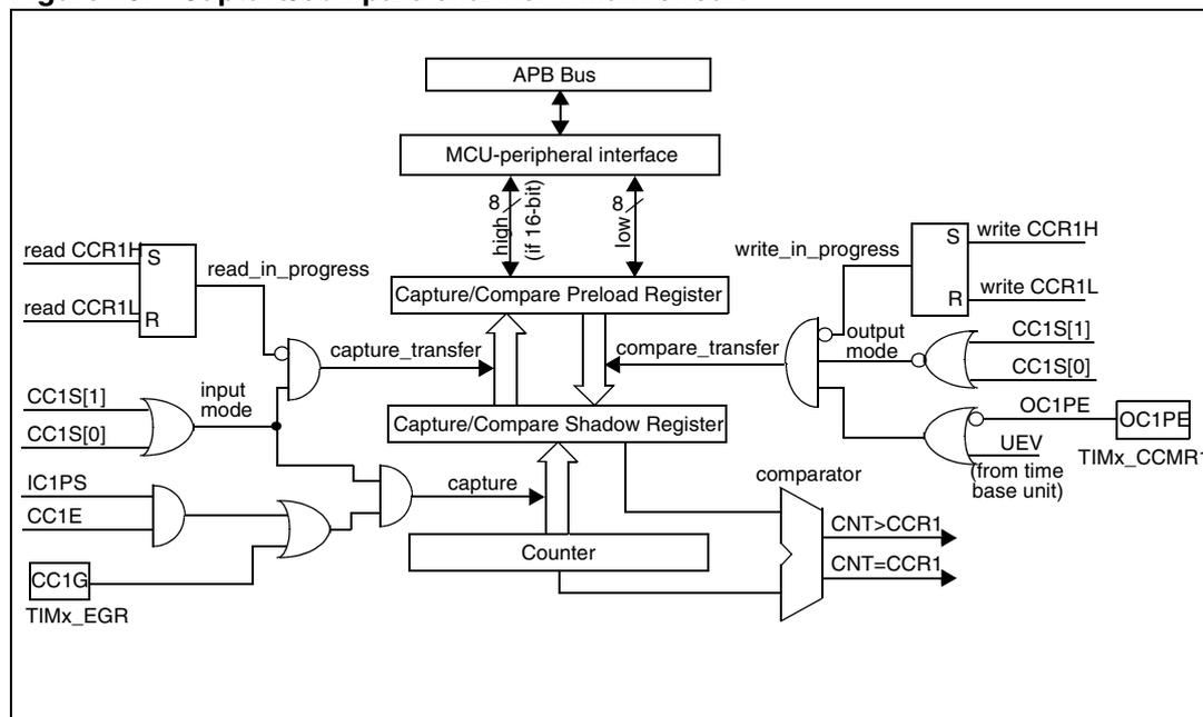
**Figure 80. Output stage of capture/compare channel (channel 1)**
