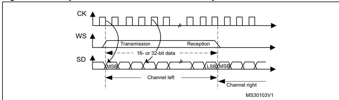
**Figure 244. LSB justified 24-bit frame length with CPOL = 0**
