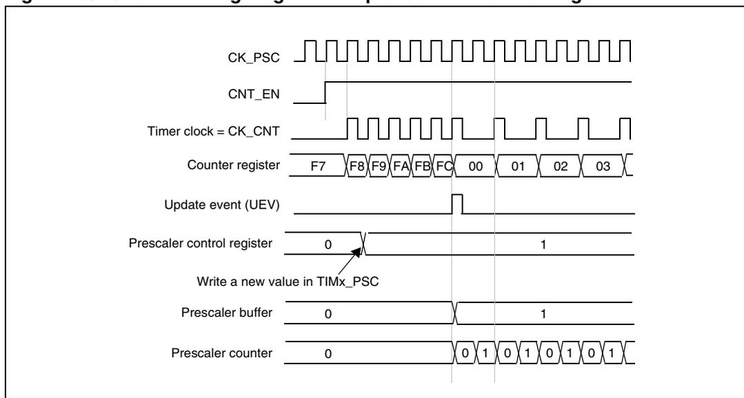
Figure 154. Counter timing diagram with prescaler division change from 1 to 4
