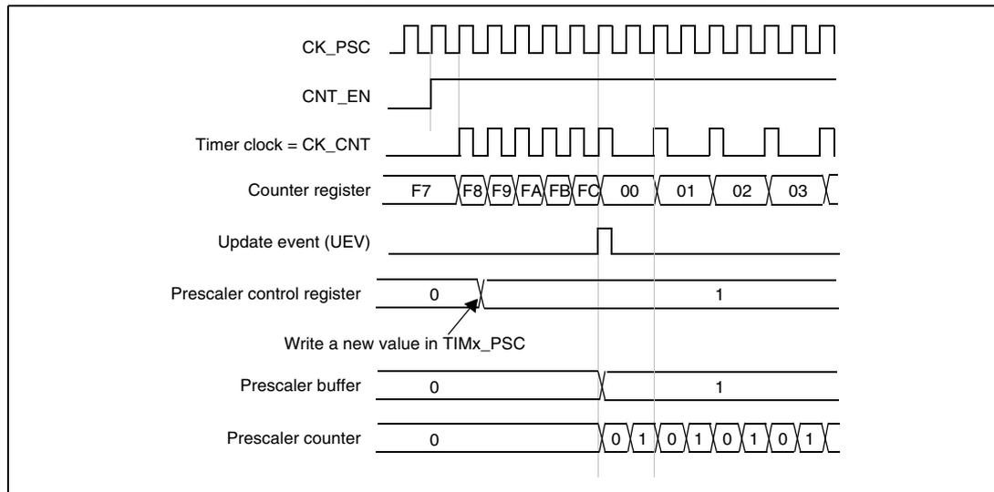
Figure 55. Counter timing diagram with prescaler division change from 1 to 4
