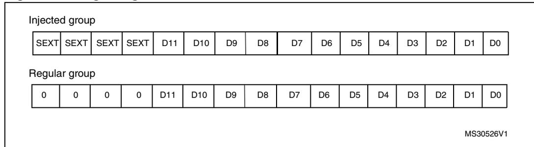
**Figure 31. Left alignment of data**
