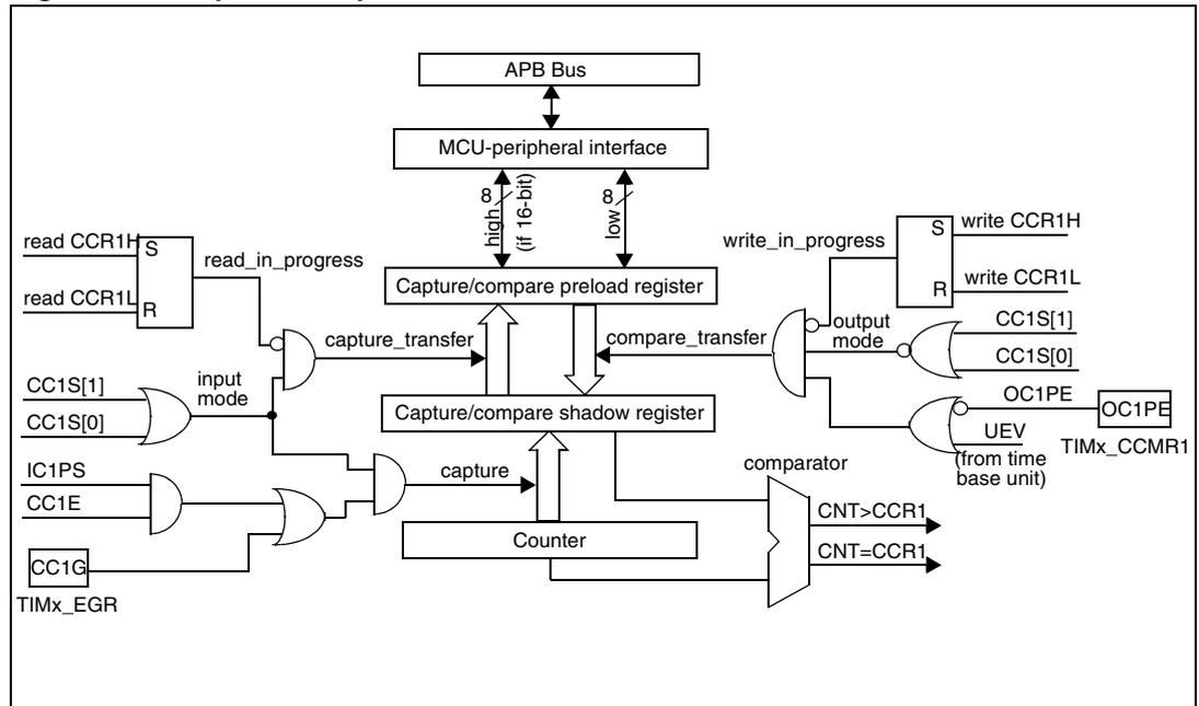
Figure 138. Output stage of capture/compare channel (channel 1)
