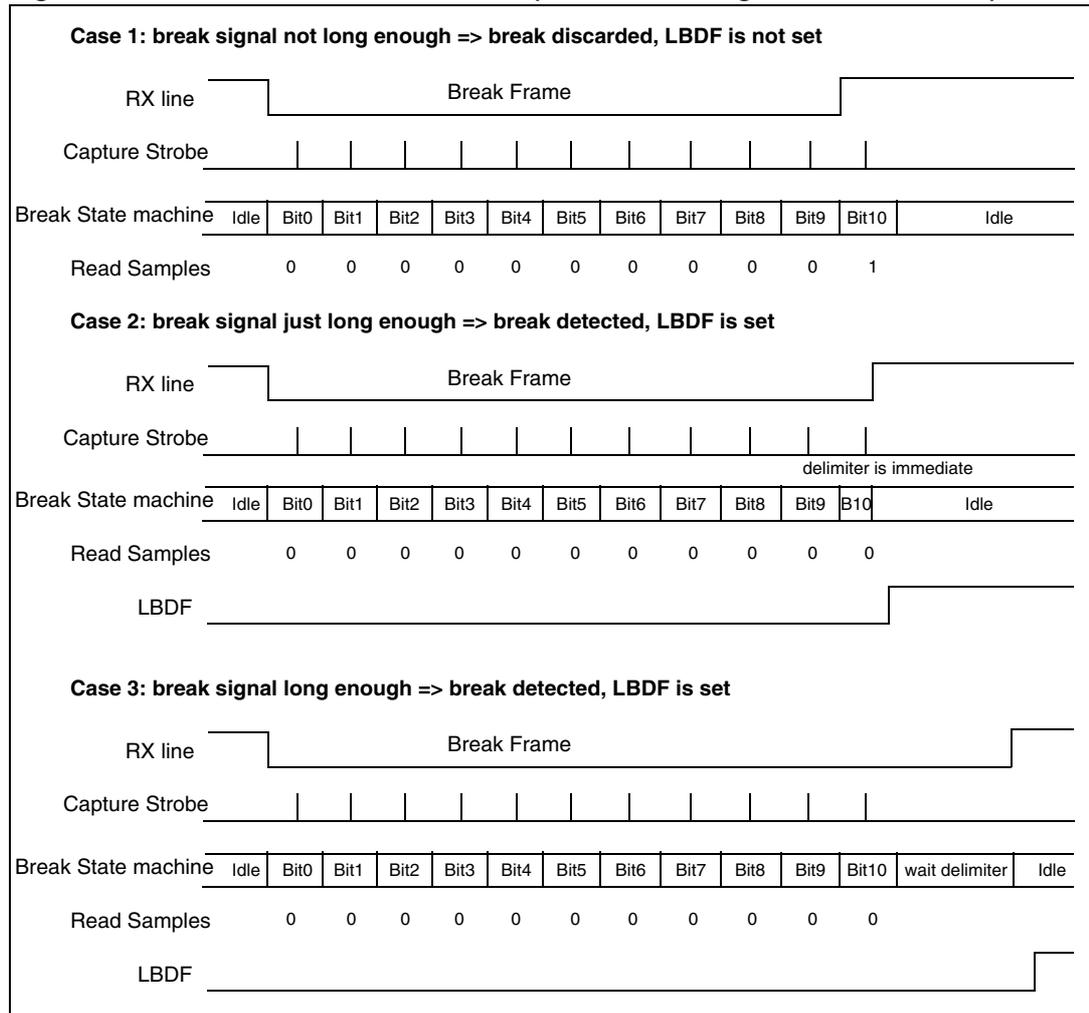
Figure 207. Break detection in LIN mode vs. Framing error detection
