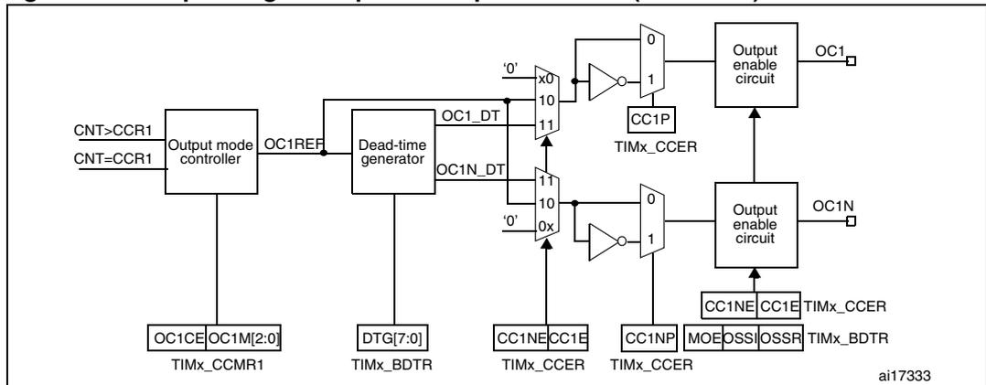
Figure 139. Output stage of capture/compare channel (channel 2 for TIM15)
