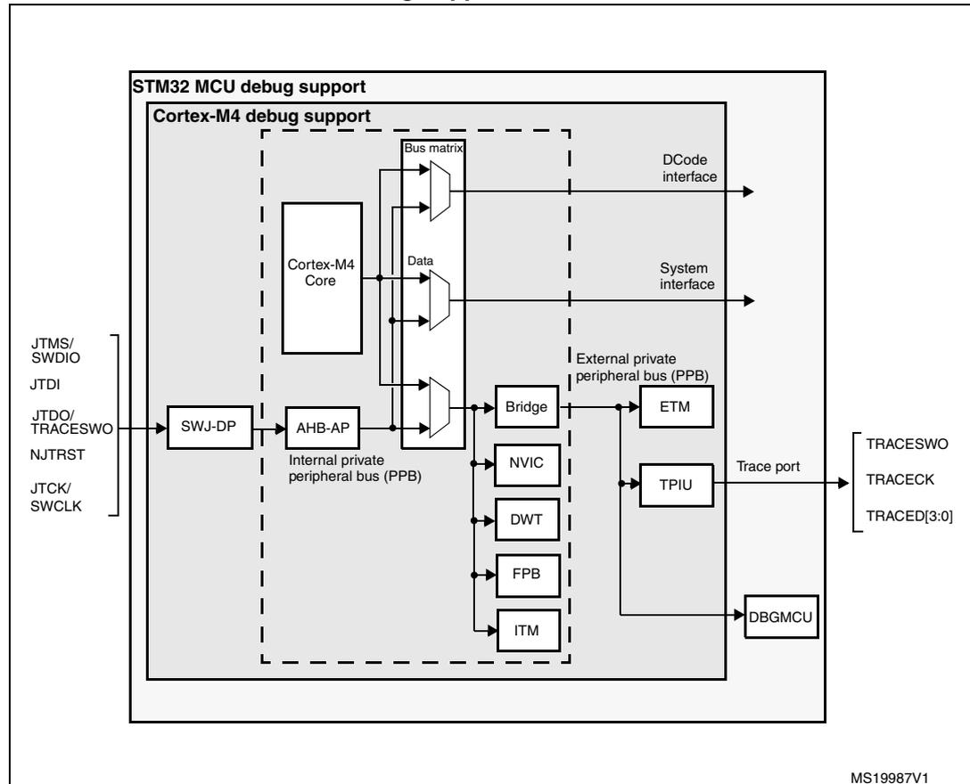
1. The debug features embedded in the Cortex-M4F core are a subset of the ARM CoreSight Design Kit.
