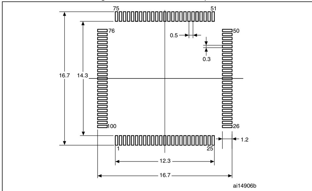
1. Dimensions are in millimeters.
