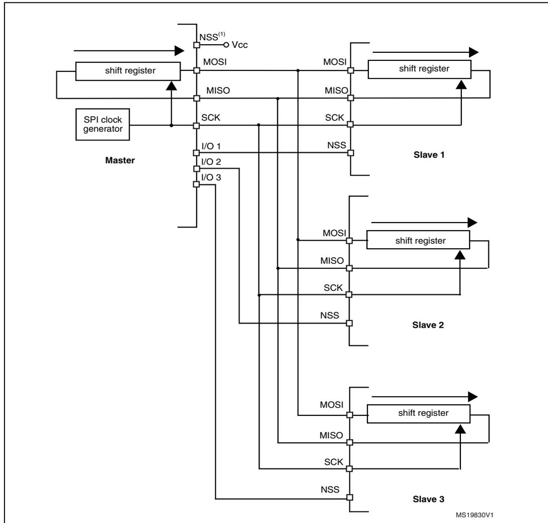
1. As MISO pins of the slaves are connected together, all slaves must have the GPIO configuration of their MISO pin set as alternate function open-drain (see [Section 8.3.7: I/O alternate function input/output on page 135](#)).
