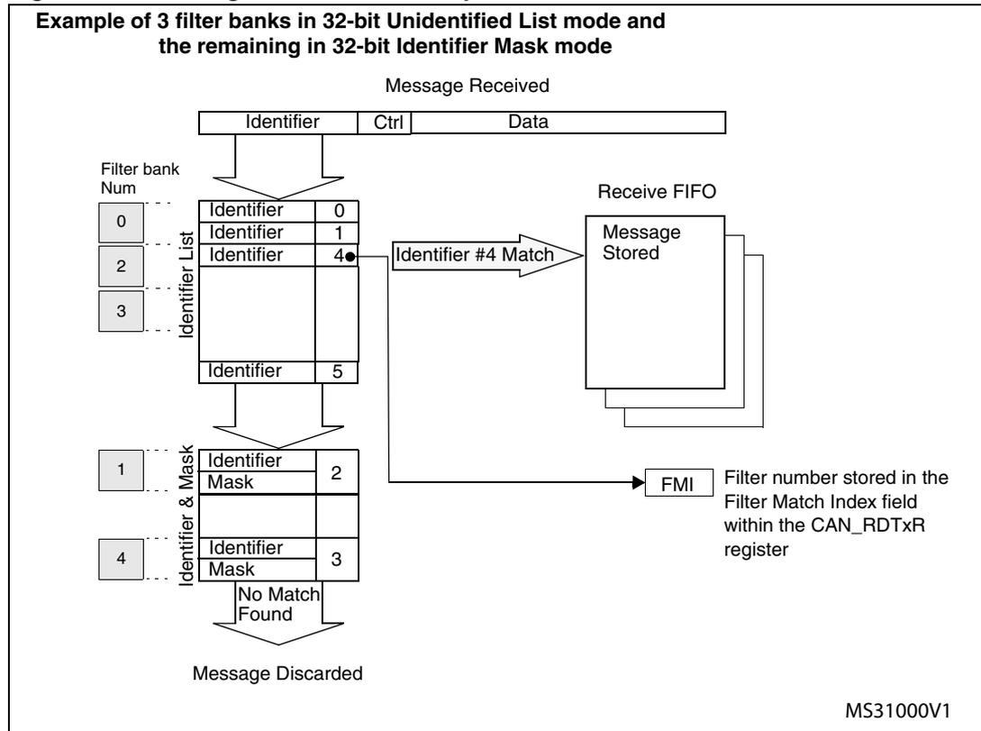
The example above shows the filtering principle of the bxCAN. On reception of a message, the identifier is compared first with the filters configured in identifier list mode. If there is a match, the message is stored in the associated FIFO and the index of the matching filter is stored in the Filter Match Index. As shown in the example, the identifier matches with Identifier #2 thus the message content and FMI 2 is stored in the FIFO.
