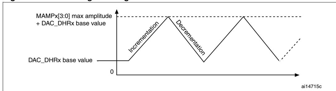
**Figure 50. DAC conversion (SW trigger enabled) with triangle wave generation**
