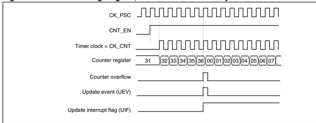
**Figure 104. Counter timing diagram, internal clock divided by 2**
