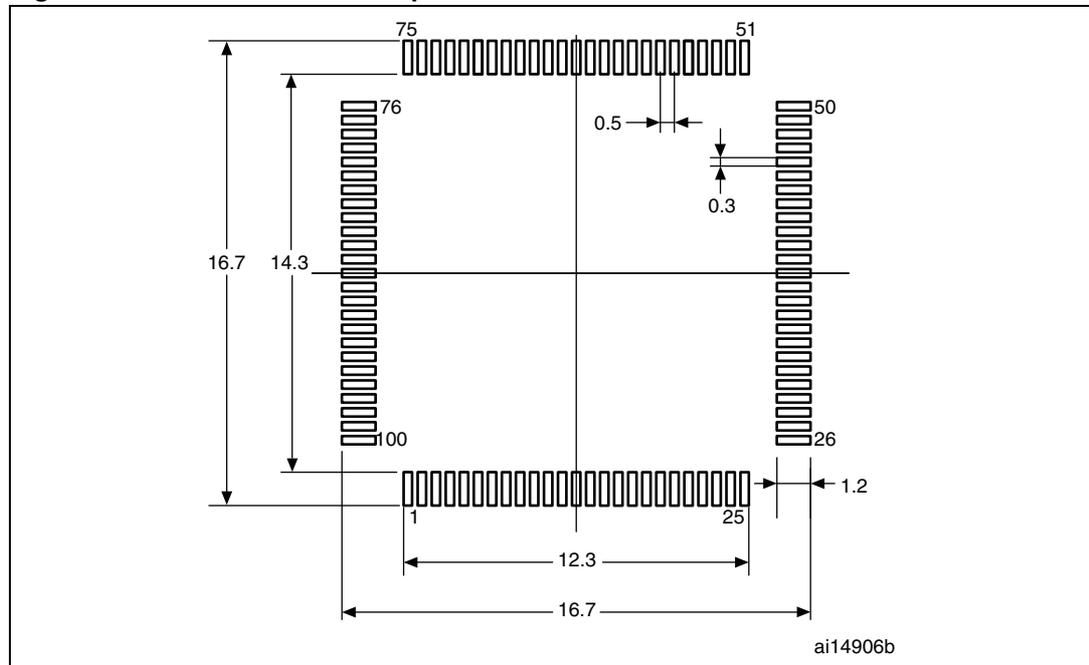
1. Dimensions are in millimeters.
