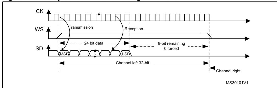
**Figure 242. MSB justified 16-bit extended to 32-bit packet frame with CPOL = 0**
