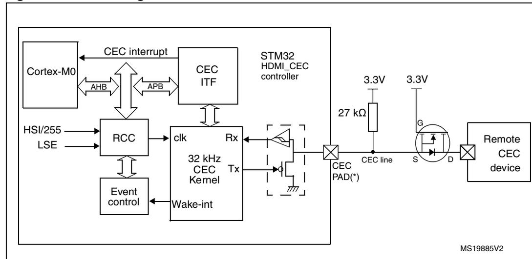
1. GPI/O configured as output open-drain alternate function
