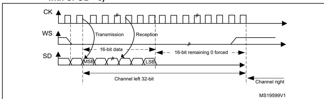
When 16-bit data frame extended to 32-bit channel frame is selected during the I<sup>2</sup>S configuration phase, only one access to the SPIx\_DR register is required. The 16 remaining bits are forced by hardware to 0x0000 to extend the data to 32-bit format.
