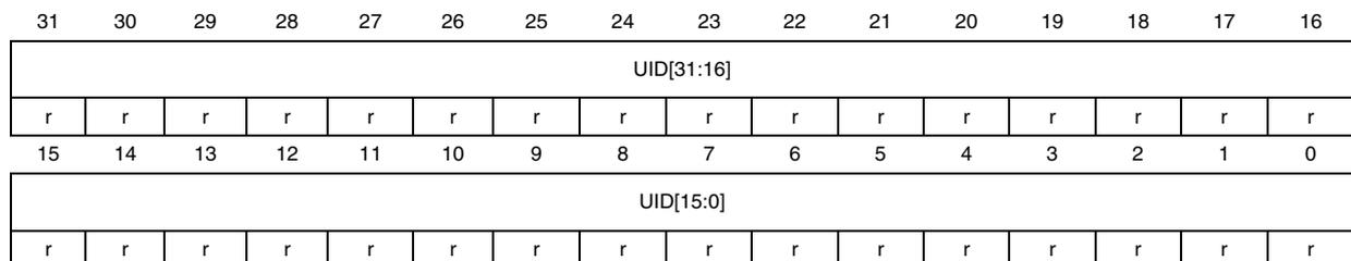
Bits 31:0 **UID[31:0]**: X and Y coordinates on the wafer expressed in BCD format
