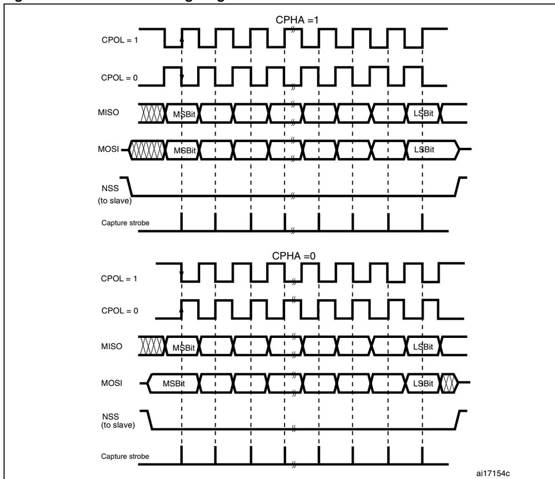
1. These timings are shown with the LSBFIRST bit reset in the SPIx\_CR1 register and 8-bit data size (bits DS[3:0]=0111).
