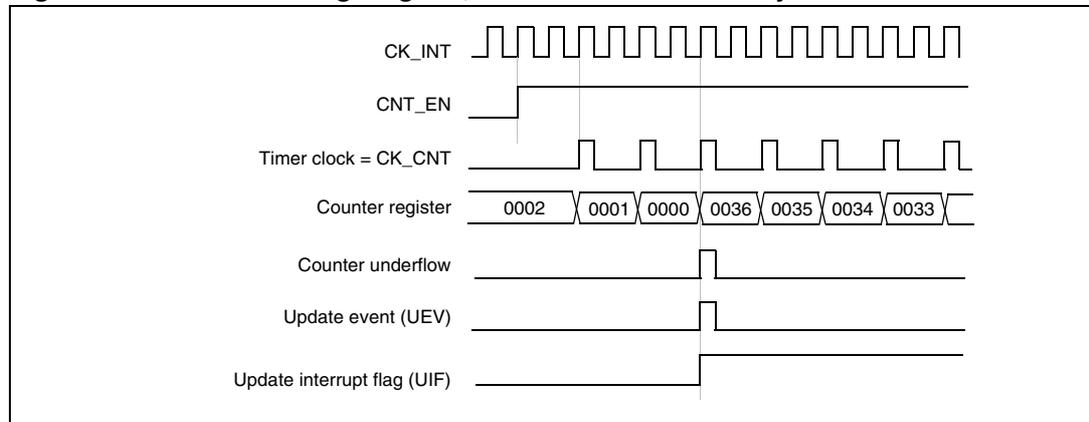
**Figure 64. Counter timing diagram, internal clock divided by 4**
