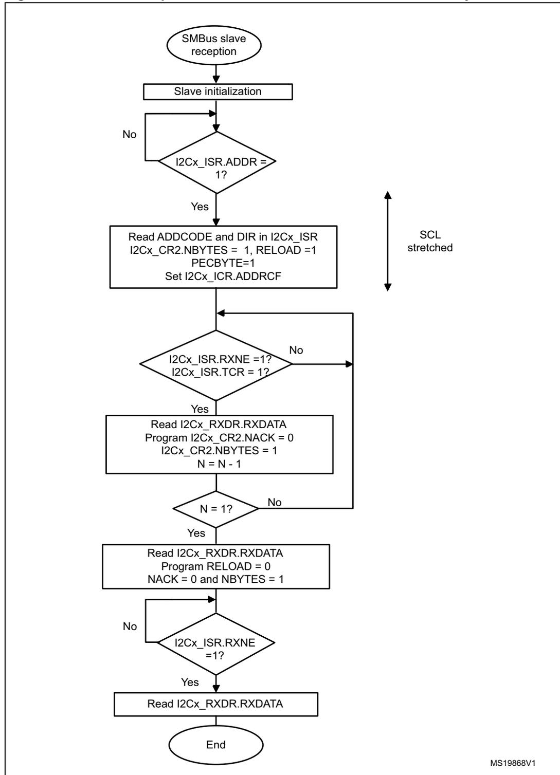
Figure 193. Bus transfer diagrams for SMBus slave receiver (SBC=1)
