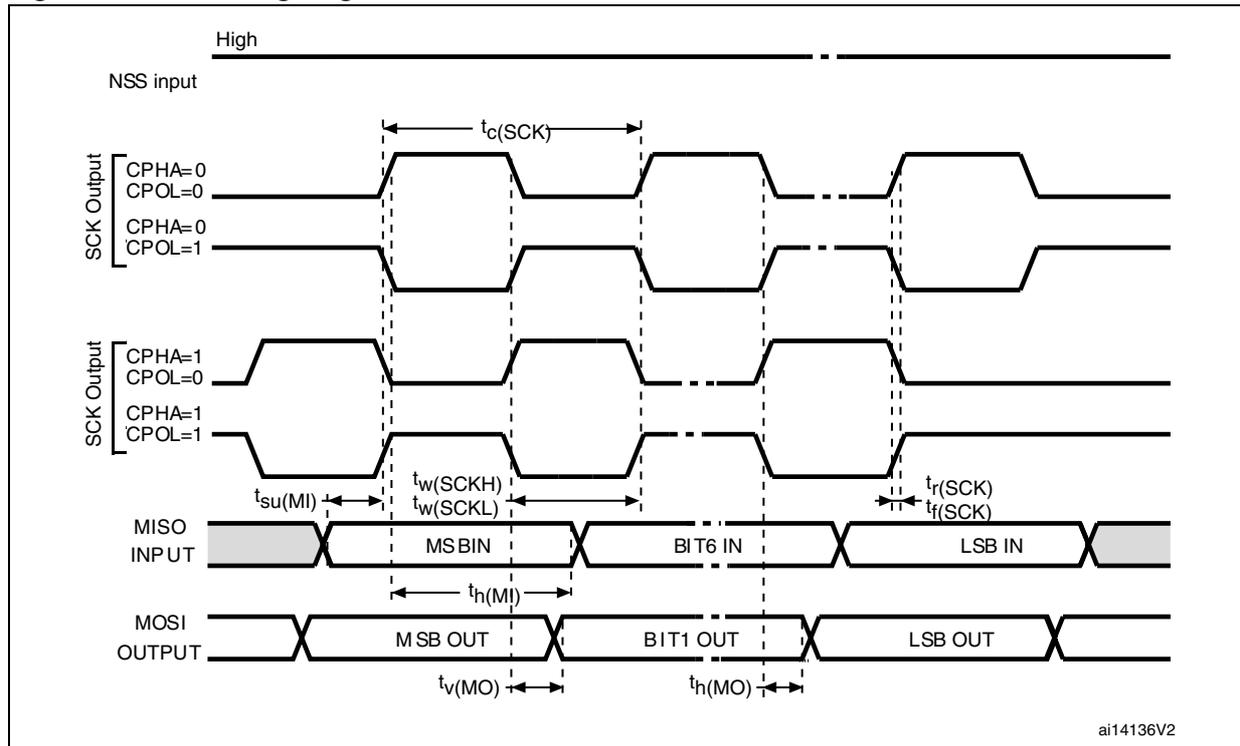
1. Measurement points are done at 0.5V<sub>DD</sub> and with external C<sub>L</sub> = 30 pF.
