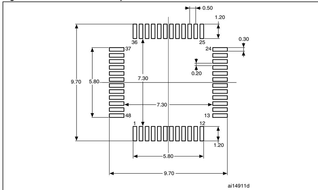
1. Dimensions are in millimeters.
