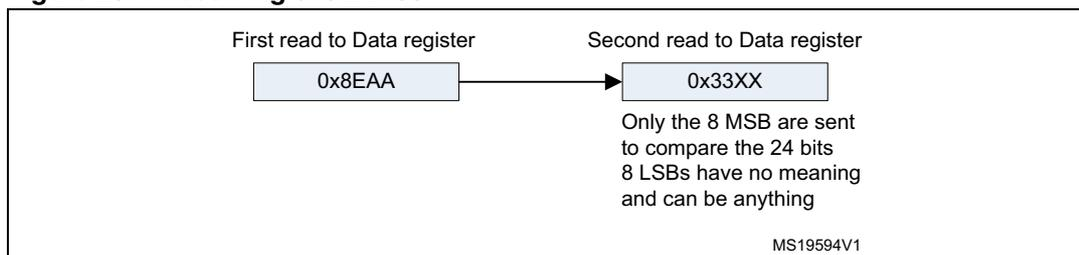
**Figure 238. I<sup>2</sup>S Philips standard (16-bit extended to 32-bit packet frame with CPOL = 0)**
