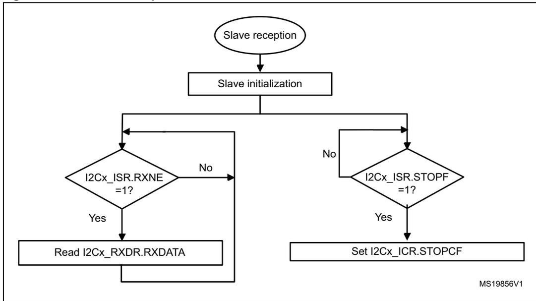
Figure 178. Transfer bus diagrams for I2C slave receiver
