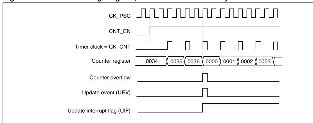
Figure 128. Counter timing diagram, internal clock divided by 4
