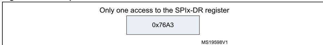
In transmission mode, when a TXE event occurs, the application has to write the data to be transmitted (in this case 0x76A3). The 0x000 field is transmitted first (extension on 32-bit). The TXE flag is set again as soon as the effective data (0x76A3) is sent on SD.
