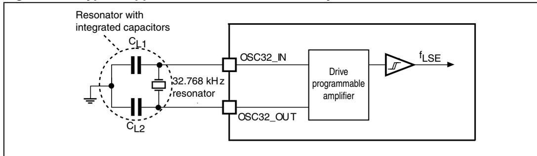
**Note:** An external resistor is not required between  $OSC32\_IN$  and  $OSC32\_OUT$  and it is forbidden to add one.
