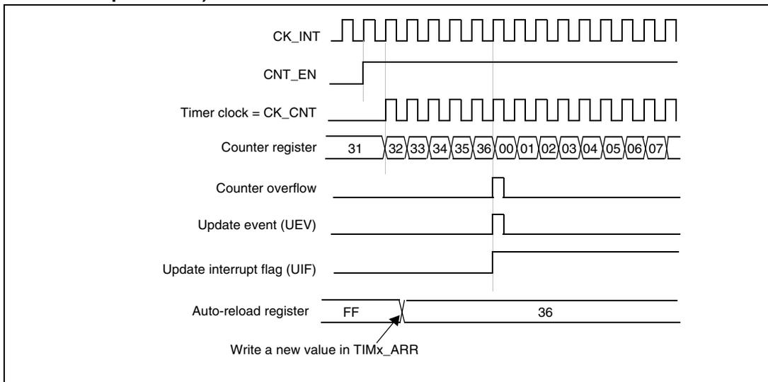
**Figure 61. Counter timing diagram, Update event when ARPE=1 (TIMx\_ARR preloaded)**
