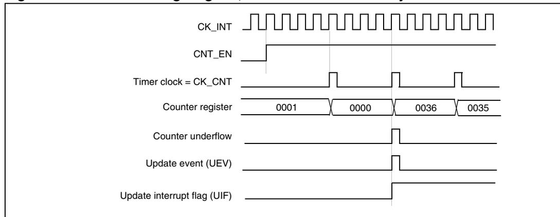
**Figure 65. Counter timing diagram, internal clock divided by N**
