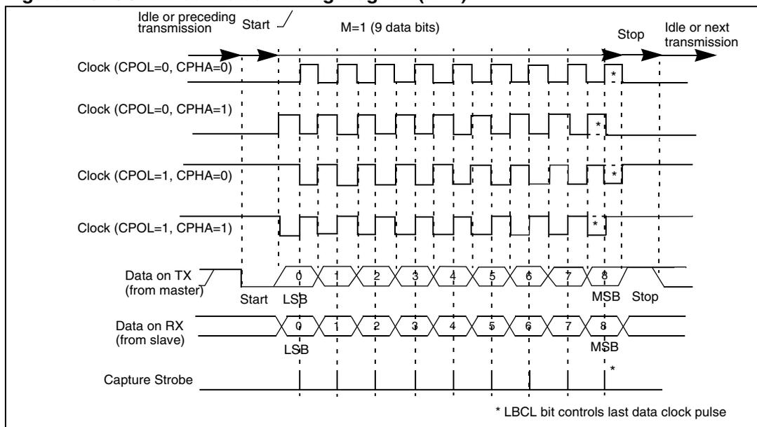
Figure 211. RX data setup/hold time
