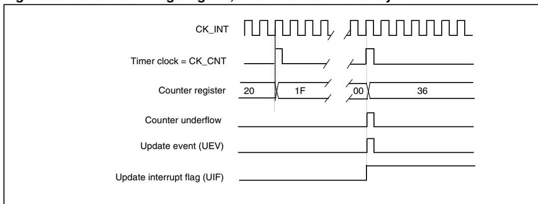
**Figure 66. Counter timing diagram, Update event when repetition counter is not used**
