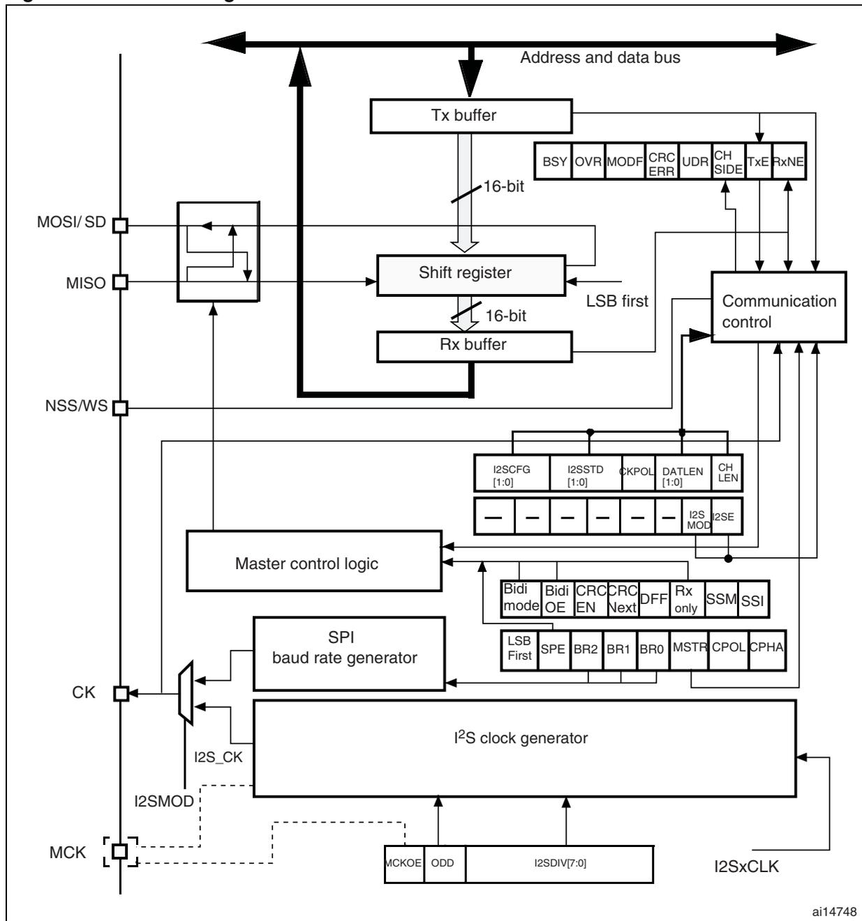
1. The MISO pin is not used in I<sup>2</sup>S mode.
