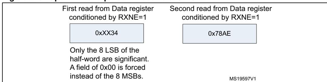
**Figure 247. LSB justified 16-bit extended to 32-bit packet frame with CPOL = 0**
