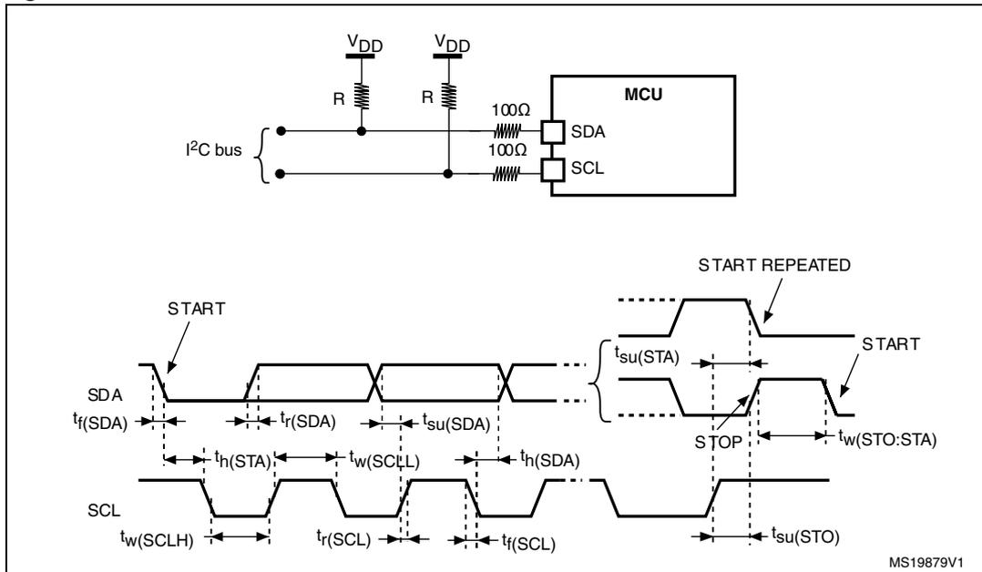
1. Measurement points are done at CMOS levels:  $0.3V_{DD}$  and  $0.7V_{DD}$ .
