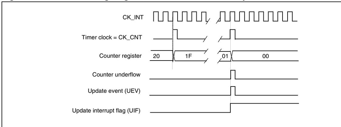
**Figure 71. Counter timing diagram, Update event with ARPE=1 (counter underflow)**
