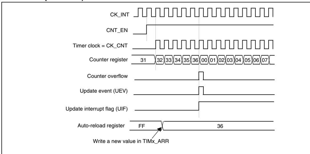
**Figure 160. Counter timing diagram, update event when ARPE=1 (TIMx\_ARR preloaded)**
