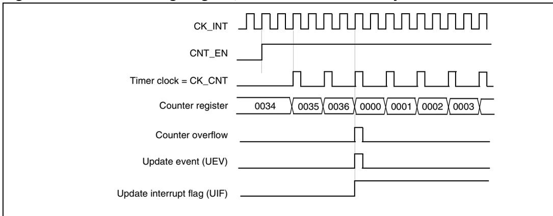
**Figure 58. Counter timing diagram, internal clock divided by 4**
