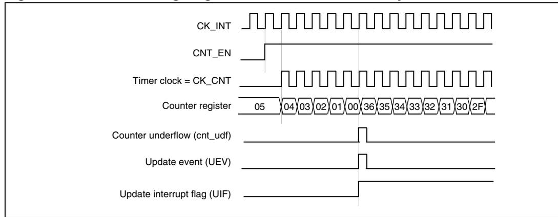
**Figure 63. Counter timing diagram, internal clock divided by 2**
