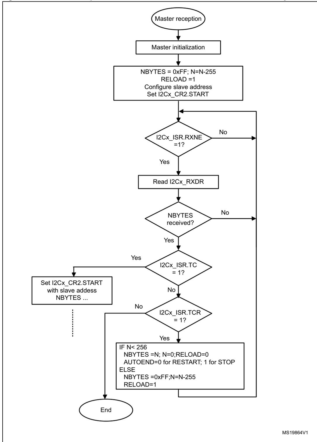
Figure 188. Transfer bus diagrams for I2C master receiver
