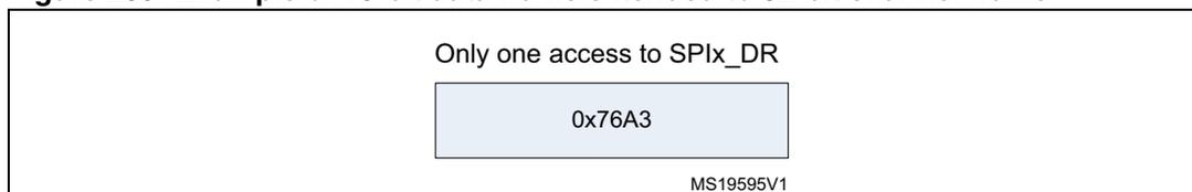
For transmission, each time an MSB is written to SPIx\_DR, the TXE flag is set and its interrupt, if allowed, is generated to load the SPIx\_DR register with the new value to send. This takes place even if 0x0000 have not yet been sent because it is done by hardware.
