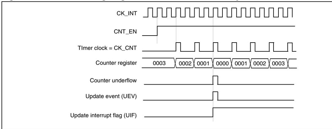
**Figure 69. Counter timing diagram, internal clock divided by 4, TIMx\_ARR=0x36**
