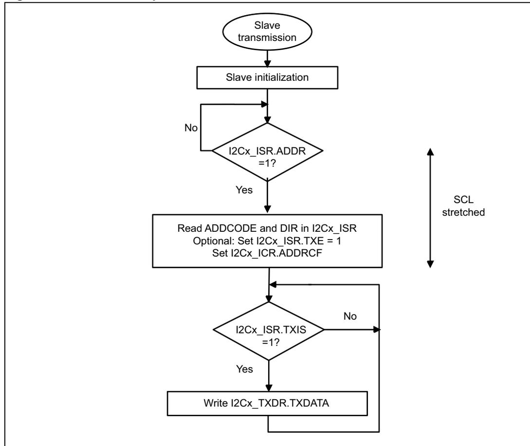
Figure 174. Transfer sequence flowchart for I2C slave transmitter, NOSTRETCH=1
