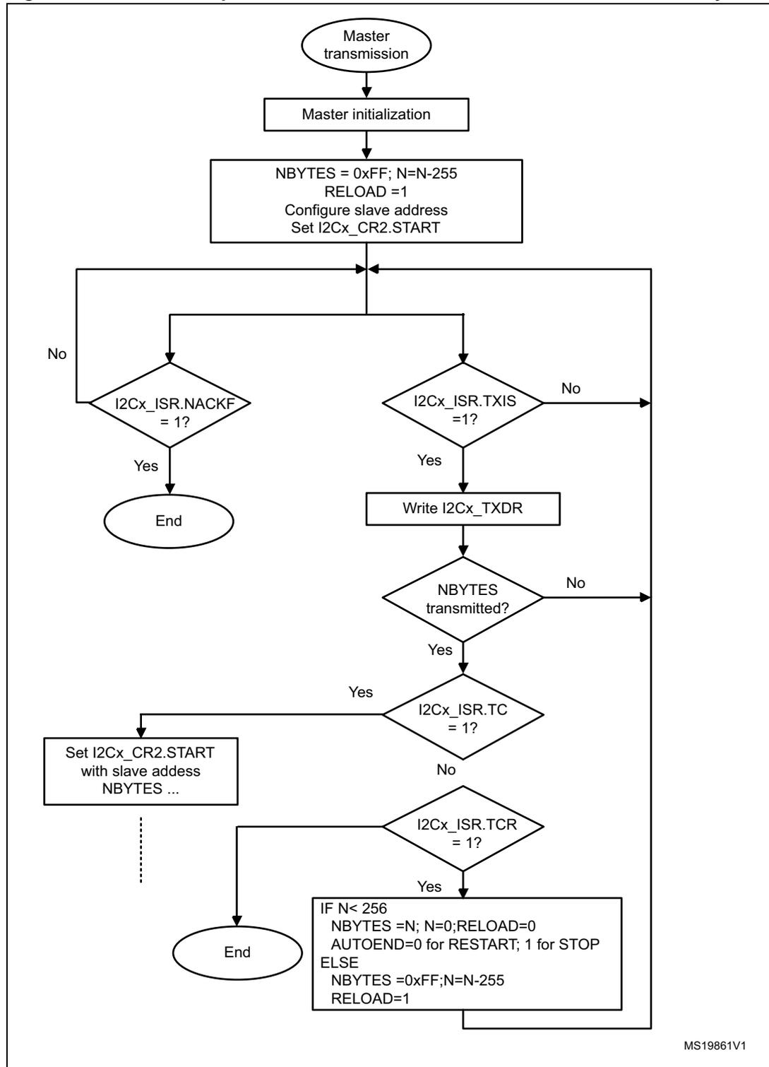
Figure 185. Transfer bus diagrams for I2C master transmitter
