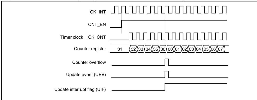
**Figure 57. Counter timing diagram, internal clock divided by 2**
