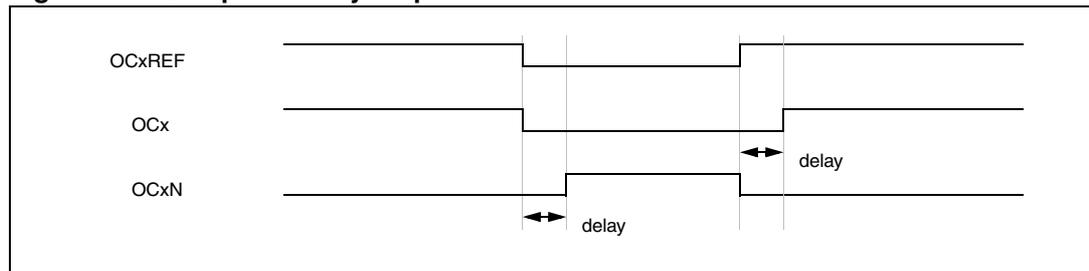
**Figure 144. Dead-time waveforms with delay greater than the negative pulse.**
