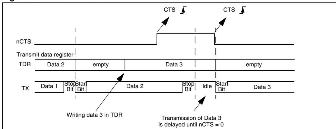
**Note:** For correct behavior, nCTS must be asserted at least 3 USART clock source periods before the end of the current character. In addition it should be noted that the CTSCF flag may not be set for pulses shorter than 2 x PCLK periods.
