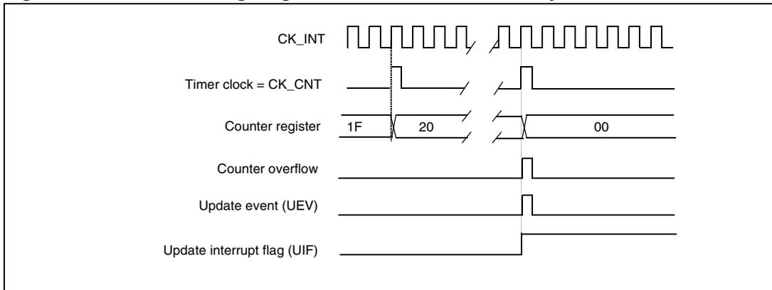
**Figure 60. Counter timing diagram, Update event when ARPE=0 (TIMx\_ARR not preloaded)**
