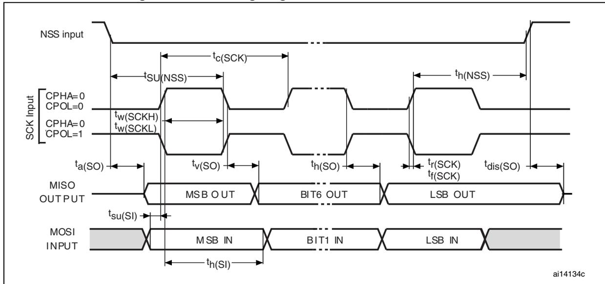
Figure 23. SPI timing diagram - slave mode and CPHA = 1<sup>(1)</sup>
