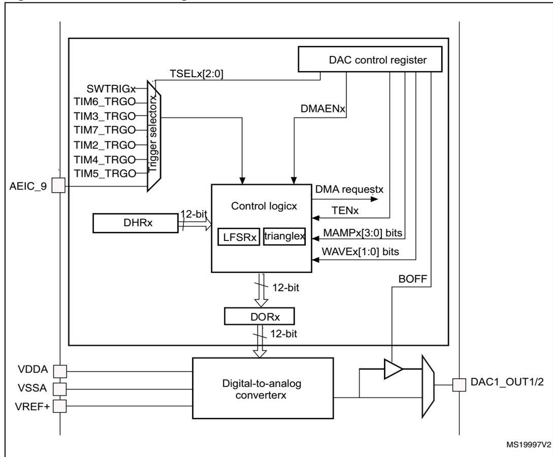
Figure 42. DAC2 block diagram
