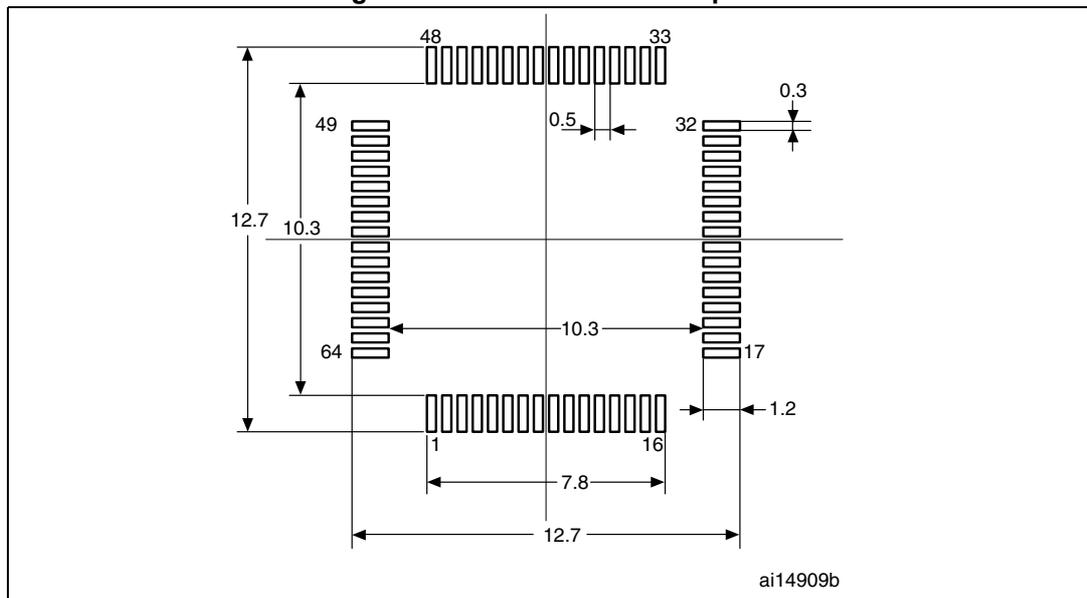
1. Dimensions are in millimeters.
