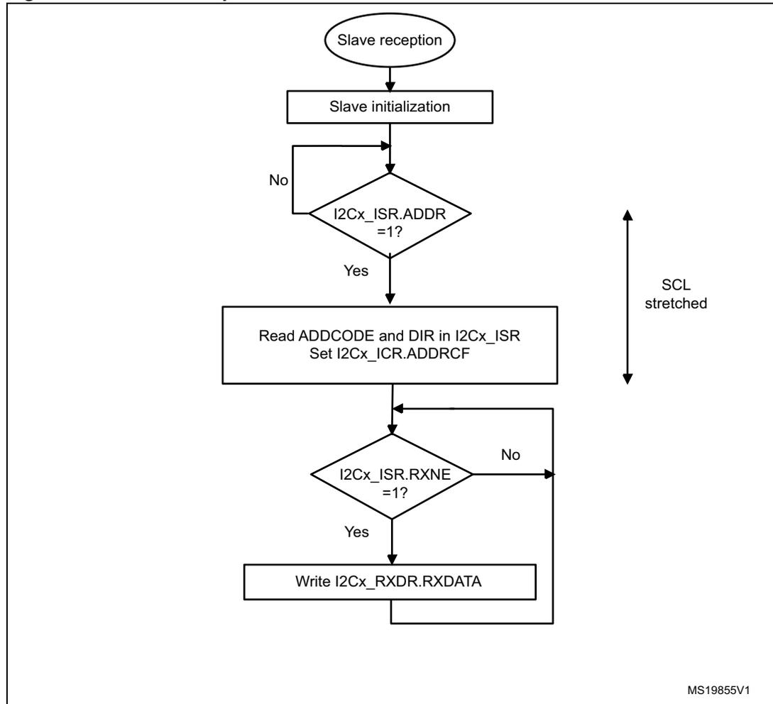
Figure 177. Transfer sequence flowchart for slave receiver with NOSTRETCH=1
