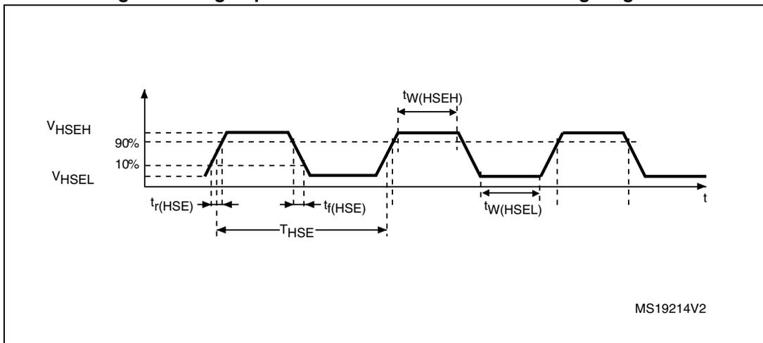
**Low-speed external user clock generated from an external source**
