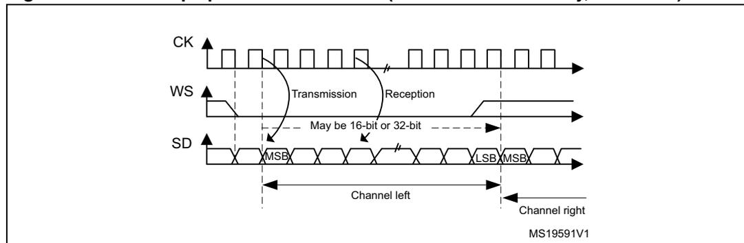
Data are latched on the falling edge of CK (for the transmitter) and are read on the rising edge (for the receiver). The WS signal is also latched on the falling edge of CK.
