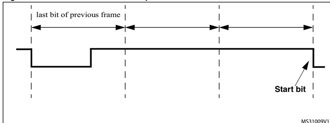
A configurable time window is counted before starting the transmission.
