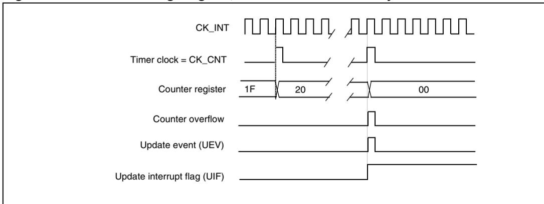
Figure 159. Counter timing diagram, update event when ARPE = 0 (TIMx\_ARR not preloaded)
