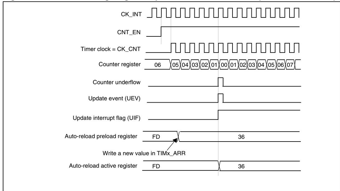
**Figure 72. Counter timing diagram, Update event with ARPE=1 (counter overflow)**
