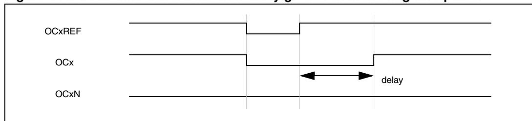
**Figure 145. Dead-time waveforms with delay greater than the positive pulse.**
