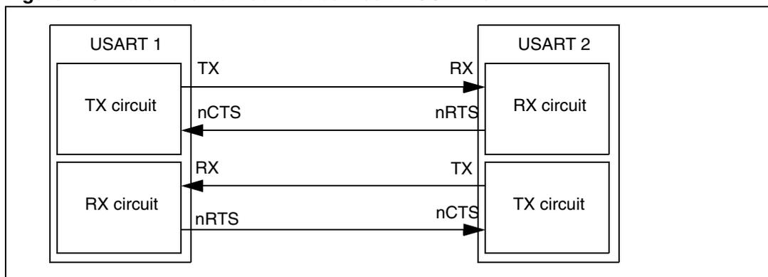
RTS and CTS flow control can be enabled independently by writing the RTSE and CTSE bits respectively to 1 (in the USART\_CR3 register).
