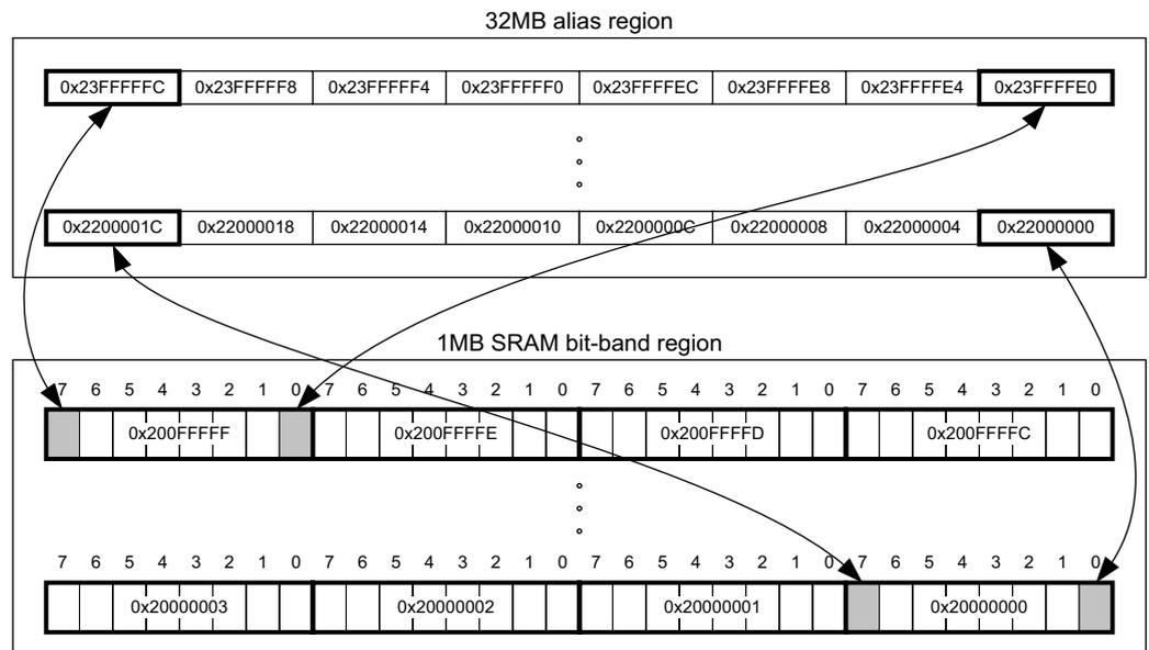
Figure 2-1 Bit-band mapping
