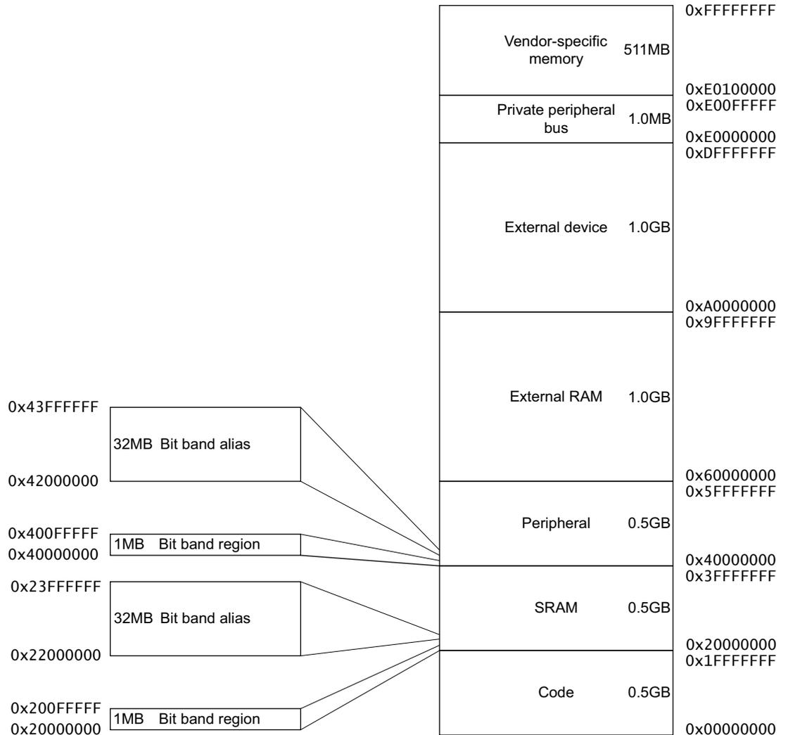
The regions for SRAM and peripherals include optional bit-band regions. Bit-banding provides atomic operations to bit data, see [Optional bit-banding on page 2-16](#).
