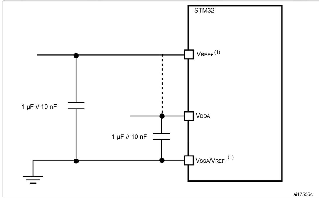
1.  $V_{REF+}$  input is available on all package whereas the  $V_{REF-}$  s available only on UFBGA176+25 and TFBGA240+25. When  $V_{REF-}$  is not available, it is internally connected to  $V_{DDA}$  and  $V_{SSA}$ .
