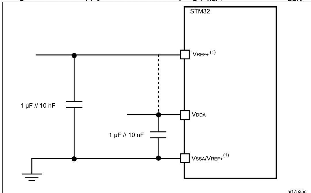
1.  $V_{REF+}$  input is available on all package whereas the  $V_{REF-}$  s available only on UFBGA176+25 and TFBGA240+25. When  $V_{REF-}$  is not available, it is internally connected to  $V_{DDA}$  and  $V_{SSA}$ .
