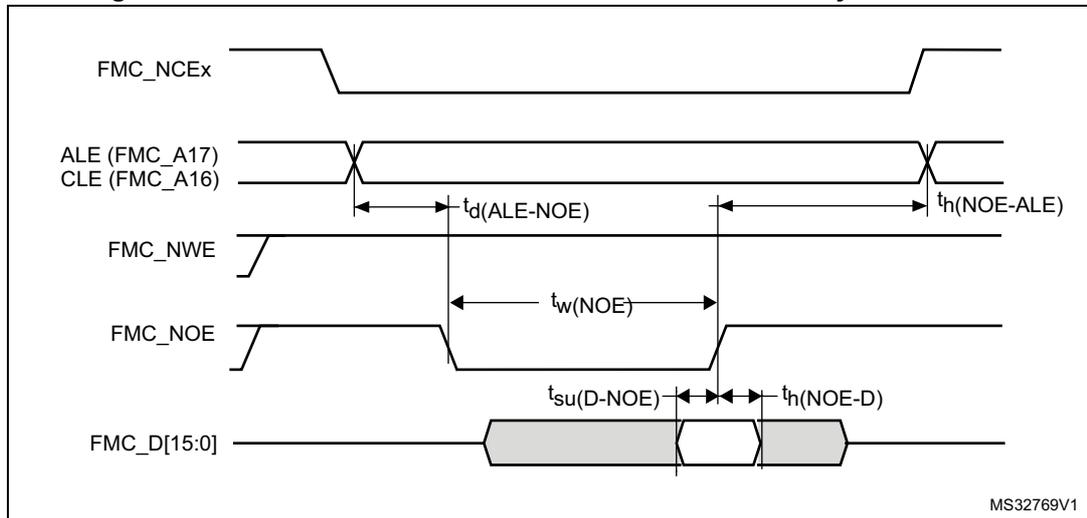
Figure 33. NAND controller waveforms for common memory write access
