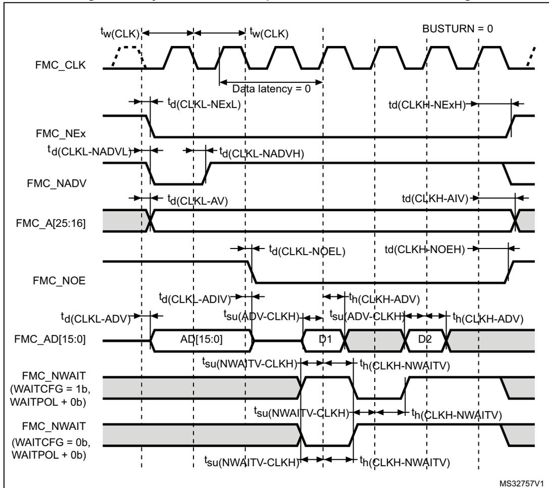
**Table 71. Synchronous multiplexed NOR/PSRAM read timings<sup>(1)</sup>**
