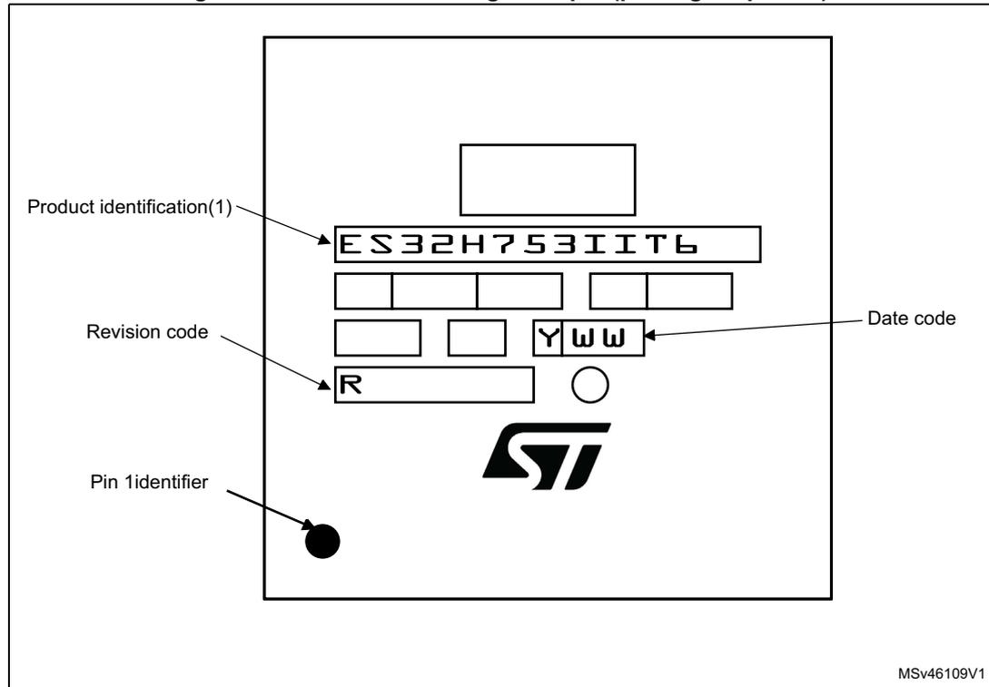
1. Parts marked as “ES”, “E” or accompanied by an Engineering Sample notification letter, are not yet qualified and therefore not approved for use in production. ST is not responsible for any consequences resulting from such use. In no event will ST be liable for the customer using any of these engineering samples in production. ST’s Quality department must be contacted prior to any decision to use these engineering samples to run a qualification activity.
