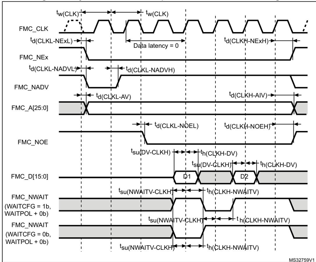
Table 73. Synchronous non-multiplexed NOR/PSRAM read timings<sup>(1)</sup>
