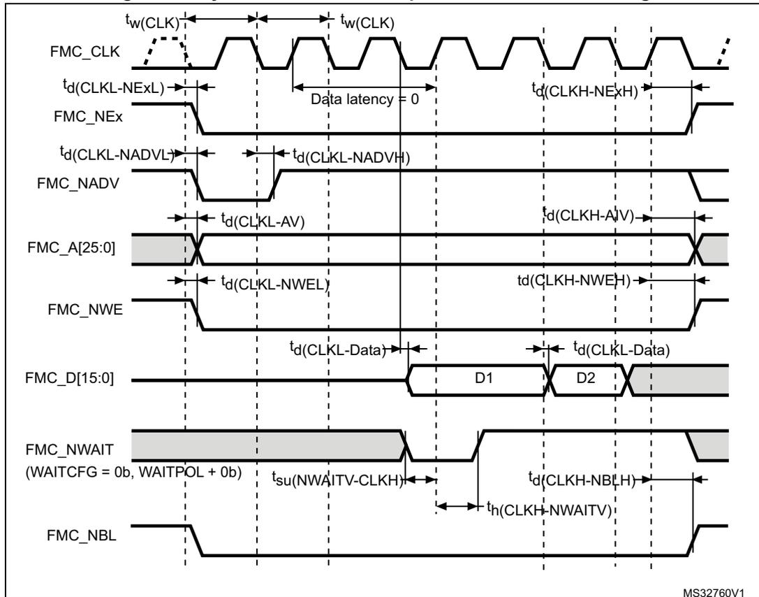
Table 74. Synchronous non-multiplexed PSRAM write timings<sup>(1)</sup>
