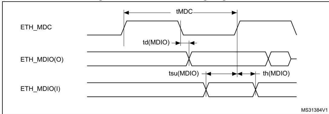
Table 111 gives the list of Ethernet MAC signals for the RMI and Figure 60 shows the corresponding timing diagram.
