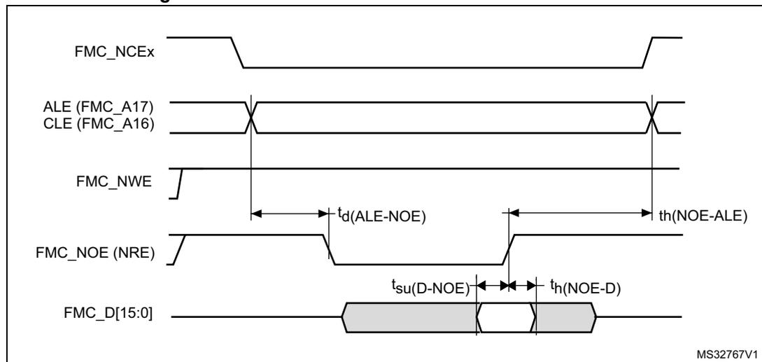
Figure 31. NAND controller waveforms for write access
