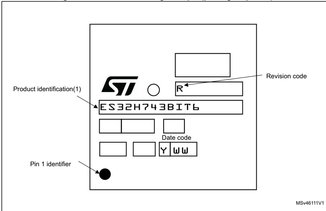
1. Parts marked as "ES", "E" or accompanied by an Engineering Sample notification letter, are not yet qualified and therefore not approved for use in production. ST is not responsible for any consequences resulting from such use. In no event will ST be liable for the customer using any of these engineering samples in production. ST's Quality department must be contacted prior to any decision to use these engineering samples to run a qualification activity.
