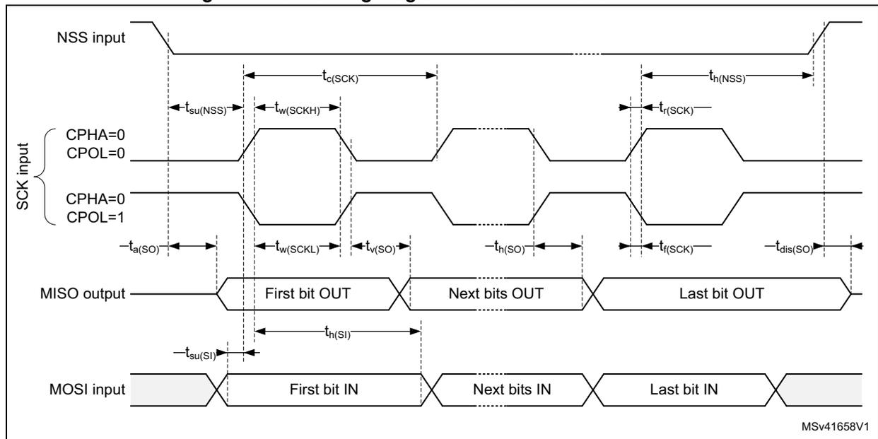
Figure 48. SPI timing diagram - slave mode and CPHA = 1<sup>(1)</sup>
