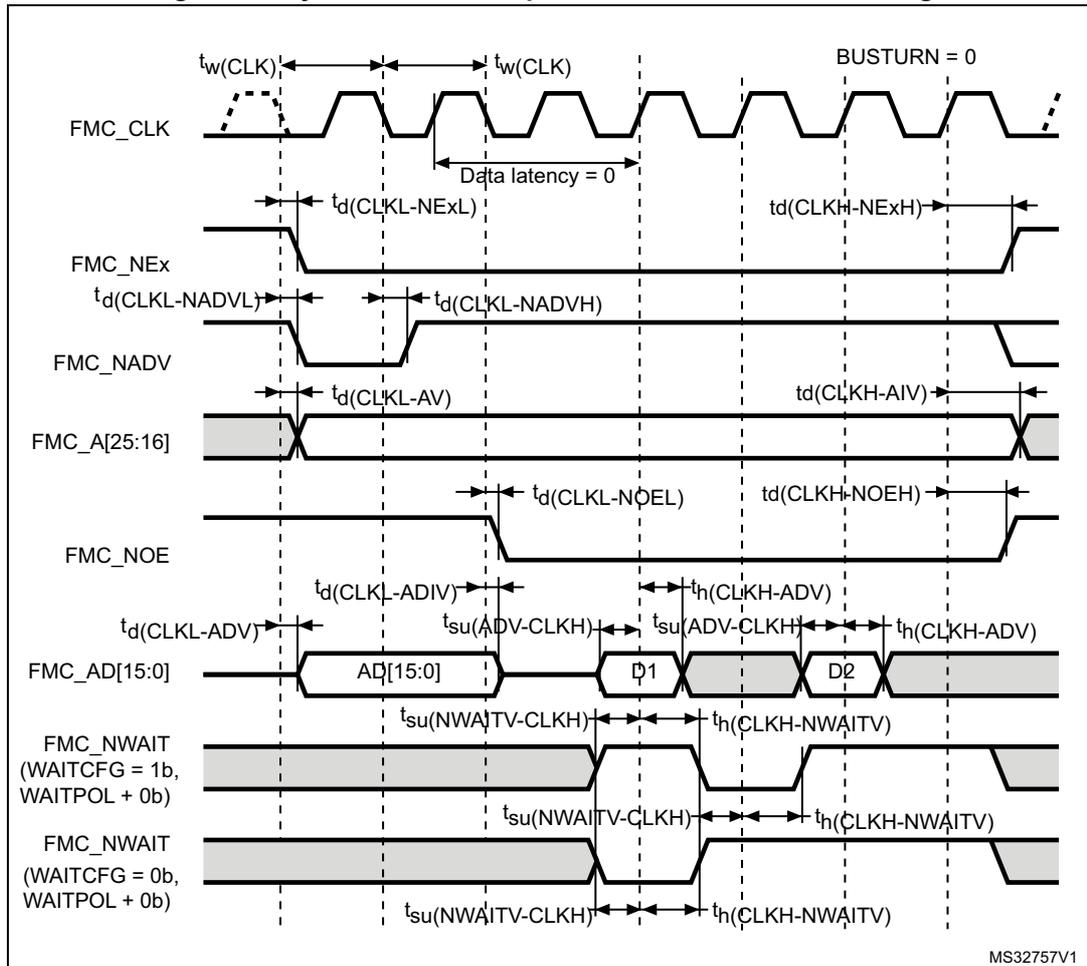
Table 71. Synchronous multiplexed NOR/PSRAM read timings<sup>(1)</sup>
