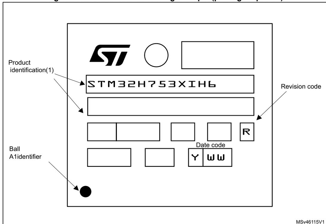
1. Parts marked as “ES”, “E” or accompanied by an Engineering Sample notification letter, are not yet qualified and therefore not approved for use in production. ST is not responsible for any consequences resulting from such use. In no event will ST be liable for the customer using any of these engineering samples in production. ST’s Quality department must be contacted prior to any decision to use these engineering samples to run a qualification activity.
