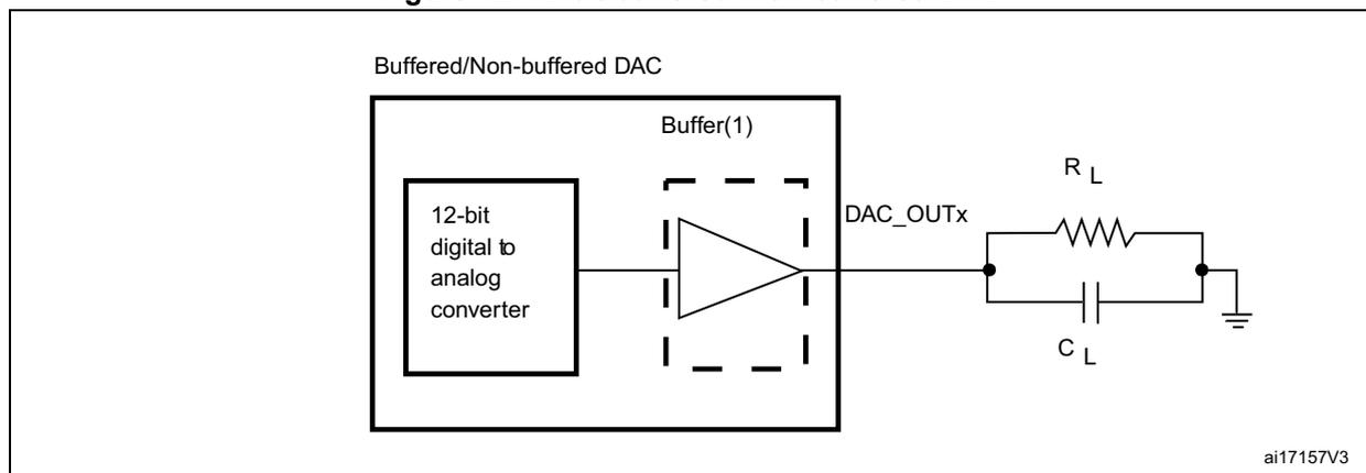
1. The DAC integrates an output buffer that can be used to reduce the output impedance and to drive external loads directly without the use of an external operational amplifier. The buffer can be bypassed by configuring the BOFFx bit in the DAC\_CR register.
