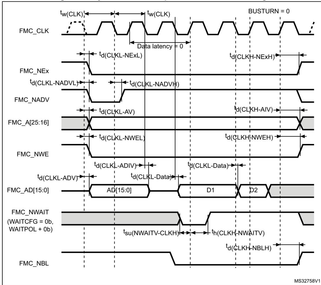
**Table 72. Synchronous multiplexed PSRAM write timings<sup>(1)</sup>**
