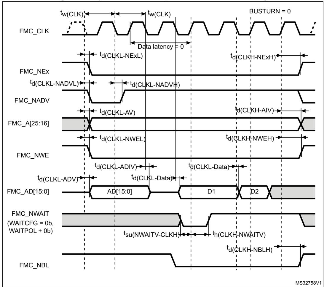
Table 72. Synchronous multiplexed PSRAM write timings<sup>(1)</sup>
