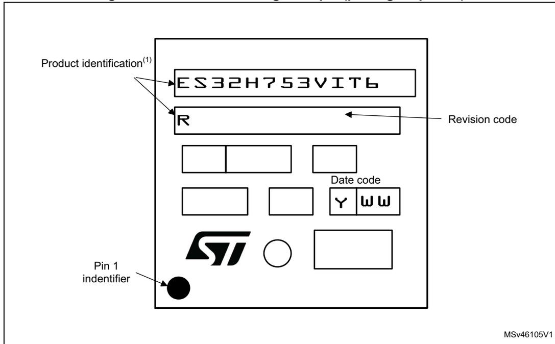
1. Parts marked as "ES", "E" or accompanied by an Engineering Sample notification letter, are not yet qualified and therefore not approved for use in production. ST is not responsible for any consequences resulting from such use. In no event will ST be liable for the customer using any of these engineering samples in production. ST's Quality department must be contacted prior to any decision to use these engineering samples to run a qualification activity.
