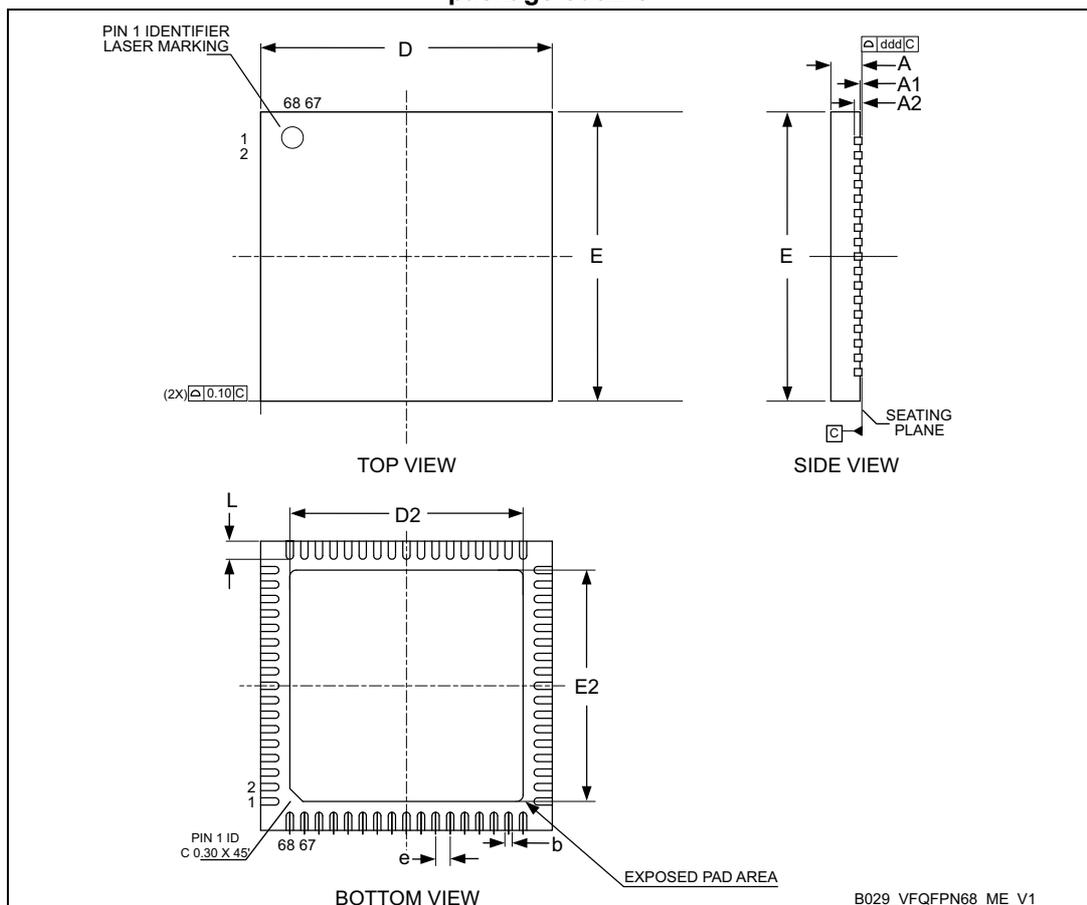
1. VFQFPN stands for Thermally Enhanced Very thin Fine pitch Quad Flat Packages No lead. Sawed version. Very thin profile:  $0.80 < A \leq 1.00$  mm.
