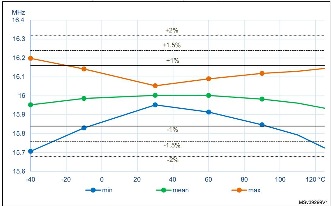
Multi-speed internal (MSI) RC oscillator
