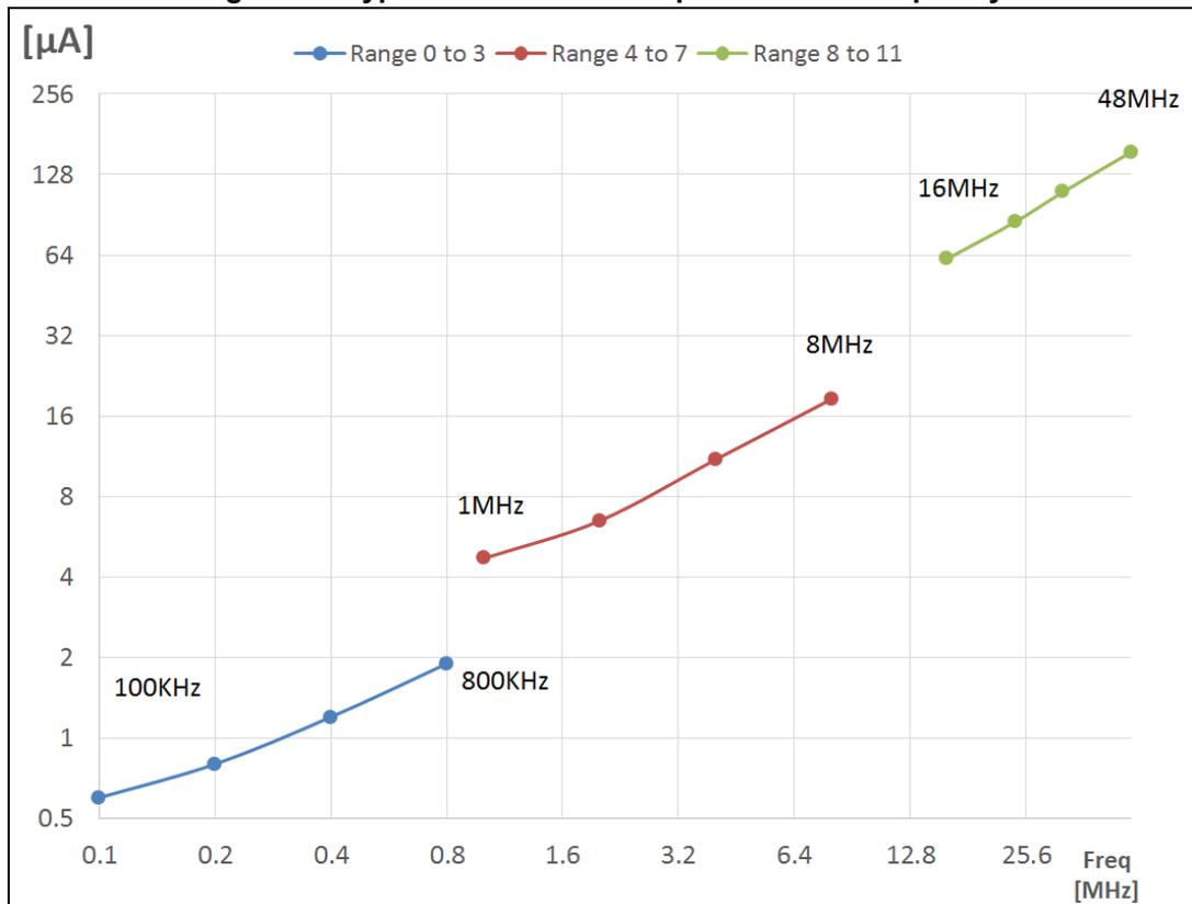
High-speed internal 48 MHz (HSI48) RC oscillator
