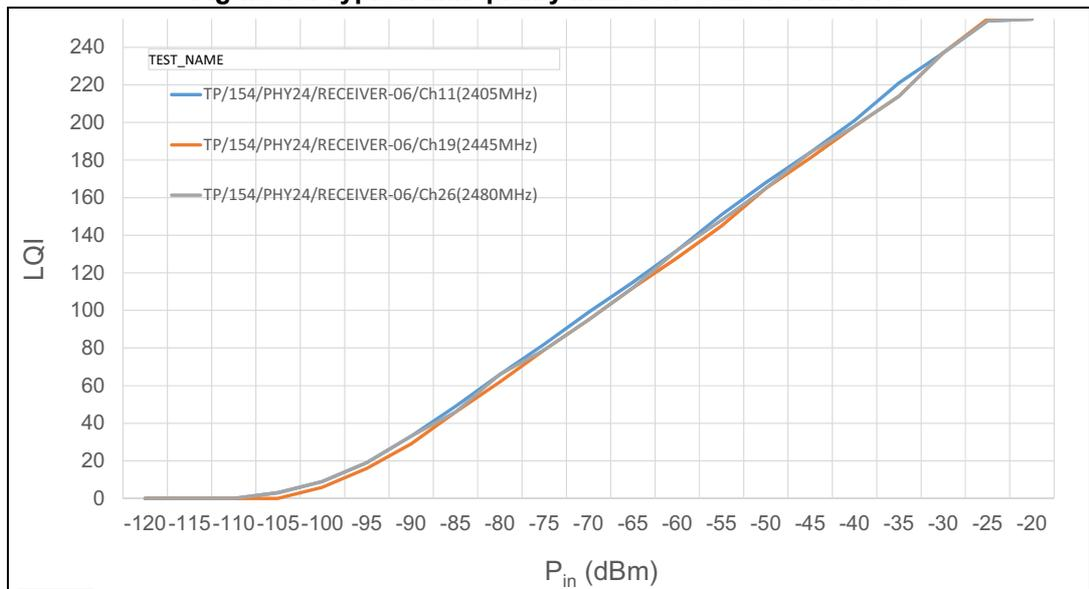
Figure 17. Typical energy detection (T = 27°C, V<sub>DD</sub> = 3.3 V)
