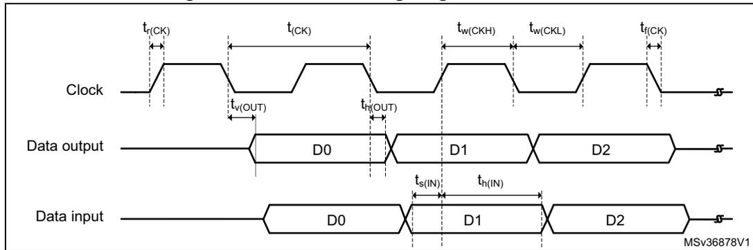
Figure 31. Quad-SPI timing diagram - DDR mode
