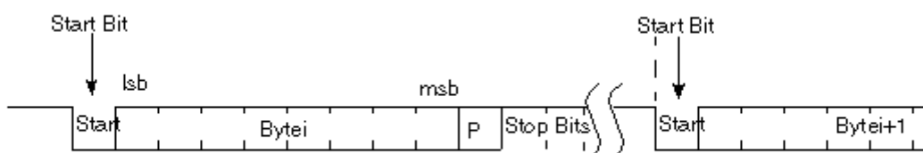
Figure 11-44. Start Bit Diagram
