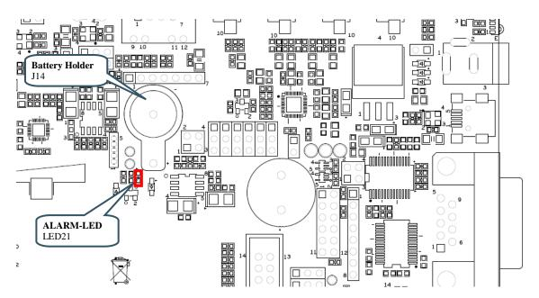
Figure 8 – VBAT and ALARM circuit
