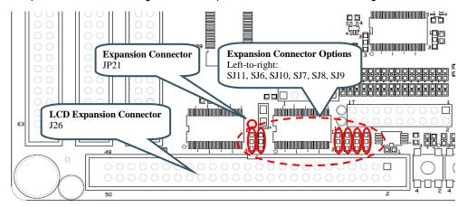
Figure 23 – LCD Expansion Interface
