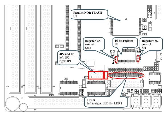
Figure 4 - External Memory Bus Circuit
