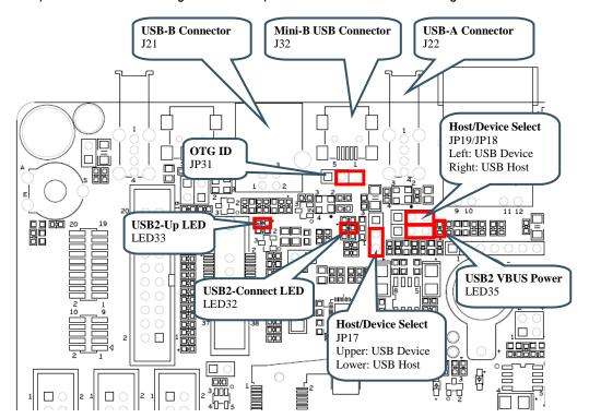
See picture below for locating relevant components. The table below lists signal connections.
