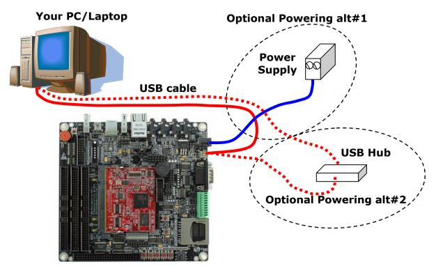
Figure 26 – Powering of OEM Base Board
