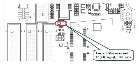
Figure 2 – Current Measurement J2
