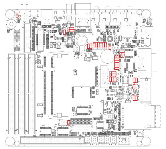
Figure 25 – OEM Base Board Default Jumper Positions
