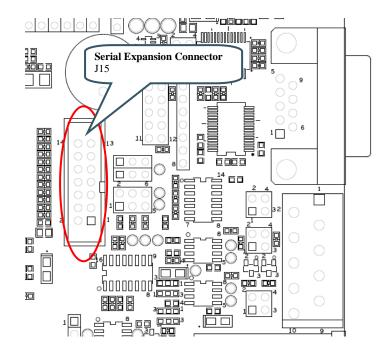
Figure 12 – Serial Expansion Connector
