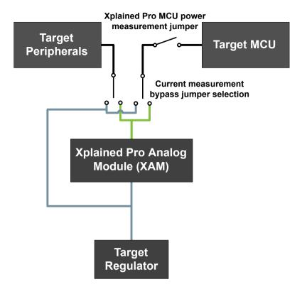
On the SAM L22 Xplained Pro the XAM can be used in four configurations:
