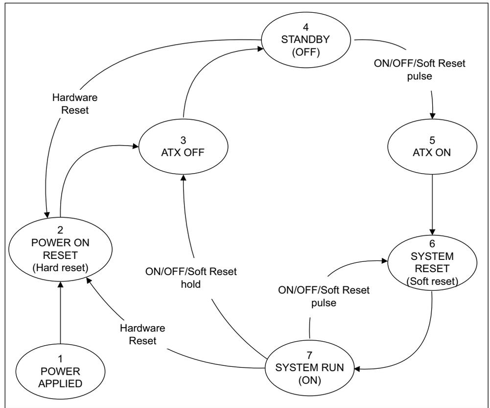
Figure 4-1 Push-button reset state diagram
