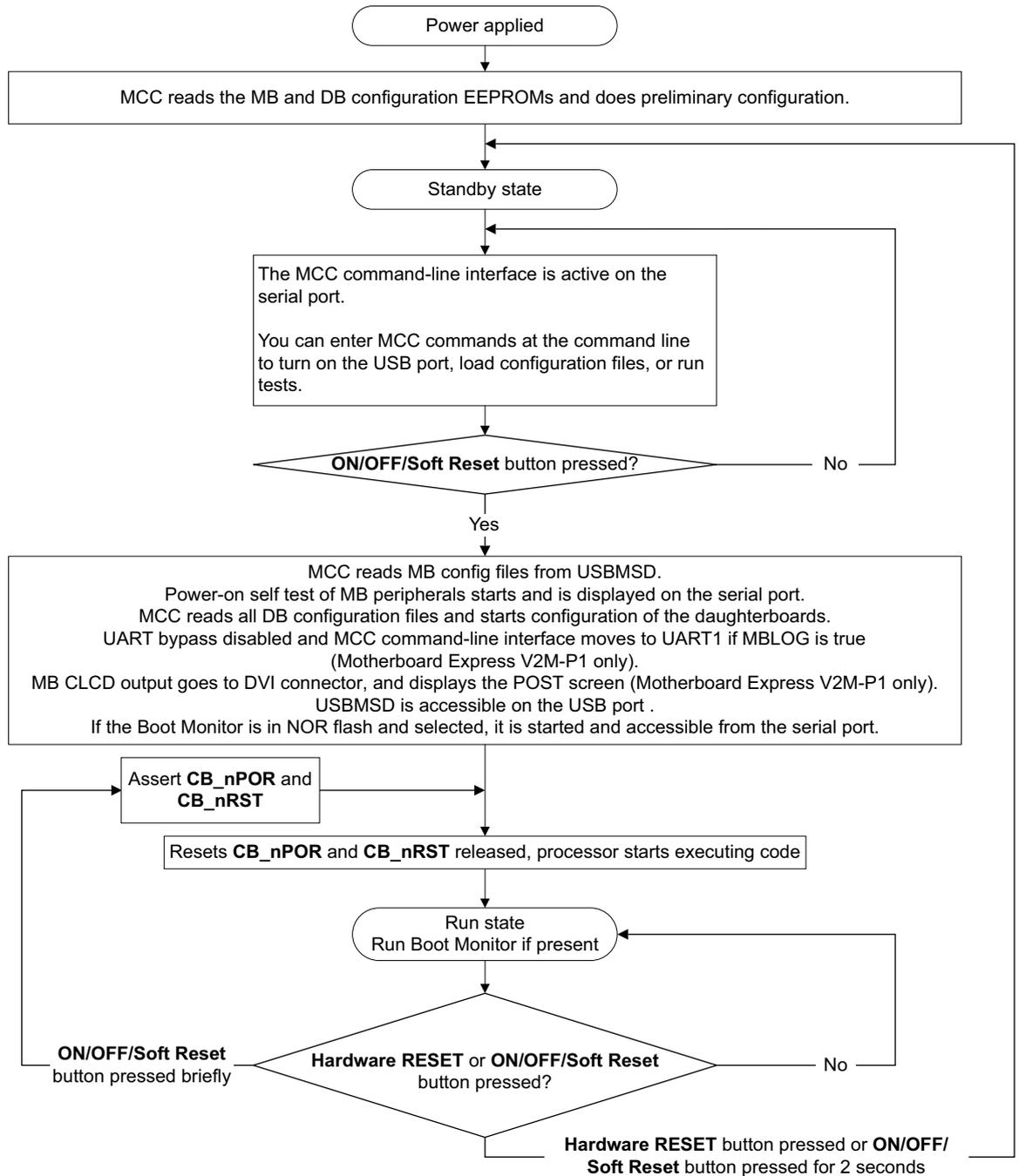
Figure 3-1 Overview of startup sequence
