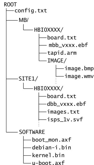
Figure 5-2 Typical custom motherboard USBMSD directory structure
