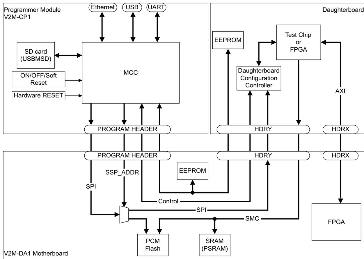
**Figure 2-2 Custom motherboard configuration architecture**
