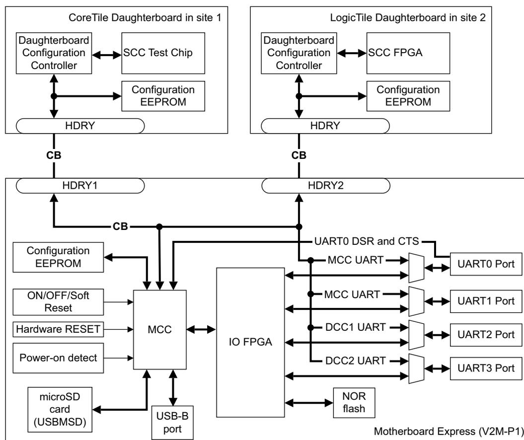
**Figure 2-1 Motherboard Express, V2M-P1, configuration architecture**
