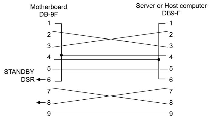
**Figure 4-2** Modem cable wiring diagram
