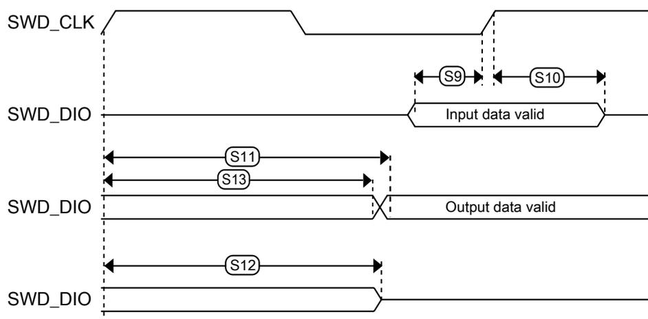
Figure 31. Serial wire data timing
