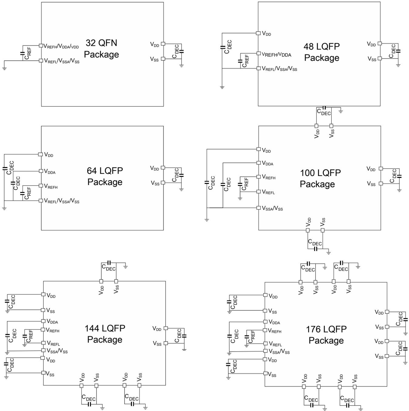
NOTE: V<sub>DD</sub> and V<sub>DDA</sub> must be shorted to a common source on PCB
