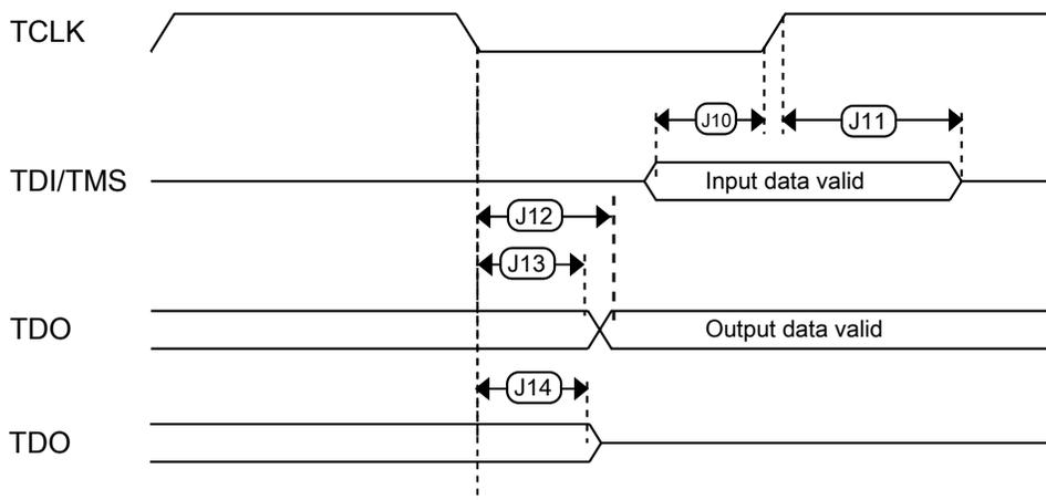
Figure 35. Test Access Port timing
