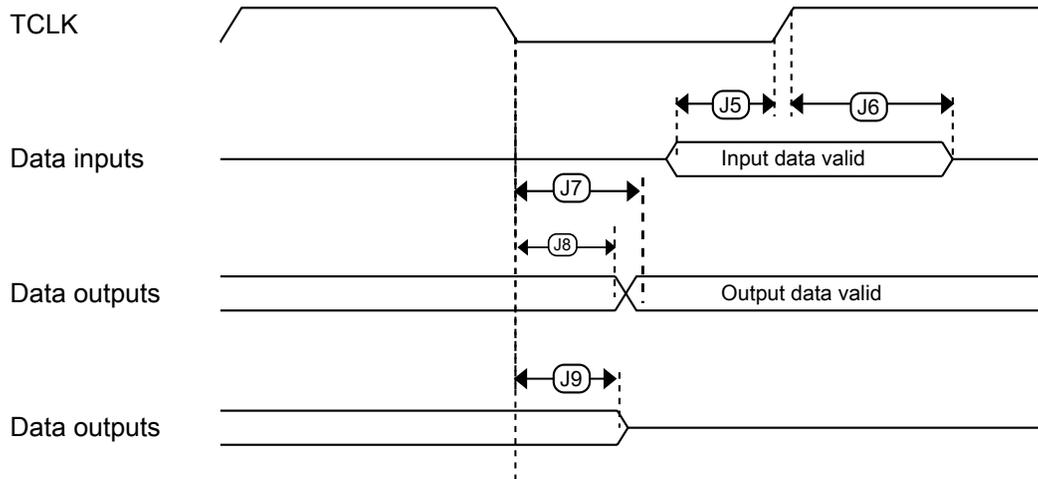
**Figure 34. Boundary scan (JTAG) timing**
