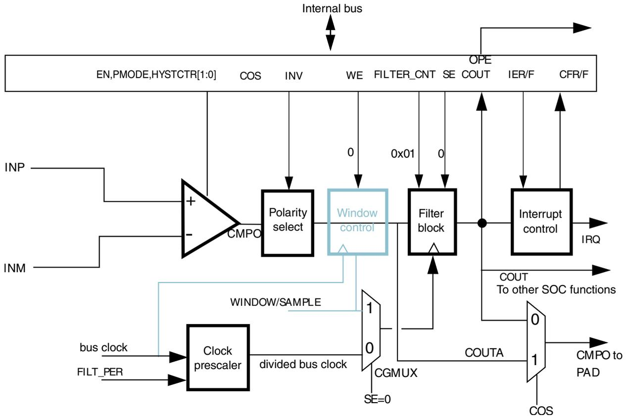
**Figure 45-6. Sampled, Non-Filtered (# 3B): sampling interval internally derived**
