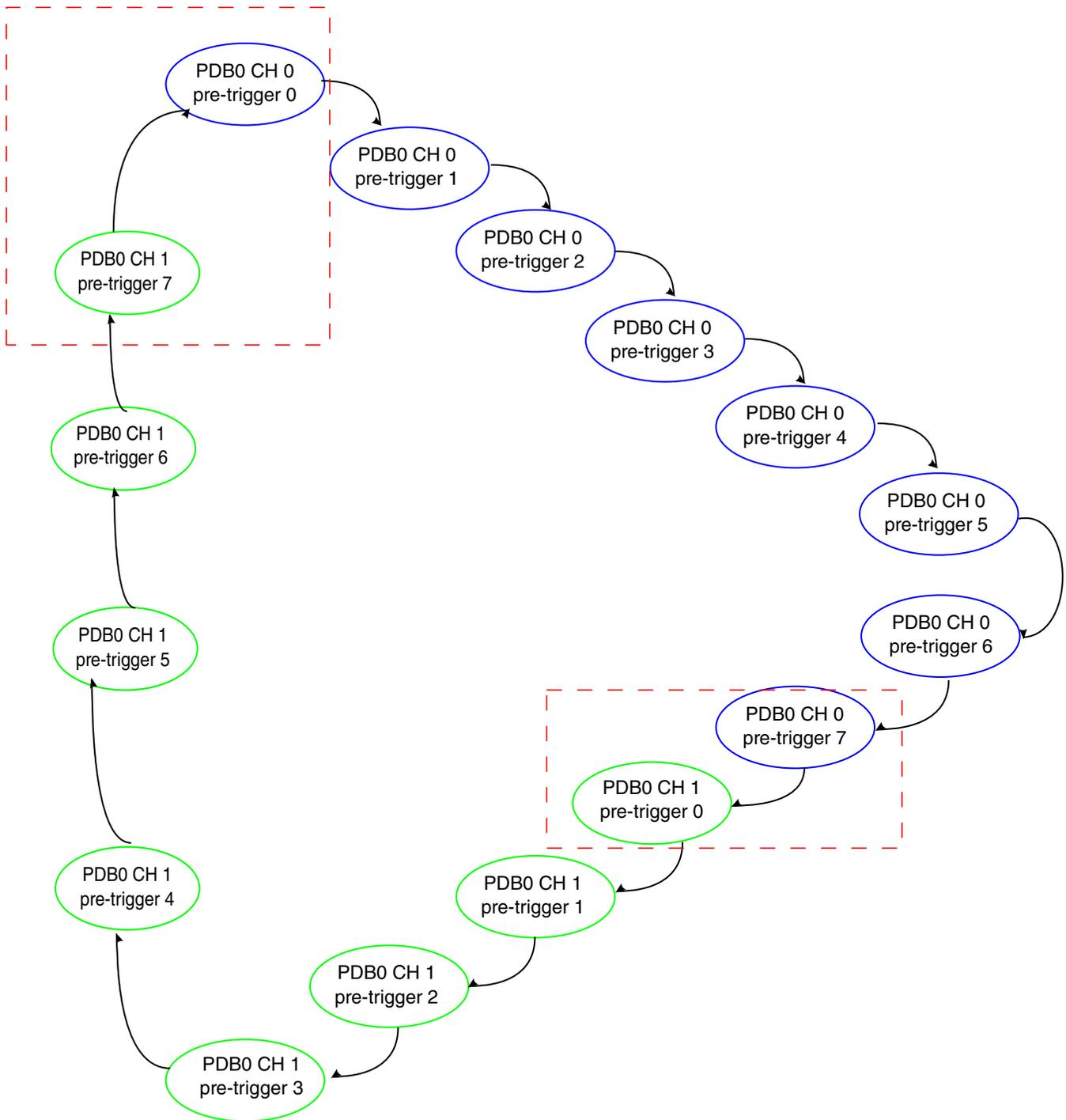
**Figure 46-4. PDB back-to-back chain forming PDB0-PDB1 ring**
