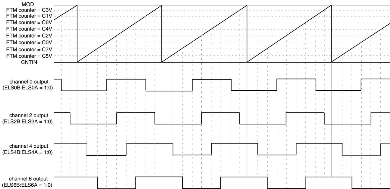
**Figure 47-49. Example of Four Pairs of Channels in Modified Combine PWM Mode**
