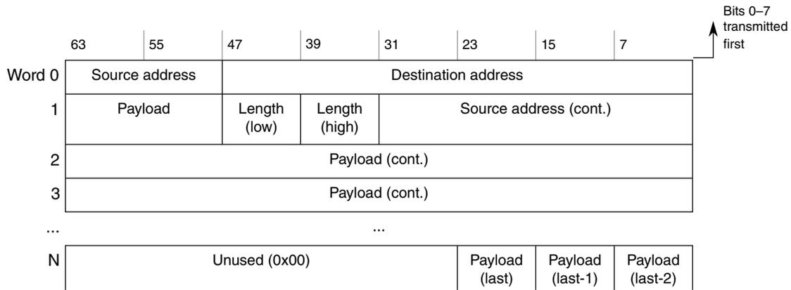
**Figure 57-14. Normal Ethernet frame 64-bit mapping example**
