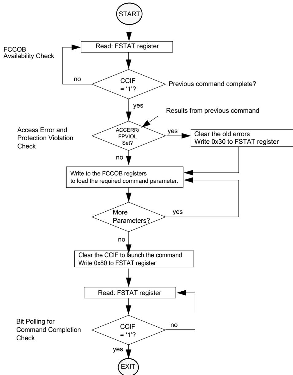
**Figure 37-6. Generic flash command write sequence flowchart**
