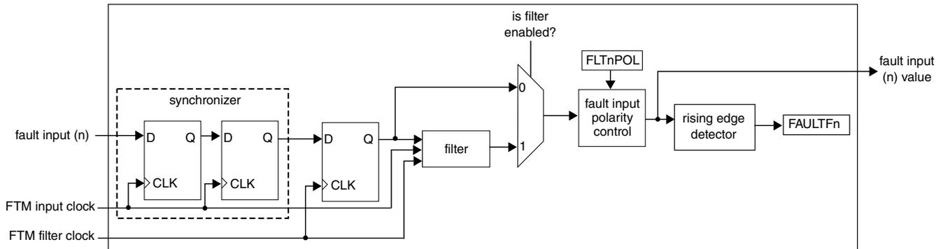
**Figure 47-82. Diagram for Fault Control when FLTPS[3:0]  $\neq$  0**
