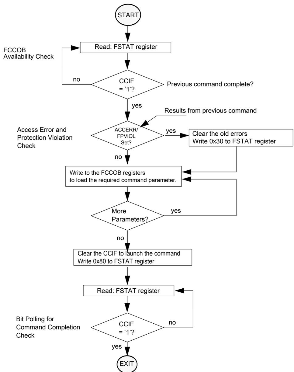
Figure 36-14. Generic flash command write sequence flowchart
