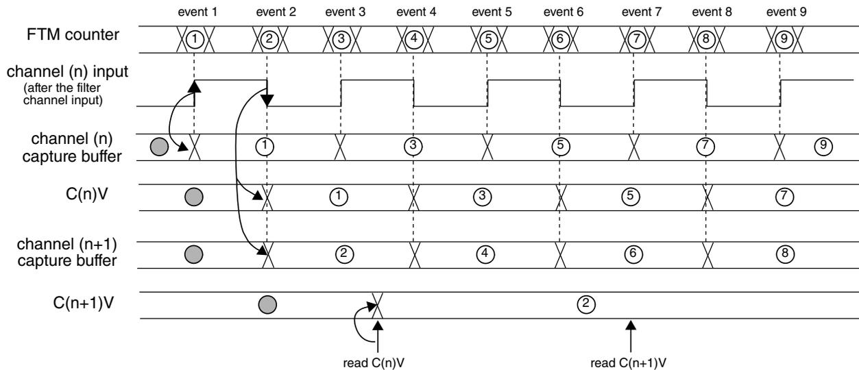
**Figure 47-100. Dual Edge Capture mode read coherency mechanism**
