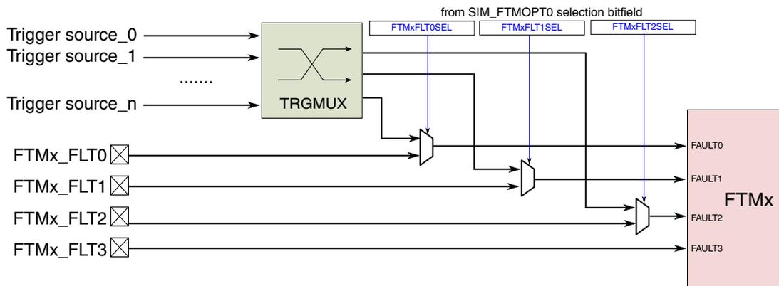
Figure 47-1. Fault detection inputs
