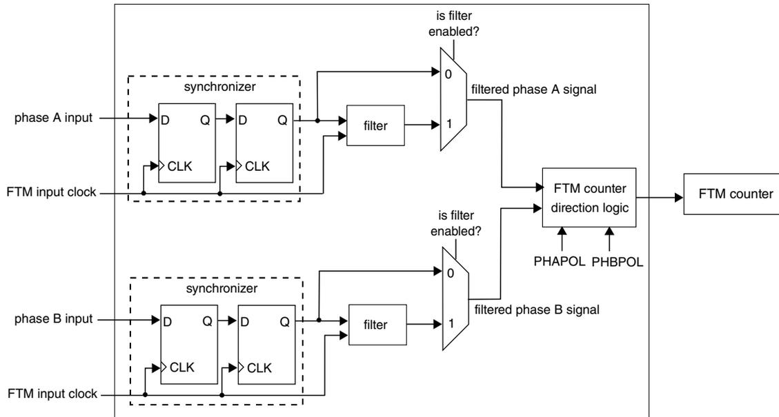
**Figure 47-101. Diagram for Quadrature Decoder when FLTIPS[3:0] = 0**
