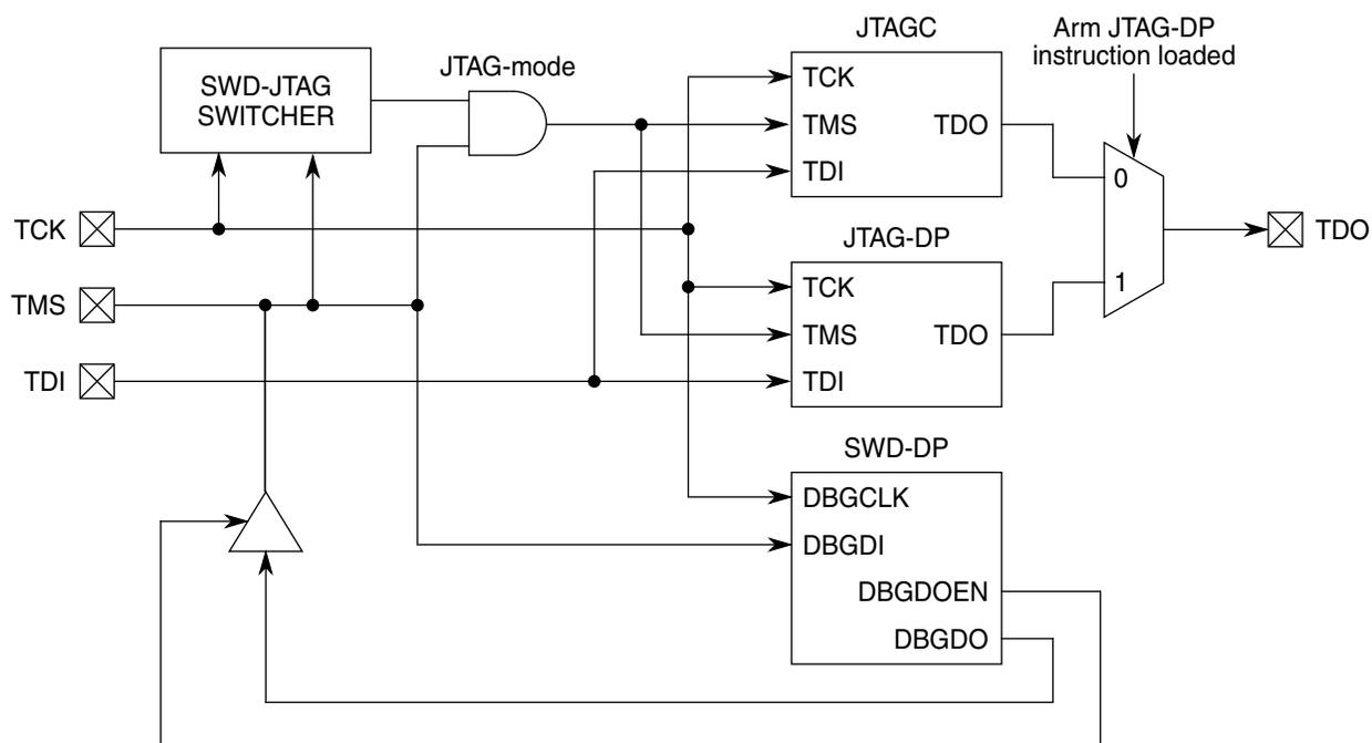
Figure 58-3. Modified debug port for CM4 core
