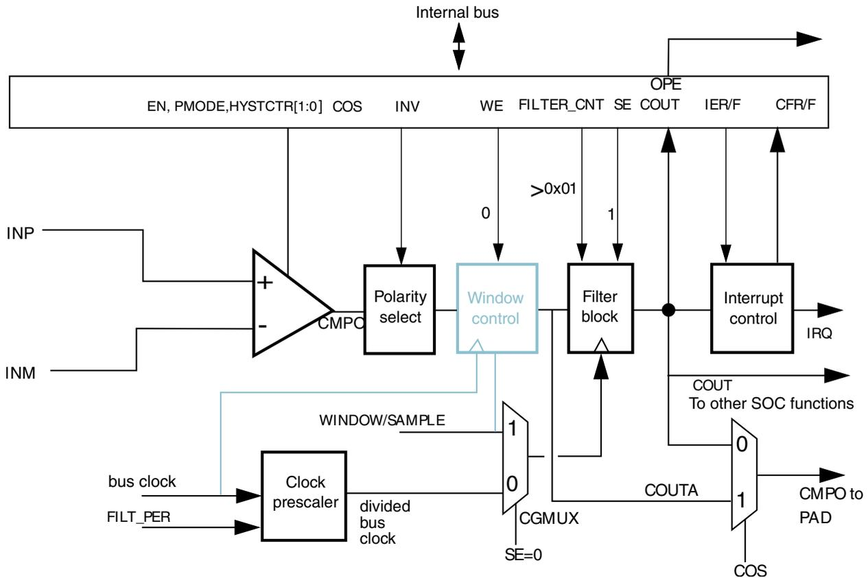
**Figure 45-9. Sampled, Filtered (# 4B): sampling point internally derived**
