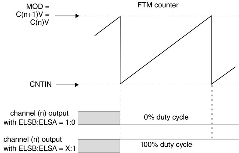
**Figure 47-39. Channel (n) output if  $(C(n)V = C(n+1)V = MOD)$**
