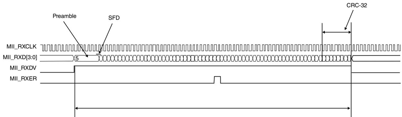
**Figure 57-26. MII receive operation — errored frame**
