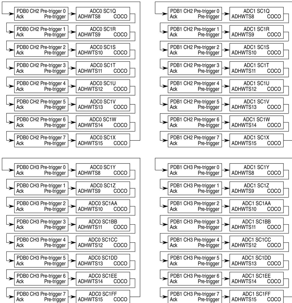
Figure 46-6. PDB-ADC back to back connection (Part 2 of 2)
