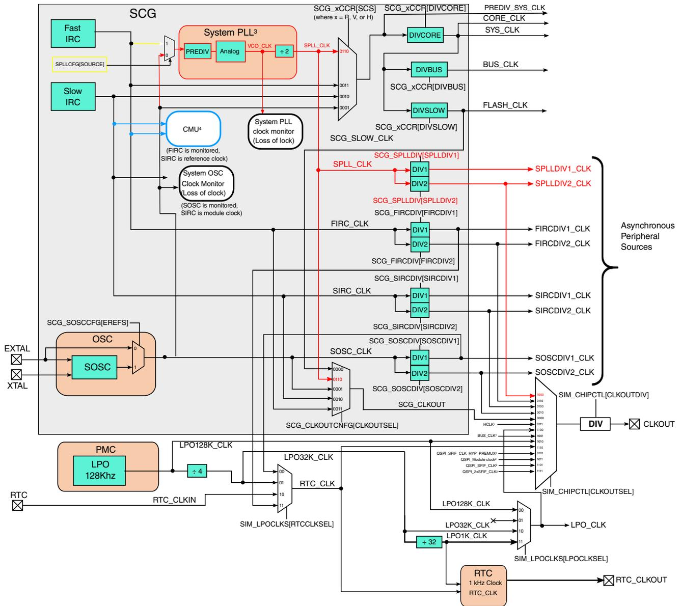
1. The source of HCLK (to Arm® Cortex® modules) is CORE\_CLK. See section 'Clock definitions' for CORE\_CLK and BUS\_CLK
