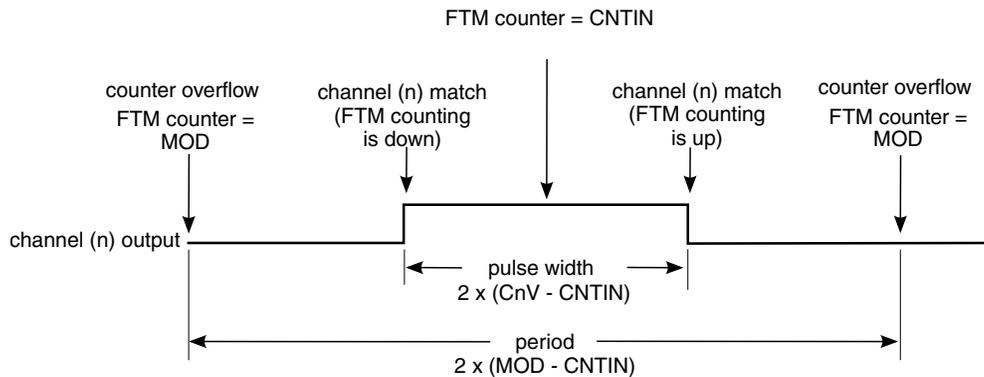
**Figure 47-27. CPWM period and pulse width with ELSB:ELSA = 1:0**
