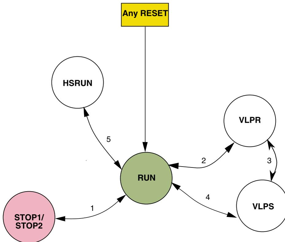
**Figure 40-1. Power mode state diagram**
