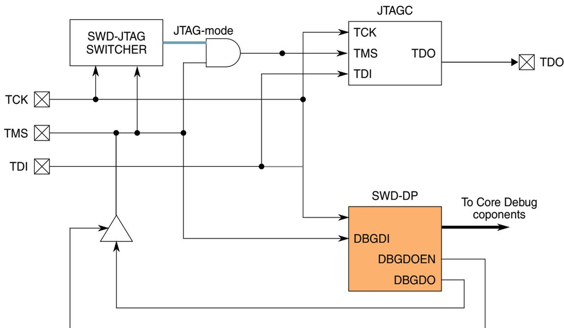
**Figure 58-4. Modified debug port for CM0+ core**
