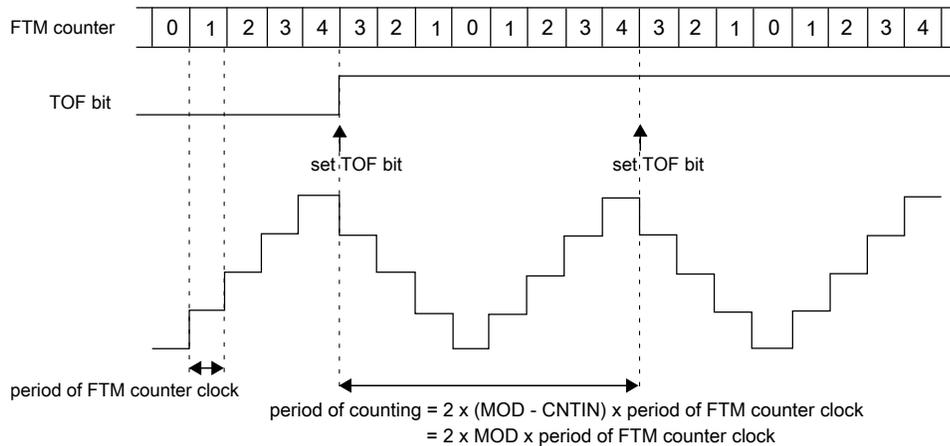
**Figure 47-11. Example of up-down counting when CNTIN = 0x0000**
