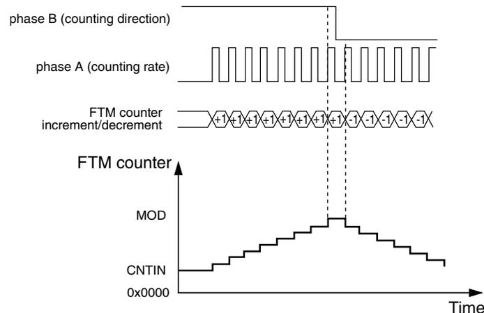
**Figure 47-103. Quadrature Decoder – Count and Direction Encoding mode**
