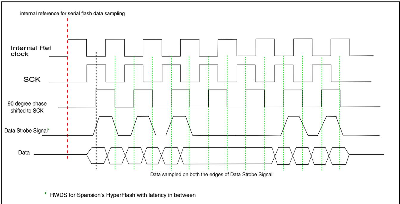
**Figure 38-12. Data Strobe functionality with latency included**
