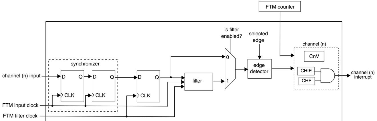
Note: The filter is only available for the channels 0, 1, 2, and 3 inputs.
