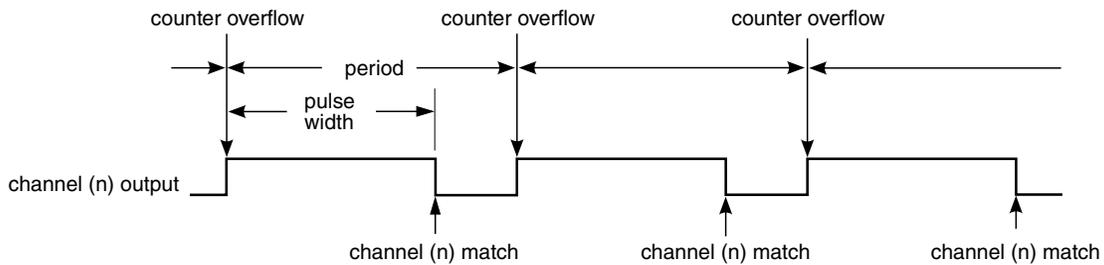
**Figure 47-24. EPWM period and pulse width with ELSB:ELSA = 1:0**
