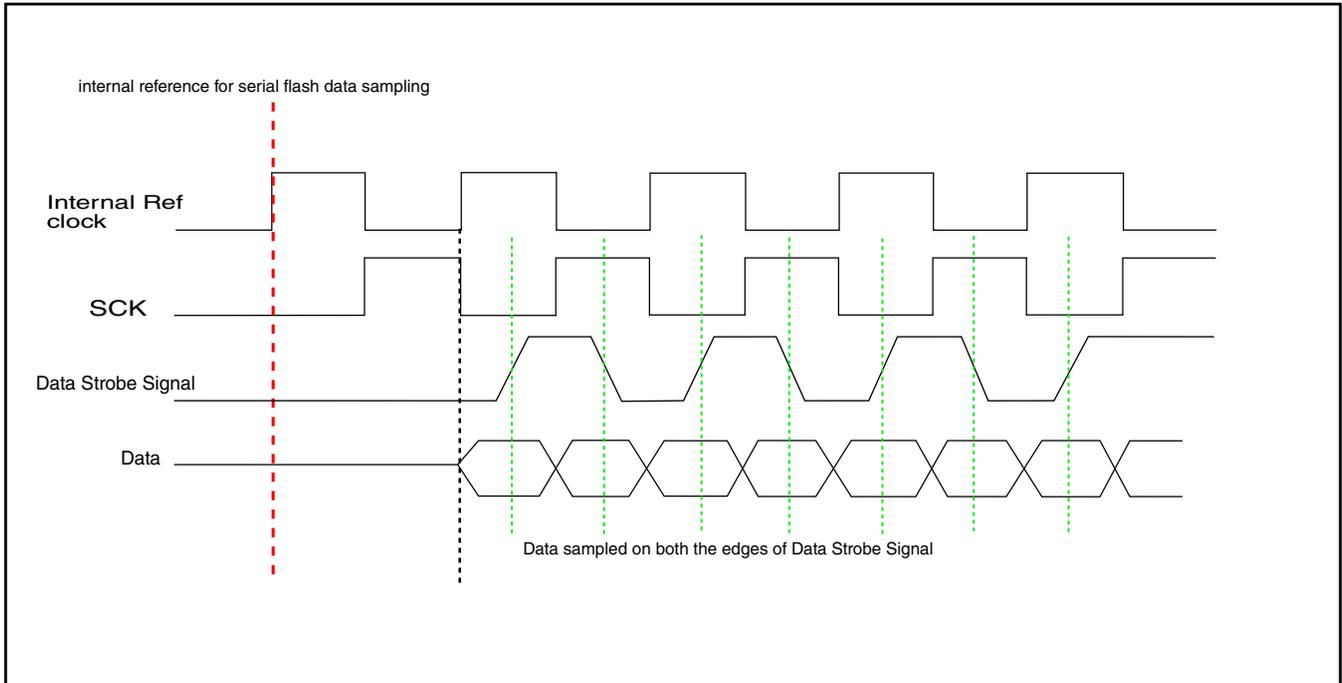
**Figure 38-11. Data Strobe functionality in DDR mode**
