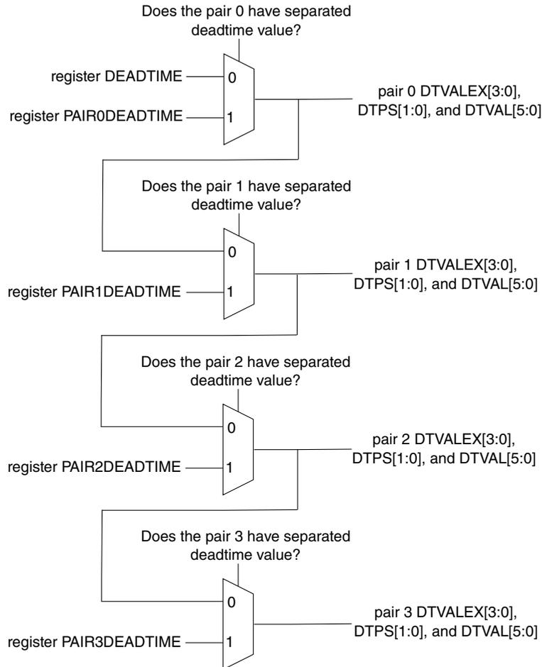
**Figure 47-77. Separated Deadtime by Pair of Channels**
