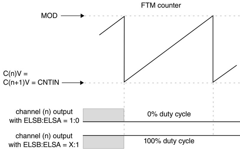
**Figure 47-38. Channel (n) output if  $(C(n)V = C(n+1)V = CNTIN)$**
