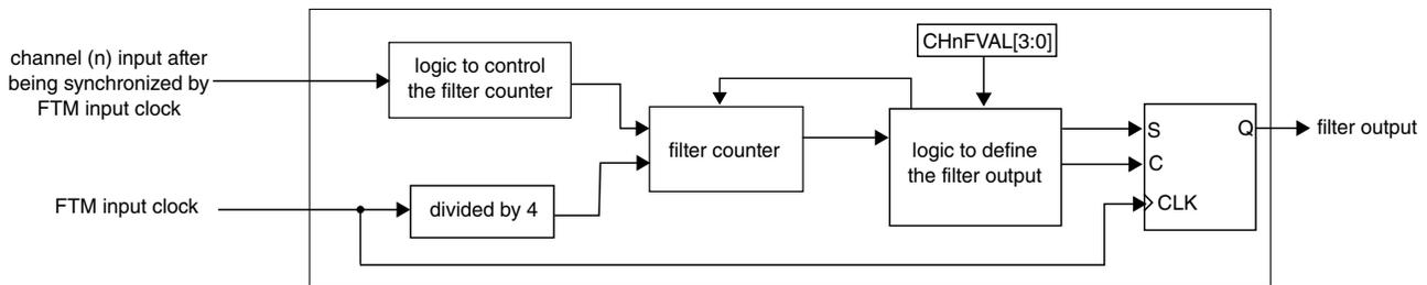
**Figure 47-16. Channel Input Filter when FLTPS[3:0] = 0**
