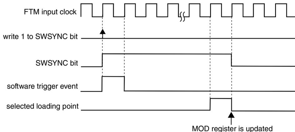
**Figure 47-60. MOD synchronization with (SYNCMODE = 0) and (PWMSYNC = 1)**
