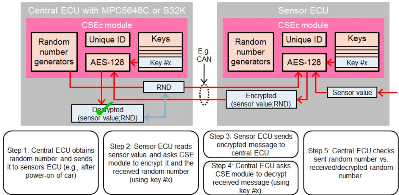
Figure 5-3. Secure communication
