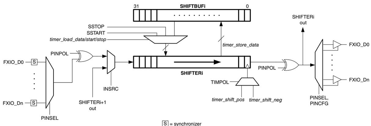
**Figure 54-2. Shifter Microarchitecture**
