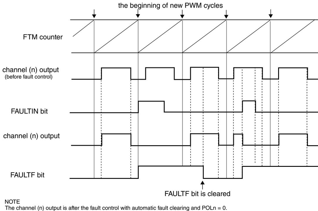
**Figure 47-84. Fault control with automatic fault clearing**
