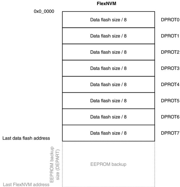
**Figure 36-11. Data flash protection ( $2^n$  data flash sizes)**
