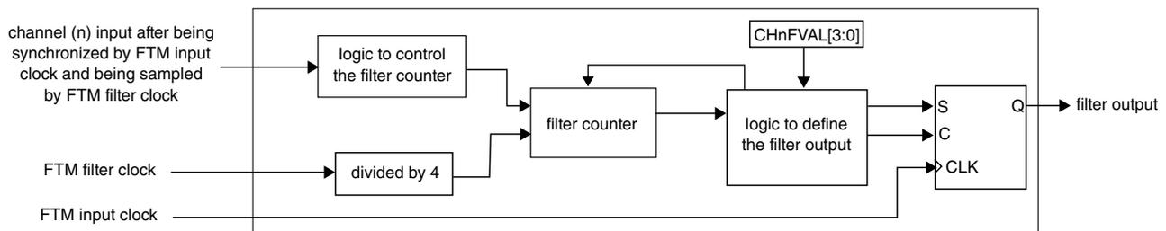
**Figure 47-17. Channel Input Filter when FLTPS[3:0]  $\neq$  0**
