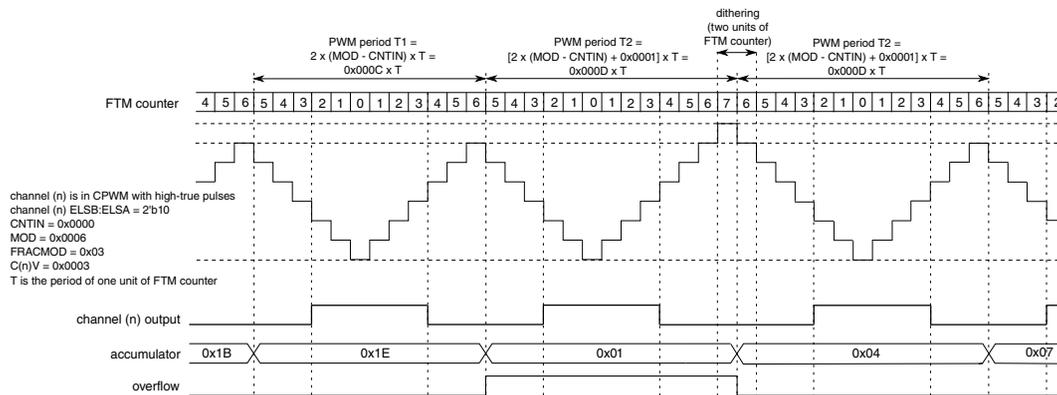
Figure 47-119. PWM Period Dithering with Up-Down Counting
