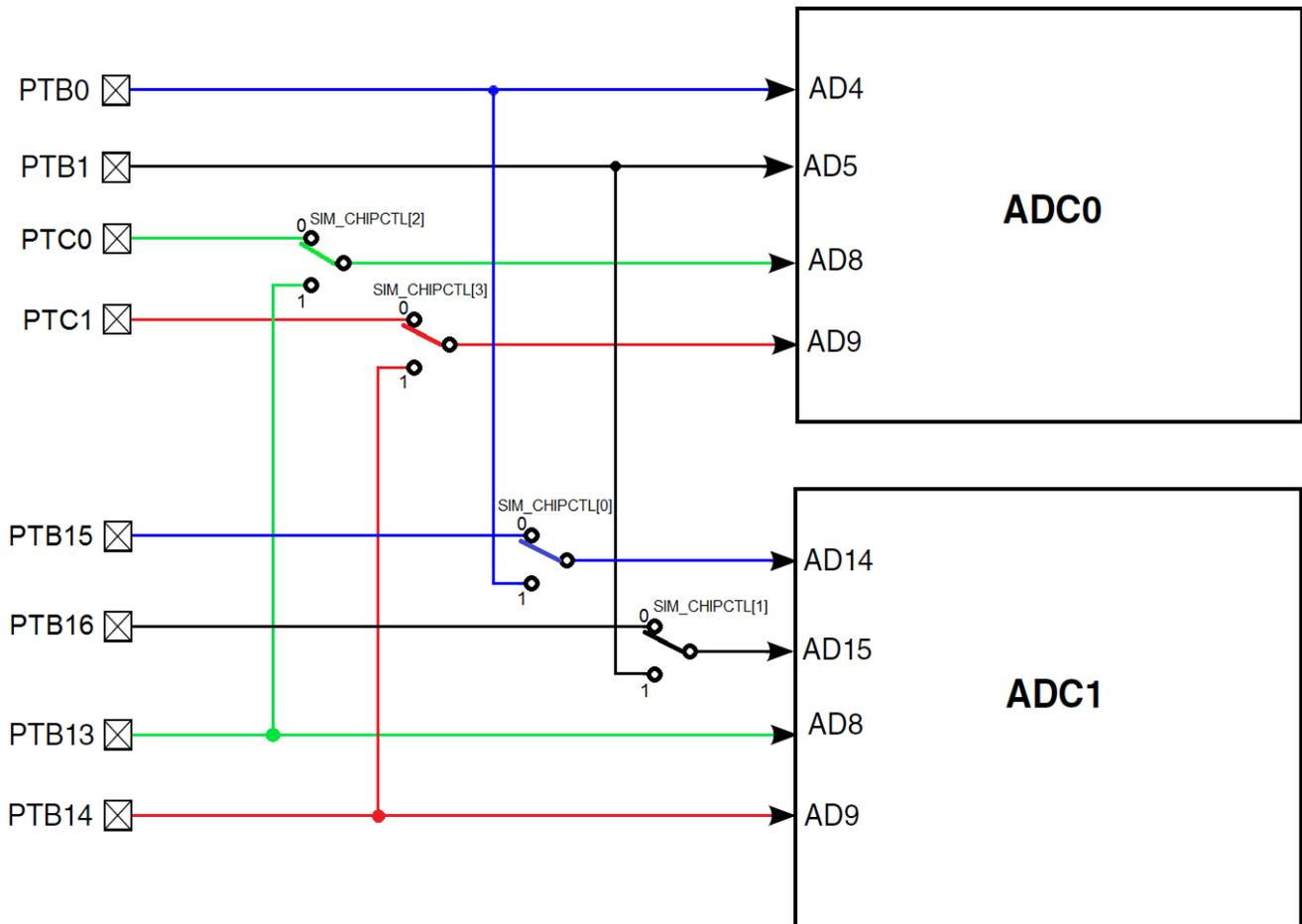
**Figure 43-1. ADC0 and ADC1 hardware interleaved channels integration**
