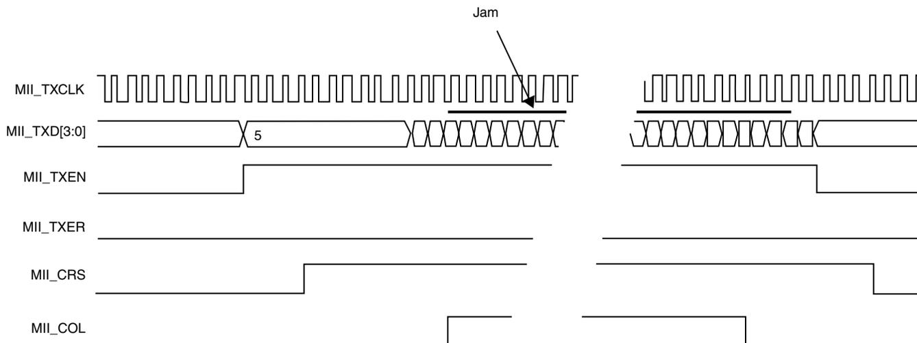
Figure 57-24. MII transmit operation — transmission with collision
