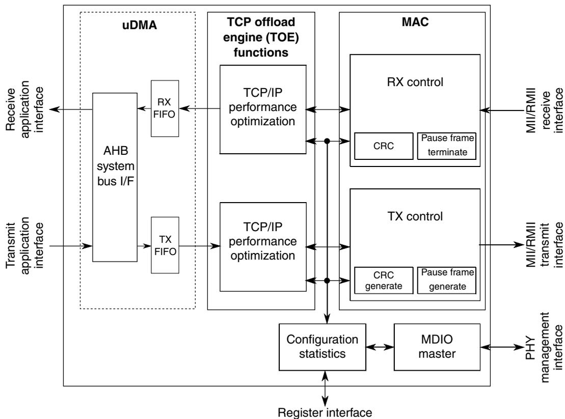
Figure 57-1. Ethernet MAC-NET core block diagram
