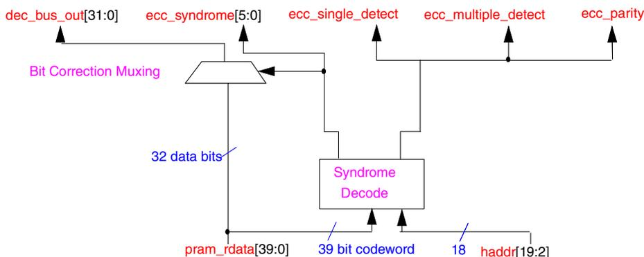
Figure 32-2. Block Diagram: 39-bit ECC Decode
