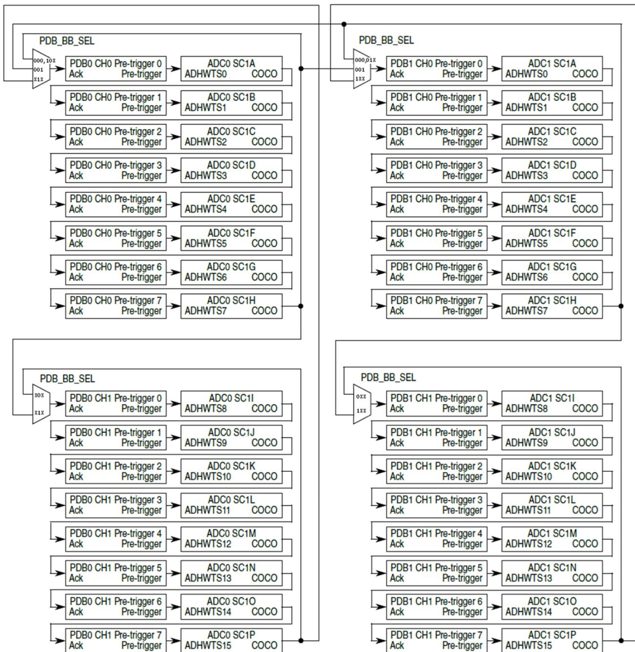
Figure 46-5. PDB-ADC back to back connection (Part 1 of 2)
