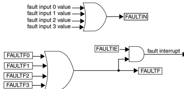
**Figure 47-83. FAULTF and FAULTIN bits and fault interrupt**
