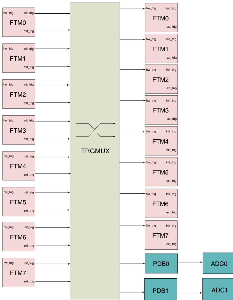
Figure 47-2. Hardware triggers
