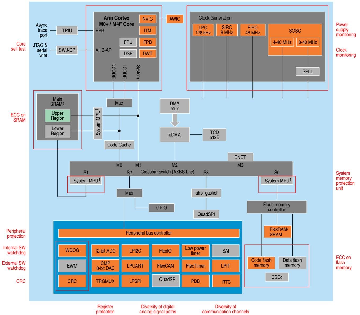
**Figure 6-2. S32K1xx safety block diagram**
