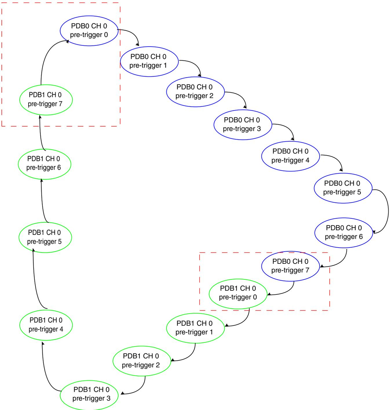
**Figure 46-3. PDB back-to-back chain forming PDB0-PDB1 ring**
