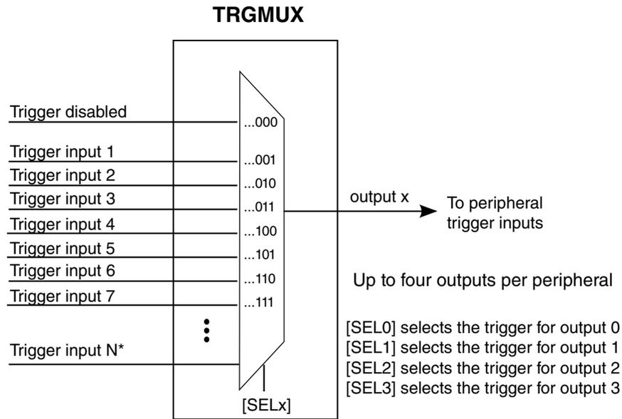
\* Up to 255 trigger inputs may be available for SEL0, SEL1, and SEL2. For SEL3, up to 127 trigger inputs may be available. When the number of trigger inputs is 255, SEL3 is not available and becomes reserved. See the chip-specific TRGMUX information for the maximum number of trigger inputs supported on this device.
