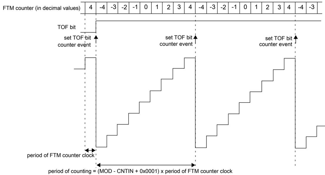
**Figure 47-8. Example of FTM up and signed counting**
