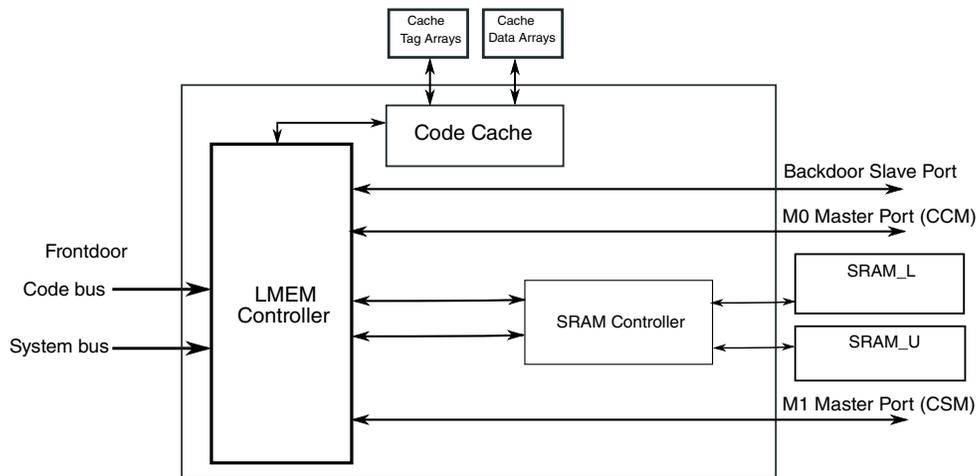
Figure 33-2. LMEM Interface to SRAM
