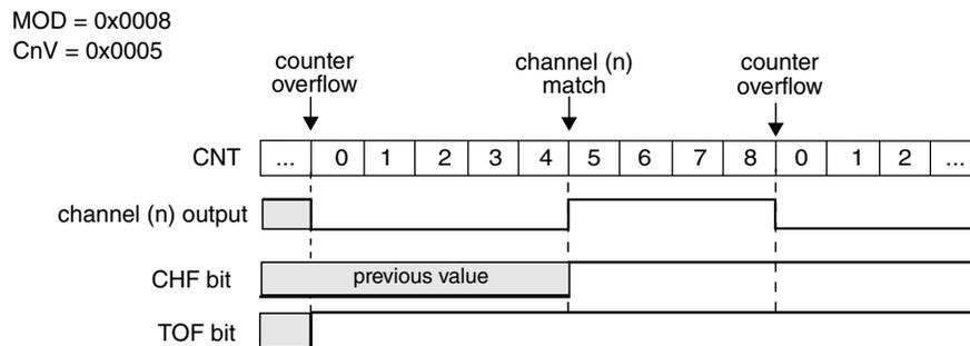
**Figure 47-26. EPWM signal with ELSB:ELSA = X:1**
