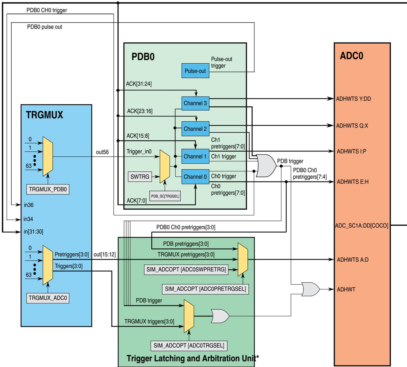
\* The block depicts simplified schematic and doesn't show detailed latching. See section 'Trigger Latching and Arbitration' of ADC chapter for details
