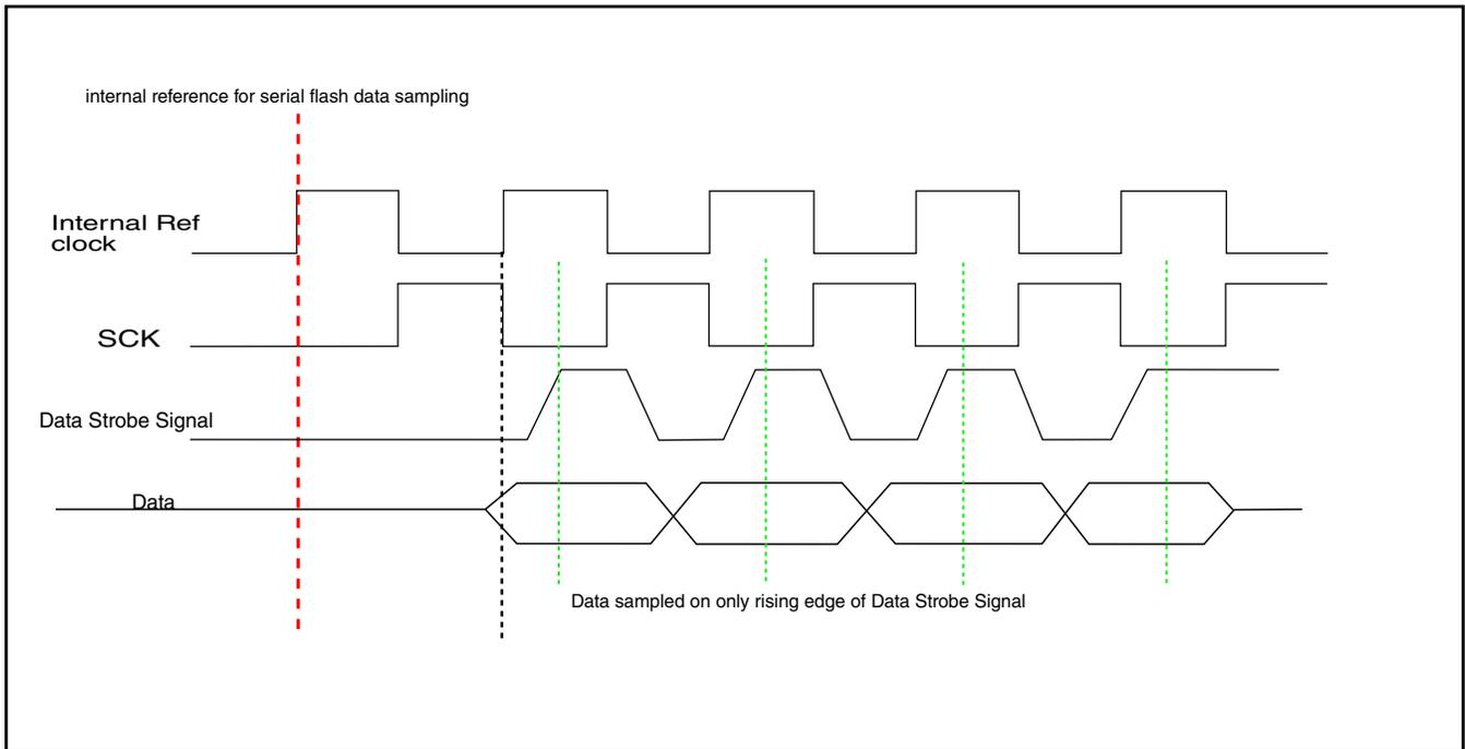
**Figure 38-10. Data Strobe functionality in SDR mode**
