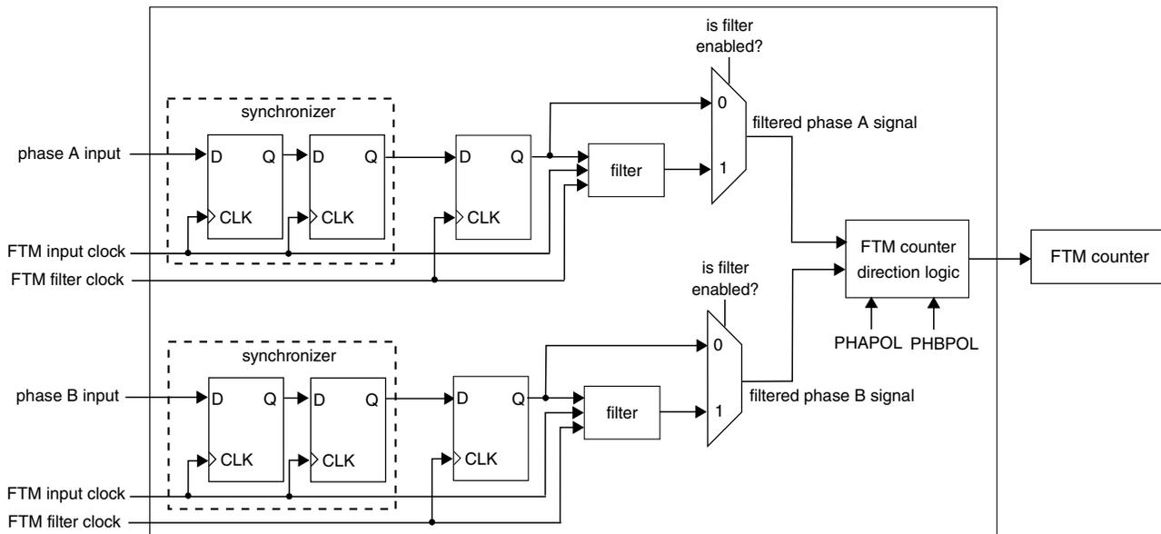
**Figure 47-102. Diagram for Quadrature Decoder when FLTIPS[3:0] ≠ 0**
