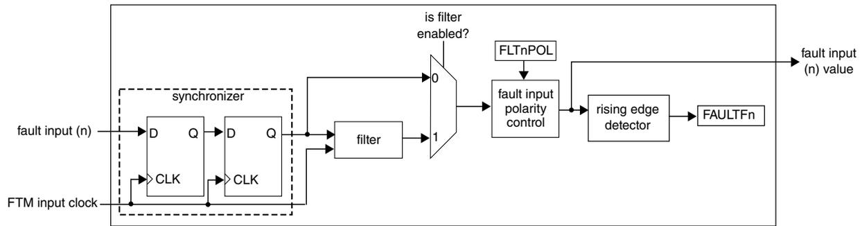
**Figure 47-81. Diagram for Fault Control when FLTPS[3:0] = 0**
