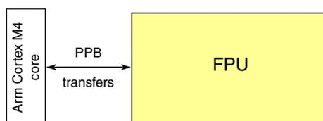
**Figure 7-4. FPU configuration****Table 7-9. Reference links to related information**
