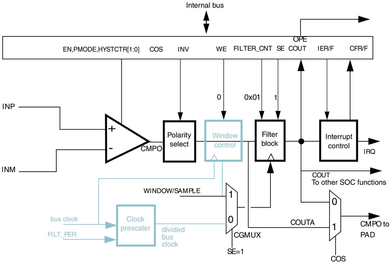
**Figure 45-5. Sampled, Non-Filtered (# 3A): sampling point externally driven**
