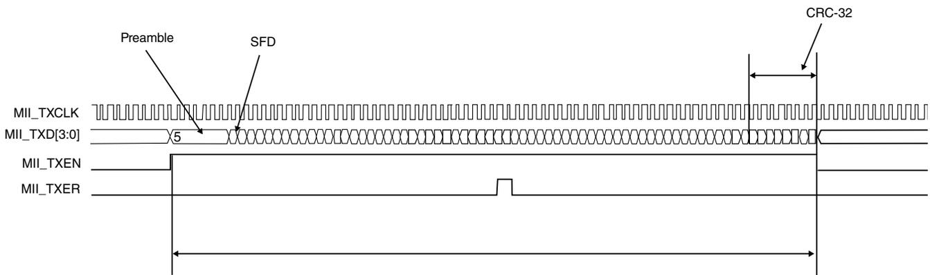
**Figure 57-23. MII transmit operation — errored frame**
