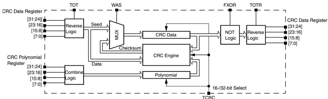
Figure 24-1. Programmable cyclic redundancy check (CRC) block diagram
