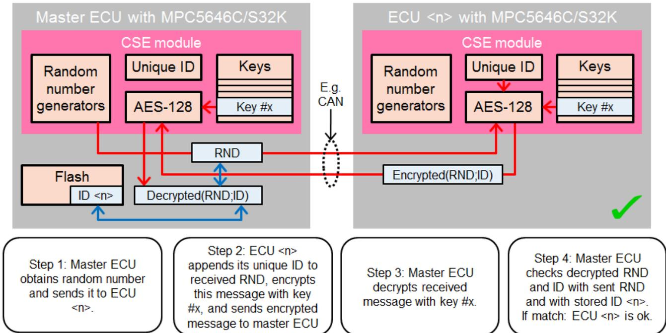
Figure 5-4. Component protection
