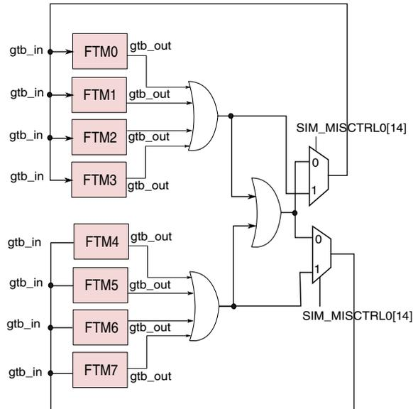
Figure 47-5. FTM global time base system interconnection
