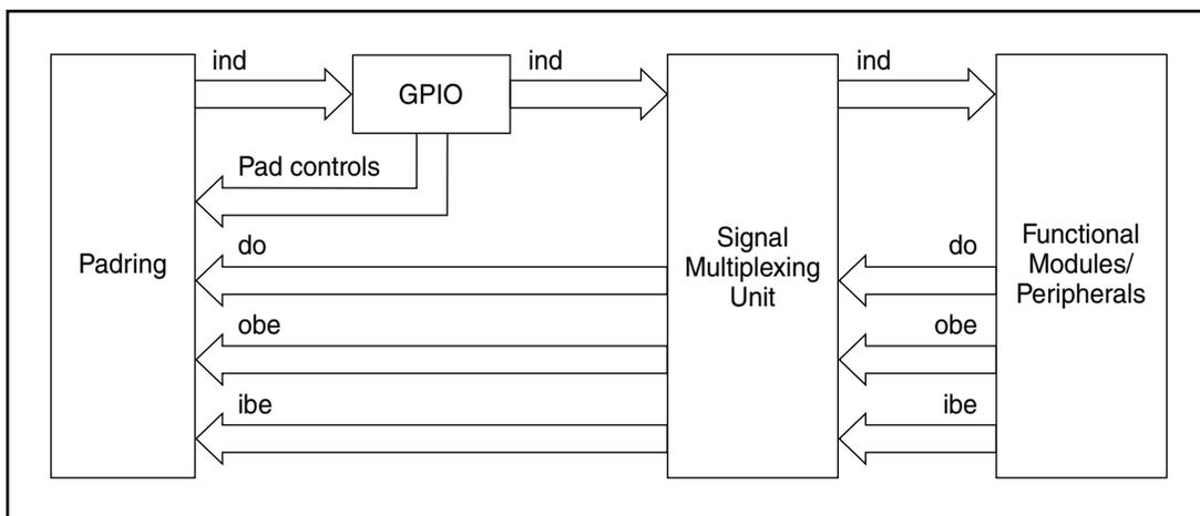
Figure 4-1. Signal Multiplexing
