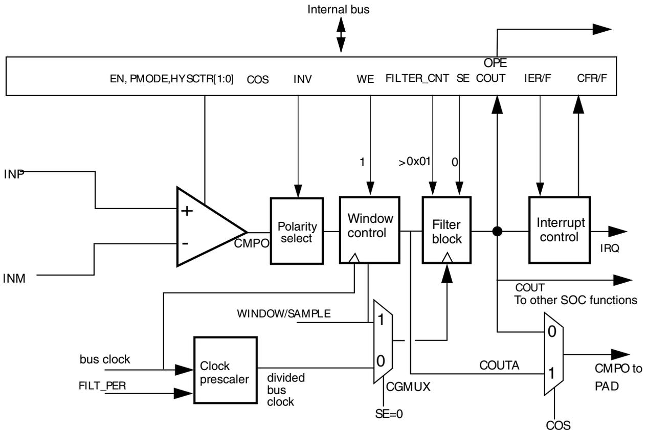
**Figure 45-13. Windowed/Filtered mode**
