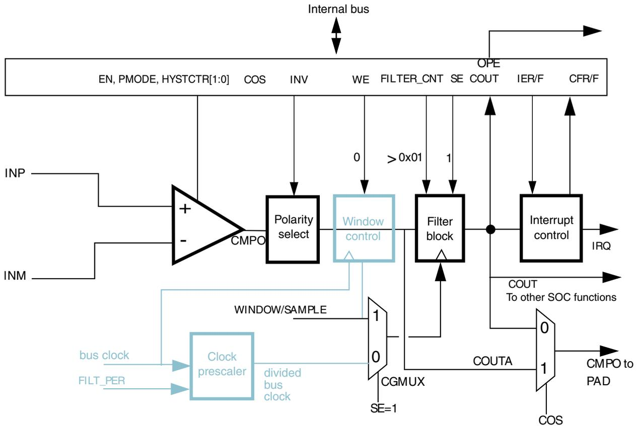
Figure 45-8. Sampled, Filtered (# 4A): sampling point externally driven
