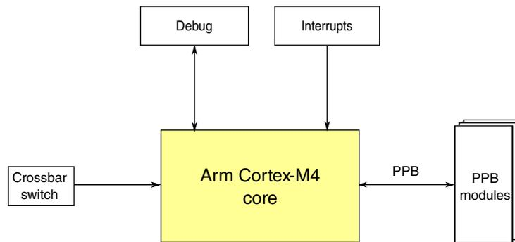
**Figure 7-1. Core configuration**
