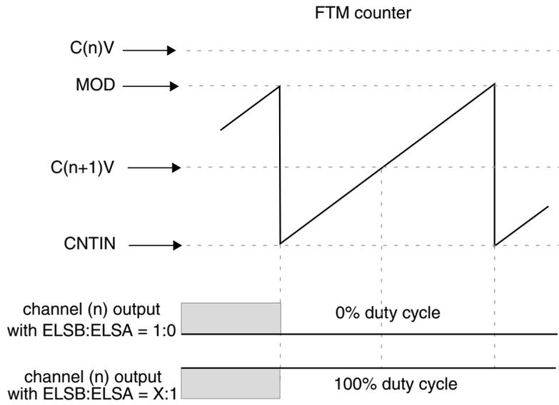
**Figure 47-43. Channel (n) output if  $(C(n)V > MOD)$  and  $(CNTIN < C(n+1)V < MOD)$**
