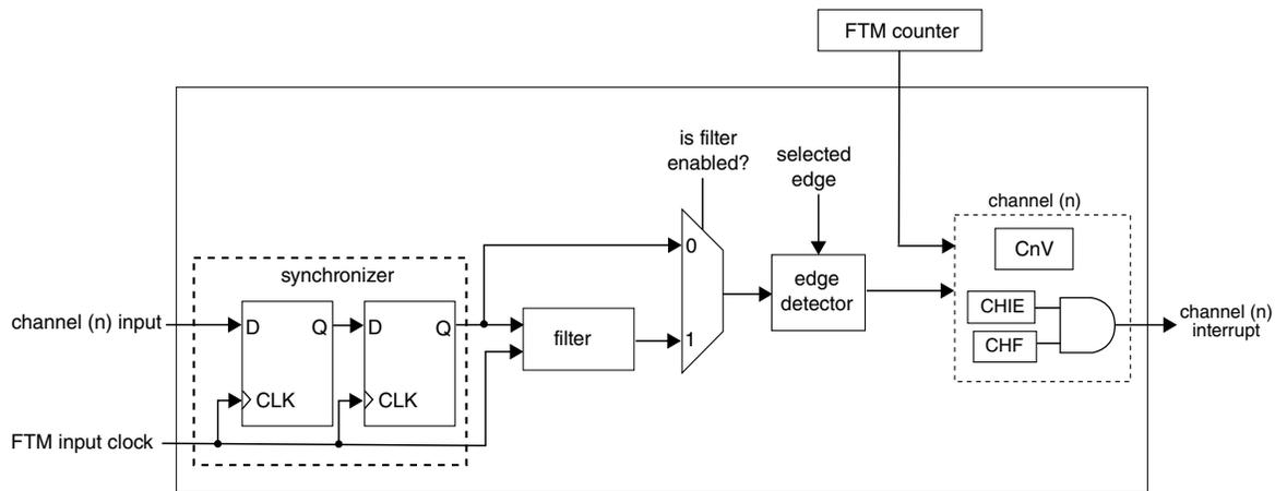
Note: The filter is only available for the channels 0, 1, 2, and 3 inputs.
