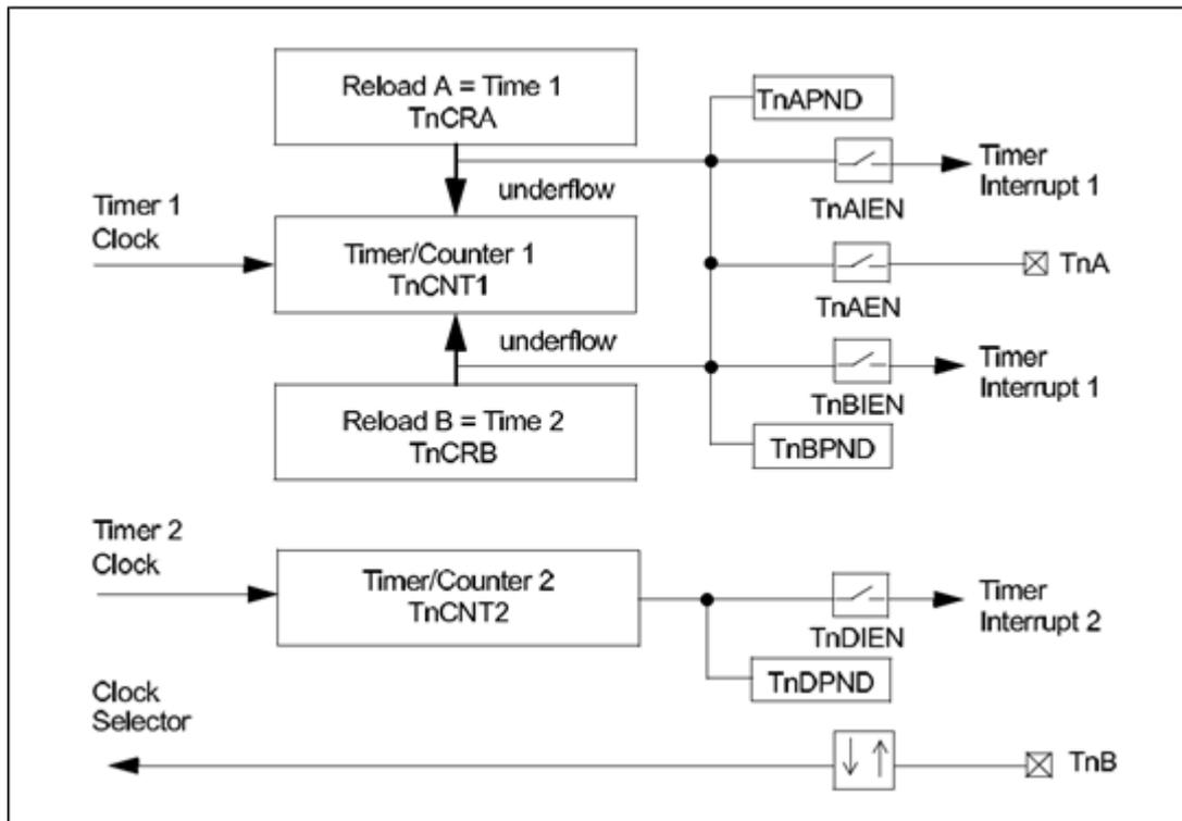
In this mode, the timer toggles the TnA output upon underflow which is connected to PWMx pin of the BlueNRG1. This generates a clock signal on TnA with the width and duty cycle controlled by the values stored in the TnCRB and TnCRB registers.
