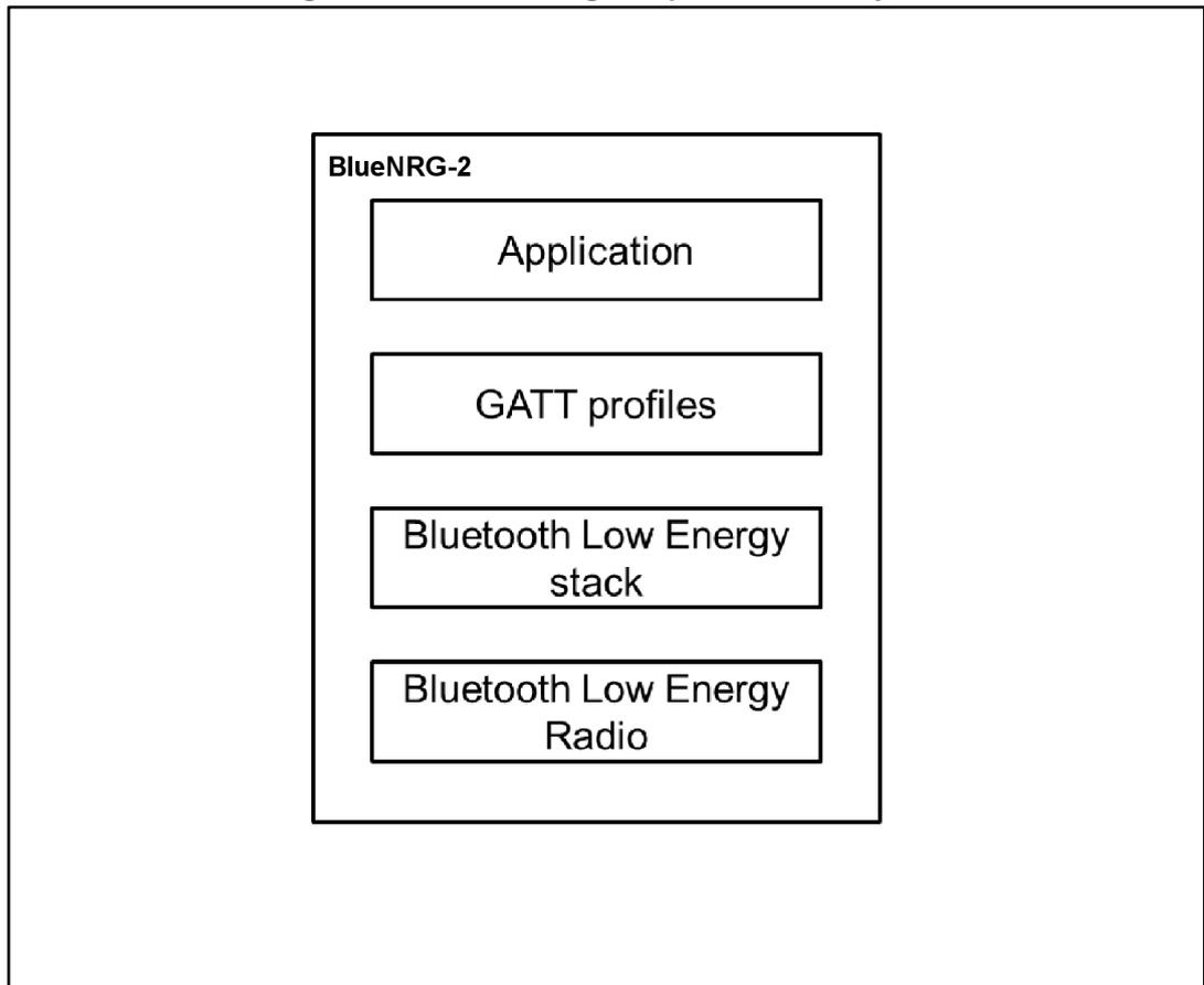
The BlueNRG-2 can be configured to operate as a network coprocessor. In this case, dedicated firmware is provided to support the interface with an external application processor. The whole Bluetooth low energy stack runs in the BlueNRG-2; the GATT profiles are provided to run in the application processor together with the application code. [Figure 3: "BlueNRG-2 single chip RF software layers"](#) shows the network processor RF software layers.
