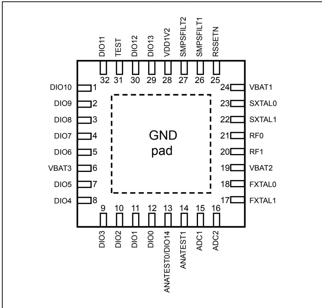
Figure 22: BlueNRG-2 pin out top view (QFN48)
