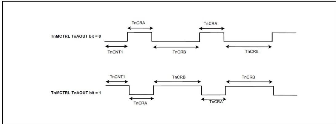
When started the first time, the TnCNT1 starts with value preprogrammed in the register and count down at the clock rate selected by the Timer/Counter 1 clock selector (TnCKC register). When an underflow occurs, the TnCNT1 is reloaded alternatively with TnCRB and TnCRA registers (in this order) and counting proceeds downward from the loaded value.
