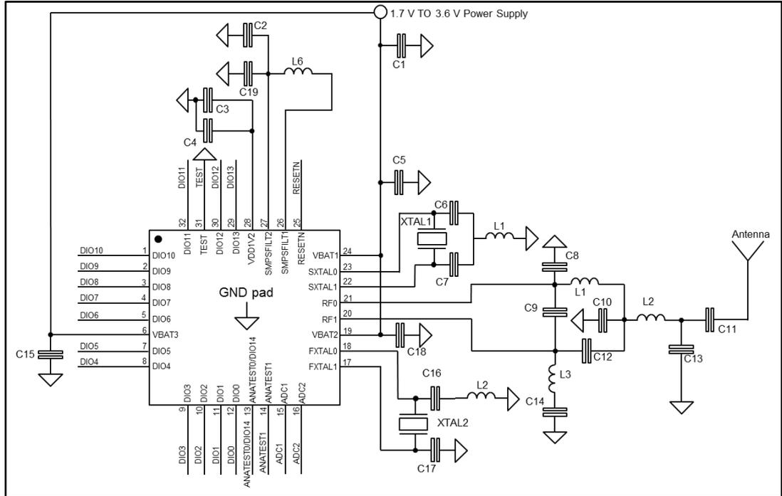
**Figure 26: Application circuit: non-active DC-DC converter QFN32 package**
