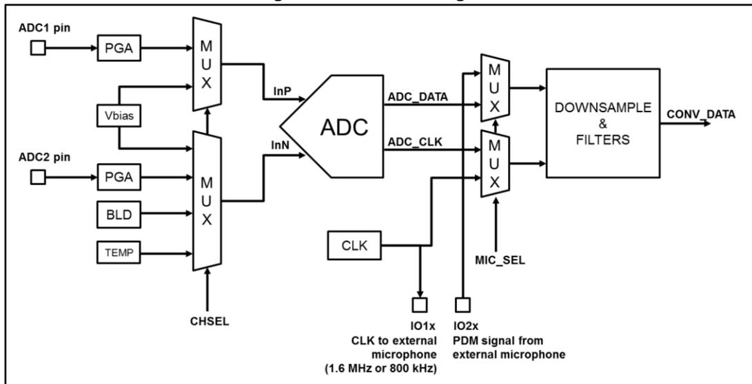
Several channels are available for conversion, the CHSEL selects the channel according to [Table 27: "ADC channels"](#).
