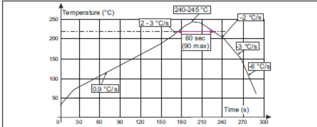
**Table 231: Flip Chip CSP (2.71 x 2.58 x 0.5 pitch 0.4 mm) package reflow profile recommendation**
