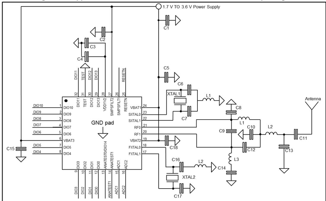
Figure 27: Application circuit: active DC-DC converter WCSP34 package
