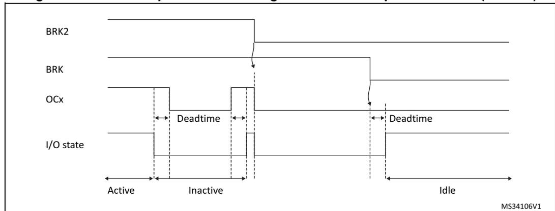
Figure 101. PWM output state following BRK assertion (OSS1=0)
