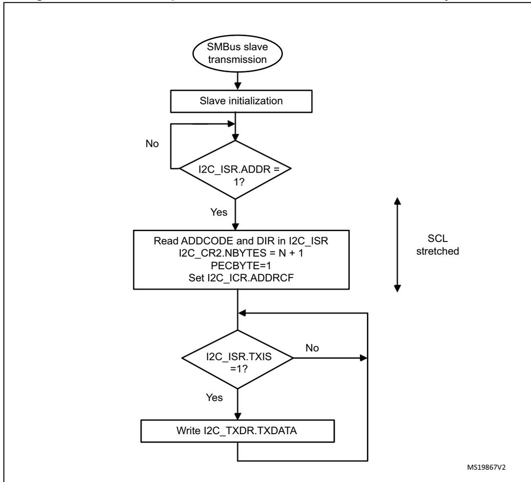
Figure 236. Transfer bus diagrams for SMBus slave transmitter (SBC = 1)
