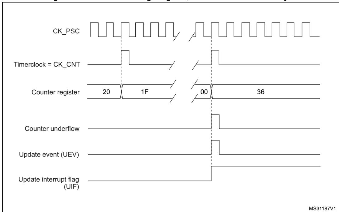
Figure 128. Counter timing diagram, Update event
