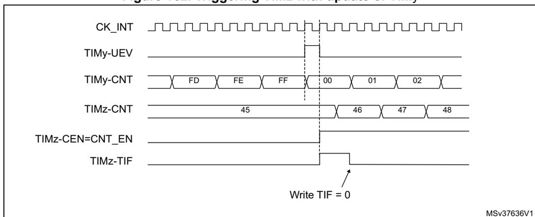
As in the previous example, both counters can be initialized before starting counting. [Figure 163](#) shows the behavior with the same configuration as in [Figure 162](#) but in trigger mode instead of gated mode (SMS=110 in the TIMz\_SMCR register).
