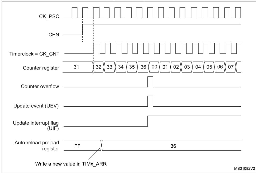
**Figure 188. Counter timing diagram, update event when ARPE=1 (TIMx\_ARR preloaded)**
