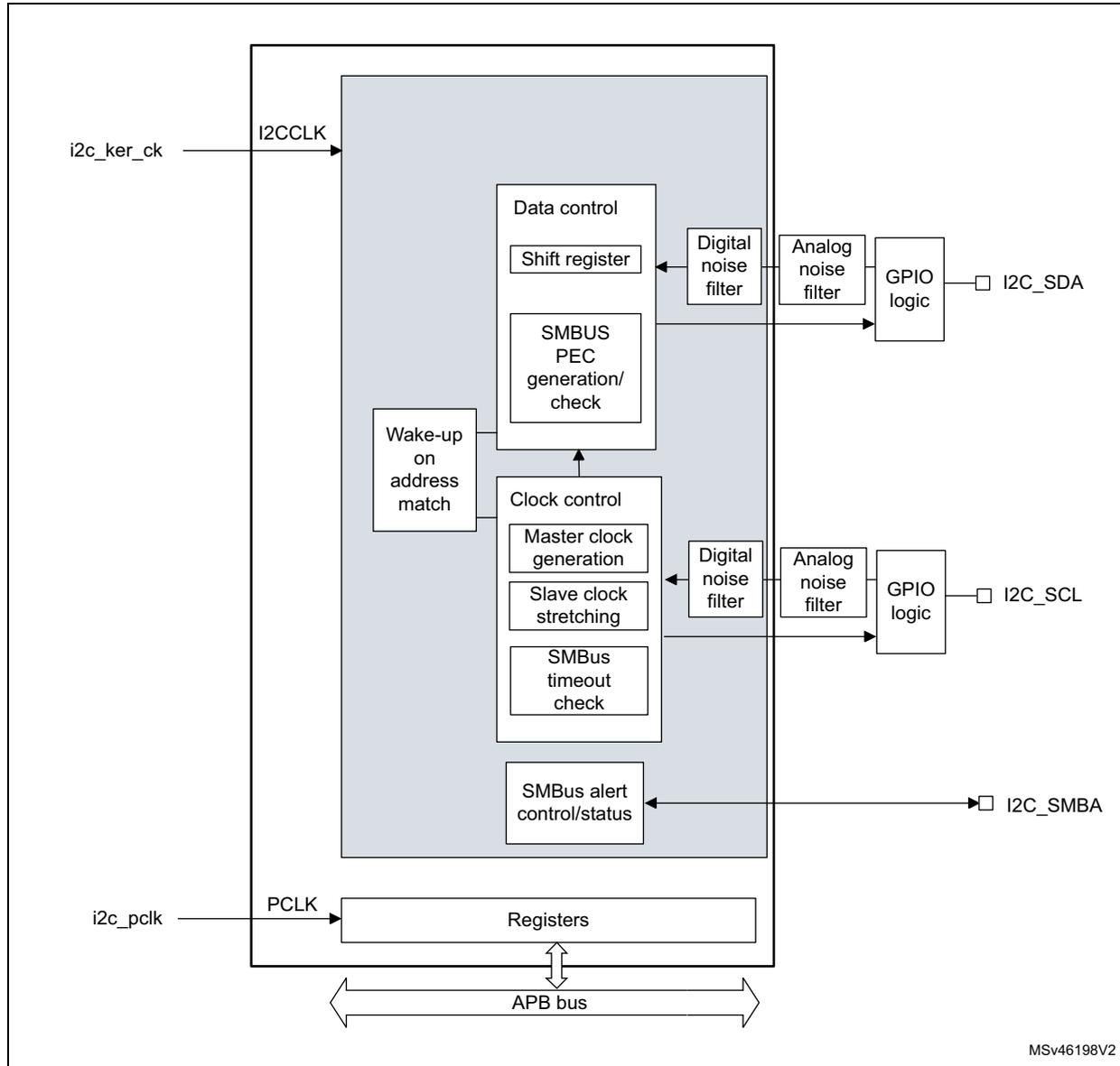
The I2C is clocked by an independent clock source, which allows the I2C to operate independently from the PCLK frequency.
