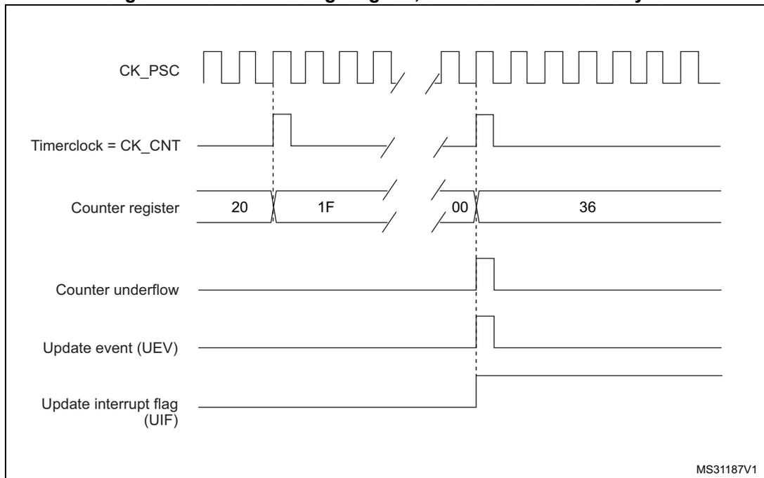
Figure 68. Counter timing diagram, update event when repetition counter is not used
