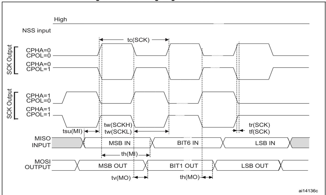
1. Measurement points are set at CMOS levels: 0.3 V<sub>DD</sub> and 0.7 V<sub>DD</sub>.
