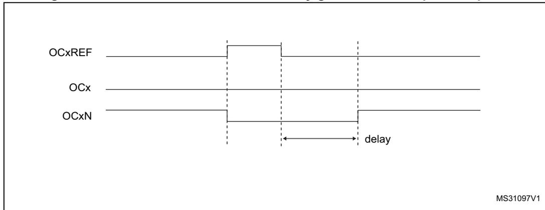
The dead-time delay is the same for each of the channels and is programmable with the DTG bits in the TIMx\_BDTR register. Refer to [Section 15.4.20: TIM1 break and dead-time register \(TIM1\\_BDTR\)](#) for delay calculation.
