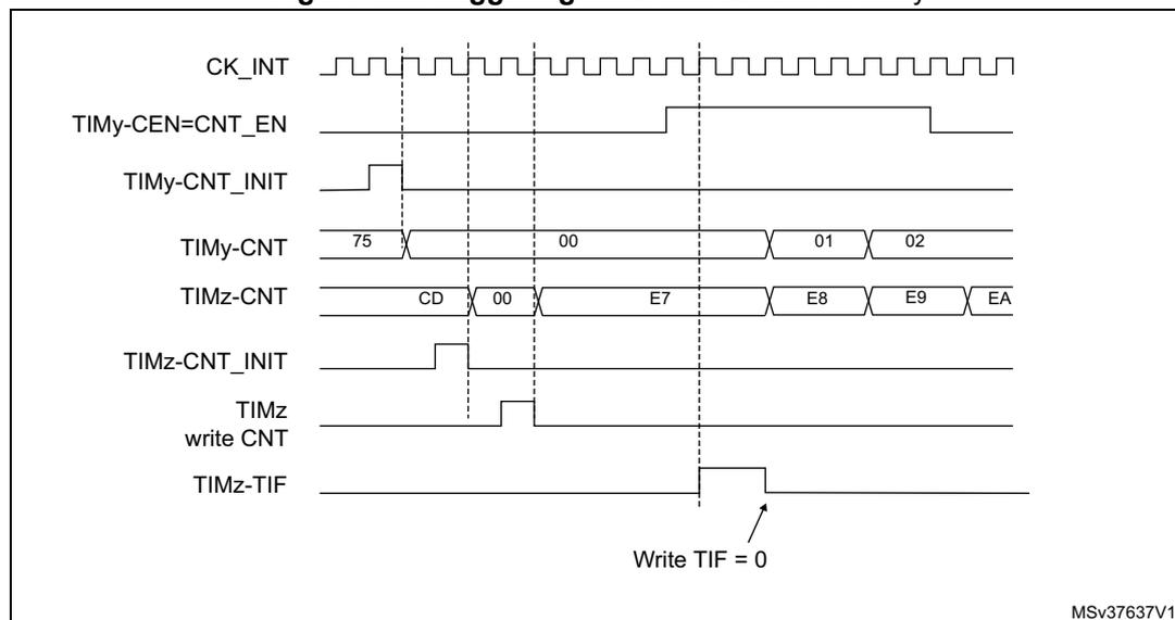
**Starting 2 timers synchronously in response to an external trigger**
