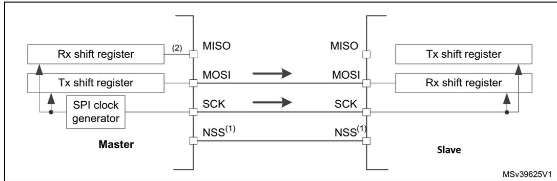
1. The NSS pins can be used to provide a hardware control flow between master and slave. Optionally, the pins can be left unused by the peripheral. Then the flow has to be handled internally for both master and slave. For more details see [Section 25.5.5: Slave select \(NSS\) pin management](#).
