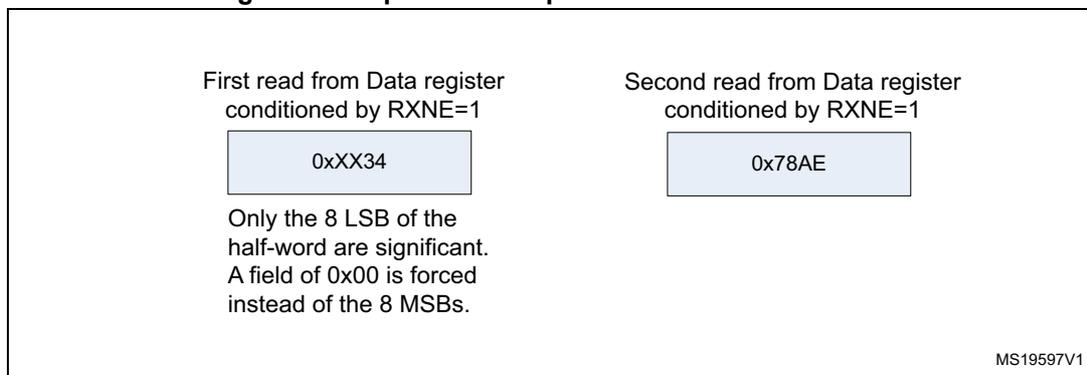
**Figure 298. LSB justified 16-bit extended to 32-bit packet frame**
