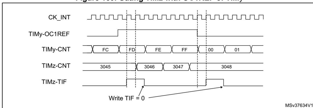
In the example in [Figure 160](#), the TIMz counter and prescaler are not initialized before being started. So they start counting from their current value. It is possible to start from a given value by resetting both timers before starting TIMy. Then any value can be written in the timer counters. The timers can easily be reset by software using the UG bit in the TIMx\_EGR registers.
