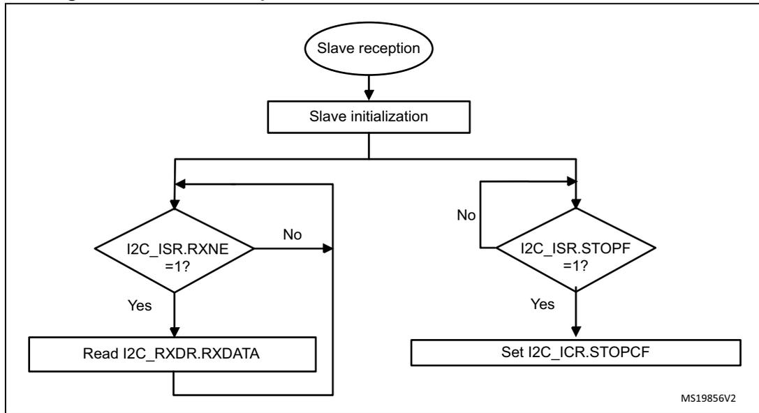
Figure 223. Transfer bus diagrams for I2C slave receiver (mandatory events only)
