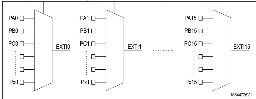
The EXTI's multiplexer outputs are available as output signals from the EXTI, to trigger other functional blocks. The EXTI multiplexer outputs are available independently of mask setting through the EXTI\_IMR and EXTI\_EMR registers.
