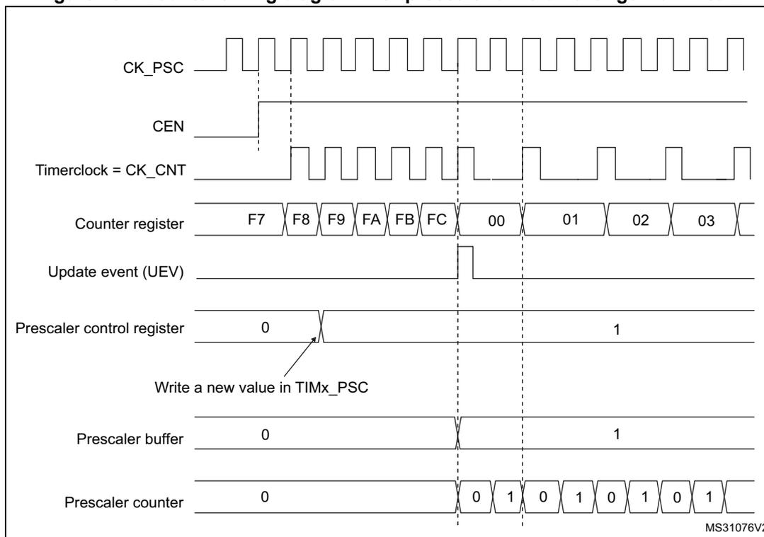
Figure 182. Counter timing diagram with prescaler division change from 1 to 4
