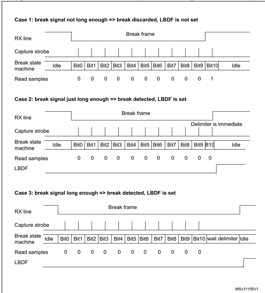
Figure 252. Break detection in LIN mode vs. Framing error detection
