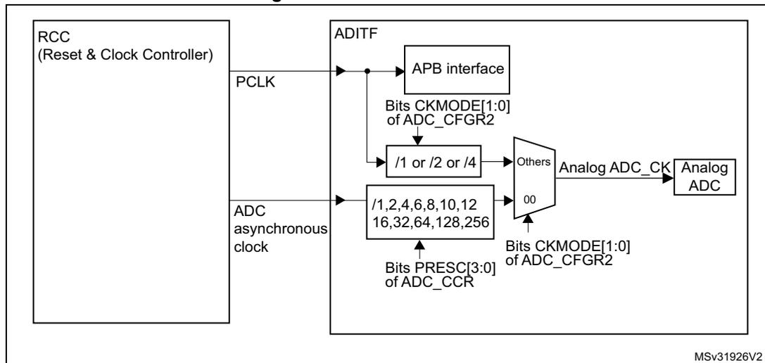
1. Refer to *Section Reset and clock control (RCC)* for how the PCLK clock and ADC asynchronous clock are enabled.
