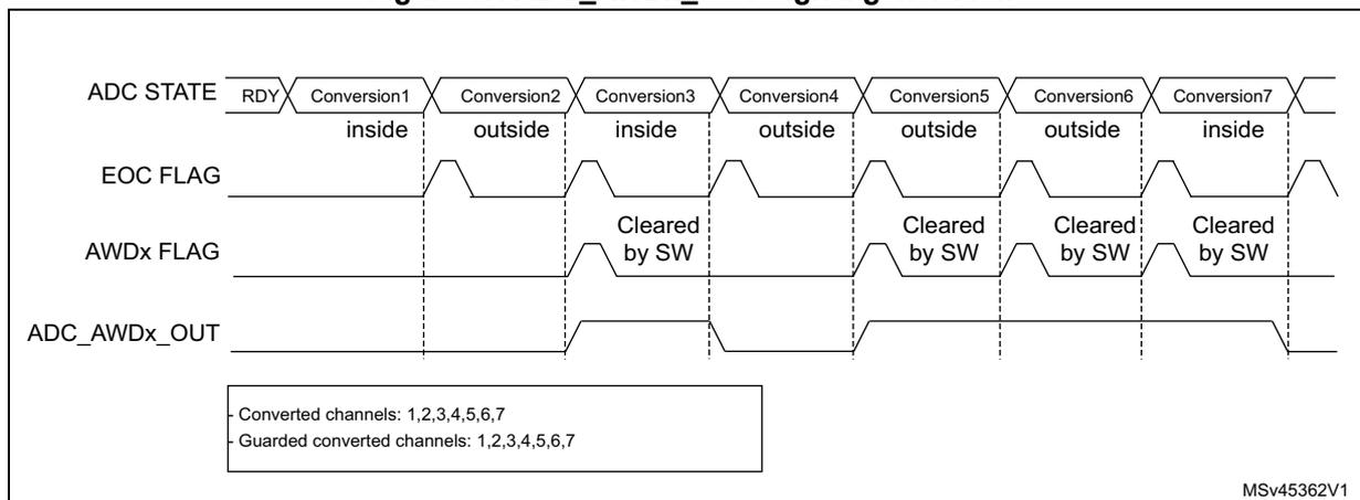
**Figure 48. ADC\_AWDx\_OUT signal generation (AWDx flag not cleared by software)**
