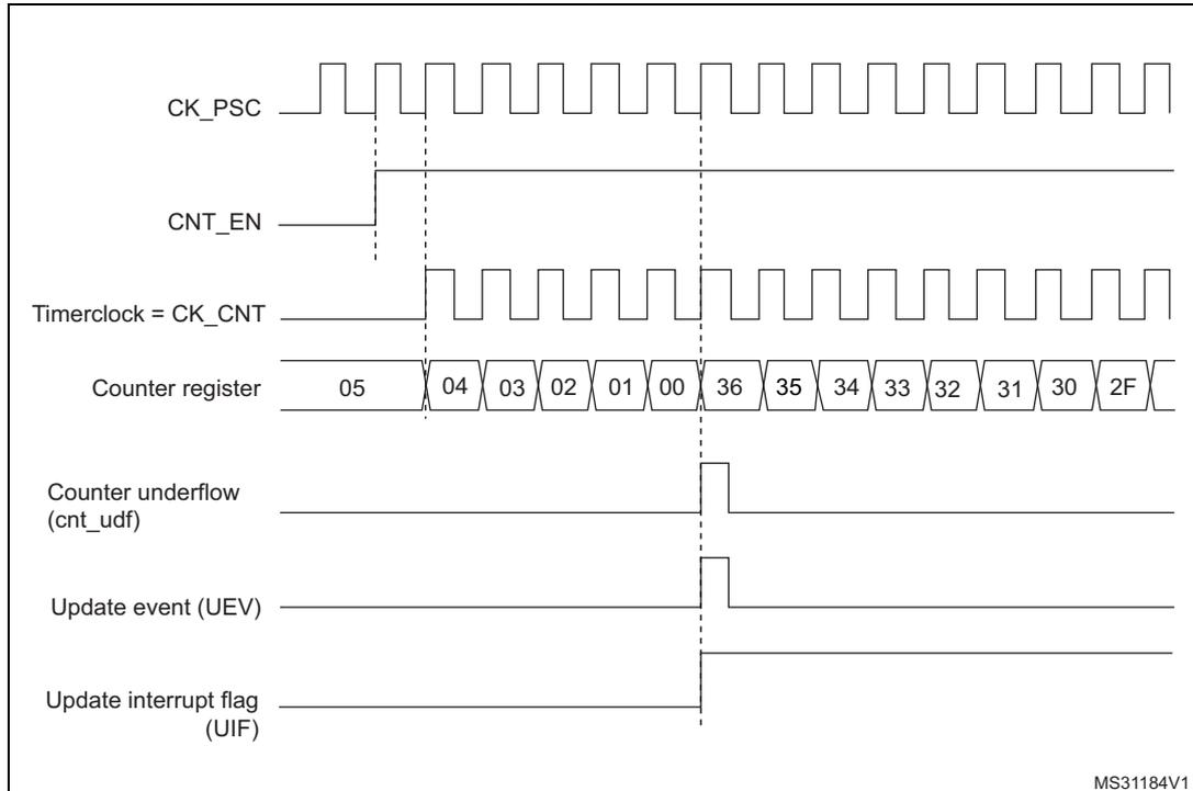
**Figure 125. Counter timing diagram, internal clock divided by 2**
