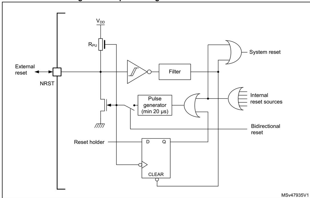
**Caution:** Upon power reset or wakeup from shutdown mode, the NRST pin is configured as Reset input/output and driven low by the system until it is reconfigured to the expected mode when the option bytes are loaded, in the fourth clock cycle after the end of  $t_{RSTEMPO}$  time (see datasheet).
