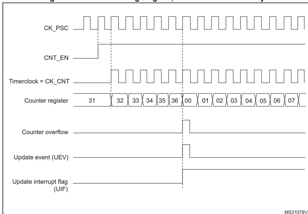
Figure 119. Counter timing diagram, internal clock divided by 2
