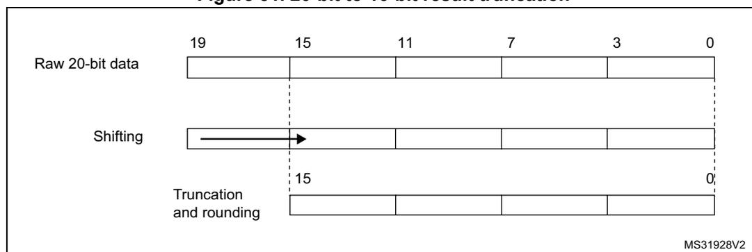
The [Figure 52](#) gives a numerical example of the processing, from a raw 20-bit accumulated data to the final 16-bit result.
