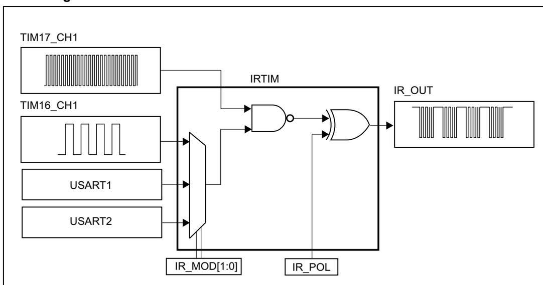
All standard IR pulse modulation modes can be obtained by programming the two timer output compare channels.
