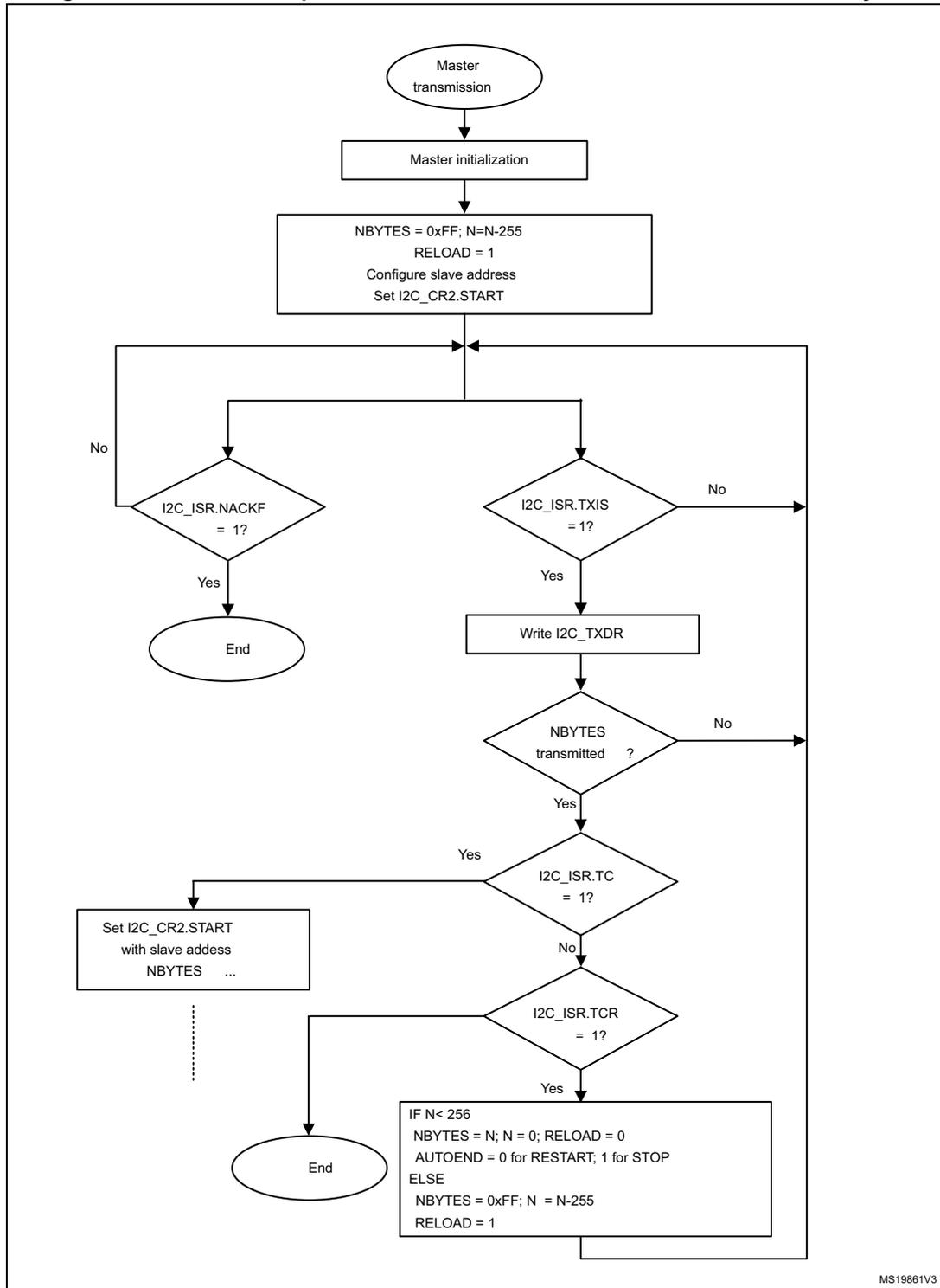
**Figure 230. Transfer bus diagrams for I2C master transmitter (mandatory events only)**
