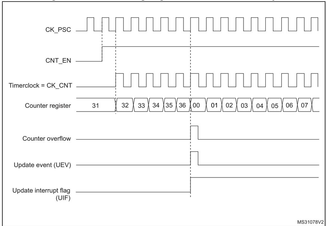
**Figure 184. Counter timing diagram, internal clock divided by 2**
