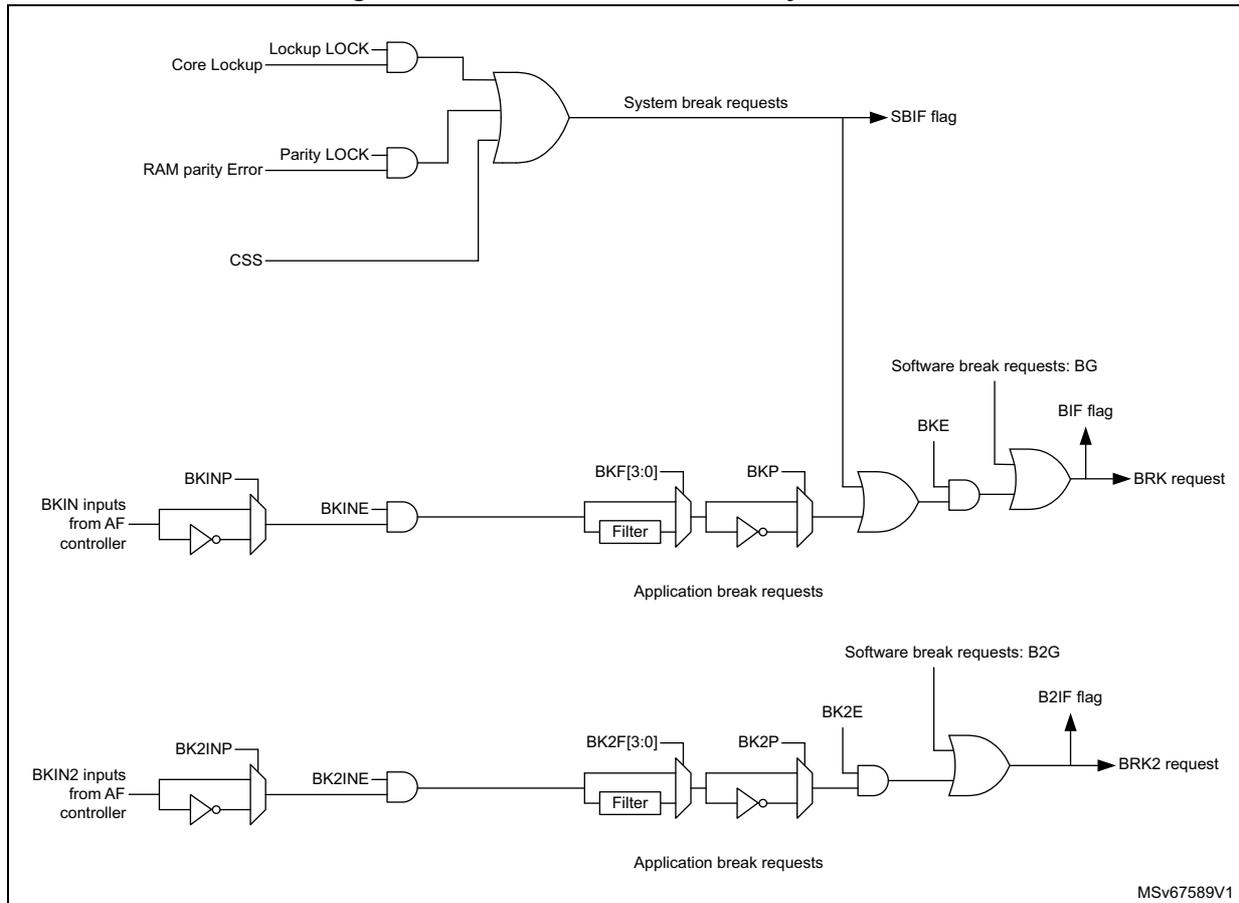
**Note:** An asynchronous (clockless) operation is only guaranteed when the programmable filter is disabled. If it is enabled, a fail safe clock mode (for example by using the CSS) must be used to guarantee that break events are handled.
