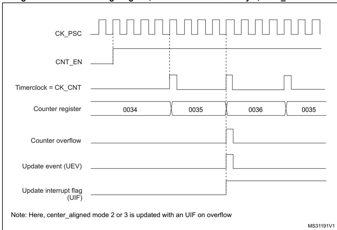
Figure 72. Counter timing diagram, internal clock divided by N
