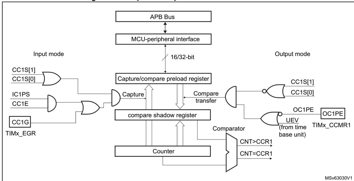
Figure 195. Output stage of capture/compare channel (channel 1)
