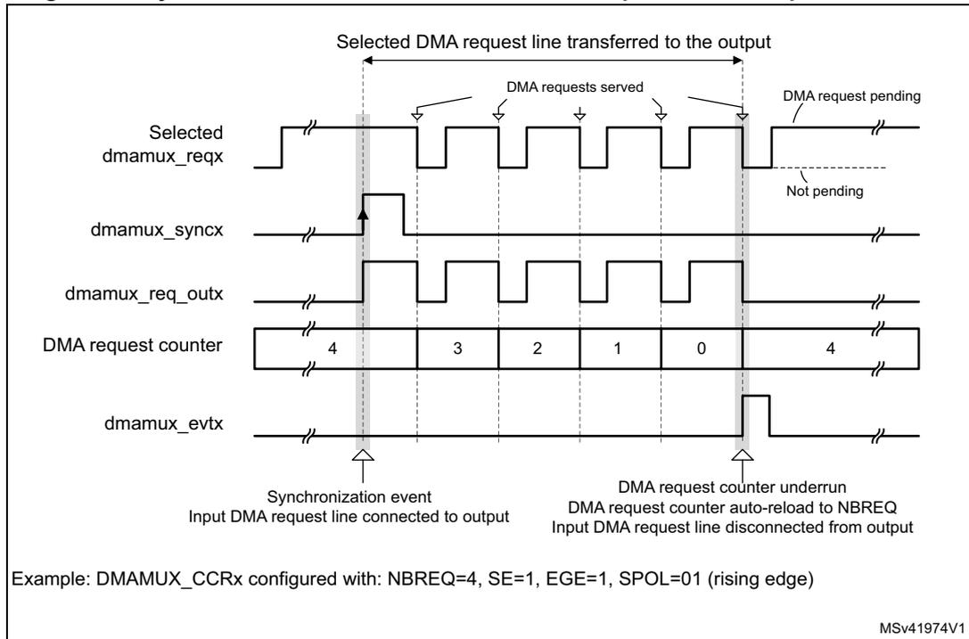
Figure 22. Event generation of the DMA request line multiplexer channel
