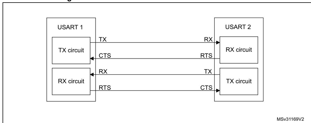
RS232 RTS and CTS flow control can be enabled independently by writing the RTSE and CTSE bits to '1' in the USART\_CR3 register.
