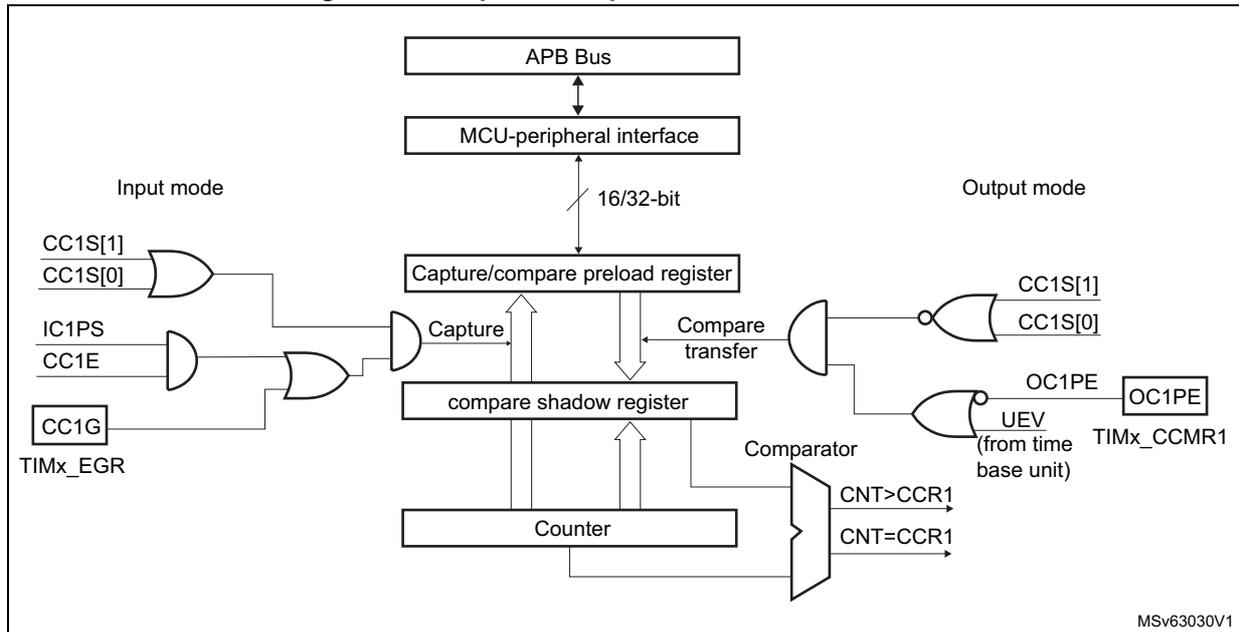
Figure 177. Output stage of capture/compare channel (channel 1)
