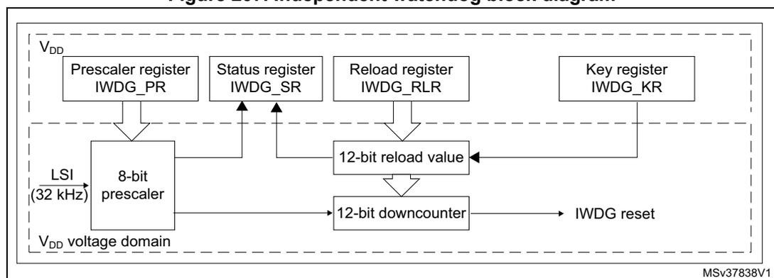
1. The register interface is located in the  $V_{DD}$  voltage domain. The watchdog function is located in the  $V_{DD}$  voltage domain, still functional in Stop and Standby modes.
