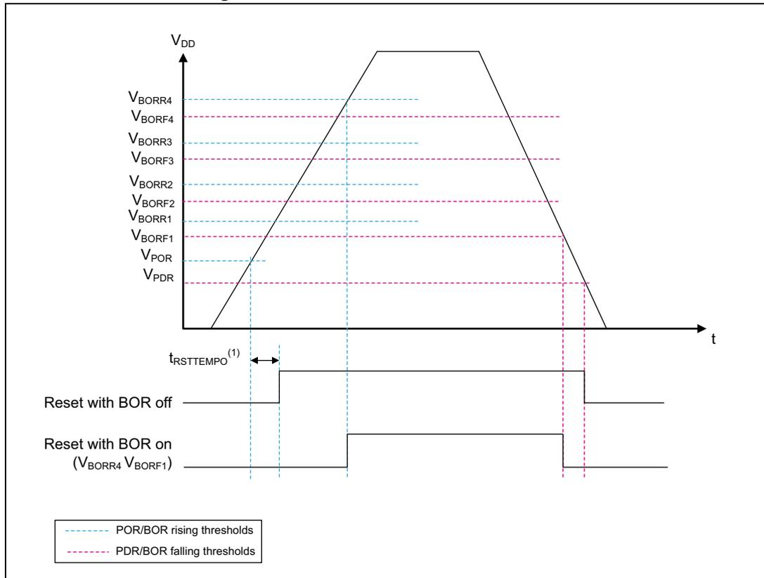
1. The reset temporization  $t_{RSTTEMPO}$  starts when  $V_{DD}$  crosses  $V_{POR}$  threshold, indifferently from the configuration of the BOR Option bits.
