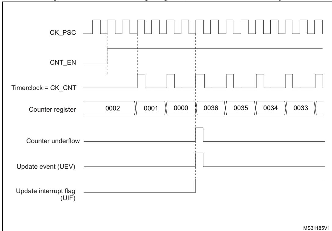
Figure 126. Counter timing diagram, internal clock divided by 4
