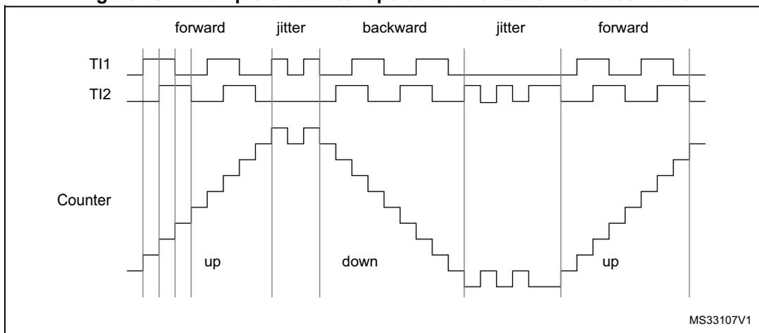
Figure 153 gives an example of counter behavior when TI1FP1 polarity is inverted (same configuration as above except CC1P=1).
