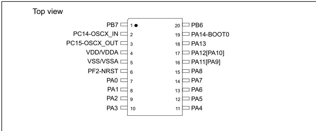
Figure 6. STM32C011Fxu UFQFPN20 pinout
