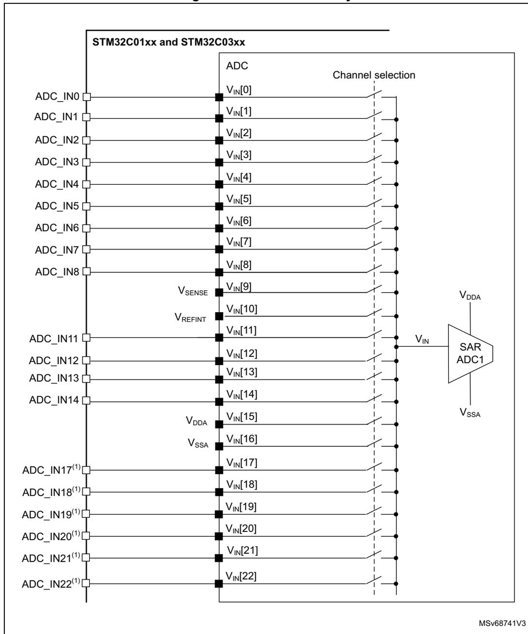
1. ADC\_IN17 to ADC\_IN22 are available only on STM32C03xx devices.
