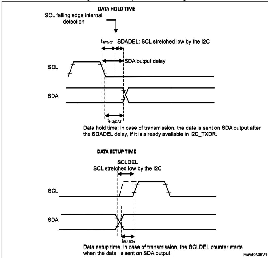
When the SCL falling edge is internally detected, a delay ( $t_{SDADEL}$ , impacting the hold time  $t_{HD,DAT}$ ) is inserted before sending SDA output:  $t_{SDADEL} = SDADEL \times t_{PRESC} + t_{I2CCLK}$ , where  $t_{PRESC} = (PRESC + 1) \times t_{I2CCLK}$ .
