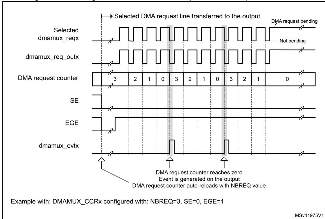
If EGE is enabled, the multiplexer channel generates a channel event, as a pulse of one AHB clock cycle, when its DMA request counter is automatically reloaded with the value of the programmed NBREQ field, as shown in [Figure 21](#) and [Figure 22](#).
