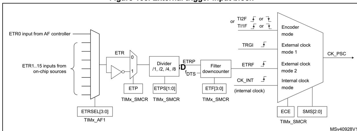
For example, to configure the upcounter to count each 2 rising edges on ETR, use the following procedure:
