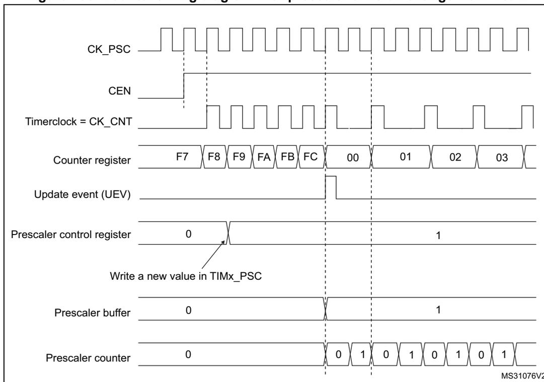
Figure 167. Counter timing diagram with prescaler division change from 1 to 4
