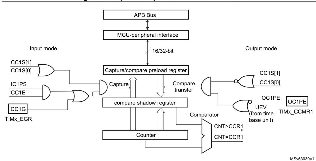
Figure 85. Output stage of capture/compare channel (channel 1, idem ch. 2 and 3)
