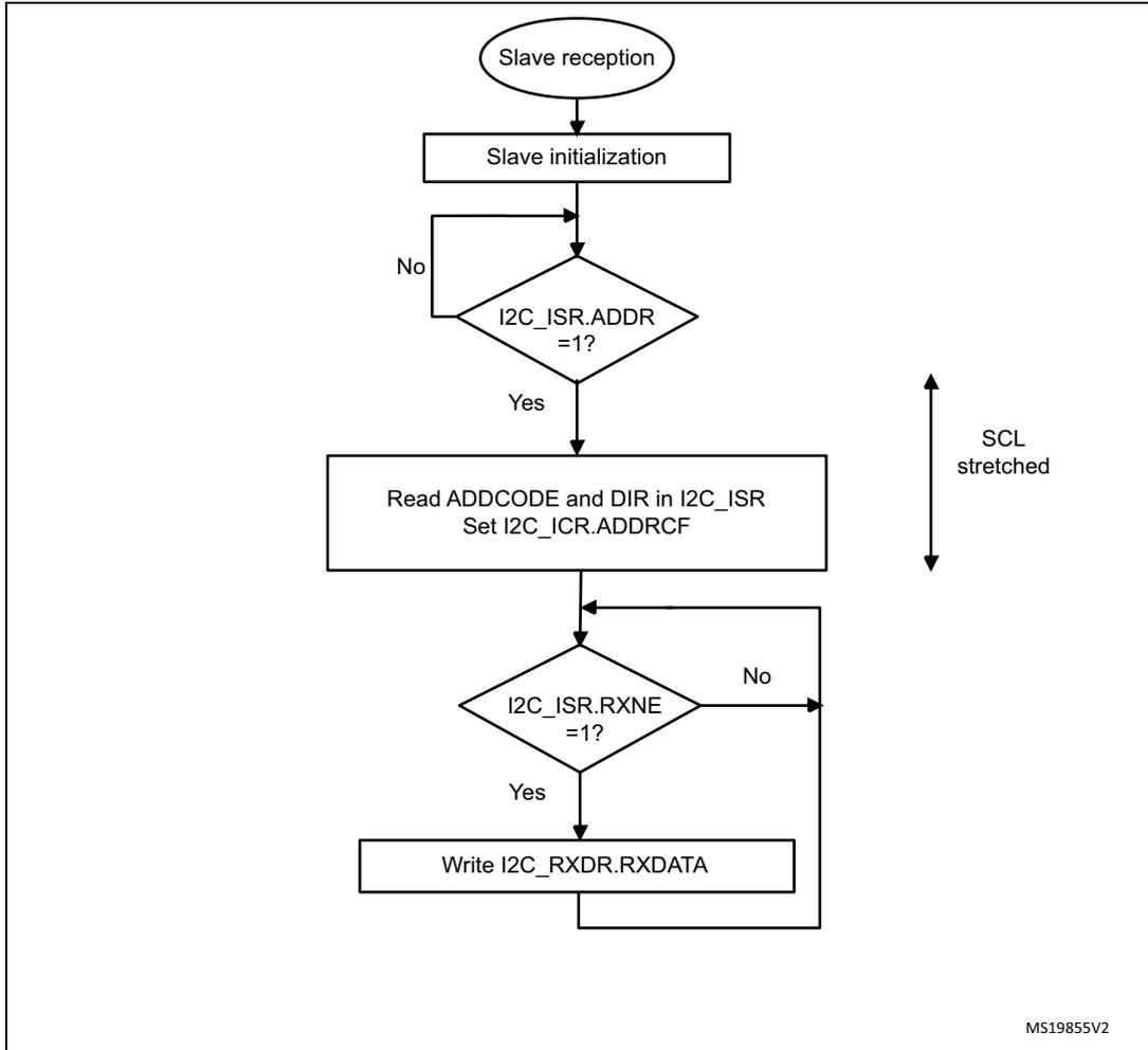
Figure 222. Transfer sequence flow for slave receiver with NOSTRETCH = 1
