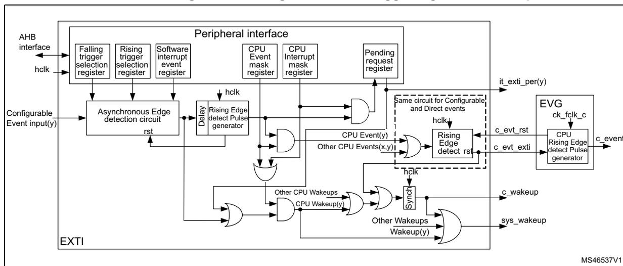
The software interrupt event register allows triggering configurable events by software, writing the corresponding register bit, irrespective of the edge selection setting.
