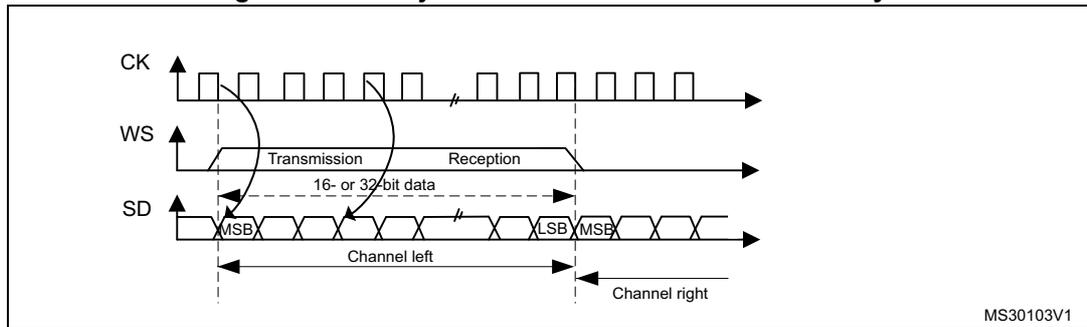
**Figure 295. LSB justified 24-bit frame length**
