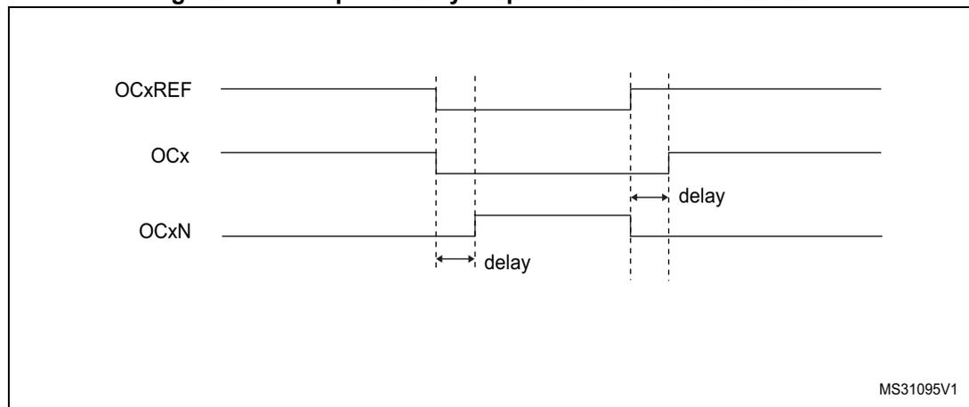
**Figure 199. Dead-time waveforms with delay greater than the negative pulse.**
