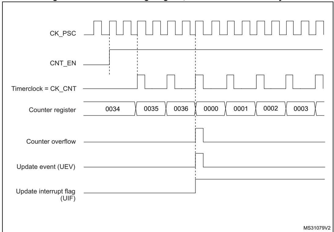
Figure 185. Counter timing diagram, internal clock divided by 4
