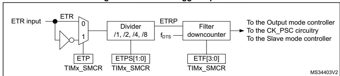
The ETR input comes from multiple sources: input pins (default configuration) and analog watchdogs. The selection is done with the ETRSEL[3:0] bitfield.
