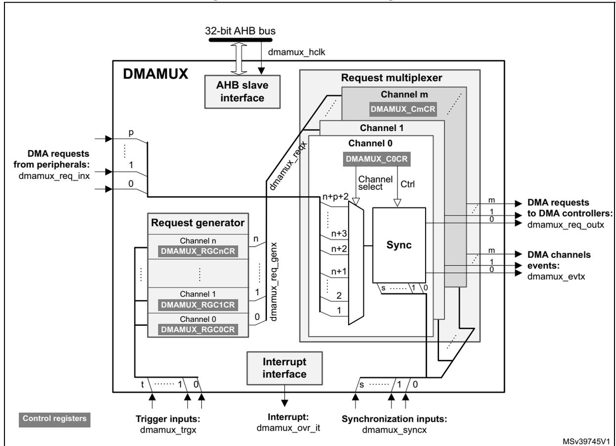
DMAMUX features two main sub-blocks: the request line multiplexer and the request line generator.
