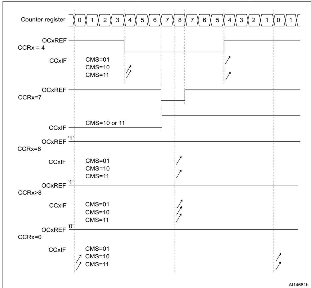
**Hints on using center-aligned mode**
