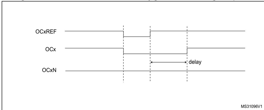
**Figure 200. Dead-time waveforms with delay greater than the positive pulse.**
