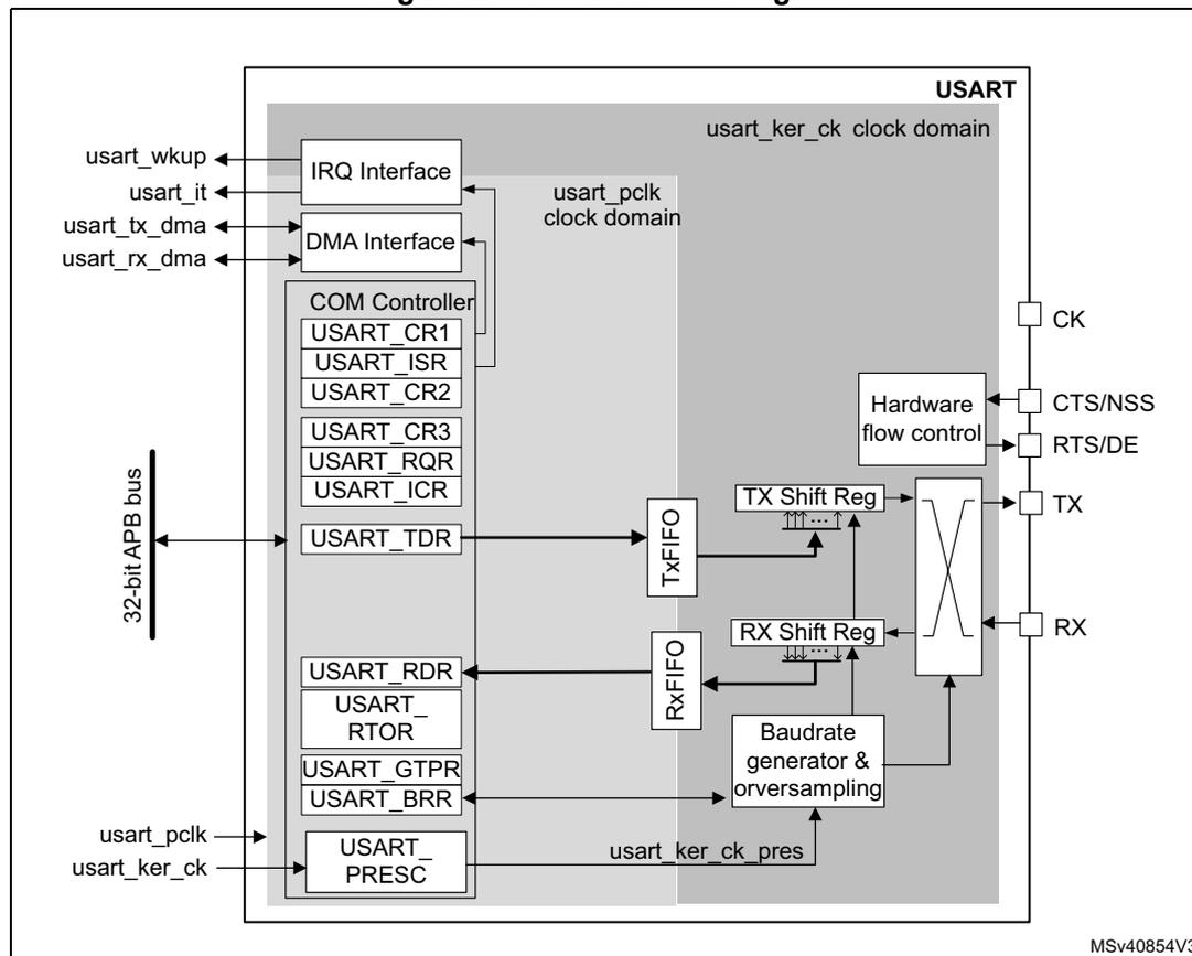
The simplified block diagram given in [Figure 241](#) shows two fully-independent clock domains:
