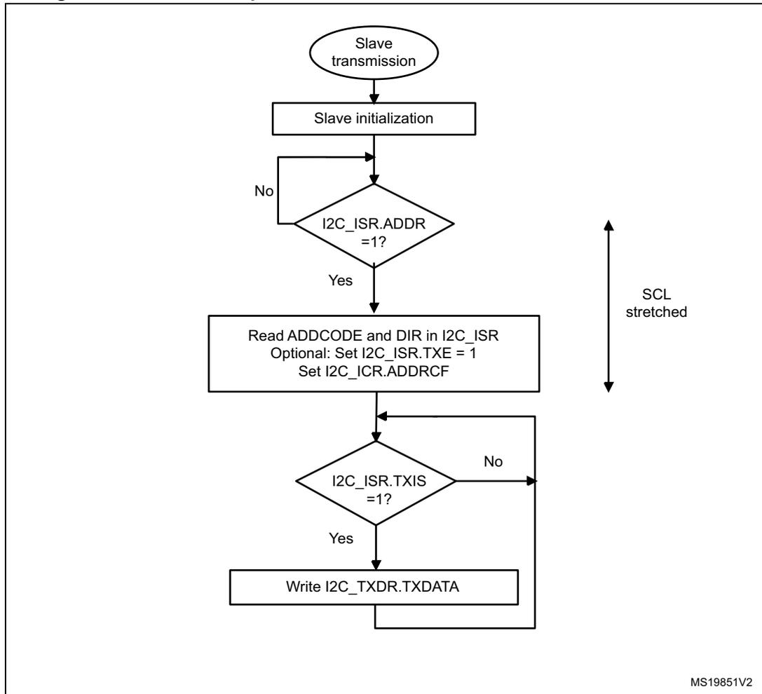
Figure 219. Transfer sequence flow for I2C slave transmitter, NOSTRETCH = 1
