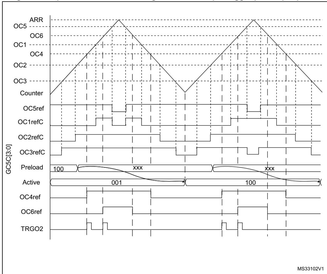
The TRGO2 waveform shows how the ADC can be synchronized on given 3-phase PWM signals. Refer to [Section 15.3.27: ADC synchronization](#) for more details.
