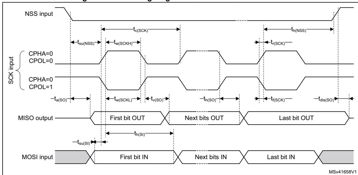
Figure 23. SPI timing diagram - slave mode and CPHA = 1
