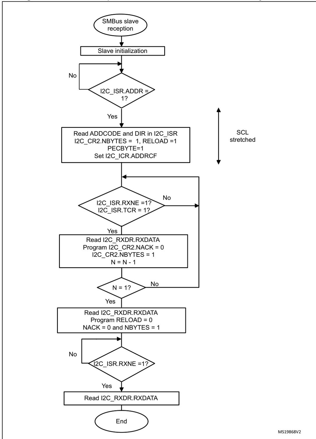
**Figure 238. Bus transfer diagrams for SMBus slave receiver (SBC = 1)**
