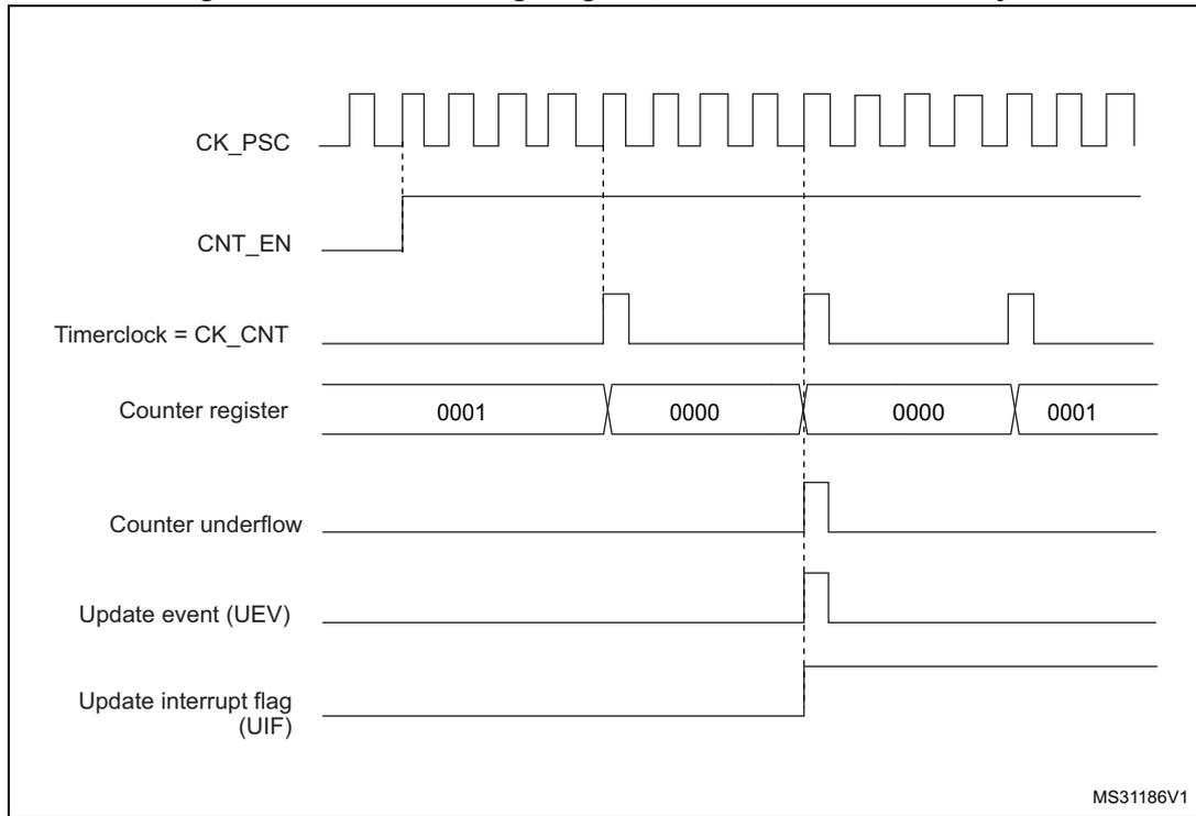
Figure 67. Counter timing diagram, internal clock divided by N
