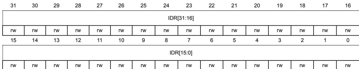
Bits 31:0 **IDR[31:0]**: General-purpose 32-bit data register bits
