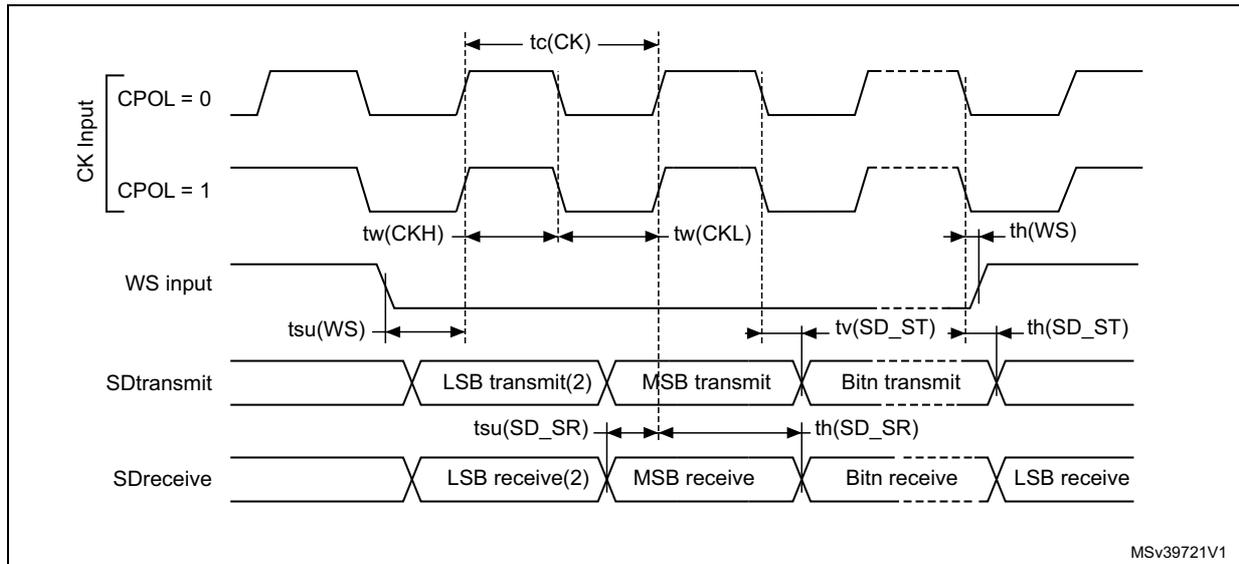
1. Measurement points are done at CMOS levels: 0.3  $V_{DDIO1}$  and 0.7  $V_{DDIO1}$ .
