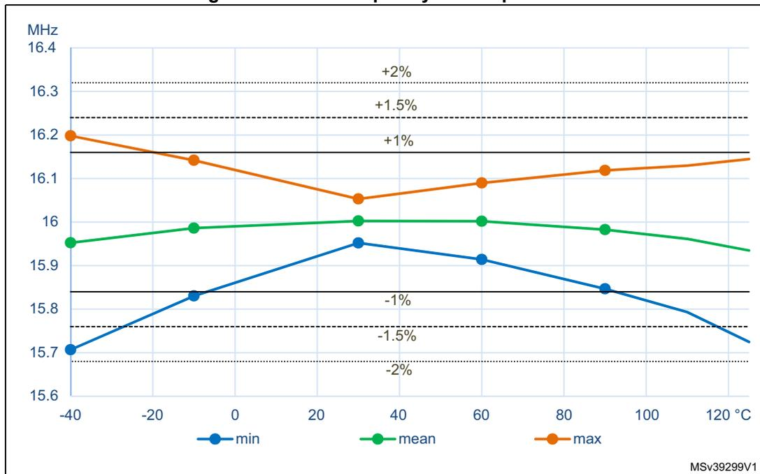
Low-speed internal (LSI) RC oscillator
