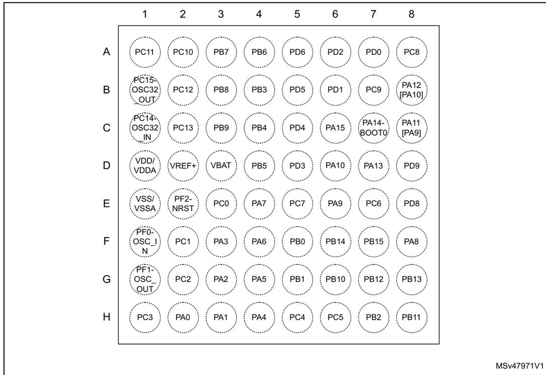
Figure 5. STM32G081CxT LQFP48 pinout
