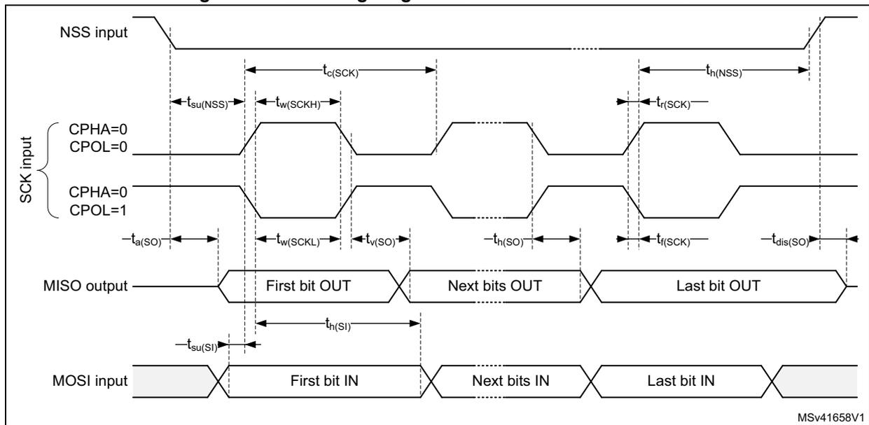
Figure 28. SPI timing diagram - slave mode and CPHA = 1
