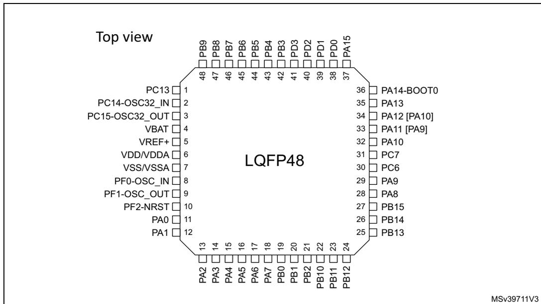
Figure 6. STM32G081CxU UFQFPN48 pinout
