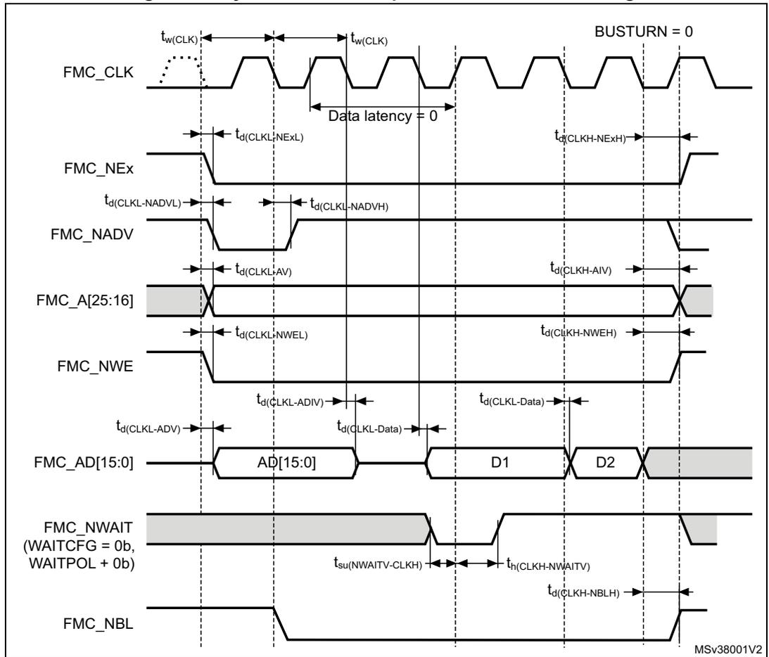
**Table 98. Synchronous multiplexed PSRAM write timings<sup>(1)(2)(3)</sup>**
