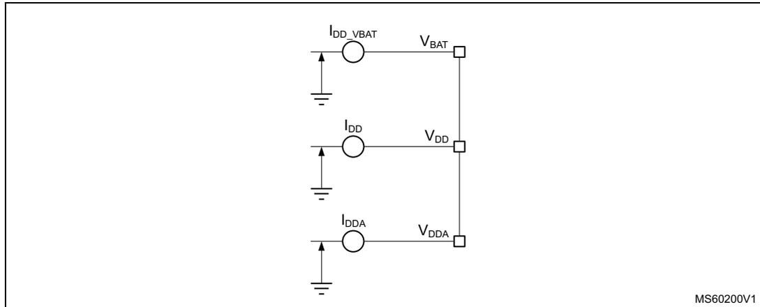
The  $I_{DD\_ALL}$  parameters given in [Table 21](#) to [Table 33](#) represent the total MCU consumption including the current supplying  $V_{DD}$ ,  $V_{DDA}$  and  $V_{BAT}$ .
