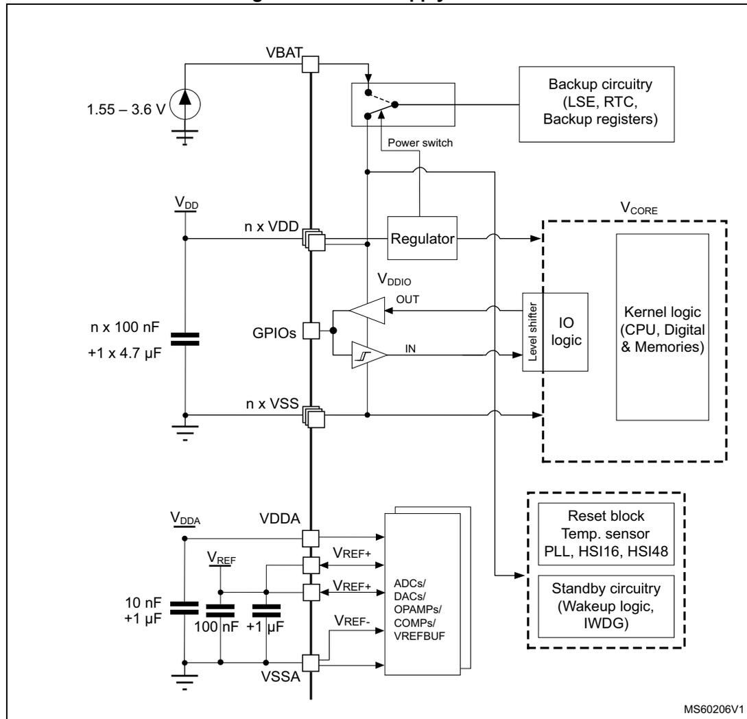
**Caution:** Each power supply pair ( $V_{DD}/V_{SS}$ ,  $V_{DDA}/V_{SSA}$  etc.) must be decoupled with filtering ceramic capacitors as shown above. These capacitors must be placed as close as possible to, or below, the appropriate pins on the underside of the PCB to ensure the good functionality of the device.
