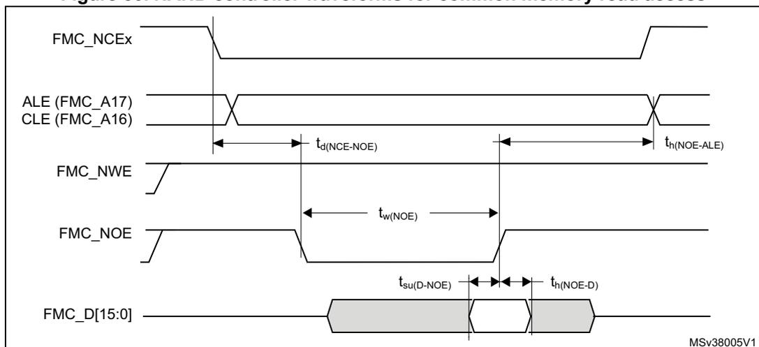
Figure 51. NAND controller waveforms for common memory write access
