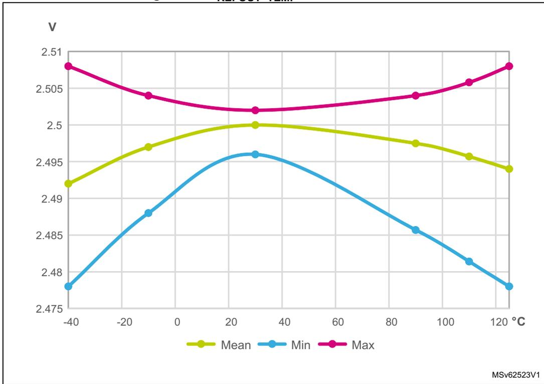
Figure 32.  $V_{REFOUT}$  TEMP in case VRS = 10
