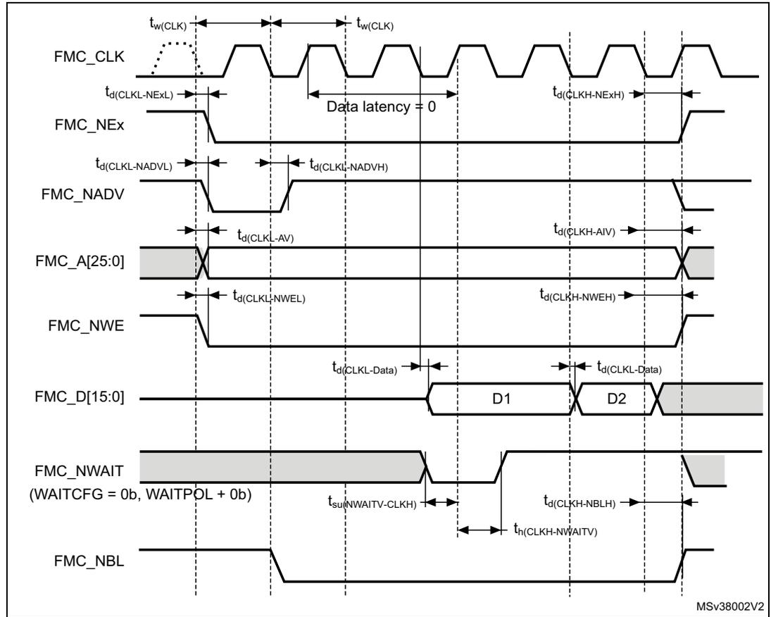
**Table 105. Synchronous non-multiplexed PSRAM write timings<sup>(1)(2)(3)</sup>**
