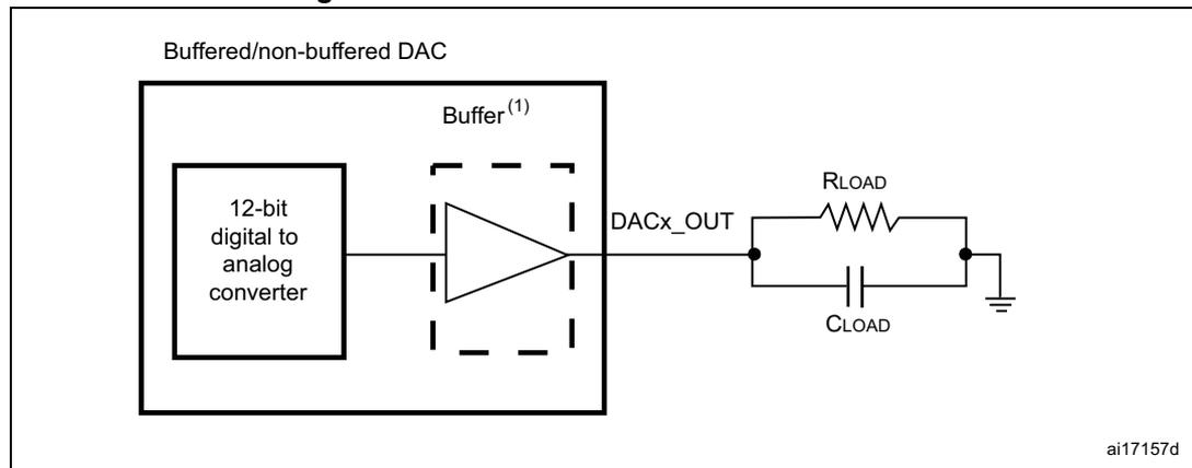
1. The DAC integrates an output buffer to reduce the output impedance and to drive external loads directly without the use of an external operational amplifier. The buffer can be bypassed by configuring the BOFFx bit in the DAC\_CR register.
