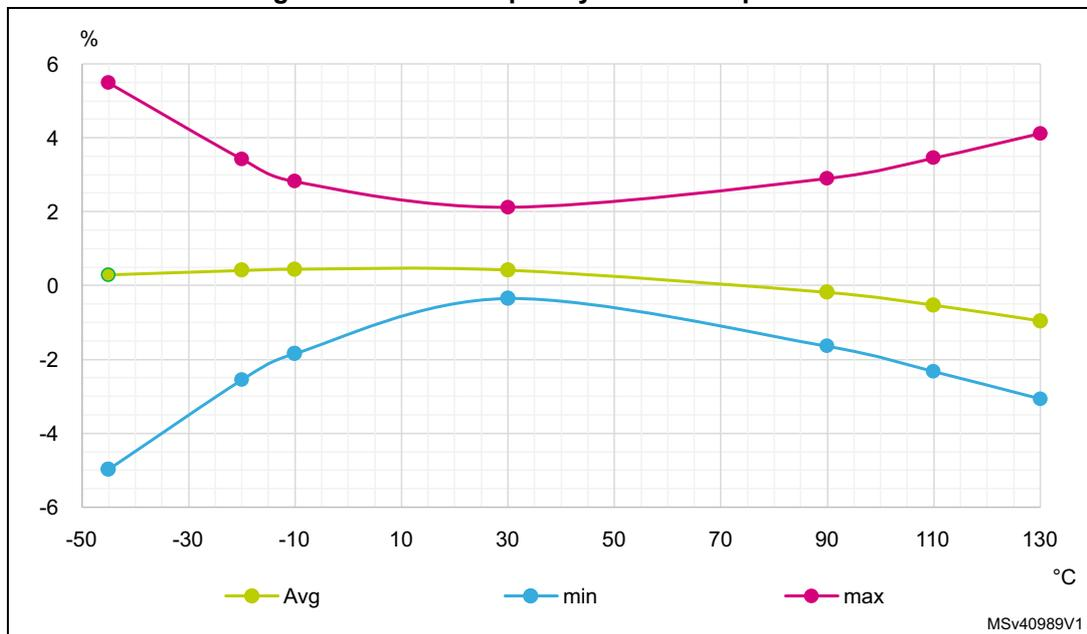
**Low-speed internal (LSI) RC oscillator**
