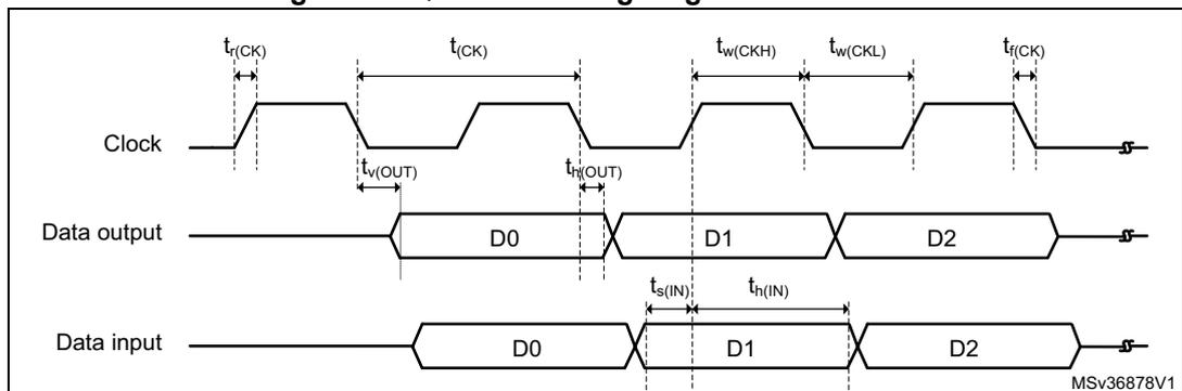
Figure 53. Quad SPI timing diagram - DDR mode
