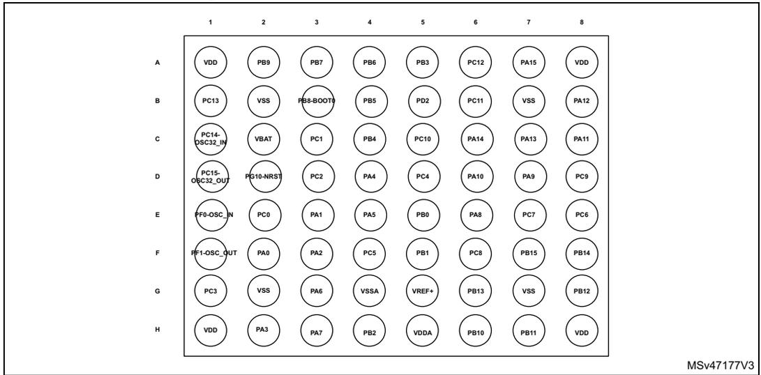
1. The above figure shows the package top view.
