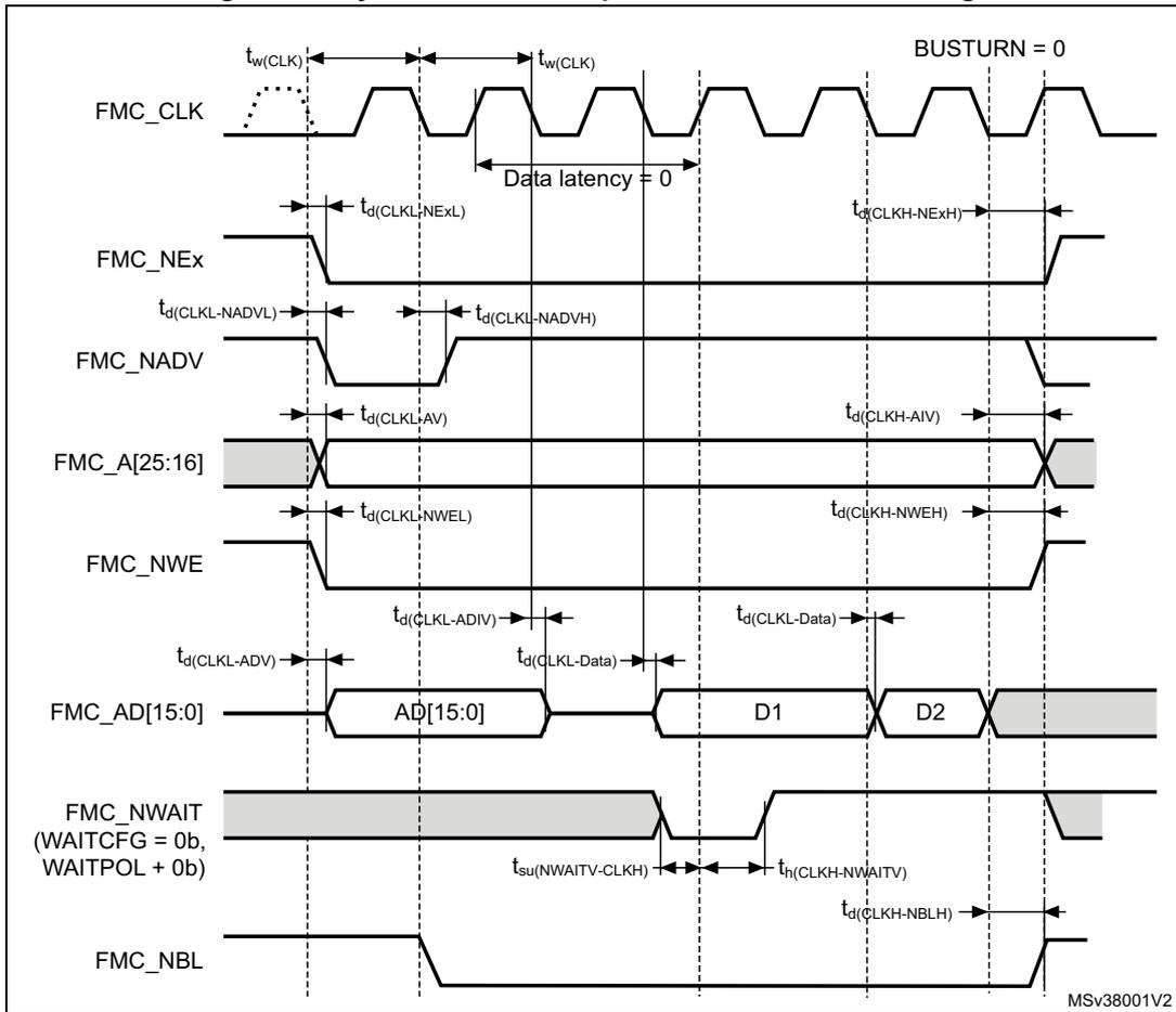
Table 103. Synchronous multiplexed PSRAM write timings<sup>(1)(2)(3)</sup>
