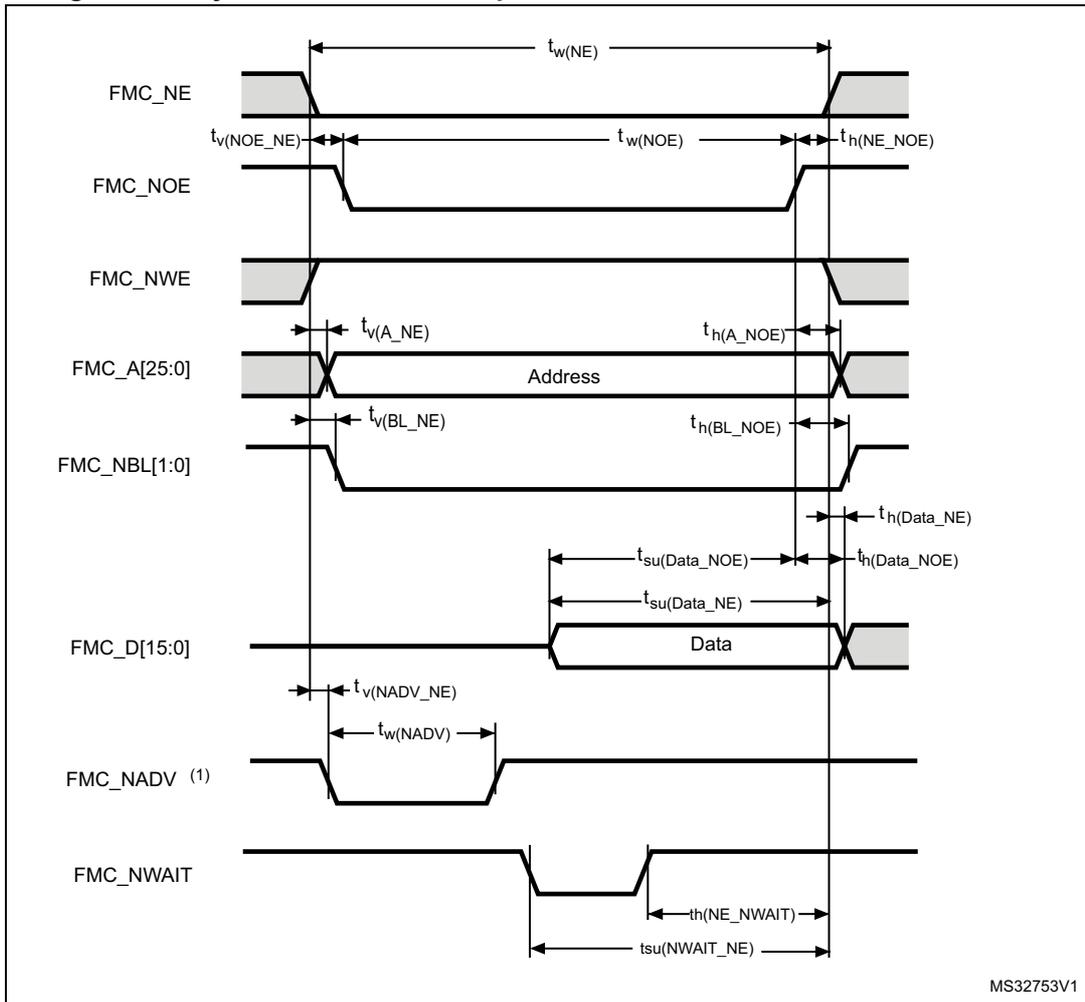
**Table 94. Asynchronous non-multiplexed SRAM/PSRAM/NOR read timings<sup>(1)(2)</sup>**
