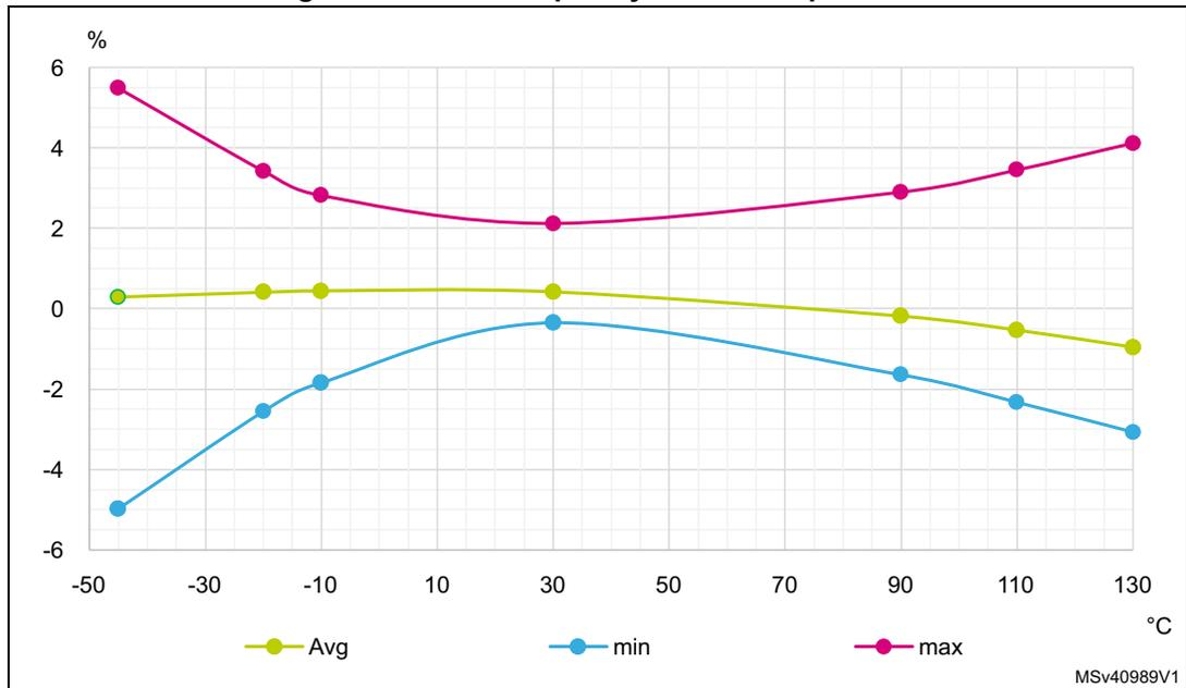
Low-speed internal (LSI) RC oscillator
