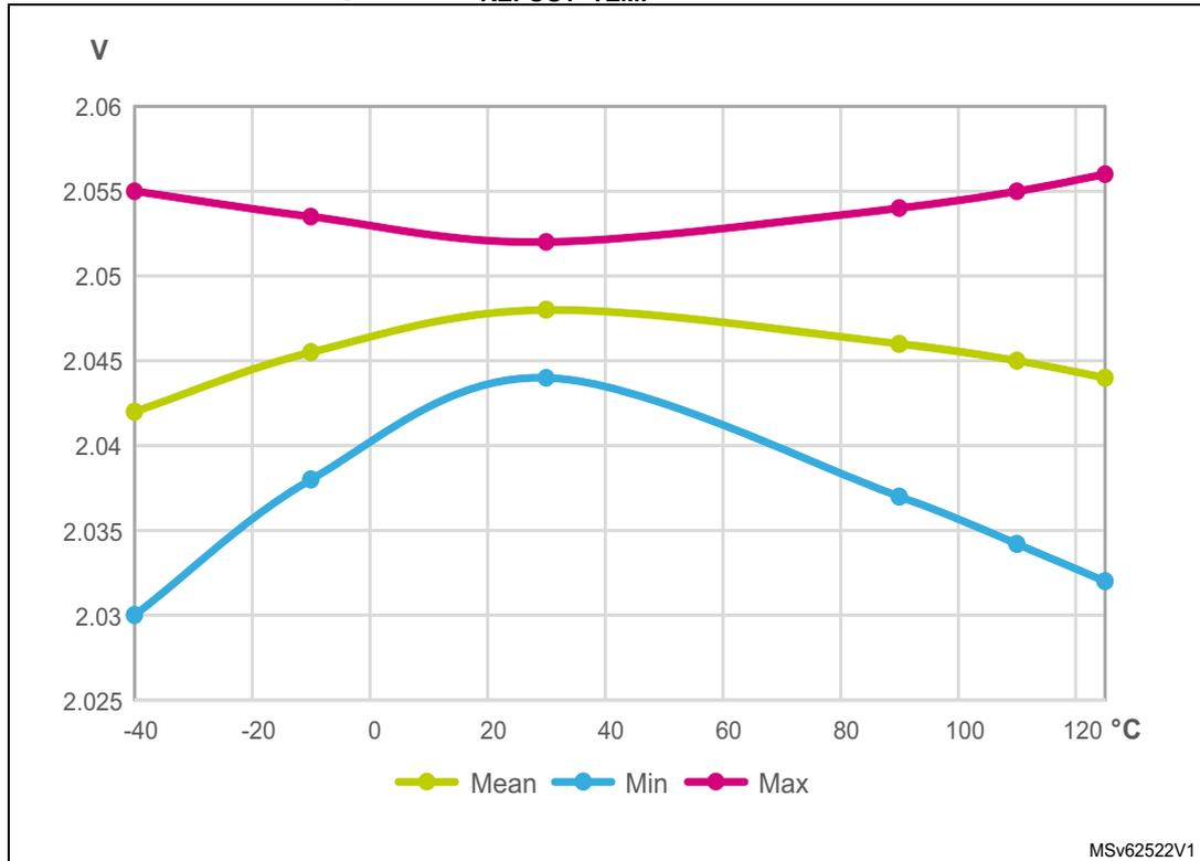
Figure 31.  $V_{REFOUT}$  TEMP in case VRS = 01
