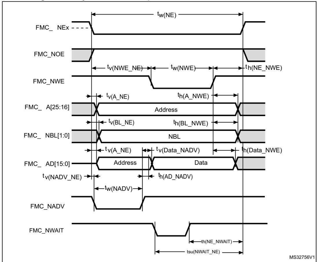
**Table 100. Asynchronous multiplexed PSRAM/NOR write timings<sup>(1)(2)</sup>**
