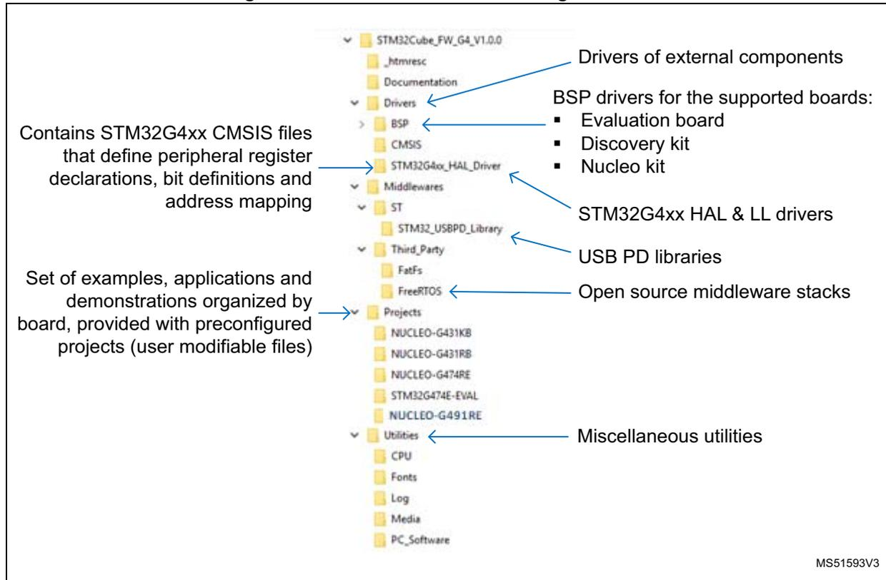
For each board, a set of examples is provided with pre-configured projects for EWARM, MDK-ARM and STM32CubeIDE toolchains.
