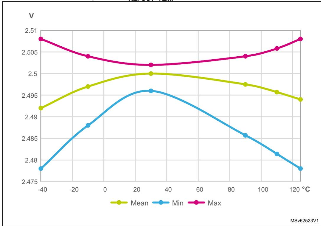
Figure 33.  $V_{REFOUT}$  TEMP in case VRS = 10
