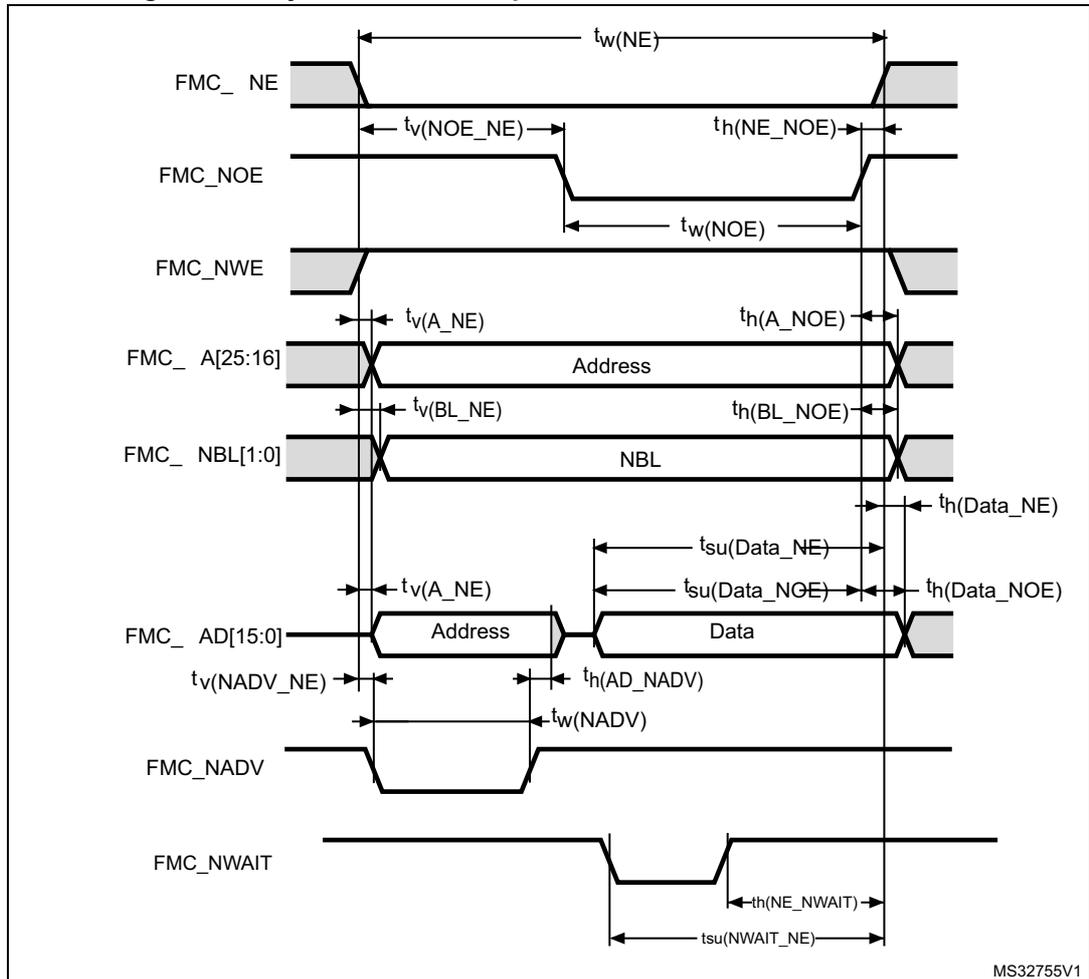
**Table 93. Asynchronous multiplexed PSRAM/NOR read timings<sup>(1)(2)</sup>**
