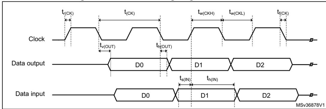
Figure 40. Quad SPI timing diagram - DDR mode
