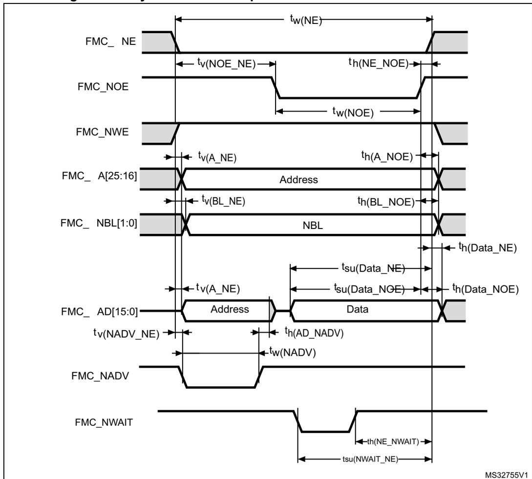
Table 98. Asynchronous multiplexed PSRAM/NOR read timings<sup>(1)(2)</sup>
