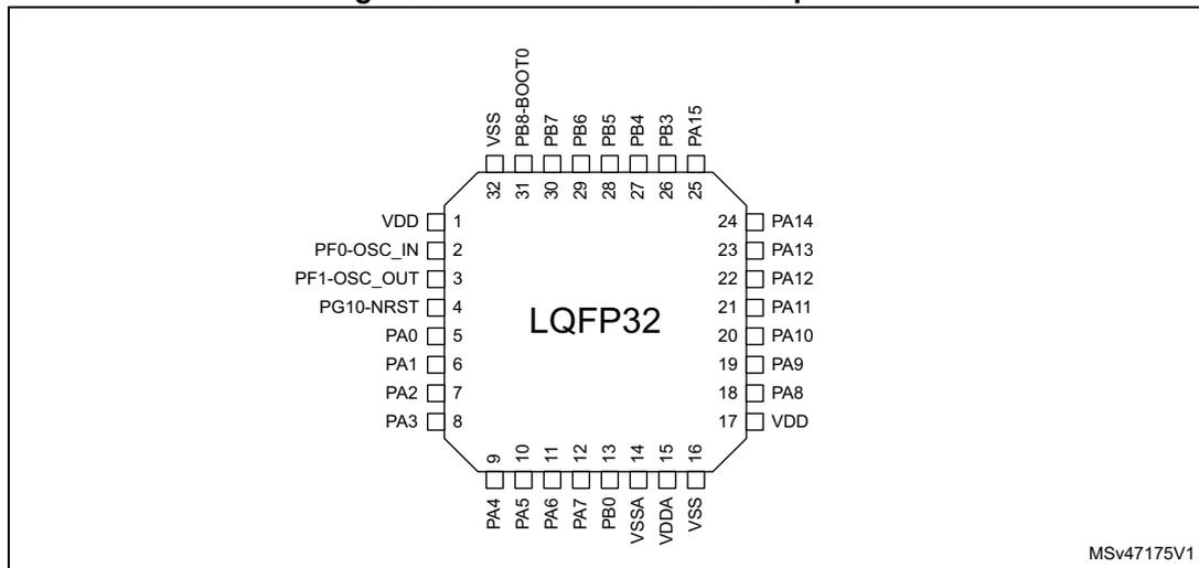
1. The above figure shows the package top view
