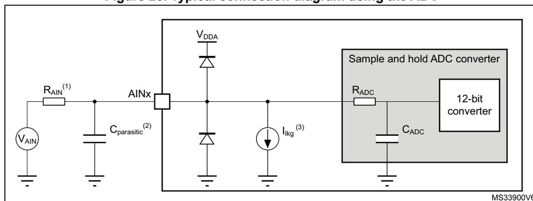
1. Refer to [Table 60: ADC characteristics](#) for the values of  $R_{AIN}$  and  $C_{ADC}$ .
