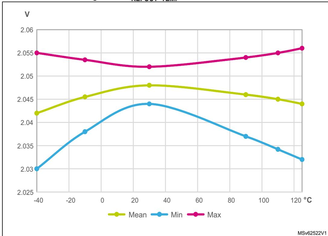
Figure 32.  $V_{REFOUT}$  TEMP in case VRS = 01
