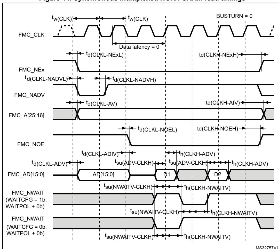
Table 102. Synchronous multiplexed NOR/PSRAM read timings<sup>(1)(2)(3)</sup>
