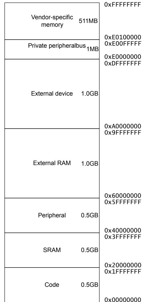
**Figure 2-3 Cortex-M33 processor memory map**
