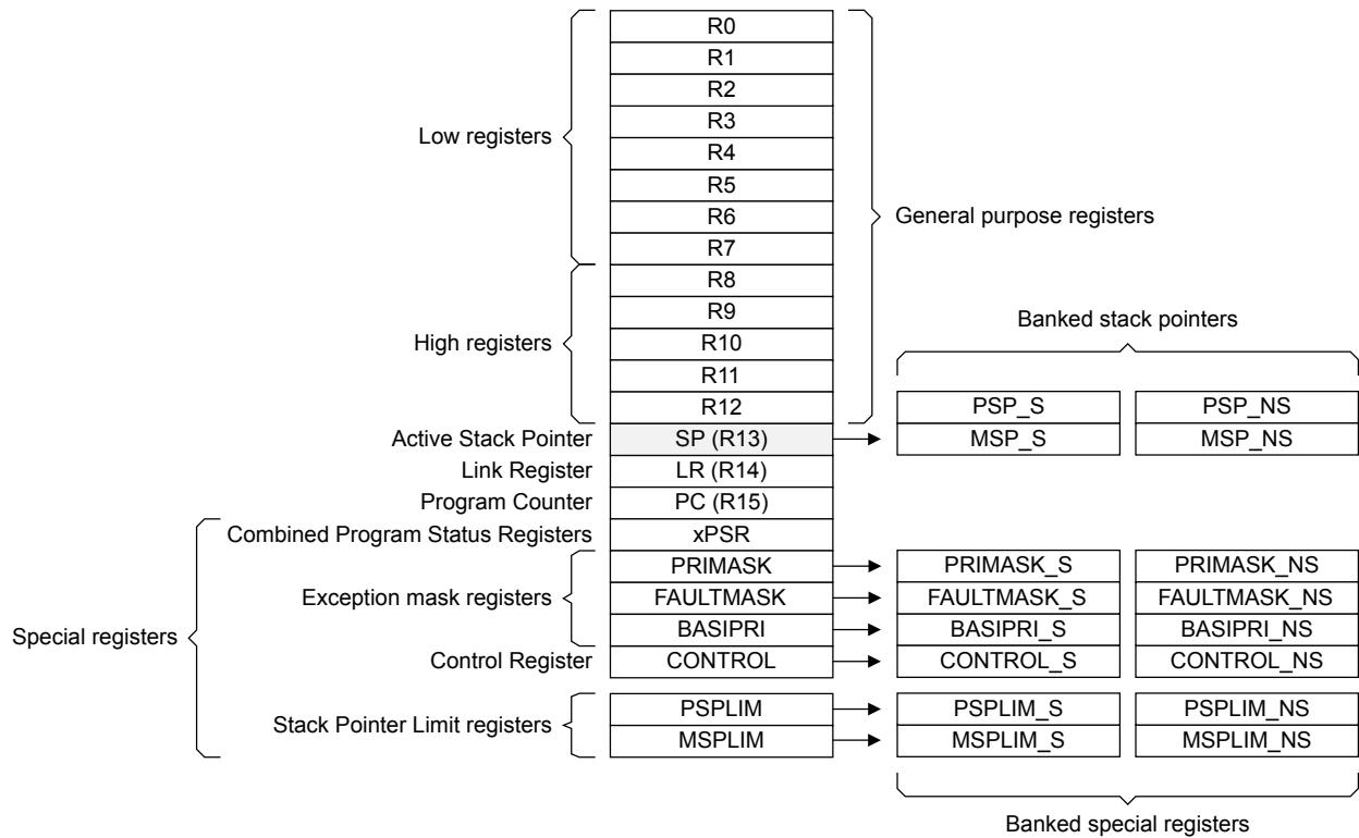
**Figure 2-2 Core registers with the Security Extension**
