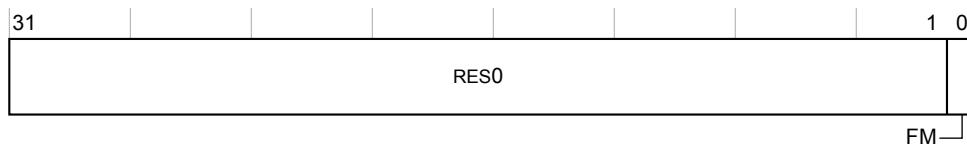
**Table 2-13 FAULTMASK register bit assignments**
