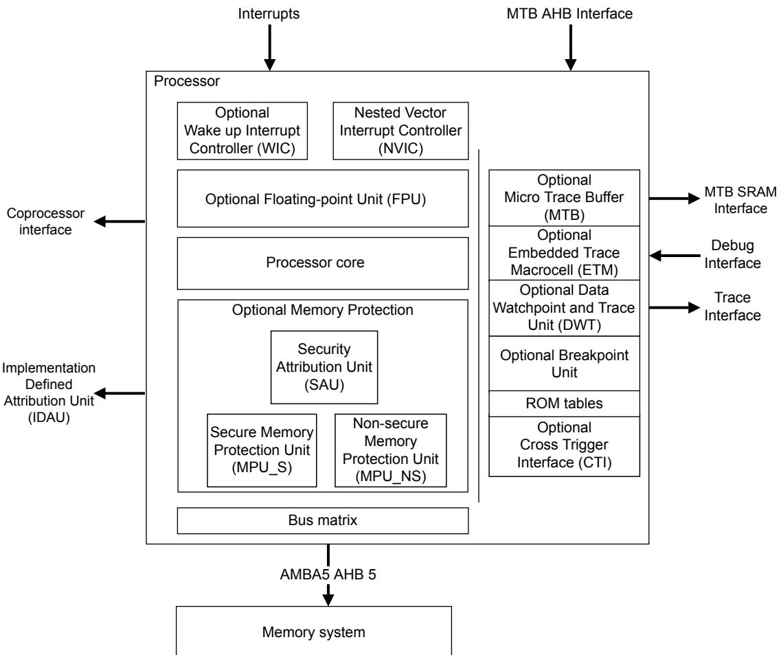
**Figure 1-2 Cortex-M33 processor implementation with the Security Extension**
