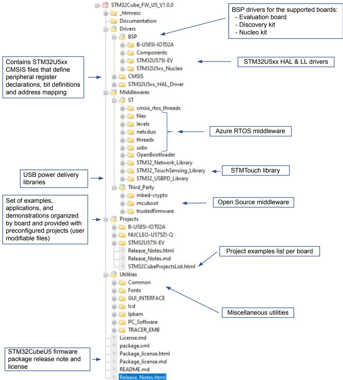
1. The component files must not be modified by the user. Only the \Projects sources are editable by the user.
