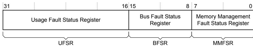
The CFSR is byte accessible. You can access the CFSR or its subregisters as follows:
